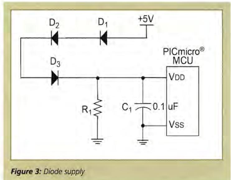
**Figure 3:** Diode supply
