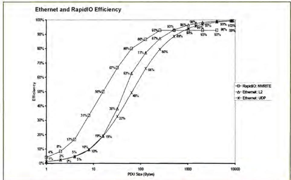
**Figure 1:** Ethernet achieves its best efficiency with a maximum payload, although this comes at the cost of increased latency jitter. By balancing large payload jitter against small payload inefficiency, an alternative interconnect standard like RapidIO technology achieves better overall efficiency across the payload sizes most common to embedded backplane applications
