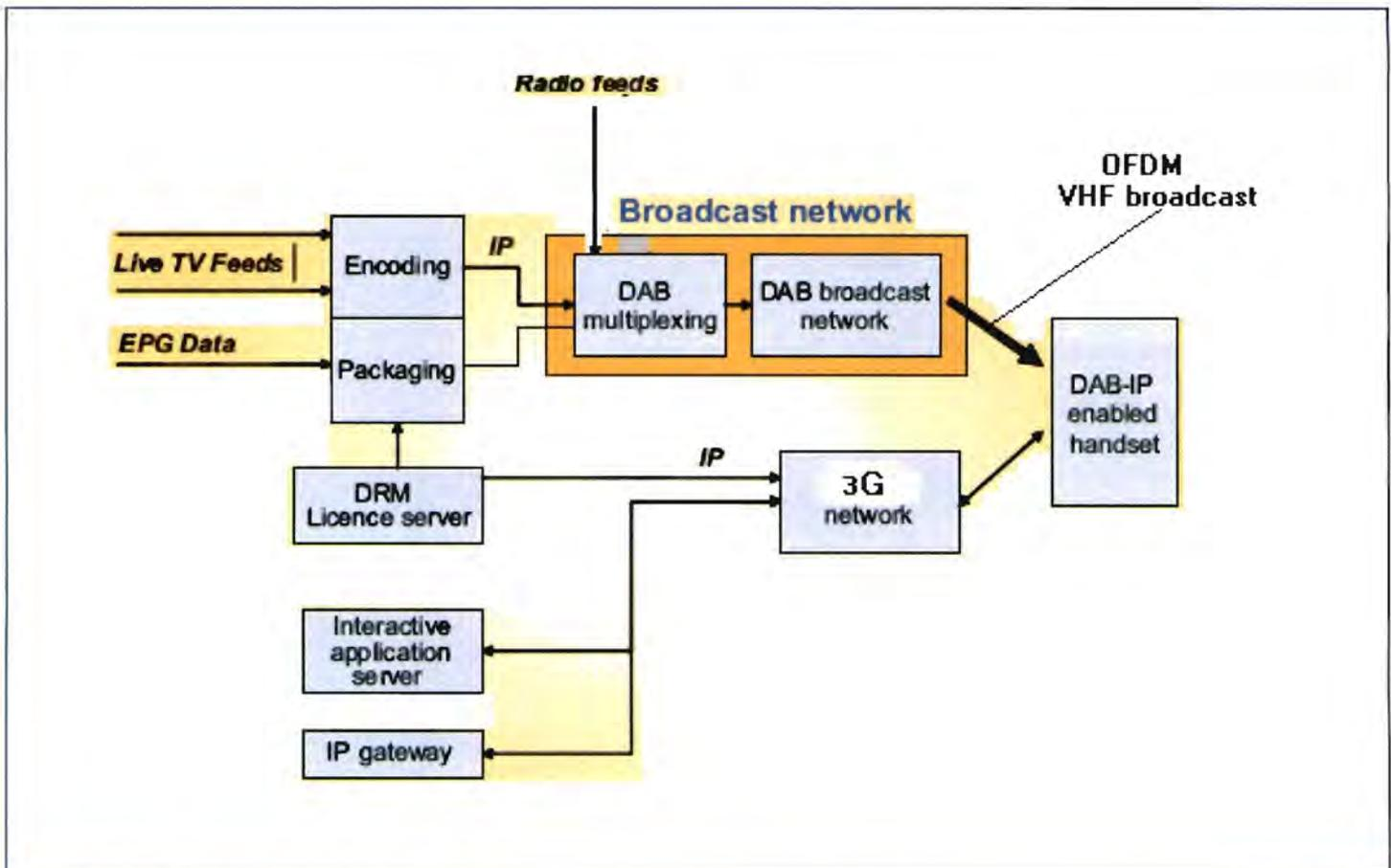
Figure 1: DAB TV system architecture
