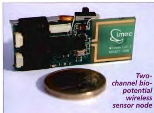
Two-channel bio-potential wireless sensor node
