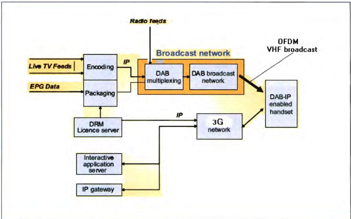
Figure 1: DAB TV system architecture
