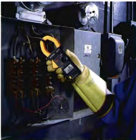
*An electrician using a True RMS 3-Phase Clamp-on Power Analyser to measure, compute and display 3-phase power on balance or unbalanced loads*
