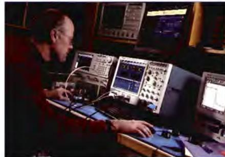
DPO/DSA72004 oscilloscope provides support on all channels for ultra-high bandwidth, deep memory, fast sample rate and fast waveform capture rate. This is
