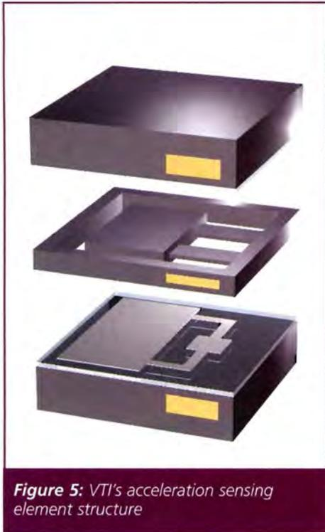
**Figure 5:** VTI's acceleration sensing element structure
