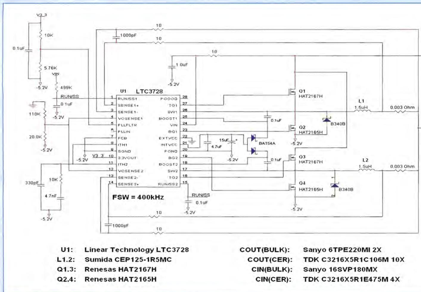
**Figure 5:** An LTC3728 +12V to -5.2V/15A dual phase inverting buck/boost supply
