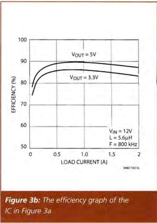
**Figure 3b:** The efficiency graph of the IC in Figure 3a
