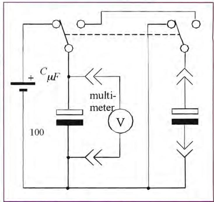
Figure 1: Capacitance meter
