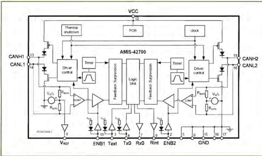
**Figure 4:** Block diagram of a CAN repeater
