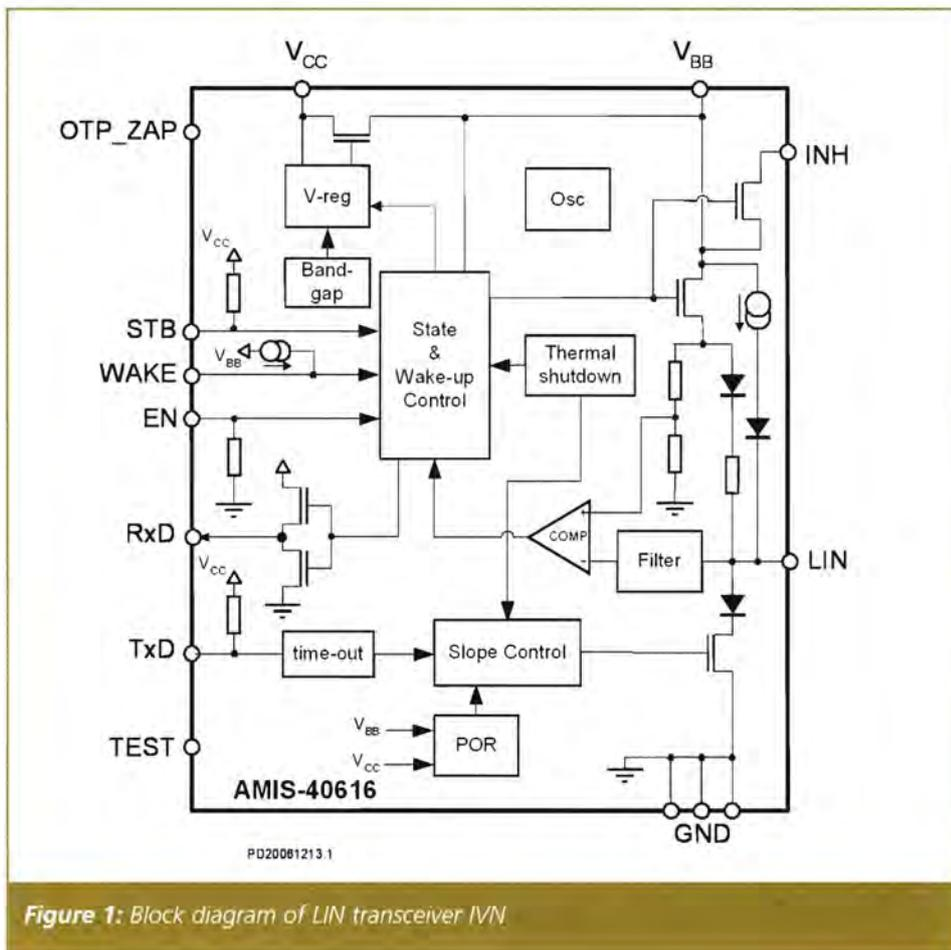
Figure 1: Block diagram of LIN transceiver IVN
