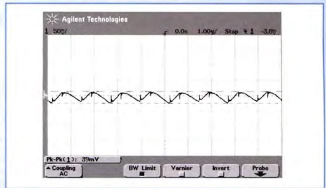
**Figure 6:** Output voltage ripple of the LTC3728 inverting buck/boost supply.  $V_{IN} = +12V$ ,  $I_{OUT} = 15A$
