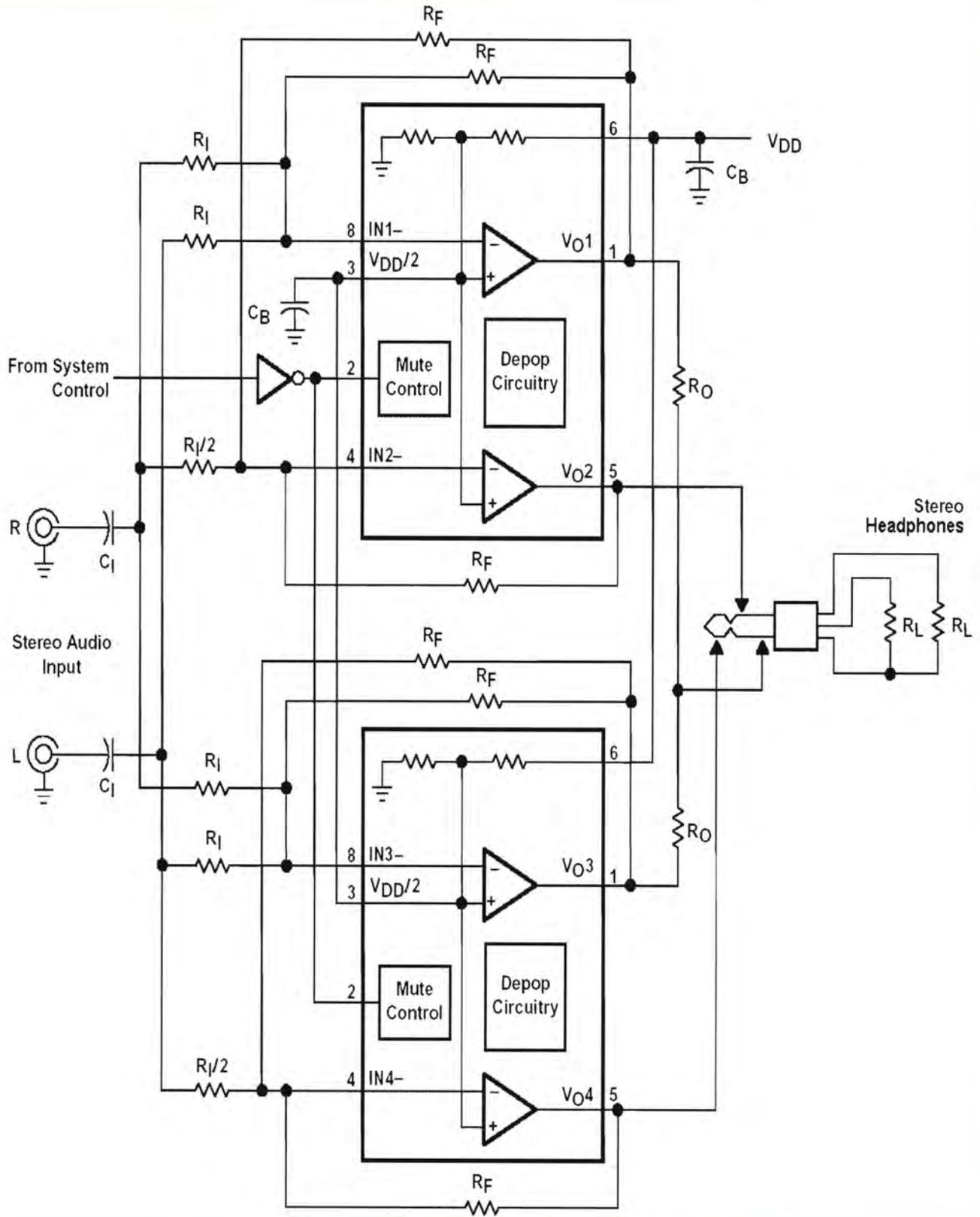
**Figure 1:** Two headphones chips and a handful of passive parts drive DC-coupled stereo headphones with common wire from the bridge circuit
