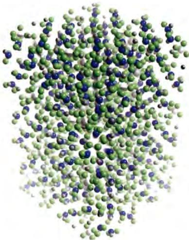
*The future in store: hydrogen atoms can be absorbed effectively into the new storage material. Hydrogen (H) atoms are shown in green, lithium (Li) atoms in dark grey, nitrogen (N) atoms in blue and boron (B) atoms in grey and inside the pyramids*
