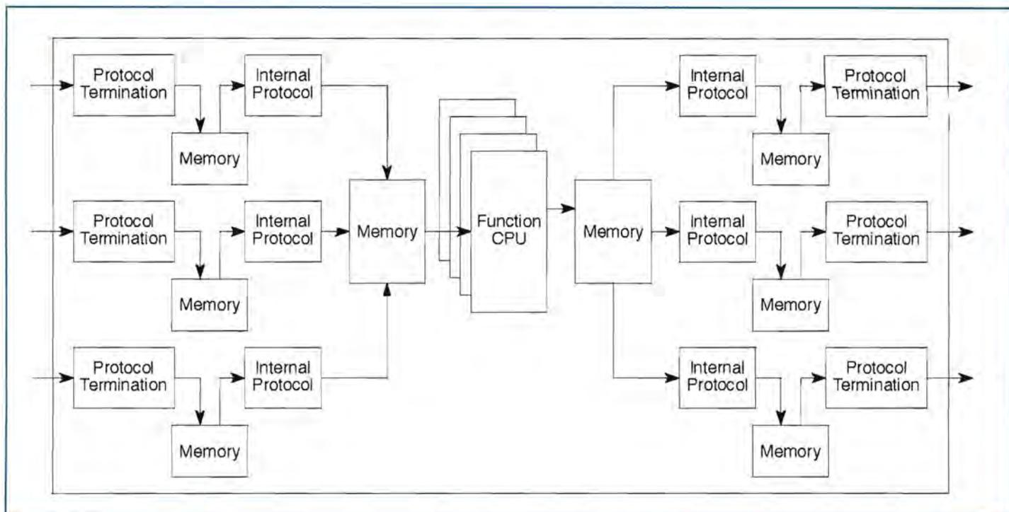
**Figure 1:** Consolidating protocols yields significant system-wide savings by eliminating processing and increasing efficiency, leading to improved system performance, throughput, reliability and cost-effectiveness
