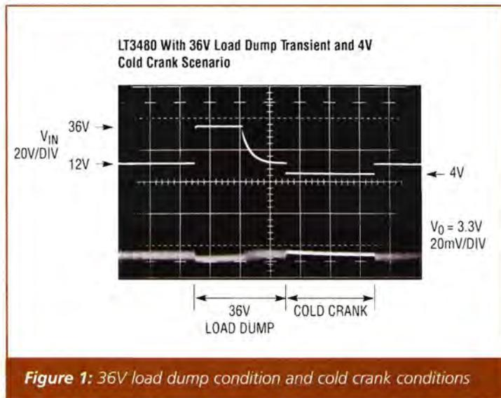
**Figure 1:** 36V load dump condition and cold crank conditions
