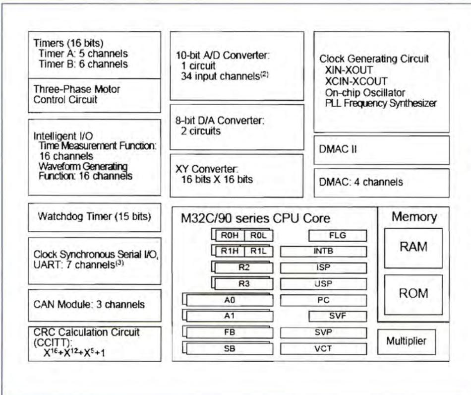
Block diagram of M32C microcontroller
