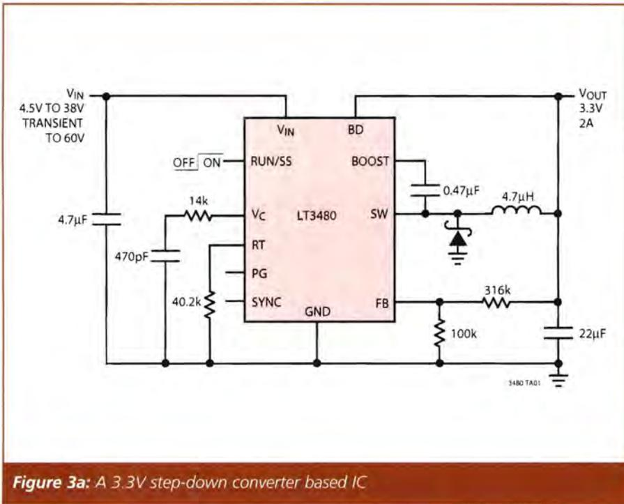
**Figure 3a:** A 3.3V step-down converter based IC
