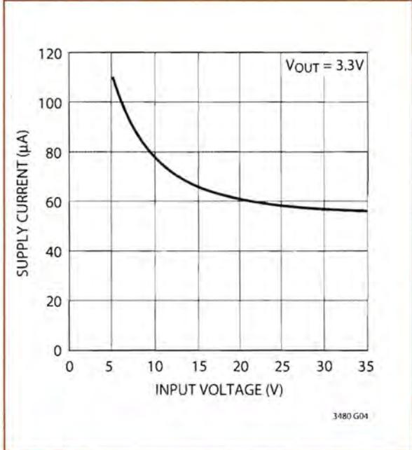
**Figure 4:** LT3480 no-load quiescent current vs input voltage
