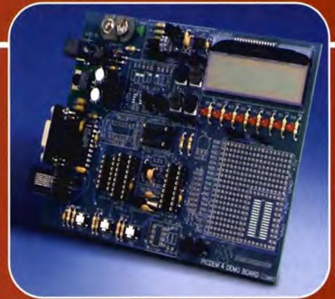
The PICDEM 4 Demonstration Board includes two PICmicro Flash microcontrollers and a CD-ROM containing sample programs, application notes and user guide. The MPLAB ICD 2 is available as a stand-alone unit and Microchip's MPLAB IDE (interactive development environment) software can be downloaded for free from Microchip web site.
