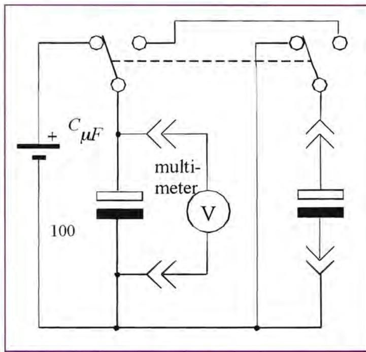
Figure 1: Capacitance meter
