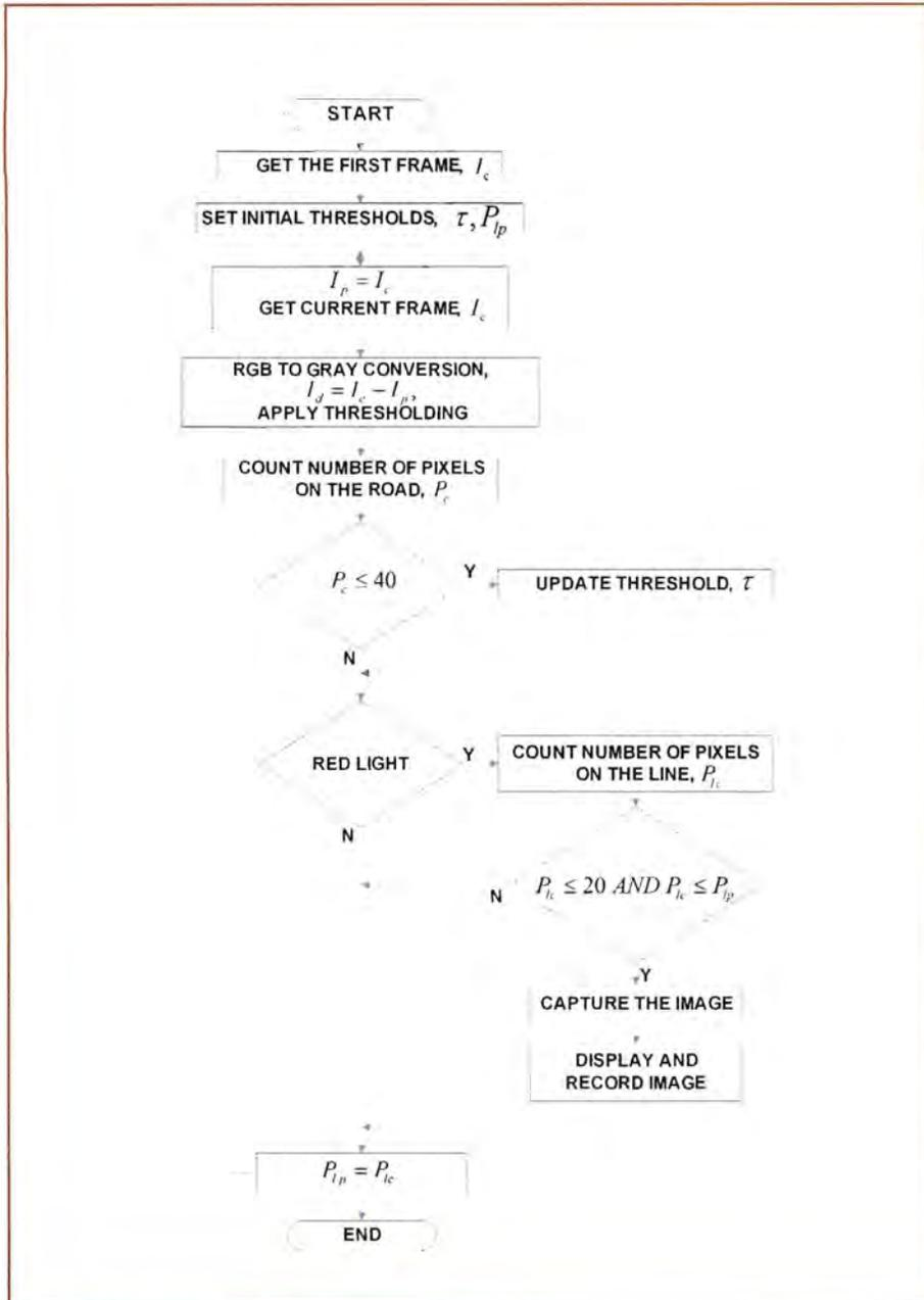
Figure 3: Flowchart of the detection software
