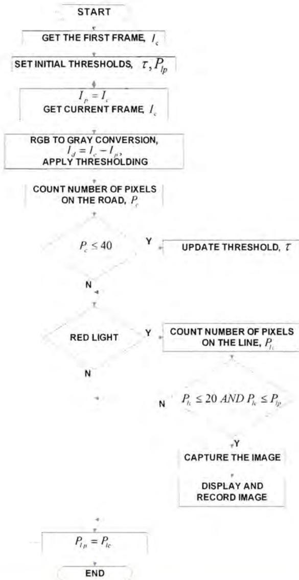
Figure 3: Flowchart of the detection software
