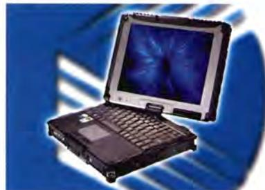
With the 1.2GHz Intel Core Duo U2500 processor, Intel 945 GMS chipset and up to 2GB DDR-RAM, the dual-core and dual-use convertible rugged PC, Kontron NotePAC Duo, offers operation time of up to nine hours with only one lightweight battery pack.
