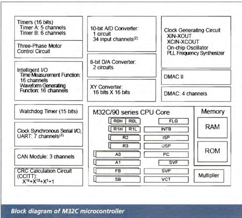
Block diagram of M32C microcontroller
