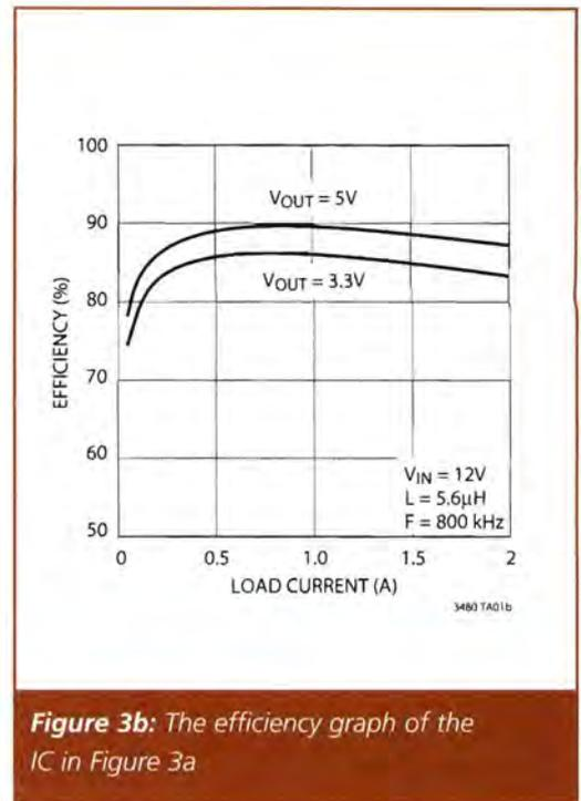
**Figure 3b:** The efficiency graph of the IC in Figure 3a
