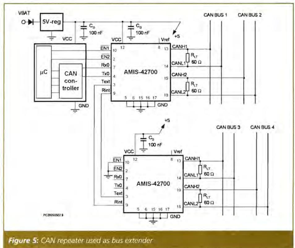
**Figure 5:** CAN repeater used as bus extender
