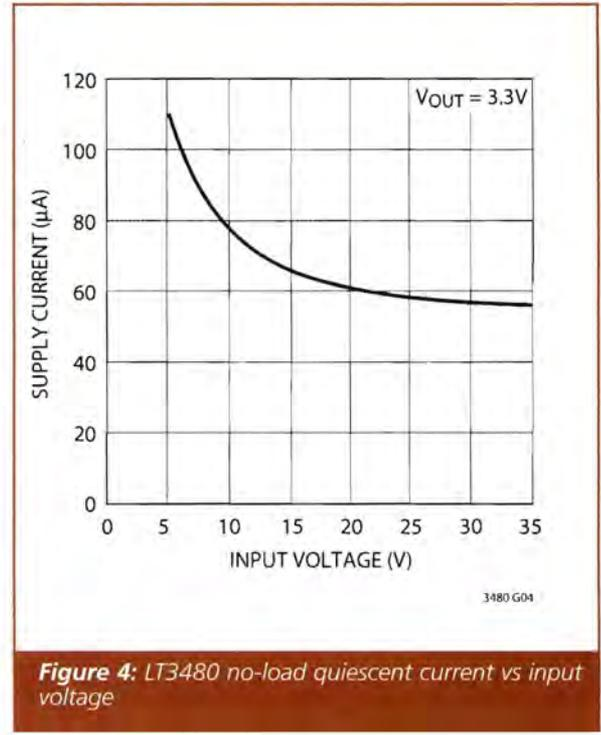
**Figure 4:** LT3480 no-load quiescent current vs input voltage
