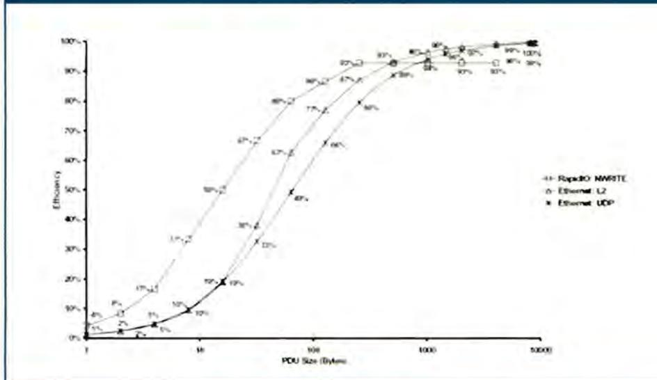
**Figure 4:** Ethernet achieves its best efficiency with a maximum payload, although increases latency jitter significantly. By balancing small payload inefficiency against large payload jitter, the RapidIO specification achieves better overall efficiency at the payload sizes most commonly used in high-speed, embedded applications
