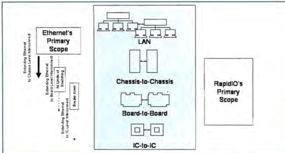
**Figure 2:** a) Ethernet was originally designed to serve in large networks with a great many endpoints, each of which was expected to have a processor available for protocol stack processing. b) The RapidIO protocol, in contrast, was designed specifically for embedded in-the-box and chassis control plane applications.
