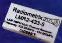
25kHz Narrow Band FM 32-channel transmitter and receiver for industrial remote control, telemetry, security and alarm applications in 433MHz (EU) or 458MHz (UK).
