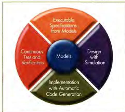
**Figure 2:** Model-Based Design places the system-level model at the centre of the development process for mechatronic systems
