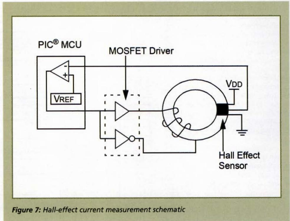
Figure 7: Hall-effect current measurement schematic
