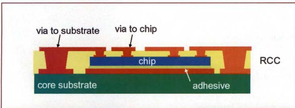
**Figure 1:** The Chip In Polymer method uses thinned chips, a very thin board core, and electrolessly plates the chip bond pads at the wafer level
