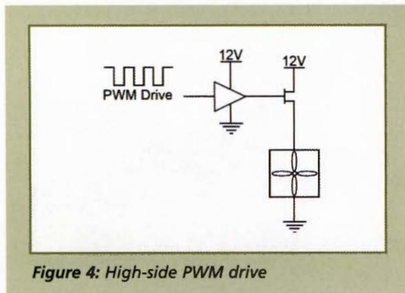
**Figure 4:** High-side PWM drive
