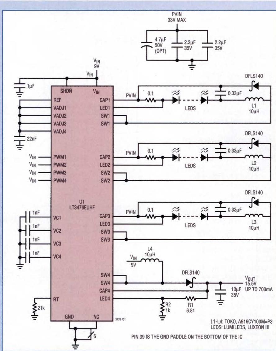
**Figure 9:** Here is a simple way to save BOM cost and reduce solution size in an LCD. A single-quad LED driver IC provides power for the LED backlight and the LCD bias of an LCD projector. Three of the channels drive R, G and B LED strings, while the fourth provides a voltage source in boost mode
