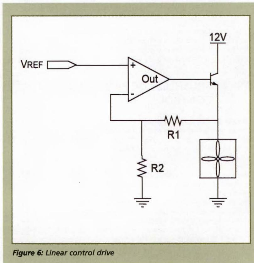
**Figure 6:** Linear control drive
