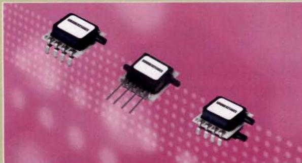
Sensortech's new HCL pressure sensors measure low gage or differential pressures from 5-75mbar. These devices are precision calibrated and temperature compensated and offer ratiometric millivolt output signals.
