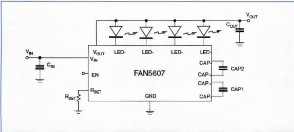
**Figure 5:** The FAN5607 uses two capacitors and has three modes, 1X, 1.5X and 2X
