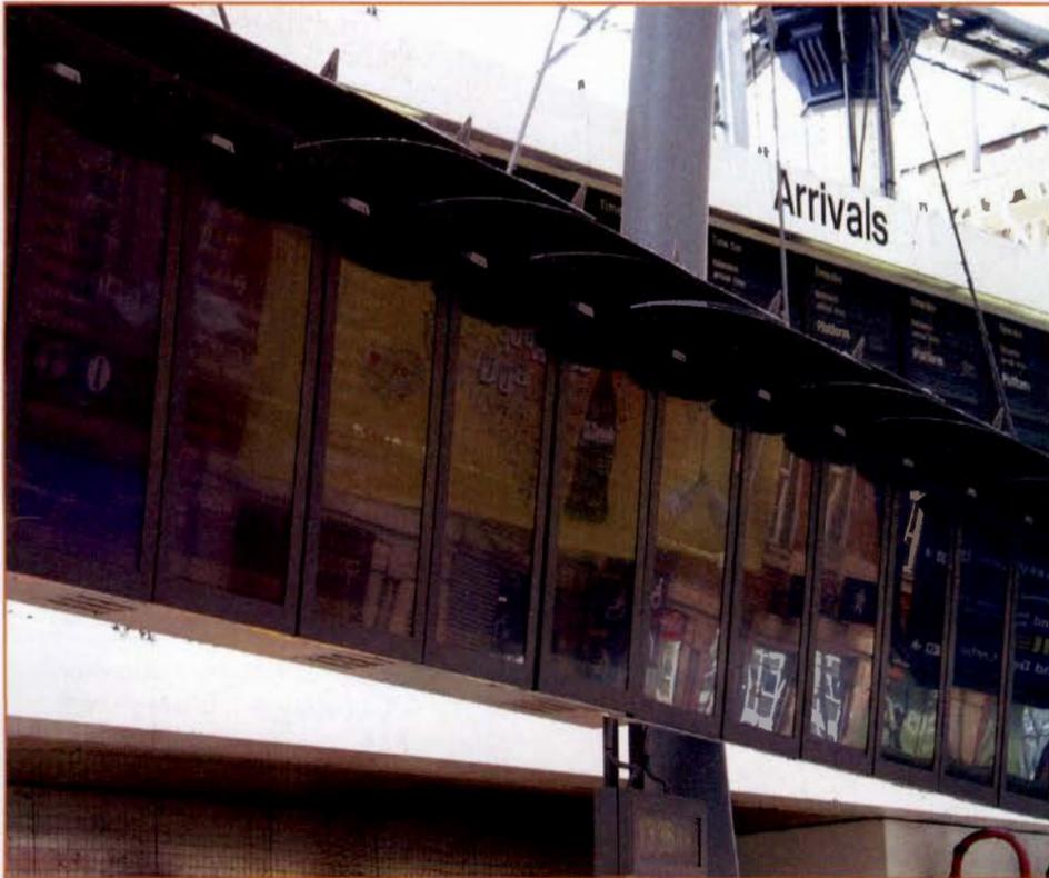
*This picture shows very clearly the reflections off the front face of the box within which the FPD displays are mounted. It wouldn't matter whether the display was plasma or LCD, the reflections off this front surface would be just as bad*
