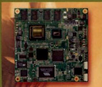
Congatec AG enhances its successful COM Express product family with the introduction of the extremely low power consuming conga-CA. It features the brand new Intel Atom processor Z5xx series and the Intel System Controller Hub US15W.
