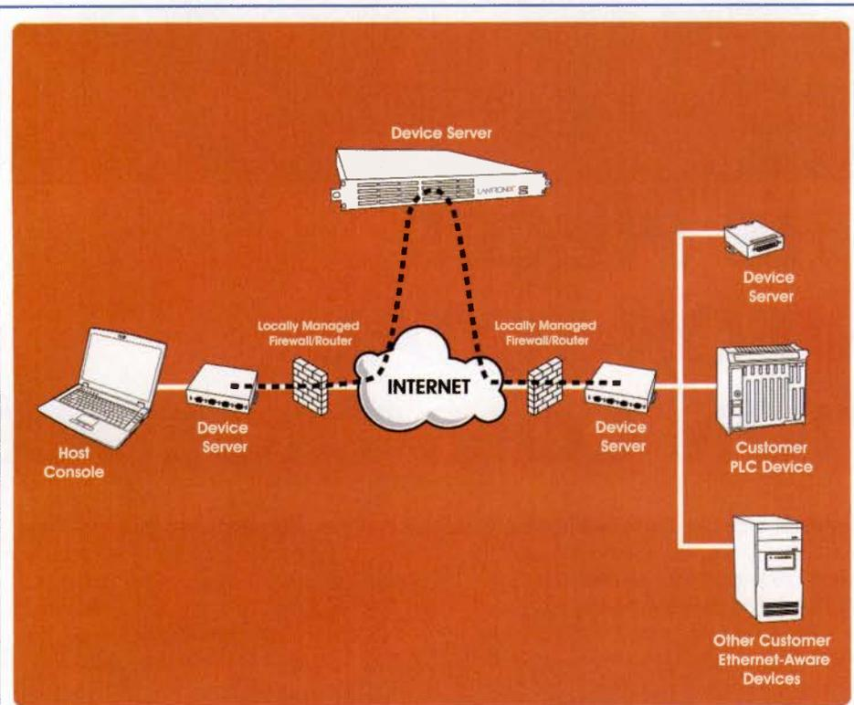
**Figure 2:** Users must be able to easily establish two-way communication that works without weakening the firewalls
