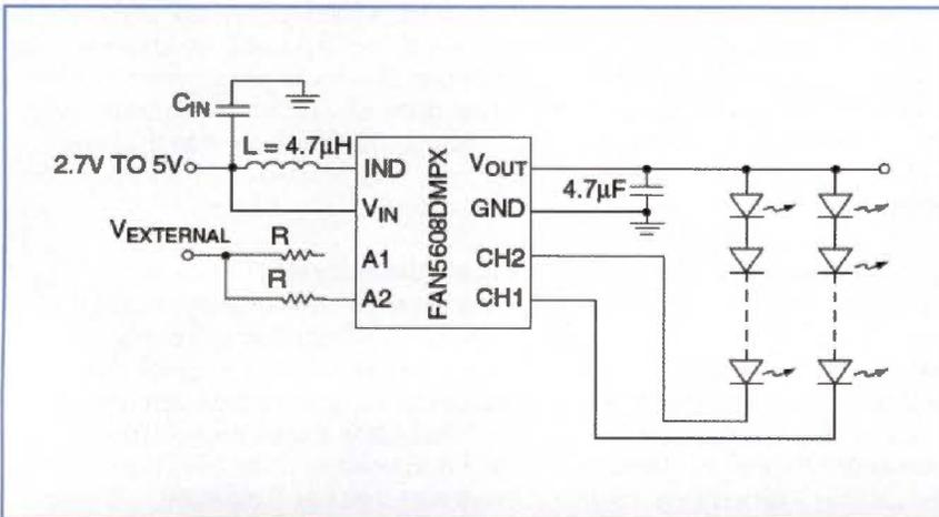
Figure 3: The FAN5608 uses the inductive boost regulator method
