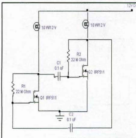
The given circuit (left) is for an 'Incandescent Lamp Flasher' using two IRF511 MOSFETs which are configured as a simple astable multivibrator to alternately switch the two lamps on and off.
