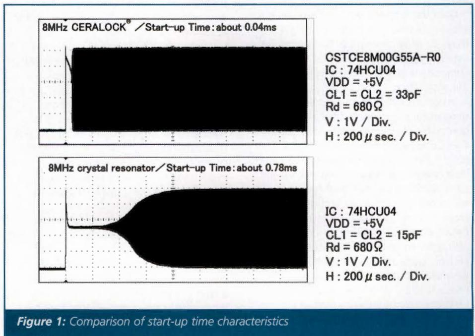
Figure 1: Comparison of start-up time characteristics
