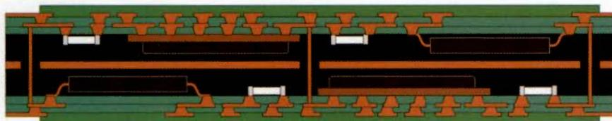
**Figure 2:** The Occam Process uses unthinned, packaged chips, and a variety of core and build-up materials. Both methods can bury active and passive components. Each chip shown here is several times thicker than the chip shown in Figure 1
