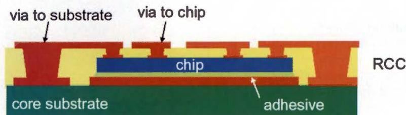
**Figure 1:** The Chip In Polymer method uses thinned chips, a very thin board core, and electrolessly plates the chip bond pads at the wafer level
