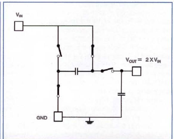
Figure 4: Capacitive charge pump
