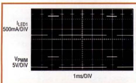
**Figure 1:** LT3476 PWM/LED current waveforms
