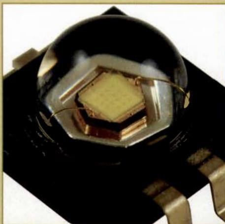
**Figure 2:** Philips Lumileds Luxeon K2 with TFFC
