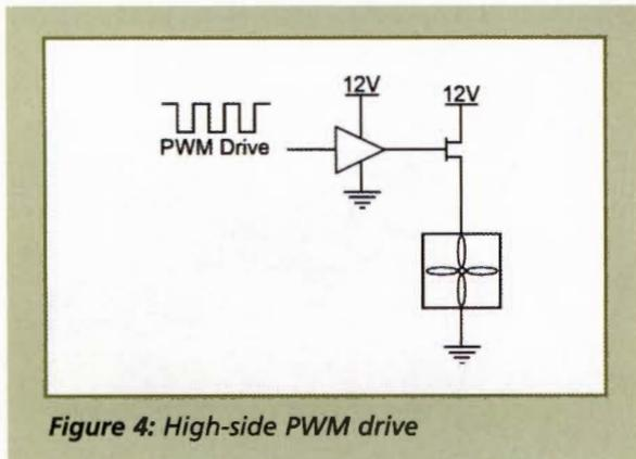
**Figure 4:** High-side PWM drive
