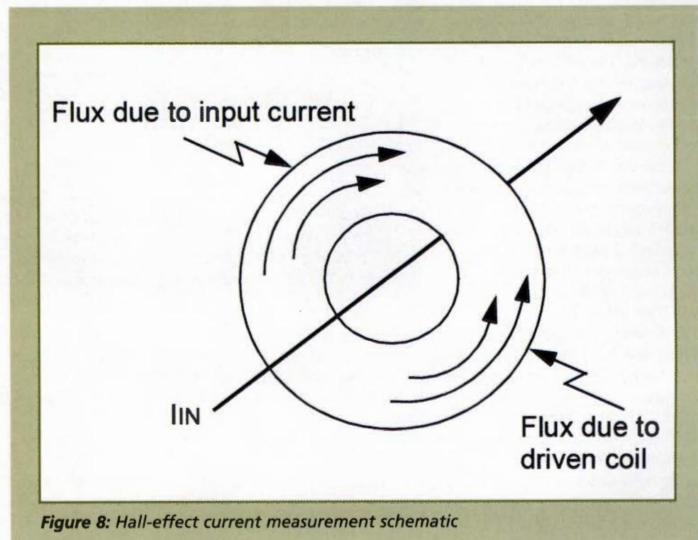
Figure 8: Hall-effect current measurement schematic
