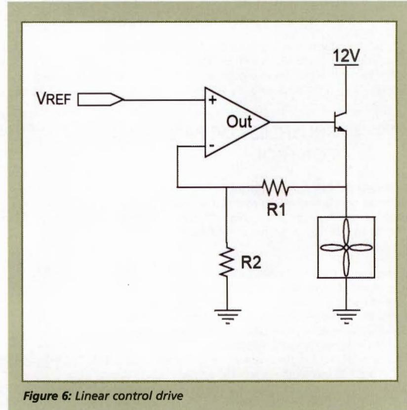
**Figure 6:** Linear control drive
