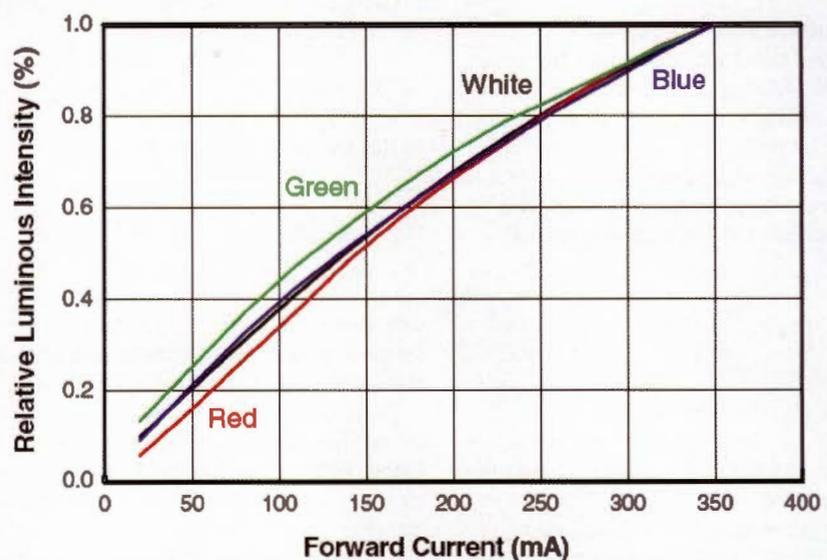
Figure 1: Relative luminous intensity vs forward current
