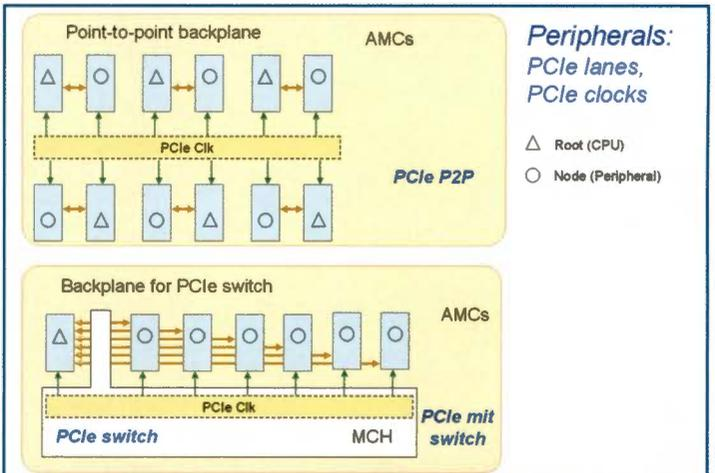
Figure 3: AMC port mapping and backplane
