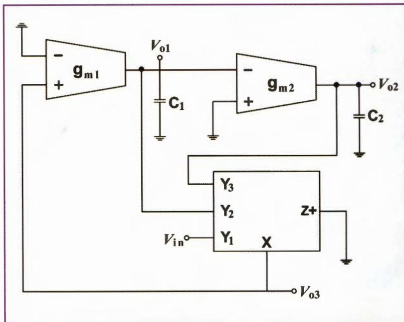
Figure 1: The proposed multifunction voltage-mode universal filter.
