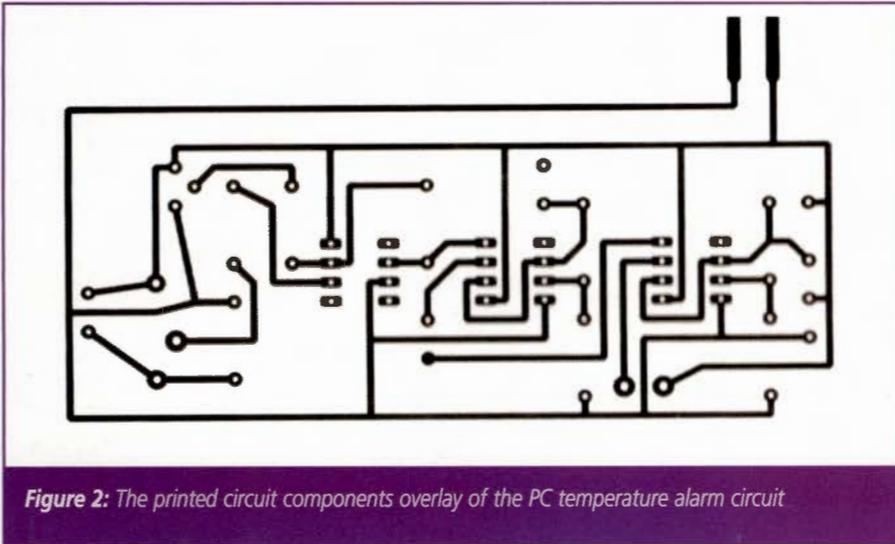
Figure 2: The printed circuit components overlay of the PC temperature alarm circuit
