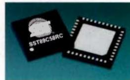
SST (Silicon Storage Technology), flash memory technology supplier, announced a new addition to its FlashFlex family of 8-bit microcontrollers (MCUs), the SST89C58RC. The new device is the industry's first 8051-based MCU to feature two system management buses (SMBus), each supporting up to 400kbit per second data throughput, in a 6mm x 6mm QFN package.
