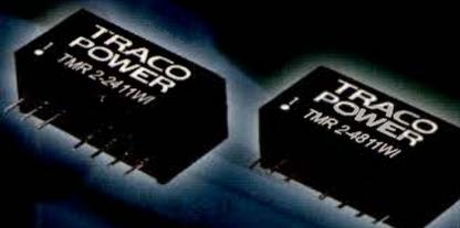
TMR2WI Series is a miniature 9 pin SIP 2 Watt DC-DC Converter with an ultra wide 4:1 input range of either 9-36V or 18-75V DC. Outputs are regulated 3.3V, 5V, 12V, 15V,  $\pm 5V$ ,  $\pm 12V$  or  $\pm 15V$  DC. An excellent efficiency of up to 84% allows operation over a temperature range of -40 to +75°C. Other features include 1500VDC input to output isolation, remote On/Off control, continuous short circuit protection and excellent line and load regulation.
