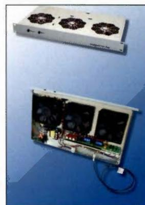
Verotec has extended its range of 19" 1U standard fan trays. Two depths are available, a 250mm deep unit fitted with three fans and a 350mm deep unit with six fans. All sizes are offered with a choice of 12, 24 or 48 VDC fans or 115 or 230 VAC fans, and each unit is available with or without a replaceable filter. Each DC fan is rated at 170m<sup>3</sup>/h, the 115 VAC fans at 180m<sup>3</sup>/h and the 230VAC fans at 160m<sup>3</sup>/h.
