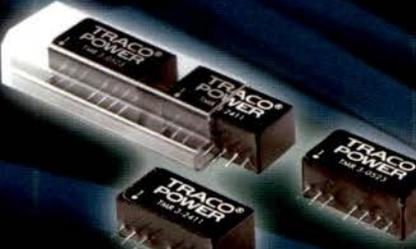
TMR3 Series DC-DC Converters offer 3 Watts of output power in an ultra compact 8 pin SIP package. Input range is wide 2:1, with either 4.5-9V, 9-18V, 18-36V or 36-75V DC. Outputs are regulated 3.3V, 5V, 12V, 15V,  $\pm 5V$ ,  $\pm 12V$  or  $\pm 15V$  DC. Efficiencies of up to 81% allows operation over a temperature range of -40 to +75°C. Other features include 1500VDC input to output isolation, remote On/Off control, continuous short circuit protection and excellent line and load regulation.
