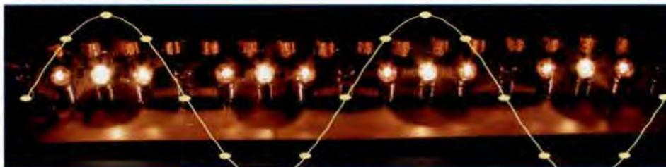
**Figure 12:** Short circuit terminated line, with sinewave superimposed. The line length corresponds to a total delay of two cycles of a 12.5 kHz signal
