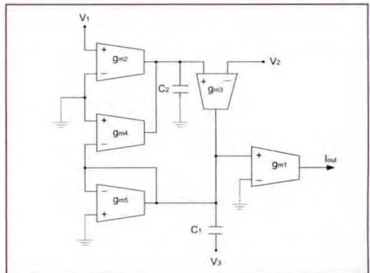
Figure 1: Proposed universal filter circuit with input voltage and output current
