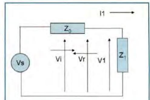
**Figure 15:** Incident and reflected waves
