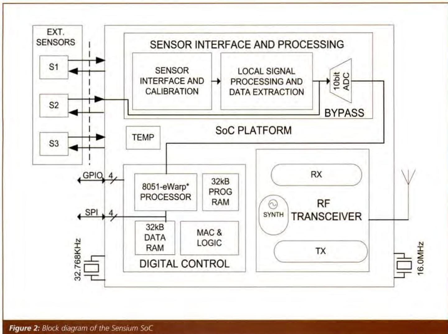
**Figure 2:** Block diagram of the Sensium SoC
