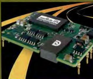
Murata Power Solutions has introduced its new UEI-series of isolated, wide-range DC/DC converters that deliver industry leading 50-60W of power output from a standard 40.6 x 50.8 x 10.16mm (1.6in x 2in x 0.4in) PCB-mounted, open frame package; plastic cased versions
