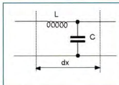
**Figure 3:** Lumped constant with single inductive and capacitive element for a line section  $dx$ ; assuming that the leakage and series resistances can be ignored
