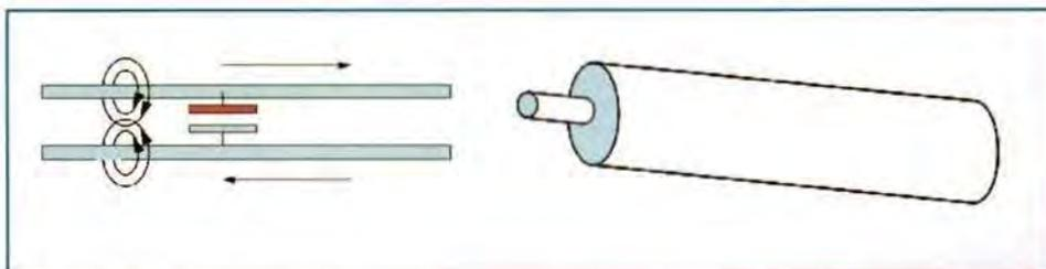
**Figure 1:** (a) A parallel wire pair, showing capacitive and inductive elements; and (b) A coaxial cable comprising an outer conductor, usually made from a braid or plain wires and having an inner wire separated by a plastic insulator
