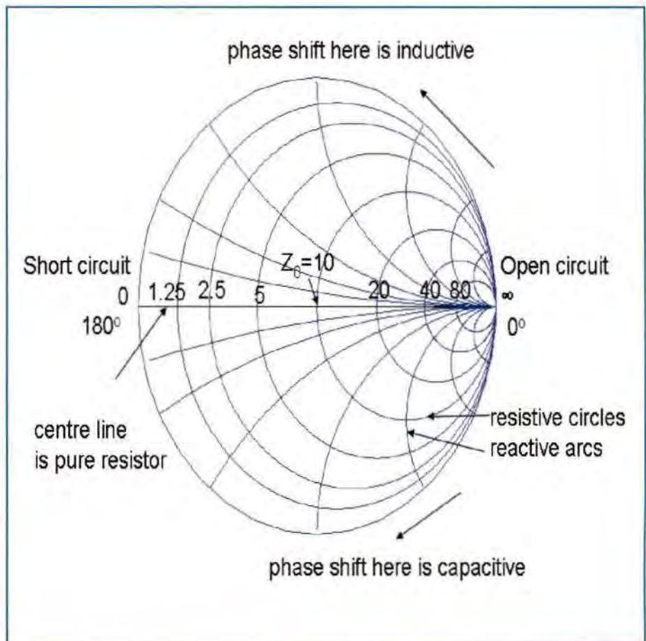
Figure 16: Smith chart, centred on 10 ohms for use with the Transmission Line Model
