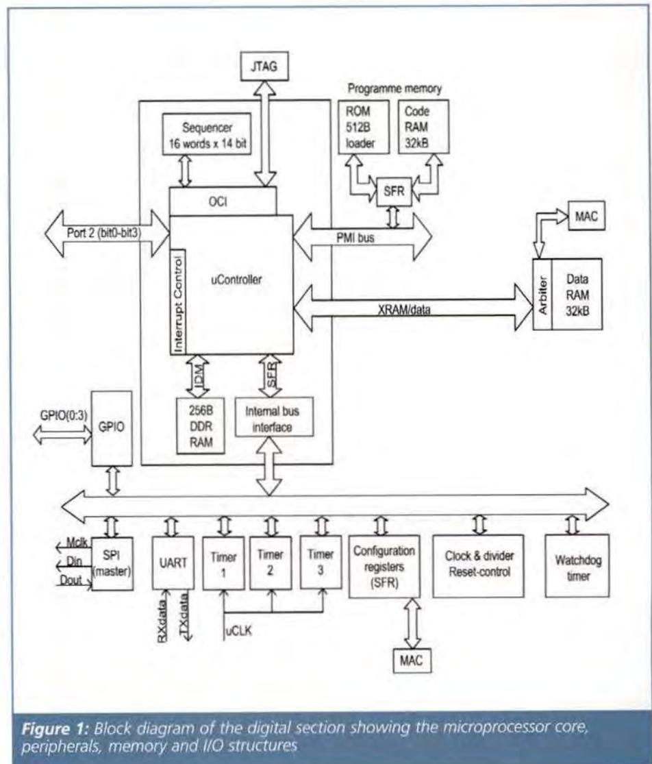
**Figure 1:** Block diagram of the digital section showing the microprocessor core, peripherals, memory and I/O structures
