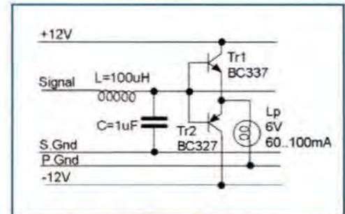
Figure 7: Line element of the model. There are 15 such sections.
