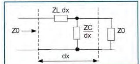
**Figure 5: Lumped element model of line showing impedances for the line section dx**
