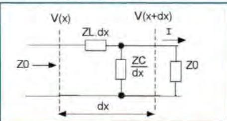
Figure 6: Lumped element model this time showing voltage and currents in line
