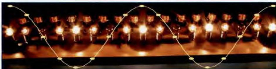
**Figure 13:** Open circuit terminated line, with sinewave superimposed. The brightest lamps are now at the line ends compared with **Figure 12**
