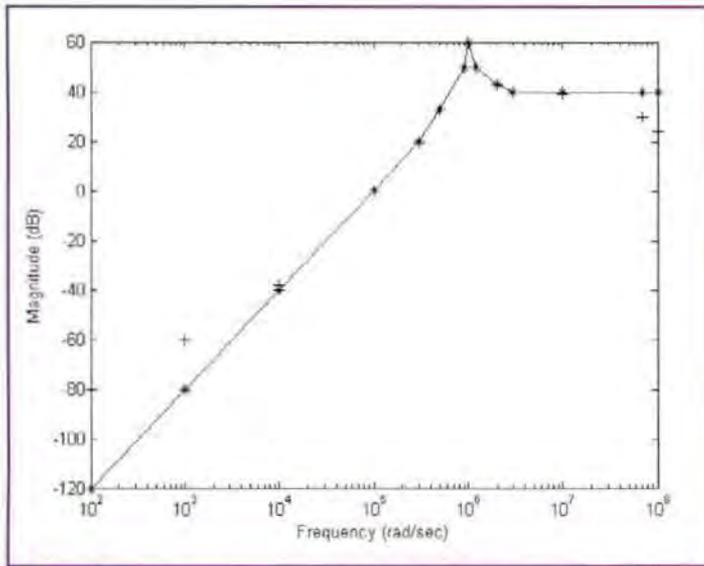
Figure 4: Experimental (+) and calculated (\*) results obtained from the highpass realisation
