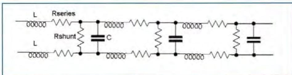
**Figure 2:** Generic equivalent circuit of a transmission line comprising inductance along the length; capacitance between the wires and resistances in series and in parallel representing the wire resistance and leakage paths between the wires
