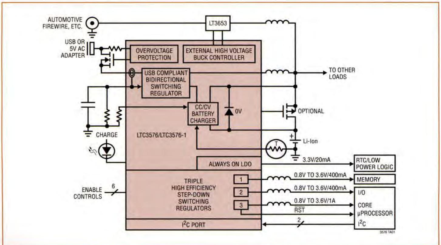
Figure 1: LTC3576 simplified block diagram
