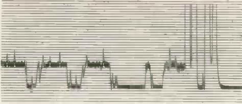
Fig. 2.—Signal from Brussels showing "Atmospherics."
