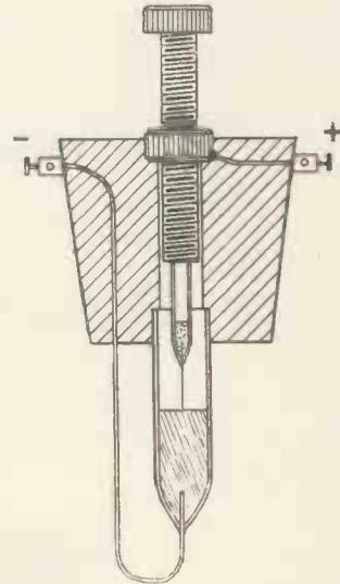
The positive electrode is put into a glass tube of a little larger diameter, which contains some sulphuric acid (10 per cent. solution) and the negative electrode of lead.
