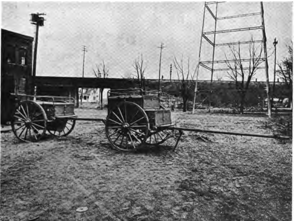
Fig. 1. Complete Installation on Two Carts. Instrument Cart in front, Power Cart behind.
