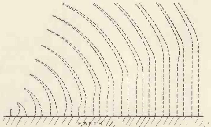
Fig. 1.—Effect on lower part of wave of potential gradient normal to the earth's surface.
