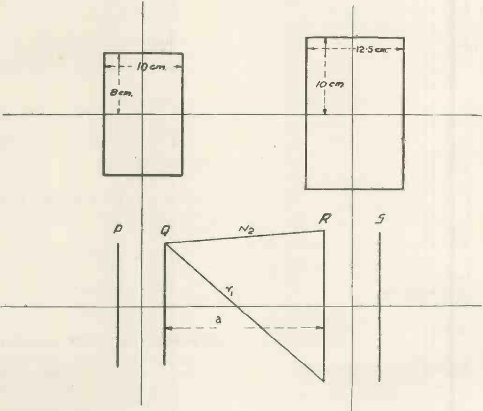
The mutual inductance of two coils can now be obtained by first calculating the mutual inductance between two circles of the same radius at a distance apart, equal to that of the middle turns of the coils, and multiplying by  $n_1 n_2$
