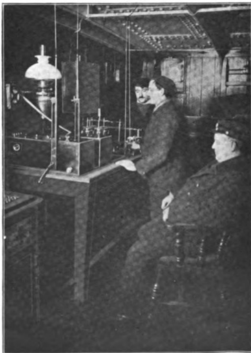
LIGHTSHIPS WERE VERY EARLY FITTED WITH WIRELESS TELEGRAPH. THIS PHOTOGRAPH SHOWS THE INSTALLATION ON BOARD THE TONGUE LIGHTSHIP IN 1900.
