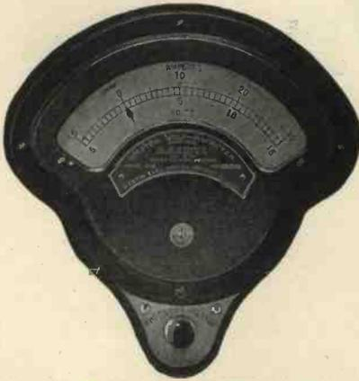
Model 268 Switchboard Volt-Ammeter.
