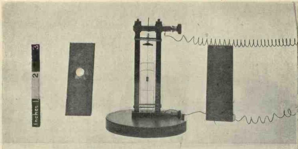
TWISTED STRIP AMMETER FROM THE INVENTOR'S LABORATORY.
