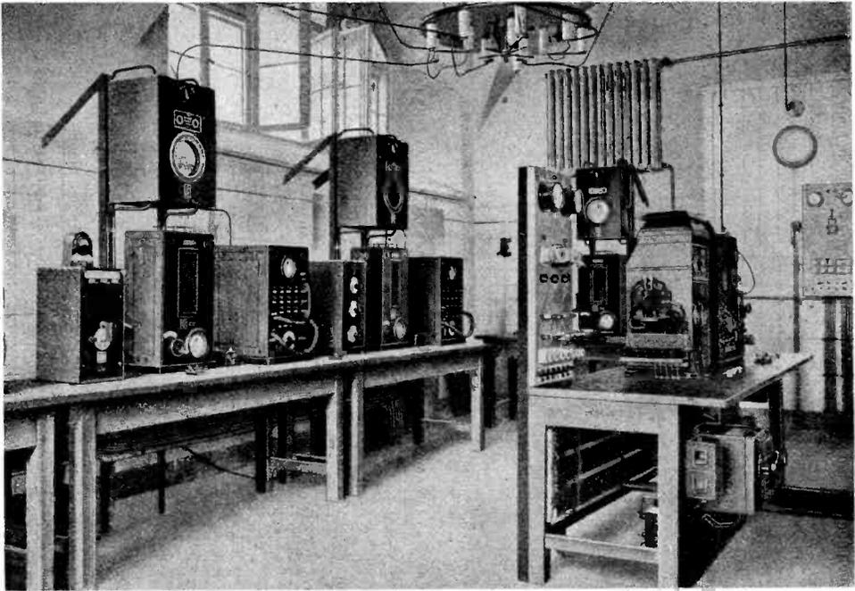
*Fig. 7. The 0.5 to 1 kW transmitting sets.*
