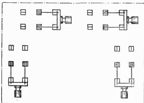
Fig. 7.—Detector valve and note magnifying valve.
