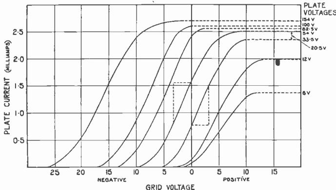
Filament current .6 amp. 20.5 volts plate
