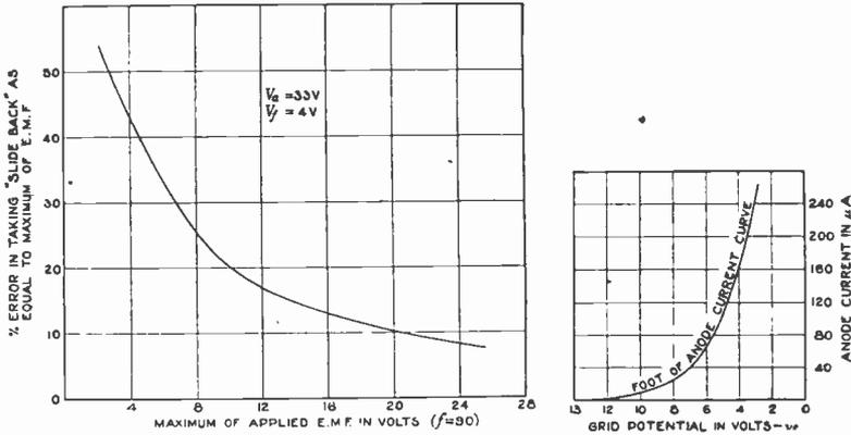
Fig. 7. Curves for R Triode No. 34817.
