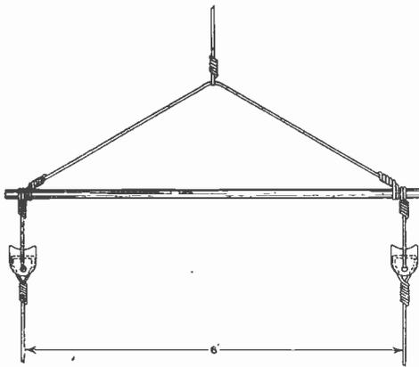
Fig. 3. Method of attaching Spreader to Rope.
