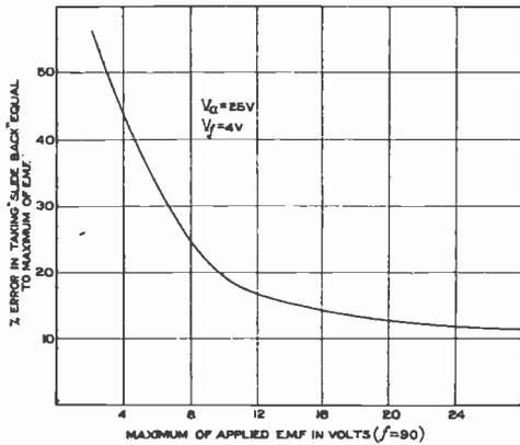
Fig. 8. Curve for R Triode No. 34817.
