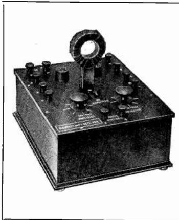
The first valve is a radio-frequency amplifier and the second a detector. The output is suitable for connection to H.R. Telephones or to any Note Magnifier. Used with a set of BURNDDEPT Patent COILS, all waves from 140 to 25,000 metres are covered. One set of BURNDDEPT Patent COILS on standard plugs can be used *both* for the Anode Reactance and for aerial tuning inductance; it is not necessary to have two separate sets of coils.
