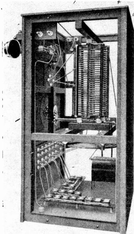
Fig. 6. A Wave Change Panel of the 5 to 10 kW transmitter.
