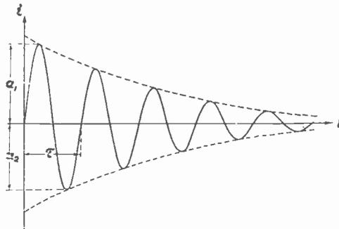
Fig. 2. Oscillating Current Curve.
