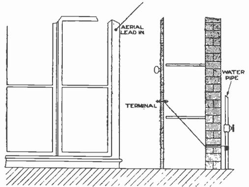
Fig. 4.—The aerial is led in through a hole drilled in the window frame. No leading in insulator is used. On the right is shown the terminal for the earth lead. It is fixed in the woodwork of a cupboard.
