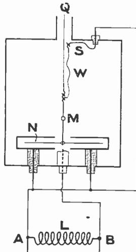
Fig. 3. Quadrant Electrometer with Connections.
