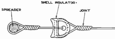
Fig. 2. Method of attaching Aerial Wire to Insulator, and Insulator, to Spreader.
