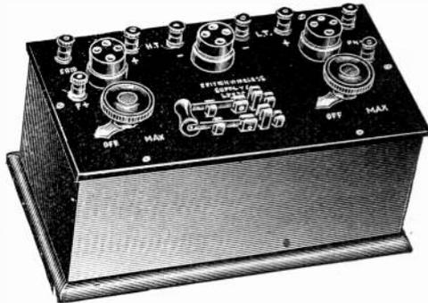
Three-valve Receiver with one H.F., one Rectifying, and one L.F. step, for all wave-lengths 150-25000 metres. Especially good for Telephony.
