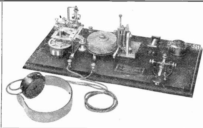
THE Omnigraph has been produced to successfully fill out a gap that has existed for years. The Omnigraph actually brings an expert operator into your home. Connected with Key and Sounder or with Wireless Buzzer and 'Phone the Omnigraph is ready, at all times, to send you perfect Morse or Wireless messages, at any speed you desire.
