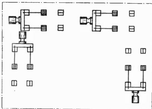
Fig. 8.—High-frequency amplifier followed by detector.
