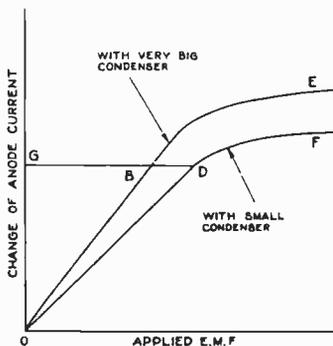
Fig. 5. Two Calibration Curves to determine Effective Resistance of Voltmeter.
