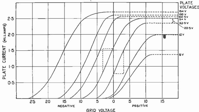
Filament current .6 amp. 20.5 volts plate = 6.833 amplification.
