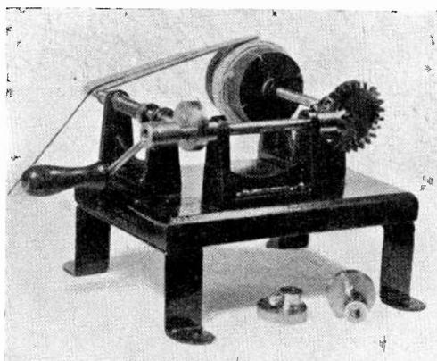
Although the manufacturer's instructions on the operation of the machine are a good guide and will lead one to the successful construction of very beautiful coils, the user is reminded that it is essential to keep a good pull on the wire while winding and to keep the oscillating rod pressed hard against the cam.
