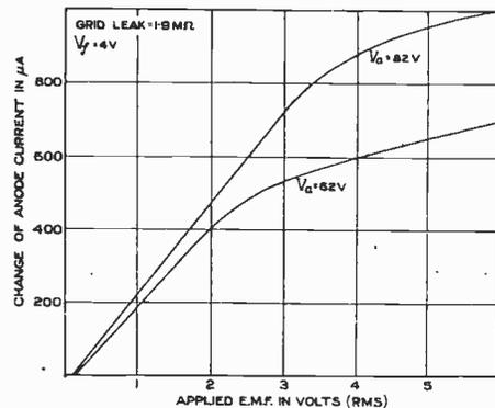
Fig. 2. Calibration Curve of Rectifier Voltmeter.
