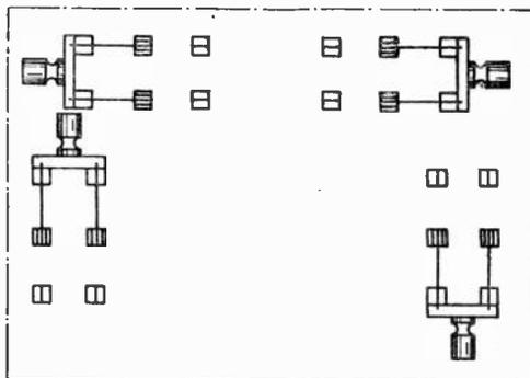
Fig. 9.—H.F., detector and note magnifier used together. Note: The switch in the right-hand corner connects the final valve either to H.T. telephones (upper position) or transformer and L.T. telephones (lower position, as shown).
