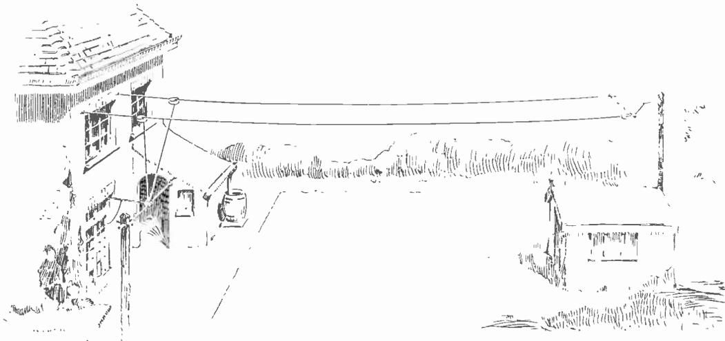
Fig. 1.—It is a mistake to think that high aeriels are necessary for long distance reception. The aerial described in this article is only 20 feet high and, as shown in the sketch, is of modest proportions. The total length of wire is 140 feet. The free end is due south.
