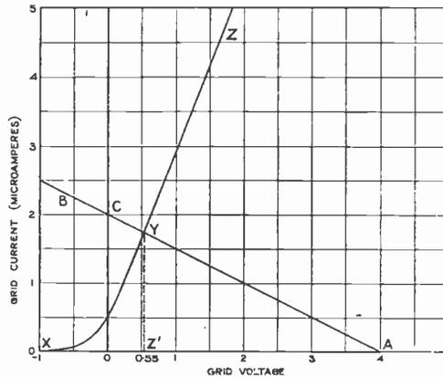
That is to say, the slope of this line should equal the resistance of the grid leak. For example, suppose, as described by Mr. Phillips, the grid leak resistance = 2 megohms, and the potential difference across the filament = 4 volts, we should set off OA = 4 volts and OC = the current passed by 2 megohms on 4 volts—
