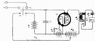
Fig. 125. A simple Call Device which rings a bell when a dash of predetermined length is received.
