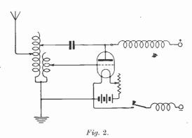
"FRAME AERIAL" (Leicester).-We sug. gest you employ the first aerial arrangement. It would be better if you could use an outdoor aerial, but you should receive signals with the proposed arrangement, although another H.F. valve will be required to make the signals of satisfactory strength. We think a three-valve set, using 1 H.F., 1 detector and 1 L.F. valves, will be required, and a suitable diagram is Fig. 4, page 147,
