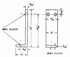
Fig. 6. Supports for coil former.
