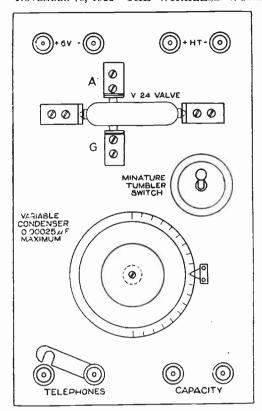
Fig. 9. Lay-out of instrument top.
