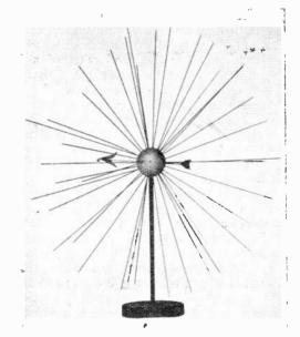
$\vec{F}_{ig}$ . 44. A golf ball with radial wires in it to represent an electron in motion. The electrolines crowd up into the equatorial plane.
