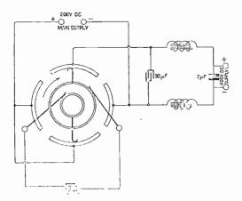
Fig. 12. Method of obtaining plate current supply.
