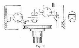
Fig. 2 shows a simple arrangement for substituting tuned anode in the place of intervalve transformers. Two tappings are taken out on the winding as it is put on, and the fitting of a three-way switch on the receiving instrument panel provides a tuned anode coil having a wide range.
