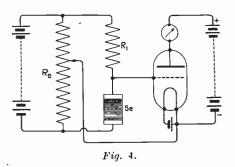
proximity. The cells are then subjected to a sensitising process, which consists of heating for about one hour at a temperature of 210° C., and then slowly allowing to cool. Then the cell is painted over with a transparent varnish for the purpose of protecting the cell from damp. A cell constructed in this manner has in the dark a resistance of 10,000 to 500,000 ohms., and a moderate illumination will change the conductivity of a good cell by 10 per cent.
