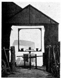
Fig. 5a. Portable single-frame direction finding set
