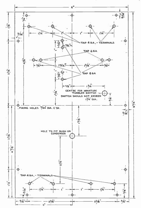
Fig. 2. Drilling diagram for ebonite top.
