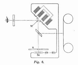
lag of the selenium cell, which can be estimated in this matter, other considerations which affect the frequency, such as the intensity of illumination, or the lag of the oscillograph being calculated and allowed for.
