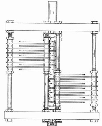
Variable Condenser for Tuning Two Circuits simultaneously.
