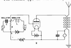
Fig. 7. Coupling arrangements.
