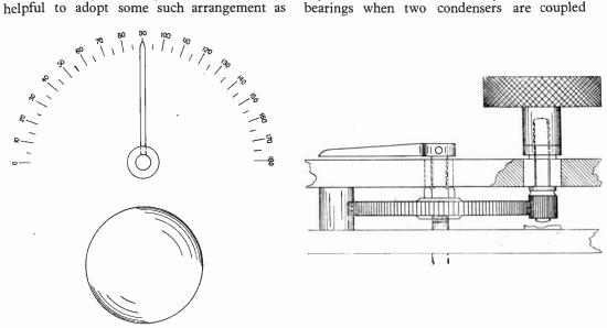
Geared Condenser Control to revolve coupled Condensers.
