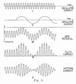
of the characteristics. This system is distortionless only to the extent that the characteristic can be assumed to be a straight line, or if some steps are taken to compensate the action of a curved characteristic.
