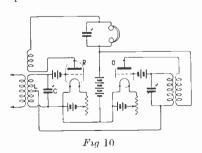
of varying the plate voltage of the amplifying tube R by means of the vacuum tube oscillator O coupled into the plate circuit. In this arrangement a third tube D acts as a detector. This is essential when an audible frequency is employed; when a super-audible frequency is used the telephones can be placed directly in the plate circuit of the amplifying tube.
