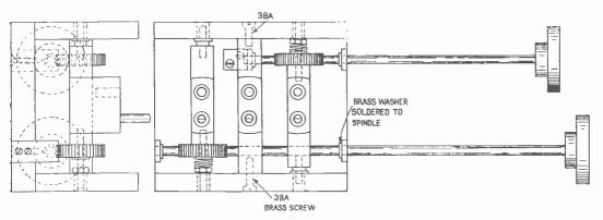
Fig. 6. Critical control for inductances with friction clip for wide movement.
