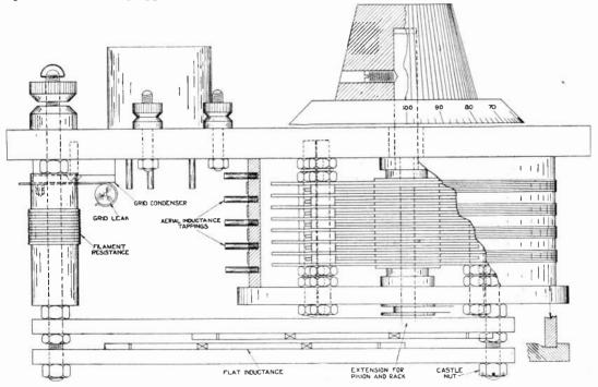
Suggested Design for a Single Valre Broadcast Receiver. The condenser spindle may be extended to carry a pinion to engage on rackwork to increase reaction coupling as the capacity of the tuning condenser advances.
