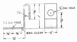
Fig. 5. Springy end clip for valve holders.
