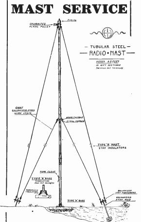
Made of best quality solid drawn steel tubes, to aircraft specification for strength and lightness. Designed for EASY ERECTION.
