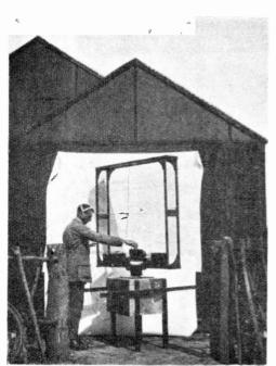
Fig. 5c. Portable single-frame direction finding set.
