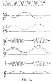
E.M.F. is removed. This free oscillation starts with an amplitude which is proportional to the impressed force, and this proportionality is maintained throughout any finite time interval (with constant impressed electromotive force).
