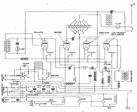
Fig. 8. Circuit diagram of the Transmitter.
