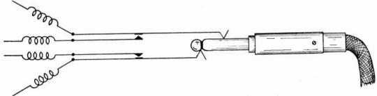
Fig. 1. L.F. Valves. Four-point break jack and plug.
