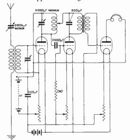
according to the degree of reaction coupling required, these turns being common to the tuned anode circuit and the plate circuit of the second valve.
