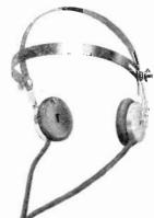
TELEPHONE HEAD SETS specially designed for wireless work. Terminals enclosed to prevent receiving circuit being interfered with. Earpieces are provided with groove on surface to minimise condensation of moisture.
