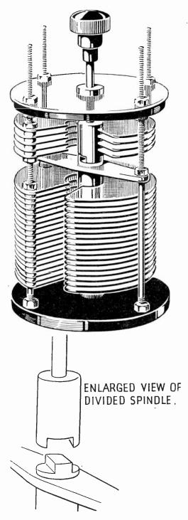
Fig. 3. A condenser in which provision is made for moving only a few of the plates.
