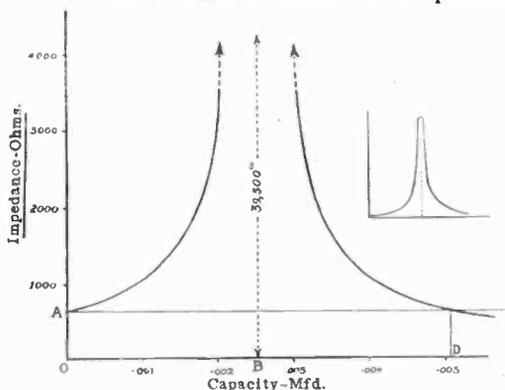
Fig. 1. Curve showing the relation between capacity and impedance. Inset: Full curve drawn to a smaller scale.
