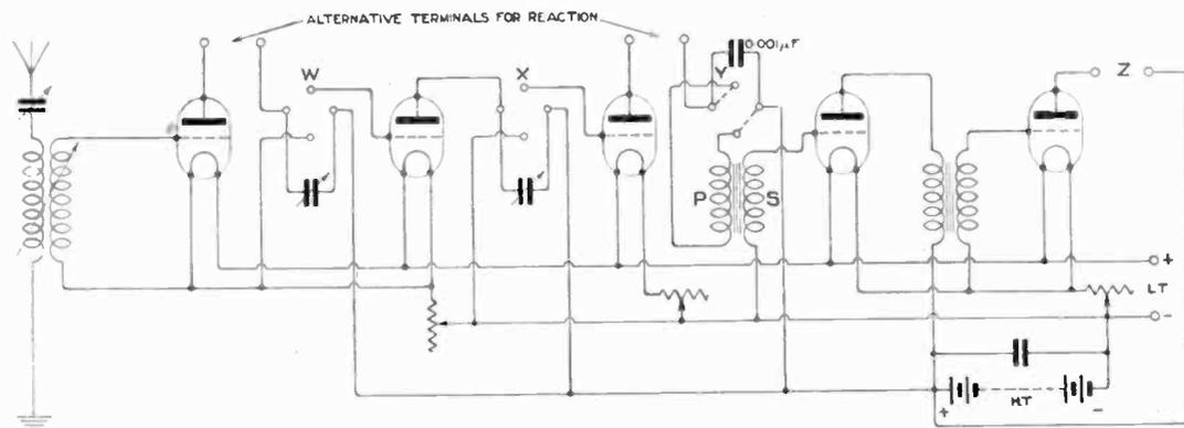
Fig. 4. Circuit diagram of the Experimental Receiver.
