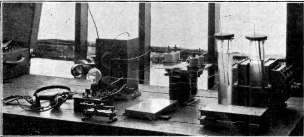
*Receiving apparatus making use of alternating current for heating the valve filament. The step-down transformer is in the centre, whilst on the right is an electrolytic rectifier arranged for supplying the H.T.*
