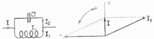
Fig. 2. Tuned circuit and Vector diagram.
