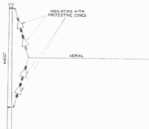
By so distributing the insulators, full advantage is taken of the shielding cones to protect the insulators themselves from the effect of rain.
