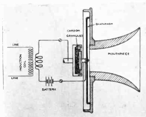
Fig. 76. A solid back granular Carbon Microphone Transmitter.
