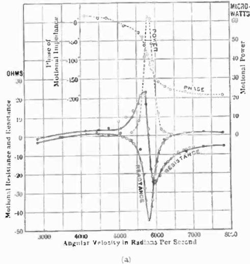
Fig. 84. Curves obtained by Dr. A. E. Kennelly for the Motional Resistance, Reactance and Power absorption of a Magneto-Telephone receiver. Note. The angular velocity signifies 6.28 times the frequency of the alternating current.
