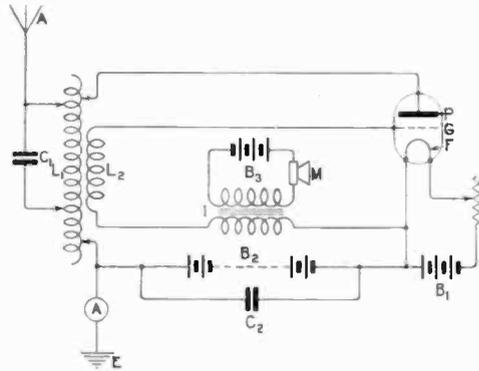
Fig. 89. Circuits of a simple form of wireless telephone transmitter showing the speaking microphone M coupled inductively through an induction coil I to the grid circuit L<sub>2</sub> of the thermionic valve.
