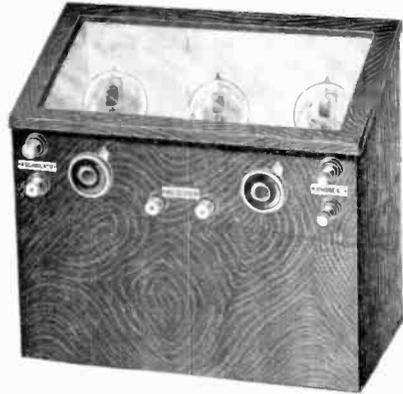
The panel, valves and high tension batteries are all enclosed in a highly finished "figured oak" cabinet, with bevelled edged plated glass top. The advantage of this arrangement will be seen at once. The terminals are so arranged on front of the cabinet that it can be used in conjunction with all Receiving Sets (Crystal or Valve) with the minimum of outside wiring. Its magnification is equal to the best on the market.
