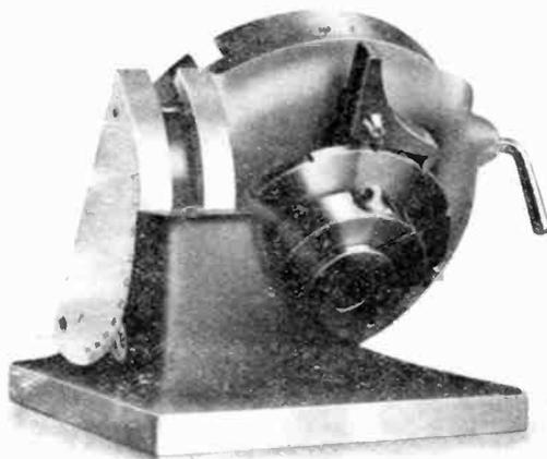
The Taylor-Hobson Dividing Head is designed for work on circular, conical and cylindrical surfaces.
