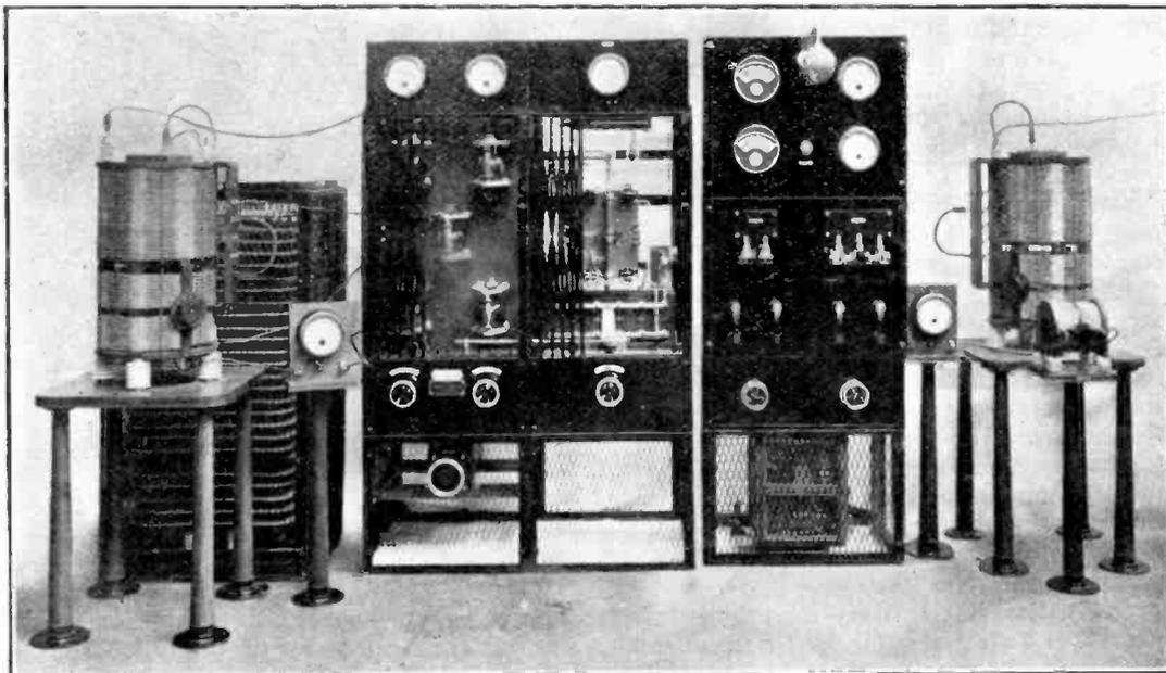
*Marconi type valve transmitter. The power panel is on the right, and the rectifier and oscillator valve panel in the centre. The air dielectric condenser is enclosed in a cage on the left. Tuning inductances are on either side.*
