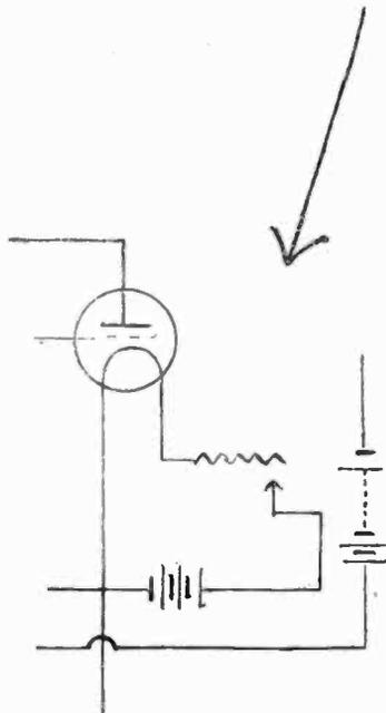
**WEAK** signals may usually be traced to the plate or filament battery. Your batteries should frequently be checked. Our two scale voltmeters reading 0/10 and 0/100 volts save the expense and inconvenience of two instruments.
