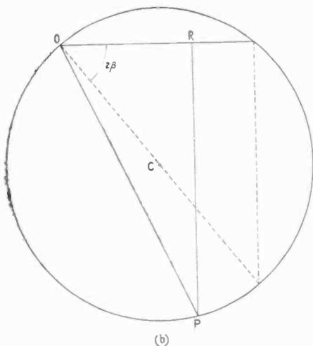
Fig. 85. Circle of motional impedance constructed by plotting the motional resistance horizontally  $OR$  and the motional reactance downwards vertically  $RP$ , the diameter of the circle measuring the impedance of the telephone.
