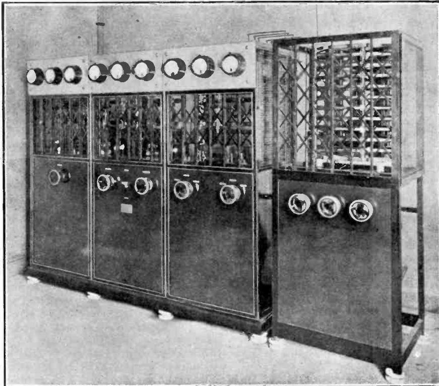
Fig. 1. The valve telephony transmitter of the "Radiola" Concerts.
