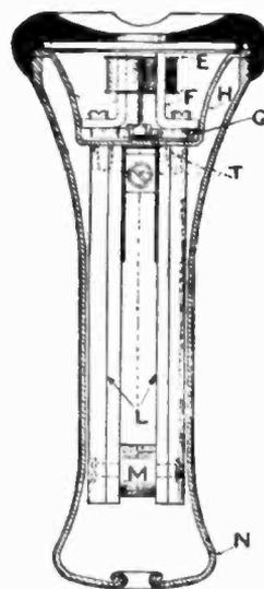
Fig. 79. British Post Office type of Magneto Telephone receiver.
