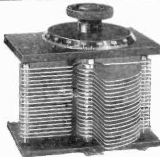
Specification of our well-known CONDENSERS. Highest grade Aluminium Plates. Brass Washers machined to a limit of + or - .001" Adjustable Brass Bush at bottom, Fixed Brass Bush at top. These Condensers are built to stand HARD continuous usage and we GUARANTEE THEM.
