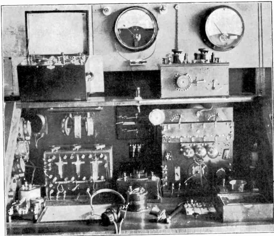
*The station of Mr. C. Maclurcan at Sydney, N.S.W. Successful communication tests employing C.W. and Tonic Train have been carried out with S.S. "Montoro" at distances of 420 and 705 miles on power estimated as only 8.7 watts.*
