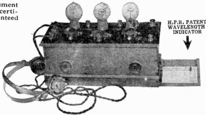
**R**ANGE of Wavelengths 300 to about 1,000 metres, covering all British Broadcasting transmissions—ship and coast stations (spark and C.W.)—aeroplane telephony. Readily tuned to incoming wavelength by the H.P.R. Patent Wavelength Indicator. The patent H.P.R. tuned high frequency coupling inductances, combined with fully variable reaction (non-interfering), render the Hilophone extremely selective. It is so sensitive that it may be tuned to receive even
