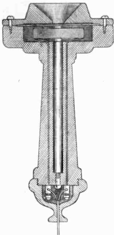
Fig. 75. Section of a Bell Magneto Telephone.
