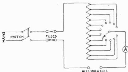
*A circuit arranged for accumulator charging from D.C. mains. Provision is made by means of a twelve point switch for varying the amount of resistance in circuit, so that the charging rate can be adjusted according to the capacity of battery on charge.*
