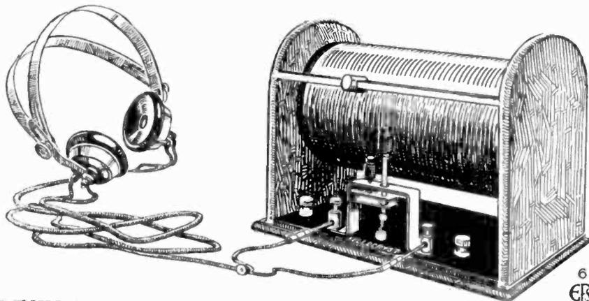
**T**HIS is an excellent crystal receiving set, which gives very good results on all wavelengths from 300-1,500 metres, and is suitable for receiving broadcasting, ships and long distance stations.
