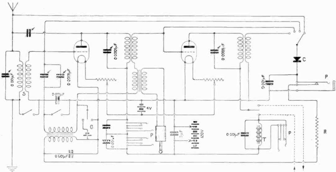
*The simultaneous amplification circuit providing two stages high-frequency amplification; crystal rectification; two stages of low-frequency amplification.*
