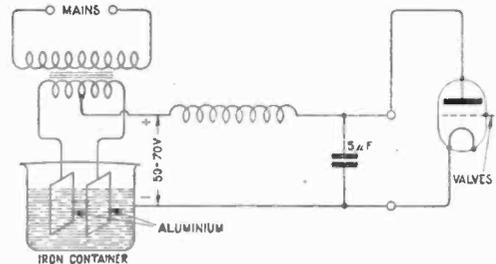
Fig. 1. The Electrolytic Rectifier and smoothing circuit.
