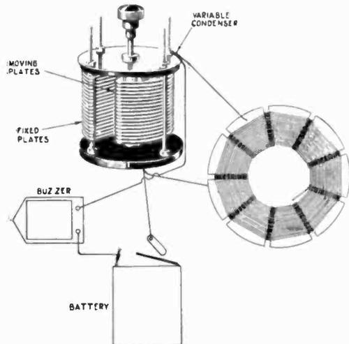
Fig. 2. The Connections. The inductance is here shown exactly  $\frac{1}{3}$  full size.
