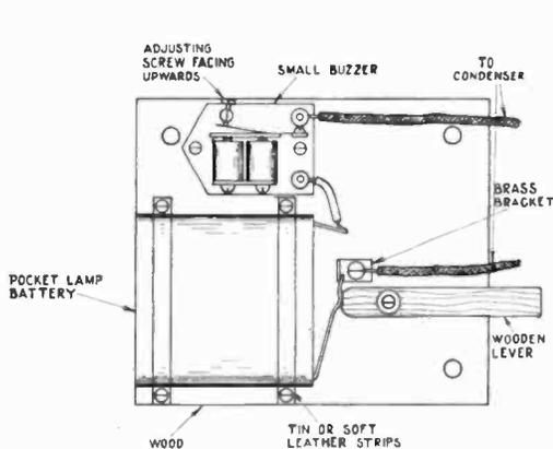
Method of assembling buzzer and battery.
