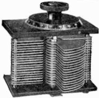
Specification of our well-known CONDENSERS. Highest grade Aluminium Plates, Brass Washers machined to a limit of  $\pm$  or  $-001$ " Adjustable Brass Bush at bottom, Fixed Brass Bush at top. These Condensers are built to stand HARD continuous usage and we GUARANTEE THEM.
