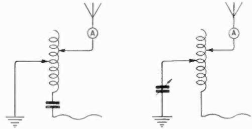
Fig. 7. An earth connection may be combined with the counterpoise in the manner indicated in the figure. The correct connection to be employed depends essentially upon the transmitter connections, and the experimenter will have no difficulty in adapting the arrangement to meet his own needs.
