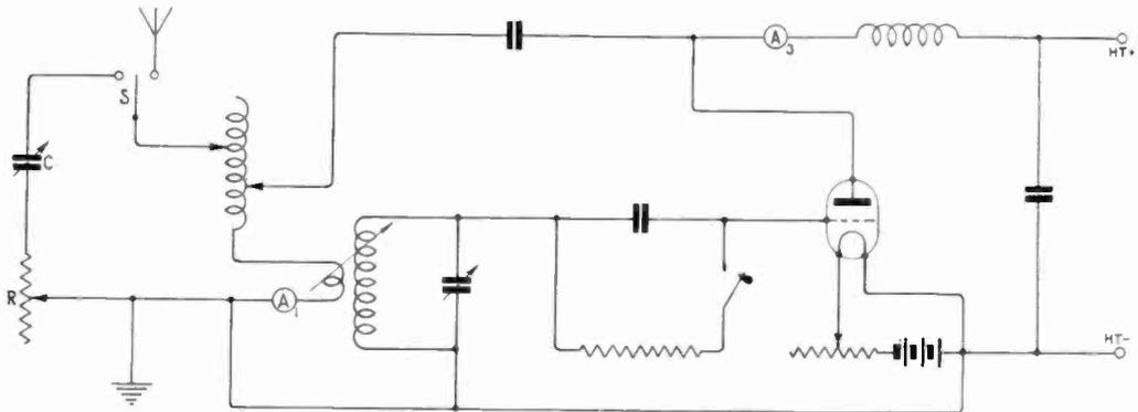
Fig. 2. Here the aerial circuit is directly coupled with the valve generator. The transmitter is the same in principle as that given in Fig. 1.
