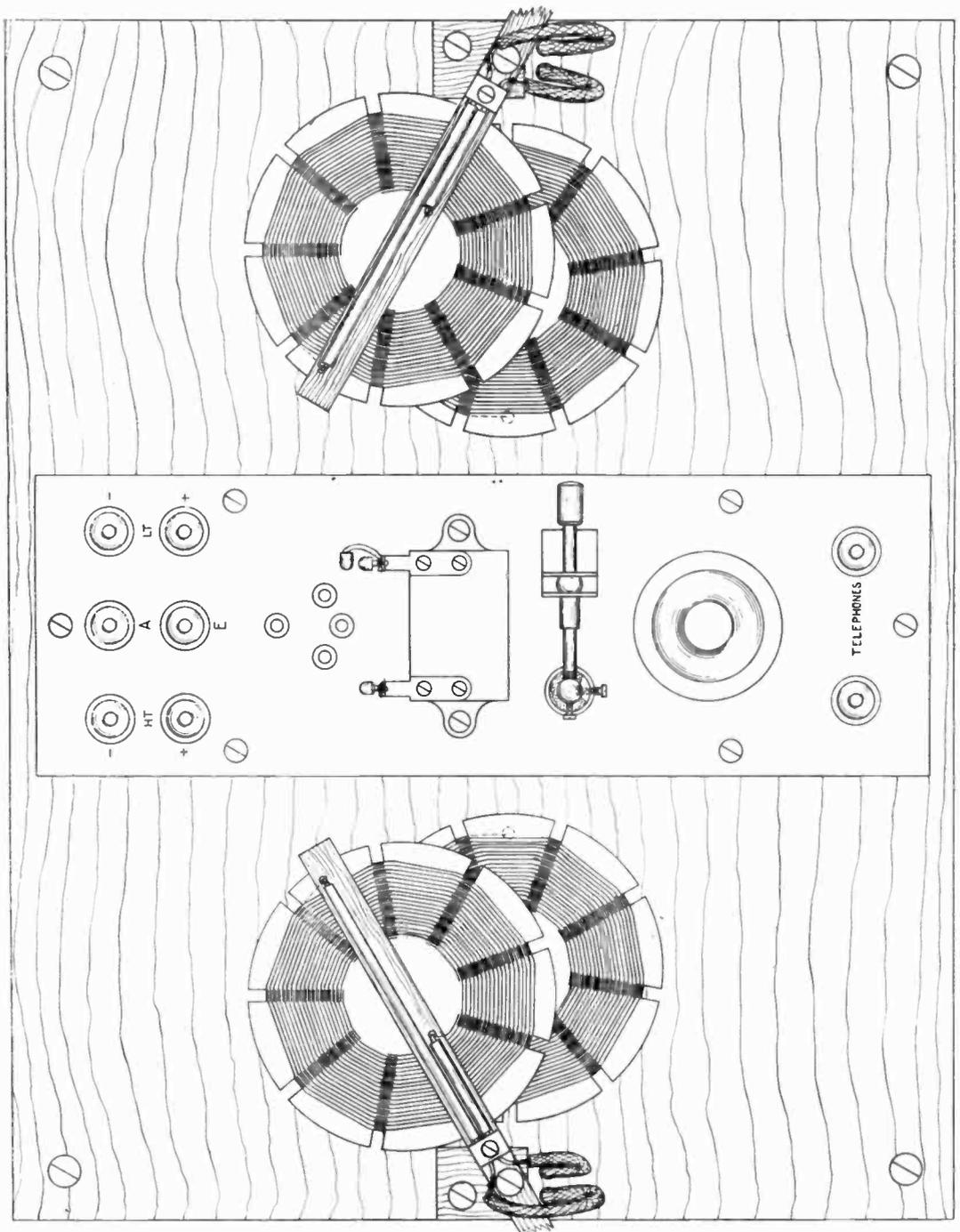
Fig. 3. The complete receiver, with H.F. amplifier and valve detector. It is drawn to scale, and the overall dimensions are 12" x 9 1/4".
