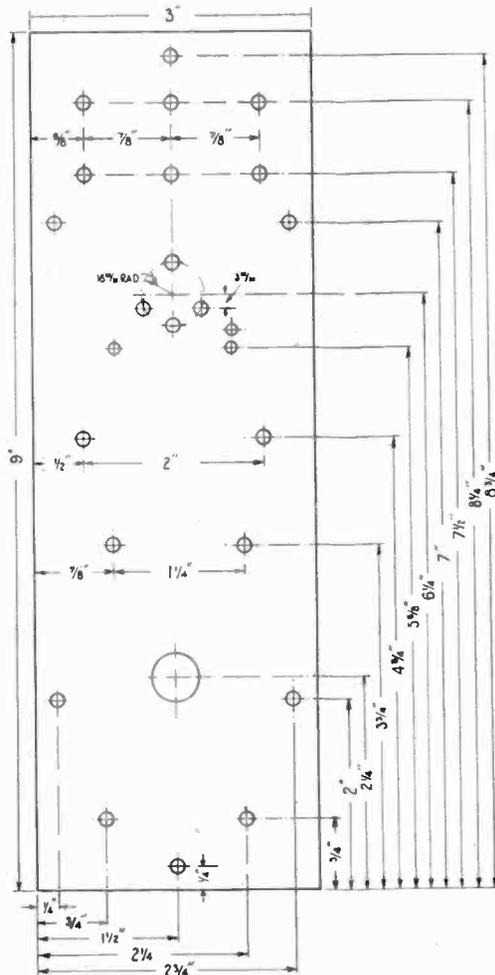
Fig. 2. The setting out of the holes in the ebonite panel.
