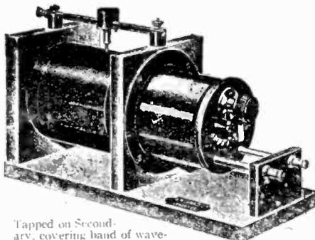
Tapped on Secondary, covering band of wavelengths 300 to 1,000 metres. Undoubtedly the most efficient for shorter wavelengths, especially with crystal receivers, for it gives greater selectivity and increases range of reception.
