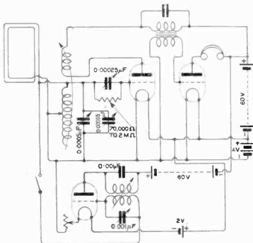
Fig. 1. Two-valve Receiving Circuit adapted for super-regenerative action.
