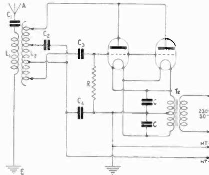
Fig. 6. Final type of oscillation circuit.
