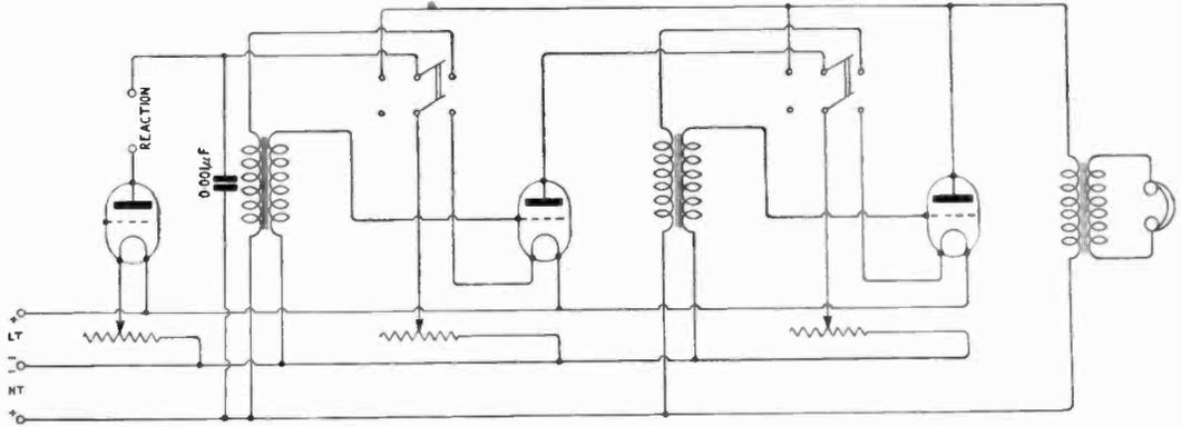
Fig. 1. The circuit shows the switching of two note magnifying valves.
