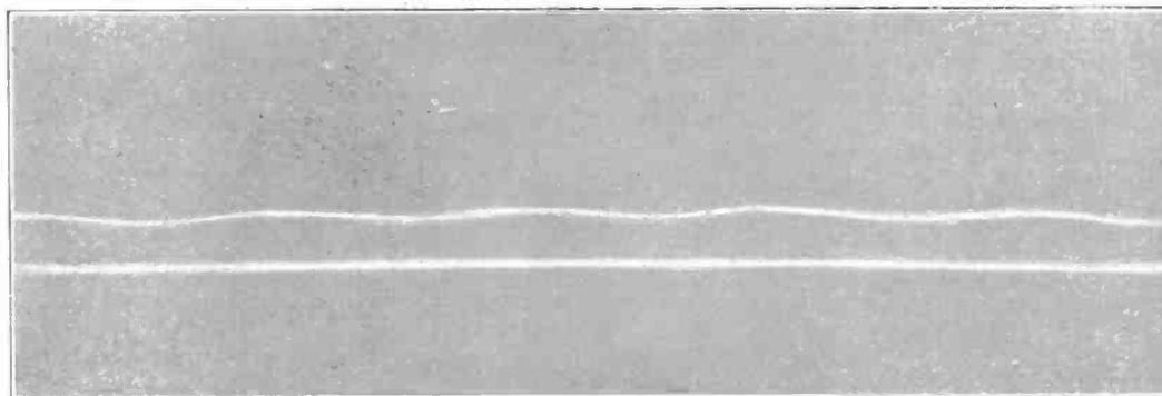
Fig. 3. Voltage after passing Rectifier and smoothing choke and condenser. Frequency 50 cycles.
