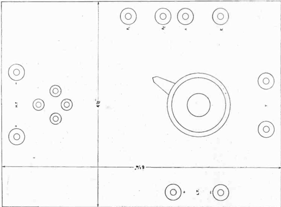
Fig. 1. Scale drawing of the top of the panel, showing lay-out of terminals and valve holder. The actual size is  $6\frac{1}{4}'' \times 4\frac{3}{4}''$ .
