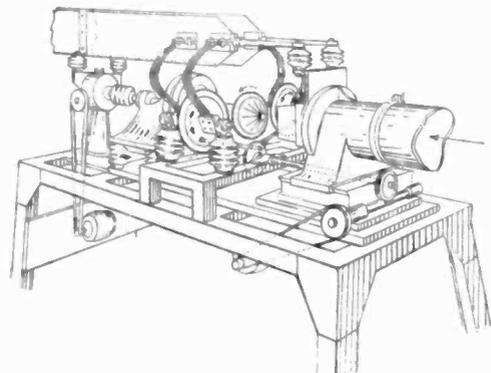
Fig. 2. The spark discharger, showing the two gaps.
