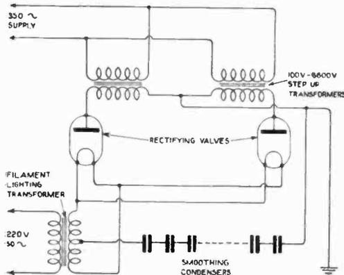
Fig. 4. The Rectifying circuit.
