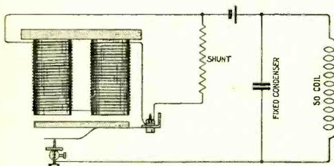
Fig. 10. The shunted buzzer arranged to produce oscillations of definite frequency for use in conjunction with the circuit shown in Fig. 11 for calibrating a variable condenser.
