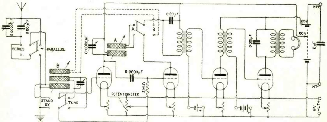
The diagram gives the connections of a four-valve receiver. The reaction coil may be connected at A or B by the switch.
