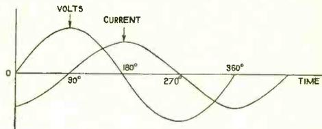
Fig. 39. When an alternating pressure is connected to a condenser, the current which flows, leads the applied pressure by 90°, that is the current flowing has its maximum value when the voltage applied to the condenser is zero. The current falls off as the pressure rises.
