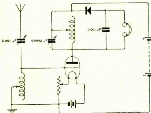
Fig. 5. “D.E.B.” (Cambridge). H.F. amplifier with crystal detector.
