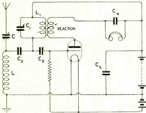
The reaction coil is coupled to a closed oscillatory circuit, which is excited by the transference of the potentials developed across the aerial tuning inductance.
