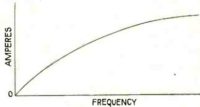
Fig. 43. The curve shows the increase in current in a circuit consisting of resistance and capacity in series. At very low frequencies, the condenser offers greatest opposition to the current flow. At infinitely great frequencies, the condenser offers little impedance to the current, and the resistance practically determines the magnitude.
