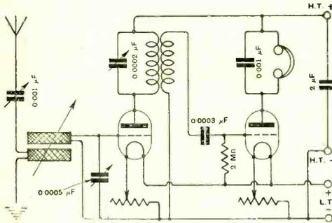
Fig. 1. "Amateur" (Cambridge). Diagram of a two-valve receiver. The first valve is coupled to the rectifier through a high-frequency transformer. The circuit is quite satisfactory for the reception of broadcast transmissions.
