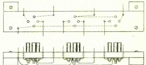
Fig. 8. Valve socket connections.
