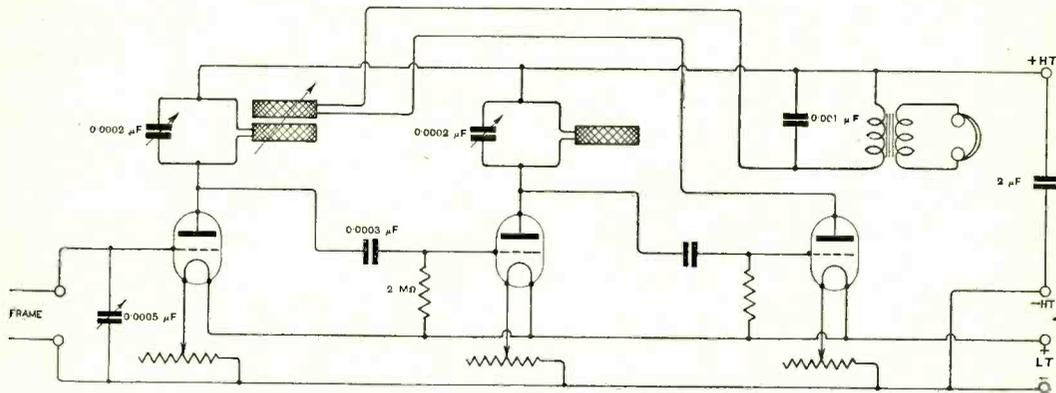
Fig. 3. "J.R.T.W." (S.W.11). The diagram gives the connections of a receiver with two high frequency and rectifier valve. The receiver may be used with a frame for short wave reception.
