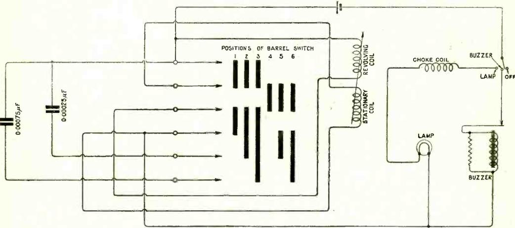
The wiring up of the wavemeter to this circuit does not produce an involved arrangement of leads to give the six wavelength ranges. The vertical strips represent the connectors on the drum switch in the six positions.
