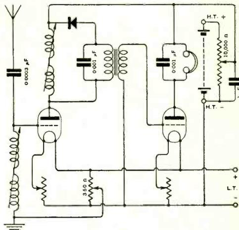
Fig. 4. "NEW READER" (Bearwood). H.F. amplifier, with crystal detector and note magnifier. The value of the H.T. is continuously variable. Care must be taken to break the battery circuit when not in use.
