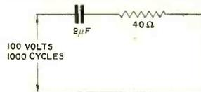
Fig. 44. Circuit consisting of capacity and resistance referred to in the example.
