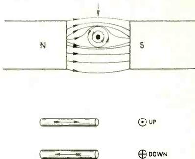
Fig. 30. With the magnetic field and the motion of the conductor as shown, the current in the wire will flow in a direction up out of the paper. When the current is flowing in the direction of the arrow, and the observer is looking at the point of the arrow, a dot is shown in the centre of the wire. When one is looking at the end of the arrow, a cross is shown on the end of the conductor.
