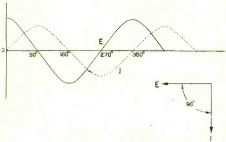
Fig. 45. The current flowing through a pure inductance lags behind the applied pressure by 90°, that is, the current has its maximum value when the pressure is passing through zero.
