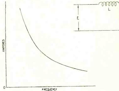
Fig. 49. The curve shows how the current flowing through a coil, when the applied pressure is held constant, varies with frequency.
