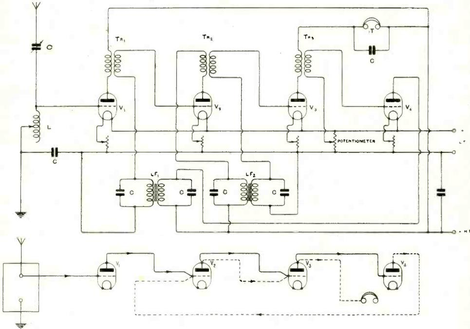
Fig. 6. Four Valves, Double Magnification.
