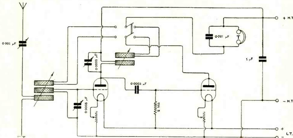
Fig. 1. "CIRCUIT" (Suffolk). The figure gives the connections of a two-valve receiver. The first valve operates as a high frequency amplifier, the second as a rectifier. The reaction coil may be coupled with either the closed circuit coil or the anode coil with the aid of the throw-over switch.
