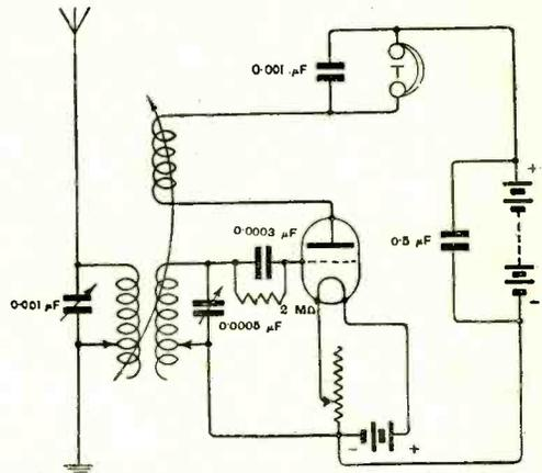
Fig. 2. **"C.M.L.S." (Surrey)**. Single-valve reacting receiver. Not suitable for the reception of broadcast transmissions, but very satisfactory for long wave work.
