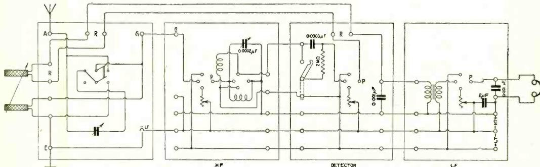
Fig. 2. "VERNIER" (Leeds). The diagram gives the connections of a unit system, comprising a tuner, high frequency amplifier, detector and note magnifier.
