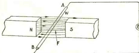
Fig. 29. When a wire moves across a magnetic field a pressure is induced in the wire, and when the external circuit is complete, a current will flow.
