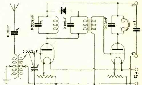
Fig. 4. "J.H.W." (Cheltenham). This diagram gives the connections of a receiver similar to that of Fig. 3, but instead of variometer tuning the coils are tuned with variable condensers.
