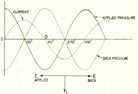
Fig. 46. While the current lags the pressure by 90°, the back pressure, or the induced pressure is 180° out of phase; that is, the back pressure acts in direct opposition to the applied pressure.
