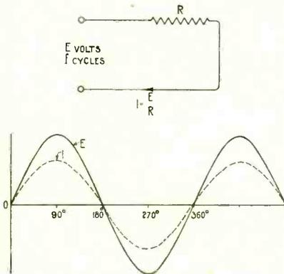
Fig. 38. When an alternating pressure is applied to a circuit consisting of resistance only, the current which flows is given by  $I = \frac{E}{R}$ . The current and pressure are in phase, that is, both rise and fall together.
