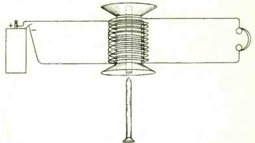
Fig. 3. Increase in signal strength with insertion of iron core.
