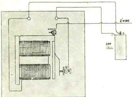
Fig. 5. Method of attaching the wire to the buzzer for the production of feeble electric waves.
