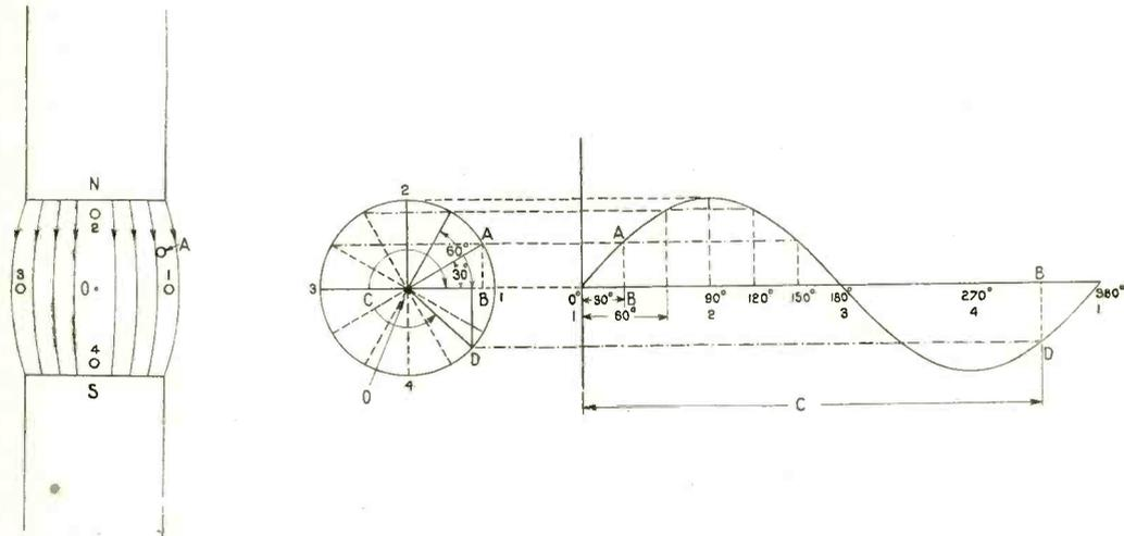
Fig. 37. The sine curve. The construction illustrated in the figure will enable one to construct a sine curve.
