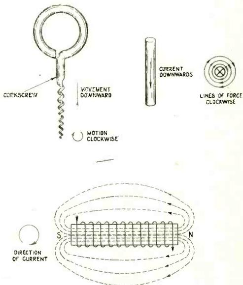
Fig. 31. The direction of the lines of force produced when a current flows in a wire may be found with the aid of the corkscrew rule. If the current is flowing down the wire, as represented by the cross, the magnetic field is as shown.
