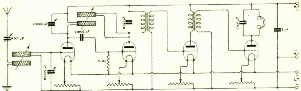
Fig. 4. “L.P.” (N.9). Four-valve receiving circuit.
