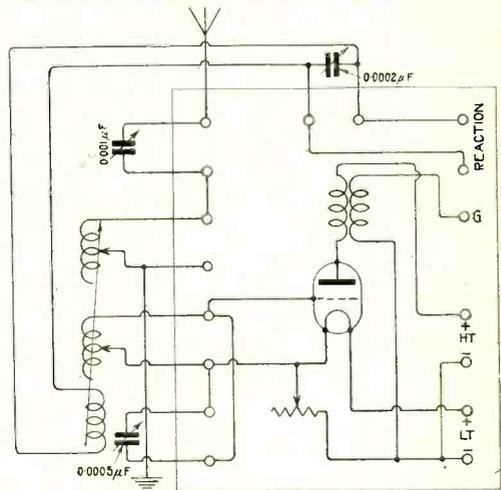
Fig. 6. **"AMATEUR ELECTRIC" (Cheshire)**. Diagram of a tuning and H.F. panel.
