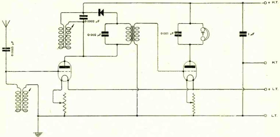
Fig. 3. "E.A.D." (Surrey). Here we have a two-valve receiver. The first valve operates as a high frequency amplifier, a crystal is used as a rectifier, and the second valve operates as a note magnifier. Variometer tuning is used. See Fig. 4.
