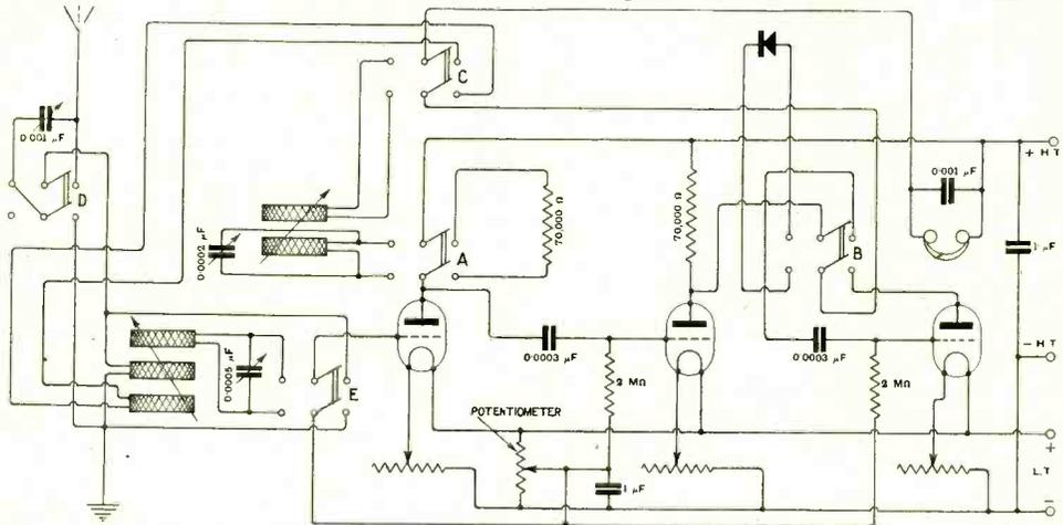
Fig. 3. "Atom" (Dulwich). This is the diagram of a three-valve receiver. Switch D [is a series-parallel switch, switch E a tune-stand-by switch. With the switch A in position A, the anode resistance is connected, while in the other position the tuned anode circuit is connected. Switch C is for reversing the reaction. With switch B in position B, the rectifying valve is connected, while when the switch is in the other position the crystal is used as a rectifier.
