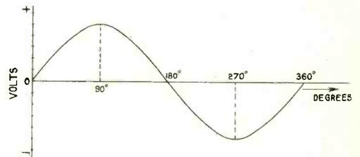
Fig. 36. The pressure induced in the loop varies as shown in the above curve, which is a sine curve, when the loop rotates in a uniform magnetic field.
