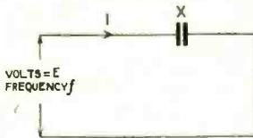
Fig. 40. The reactance of a condenser with capacity of  $C$  farads is  $\frac{1}{2\pi fC}$  and is represented by  $X$ .
