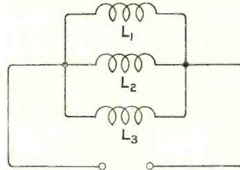
Fig. 28. When inductances are joined in parallel, the total inductance is less than that of the smallest, in the same way that the net resistance of resistances in parallel is less than that of the smallest resistance.
