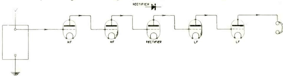
Fig. 1. Schematic Layout of Receiver.
