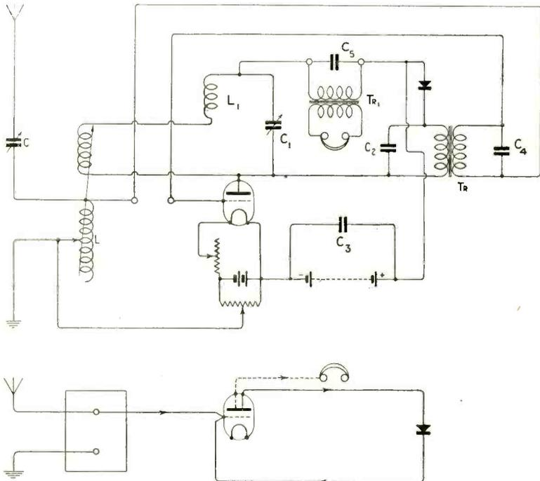
Fig. 3. Single-Valve Double Magnification.
