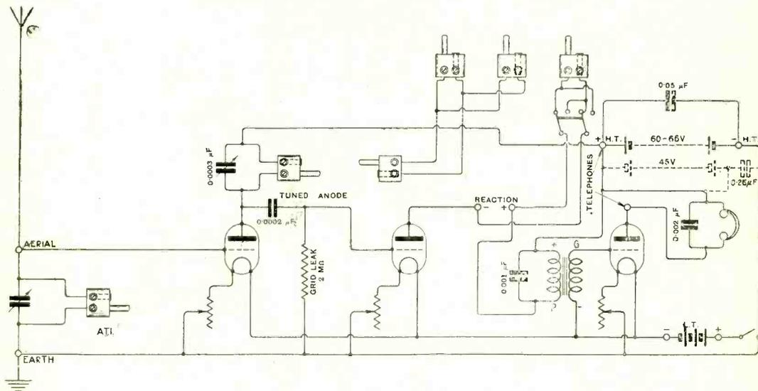
*The circuit provides for the transferring of reaction coupling from the tuned anode to the aerial circuit by means of the plug-in connectors.*
