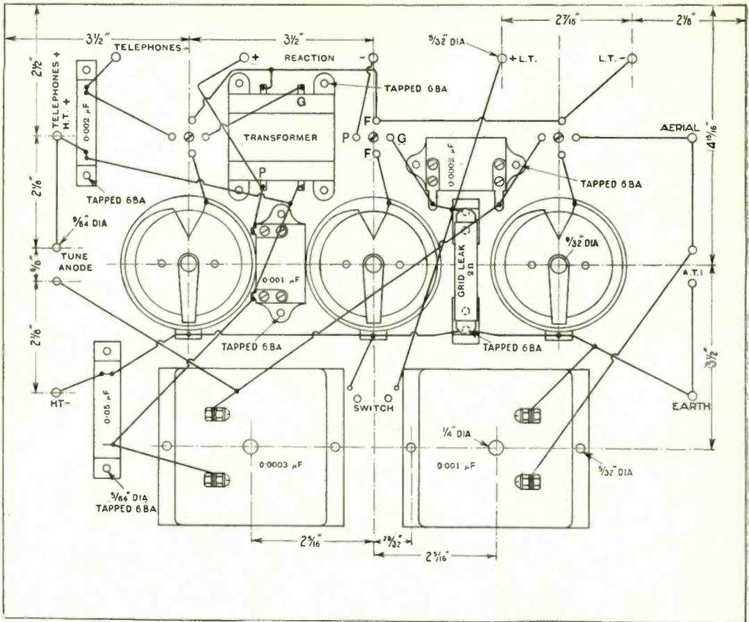
The lay-out of the components, showing the principal dimensions and practical wiring.
