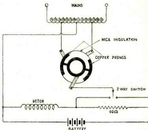
Fig. 3. The connection of the rectifier and the arrangement of the brushes.
