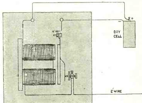
Fig. 6. Should the wiring up of the buzzer be as shown in this figure then the wire must be attached to the contact screw instead of the bracket which supports the armature
