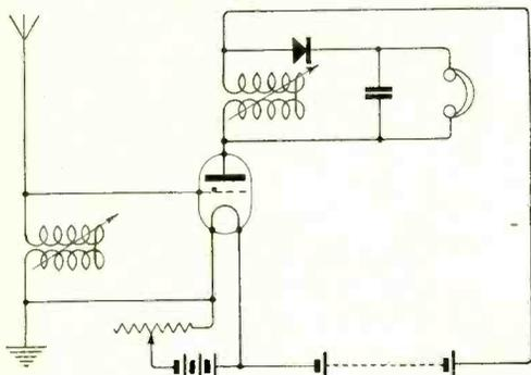
Fig. 5. Position 3. H.F. amplifier and crystal detector.
