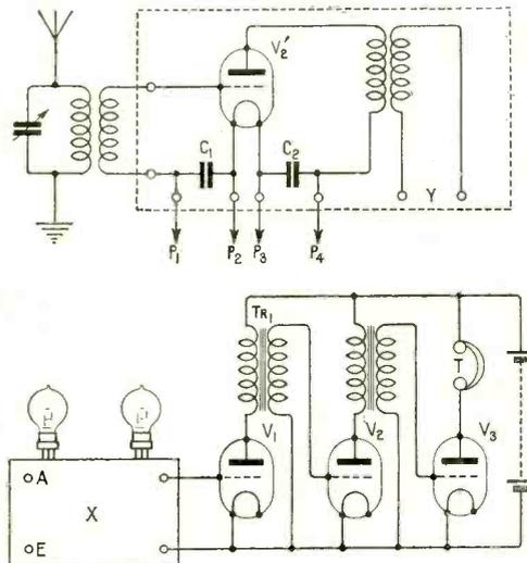
*Circuit and method of connecting component instruments for introducing dual amplification.*
