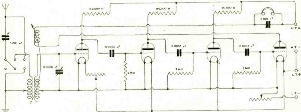
Fig. 2. "E.G.J." (Catford, S.E.6). Three H.F. resistance-coupled valves with valve rectifier and reaction.
