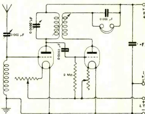
Fig. 2. "IND" (Manchester). Receiver with one stage of H.F. amplification with valve rectifier (1-v-0).
