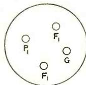
Fig. 16. The three-electrode valve, showing the method of connection between electrodes and connecting pins.
