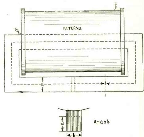
Fig. 76. A useful form of choke. The coil has  $N$  turns, and the cross sectional area of the iron  $A = a \times b$ . If the core is  $1\frac{1}{4}$ " by  $1\frac{1}{8}$ ", and the bobbin is 3" in diameter and  $4\frac{1}{2}$ " long wound with 5,500 turns of No. 26 D.S.C., the inductance will be approximately 6 henries and the resistance 115 ohms.
