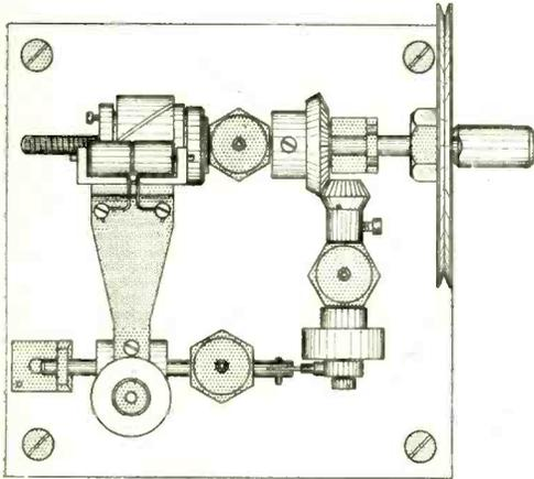
Fig. 2. Plan (drawn to scale). The dimensions of the base are  $5\frac{1}{2} \times 5\frac{1}{2}$ ". Other dimensions can be readily calculated by applying a rule to the drawing.
