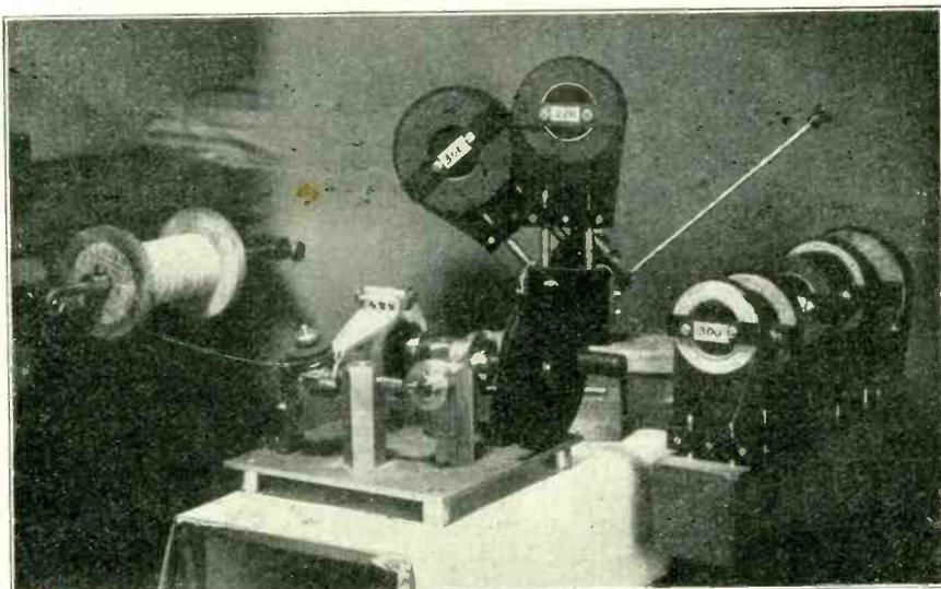
Fig. 1. The coil winder in operation showing a number of completed coils supported in suitable mountings.
