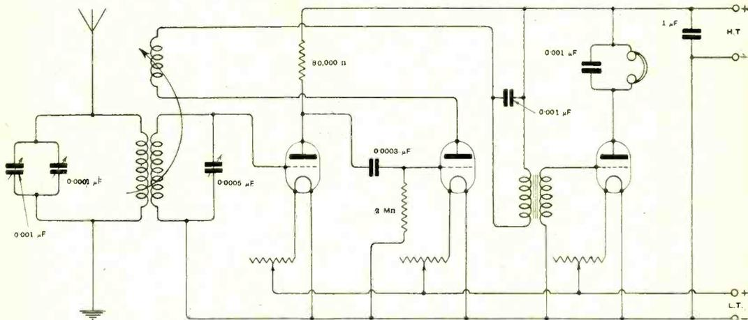
Fig. 1. "A.W.B." (Walthamstow). Diagram of a receiver with one stage of resistance capacity amplification, valve rectifier and note magnifier. (1 - v - 1).
