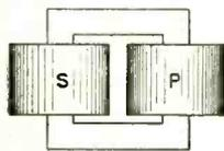
Fig. 87. Core type transformer.
