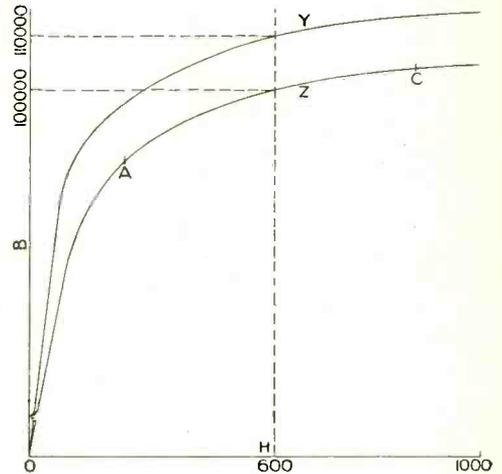
Fig. 72. Magnetisation curves of specimens of annealed sheet iron (curve  $Y$ ) and cast steel (curve  $Z$ ). The curves are the result of plotting the flux density  $B$  in lines per square inch against the magnetising force  $H$ . The curves are known as  $B$ - $H$  curves.
