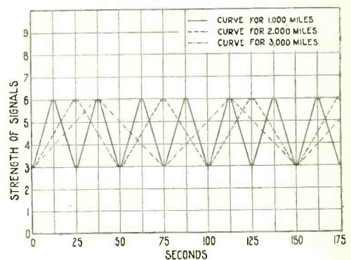
Fig. 3. Fading curves of signals 1,000, 2,000, and 3,000 miles.
