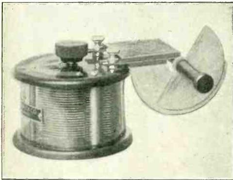
Variable Condenser with simple Vernier attachment.
