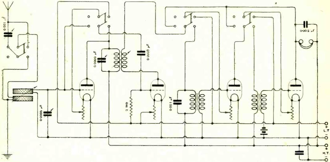
Fig. 3a. "EXPERIMENTAL" (Grove Park). Diagram and suitable layout of receiver with H.F. valve rectifier and two stages of note magnification, with switches to vary the valves in circuit.
