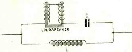
Fig. 3. An arrangement for preventing the steady plate current from passing through the windings of the Loud Speaker.
