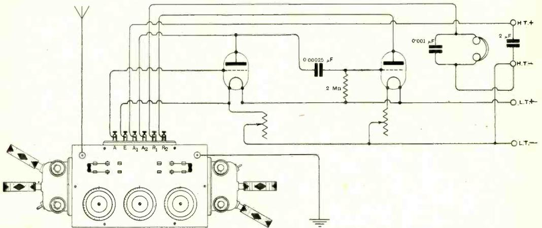
Diagram showing the method of connecting the tuner in circuit with a high frequency amplifier and detector valve set.
