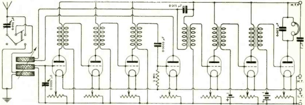
Fig. 6. "A.H." (Sweden). Connections of a 7-valve receiver with three stages of H.F. amplification, value rectifier and three stages of note magnification (3-v-3).
