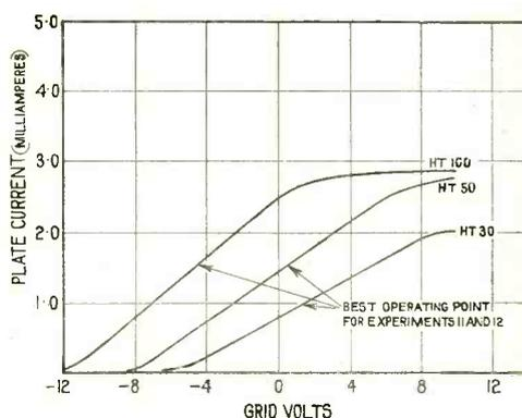
Fig. 19. Curves plotted from the results obtained in this experiment, showing the relationship between grid potential and plate current.
