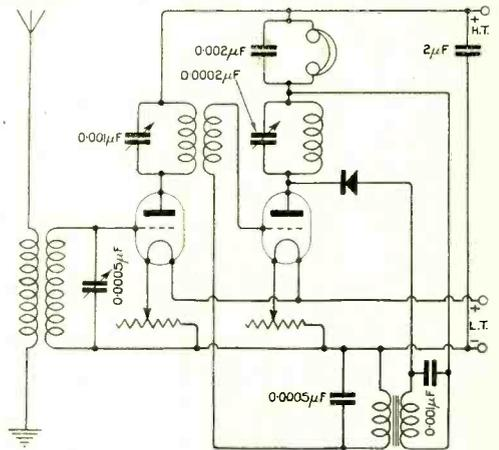
Fig. 1. "Queries" (Surrey). Receiver with two stages of H.F., crystal rectifier, the second valve also operating as a note magnifier.
