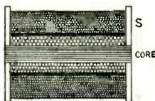
Fig. 88. Open core type transformer.
