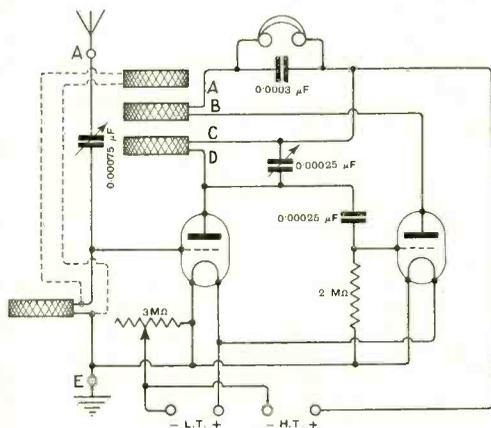
The principle of this circuit is the usual arrangement of reacting on to the tuned anode inductance.
