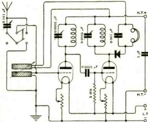
Fig. 3. **"DONEGAL" (Ireland).** The diagram shows the method of connecting a high frequency amplifier and a crystal rectifier (2-c-0). The two valves have tuned anode circuits.
