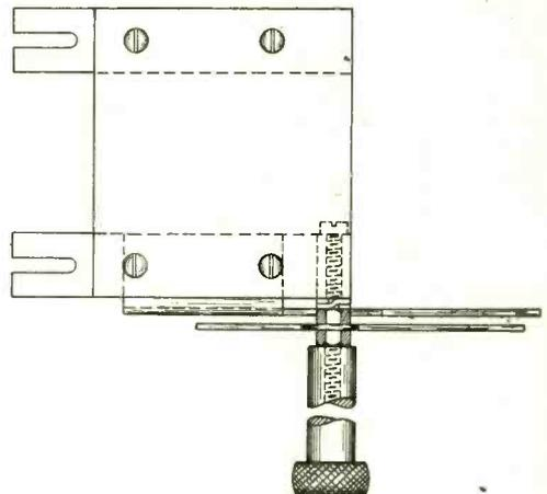
Constructional details of Vernier condenser design for fitting across the terminals of a variable.
