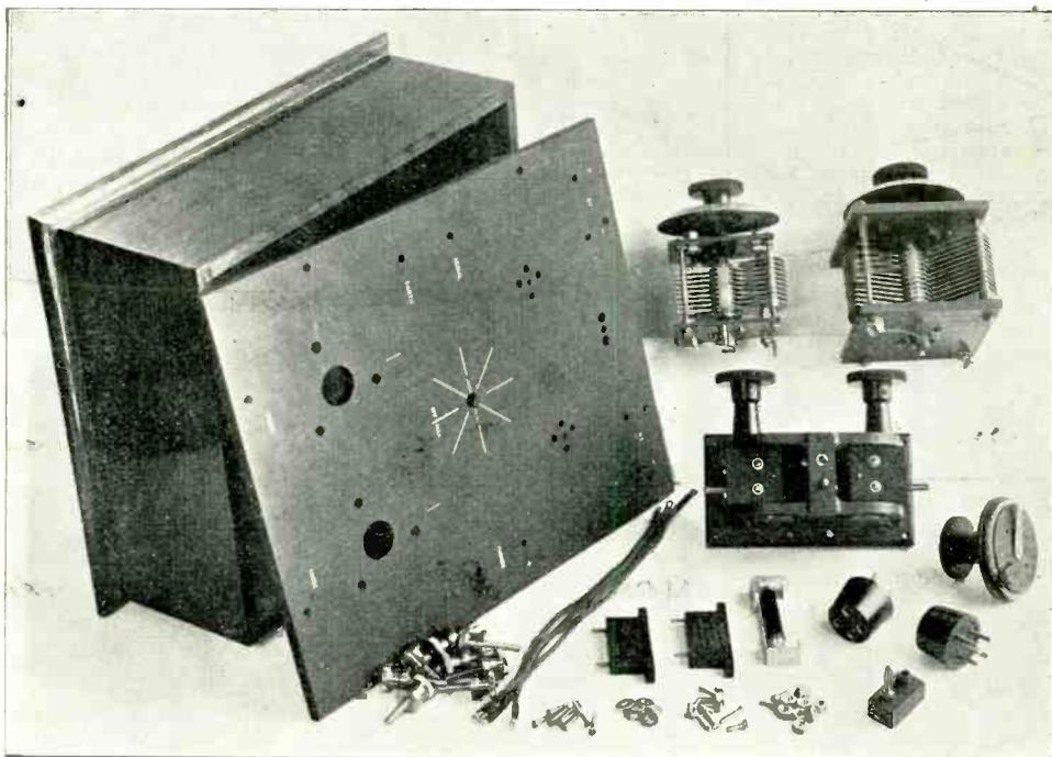
*Complete set of components designed by Messrs. Burndept, Ltd., for constructing the reacting H.F. and detector valve receiver.*
