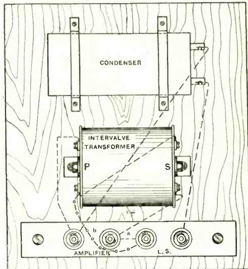
Fig. 5. Constructional details of an instrument for operating the Loud Speaker, embodying the principles described.
