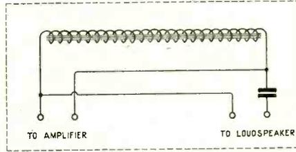
Fig. 4. Connections of an instrument for preventing the steady plate current from passing through the Loud Speaker winding. The fluctuating component of the plate current is fed through the condenser to the Loud Speaker.
