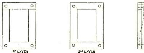
Fig. 90. Laminations used in the construction of a core type transformer. The bolts which hold the laminations together should not make contact with them, otherwise the eddy current loss will be larger than will be the case when the bolts are insulated.
