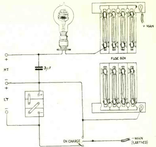
It is essential to employ a loose-coupled receiving circuit in cases where the source of high tension or filament current is earth connected.
