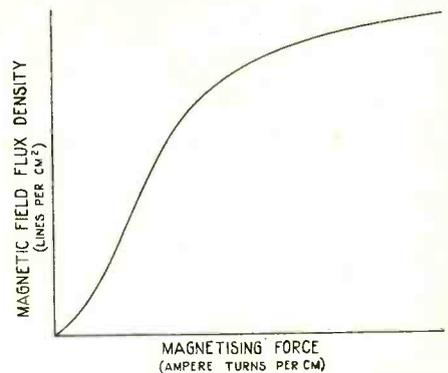
Fig. 1. Curve showing that the relationship between magnetising force and magnetic pull is not uniform. This is one of the contributory causes of distortion in amplifying apparatus having iron cores.
