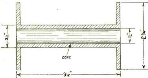
Fig. 78. Open core choke. If the former is wound with 6,000 turns, the inductance will be approximately 2 henries.
