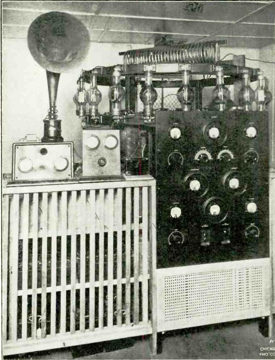
The layout of the transmitting gear at the Chicago Broadcasting Station, shown above, is of interest as it differs very much from the arrangement employed at the British broadcasting stations. Power is derived from a 10 kW. generator at 4,000 v.
