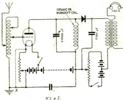
Fig. 21. This circuit is employed to amplify the oscillations prior to detection by the crystal.
