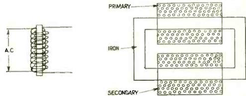
Fig. 80. A transformer consists of a core with a primary and secondary winding.
