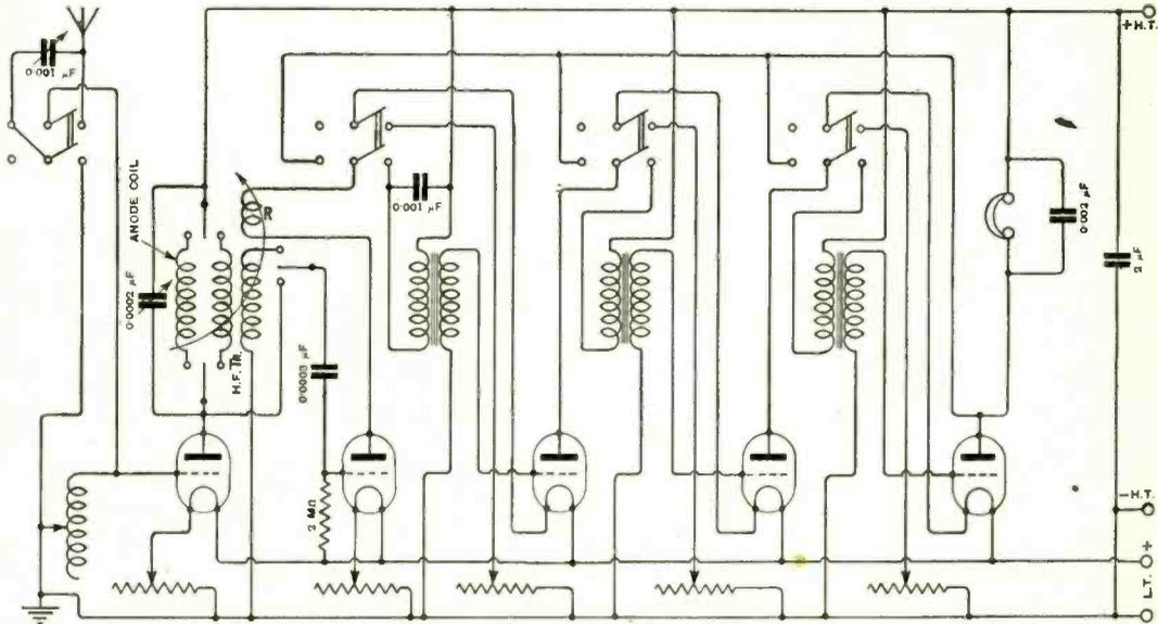
Fig. 4. **"A.G.B." (Essex).** This receiver has one stage of H.F. amplification, rectifier, and three stages of notes magnification (1-v-3). Switches are provided to vary the number of valves in circuit. The tuned anode or the transformer method of coupling the H.F. valve may be used.
