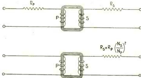
Fig. 83. The resistance of the primary winding may be designated by  $R_p$  and that of the secondary  $R_s$ . The equivalent resistance of the transformer referred to the secondary is equal to  $R_s + R_p \left(\frac{N_s}{N_p}\right)^2$
