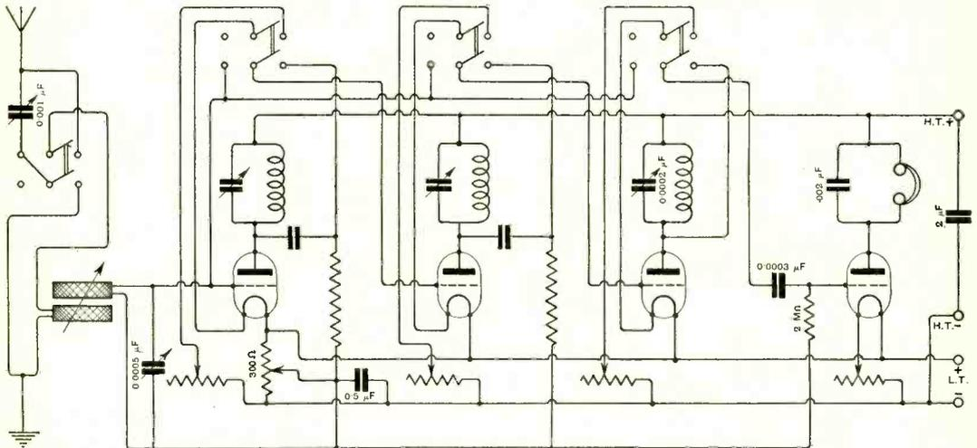
Fig. 3. "H.F." (Oldham). This diagram shows the method of connecting three stages of H.F. amplification with a valve rectifier.
