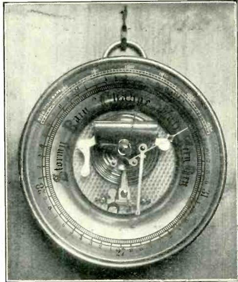
*An Aneroid barometer with the new scale fitted, by means of which it is possible to take readings direct in millibars.*
