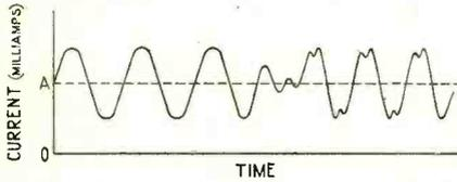
Fig. 2. Typical form of current fluctuations in the plate circuit of note magnifying valve.
