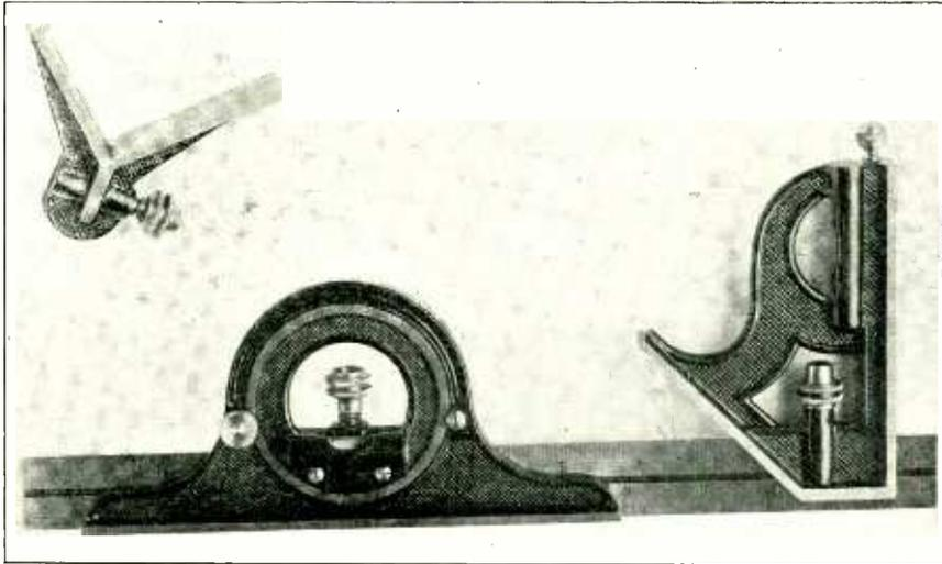
Fig. 2. A combination square and protractor.
