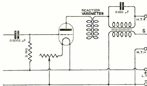
Fig. 2. "S.B.H." (Sidcup). Method of connecting variometer to secure reaction effects.
