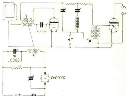
Fig. 4. In this circuit, damping is produced by a coupled circuit and interrupter.
