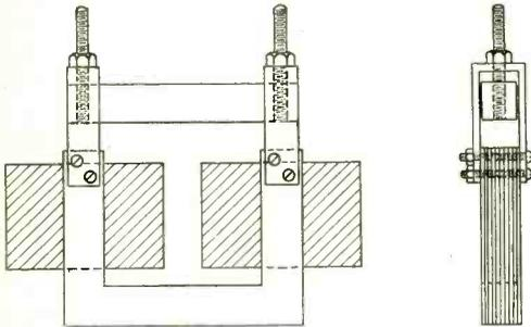
Fig. 77. A choke suitable for the experimenter. The inductance may be varied over a wide range by moving the top limb of the core which is mounted so that it may be moved between the brass end pieces.
