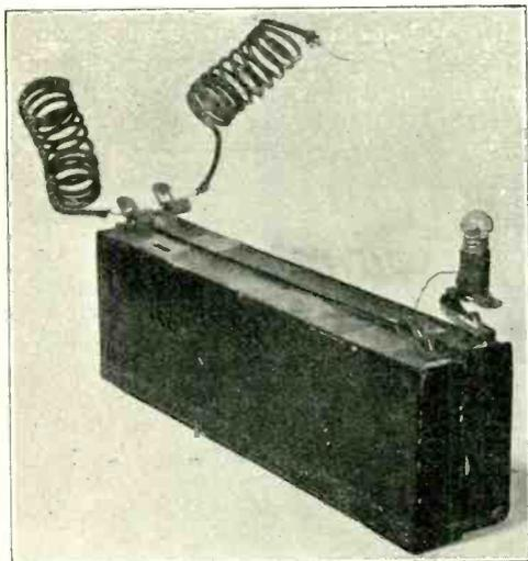
Fig. 17. The fitting of a small lamp in place of a connecting strap in the H.T. battery will protect it from damage by short circuit.
