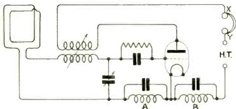
Fig. 1. Simple super-regenerative arrangement without filter circuit.
