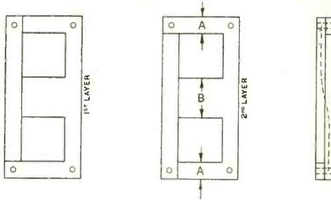
Fig. 89. A usual shape of laminations used in the construction of shell type transformers. The layers are arranged as indicated to reduce the reluctance of the core by reducing the effect of the joints.
