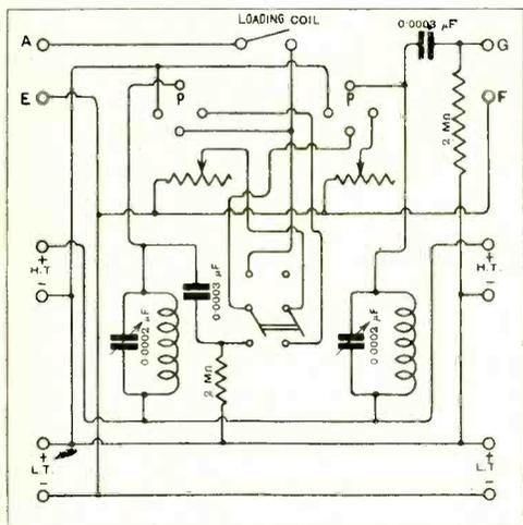
Fig. 1. "H.W." (Brixton). Diagram of a two-valve H.F. panel (2-0-0).
