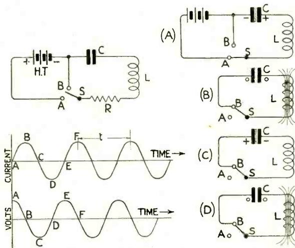
Fig. 68. Showing the various conditions in an oscillatory circuit during the generation of oscillations.
