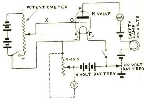
Fig. 18. Connections of apparatus for showing the effect of the potential of the grid on the current which flows in the H.T. battery circuit.
