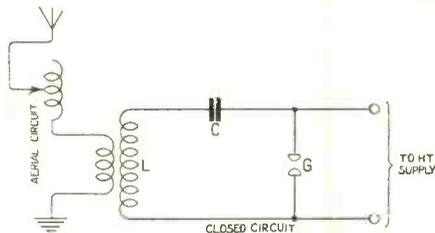
Fig. 71. Portion of a spark transmitter. The closed oscillatory circuit consists of L, C and G.
