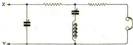
Fig. 2. Filter circuit for connection between telephones and telephone terminals.
