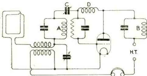
Fig. 3. An elaborated and particularly good super-regenerative circuit.
