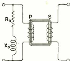
Fig. 85. The effect of the core losses may be represented as an impedance consisting of  $X_0$  and  $R_0$  connected across the ideal transformer.
