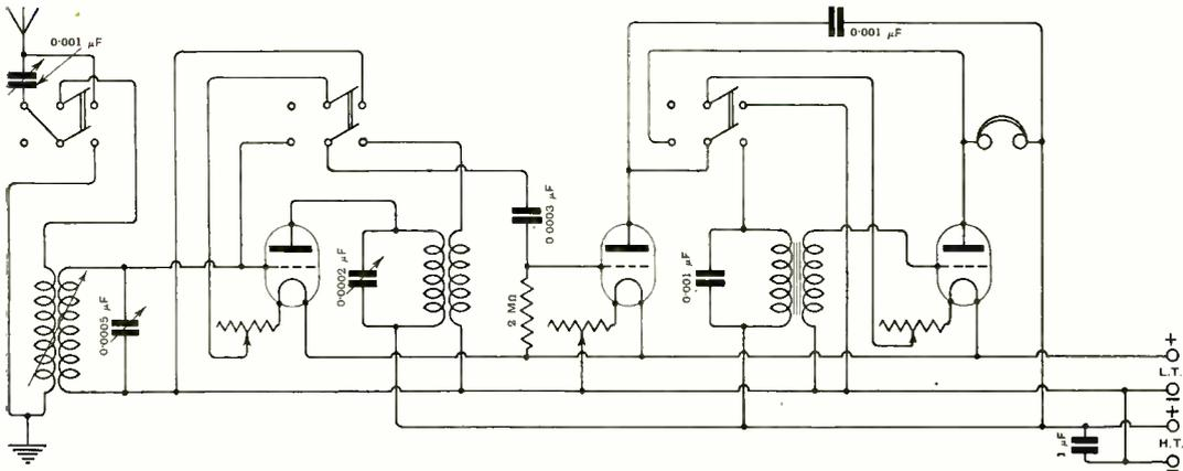
Fig. 1. "H.K." (Dorset). Receiver with H.F., valve rectifier and note magnifier with switches to switch the H.F. or L.F. valve circuits.
