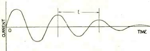
Fig. 69. The curve represents the current flow in an oscillatory circuit possessing resistance. The greater the resistance the quicker will oscillations cease. The time between any two successive crests or troughs, as at  $t$ , is called the periodic time.
