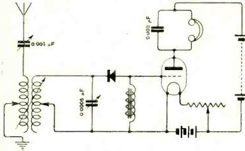
Fig. 4. "L.G.C." (Bucks). Crystal receiver with note magnifier.
