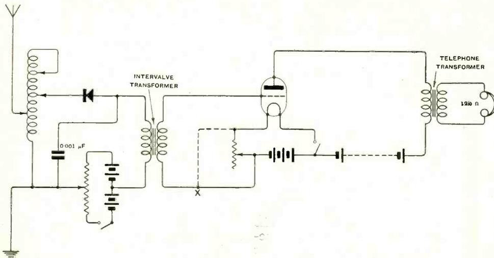
Fig. 20. Experimental circuit for demonstrating the action of a valve as a low frequency amplifier.
