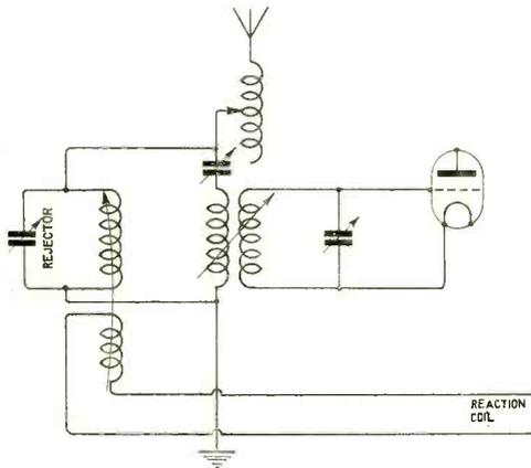
*A simple rejector circuit. The reaction coil may be coupled with the coil of the rejector circuit to compensate for resistance losses.*
