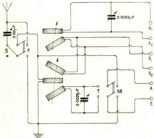
*Circuit diagram from which the principles can be readily seen.*
