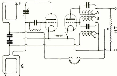
Fig. 6. An improved circuit embodying the super-regenerative principle.
