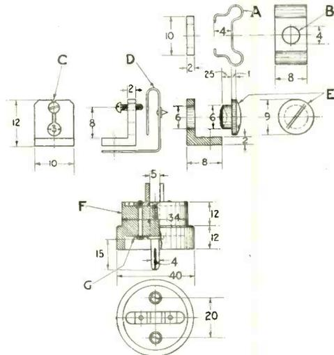
Fig. 2. Dimensional drawings of the component parts of a compact crystal detector.
