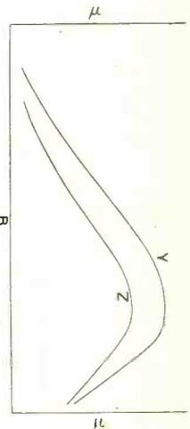
required until, as higher values of  $H$  are reached, only a small response is secured by an increase in  $H$ . At this point (say point  $C$ ) we have reached magnetic saturation, that is, the iron
