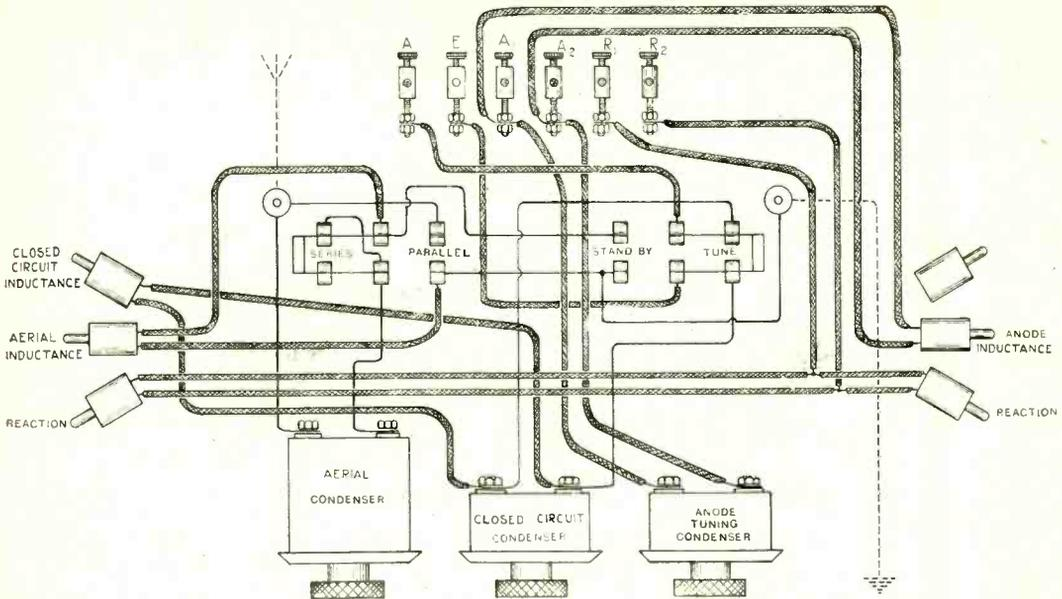
*Wiring Diagram. Wiring up is carried out with flexible wire between terminals and coil holders and No. 16 S.W.G. tinned copper wire between condensers and switches. Tests must be made to determine the correct direction for connecting up the leads to the reaction coil sockets.*
