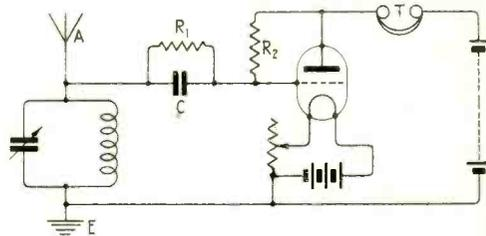
Fig. 2. A Single Valve Receiving Circuit, introducing an additional grid leak resistance.
