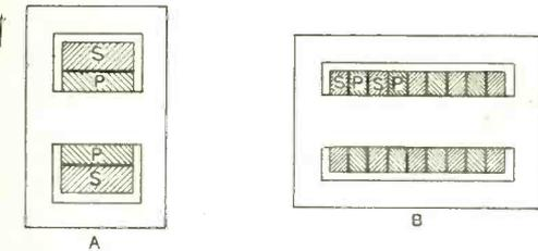
Fig. 86. To reduce magnetic leakage the windings should be split up and interleaved as in B. The transformers are of the shell type.
