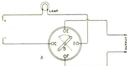
Fig. 1. Electrolytic Potentiometer.
