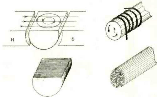
Fig. 75. A varying flux produces circulating currents in the core. The core is therefore split up or laminated so that there is considerable opposition to current flow. The arrows show the direction of the induced (eddy) currents, and the lower figures the method of reducing the magnitude of the currents by building the core of laminations or a bundle of iron wires.
