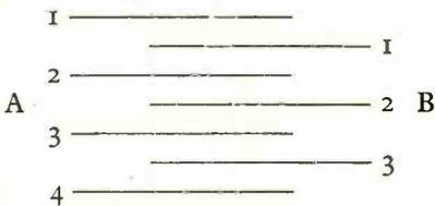
Here A<sub>1</sub>, B<sub>1</sub> form one condenser, B<sub>1</sub> and A<sub>2</sub>, A<sub>2</sub> and B<sub>2</sub>, B<sub>2</sub> and A<sub>3</sub>, and so on, and with the seven plates I have shown we get a condenser six times as large as with one pair. Similarly if we have 19 plates the capacity will be 18 times that of a single pair, and if there are n plates, the capacity will be n-1 times.
