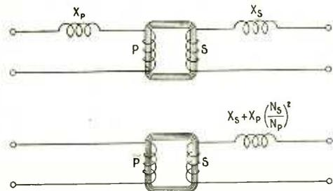
Fig. 84. On account of magnetic leakage the transformer may be represented as an ideal transformer with a choke  $X_p$  and  $X_s$  joined in the primary and secondary. The equivalent reactance of the transformer referred to the secondary is equal to
