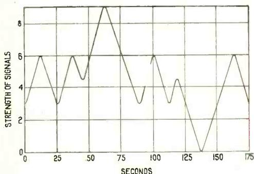
Fig. 4. "Double fade" and "Double increase" of signal strength at 1,000 miles.
