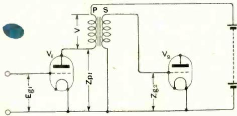
Fig. 94. Valves transformer coupled.  $E_{g1}$  = grid applied volts.  $Z_{p1}$  = average anode impedance.  $V$  = volts across primary winding P.  $Z_{g2}$  = impedance of grid circuit of valve  $V_2$ .
