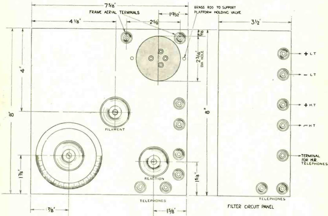
Scale drawing of tuner and filter panels.
