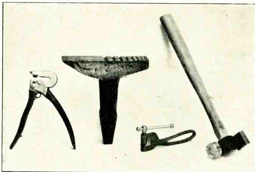
(1) Punch. (2) Bick iron. (3) Screw punch. (4) Square-faced hammer.
