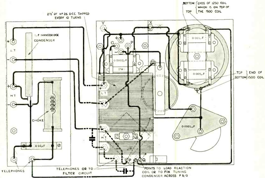
Wiring diagram of filter and tuner panels.
