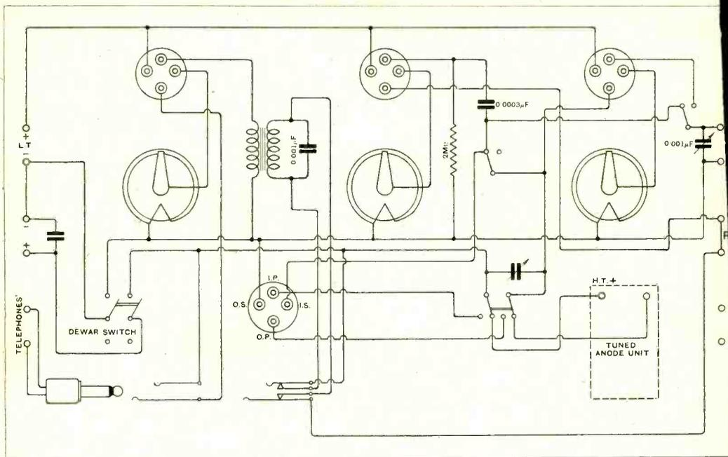
Fig. 6. "P.R.K." (Philadelphia). Wiring diagram of three-valve receiver (1-V-1.)
