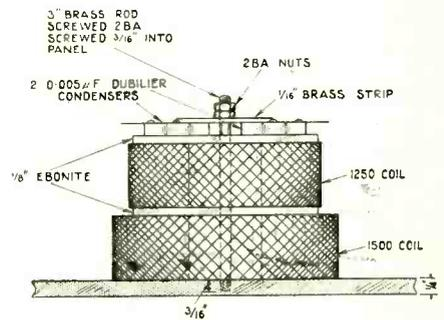
certain foundation on which to build new gadgets. It will be seen from the theoretical diagram that provision is made at the terminals X Y for additional tuning capacity, if needed, to raise the wavelength.
