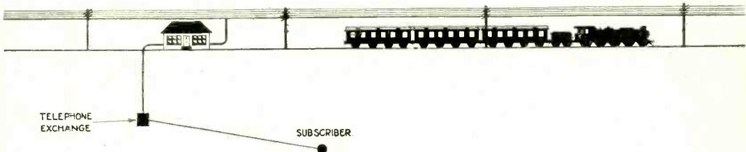
Fig. 1. Schematic diagram showing how communication is established between a subscriber on the public telephone system and the moving train.
