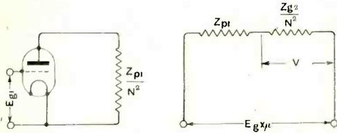
Fig. 95. Equivalent circuit of Fig. 94 when ideal transformer is used.
