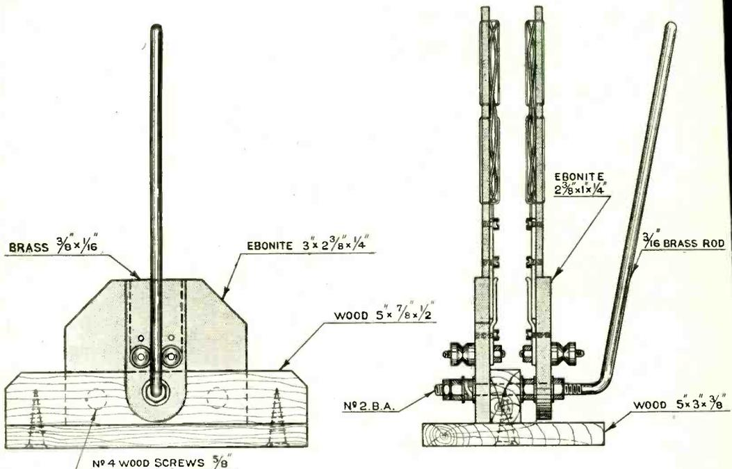
Scale drawing of simple yet effective coil holder.
