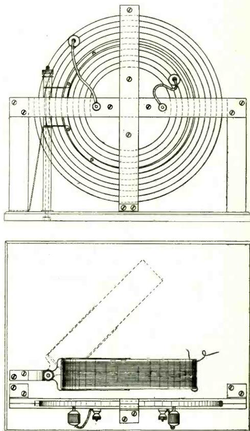
Fig. 4. Suitable for a larger power transmitter as described. The helix consists of 10 turns spaced  $\frac{1}{4}$ " apart, outside diameter about 9". Connection for aerial and anode tap is made with clips. The grid coupling coil is the small cylindrical coil, 5" in diameter wound with 20 to 30 turns of No. 22 D.C.C. suitably mounted.
