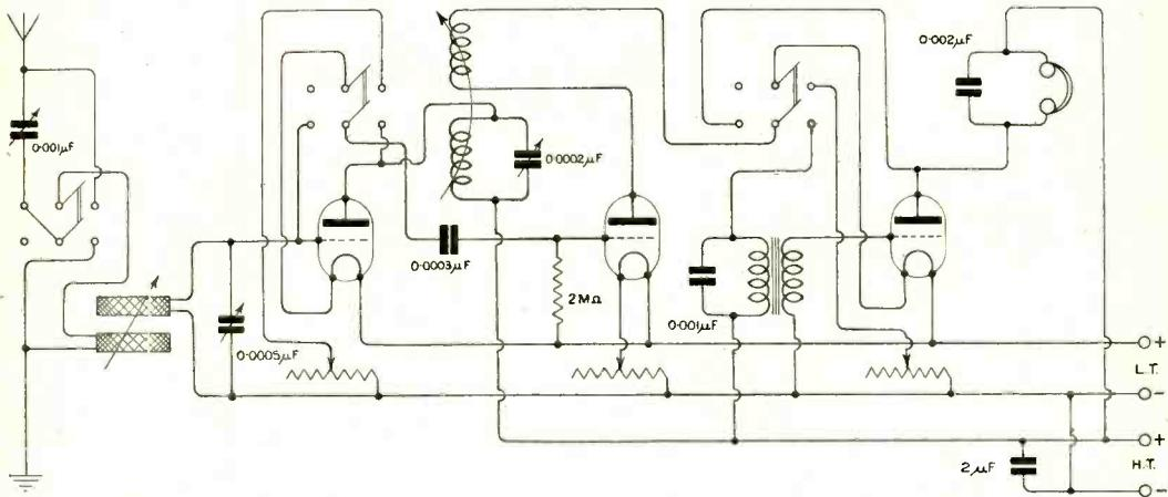
Fig. 3. **"E.J." (Brondesbury N.W.6.)** A three-valve receiver employing one H.F., detector, and one L.F. valves. The H.F. and L.F. valves may be switched out of circuit by means of double pole change-over switches.
