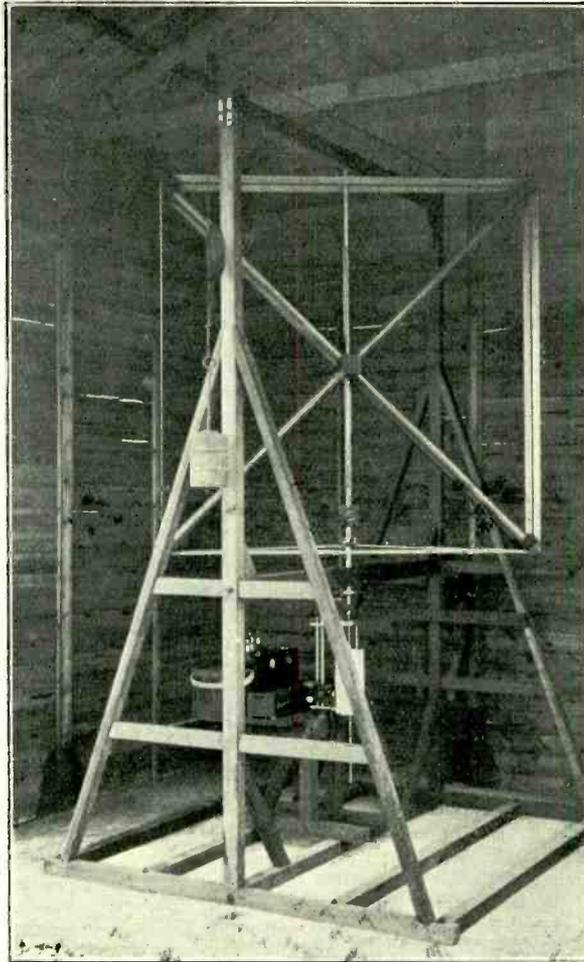
Fig. 5. Directional frame and apparatus used in recording atmospherics.
