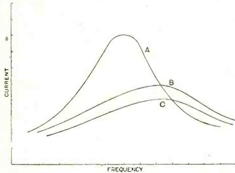
Fig. 109. Curve A represents the resonance curve for circuit (1) above. When circuit (2) is coupled, the resonance curve is as shown by curve B. If the resistance of circuit (2) is increased, or if the coupling is increased, the curve will be as represented by C.
