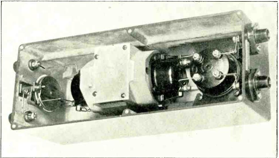
This instrument, manufactured by the M. L. Magneto Syndicate, Ltd., is for the purpose of providing valve H.T. current from a low voltage source, such as the accumulator battery used for filament heating. The outfit consists of variable resistance, motor generator and smoothing inductances and condensers. It is constructed in three
