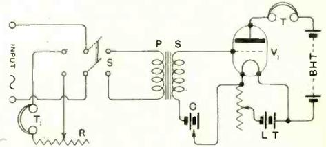
Fig. 104. Method of measuring the effective impedance of primary of transformer.  $R$  = variable known resistance up to about 100,000 ohms.  $T$  and  $T_1$  = telephones.  $S$  = throw-over switch.  $P$  and  $S$  = transformer.  $C$  = grid battery. The voltage of known frequency is applied to the terminals marked input.
