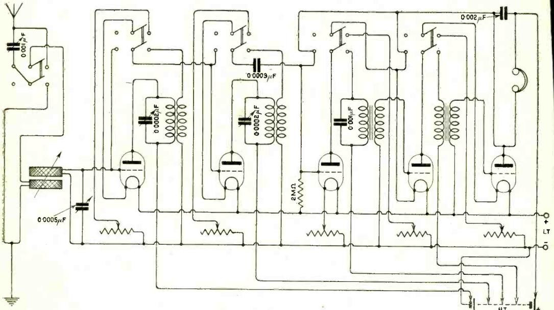
Fig. 2 "E.C.G." (Luton). Receiver with 2-v-2. A separate anode voltage may be provided to each circuit.
