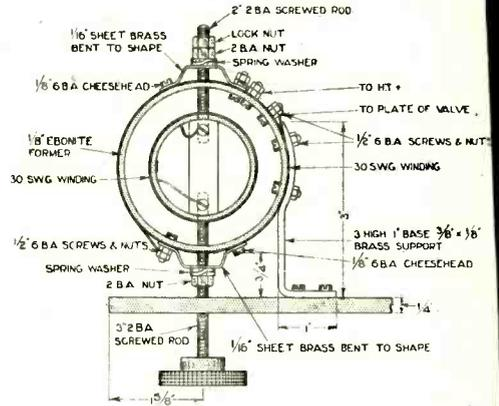
Constructional details of the reaction coupling.
