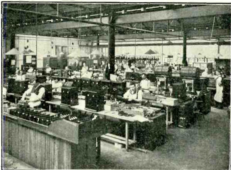
One of the assembly shops at the works of Marconi's Wireless Telegraph Co., Ltd., at Chelmsford. The component parts of transmitting, receiving and "Marconiphone" equipments are shown being brought together.
