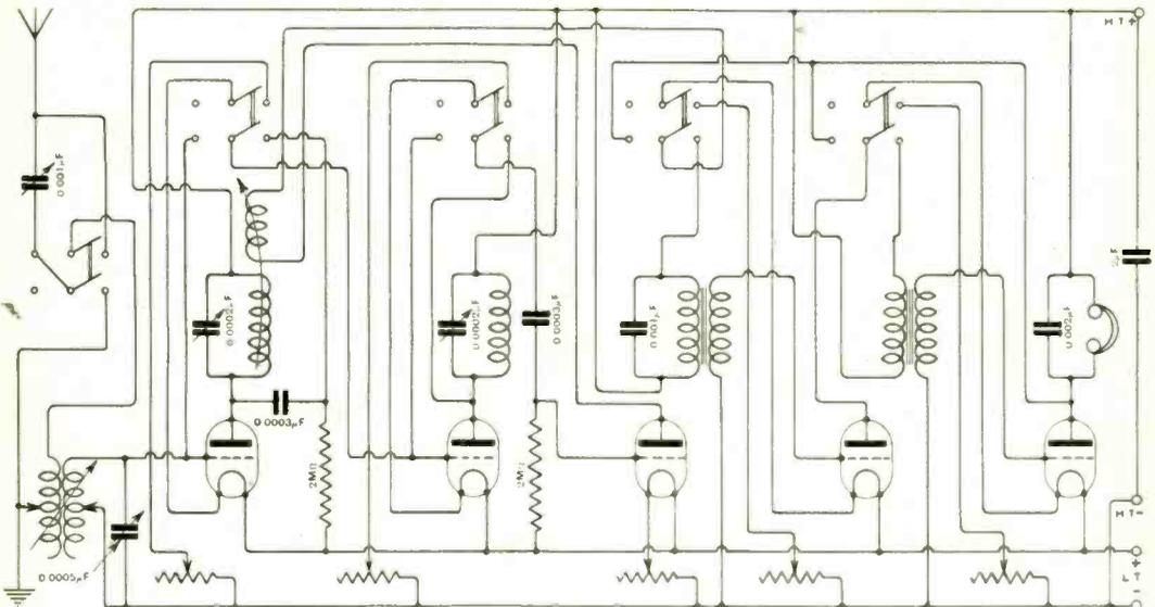
Fig. 4. "C.V." (Devon). Diagram of a receiver with two stages of tuned anode H.F. amplification, rectifier and two note magnifiers (2-V-2). The reaction coil is coupled with the first anode coil.
