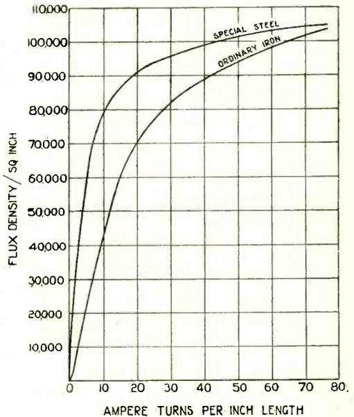
Fig. 93. The upper curves show the watts lost per pound of transformer steel at various flux densities. The lower curves show the ampere turns per inch length of the magnetic circuit required to produce various flux densities.
