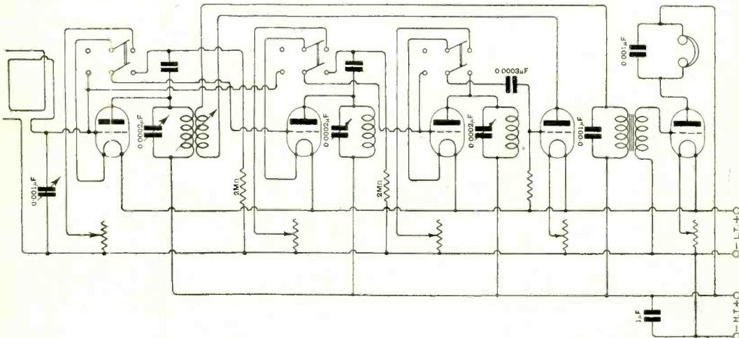
Fig. 1. "A.A.B." (London, N.W.8). A five-valve receiver for use with a frame aerial. Three H.F., detector, and one L.F. valves are employed, with switches for varying the number of valves in circuit.
