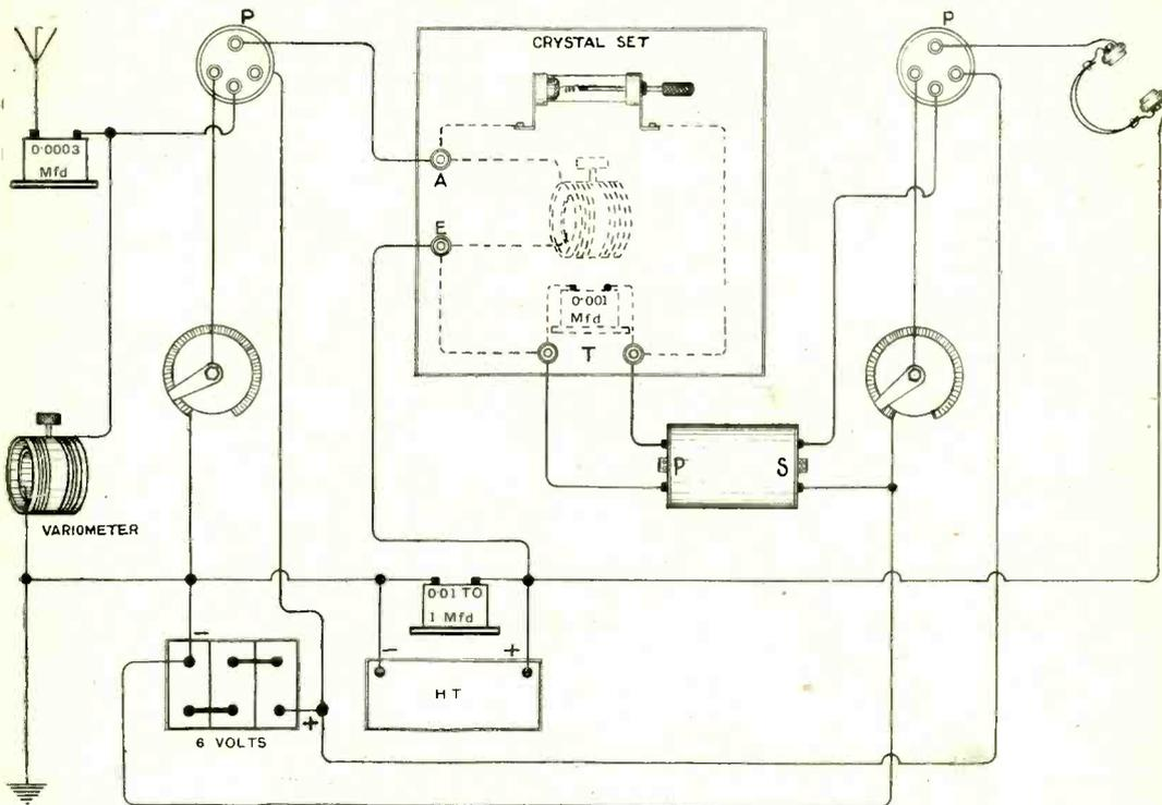
The principle of the circuit employed can be followed from this diagram. The aerial tuning inductor of the crystal receiver is used as the tuned anode coil. If it is not desired to go to the trouble of incorporating the components into a complete instrument they may be set out as shown and secured to a base board.
