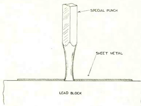
Fig. 3. Method of punching holes in thin sheet metal.
