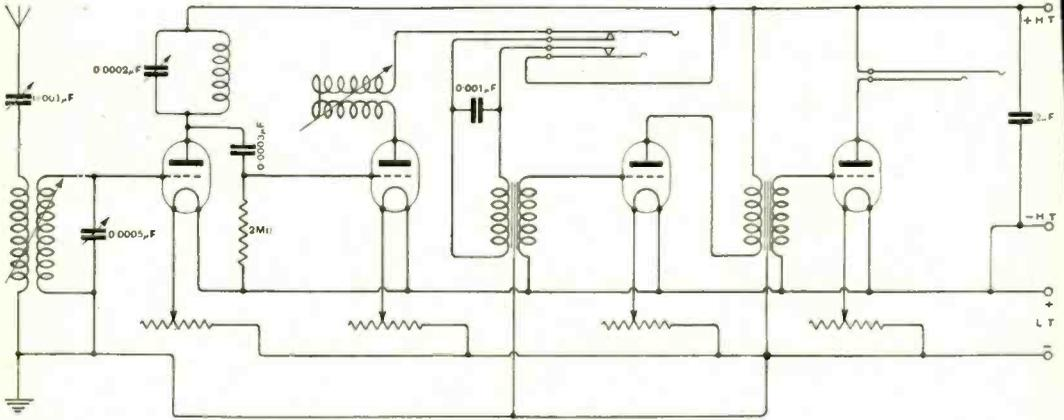
Fig. 3. "YANK" (Doncaster). Receiver with H.F., rectifier and optional note magnifiers (1-V-2). The telephones are connected to a plug. The purpose of the variometer in the anode circuit of the rectifier is to provide reaction effects.
