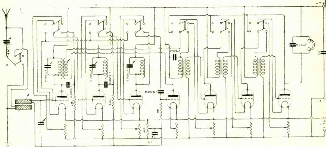
Fig. 2. “S.B.” (Norway). Diagram of receiver with three stages of H.F., rectifier, and three note magnifiers.
