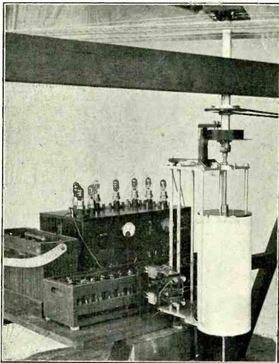
Fig. 6. Showing details of the directional recording apparatus.
