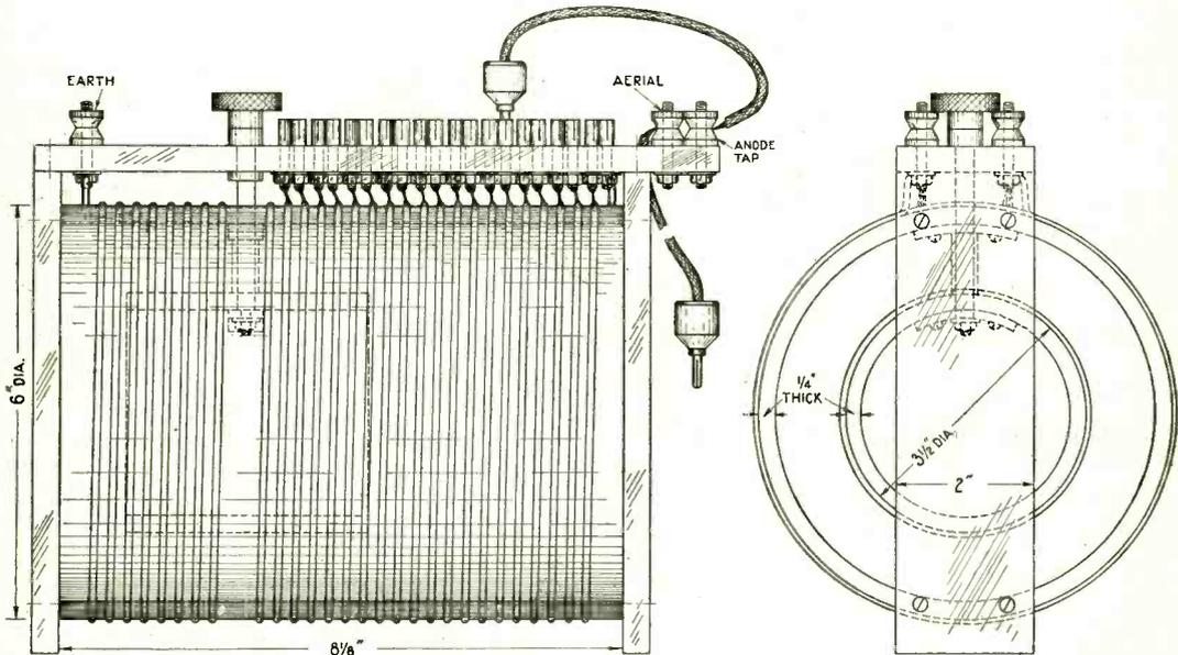
Fig. 5. Here the aerial coil is wound with bare No. 14 wire with the turns spaced. Tappings are taken to sockets, and connections for the aerial and anode tap are made with plugs. The grid coil rotates inside the large coil. The dimensions are given.
