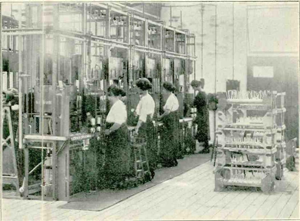
*The valve pumping plant. Each operator deals with a batch of about 20 valves. The filaments are run at a high temperature and a high voltage is applied to the anodes. The filament current of each valve is adjustable by the operator, and during the pump ing the current is varied according to the degree of vacuum.*
