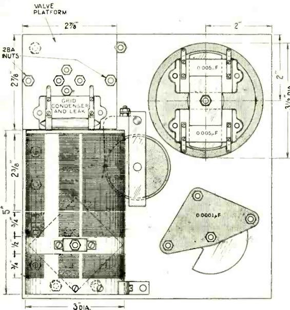
Underside of panel and the method of mounting the oscillator inductances.
