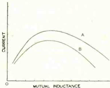
Fig. 111. The secondary current varies with the mutual inductance in the manner shown. There is one best value of coupling which gives the maximum secondary current. If the secondary resistance is increased, the relationship between secondary current and the coupling is as shown by curve B.
