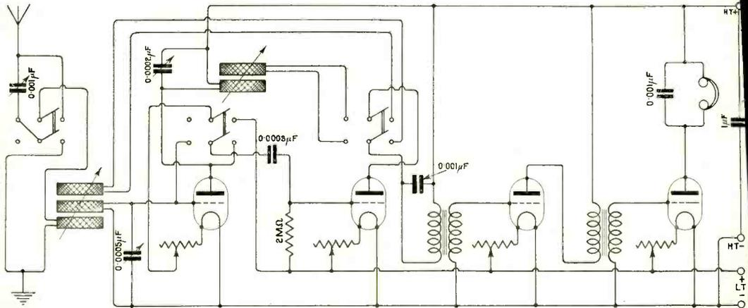
Fig. 3. "F.J.F." (West Bromwich). Connections of a four-valve receiver employing one H.F., detector and two L.F. valves. Switches are provided for disconnecting the H.F. valve, and for employing reaction on either the closed circuit or anode coils.
