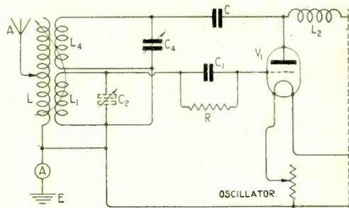
Fig. 2. Coupled or Meissner circuit. Valves as in Fig. 1, also  $L_4 = 25$  to  $30$  turns of No. 22 D.C.C. on former  $5''$  diameter,  $C_4 =$  variable condenser  $0.0002 \mu F$ .
