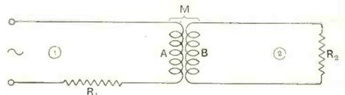
Fig. 108. Coupled circuits with resistances  $R_1$  and  $R_2$  in each circuit. The effect of the resistance of circuit (2) is to increase the apparent resistance of circuit (1) and vice versa.
