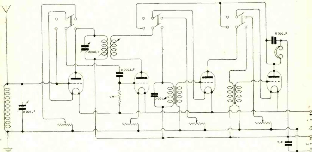
Fig. 1. "C.H.S." (Derby). Diagram of 4-valve receiver with one H.F., tuned anode coupled, rectifier and two note magnifiers (1-V-2). Switches are provided so that any valve except the rectifier may be cut out of circuit.
