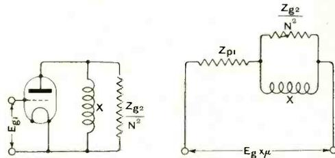
Fig. 96. Equivalent of Fig. 94 when transformer takes magnetising current (no load current).
