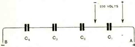
Fig. 1. Condensers in series and arranged to be charged separately.
