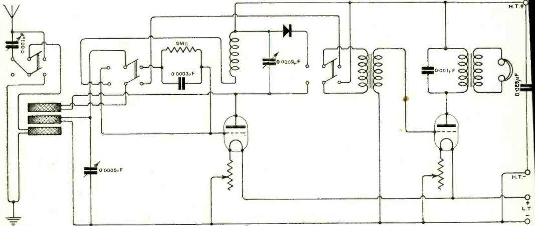
Fig. 6. "J.E." (Arbroath). Experimental receiver employing two valves and a crystal rectifier. Switches are provided so that valve or crystal rectification may be used. When the latter method is employed, both valves may operate as low frequency amplifiers.
