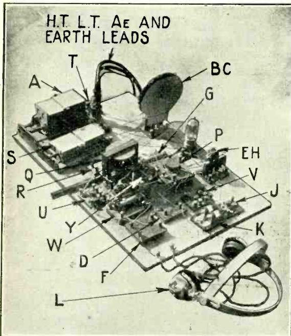
Fig. 8. Complete dual and crystal receiver.
