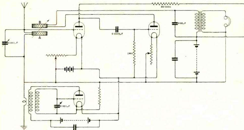
Fig. 26. Long-wave receiving circuit with separate heterodyne wavemeter.
