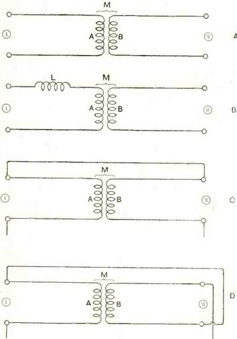
Fig. 107. To obtain the mutual inductance, measure the inductance with the coils in series as at (C), and then with the connections as at D. If the inductances
