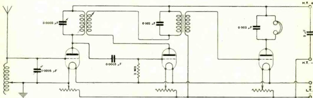
Fig. 1. **"A.C.H." (Tonbridge.)** Three valve receiver with one H.F., detector, and one L.F. valves. Tuned anode H.F. coupling is employed, with reaction to the anode coil.
