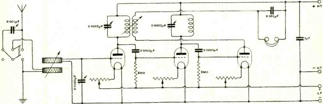
Fig. 1. "R.L.S." (Geneva). A three-valve receiver is shown, employing two H.F. amplifying valves and detector. Tuned anode H.F. coupling is used, with reaction to the anode coil of the first valve.
