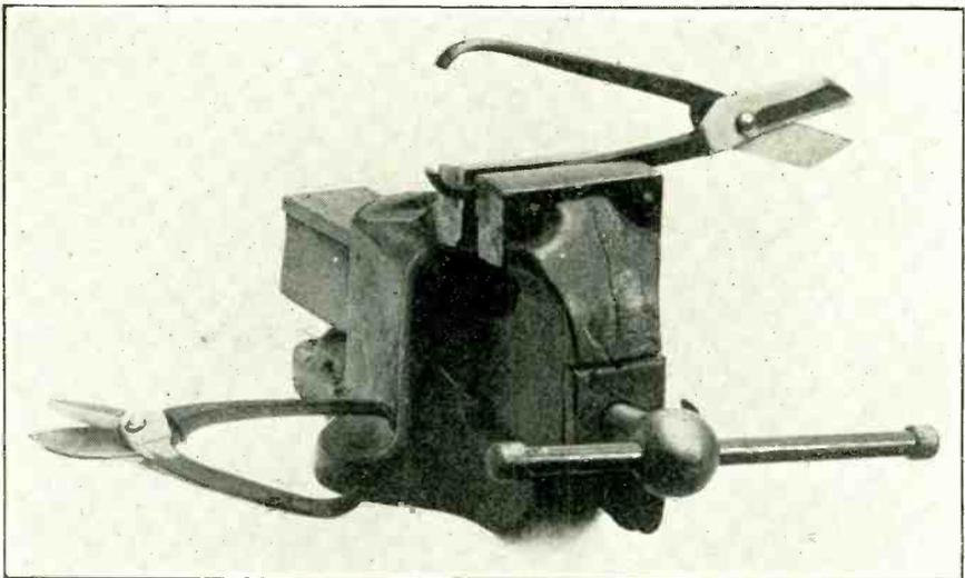
*Fig. 1. Tinman's snips mounted in the vice for accurately cutting sheet metal.*
