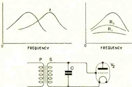
Fig. 97. The effect of transformer capacity is to give it a resonant frequency which may be shown by plotting frequency and amplitude of signal. The curve is moved to the left from say position 2 to position 1 by adding a capacity  $C$  across the windings. The effect of adding a resistance across the windings is shown. A high resistance produces a reduction in amplitude and a broader peak as at  $R_2$ . A lower resistance produces a flatter curve altogether, represented by  $R_1$ .
