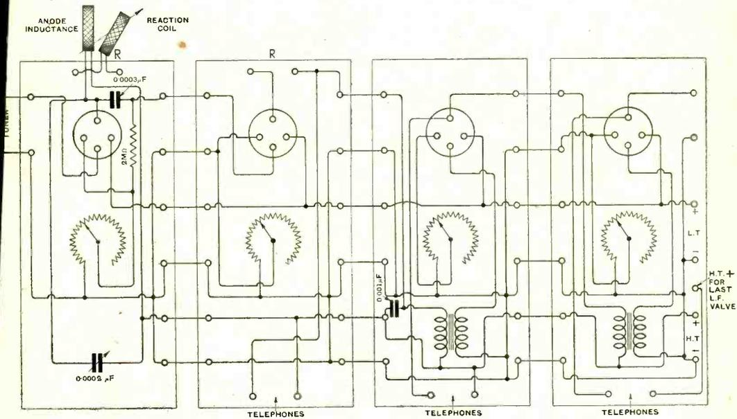
Fig. 5. “G.C.” (Burton-on-Trent). A four-valve receiver arranged on the unit system. One H.F., detector and two L.F. valves are used. The tuned anode method of H.F. coupling is employed.
