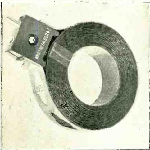
Fig. 5. A completed plug-in type of coil.
