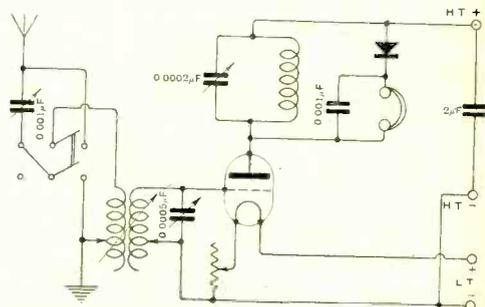
Fig. 4. "J.M." (Manchester) A receiver with one H.F. valve, and employing crystal rectification.
