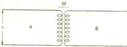
Fig. 105. Two circuits magnetically coupled.
