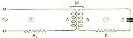
Fig. 110. Coupled circuit with condenser C in the secondary circuit (2).
