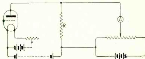
Fig. 2. Method of determining current change in the anode circuit.
