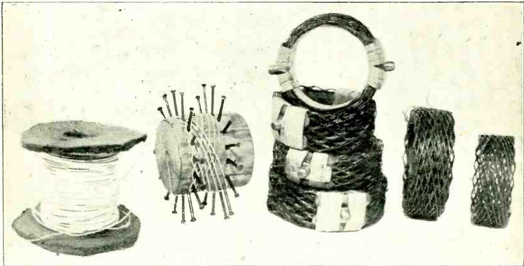
*Honeycomb coils wound on the principle described in this article.*
