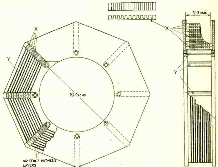
Fig. 149. The coil designed by Prof. Morecroft, called a Morecroft coil. The cheeks of the former are of wood, held apart with wooden pins Y. The turns and layers are spaced through the use of the separators X, shown larger in the upper drawing. This was probably the first coil of its kind.
