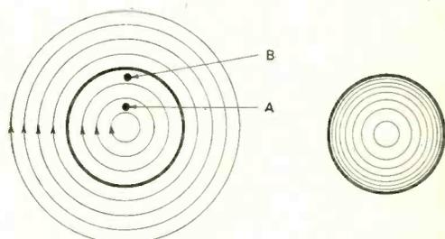
Fig. 120. The heavy circle represents the surface of a conductor. When current flows, an element situated at A is linked with more lines of force than another at B. Consequently the back pressure developed is not equal over the cross-section. The current distribution is similar to the arrangement of the circles in the small figure, the current density near the surface being greatest.
