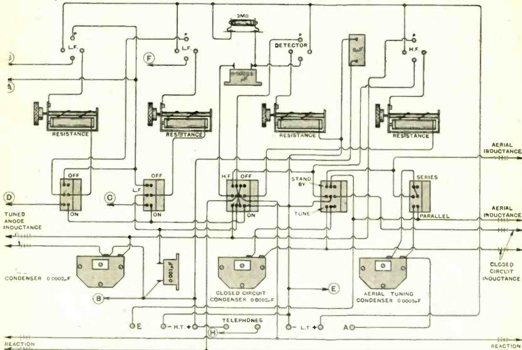
Practical wiring diagram. Leads can be marked off as they are fitted. Flexibles are indicated by cross lines.
