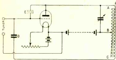
Fig. 1. Showing the principle of capacity neutralisation, using a coil BC and condenser D.
