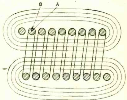
Fig. 121. When the wire is wound in the form of a coil, the current distribution is again changed. The current density is greatest in the portion of the wire on the inside of the coil.
