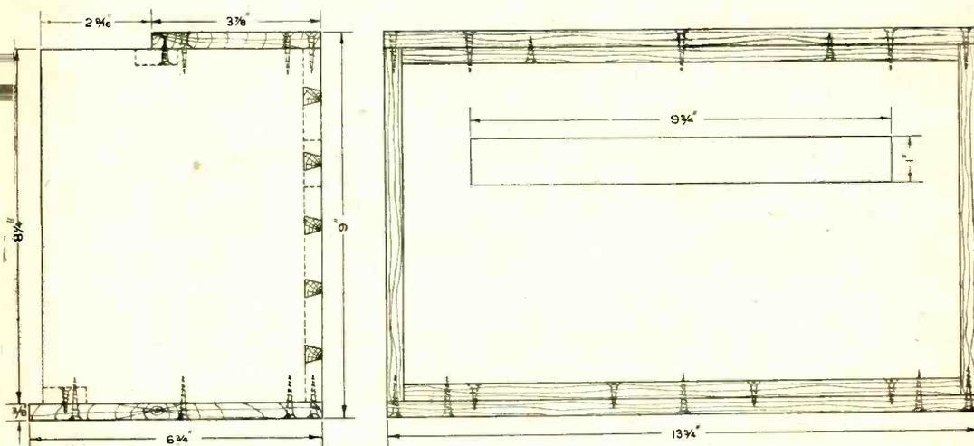
*Dimensional drawing of the box work. The location of the slot for the terminal strip must be carefully set out.*
