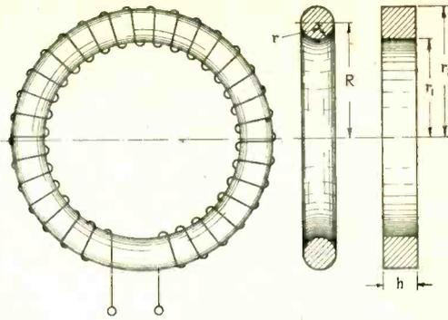
Fig. 134. Data of circular coils required in inductance calculations.
