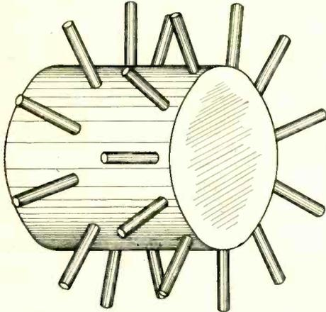
Fig. 147. The former used in the construction of home-made coils, such as Figs. 144 and 145.
