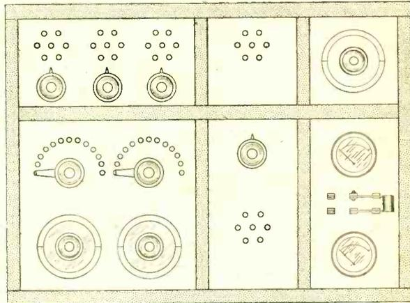
Front of equipped Apparatus Frame.
