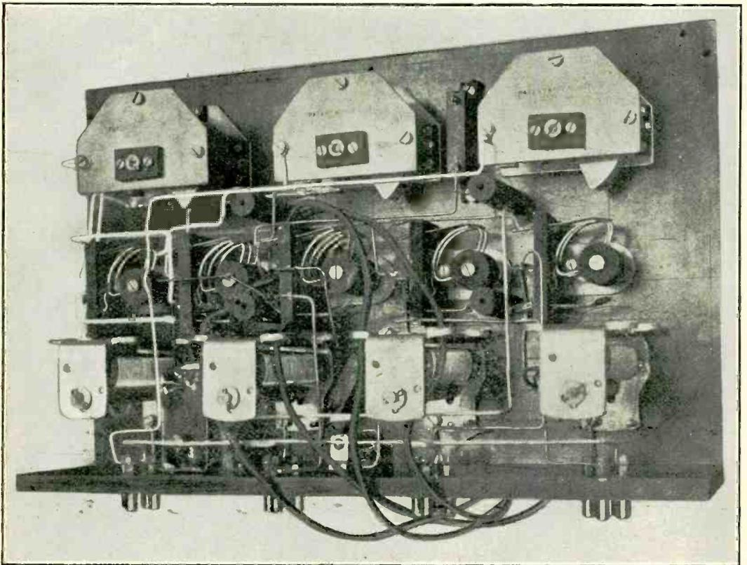
Back view of panel with components assembled and wired prior to placing the transformer platform in position.
