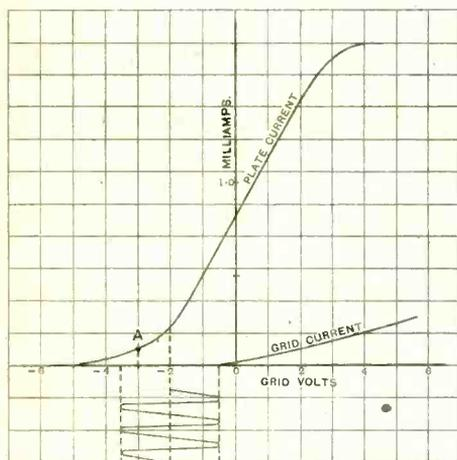
Fig. 1. Typical characteristic curve of a receiving valve showing plate and grid current values for various grid potentials.
