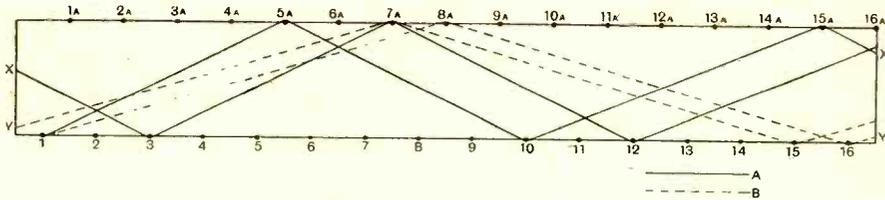
Method of winding the coils.
