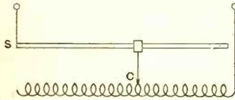
Fig. 127. A variation of inductance may be obtained by providing a rod S, along which may be moved the slider which makes contact at C with the turns.
