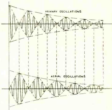
Fig. 113. The upper curve shows the amplitude of the oscillation in the primary circuit, and the lower curve those in the secondary or aerial circuit. Notice the amplitude of the primary oscillations is a minimum, when that of the secondary is a maximum. The oscillations are not symmetrical as shown by the dotted outline. The amplitude of the maximum values decrease as indicated by the dotted lines.
