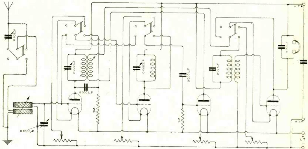
Fig. 3. "S.B." (Midhurst). This is the diagram of a receiver with two H.F., rectifier and a note magnifier with switches to vary the valves in circuit.
