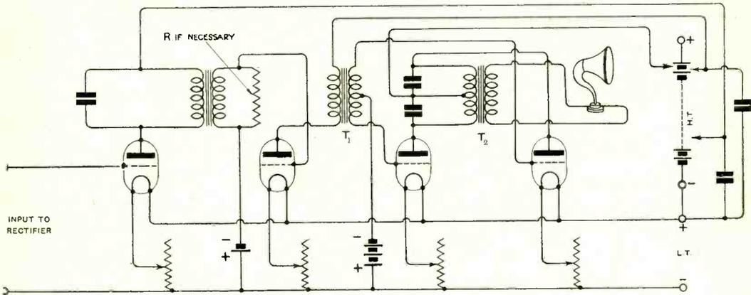
Fig. 4. Connections of the push-bell amplifier.
