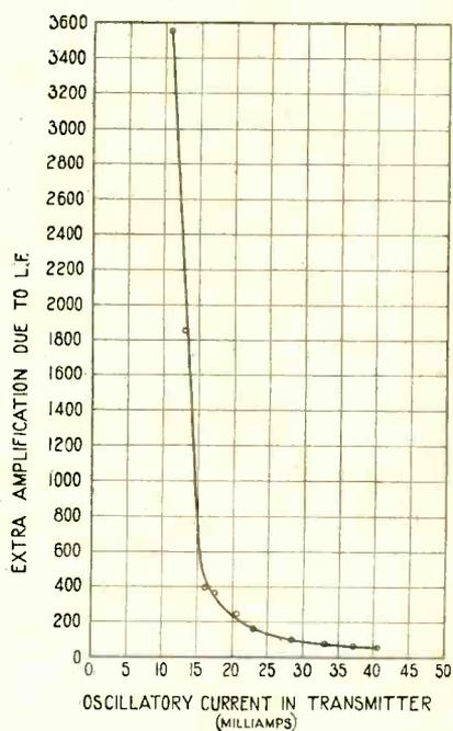
Fig. 4. Graph indicating the relationship between the signal strength and the amplification obtained.
