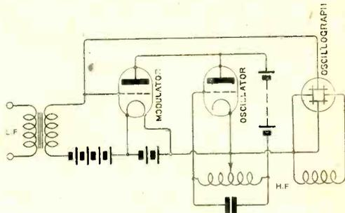
Fig. 2. Method of connecting the oscillograph for measuring the modulation of high frequency currents.
