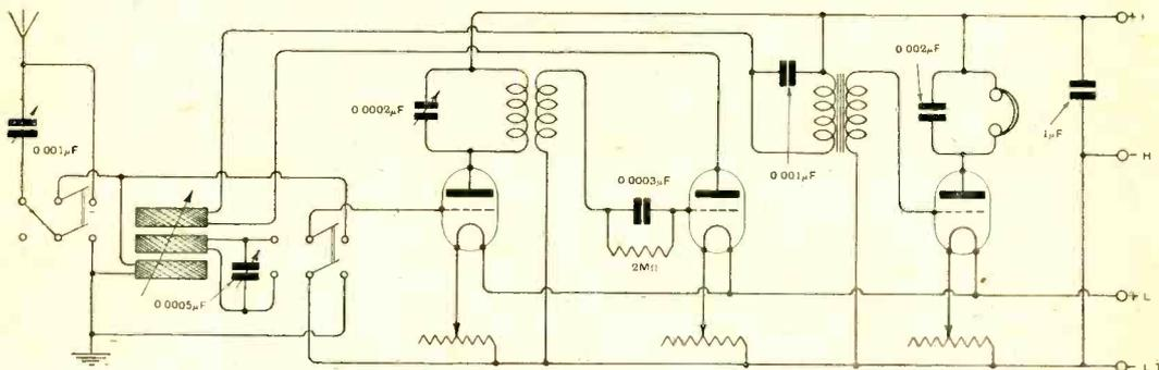
Fig. 5. "A.V.D." (New Barnet). Receiver with one H.F., rectifier and one L.F. The switch is used to connect either the aerial or closed circuits to the first valve.
