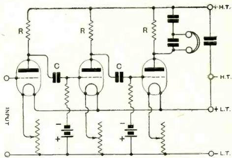
Fig. 5. Resistance amplifier. The telephones only carry the varying current; the steady anode current is carried by the resistance  $R$ . Suitable values are  $R = 70,000 - 100,000$  ohms, coupling condensers  $C = 0.005 \mu F$  to  $0.05 \mu F$ . Grid leaks  $0.5 - 2 M.\Omega$ .
