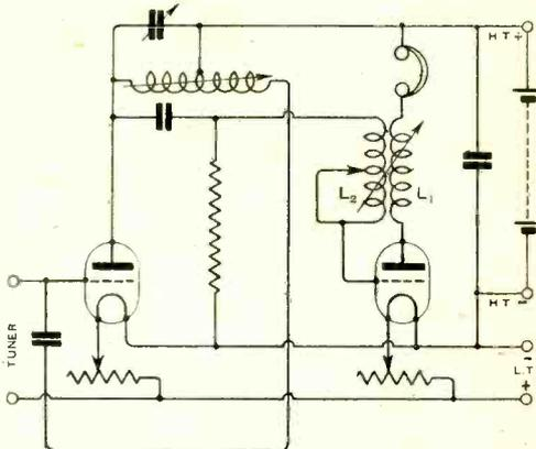
Fig. 3. Reaction effects may be obtained between coils  $L_1$  and  $L_2$  without changing the tuning of the amplifier circuits.
