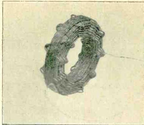
Fig. 145. An amateur-made coil wound like Fig. 144, on a former such as Fig. 147.
