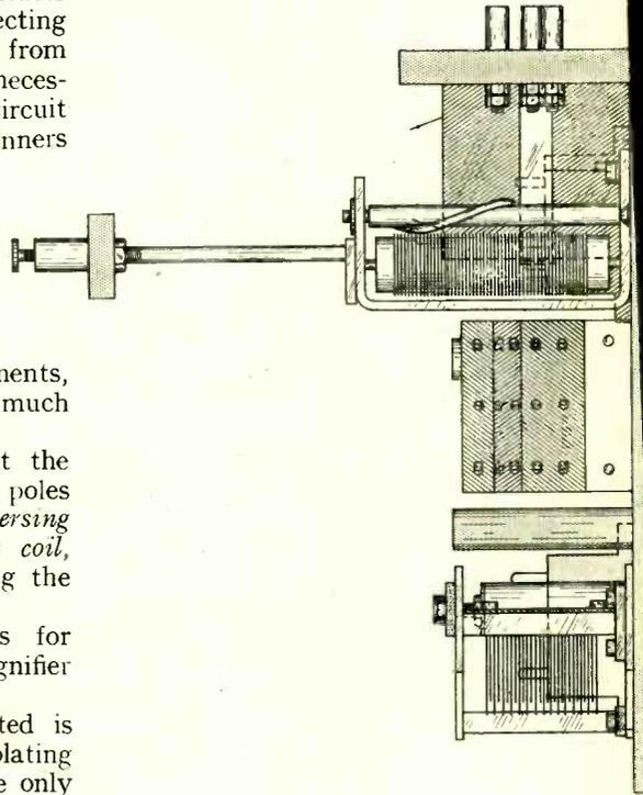
Side view showing only the apparatus on the back of the panel. The terminal strip is supported by two 3/16" brass rods attached in this instance to the end of filament resistances.
