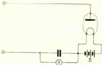
Fig. 3. Showing how the peak value of the voltage is determined.
