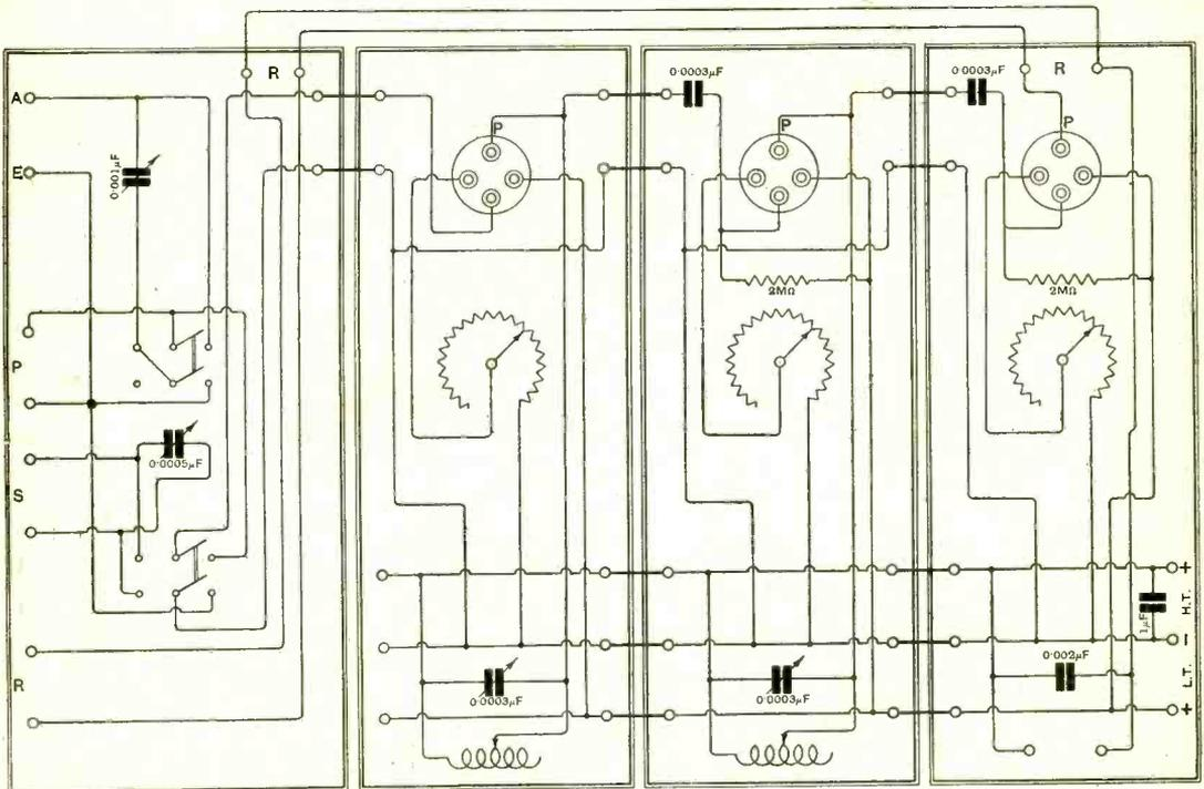
Fig. 1. "F.P." (Shoreham). Tuner, 2 H.F. and rectifier units. If one is not required it may be removed and the remainder connected.
