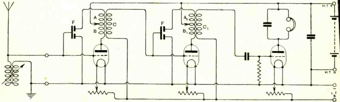
Fig. 4. A receiver with provision for neutralising capacity coupling. The transformers may be tuned with condensers in the usual manner, or a special transformer wound like a variometer may be used. If the tuned anode method of amplification is preferred, in place of the secondary windings C and  $C_1$ , connect grid condensers and leaks in the usual way.
