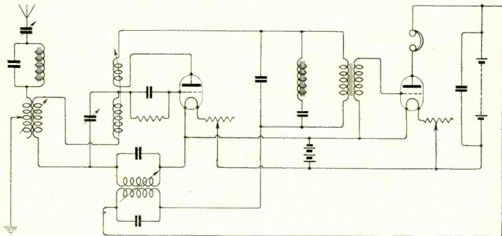
Fig. 6. A suggested circuit diagram for a two-valve receiver embodying the Armstrong principle.
