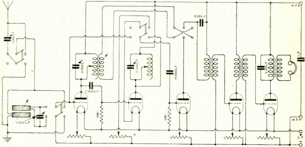
Fig. 2. "S.B." (Midhurst). Receiver with two H.F., rectifier and two note magnifiers. The reaction coil is coupled with the first anode circuit, and a reversing switch is fitted.
