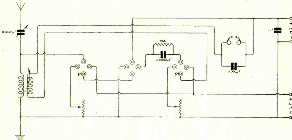
Fig. 3. "P.G.S.J." (Ryde, I.W.). A two-valve receiver with H.F. and rectifier. The valves are transformer coupled.
