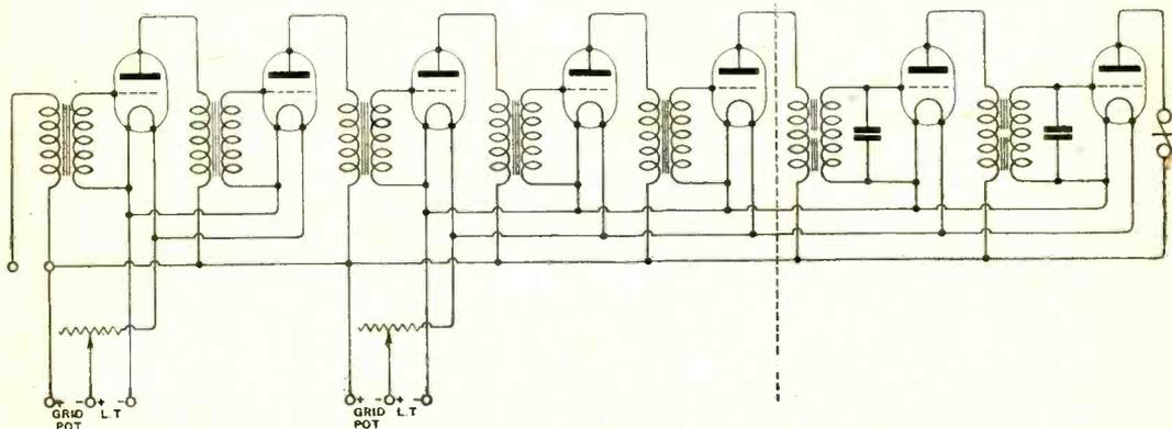
Fig. 2. A diagram of the circuit employed in the new interference eliminating device.
