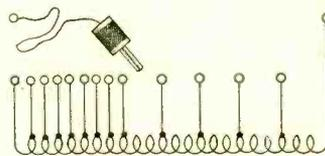
Fig. 128. A coil may be provided with taps, so that only part of the coil is in circuit.
