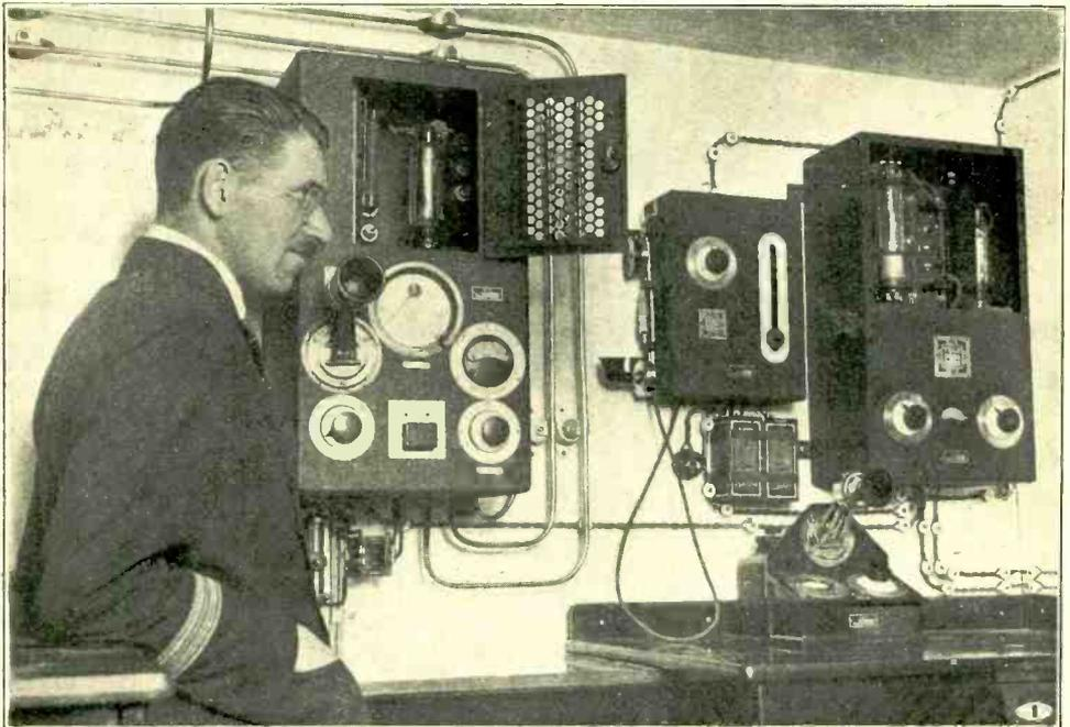
*A typical Telefunken telephony transmitter. The instrument shown has been installed on board the new German liner "Albert Ballin," and will be employed in ship to shore work off the American coast. The compact arrangement of the apparatus and the simplicity of the design will be specially noted.*
