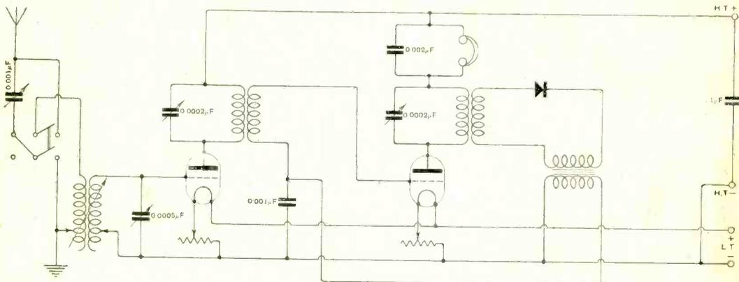
Fig. 6. "Dual" (Kingsland, N.I.). A double magnification receiver with two stages of H.F., rectifier and one note magnifier.
