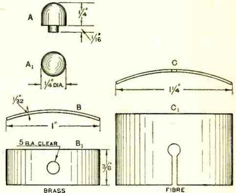
Construction of the coil contact pins.
