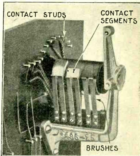
Fig. 132. Photograph of dead end and tapping switch. The connections are given in Fig. 130.
