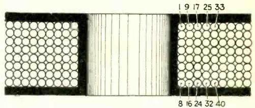
Fig. 143. A multilayer coil with lower capacity than one wound like that of Fig. 136. Notice the difference in the windings. When the coils are thin they are called "slab" coils.
