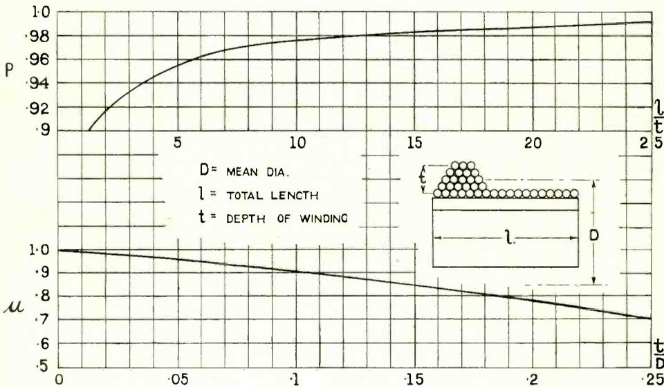
Fig. 140. Curves giving the value of the factors  $p$  and  $\mu$  which have to be taken into account when finding the inductance of a bank-wound coil.
