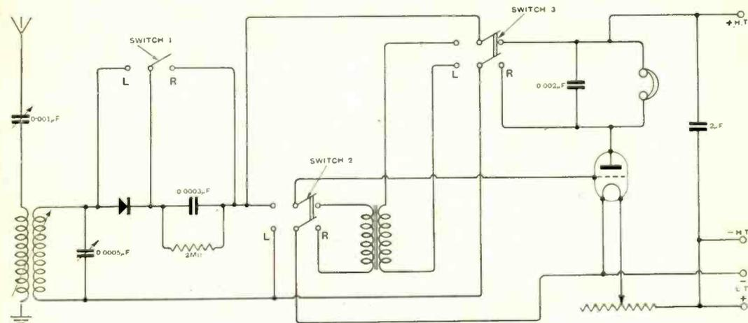
Fig. 4. "D.C.S." (Birmingham). Crystal and valve receiver with switches to use combinations of valve and crystal.
