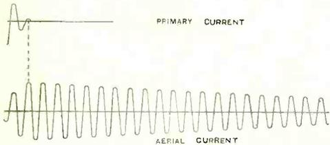
Fig. 116. If the primary circuit is broken at the end of the first few oscillations (i.e., when the current has reached its first maximum value), the secondary circuit will oscillate at its own natural frequency, the current only gradually falling in amplitude because of the small damping. At the beginning of the oscillations in the secondary circuit, while the oscillations are building up, two currents, with two frequencies are produced as before.
