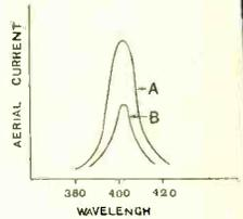
Fig. 119. When the coupling is loosened or made weaker, the energy in the secondary circuit approaches that represented by curve A. Tuning in this case is fairly sharp, the energy oscillating in a narrow band of frequencies with the resonance point well defined. If the coupling is made still weaker, the resonance curve is sharper but there is a loss of energy, represented by curve B.
