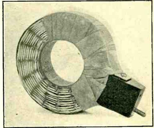
Fig. 148. The layers of this coil are spaced with string. The turns in the layers are not spaced.
