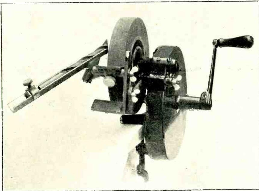
Fig. 3. A hand-operated grinder, with special attachment for correctly sharpening twist drills.
