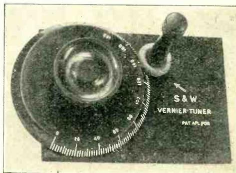
The device for critical adjustment of variable condensers.
