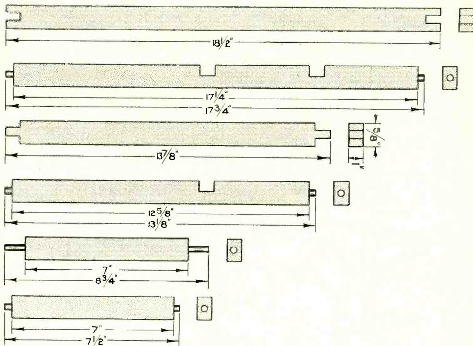
*Constructional details of wooden rods.*
