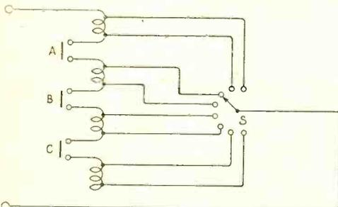
Fig. 130. The switch S is provided to tap out the turns, and the coil is split up into sections to reduce dead end effects by the isolating switch with contacts A, B and C.
