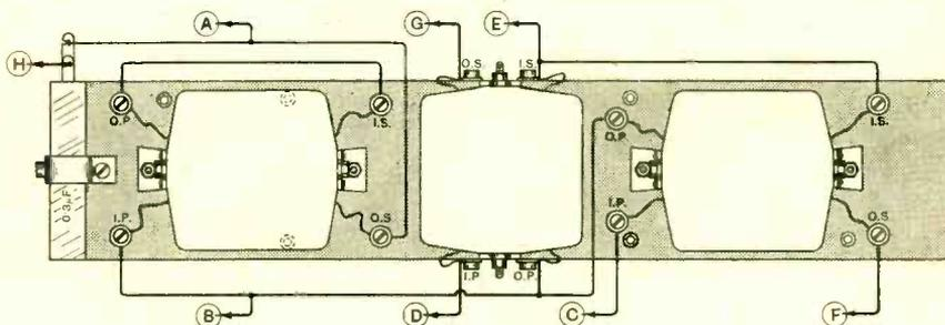
Practical wiring of transformer panel.
