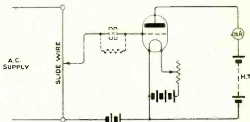
Fig. 2. Method of providing suitable values of alternating grid potential.
