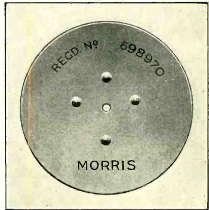
useful jig for the purpose of marking out the positions of valve legs on ebonite. It is constructed of sheet steel, and should last indefinitely.
