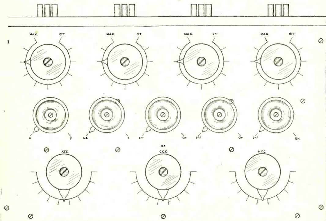
Front view with components attached. On the previous page is the setting out and engraving diagram (ivorine scales can be attached or the panel handed over to an engraver with the diagram) together with a view of the back of the panel.
