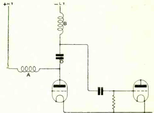
Fig. 5. This is a special arrangement in which the coil B and condenser D are joined in series. The anode current is fed through a choke coil of low self-capacity A.
