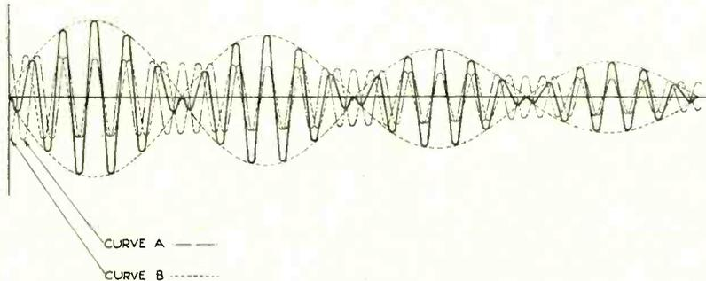
Fig. 114. Curves A and B, represent currents with frequencies of  $f_1$  and  $f_2$ . Each circuit, primary and secondary, have flowing in them at the same time two currents with frequencies  $f_1$  and  $f_2$ . The resultant current obtained by adding curves A and B is shown by the full line, and again in Fig. 115 below.
