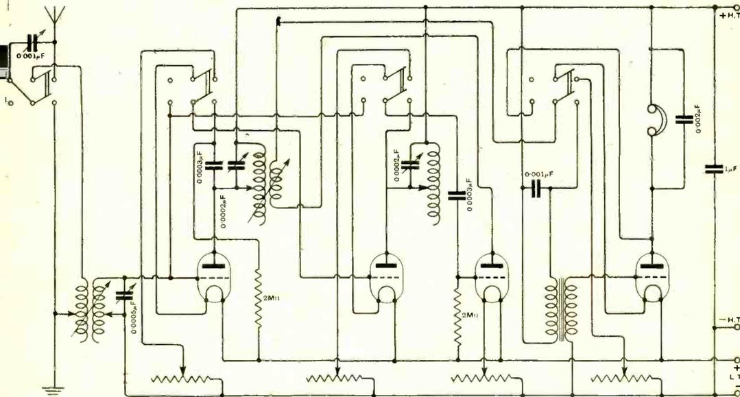
Fig. 2. "E.S." (Aberargoed). Receiver with 2 H.F., rectifier and note magnifier. The switches connected are as follows: Aerial condenser connected in series or parallel with tuning coil; first or second H.F. valves on or off; note magnifier on or off.
