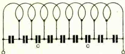
Fig. 122. The coil possesses capacity as well as inductance. The capacity is represented by condensers between turns.
