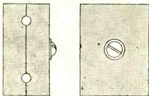
*An easily constructed ebonite cleat for providing additional support to connecting leads.*
