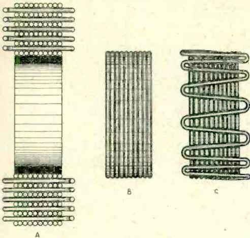
Fig 144. Showing the construction of a Burndept coil. A is a section. B shows the first layer, and C the second layer. Then another layer is wound as at B, and so on.
