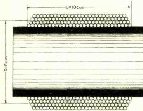
Fig. 141. A coil of this size, wound with five turns per cm., has an inductance of 1677  $\mu H$ .
