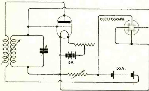
Fig. 6. Connections for the examination of potential variations in oscillatory circuits.
