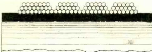
Fig. 142. To easily make tapings, the coil may be wound in sections. This construction gives less coil capacity and losses.
