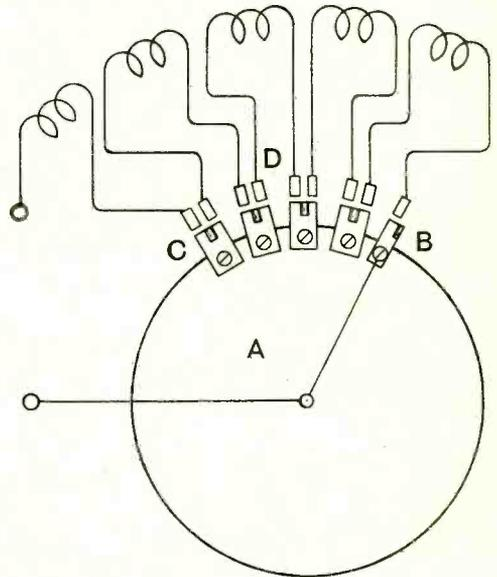
Fig. 133A. This is another form of dead end switch. The contacts C to B are mounted on a piece of ebonite (A) attached to the knob. The coil sections are joined as at D. As the knob is turned, say to the right, more sections are brought into circuit, the contacts D being bridged by the contacts C to B.
