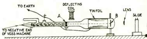
Fig. 1. Diagrammatic arrangement of the early gas discharge oscillograph.
