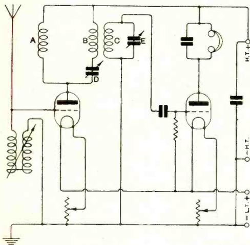
Fig. 6. Connections of a receiver built up on the principle of Fig. 5, but a transformer is used for coupling the valves. The arrangement of Fig. 5. may be used equally well, but a grid condenser and leak is connected to the bottom of coil B in the usual manner.
