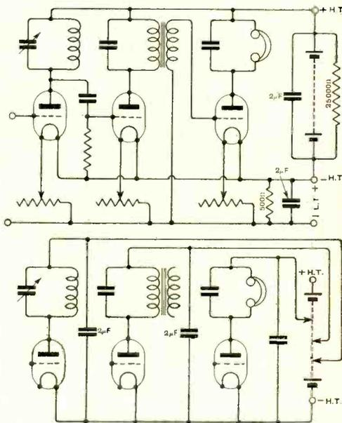
Fig. 1. The upper figure shows the method of connecting a condenser and resistances across the H.T. battery and the accumulator to help in the reduction of noise. In the lower figure a separate voltage tap is provided for each anode circuit.
