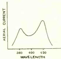
Fig. 118. If we couple a wavemeter near the secondary circuit and measure the current (or watts) induced in the wavemeter circuit when it is adjusted to various frequencies, a curve as above may be plotted. When the primary and secondary circuits are tightly coupled, a wide band of frequencies may be occupied. The curve is not flat, but has two peaks which correspond with the two frequencies produced.
