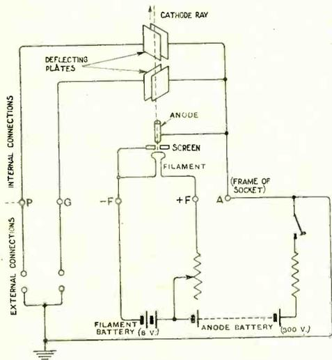
Fig. 5. Connections for the operation of the oscillograph.
