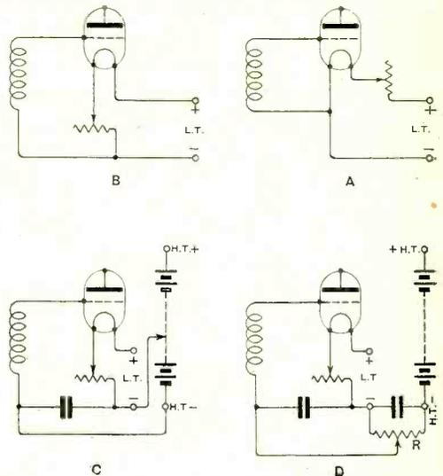
Fig. 3. Methods of connecting the grid circuit to obtain a suitable operating potential. In (A), the normal grid voltage is the same as the negative side of the filament. In (B), the grid is negative by the voltage drop in the filament resistance. Diagram (C) shows how the potential is obtained by tapping the H.T. battery. The scheme shown at (D) is probably the best of all.
