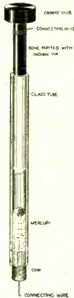
piece 5 ins. long cut off. A cork to plug one end was obtained by boring a cork with a cork borer such as is used in laboratories, and carefully pushing out the boring and using that. A connecting wire was soldered to the eye end of a small sewing needle, and the latter was pushed through the cork and the cork plugged into one end of the tube. About  $\frac{1}{4}$  in. of the pointed end of the needle was now projecting inside the tube.
