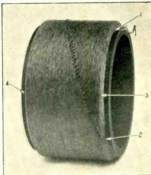
Fig. 137. A well-made banked or Telefunken coil. It has five piles or layers. Notice the end of the winding (1); the bends in the upper turns where the wire is led down to the first layer (2); the lie of the end turns (3); and the grooved former (4).
