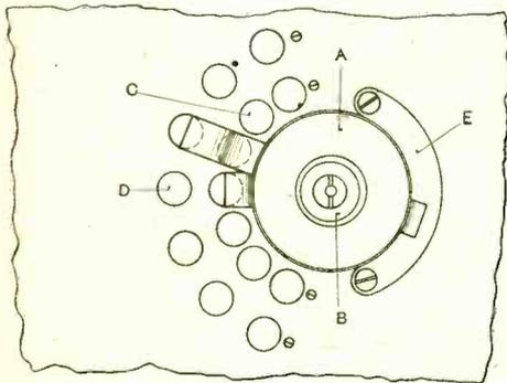
Fig. 129C. An arrangement consisting of two switches used to tap units and groups of turns. The single turns are connected with contacts C, and the groups with contacts D. Knob B moves the contact brush over the contacts C, and knob A moves the second contact brush over the studs D. The connection with studs D is made through the brush and contact E. The connection from contacts C is made through the brush and the spindle attached to knob B.
