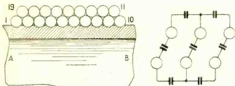
Fig. 135. A two-layer coil wound upon a former AB. There is capacity between each turn and between layers, consequently the coil capacity is prohibitively high.
