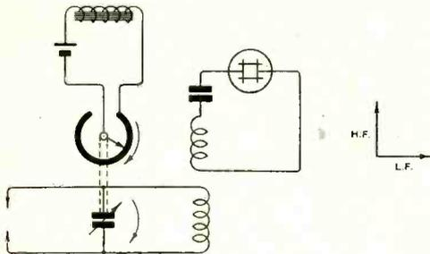
Fig. 4. Arrangement of apparatus for examination of the resonance point in reactive circuits.
