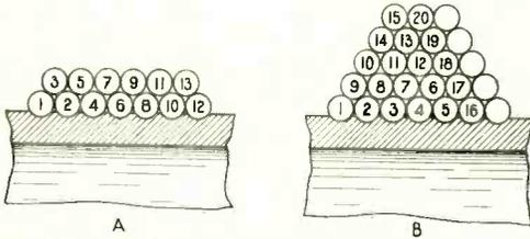
Fig. 138. Coil A is a two-pile bank winding; coil B, a five-pile bank winding. Notice the order of the turns, indicated by the numbers. Compare with Figs. 135 and 136.
