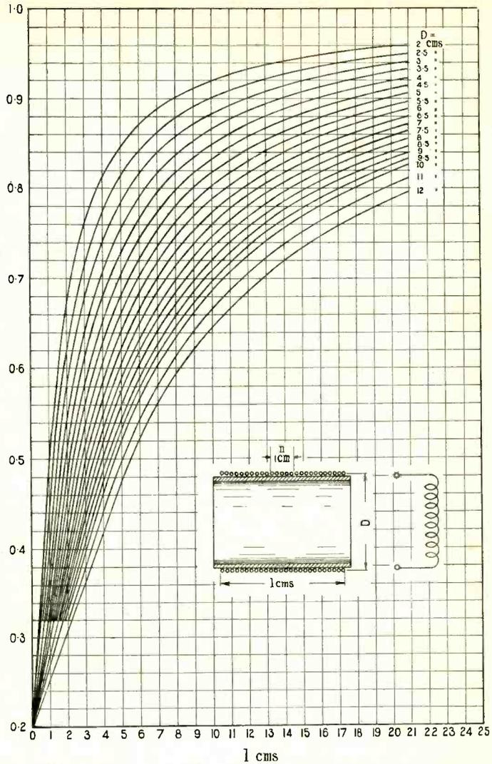
Fig. 126. Curves giving the value of  $k$  for use in the inductance formula. Thus if  $D = 10$  cms., and  $l = 18$  cms., the value of  $k = 0.8$ .
