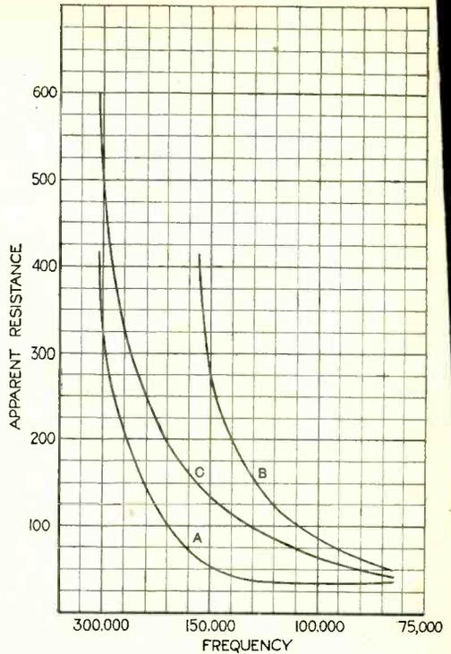
Fig. 125. Curves giving the apparent resistance of coils wound with stranded cable (A and B) and solid wire (C) at various frequencies.
