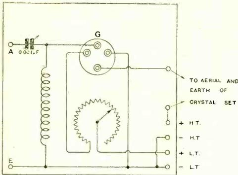
Fig. 2. "E.J.W." (New Cross, S.E.14). Diagram of an amplifying valve to be added to a crystal receiver for H.F. amplification.
