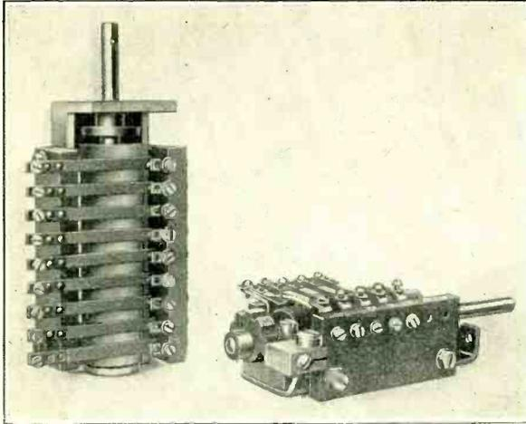
Fig. 133. A barrel-type switch may be used to tap out the coil and at the same time disconnect the portion not in use.
