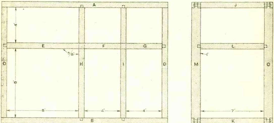
*Front and end views of an Apparatus Frame with suggested dimensions.*
