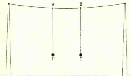
Fig. 112. An arrangement consisting of two pendulums, P and S, fastened at points A and B to the supporting cord, used to show the effects of coupled circuits.
