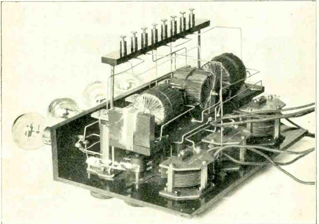
Interior view with transformer panel in position and wiring up completed.
