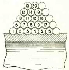
Fig. 139. A special method of bank winding, which, however, is difficult to wind. Compare with previous figures.
