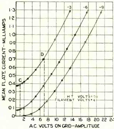
Fig. 3. The curves show plate current values obtained with various applied and fluctuating grid potentials.
