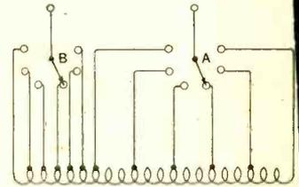
Fig. 129. A fine adjustment of inductance is possible by using two sets of tappings, one set being from single turns B, and the other from groups of turns A.
