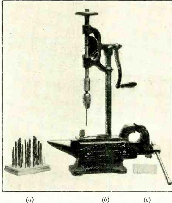
Fig. 3. (a) Set of twist drills in stand. (b) Combination tool incorporating a drilling machine. (c) A drill gauge-plate.
