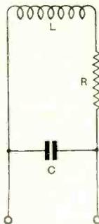
Fig. 123. Here the ideal coil is represented by  $L$ , its resistance by  $R$ , and its self-capacity by  $C$ .
