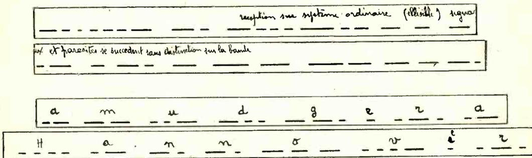
Fig. 1. Specimens of tape signals received on Mons. Y. Marrec's interference eliminator. The two upper strips, which are illegible, were received before the apparatus was placed in circuit. The lower portions were obtained with the apparatus in operation.
