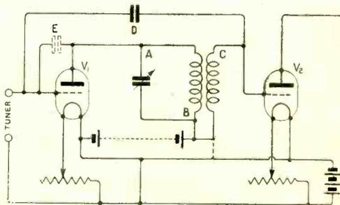
Fig. 2. The arrangement of Fig. 1 with the coil BC operating as the secondary winding of a transformer.
