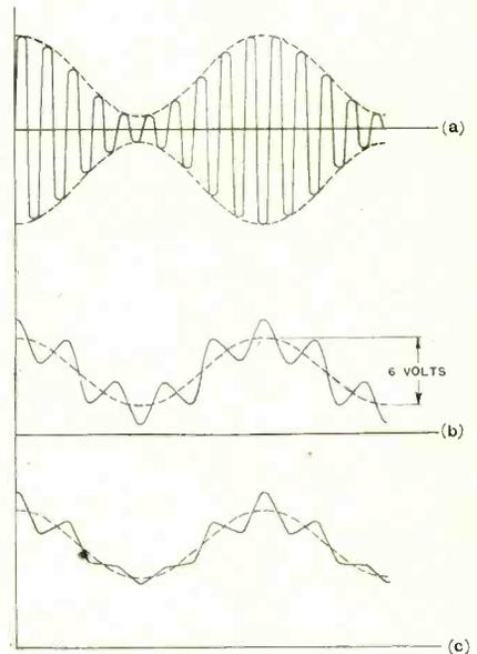
Fig. 4. Modulated oscillation trains.
