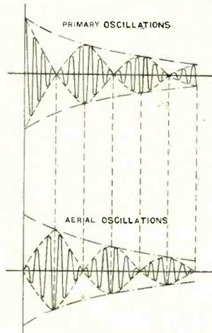
Fig. 117. When the circuits are tightly coupled, the oscillations are more quickly damped out.
