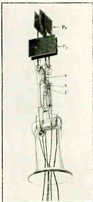
Fig. 3. Internal construction. [By courtesy of the Western Electric Co., Ltd.]
