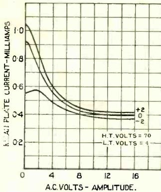
Fig. 5. Curves obtained by plotting plate current against oscillation amplitude.
