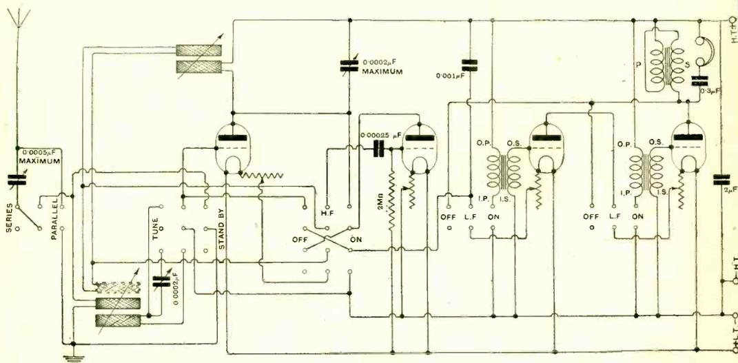
The circuit showing the principles employed. It will be observed that the closed oscillatory circuit is broken when in the "stand by" position, whilst reaction is reversed when the H.F. amplifier is taken out of circuit.
