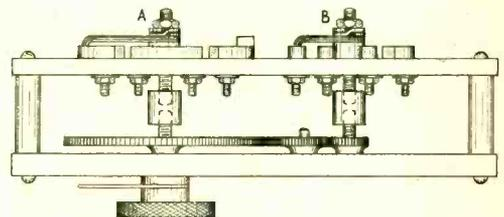
Fig. 129B. The unit and group switches may be operated by one knob through gear wheels. The groups of turns are taken to contacts A, and the single turns to contacts B. The single turns, in this case from 1 to 6, are tapped out while switch A moves over the contact section 1 and so on.
