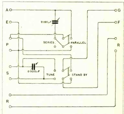
Fig. 3. "O.H." (West Byfleet). Connections of a three coil tuner.
