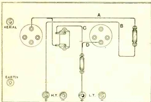
Fig. 29. An arrangement of wiring to be avoided.
