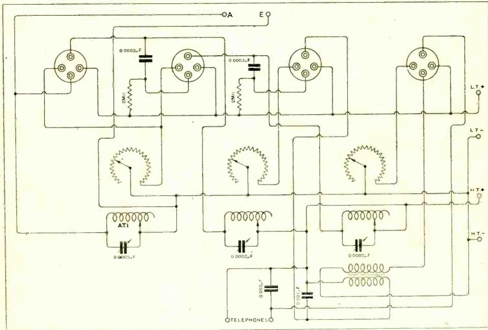
Fig. 1. “E.G.S.” (Whitstable). This receiver has two stages of H.F. (tuned anode) amplification, valve rectifier and one note magnifier.
