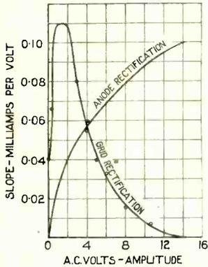
Fig. 6. The comparative sensitivity of grid and anode rectification with various oscillation amplitudes.
