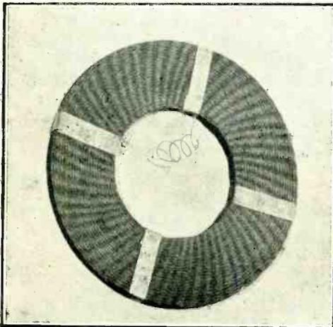
A slab coil. This coil is machine-wound, and the turns are wound from side to side, giving a wave winding.
