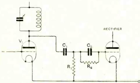
Fig. 2. Condenser  $C_1$  is the coupling condenser,  $C_2$  and  $R_2$  the grid condenser and leak resistance. Resistance  $R_1$  fixes the potential of the point joining  $C_1$  and  $C_2$ .
