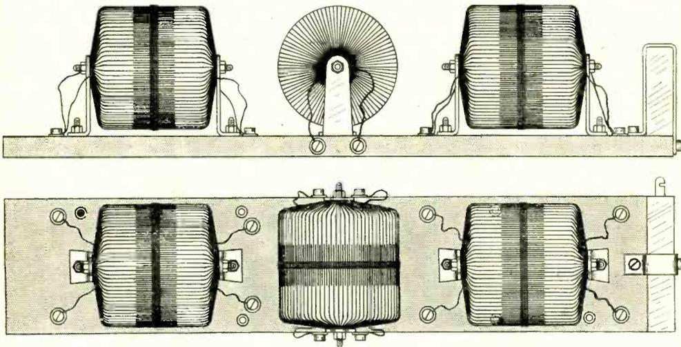
The transformer platform. One transformer has its windings connected in series to form a choke, and is employed in conjunction with the condenser ( $\frac{1}{2}$  mfd.) to feed the telephones or loud speaker.
