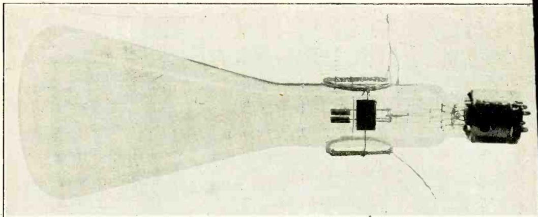
Fig. 2. Cathode ray oscillograph tube. [By courtesy of the Western Electric Co., Ltd.]
