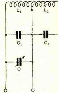
Fig. 124. When part of the coil only is used, the end not used acts to modify the behaviour of the circuit with which the coil is connected.
