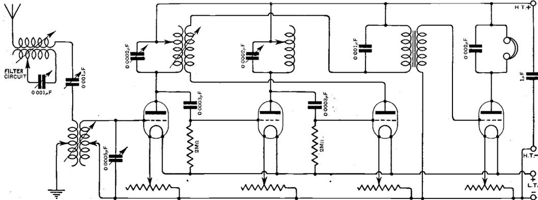
Fig. 1. "A.L." (Stavanger). Receiver with two H.F. (tuned anode) rectifier and note magnifier. A filter is connected in the aerial circuit.
