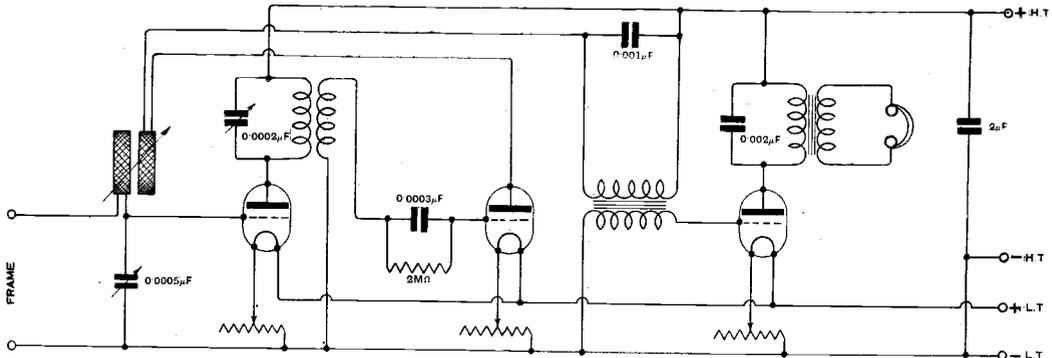
Fig. 2. "X.Y.Z." (Gosport). Connections of a receiver with H.F., rectifier and note magnifier.
