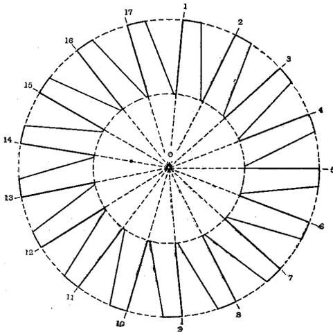
Fig. 1. A pattern to assist in rapidly making formers for basket coils. The inside diameter is 2" and the outside 4".
