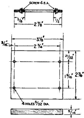
Bolts and wooden piece for clamping up grid condensers.
