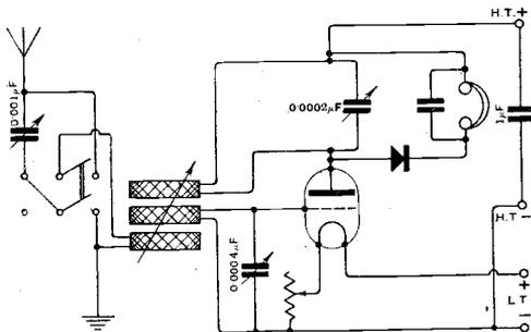
Fig. 1. "S.A.R." (Llandaff). This receiver has one valve operating as an H.F. amplifier, using a tuned anode circuit coupled to the closed circuit to obtain reaction, and a crystal rectifier.
