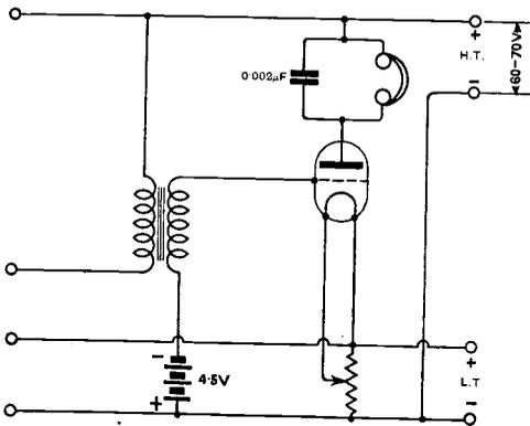
Fig. 1. "E.W.B." (Highbury). Method of applying negative potential to grid of L.F. amplifying valve.
