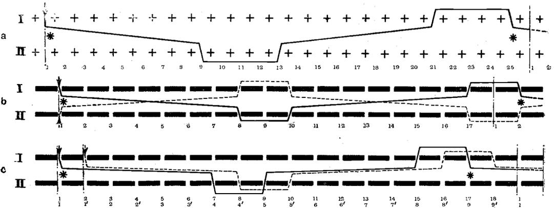
Fig. 7. Examples of methods of winding plaited unilateral honeycomb coils with one and two wires. The pitch is shown thus \*\*.
