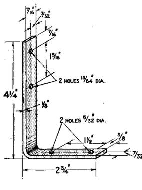
Iron bracket for supporting condenser and resistance rack.
