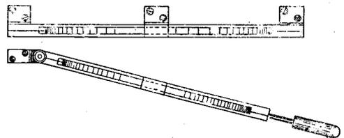
Fig. 5. This type is often employed in transmitters, the two spiral windings being connected in series, and one movable with respect to the other.
