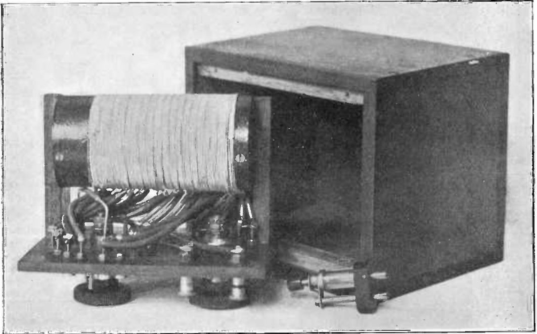
*The providing of the tapping loops while winding the coil requires care in order to avoid the possibility of turns becoming loose. The paths taken by the leads must be carefully considered to give a neat arrangement.*
