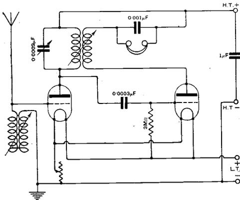
Fig. 7. “B. Mc.C.” (Ilkley). A receiver with one stage of H.F. amplification (tuned anode) and valve rectifier. The reaction coil is coupled with the anode coil.
