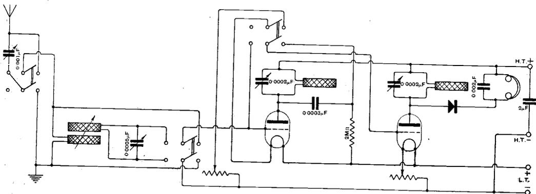
Fig. 4. "D.P." (Eliot Park, S.E.13). Receiver with two stages of H.F. (tuned anode) amplification with crystal rectifier. There is a series-parallel and a tune-stand-by switch connected. The other is for switching the first valve circuit.
