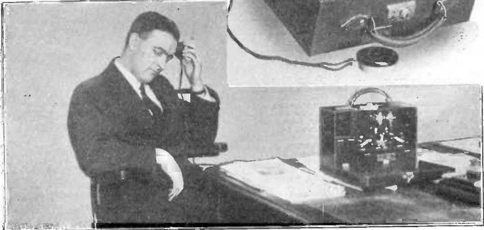
*The Otophone in use. It is not necessary to open the case as shown in the picture. The earpiece is put into circuit by means of a plug and socket and when not in use is contained in the compartment on the right.*
