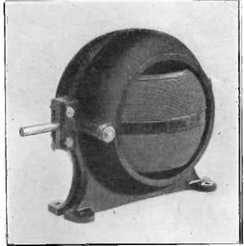
*Fig. 9. This variometer is specially useful for experimental work because it is provided with feet for easy fixing to a board. The stator is internally wound, and connections from the rotor are made through the split shaft. (G. E. Marbaix.)*
