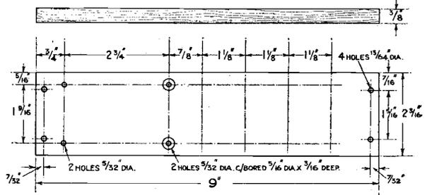
Details of the wooden panel on which the resistances and condensers are mounted.
