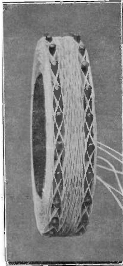
Fig. 6. Specimen of plaited honeycomb coil, having 600 turns and an inductance of 60 mH.
