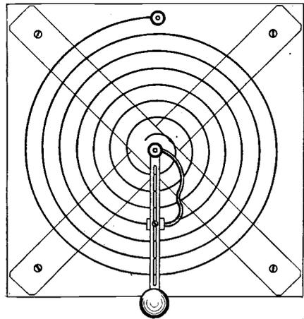
Fig. 9. A spiral inductance, as used in some types of transmitter. The amount of inductance in circuit is varied by shifting the clip.
