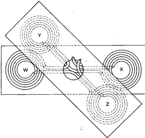
Fig. 10. A simple variometer which provides the means of obtaining a larger inductance change than is possible with an arrangement such as Fig. 4.
