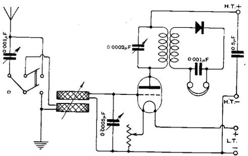
Fig. 6. "C.P.E." (Edgbaston). A single valve amplifier with crystal rectifier.
