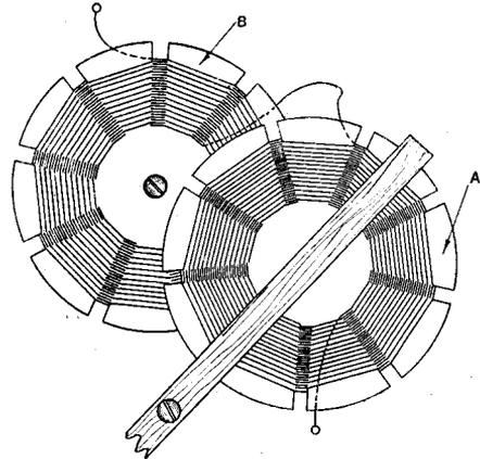
Fig. 4. Perhaps the simplest form of variometer consists of two basket coils connected in series, one of which, A, is movable with respect to B.
