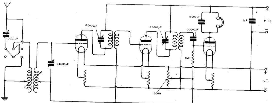
Fig. 2. "H.E." (Hammersmith). Three-valve receiver (2-v-0) with potentiometer grid control.
