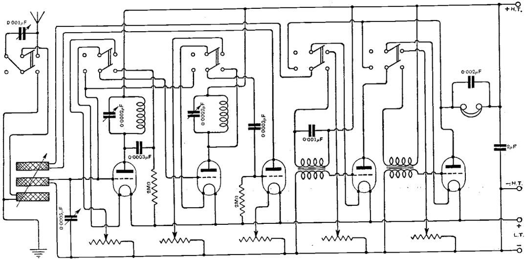
Fig. 3. "H.N." (Northwich). A five-valve receiver with switches.
