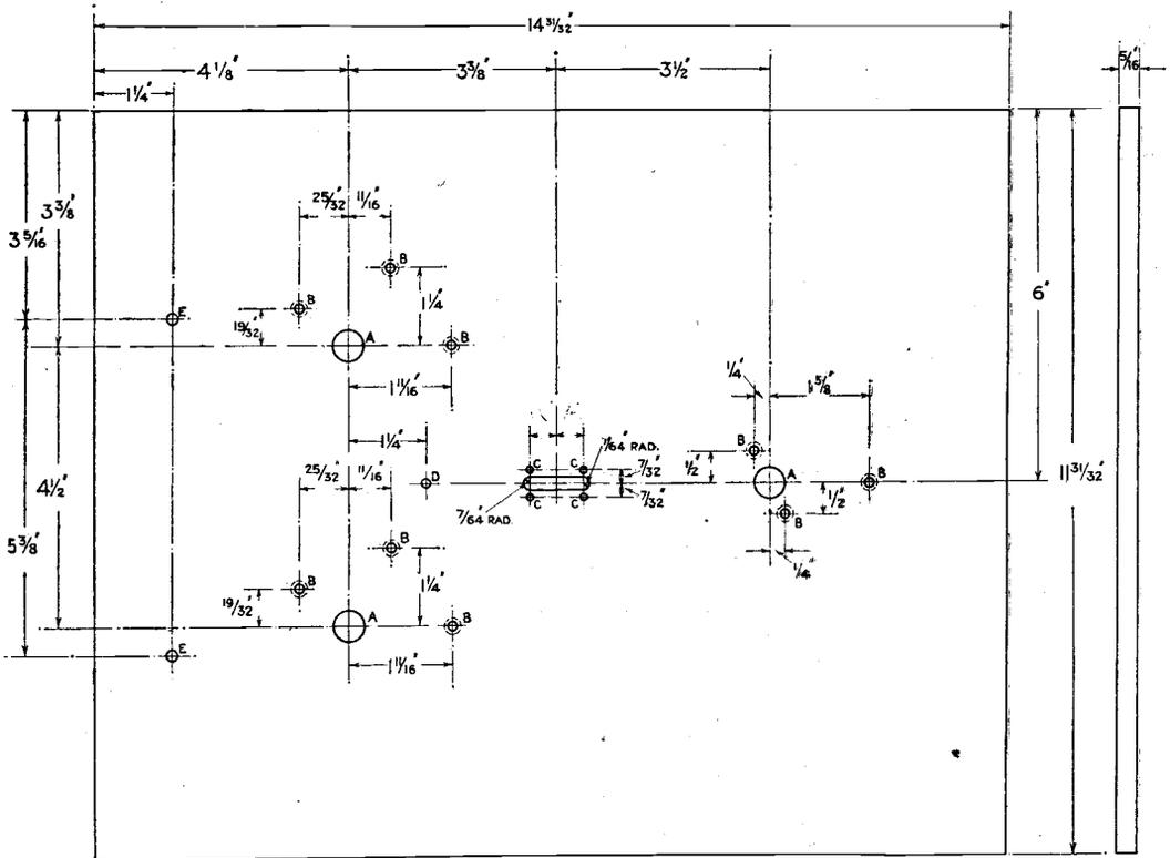
Scale drawing of the front panel. The positions and sizes of the holes are arranged to suit the particular components mentioned. The poles for attaching the switch are  $9/16''$  from the centre line. Sizes of holes: A,  $1/8''$ . B,  $5/32''$  and countersink on top side for No. 4 BA screws. C,  $1/8''$ . D tap 4 BA x  $3/16''$  deep. E, tap 2 BA x  $3/16''$  deep.
