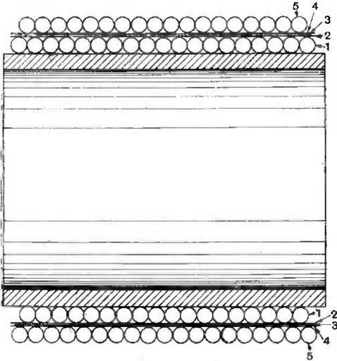
Fig. 3. Another method of shielding the secondary winding. A layer of metal foil is placed between the primary and secondary windings marked 1 and 5.
