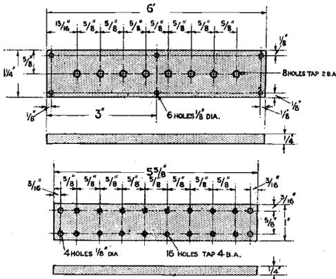
Dimensional drawings of the terminal and connector strips.
