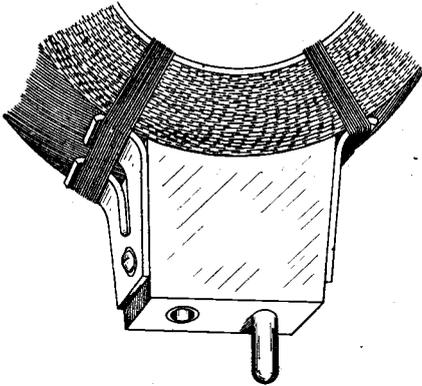
(b) The plug here has metal side-pieces which are tied to the coil with cord.
