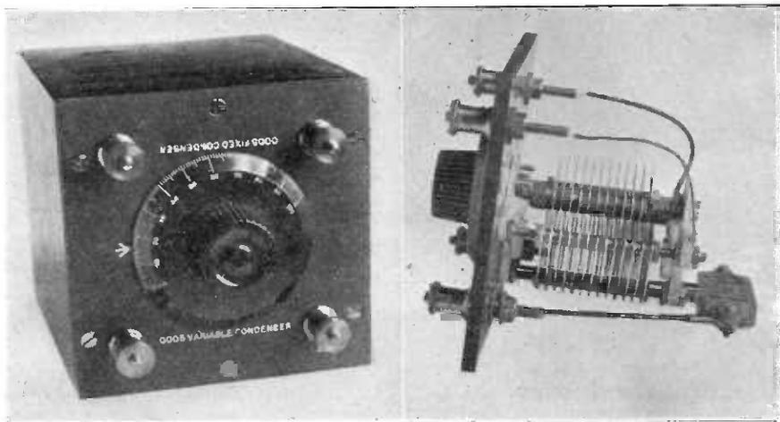
*A useful condenser arrangement suggested by Mr. J. R. Hoult, in which a small condenser (0.0005 mfd.) is mounted with the variable condenser and brought out to separate terminals. By connecting the fixed condenser in parallel or series with the variable, the capacity range is extended.*
