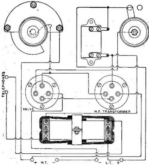
Fig. 6. Connections of the testing instrument.
