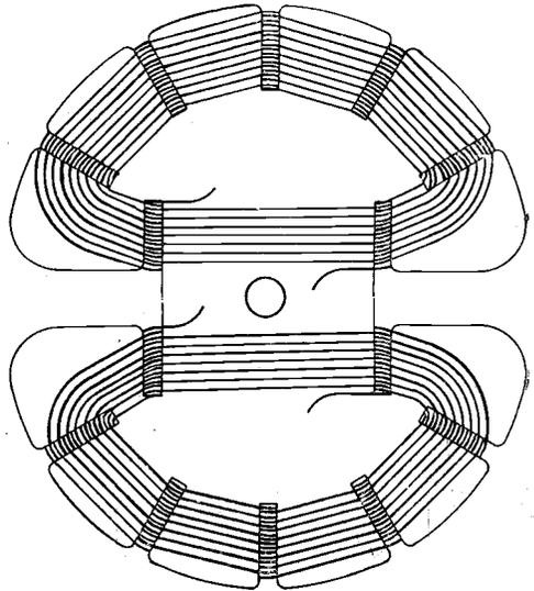
Fig. 11. One winding of a D type variometer. Two of these are made. One is fixed, and the other mounted above it so that it may be rotated.
