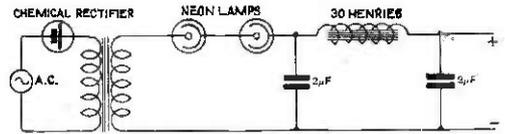
Fig. 3. Pulsating high potentials suitable for neon lamp rectification are obtained from an A.C. source by the insertion of a chemical rectifier in the transformer primary.
