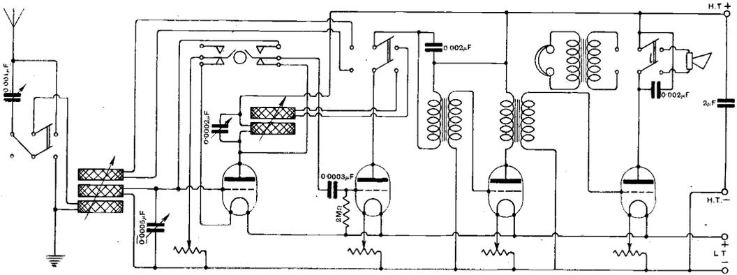
Fig. 1. "F.W.L." (Sheffield). Receiver with H.F., valve rectifier and two note magnifiers. Switches are provided to switch the first valve, change the reaction coil connections, and to join telephones or a loud speaker to the last valve.
