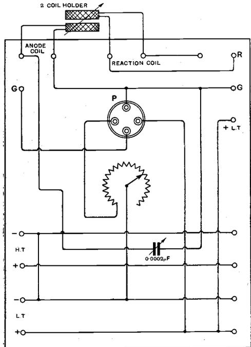
Fig. 2. "ROY" (Solworth). Connections of a H.F. amplifier suitable for adding to the receiver given in the issue of May 26th.
