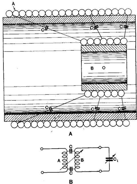
Fig. 1. Showing the capacity coupling between coils. Winding A represents the primary of a coupling, and B the secondary. Capacity coupling is indicated by the condensers C.
