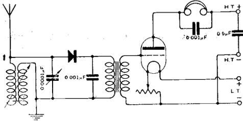
Fig. 3. "E.A.T." (W. Kilburn). A simple set consisting of a note magnifier added to a crystal receiver.
