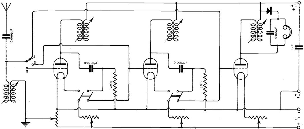
Fig. 3. "RAW RECRUIT" (W.1). Variometer tuned three-valve receiver (3-c-0) with switches to control the number of H.F. valves in use.
