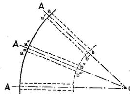
Fig. 2. When the former has been marked out with the aid of the pattern, the slots are cut as at ab-a'b', etc.
