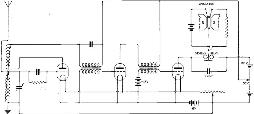
Fig. 3. Complete diagram of the receiver and recorder.
