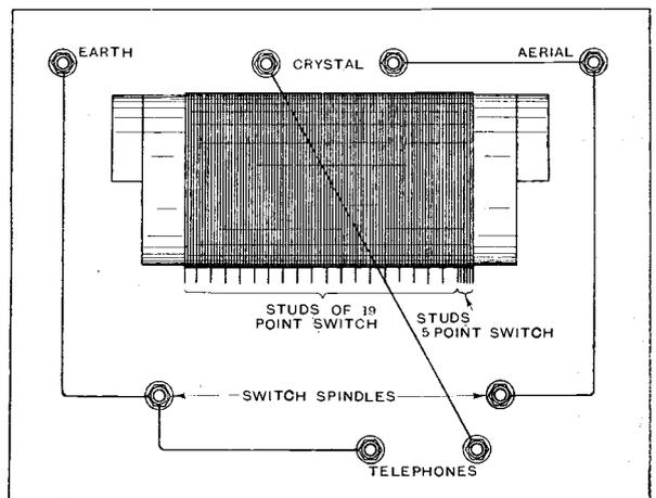
Theoretical and practical wiring diagrams. Should reception from the desired station be obtained with more than half of the coil in circuit, then signal strength can probably be improved by connecting a small fixed condenser (0.0003 mfd.) in the aerial lead and returning.
