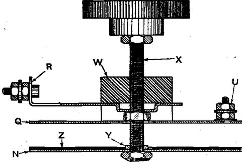
The variable condensers. Q, N the plates; Z mica and shellac; Y holding-down collar; W insulating mounting piece; X 2BA spindle; R, U terminals. A copper clip, insulated with mica, secured to the strip leading to the terminal R, serves as a grid condenser.
