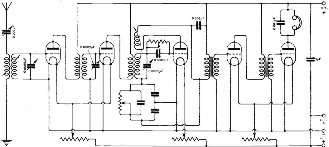
Fig. 1. "R.A.G." (Broxton). A suggested method of adding two stages of high frequency amplification and two note magnifiers to a Flewelling receiver. It may be necessary to omit the condenser in the anode circuit of the rectifier.
