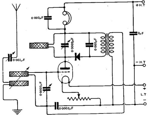
Fig. 3. "A.R.A." (Victoria Park, E.9.) Simple dual amplification receiver.
