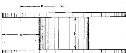
Fig. 6. Shape of former used in construction of certain multilayer coils. Honeycomb or duolateral coils have this cross section.
