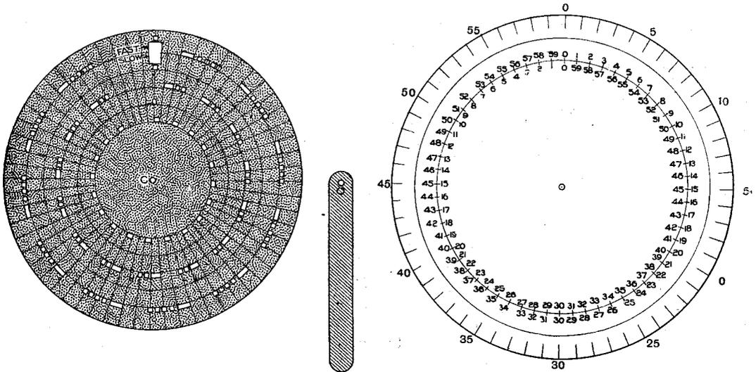
The revolving disc and the fixed dial of the time indicator. In constructing the indicator it should be made to a bigger scale than the illustration, to facilitate both the preparation and subsequent reading from the figures. The particular revolving disc illustrated is for use with the Paris time signals.
