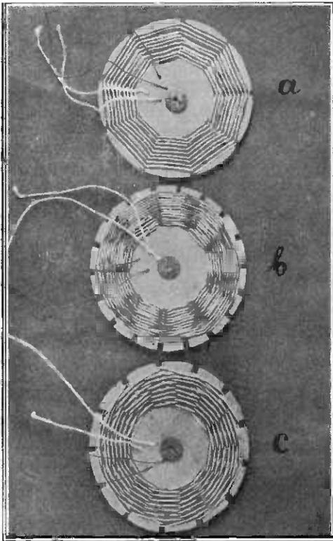
Fig. 8. Specimens of basket coils with two windings. Both windings are put on together.
