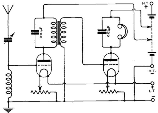
Fig. 2. Detector valve circuit and note magnifier.
