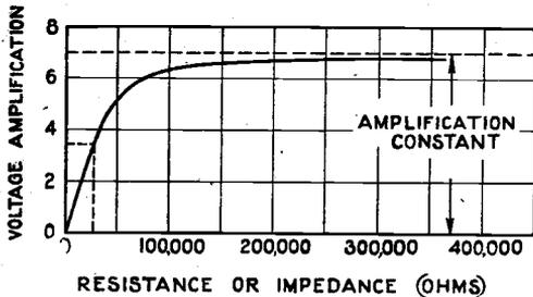
Fig. 2. Curve giving the relation between resistance or impedance in the plate circuit, and the voltage amplification.
