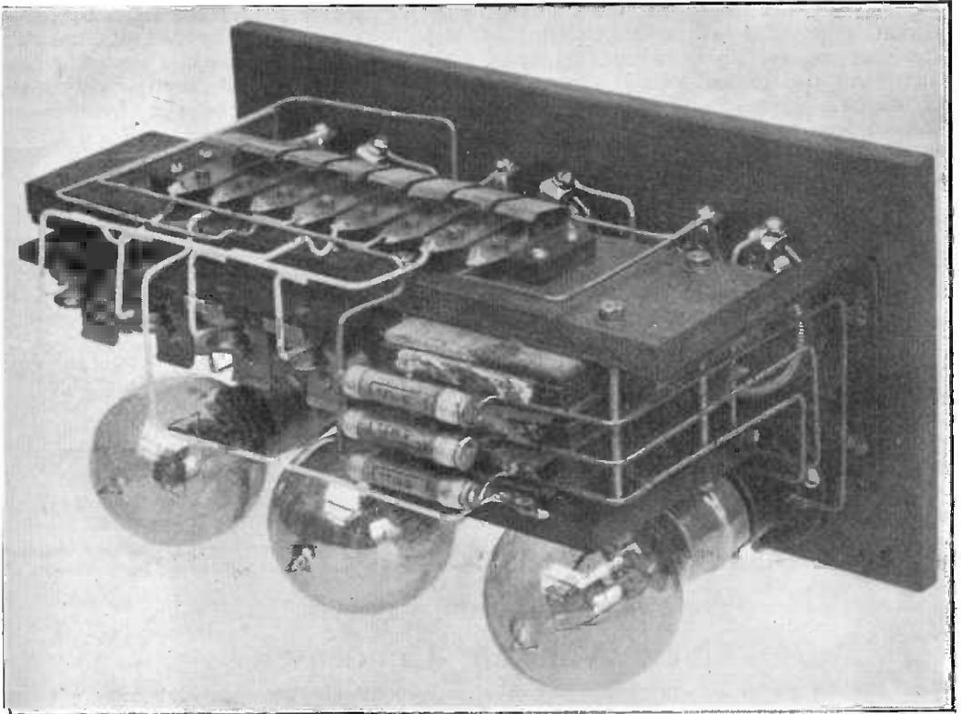
*This view shows the general arrangement of the components. For clearness and good appearance only right-angle bends are made in the leads, which are enamelled in various bright colours.*
