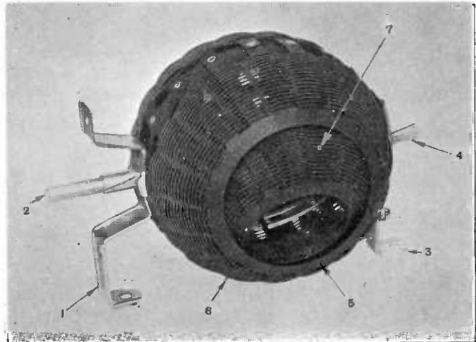
An American basket ball variometer. The construction may be understood by examining the photograph. Both windings are wound as basket balls. 1 and 3 are the supports, 2 the shaft to which is fastened the knob, 4 is the back end of the shaft, 5 the prepared former, 6 the stator winding and 7 the rotor winding.
