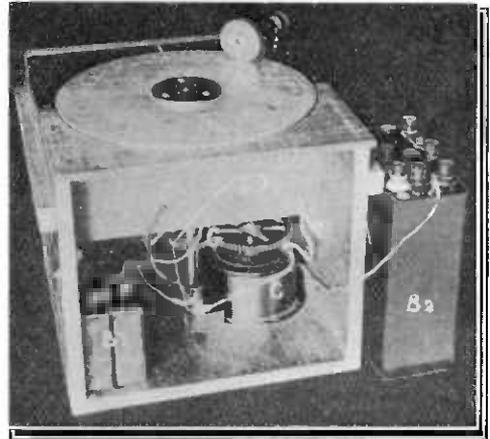
Side removed to show gearing for extending the scale from 180° to 360°. G. 2:1 gearing. C. Variable condenser. B2. 6-volt accumulator. B3. 30-volt H.T. battery.
