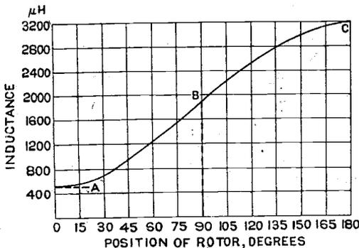
Fig. 3. The curve shows the inductance of a variometer for different settings of the rotor.
