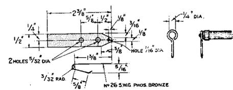
Dimensions of connector springs. The method of making connection to the grid leaks is also shown, and care must be taken not to overheat the leaks as they are wax filled.
