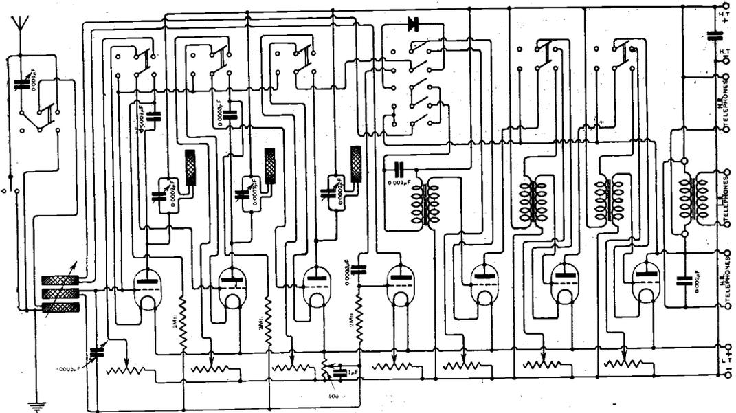
Fig. 2. "E.S.E." (Middlesex). A seven-valve receiver with three H.F., valve or crystal rectifier, and three note magnifiers.
