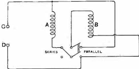
Fig. 14A. Method of connecting a throw-over switch to join coils in series or parallel.
