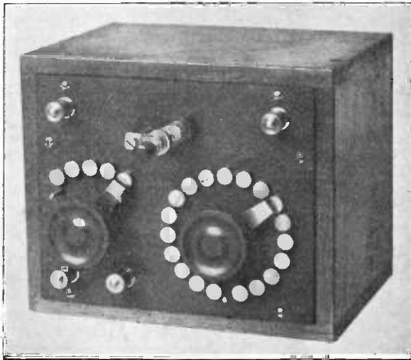
*The aerial and earth terminals are at the top, and those for the telephones beneath the five-stud switch. The face of the panel is slightly raised above the edge of the box.*
