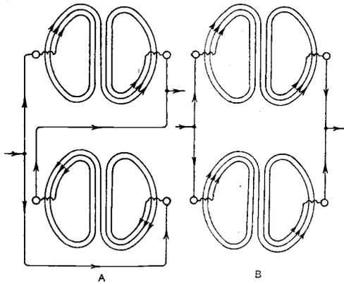
Fig. 12. Explaining the operation of a D type variometer when the coils are in parallel. The inductance is low at A and high at B.
