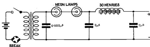
Fig. 2. Rectifier and smoothing circuit for use with induction coil and vibrator or motor-driven interrupter.
