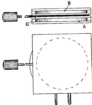
Fig. 17. This is a variometer which has two windings A and B. The metal plate C is arranged so that it may be moved in between the two coils.
