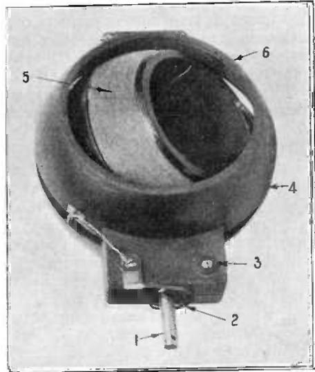
Fig. 7. This variometer is represented in Fig. 2C. Here, 1 is the spindle carrying the rotor 5. The spring 2 makes connection between the rotor and stator 4. Notice the rotor winding 6 is on the inner surface of the stator former. The other end of the coil is connected at 3. (Igranic Electric Co., Ltd.)
