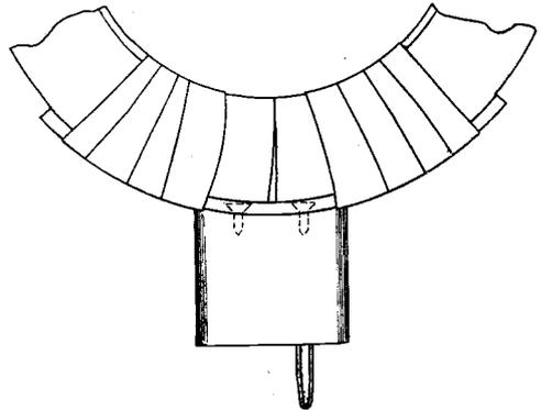
(a) A simple method of fixing the plug to the coil. A strip of fibre is held with screws to the plug, and the fibre is secured with tape to the coil.
