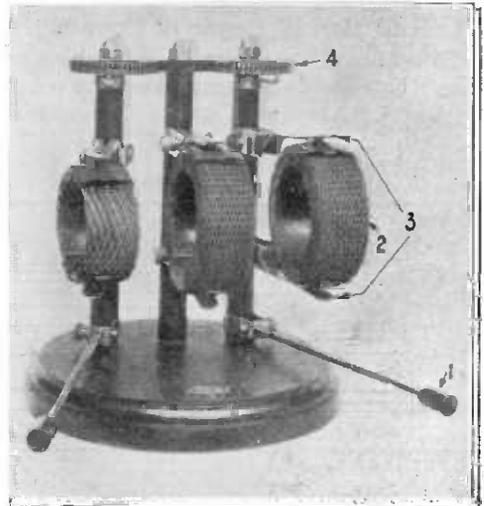
Fig. 6. A three-coil holder for Gimbal coils. The position of the outer coils is varied with the handles 1. The coils are marked 2, coil holding clips 3, and the scales 4.
