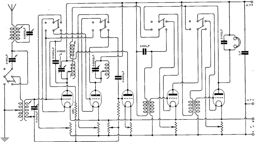
Fig. 4. "C.P.E." (Birmingham). A five-valve receiver, two H.F. tuned anode, detector and two L.F. valves with switches.
