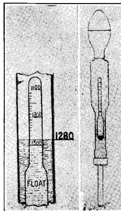
*Convenient type of hydrometer for easily testing the gravity.*
