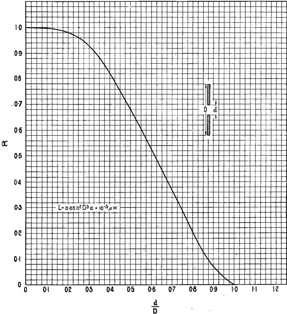
Fig. 10. The inductance of basket or spiral coils may be calculated with the formula  $L = 0.85 n^2 D^2 \alpha \times 10^{-3} \mu H$ . Values of  $\alpha$  corresponding with values of the ratio  $\frac{d}{D}$  are obtained from the curve above.
