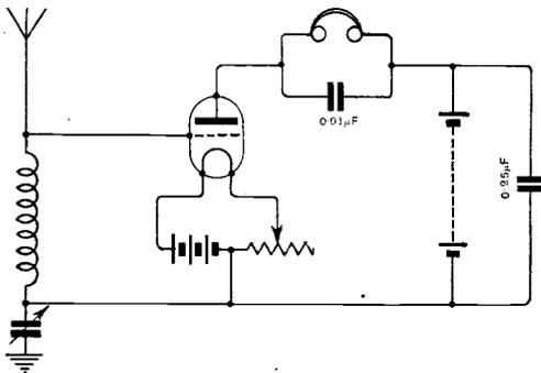
Fig. 1. Simple detector valve circuit in which a soft valve functions well.
