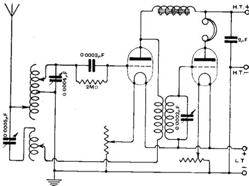
Fig. 5. "D.M." (Belgium). Connections of a Reinartz receiver with one stage of H.F. amplification.
