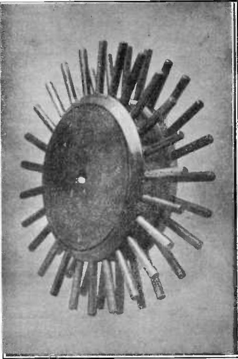
Fig. 5. The wooden former used in the construction of plaited honeycomb coils.
