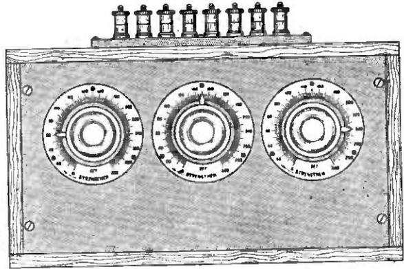
View of top of the finished amplifier. Ivorine scales have been added to indicate the settings for the resistances.
