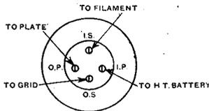
Fig. 2. Usual method of connecting the plug-in type of H.F. transformer.
