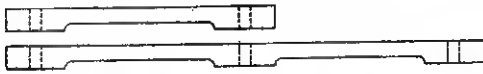
Fig. 3. Ebonite spacing strips. A hollow on the underside gives clearance to the windings.
