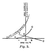
rate dependent on the resistance of the leak and the potential of the point to which its lower end is connected. The resultant steady potential of the grid can be conveniently found by a graphical method.
