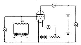
Fig. 1. Circuit for plotting grid voltage—anode current characteristic. The potential applied to the grid is varied by means of the potentiometer P and indicated by the voltmeter V<sub>1</sub> while the plate current is read off on the milliammeter mA. Filament current and plate voltage remain constant.
