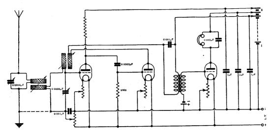
Fig. 2. "F.M.D." (Bristol). A three-valve receiver designed for long wave reception.
