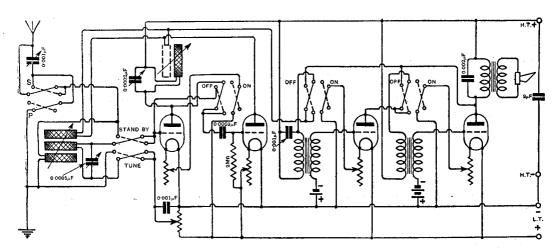
Fig. 1. "A.H.M." (Dublin). A four-valve receiver controlled by means of double pole radial switches.
