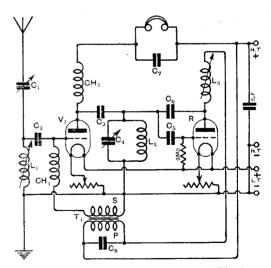
Fig. 3. A reflex receiver similar to that of Fig. 2, but a valve detector is employed, and reaction introduced into the intervalve H.F. coupling.
