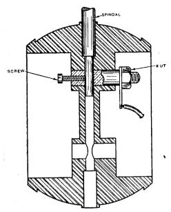
Fig. 3. The threaded portion of the spindle is omitted, which facilitates withdrawal.
