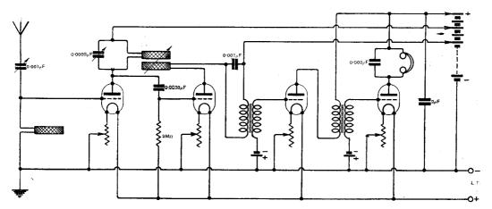
Fig. 1. "J.B." (Milan). A four-valve receiver with one stage of H.F. and two stages of L.F. amplification.
