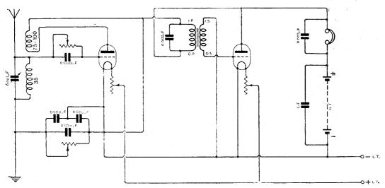
Fig. 3. Flewelling circuit with note magnifier.
