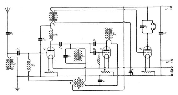
Fig. 4. A reflex receiver provided with a reaction control and giving one stage of H.F. amplification, valve rectification and two stages of L.F. amplification.
