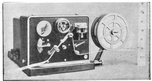
An ingenious inker of German manufacture, making use of the Johnsen-Rahbek effect. Adhesion between a metal plate and semi-conductor holds the needle over when a potential is applied.
