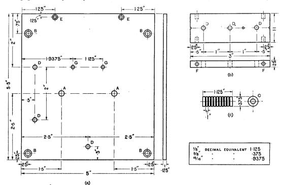
Fig. 1. Component parts of the inductance unit. Decimal dimensions are shown for uniformity and fractional equivalents are given. Sizes of holes: A, Drill 7/32" dia.; B, Drill 3/16" dia. and countersunk on topside for No. 3 B.A. screws; C, Tapped No. 3 B.A.; D, Drill 5/32" dia.; E, Drill 1/8" dia. and countersunk on topside for No. 6 B.A. screws; F, Tapped No. 6 B.A. × 3/16" deep; G, Tapped No. 4 B.A.
