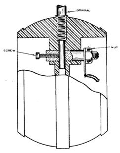
Fig. 2. A set screw is here introduced to prevent the spindle from being pulled out of alignment.
