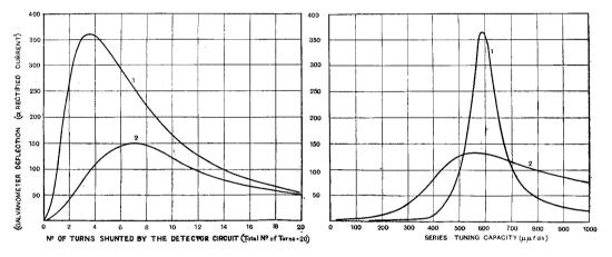
Fig. 4. Curve showing the reduction of the maximum signal intensity when the effective resistance of the aerial is increased.
