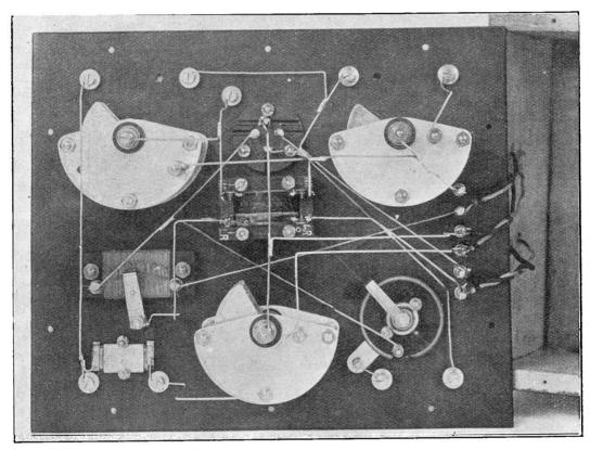
Underside view showing the wiring.
