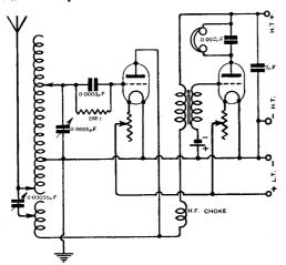
" F.R." (Bristol). A Reinartz receiver with one stage of L.F. amplification
