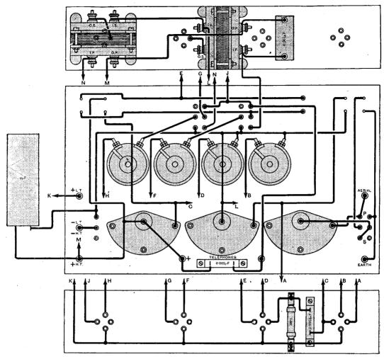
Diagram showing the actual points between which leads are run.
