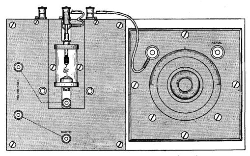
Fig. 4. The arrangement of inductances, detector and tuning condenser.
