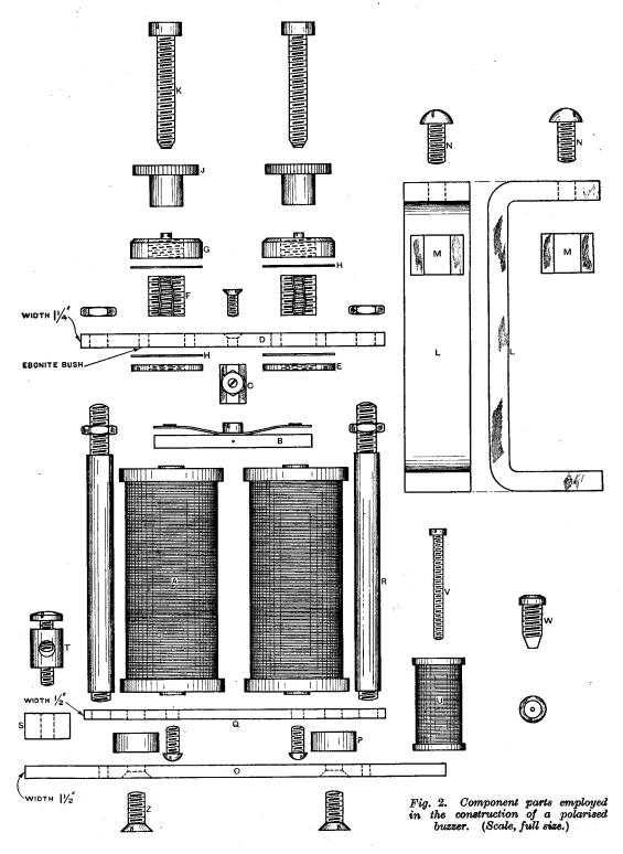
bobbins with two inner ends and two outer ends each, together with their iron cores are constructed. The back bar (Q) is modified somewhat as regards shape at the ends, as in the standard instruments these are provided at one end with a hole and at the other with a slot for fixing to the instrument box; these holes and slots are cut away, leaving a plain straight back bar with the uprights marked R in Figs. I and 2.
