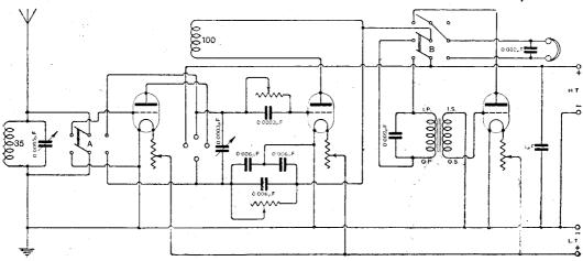
Fig. 4. Flewelling circuit showing method of adding H.F. amplification. Switches are introduced for bringing the H.F. and L.F. circuits into operation.
