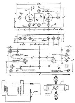
Fig. 3. Drilling dimensions and circuit adopted.
