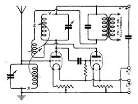
Fig. 5. Increasing the tuning range of set fitted with H.F. amplification.
