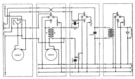
Fig. 2. "K.D.C." (London, S.W.16). A three-valve receiver built on the unit system.
