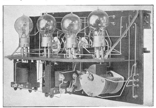
Rear view showing the valve platform and arrangement of the components. In emethod of wiring up the valve sockets so that the leads are conveniently distributed above and below the valve platform can be clearly seen.
