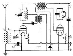
Fig. 1. A simple reflex receiver giving one stage of H.F. amplification and two of L.F. amplification. Notice that the crystal circuit is connected across only part of the anode coil  $L_3$ .
