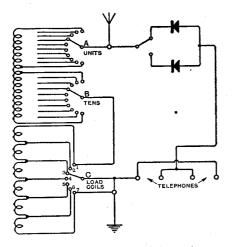
Fig. 3. The connections of the receiver.
