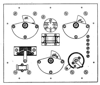
Fig. 3. Arrangement of the components on the underside of the panel. (Scale \( \frac{1}{3} \) full size.)
