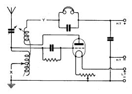
Fig. 4. Typical amateur single-valve set. Both aerial and reaction inductances need to be loaded as shown at the points X and Y.
