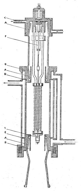
Sectional view of demountable transmitting valve, showing the location and construction of the joints.
