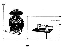
Fig. 1. Position (X) for connecting a loading coil for extending the wavelength of a variometer-tuned crystal set to 1,600 metres.
