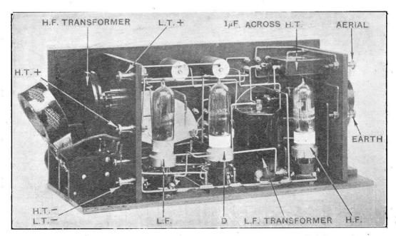
Rear view. The vertical brackets not only support the front panel, but carry several of the components.
