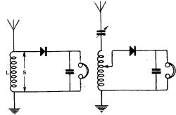
Fig. 3. A typical crystal receiving circuit.
