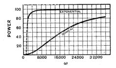
Fig. 1. Comparison of loading of exponential and conical horns.
