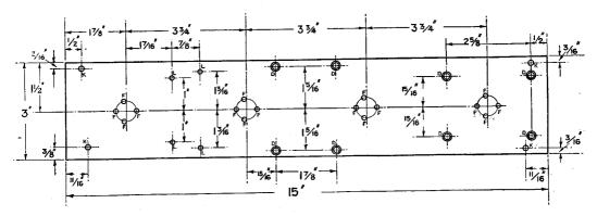
Sizes of holes: D, drill 5/32" dia., and c/sink on topside for No. 4B.A. Details of the valve platform. screws, F, drill \( \frac{1}{8} \) dia., K, tap 4B.A., L, tap 6B.A.
