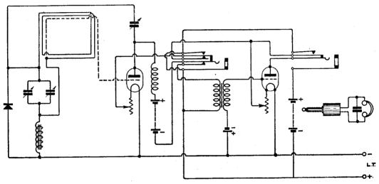
Fig. 1. "H.R.W." (Bridgewater). The method of adding a note magnifier to the portable receiver described in the issue of April 9th, 1924.
