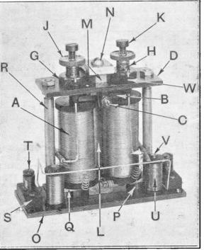
Fig. 1. The complete buzzer.
