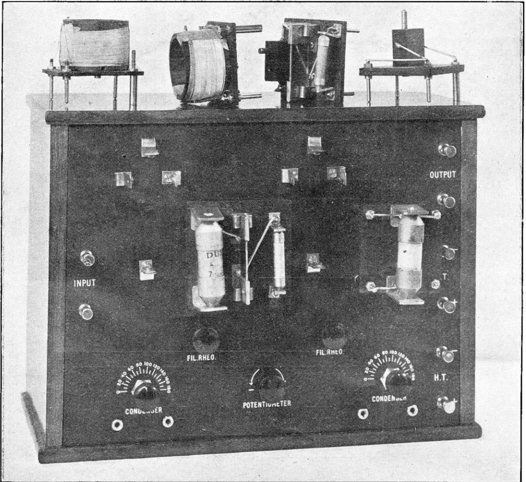
A receiver with two stages of H.F. amplification with interchangeable range units.
