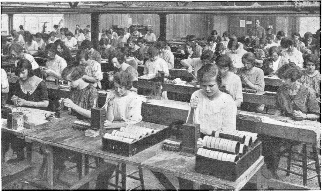
The assembly of tuning coils in progress at the works of the Igranic Electric Co., Ltd.
