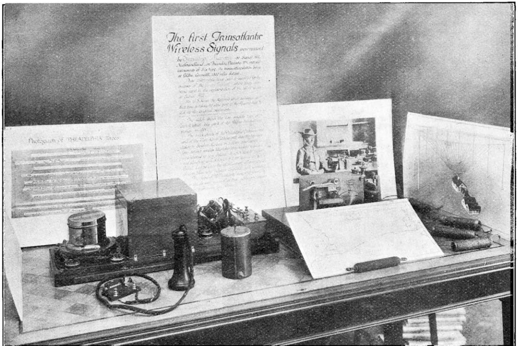
The original apparatus employed by Senatore Marconi in 1901, with which to receive signals across the Atlantic. When not in use in the Pageant the apparatus is on view in the Newfoundland pavilion at the British Empire Exhibition.
