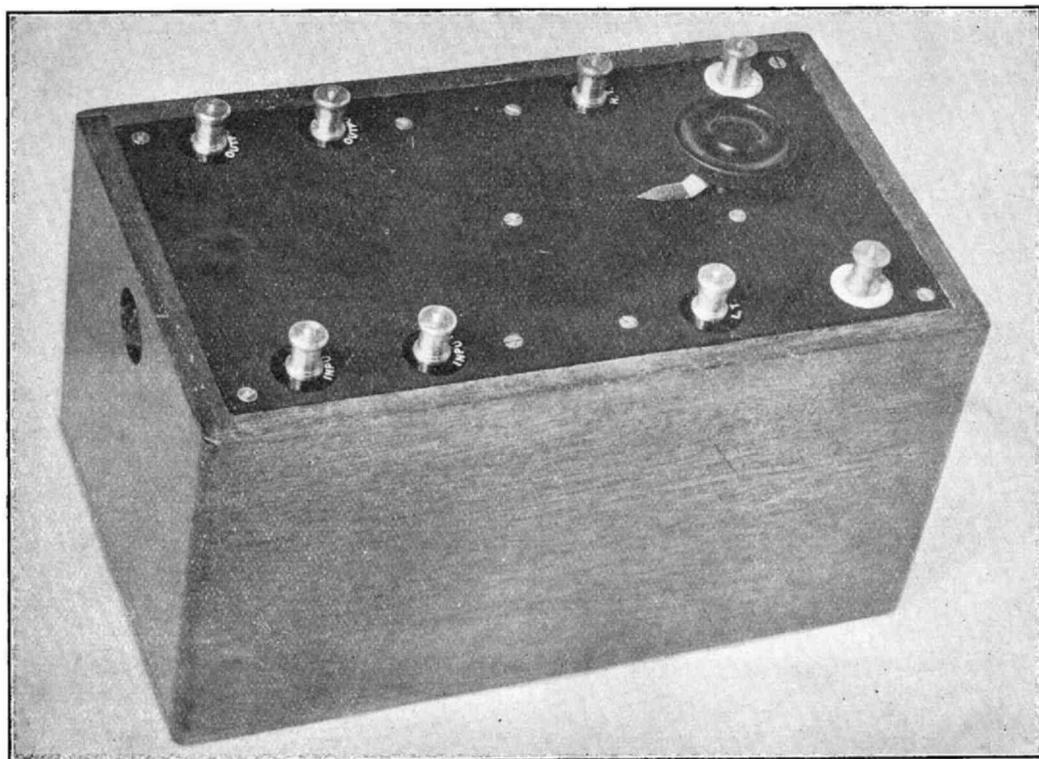
*The complete instrument, suitable for measuring small potentials at high frequencies.*
