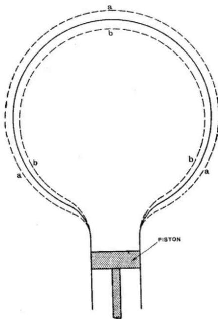
Fig. 1. Section of a toy balloon used in illustration of the production of sound waves.
