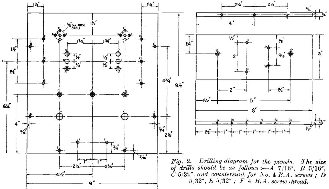
Fig. 2. Drilling diagram for the panels. The size of drills should be as follows:—A 7/16", B 5/16", C 5/32", and countersunk for No. 4 P.A. screws; D 5/32", E 5/32"; F 4 B.A. screw thread.
