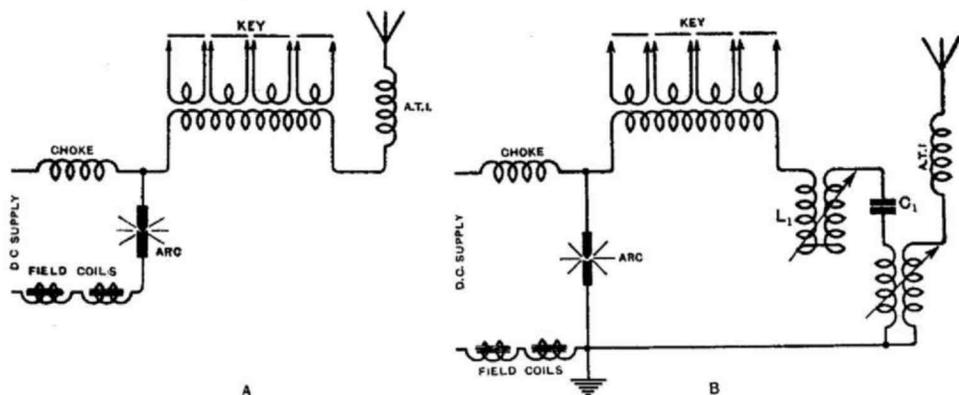
Fig. 1. (A) the original circuit at Leafield; (B) the new coupled circuit.
