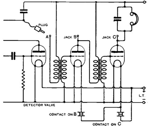
*Connections of switching device for two stages of L.F. amplification.*
