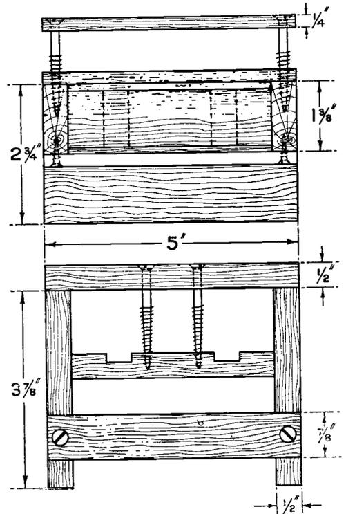
Fig. 3. Details of the wooden framework which carries the Weston relay, grid battery and valve platform.
