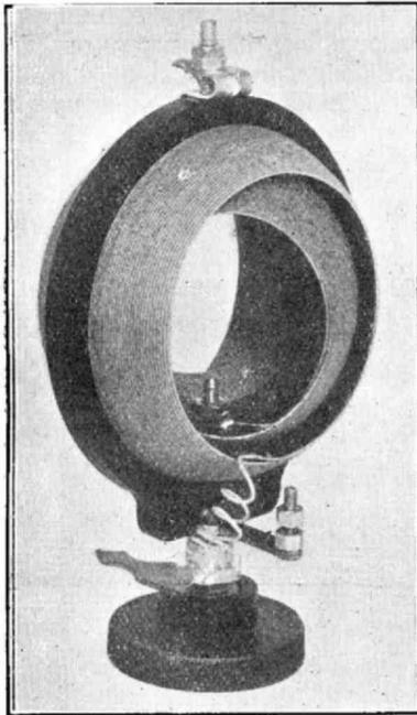
Hence in well-designed variometers we find the windings are separated by a distance which is considerably more than is required from a mechanical point of view. It is well known that the effective resistance of a coil may be reduced by the employment of a large gauge of wire, and by reducing the amount of material in the supports of the coils to a minimum.
