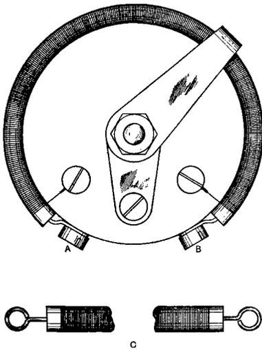
insulated covering. A suitable winding is No. 36 Eureka wire.
