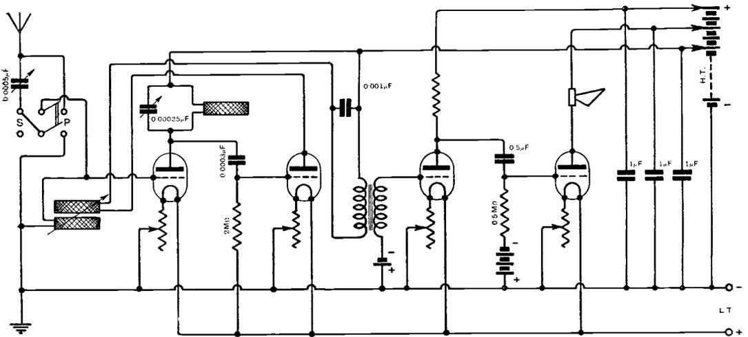
*Circuit for a four-valve receiver.*
