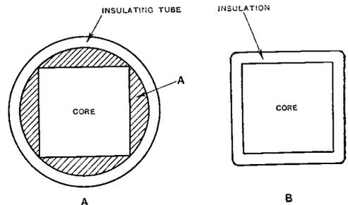
Fig. 1. In sketch A, a circular former which just fits over the core is employed; hence, the space marked A is wasted. In sketch B, the coil is wound on a rectangular former.
