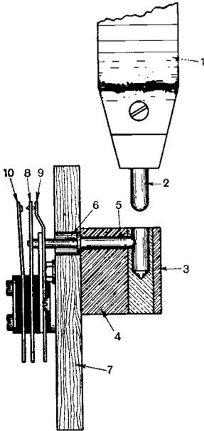
Fig. 3. A coil holder provided with a switching arrangement.
