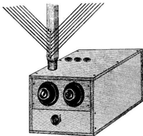
Fig. 7. The containing cabinet with lower portion for accommodating the H.T. and L.T. batteries. The stem of the frame aerial passes clear through the wiring of the instrument, and the weight of the batteries makes a suitable base for giving vertical support to the frame.
