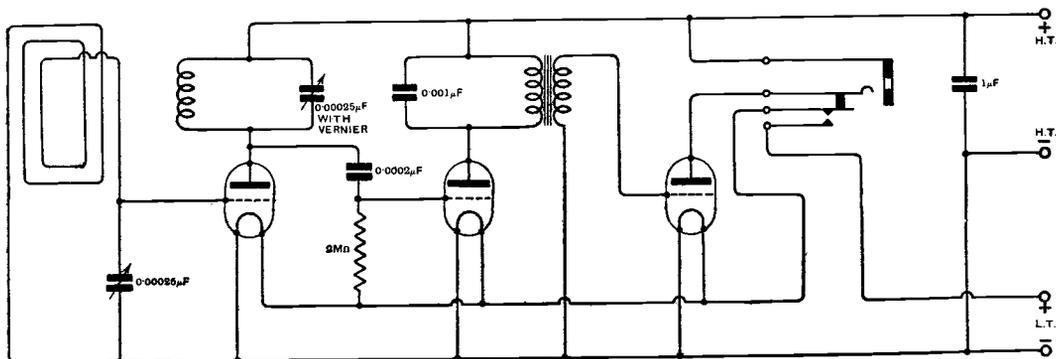
Fig. 1. Circuit of frame aerial receiver, with tuned anode high frequency amplifier, valve detector, and note magnifier. Reaction coupling is unnecessary owing to the low degree of damping possessed by the frame aerial.
