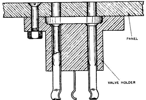
Fig. 5. Sketch of a valve-holder which is designed to be fitted below the panel.
