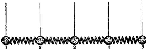
Fig. 2. A mechanical analogy to illustrate wave motion.
