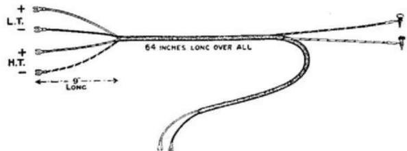
*The Easifix battery connecting cable.*
