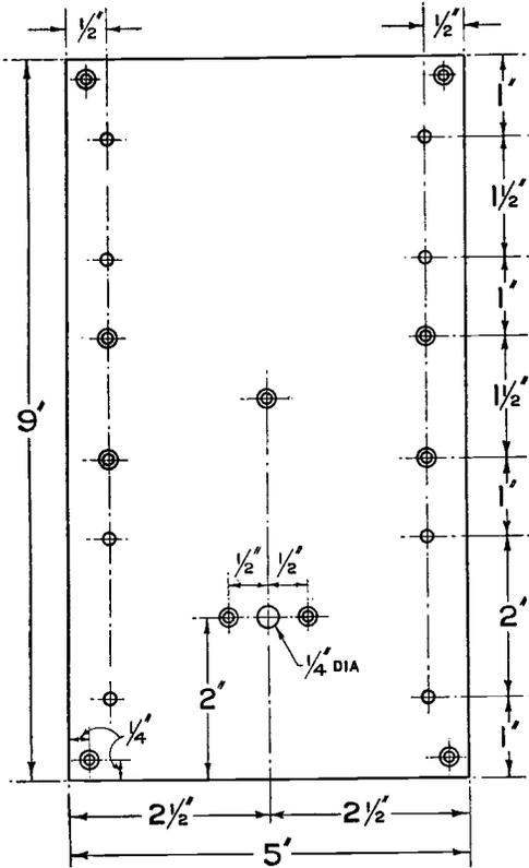
Fig. 1. Details for setting out the top panel.
