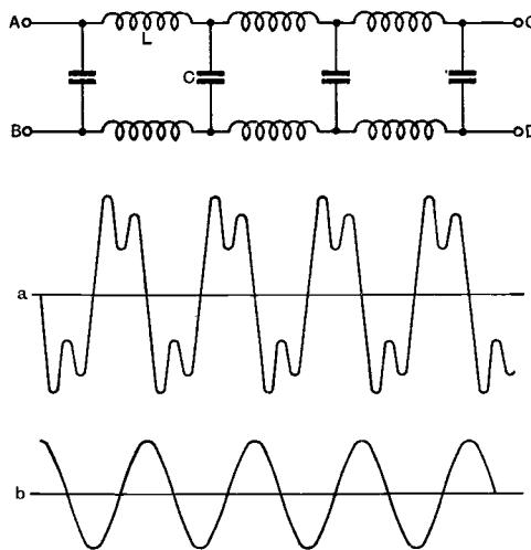
Fig. 15. An electric filter circuit which will remove overtones.
