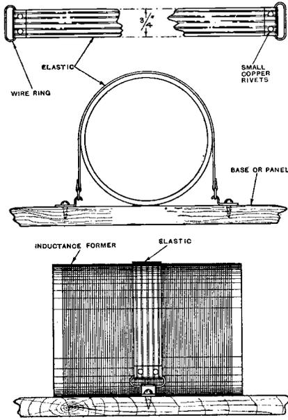
Coil fixing with elastic band.
