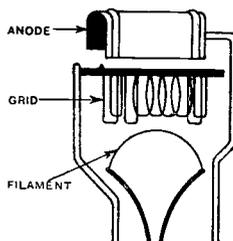
*Sketch showing details of the construction of the electrodes.*
