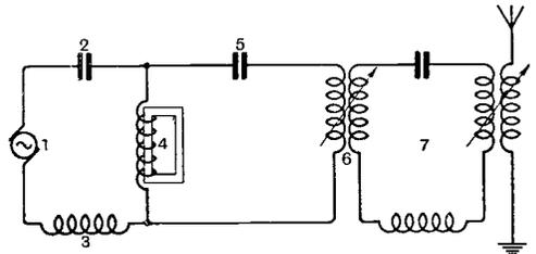
Fig. 2 Showing the use of a tuned circuit to reduce the strength of harmonics generated by the machine generator.
