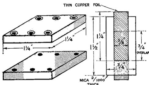
Fig. 4. Details for assembling the small condensers.
