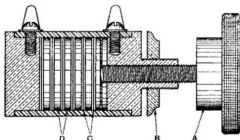
The "Oojah" rheostat. A is the knob, B the fixing nut, C the discs of copper foil, and D the resistance elements (graphite).
