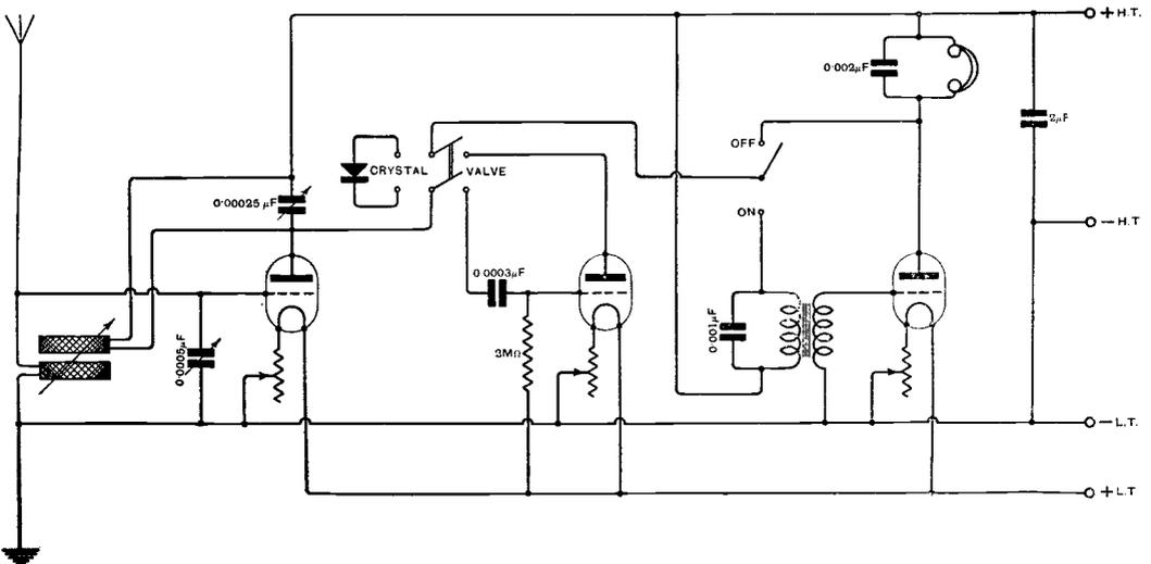
*A three-valve and crystal circuit.*
