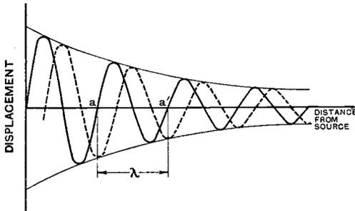
Fig. 6. Showing relationship between displacement and distance from the source of the sound wave.
