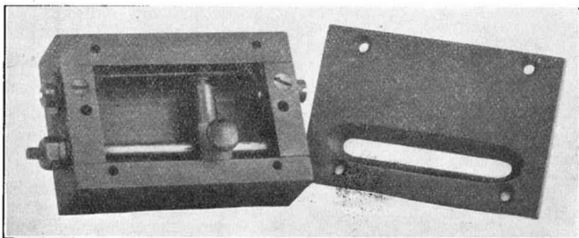
A potentiometer utilising a length of pencil graphite for the resistance element.
