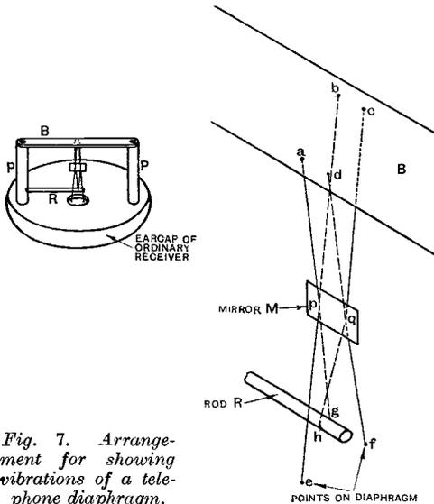
Fig. 7. Arrangement for showing vibrations of a telephone diaphragm.
