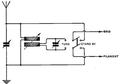
used as a wave trap on the absorption principle.
