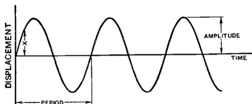
Fig. 4. Displacements of a sounding body producing a pure tone.
