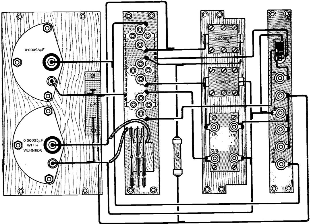
Fig. 6. Diagram of connections showing the actual points between which leads are run.
