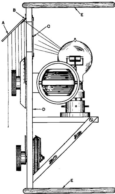
A mirror may be provided to reflect the light from the valve on to the tuning dial.
