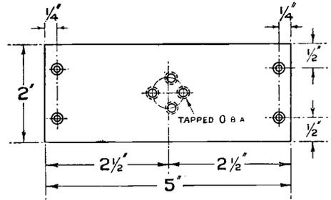
Fig. 5. The valve platform.
