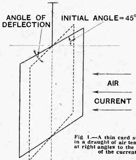
Fig. 1.—A thin card suspended in a draught of air tends to set at right angles to the direction of the current.
