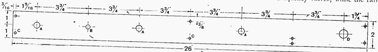
Fig. 4. Details of the ebonite strip for carrying the tuning and the balancing condensers. A, holes to take spindles of Ormond tuning condensers; D, for the Utility tuning condenser; B, for the Colvera balancing condenser; C,  $\frac{1}{8}$ in. dia. for No. 4 fixing screws to brackets.
