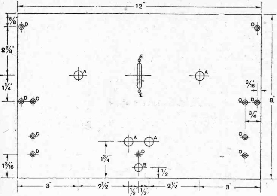
Drilling details of the front panel. A, 3/8in.; B, 7/16in.; C, 5/32in. and countersunk; D, 1/8in. and countersunk.
