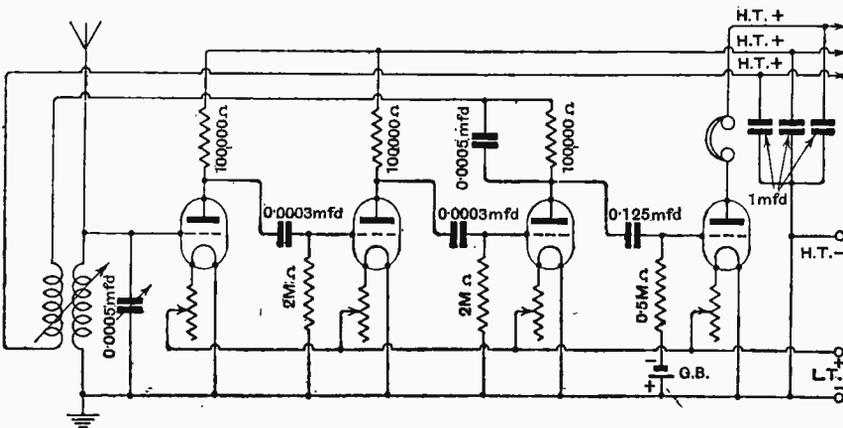
Fig. 3.—Four-valve receiver specially designed for the reception of Daventry and Radio-Paris.
