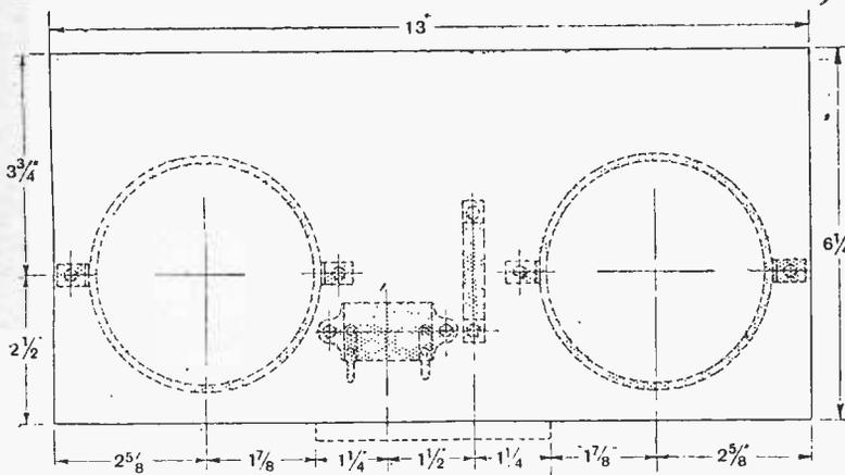
Fig. 5.—Plan view of the baseboard, showing the position of the parts.
