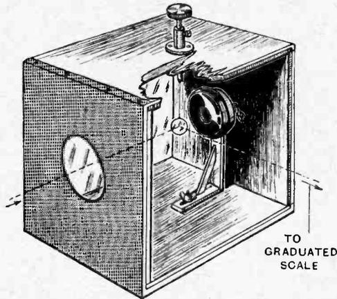
Fig. 5.—Experimental arrangement for testing telephone receivers.
