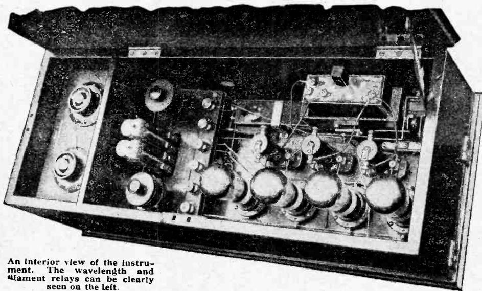
An interior view of the instrument. The wavelenght and filament relays can be clearly seen on the left.
