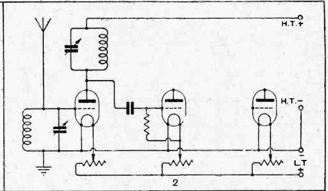
—connected in series with its anode a "tuned rejector" circuit, acting as a high resistance to oscillatory currents of the frequency to which it is tuned. Therefore, voltages are set up across it, and are applied to the grid of the detector valve through the condenser, which, in conjunction with the leak, effects rectification.
