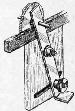
Device for marking spacing strips.
