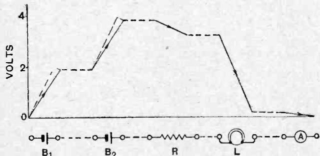
Fig. 4.—Potential gradients in the circuit of Fig. 3 illustrated graphically.
