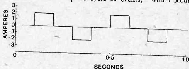
Fig. 5.—Wave-form of the current produced by the circuit in Fig. 4.
