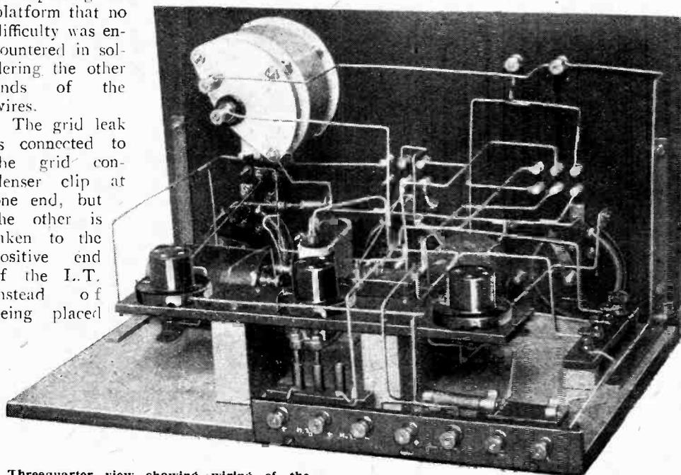
Threequarter view showing wiring of the change-over switches.
