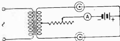
Fig. 1.—Connections of a full-wave electrolytic rectifier.
