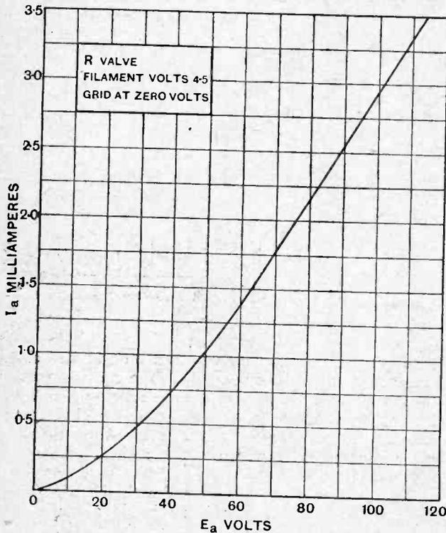
Fig. 4.—Anode volts—anode current characteristic of the valve used in these experiments.
