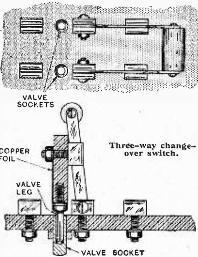
gram. The switch might be used to provide alternative connections to three loud-speakers, and there are innumerable other applications which
