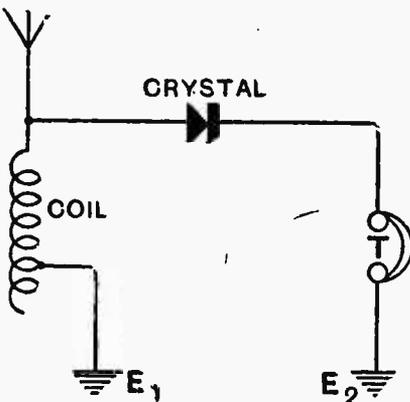
Fig. 1.—Circuit diagram of the receiver.  $E_1$  is a galvanised iron pipe, and  $E_2$  a brass rod. The cell formed by the two earth plates in contact with the soil provides the potential necessary for the carborundum detector, the crystal of which is connected to the aerial.
