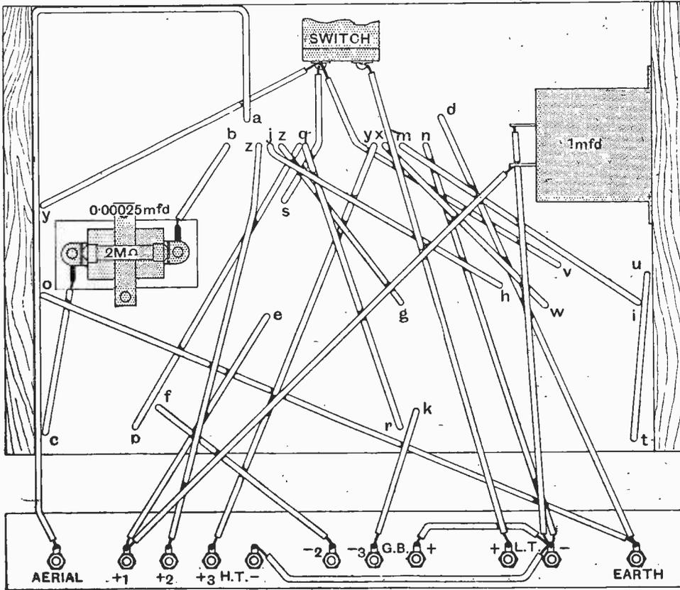
In conjunction with the diagram on the next page, the actual path taken by the various leads beneath the panel is shown.
