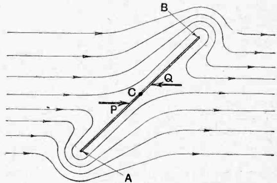
Fig. 2.—Forces acting on a card suspended in an air current at an angle of 45 degrees.
