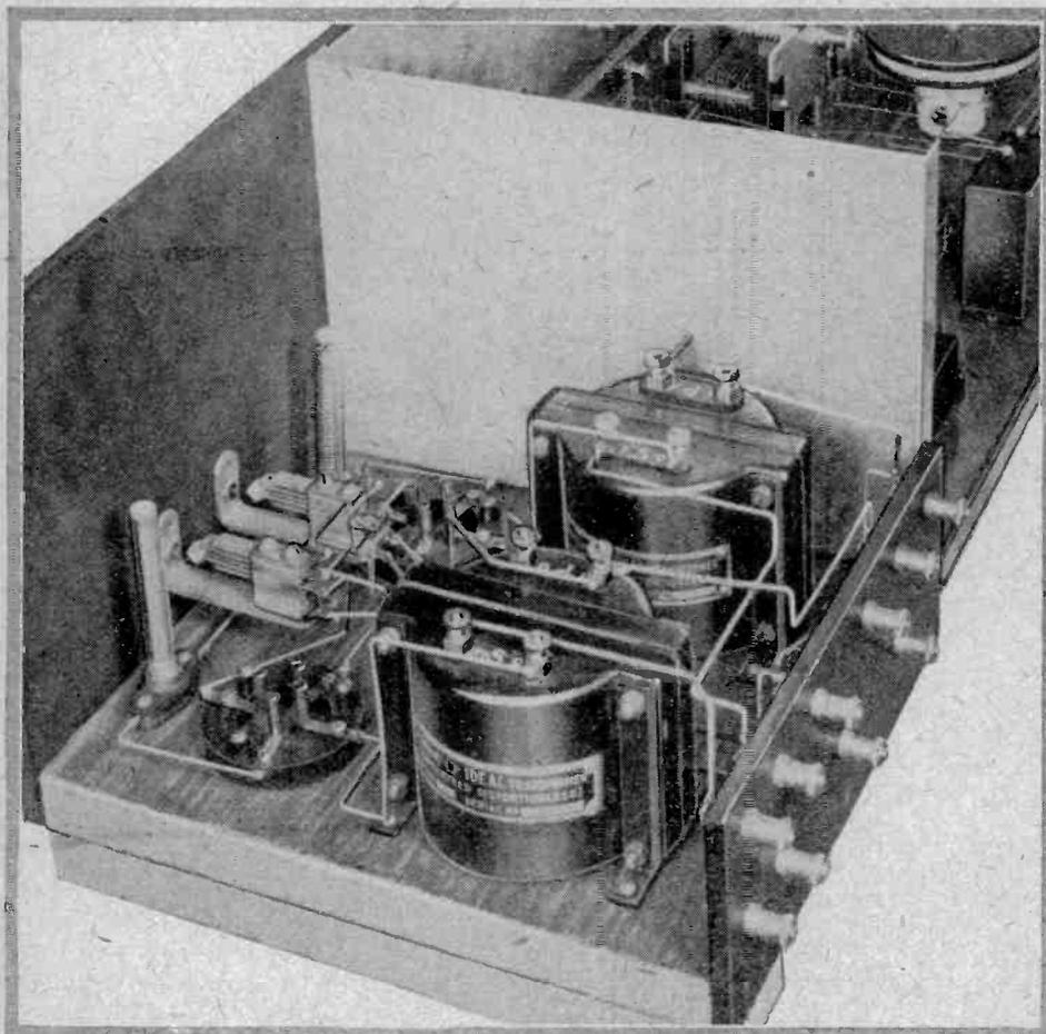
Fig. 5.—The audio-frequency amplifier portion of the receiver.
