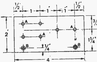
Fig. 6.—The terminal strip. A, 5/32in. and B, 1/8in. dia.
