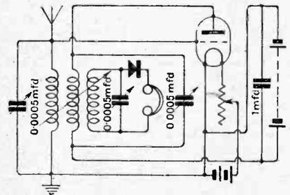
Fig. 1.—"Straight" valve-crystal circuit.
