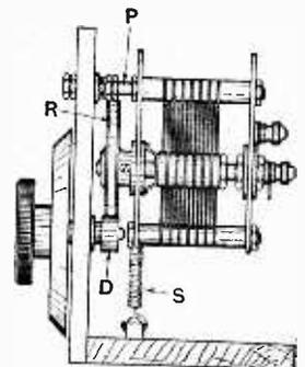
Vernier movement for condenser with compensated friction drive.
