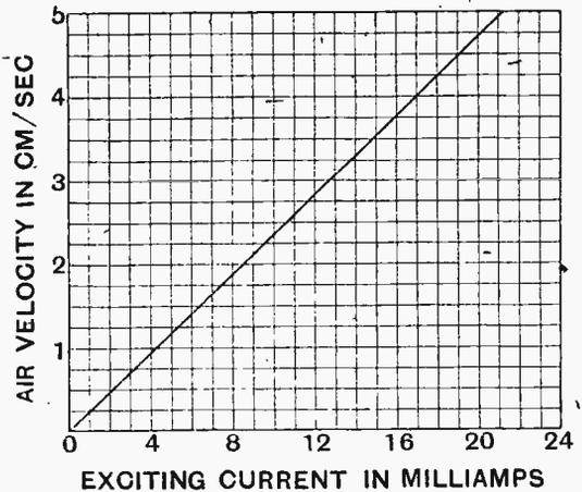
Fig. 4.—Curve showing relation between the air velocity and exciting current for a telephone receiver mounted in a resonator tube.
