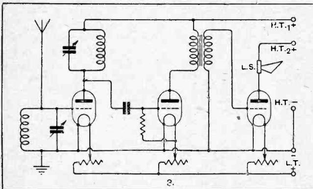
The plate circuit of the detector valve is completed through the primary winding of an L.F. transformer, the secondary of which is connected between grid and filament of the L.F. amplifying valve. Magnified pulses in the anode circuit of this valve operate the loud-speaker.
