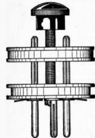
The Polar coil unit which provides variable reaction
