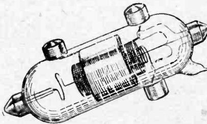
Tubular type four-electrode valve.
