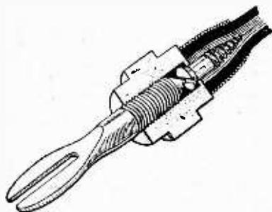
Spade terminal connection for heavy cables.
