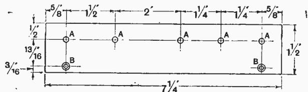
Fig. 3 —The terminal strip. A, 5/32in. dia.; B, 1/8in. dia., counter-sunk for No. 4 wood screws.
