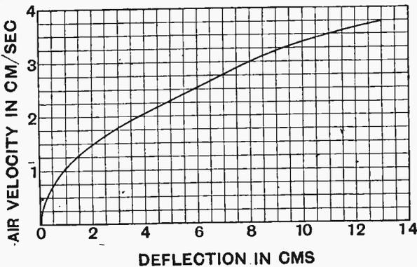
Fig. 3.—Calibration curve for Rayleigh disc
