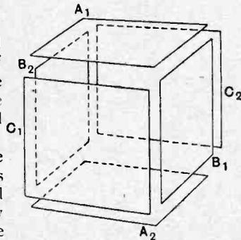
Fig. 4.—Six closed loops arranged mutually at right angles to screen a cubic space.
