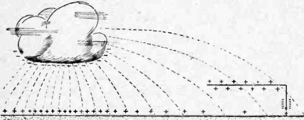
Fig. 4.—Negative charge induced on the upper electrode of a spark gap connected in the aerial down-lead.
