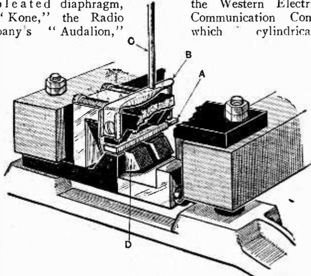
Fig. 9.—Sectional diagram of the "Kone" loud-speaker movement. Vibrations of the armature A corresponding to variations of current in the speech coils D are transmitted through a short metal rod to a spring lever B. The rod C is attached to the apex of the cone diaphragm.
