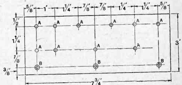
Fig. 3. The terminal strip. A, 5/32 in. dia.; B, 1/4 in. dia. and countersunk for No. 4 wood screws
