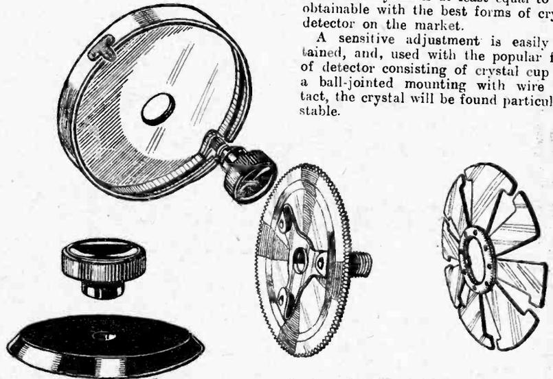
Component parts of the Wilkins & Wright vernier dial showing the friction spring plate with centre ball race and the interesting arrangement making use of three balls in a spring mount for producing an additional half reduction gearing between the condenser spindle and the toothed disc.
