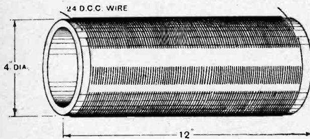
Fig. 2.—Dimensions of the aerial tuning coil.
