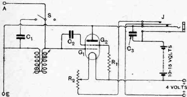
Fig. 1.—Circuit diagram. The connections are similar to those of the Numans oscillator.
