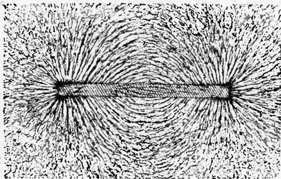
Fig 1.—Lines of magnetic force surrounding a magnet as revealed by iron filings.
