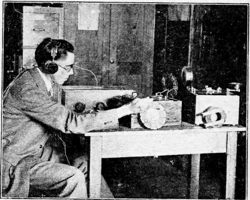
**TESTING BROADCAST FREQUENCIES** Considering the extraordinary number of broadcasting stations in America it is not surprising that interference presents a difficult problem. Mr. M. S. Stroek, of the U.S. Bureau of Standards, is seen in the photograph with a device of his invention for checking the frequencies of distant stations. Doubt exists as to whether stations digress from their allotted wavelengths.
