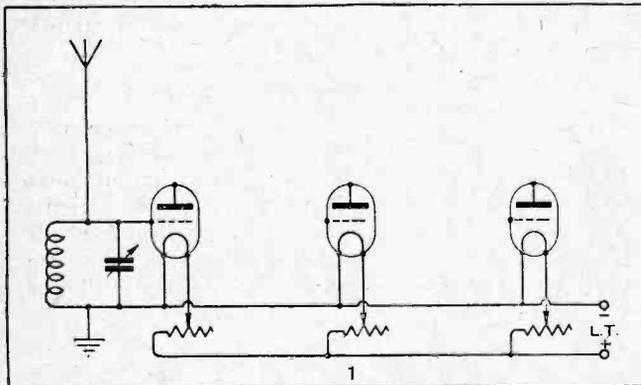
Three valves, connected in the usual manner across a filament battery, with rheostats in series with each filament. Voltages built up across an oscillatory circuit, connected to aerial and earth, are applied between grid and filament of the H.F. valve, which has—
