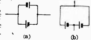
Fig. 8.—Cells incorrectly connected in parallel, resulting in the complete discharge of both cells.
