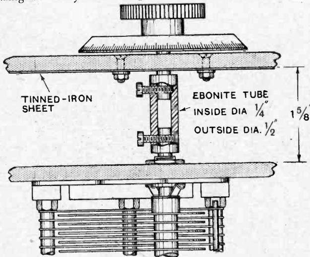
Fig. 2. Details of the method of mounting the tuning condensers and of fixing the ebonite distance pieces.
