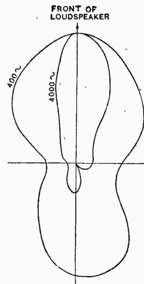
Fig. 19.—Polar curves of sound distribution round the G.E.C. small cone loud-speaker at frequencies of 400 and 4,000 cycles.
