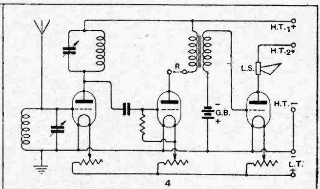
Here a few refinements are introduced. Provision is made for the insertion of a reaction coil at R, while a fixed negative bias is impressed on the grid of the L.F. valve by the inclusion of a battery, G.B. Note that a separate H.T. terminal is provided for the last valve.
