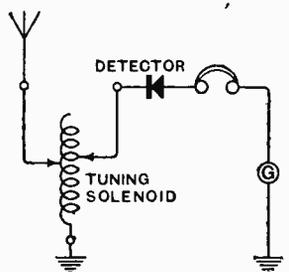
Fig. 21.—Crystal receiver for large signal amplitudes.
