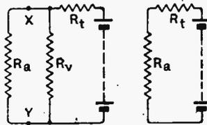
Fig. 2.—Analysis of the circuit in Fig. 1. The right-hand diagram shows the voltmeter disconnected.
