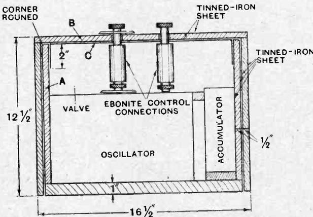
Fig. 8.—Sectional elevation of screened oscillator, showing control connections.
