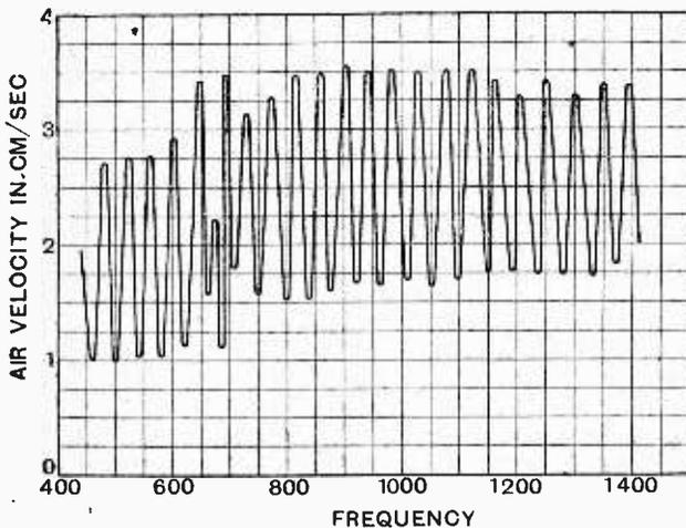
Fig. 10.—Resonance curve of the loud-speaker of Fig. 9, with a 15ft. tube 3/4in. in diameter substituted for the horn.
