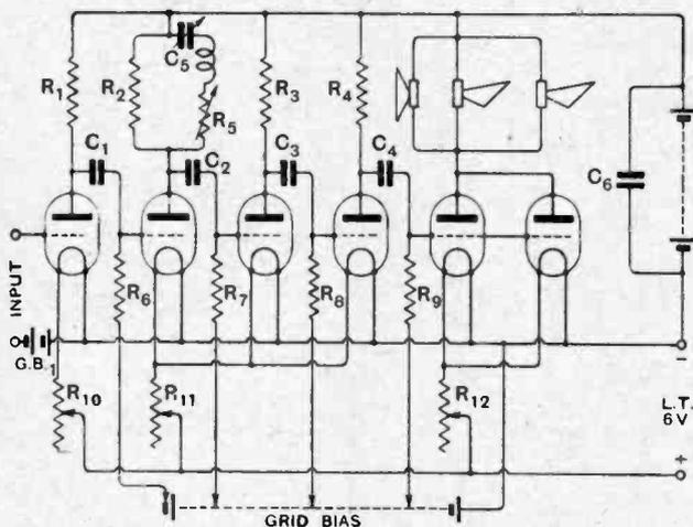
Fig 3.—Circuit connections of an amplifier specially designed for the electrical reproduction of gramophone records.
