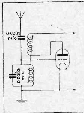
Reaction coupling sharpens the tuning by reducing the damping in the aerial circuit
