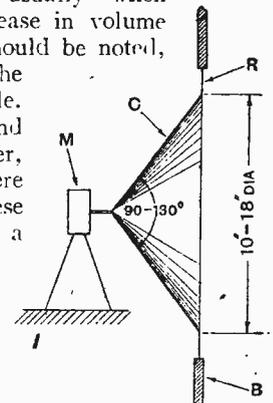
Fig. 12.—Typical example of the "free-edge" cone principle of construction. The cone C of cartridge paper from 5 to 10 mils thick is supported in a sound baffle B from 2 to 4ft. square by a thin sheet rubber ring R. The cone is driven through the medium of a short thin rod by a magnetophone or reed type movement M.
