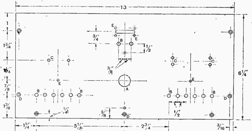
Fig. 3.—Details of the front ebonite panel. A, 11/16in. dia.; B, 3/16in. dia.; C, 5/32in. dia.; D, 1/8in. dia. and countersunk; E, 1/8in. dia.
