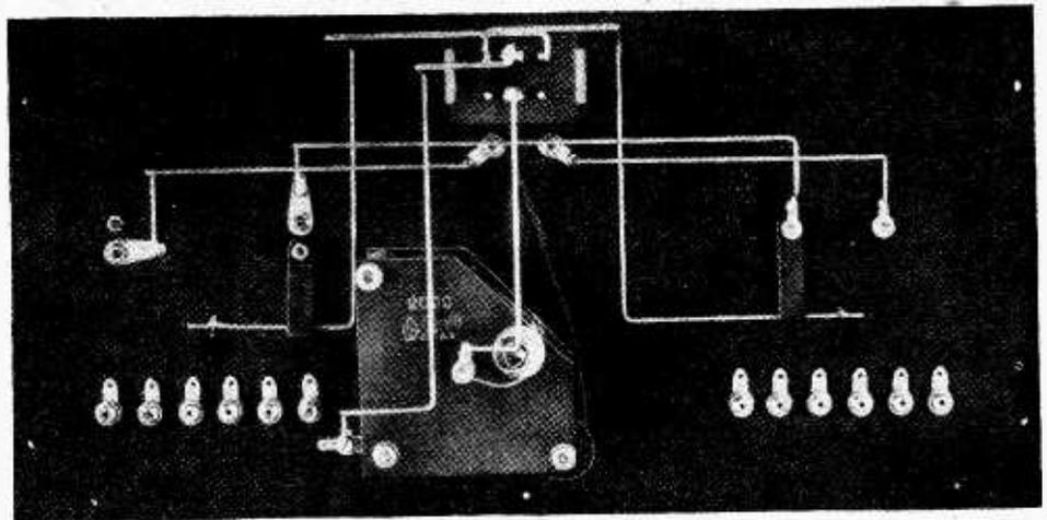
Fig. 7.—View of the panel with some of the wires in position. Notice the two ebonite cleats holding the two stiff wires to which the flexible wires are soldered.
