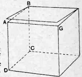
Fig. 5.—Faulty screen in which only the end surfaces are effective in screening fields perpendicular to A B C D.
