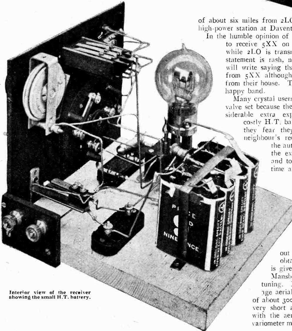
Interior view of the receiver showing the small H.T. battery.
