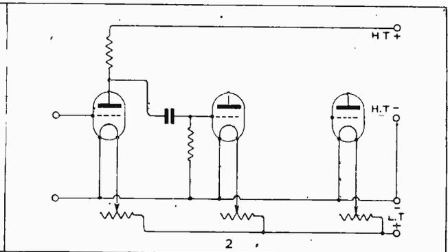
The anode-circuit of this valve is completed through a resistance and high-tension battery. Amplified differences of potential across this resistance are communicated to the grid-filament circuit of the second valve through a condenser provided with a leak.
