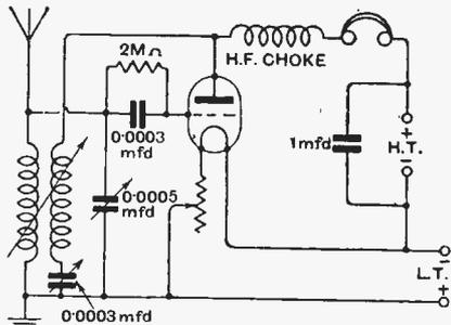
Fig. 1.—Combined capacity and magnetic reaction.
