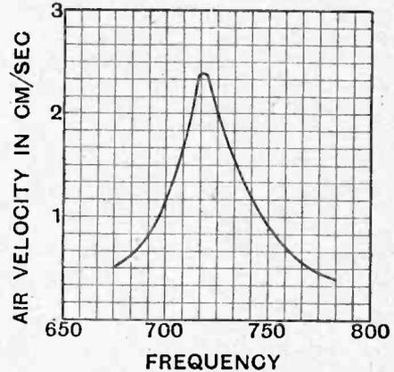
Fig. 7.—Air velocities produced by a telephone receiver when supplied with the same value of current at different frequencies.
