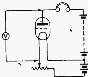
Fig. 1.—A simple and direct method of measuring anode potential, which is, however, subject to error when a voltmeter of finite resistance is used.
