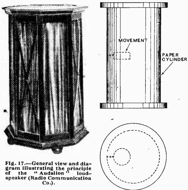
Fig. 17.—General view and diagram illustrating the principle of the "Audalton" loud-speaker (Radio Communication Co.).
