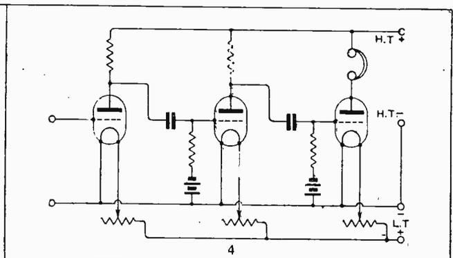
Here the amplifier is modified to deal with low frequencies. Coupling condensers and leaks of suitable values are used, while grids are biased negatively. The last valve will be of a type capable of handling a considerable amount of power.
