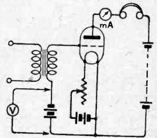
Fig. 5.—Circuit connections for measuring the anode voltage in terms of the grid voltage and anode current.
