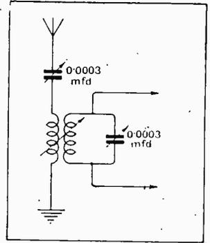
A highly selective receiving circuit with separately tuned aerial and closed circuits, and variable coupling between the coils.
