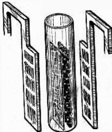
A cell from the Mars H.T. accumulator, type "C."
