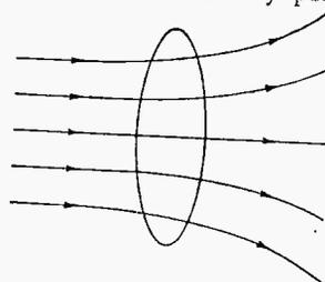
Fig. 1.—The magnetic field threading a conducting ring is opposed by the current which it induces in the ring.
