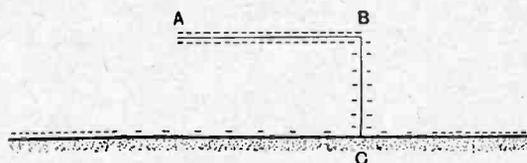
Fig. 1.—Distribution of the negative charge on an aerial and surrounding ground during fine weather.
