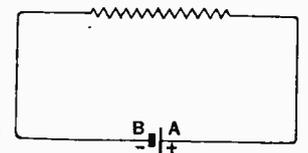
Fig. 2.—The current in the circuit external to the battery flows from A, which is a point of positive or high potential, to B, a point of negative or low potential.
