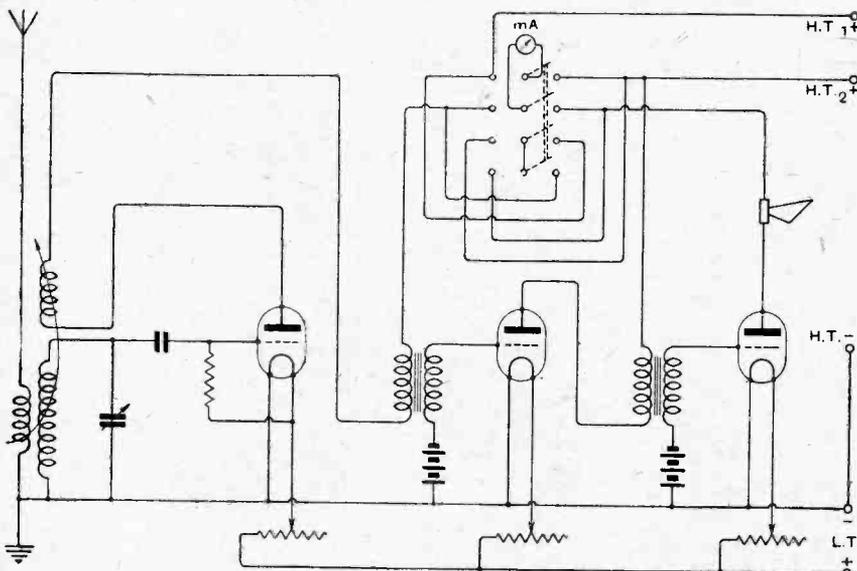
Fig. 1.—Connections for a plate milliammeter.
