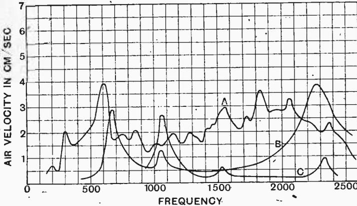
Fig. 9.—Frequency characteristics of a horn type loud-speaker. A, at the mouth of the horn; B, at the mouth of the nozzle with horn removed; C, at the diaphragm with nozzle removed.
