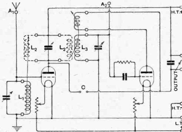
Four-circuit two-valve receiver.
