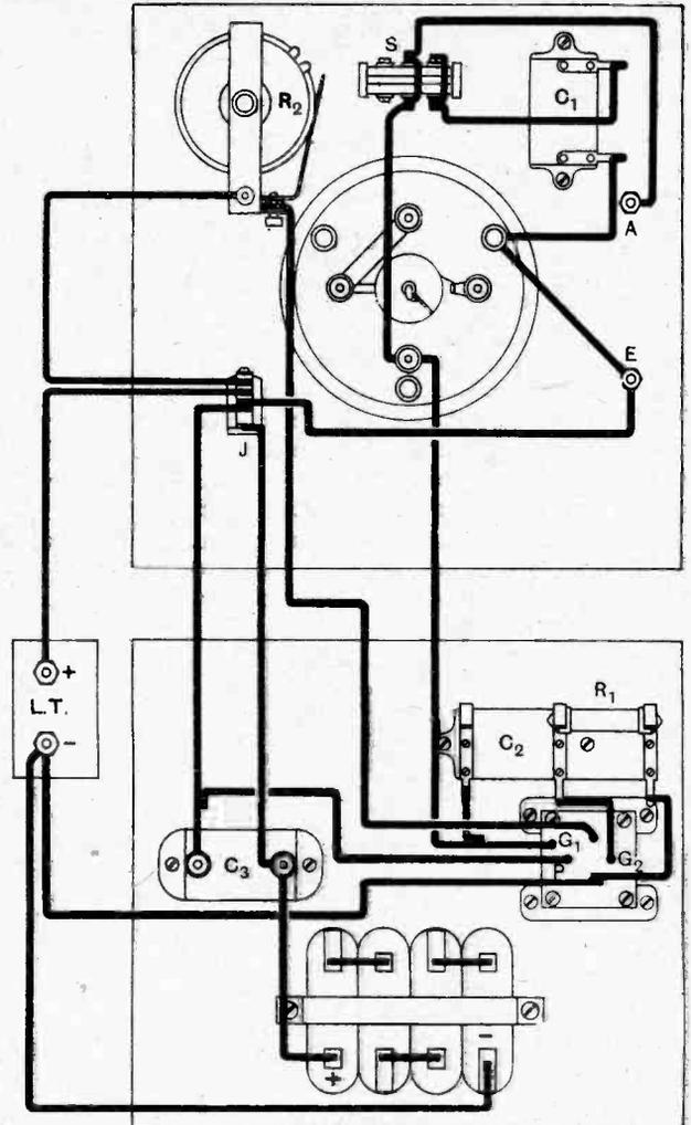
Fig. 2.—Practical wiring diagram.
