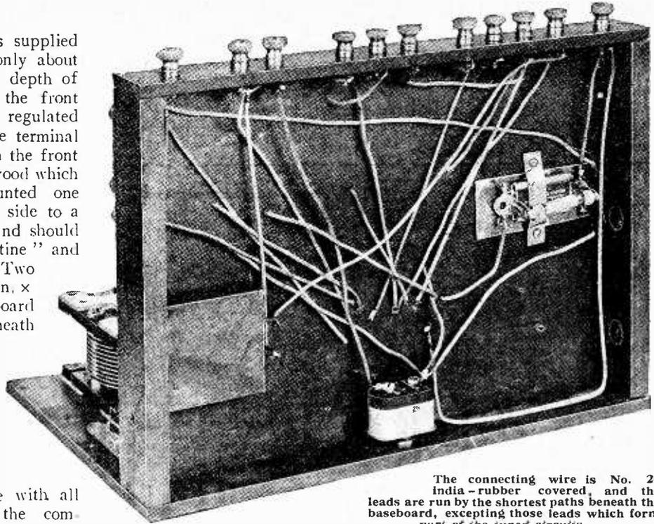
The connecting wire is No. 20 india-rubber covered, and the leads are run by the shortest paths beneath the baseboard, excepting those leads which form part of the tuned circuits.
