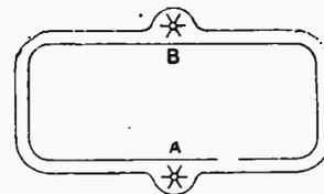
Fig. 3.—Hydraulic circuit illustrating the transfer of energy by direct and alternating currents.
