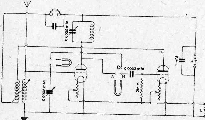
Fig. 3.—Switching H.F. receiver circuits.
