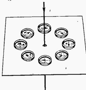
Fig. 3.—Small compass needles arranged to give an indication of the magnetic field surrounding an electric current.
