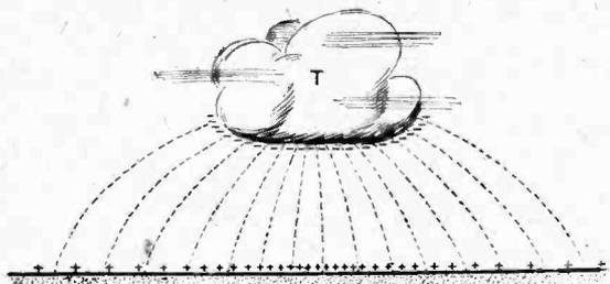
Fig. 2.—Positive charge induced on the earth's surface by a negatively charged thundercloud.
