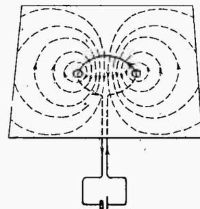
Fig. 4.—Magnetic field produced by an electric current flowing in a single turn of wire.
