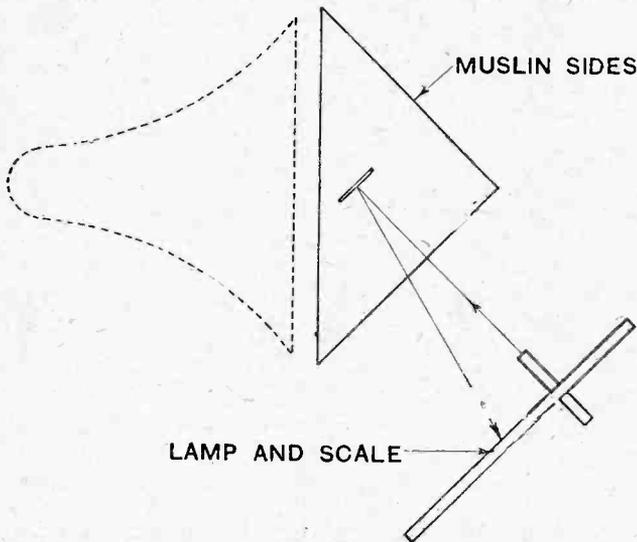
Fig. 6.—Method of setting up the apparatus to test loud-speakers. In this case a screening box of triangular section is used.
