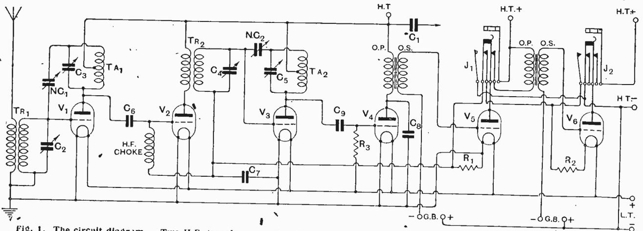
Fig. 1. The circuit diagram. Two H.F. transformers,  $TR_1$ ,  $TR_2$ , and two tuned anode circuits,  $TA_1$ ,  $TA_2$ , are used.  $C_2$ ,  $C_3$ ,  $C_1$ ,  $C_4$  = 0.0005 mfd.;  $NC_1$ ,  $NC_2$ , neutrodyne condensers;  $C_5$ ,  $C_6$  = 0.00025 mfd.;  $C_7$  = 0.005 mfd.;  $C_8$  = 2 mfd.;  $C_9$  = 0.0005 mfd.;  $R_1$ ,  $R_2$  = fixed resistors;  $R_3$  = 1 megohm grid leak.
