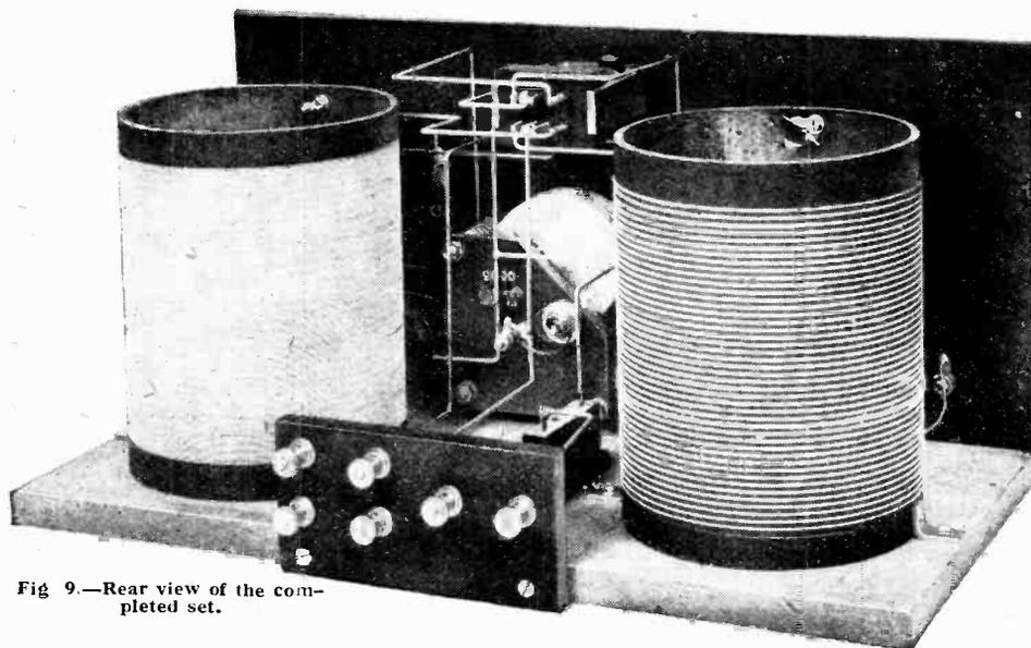
Fig. 9.—Rear view of the completed set.
