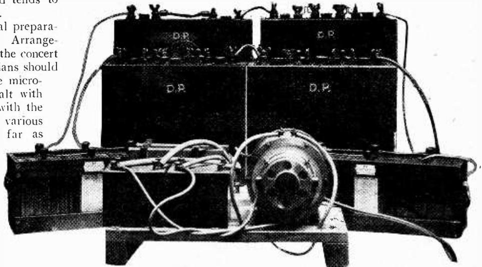
High tension generator and batteries installed in the cabin.
