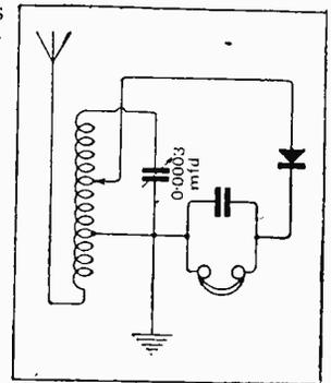
This is virtually a loose-coupled circuit in which the loss of selectivity brought about by connecting the crystal and telephones across the coil tuning inductance is limited by making use of a tapping point on the coil.
