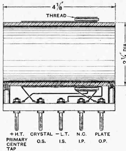
Fig. 4.—The short wave H.F. transformer shown in section. Connections of the winding to the pins and the ultimate connections to the remainder of the circuit are given.
