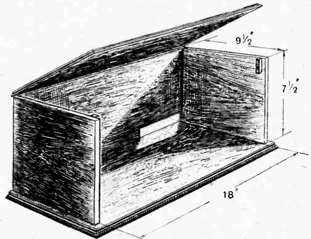
Fig. 6.—Cabinet for the receiver. Note slot cut out of the back to accommodate the terminal strip.
