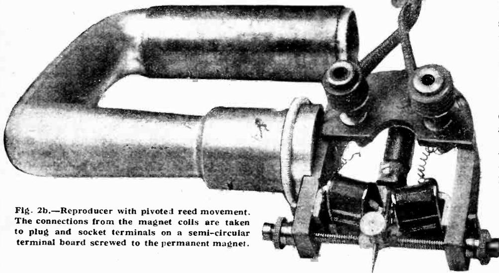
Fig. 2b.—Reproducer with pivoted reed movement. The connections from the magnet coils are taken to plug and socket terminals on a semi-circular terminal board screwed to the permanent magnet.
