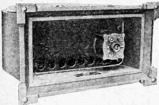
Fig. 6.—View under the base of the "Radiolux" loud-speaker, showing position of adjustable movement.
