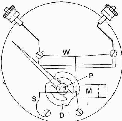
Principle of the hot-wire ammeter. W, heater wire; P, pulley; S, control spring; D, damping disc; M, damping magnet.
