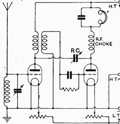
Fig. 2.—Capacity-controlled reaction.
