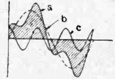
Resultant curve *a* produced by the combination of a sine wave *b* and its third harmonic *c*.
