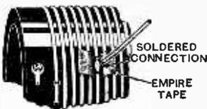
Fig. 2.—Method of tapping the coils.
