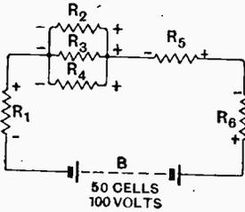
Fig. 6.—In this circuit the resistances R<sub>2</sub>, R<sub>3</sub> and R<sub>4</sub> are connected in parallel, the unit so formed being connected in series with the remaining resistances R<sub>1</sub>, R<sub>5</sub> and R<sub>6</sub>.
