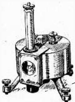
Suspended coil galvanometer.
