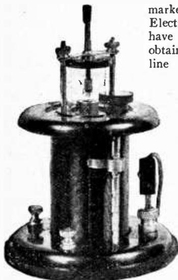
Goltone crystal receiving set. By means of a plug and socket switch the wavelength can be extended for reception on wavelengths up to 1,850 metres.
