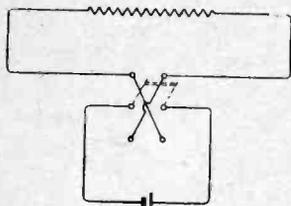
Fig. 4.—Switching arrangement for reversing the direction of current in a circuit
