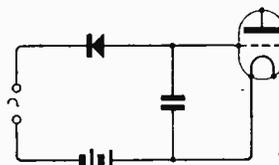
Fig. 23.—Crystal detector connected for potential rectification.
