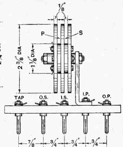
Fig. 5.—The long wave H.F. transformer. The markings correspond to the connections between the pins and the windings.
