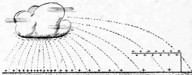
Fig. 3.—Distribution of induced charge on an inverted L aerial connected to earth.
