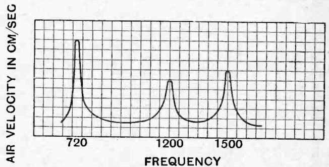
Fig. 8.—Typical telephone characteristic, showing the principle resonance at a frequency of 720, and subsidiary resonances at 1,200 and 1,500.
