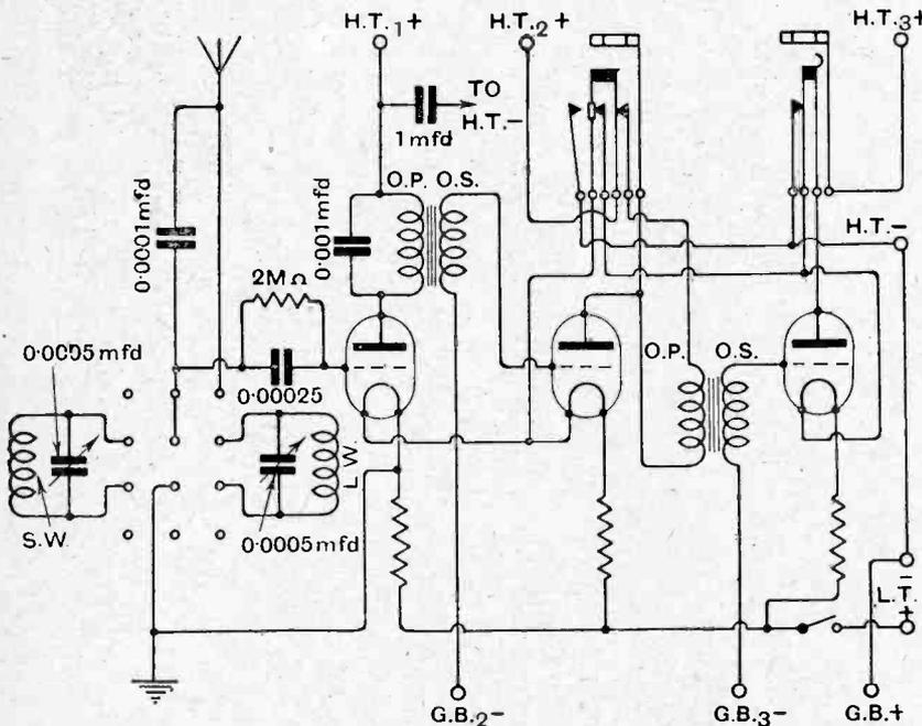
The tuning apparatus is duplicated, providing a choice of two transmissions by the action of a two-position switch. The additional contacts on the change-over switch may, if desired, be connected to fixed reaction coils arranged near the long and short wave tuning inductances. By means of plugs and jacks, one of the amplifying valves may be removed from circuit.
