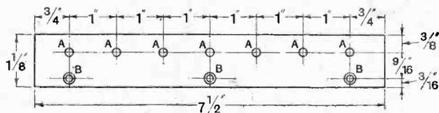
Fig. 4.—The terminal panel. Sizes of holes are as follow: A, 5/32in. dia.; B, 1/8in. dia., and countersunk for No. 4 wood screws.
