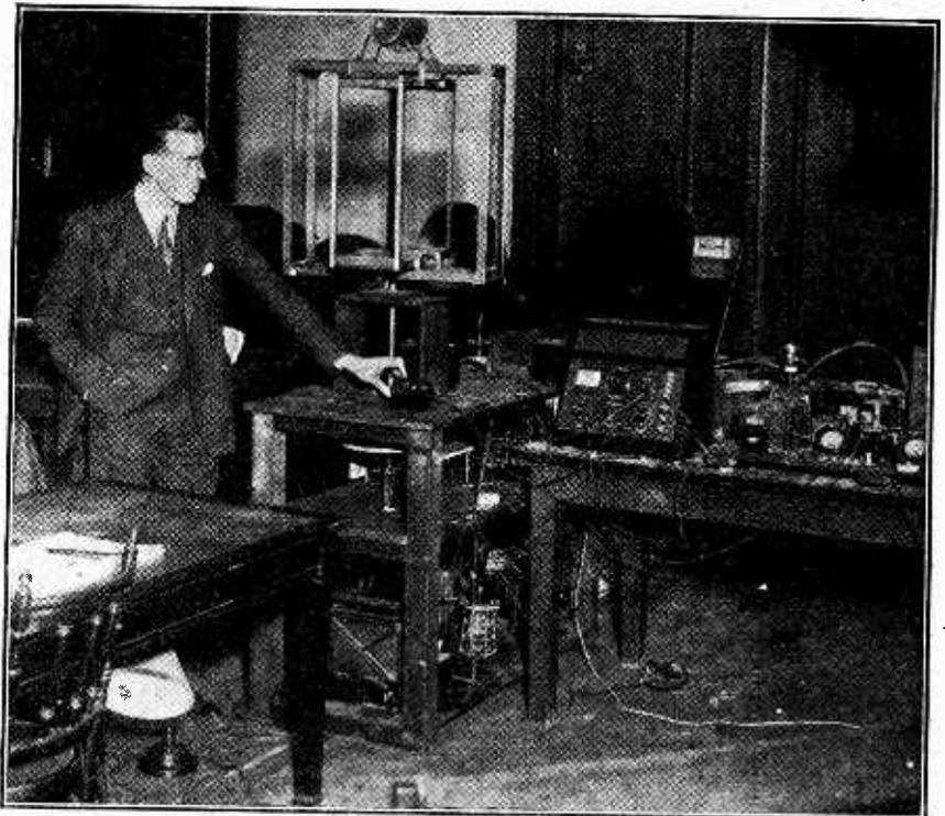
**AUTOMATIC DIRECTION FINDER.** Major Basil Binyon demonstrating his new D.F. instrument before the Wireless Section of the Institution of Electrical Engineers. The device automatically points in the direction of a distant transmitting station, and its value to navigators would thus be immense.
