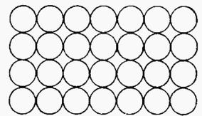
Fig. 2.—A series of rings arranged to screen a plane area from a varying magnetic field.
