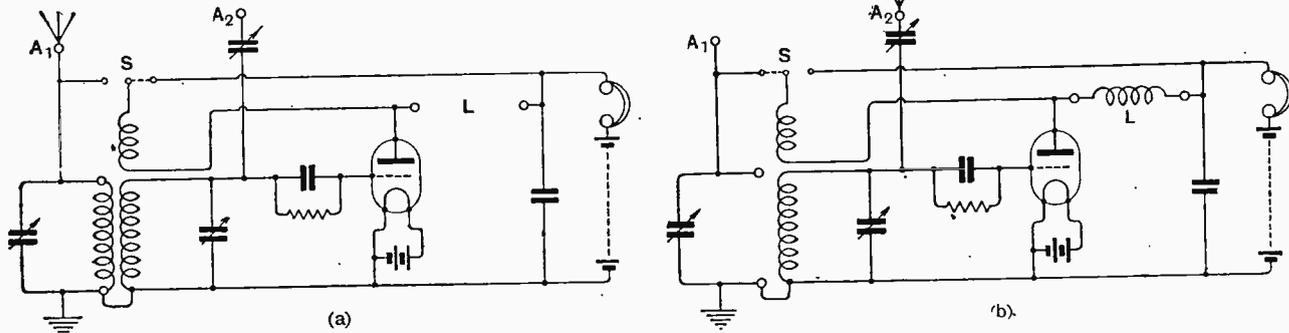
Circuit connections of a single-valve receiver arranged to give (a) a simple reacting single-valve set with coupled tuner and (b) a modified Reinartz circuit.
