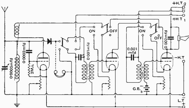
Fig. 1.—Diagram showing the switching arrangements for changing the circuit connections.
