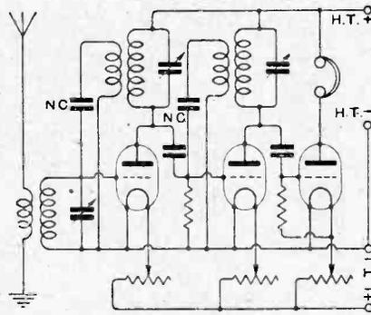
Fig. 2.—A neutralised H.F. amplifier.
