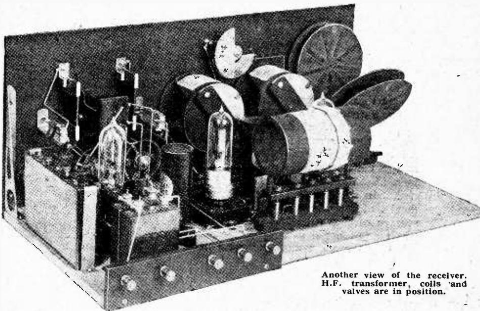
Another view of the receiver. H.F. transformer, coils and valves are in position.
