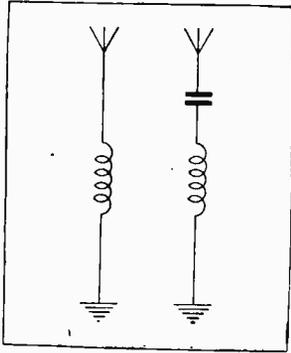
A variable condenser connected in the aerial lead sharpens the tuning of the aerial circuit, reduces jamming, and usually brings about an increase in signal strength, though if used with an oscillating valve set renders oscillation control erratic.
