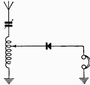
Fig. 22.—Circuit suitable for crystal reception of weak signals.
