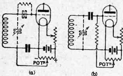
Alternative connections of grid potentiometer.
