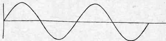
Fig. 6.—A more usual wave-form for alternating currents—the sine wave.
