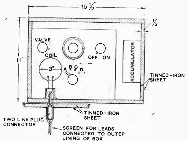
Fig. 7.—Sectional plan of screened oscillator, showing method of leading out telephone connections.
