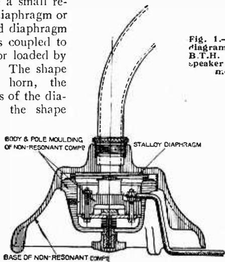
Fig. 1.—Sectional diagram of the B.T.H. loud-speaker movement.
