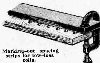
Marking-out spacing strips for low-loss coils.
