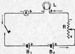
Fig. 3.—Simple electrical circuit. The lamp L is rated at 3 volts and 6 watts, and the two cells have each an e.m.f. of 2 volts.
