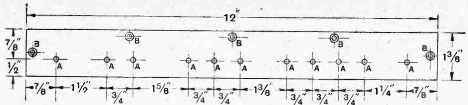
The terminal strip is drilled with  $\frac{5}{32}$ in. holes for the terminals and countersunk  $\frac{1}{16}$ in. holes for the securing screws.
