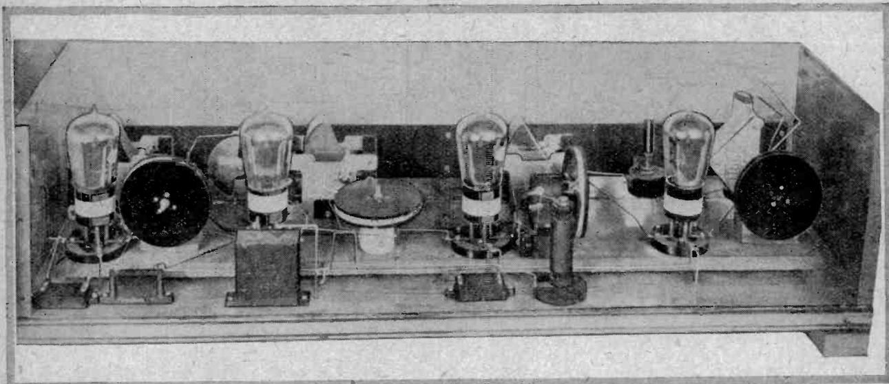
Fig 4.—View of the right-hand end of the set looking at the back. Most of the high-frequency amplifier can be seen.
