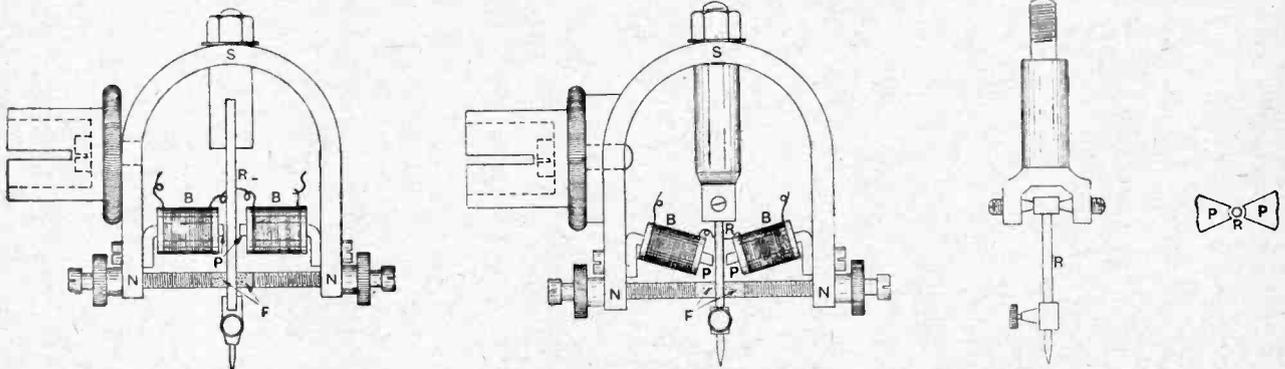
Fig. 1.—Two experimental reproducers fitted (left) with flat clamped reed and (right) with pivoted cylindrical reed.
