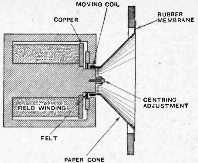
Fig. 15.—Section of the driving mechanism of the small cone loud-speaker.
