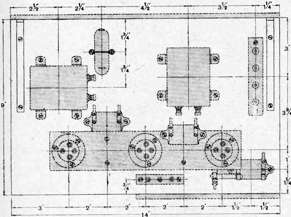
Fig. 3.—Layout of components on the baseboard and valve panel.
