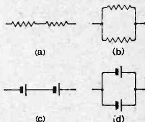
Fig. 5.—Resistances and batteries in series—(a) and (c), and in parallel—(b) and (d).
