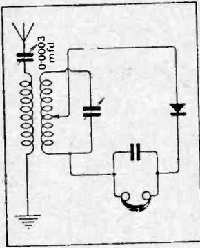
Selective crystal circuit in which two tuning adjustments are provided, as well as a tapping point on the coil.
