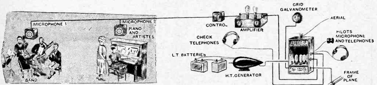
Schematic diagram showing the arrangement of the microphones and apparatus.
