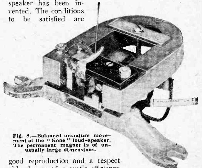
Fig. 8.—Balanced armature movement of the "Kone" loud-speaker. The permanent magnet is of unusually large dimensions.
