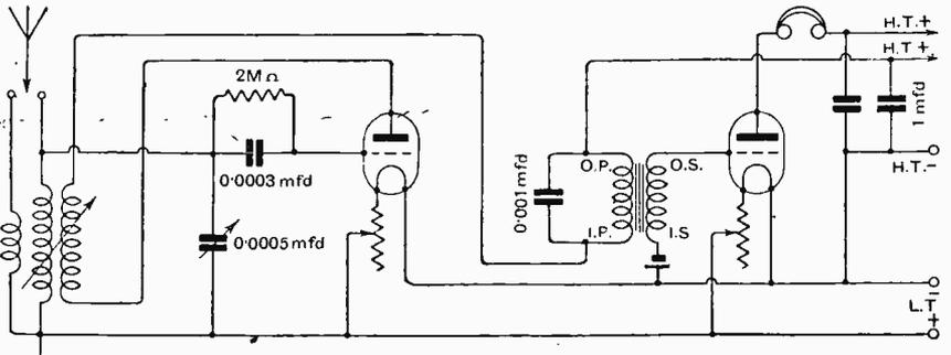
Fig. 3. — Alternative "aperiodic" and direct coupling in the aerial circuit.
