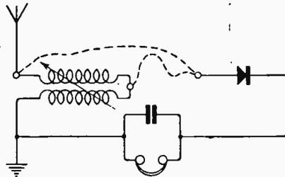
Fig. 2.—Alternative crystal connections.
