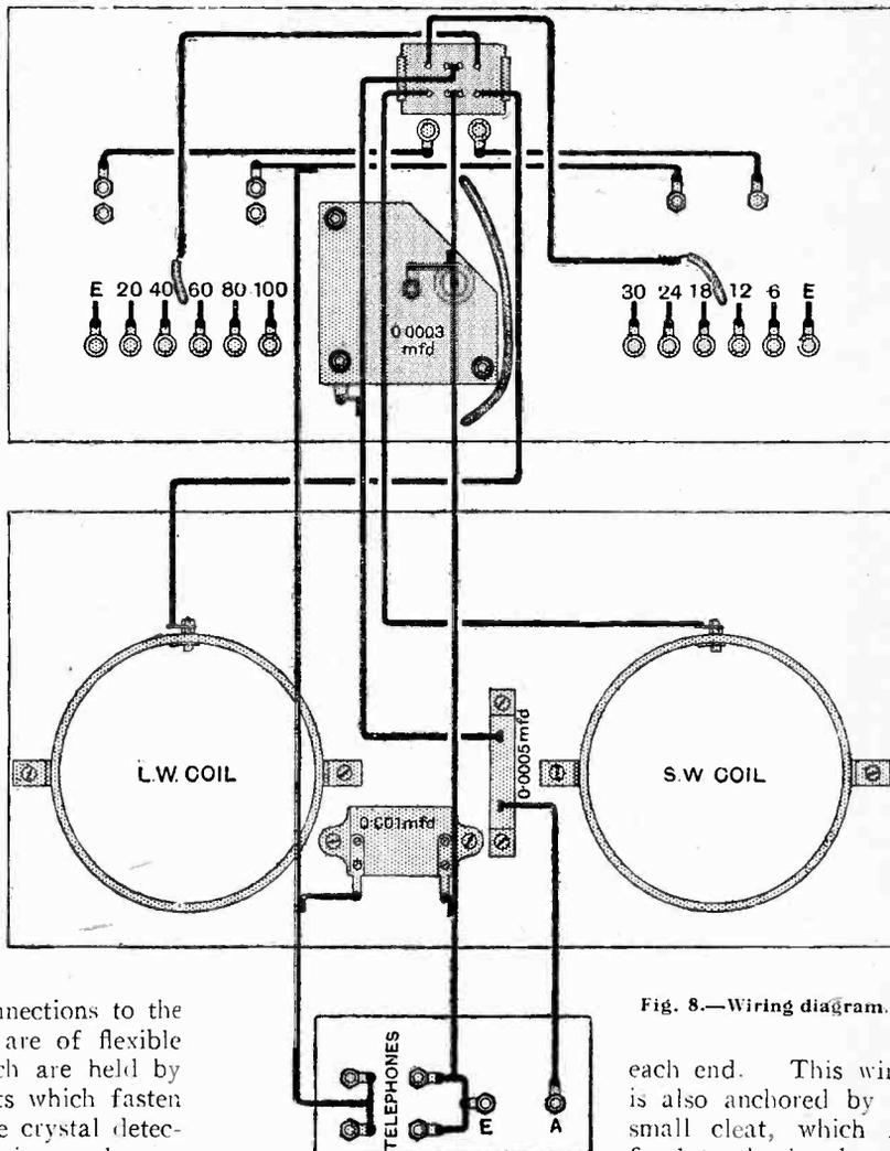
Fig. 8.—Wiring diagram.
