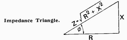
angled triangle, the two sides adjacent to the right angle representing R and X respectively, and the side opposite (the hypotenuse) representing Z. If φ is the angle opposite the side representing X,  $\tan \phi = X/R$  (see ALTERNATING CURRENT CIRCUITS),
