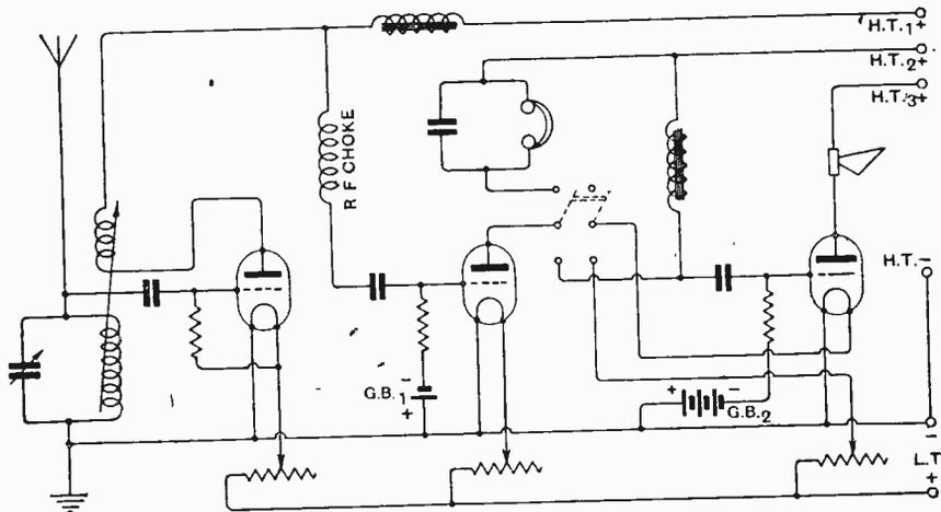
Fig. 1.—Switching from telephones to loud-speaker.
