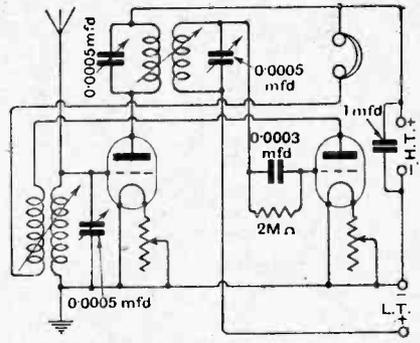
Fig. 2.—Two-valve receiver (H.F. and det.) with tuned transformer coupling.
