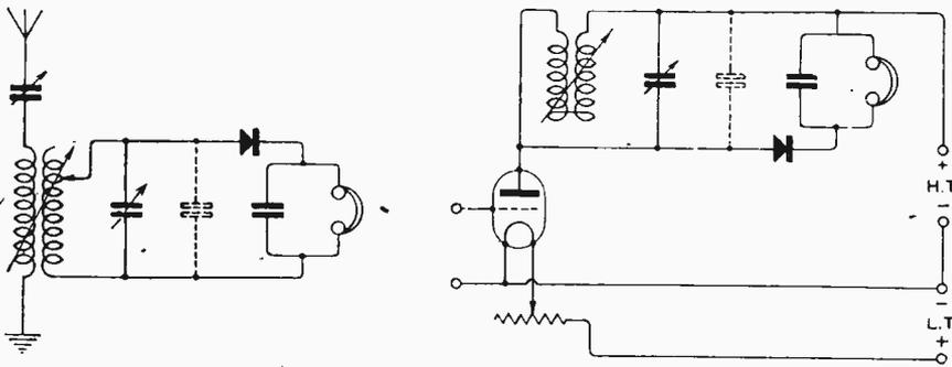
Fig. 1.—Reduction of damping in crystal circuits.
