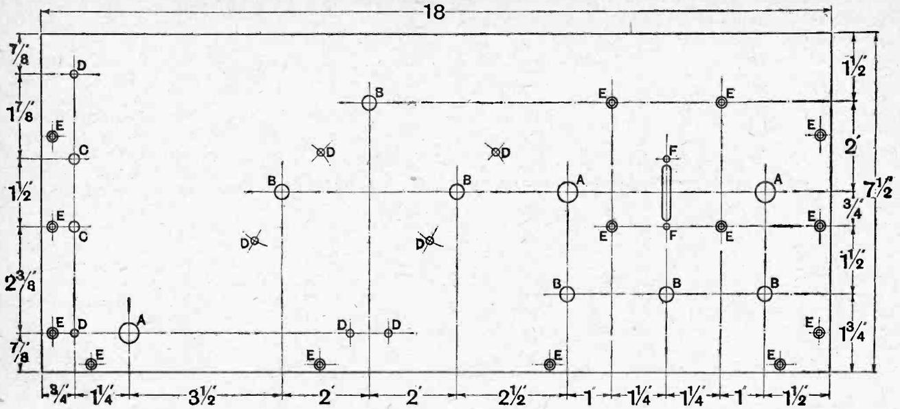
Fig. 1.—Drilling details of front panel. Sizes of holes are as follow : A, 7/16in. dia. ; B, 5/16in. dia. ; C, 7/32in. dia. ; D, 5/32in. dia. ; E, 1/8in. dia. coun.ersunk for No. 4 wood screws ; F, 1/8in. dia.
