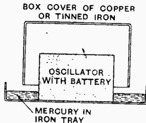
Fig. 6.— Experiment to show that screening is not complete until the screening box is completely closed
