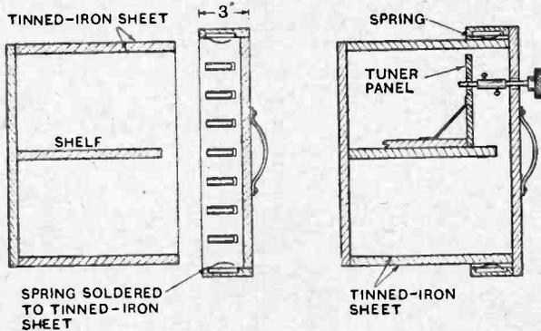
Fig. 11.—Screening box with spring contacts between the metal-covered lid and sides.
