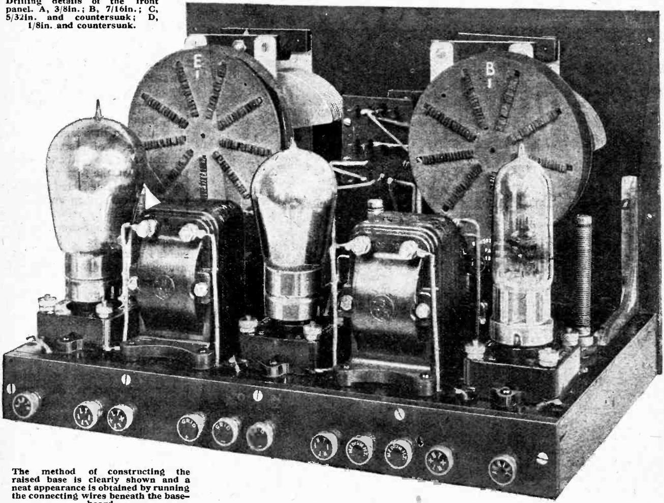
The method of constructing the raised base is clearly shown and a neat appearance is obtained by running the connecting wires beneath the base-board.
