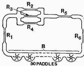
Fig. 7.—Hydraulic analogy to the circuit of Fig. 6.
