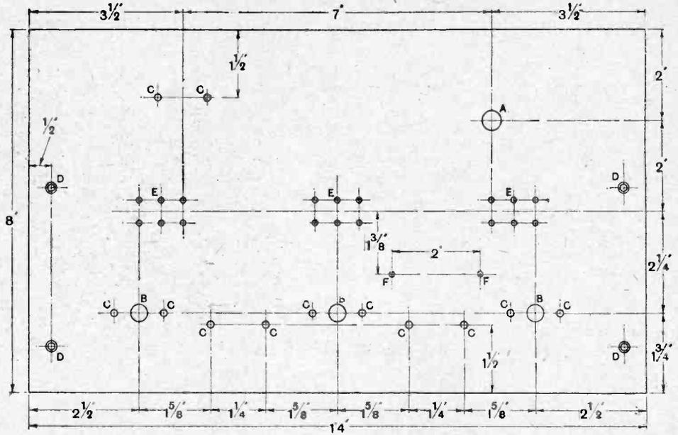
Fig. 2.—Drilling details of the front panel. Sizes of holes are as follow: A, 7/16 in. dia.; B, 3/8 in. dia.; C, 5/32 in. dia.; D, 5/32 in. dia. and countersunk for No. 4 B.A. screws; E, 1/8 in. dia.; F, 7/64 in. dia., tapped for No. 4 B.A.
