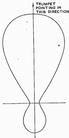
Fig. 18.—Rough sound distribution curve for a typical horn type loud-speaker.
