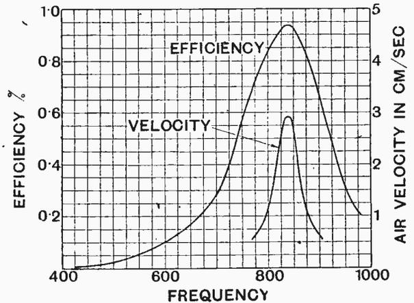
Fig. 11.—Variation with frequency of the air velocity and efficiency in a telephone receiver.
