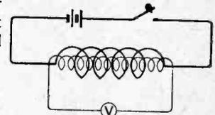
Fig. 6.—Simple circuit illustrating the principle of the induction coil.
