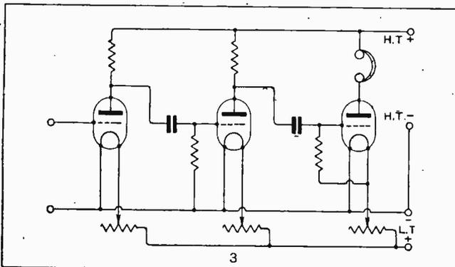
The same procedure is repeated in the case of the plate circuit of the second valve and the grid circuit of the third valve, except that the leak is connected to give a positive grid bias for detection; 'phones in the output circuit.
