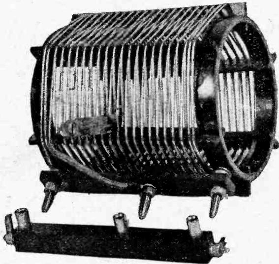
The Baltic low-loss coil. The winding, which is about 4in. in diameter, consists of 40 turns, giving an inductance of 98.5 microhenries, with a natural wavelength of 31.5 metres, and when bridged with a parallel capacity of 0.00055 mfd. a wavelength of 425 metres is produced.
