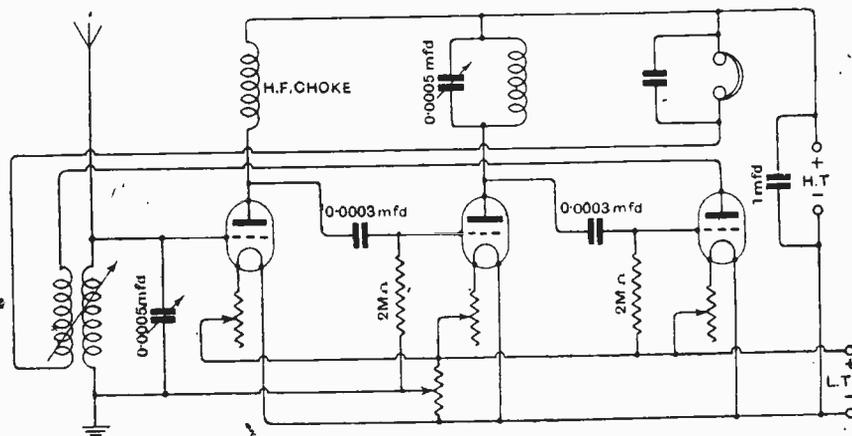
Fig. 2.—Tuned anode and choke-coupled H.F. amplification incorporated in a three-valve receiver.
