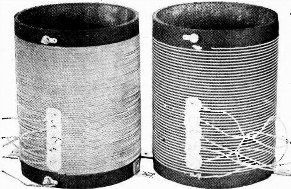
Fig. 4.—View showing the construction of the two tuning coils.
