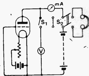
Fig. 3.—Experiment to illustrate the reduction in anode voltage due to the insertion of the voltmeter V.
