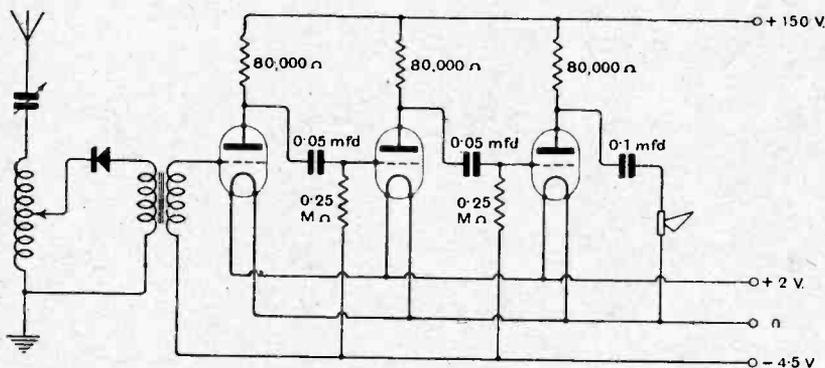
Fig. 24.—Practical circuit for a crystal receiver with resistance-coupled low-frequency amplifier.
