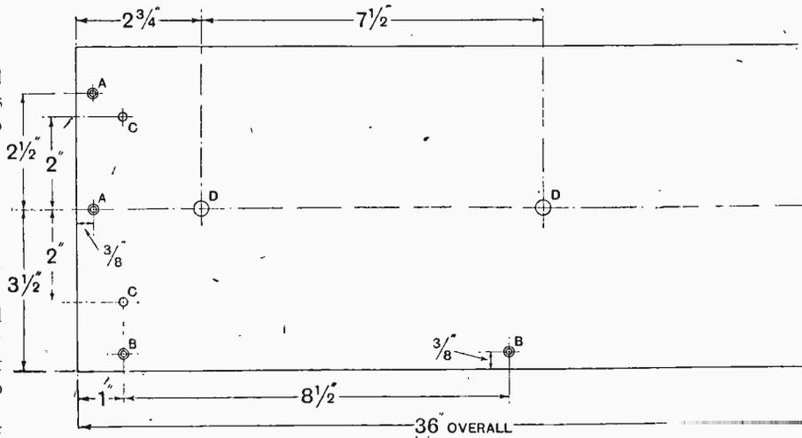
Fig. 2.—Details of the front panel. A, 1/8in. dia., countersunk for No. 6 B.A. fixing dia.; E, 3/8in. dia.;
