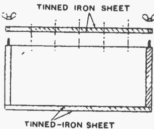
Fig. 10.—Screening box with close fitting bolted-down lid.
