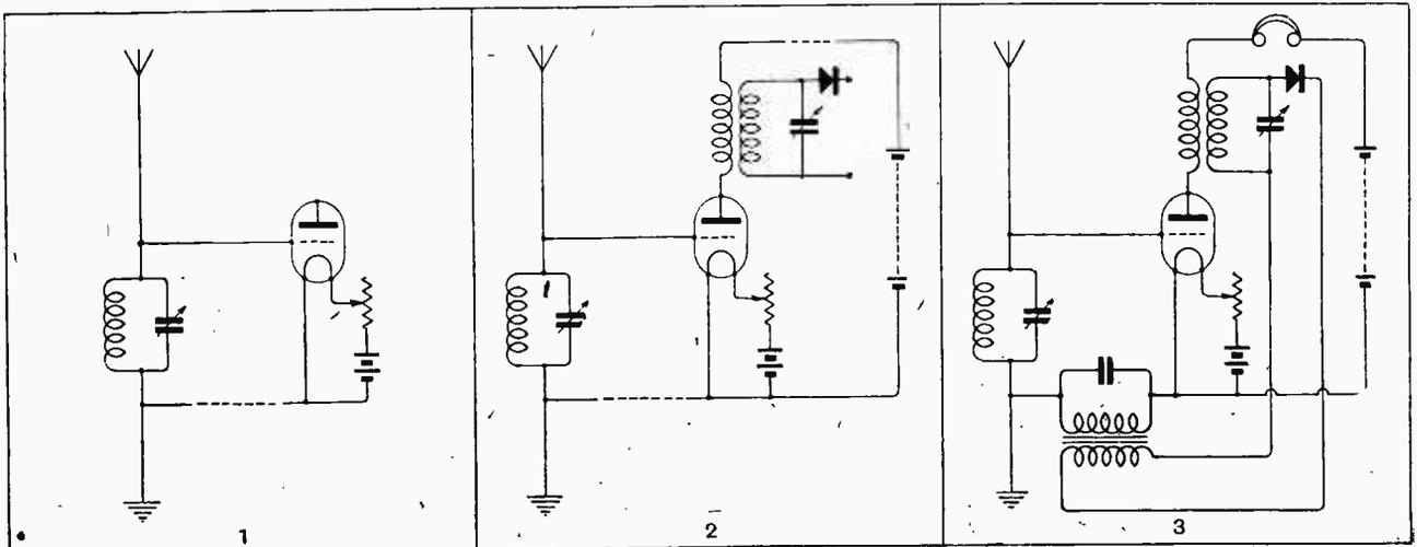
An oscillatory circuit, connected to aerial and earth. High-frequency voltages built up across it are applied to the grid circuit of a valve. The filament is heated by an L.T. battery, the external circuit being connected to its negative end.
