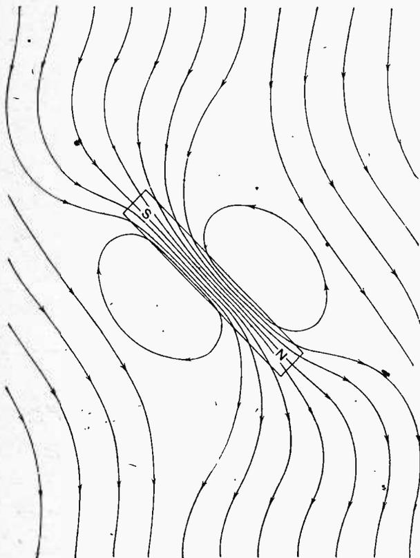
Fig. 2.—Lines of force in the earth's magnetic field distorted by a bar magnet.
