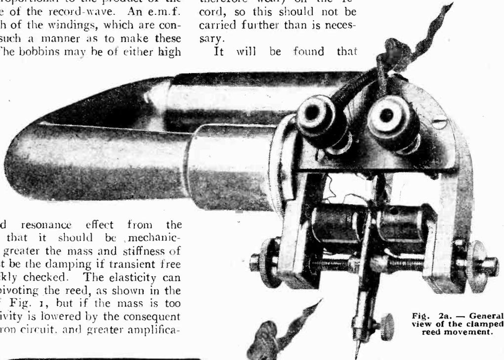
Fig. 2a. — General view of the clamped reed movement.
