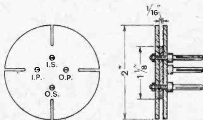
Fig. 1.—A typical H.F. transformer bobbin.
