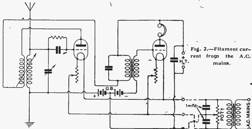
Fig. 2.—Filament current from the A.C. mains.
