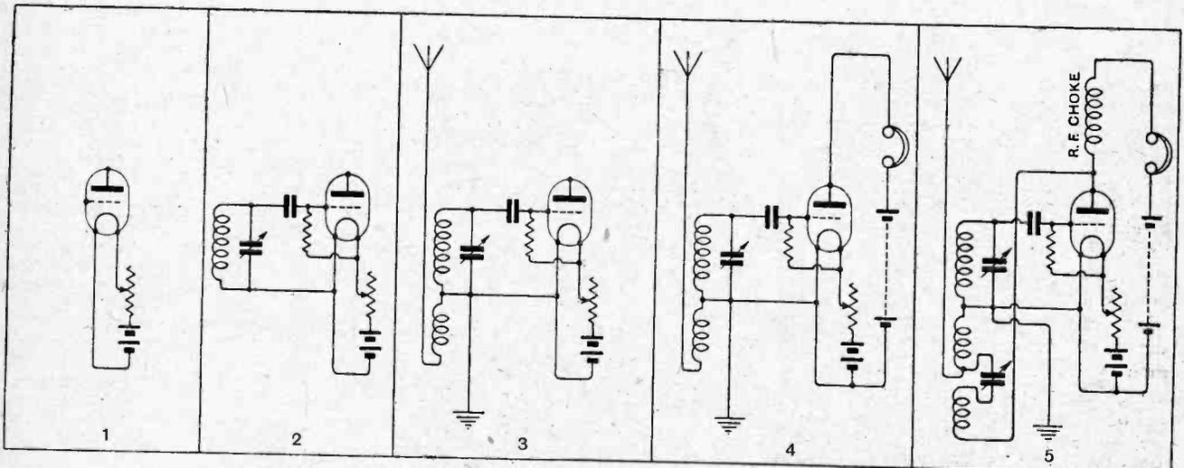
The valve, with its filament heated by a low tension battery through a variable resistance connected as usual in the positive lead.
