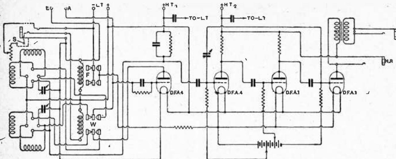
Theoretical diagram of connections in the "Polar Four" receiver
