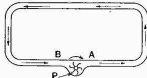
Fig. 1.—The distribution of pressure in this hydraulic circuit is analogous to the distribution of potential in the electrical circuit shown in Fig. 2.
