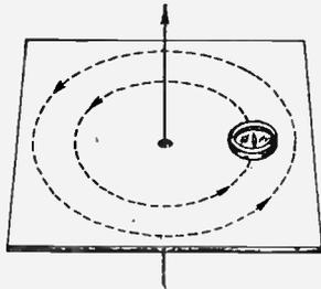
Fig. 1.—Magnetic field surrounding a straight conductor.
