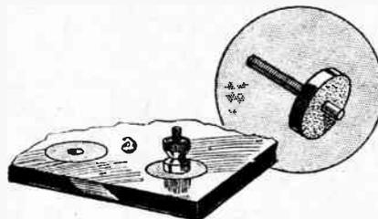
Improving the surface insulation of ebonite.
