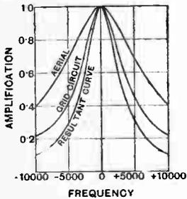
Fig. 11b.—Selectivity curves for aerial and tuned grid circuit, with resultant curve of the two circuits in combination. A loose coupling between the two circuits has been assumed.
