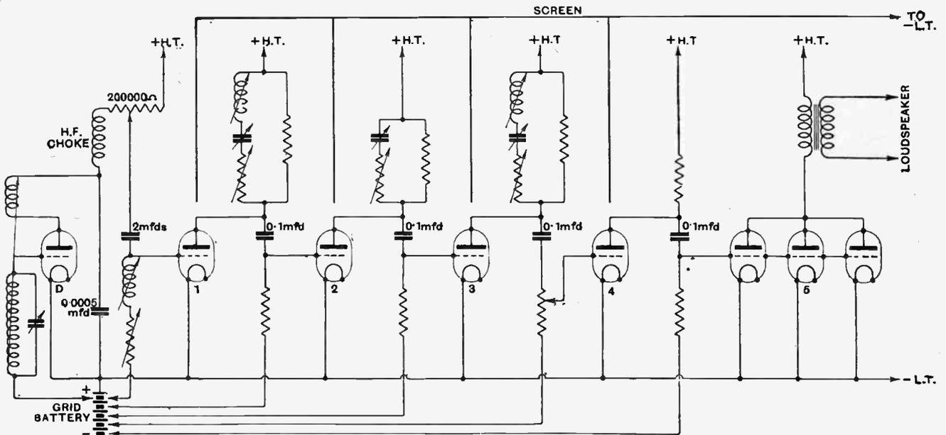
Fig. 11.—Connections of a practical amplifier equipped with tone correcting devices.
