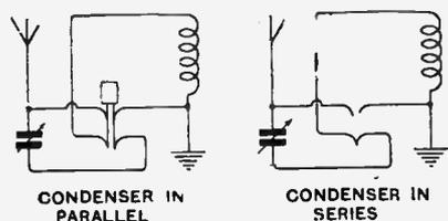
securing screws must therefore be inserted alternately. The two circuit diagrams at the bottom of the figure show that the tuning condenser will be connected in parallel with the plug inserted and in series with the plug withdrawn.—B. V.
