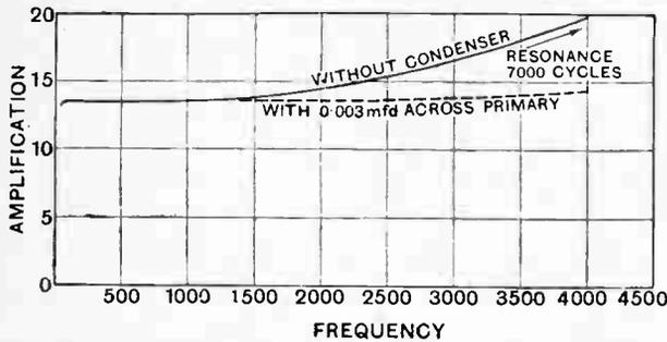
Fig. 2.—Characteristic curve of 2 : 1 ratio transformer and D.E.5 valve. Anode volts, 160; grid volts, 9. Primary inductance (15,000 turns) at 1,000 cycles, 225 henries; secondary inductance (30,000 turns) 900 henries. Secondary self-capacity 100 micro-mfd.
