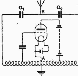
Suppression of carrier wave in intervals between signals or speech. (No. 241,417.)
