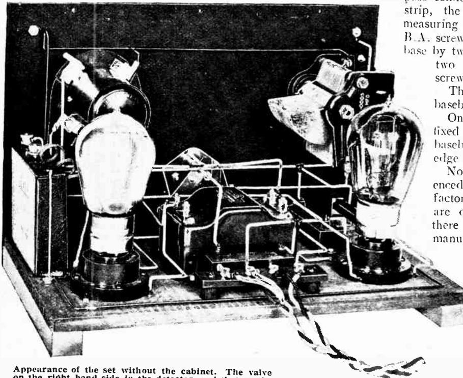
Appearance of the set without the cabinet. The valve on the right hand side is the detector, and that on the left the L.F. magnifier. It should be noted that the grid bias connection as described in the text was not fitted when this illustration was taken.
