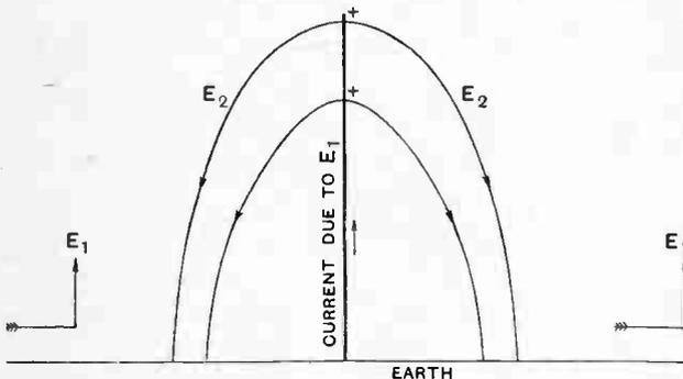
Fig. 4.—Secondary electric field  $E_2$  due to the current charge induced in an untuned aerial by the electric field  $E_1$  in arriving waves. The reduction of the field  $E_1$  by  $E_2$  is the same on both sides of the aerial.
