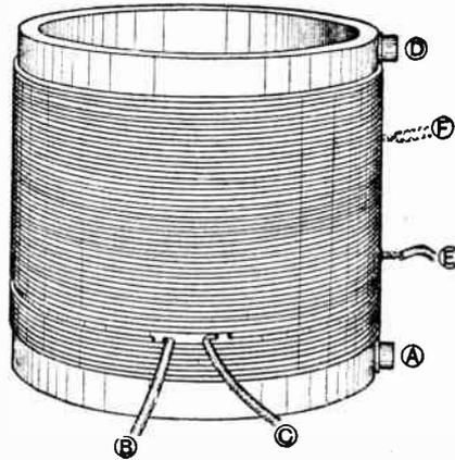
**TUNING COILS.** The formers are  $2\frac{1}{2}$  in. in length and diameter. The primary consists of 10 turns, and leaving a space of one turn to ensure good insulation between primary and secondary, the secondary is wound on in the same direction and consists of 60 turns. (A) and (B) are the ends of the primary, (C) and (D) the secondary, (E) the stabilising tap on the 10th secondary turn and (F) the detector valve tap at the 40th.
