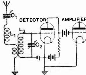
Fig. 11a.—High-frequency circuits associated with the detector valve. Inductance values are as follow:  $L_1$  400 mhs.;  $L_2$  250 mhs. H.F. resistance of aerial circuit, 22 ohms, and of secondary circuit  $L_2$   $C_2$ , 7 ohms, both measured at 360 metres.
