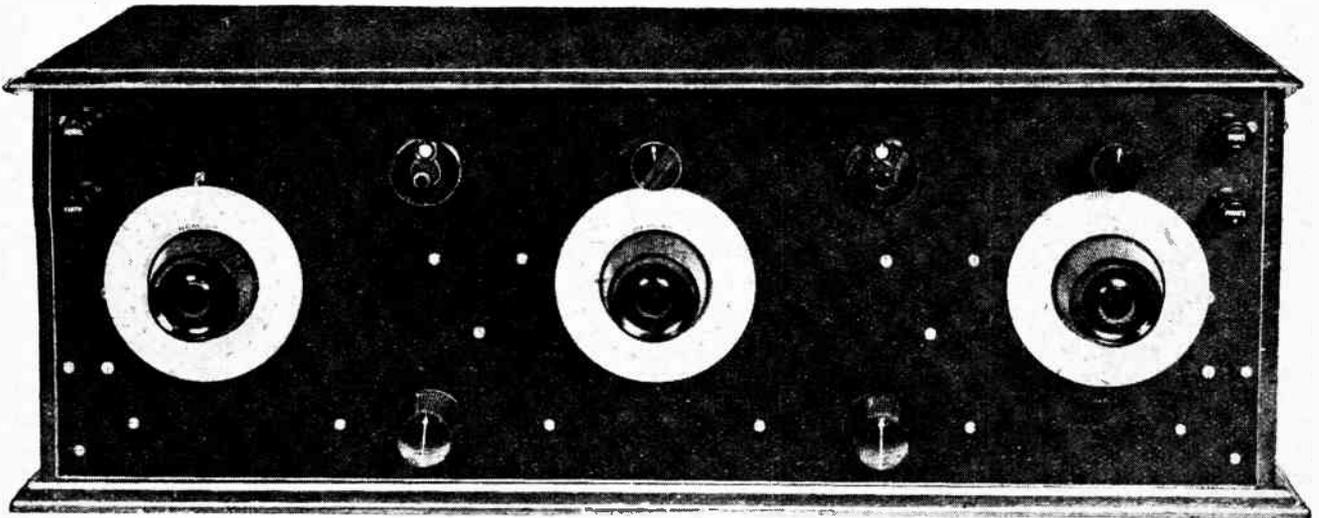
**FRONT VIEW OF THE RECEIVER.** The securing holes for two of the tuning condensers, here shown white, are recessed so that the heads of the screws may be covered with black filling or plugged with pieces of 1/4in. ebonite rod, and rubbed down smooth. The heads of all other screws may be treated with steel bronzing solution or camera black.
