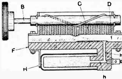
**Variable condenser with mercury electrode.**
