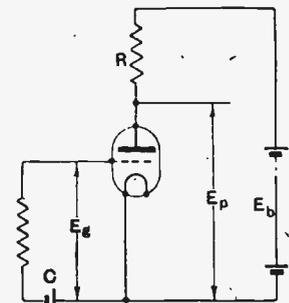
Fig. 1.—Single-stage resistance-coupled amplifier.
