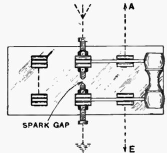
Safety gap incorporated in D.P.D.T. earthing switch.
