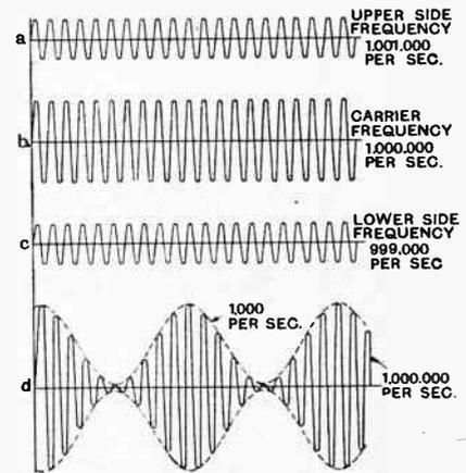
Modulated H.F. oscillations analysed into carrier wave and side bands.
