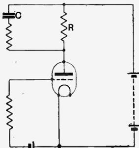
Fig. 3.—Capacity C connected in parallel with R to reduce the impedance at high frequencies.
