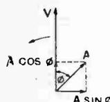
(Left) Current vector OA lagging behind voltage vector OV by an angle  $\phi$ .
