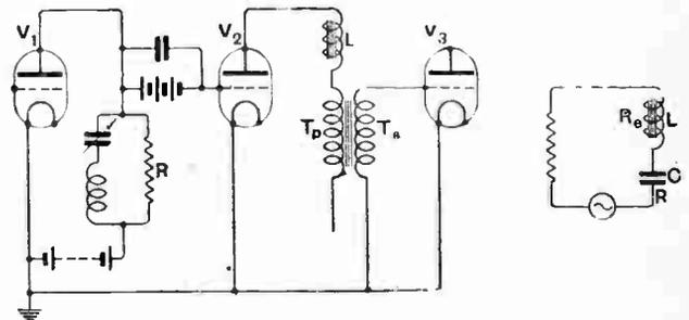
Fig. 7 (b).—Auxiliary inductance L of low effective resistance and low self-capacity for obtaining resonance at the upper audio-frequencies. The amplification at resonance depends upon  $\rho + R_c + R$  and upon the reactance  $\frac{1}{\omega C}$ . The resonance frequency can be varied by varying L and by connecting a variable condenser across the secondary winding. The purpose of the choke and condenser in parallel with R is to produce a dip in the characteristic.
