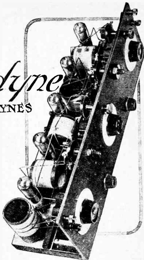
lower scale settings of the tuning condensers, while the manipulation of the four tuning dials almost rendered it impossible to search for a given station without the aid of a wavemeter. The open scale provided by 360° tuning dials solved, to some extent, the tuning difficulty, for the discrepancies in the settings of the three intermediate dials were more obvious, yet it was considered advisable to endeavour to limit the tuning controls, including the aerial circuit tuning, to three.
