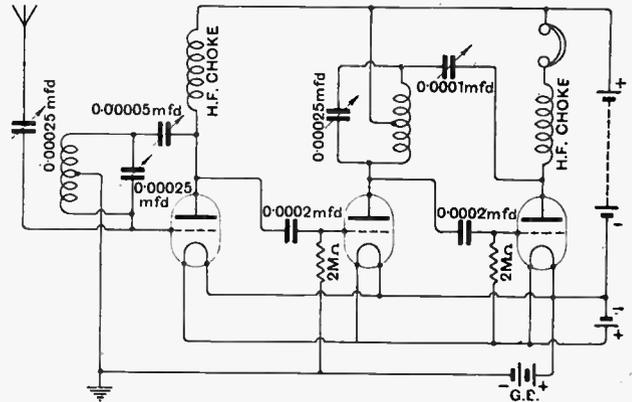
Fig. 8.—Practical H.F. amplifier, with Hartley circuit applied to the tuned anode coupling.
