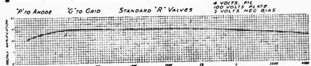
We strongly recommend the use of the 3½ to 1 ratio to follow the detector valve and the 5 to 1 for power stages or following a crystal.
