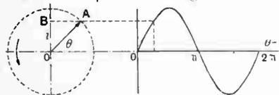
(Above) Sine curve developed from a rotating vector OA. OB = instantaneous value of the current.
