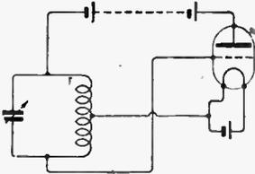
Fig. 1.—The Hartley circuit in its simplest form.
