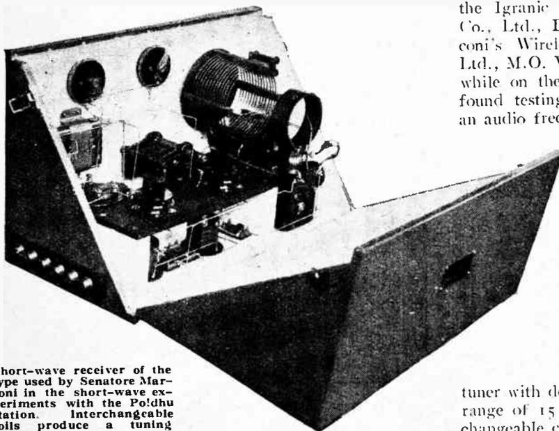
Short-wave receiver of the type used by Senatore Marconi in the short-wave experiments with the Po'dhu station. Interchangeable coils produce a tuning range of 15 to 100 metres.
