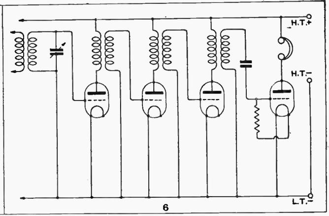
The secondary winding of the input transformer (which is usually tuned by a fixed, semi-variab.e, or variable condenser) is connected between grid and filament of the first intermediate frequency amplifying valve. Coupling between this and the succeeding valves is by transformers—
