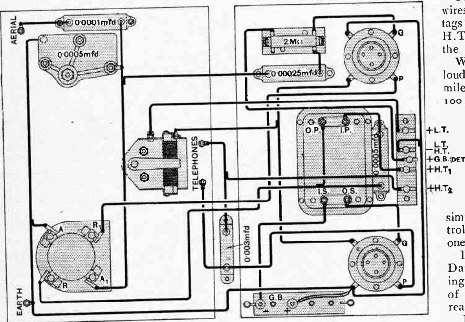
Fig. 4.—Wiring diagram. Some of the connecting wires are run beneath the baseboard, as explained in the text.
