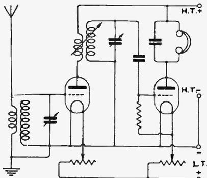
Fig. 1.—H.F. amplifier-detector with loosely-coupled transformer.
