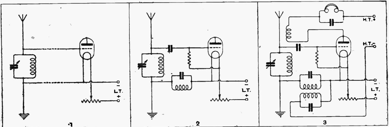
A tuned oscillatory circuit, connected between grid and filament of a valve. A short indoor aerial, or a frame, is often used, partly to minimise the risk of causing interference by radiation.
