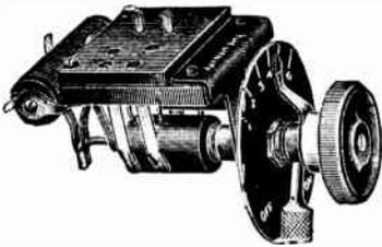
"Utility" Valve Switch Unit embodies in one unit our well known "Utility" switch, a valve holder and rheostat. It is for use in multi-valve sets, to control a valve and to switch it in and out whilst still preserving the continuity of the circuit. It has many advantages over separate components, such as lower self-capacity, less wiring, one-hole fixing and lower cost. Resistance 6 ohms or 30 ohms as desired. Nickel-plated 6d. extra. Price (complete with wiring diagrams) 8/6 each.
