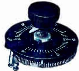
**B.599. SILVERTOWN FILAMENT RHEOSTAT. ONE-HOLE FIXING.** Circular pattern on ebonite former, complete with knob, pointer, black celluloid scale engraved in white, and two terminals for connections. The resistance wire is wound on an insulating rod, thereby giving a perfectly smooth adjustment. B.599—Wound to approximately 5 ohms resistance. Price 3/- each. B.600—Wound to approximately 30 ohms resistance. Price 3/6 each.
