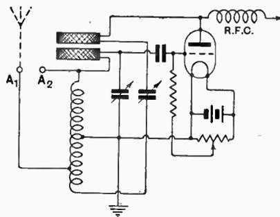
Fig. 2.—Adapting a "Reinartz" receiver for long waves.
