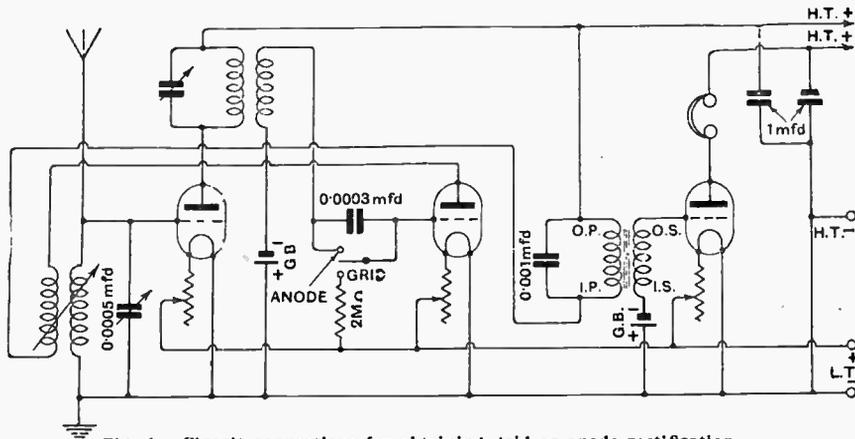
Fig. 1.—Circuit connections for obtaining grid or anode rectification.
