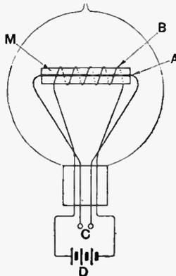
Valve filament with auxiliary A.C. heater. (No. 234,480.)
