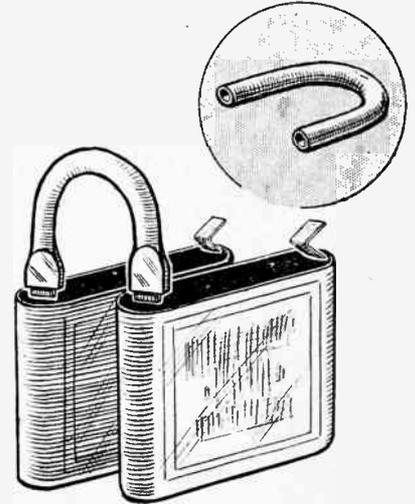
Flash lamp battery connections.
