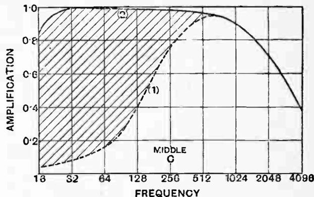
Fig. 12b.—Comparison of composite curves of H.F. circuits with variable characteristic amplifier (solid line) and ordinary transformer coupled amplifier (dotted line). The shaded area represents the loss due to the use of the ordinary amplifier (D.E.3 with 2.7:1 transformer followed by D.E.5 with 4:1 transformer).
