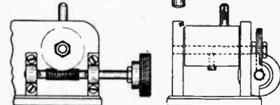
Jig for cutting worm gear wheels and (below) method of fitting vernier movement to variable coil holder.
