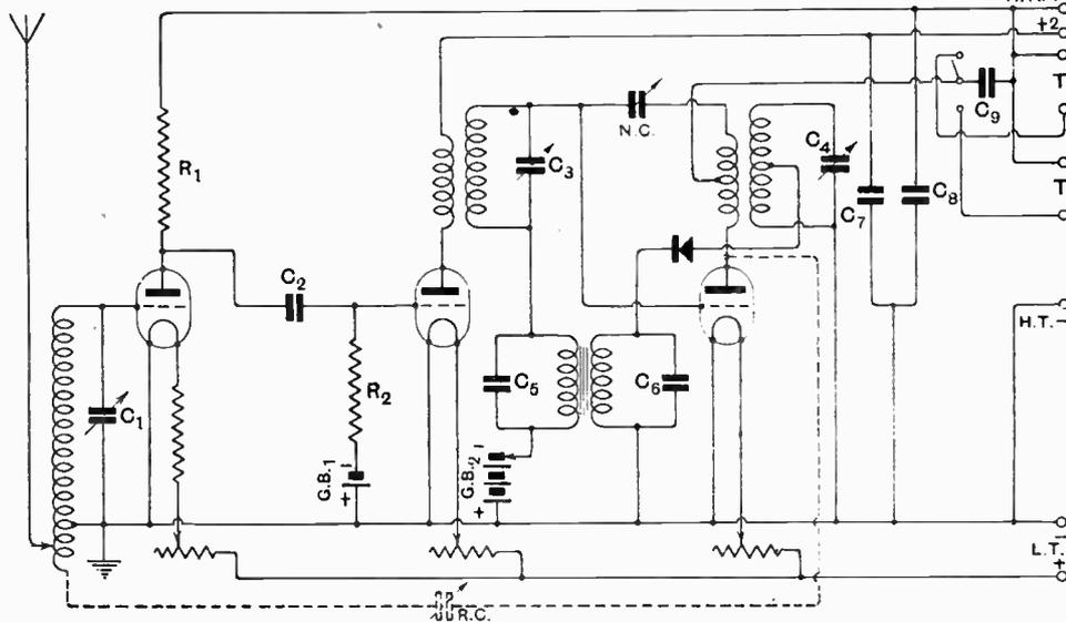
Fig. 1.—Theoretical circuit diagram.  $C_1, C_2, C_3 = 0.0005$  mfd.  $C_4 = 0.0002$  mfd.  $C_5 = 0.0001$  mfd.  $C_6 = 0.0003$  mfd.  $C_7, C_8 = 1$  mfd.  $C_9 = 0.001$  mfd.  $R_1 = 1$  megohm;  $R_2 = 5$  megohms. R.C. = Optional reaction condenser, 0.00005 mfd.
