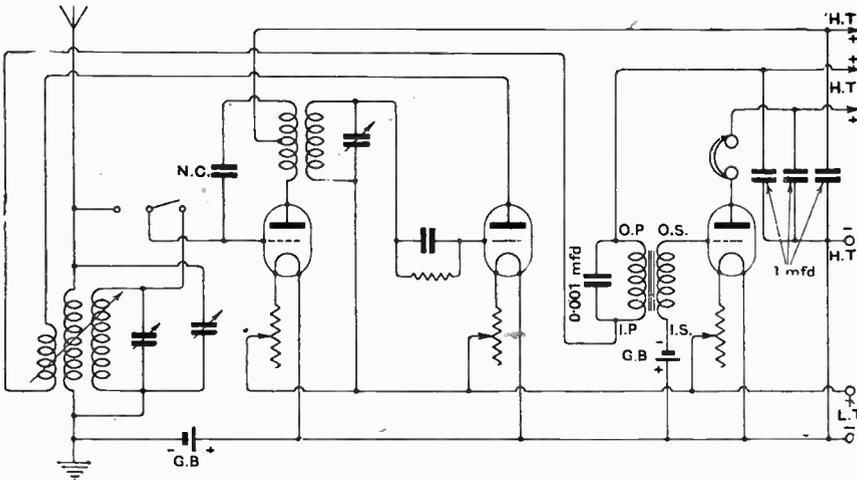
Fig. 2.—Selective three-valve circuit.
