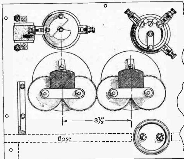
**THE TUNING CONDENSERS.** The pinions are interlocked and care must be taken to accurately set out the spacing between the condensers so that the pinions will mesh smoothly. Ordinary soldering tags are used to secure the blocking condenser to the telephone terminals.
