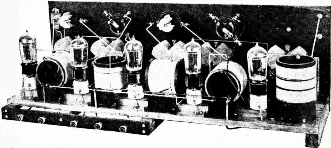
**THE FINISHED AMPLIFIER.** The tin plate which covers the base forms part of a screening case which may be fitted should it be considered necessary after the set has been completed. It is omitted here as it is somewhat difficult to construct.
