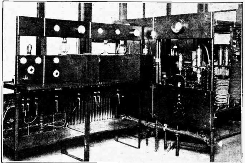
**FAMOUS SHORT-WAVE TRANSMITTER.** A new photograph of the transmitting apparatus at KDKA, Pittsburg, Pa. On the extreme left is the quartz crystal oscillator which serves to maintain transmission at a constant frequency.
