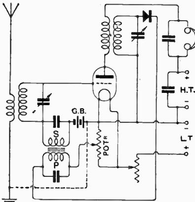
Fig. 1.—A reflex receiver with carborundum detector.
