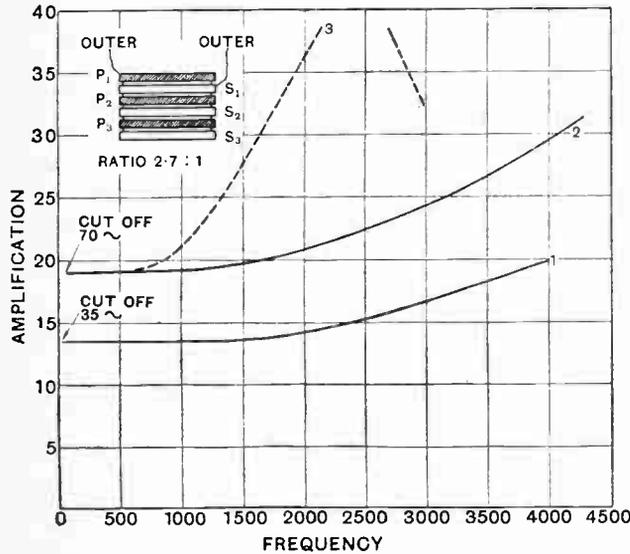
Fig. 5.—Curves of D.E.5 valve (anode volts 160, grid bias, -7.5 volts) and tapped transformer with idle primary section in different relative positions. (1) 2:1 ratio transformer without primary condenser. (2) Special 2.7:1 transformer (primary 100 henries) with P<sub>1</sub> as the idle section. (3) Special 2.7:1 transformer with idle section P<sub>3</sub> between S<sub>2</sub> and S<sub>3</sub>.
