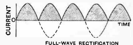
Wave-forms of half-wave and full-wave rectification.
