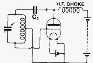
Fig. 2.—Circuit arrangement permitting a common negative connection between H.T. and L.T. batteries.
