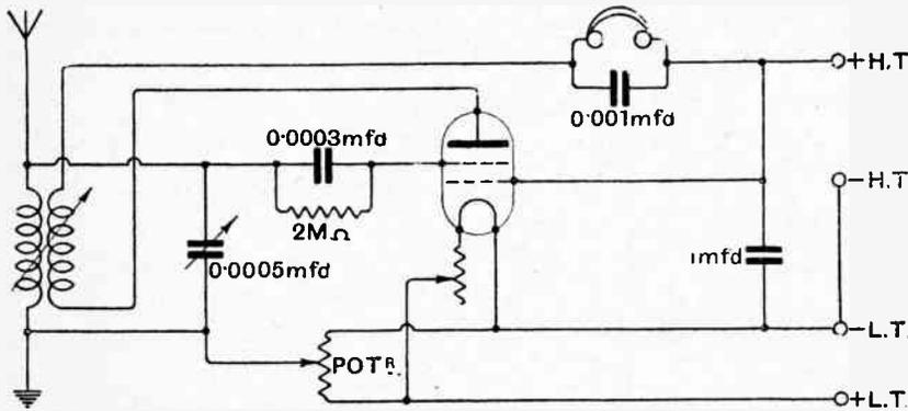
Fig. 1.—Four-electrode valve circuit for distant reception with headphones.
