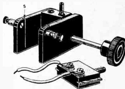
Plug-in coil-holder adapted for short-wave coils.
