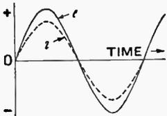
Fig. 3.—Alternating current and E.M.F. waves in phase.
