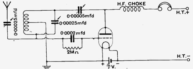
Fig. 5.—Capacity coupling to the aerial.
