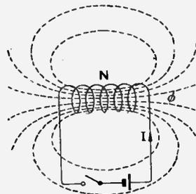
Fig. 2.—Magnetic field surrounding a cylindrical coil.
