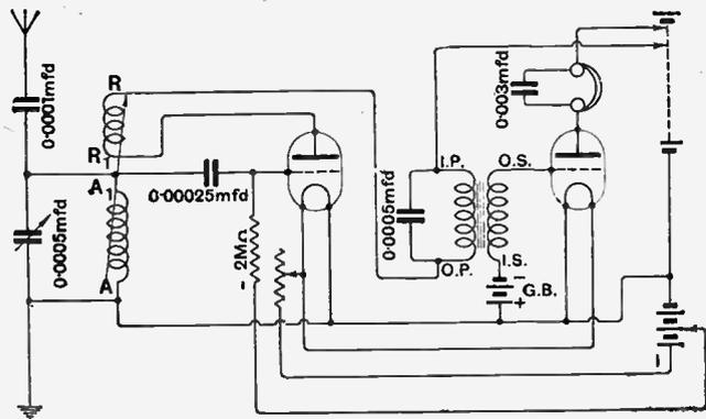
Fig. 1.—Theoretical connections of the receiver.
