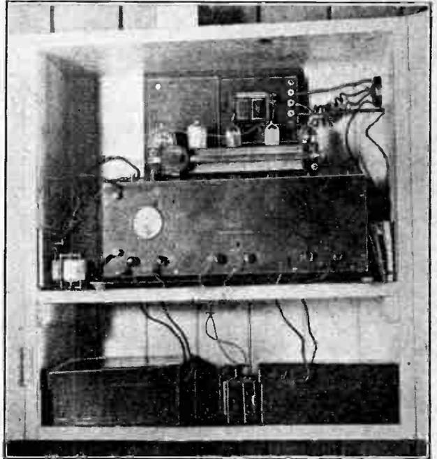
Valve amplifier and relays which amplify the fluctuating output from the photo-electric cell.
