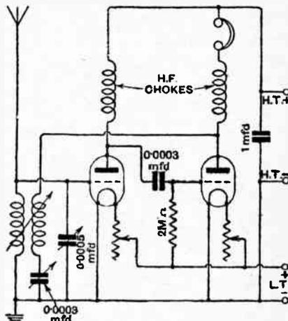
Fig. 2.—Choke-coupled H.F. amplification
