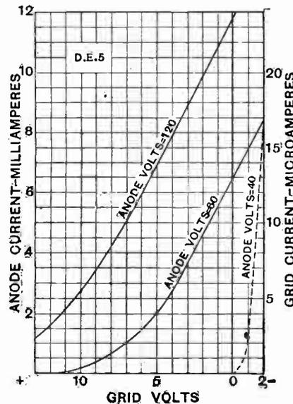
Fig. 3.—Anode and grid current curves for a D.E.5 valve.
