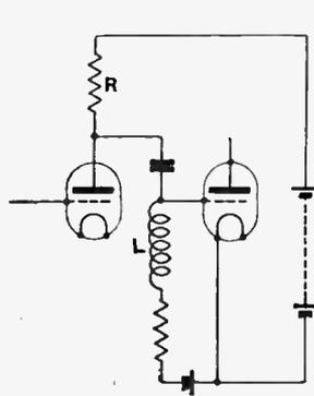
Fig. 6.—Practical method of introducing inductive reactance.
