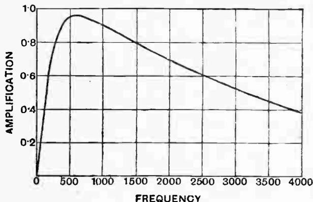
Fig. 12a.—Relative amplification curve of H.F. circuits with ordinary double noise magnifier (D.E.3 with 2.7:1 transformer followed by D.E.5 with 4:1 transformer).
