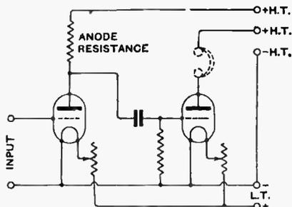
Resistance-capacity coupled valves.
