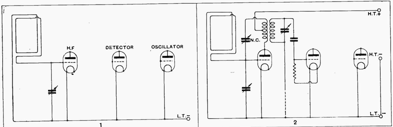
Three valves, operating respectively as H.F. (fundamental frequency), first detector, and oscillator. To avoid unnecessary complication, the filament circuits are not completed. A frame aerial and tuning condenser are connected between grid and filament of the H.F. valve.
