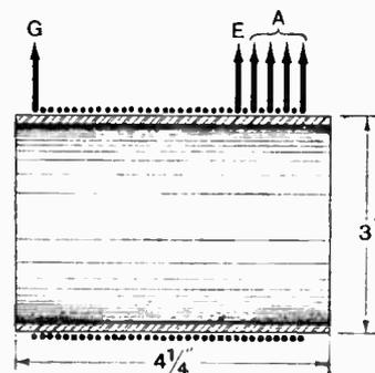
Fig. 4.—Constructional details of the aerial-grid coil.
