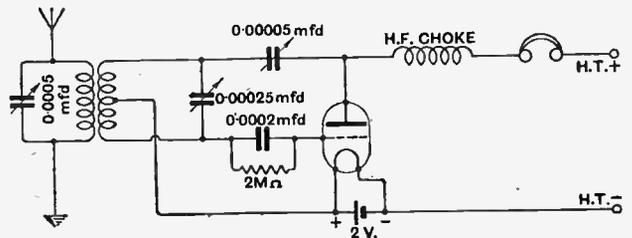
Fig. 6.—Loose-coupled tuned aerial circuit for maximum selectivity.
