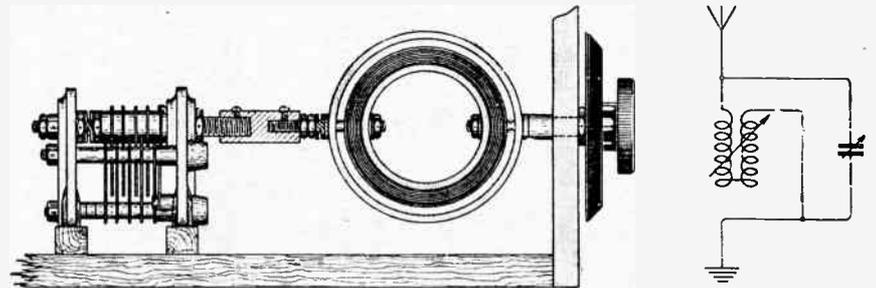
Variometer and variable condenser coupled to give increased wavelength range.
