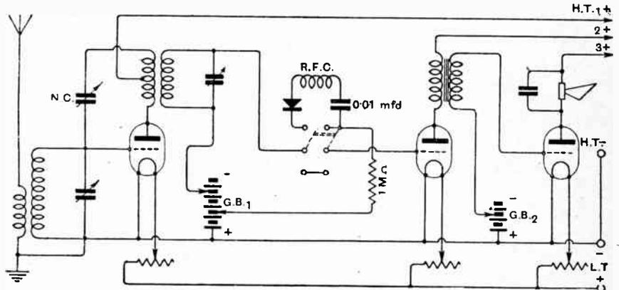
Fig. 2.—Alternative rectification methods.
