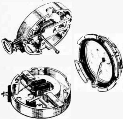
The mechanism of the Puremax loud-speaker, in which a double electromagnetic action is applied to a stiff reed and the vibrations transmitted to a mica diaphragm.
