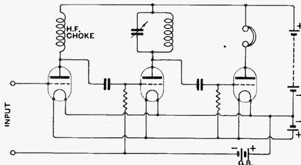
Fig. 7.—Aperiodic coupling introduced to stabilise H.F. amplifier.
