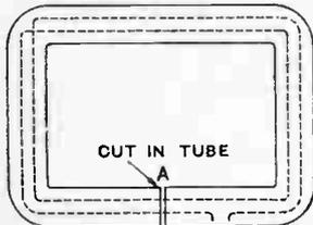
Fig. 3.—Frame aerial enclosed in metal tube.
