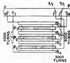
Fig. 4 (a).—Distribution of sections in high inductance tapped transformer.  $S_1$  is used to give the correct turn ratio, the other sections being standard. A better arrangement would be to have 4,500 turns on the primaries, giving an inductance of 182 henries. A 3 : 1 ratio can be obtained by connecting  $P_2$   $P_3$  in parallel.
