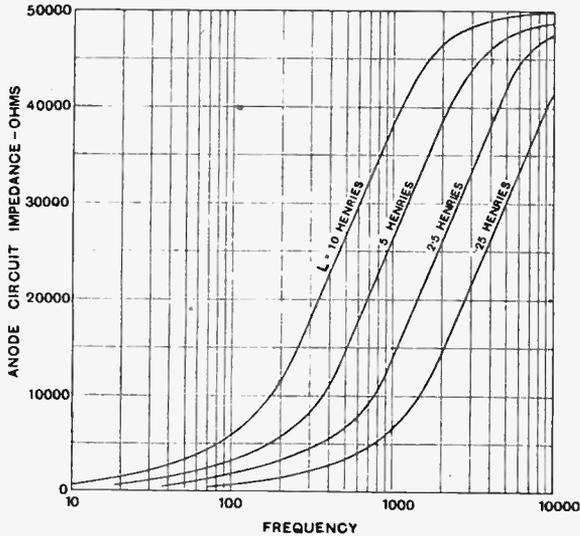
Fig. 5.—Impedance curves, showing the effect of inductive reactance in the anode circuit.
