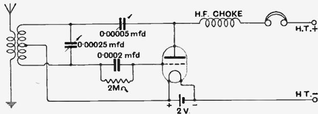
Fig. 4.—Aperiodic coupling to open aerial.
