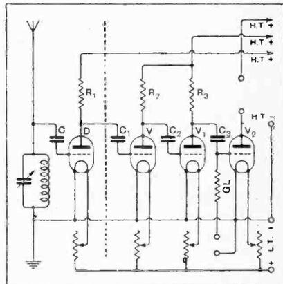
"Free grid" resistance amplifier circuit.
