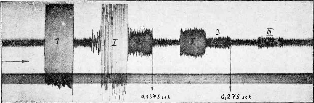
Fig. 3.—Oscillograph record of two "dots" sent from Rio de Janeiro and received at Geltow; the record shows two groups of echoes produced by waves which have travelled once and twice round the earth respectively.
