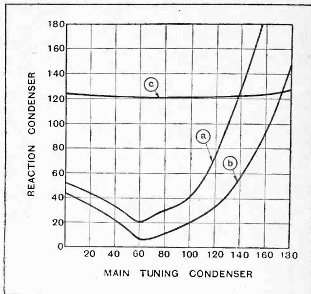
Fig. 4.—Experimental curves of relation between reaction and tuning controls; (a) small capacity, large coil and loose coupling, (b) same as (a) but with increased H.T., (c) large capacity (0.0005 mfd. max.) and small coil tightly coupled.
