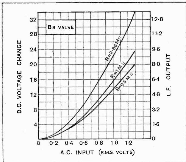
Fig. 3.—D.C. potential changes produced by various values of A.C. potential applied to the grid of a B8 valve arranged as an anode bend detector.
