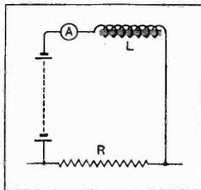
Fig. 3.—Modification of the inductance arm of the bridge for measuring the effect of a steady D.C. "polarising" current.
