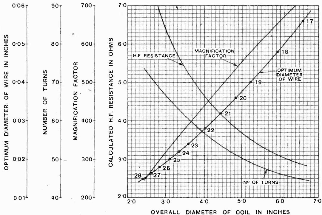
Design data for 200-microhenry coils (upper set of curves) and 325-microhenry coils (lower set of curves). The winding length for both sets of curves is  $\frac{8}{15} \times$  diameter.
