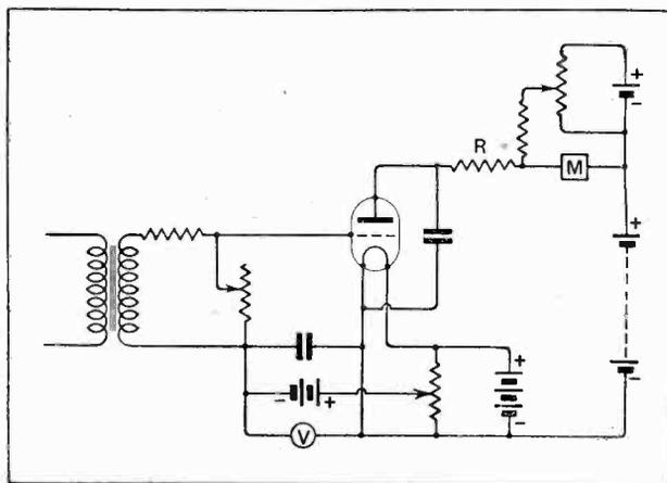
Fig. 2.—Circuit for examining the performance of a valve adjusted as an anode bend rectifier. Alternating input potentials are obtained from a 50-cycle alternating supply and the change of anode current is observed on the microammeter M set for reading from zero.
