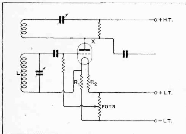
Circuit for alternative grid or anode rectification.
