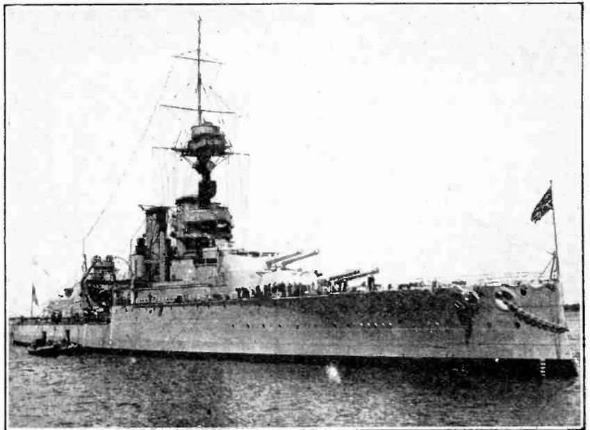
**WIRELESS-CONTROLLED TARGET SHIP.** H.M.S. "Centurion," the discarded battleship, which has been fitted with wireless-controlled machinery for use in gunnery practice. The ship is directed from a destroyer five miles distant and can cruise for four or five hours with no one on board.
