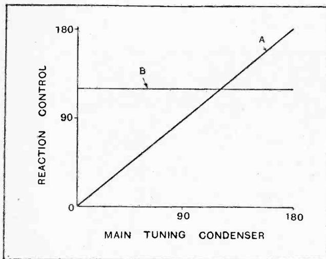
Fig. 3.—Two ideal conditions of reaction control; A, in which reaction setting is exactly proportional to tuning condenser setting, and, B, constant over the whole of the tuning scale.
