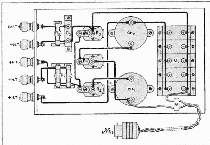
Fig. 9.—Wiring diagram of the D.C. eliminator.
