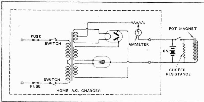
Fig. 1.—Method of energising 6-volt field winding of moving-coil loud-speaker from A.C. mains.
