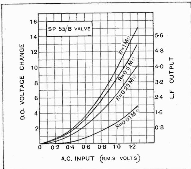
Fig. 4.—Rectification obtained with the SP.55B valve.
