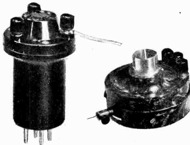
Fig. 7.—Dubilier electrostatic pick-up. On the left is shown an adapter to the plug into the detector valve holder which effects the necessary circuit alteration in a receiver when employing the pick-up.
