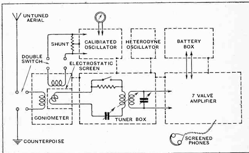
Fig. 4.—Schematic circuit diagram of apparatus.
