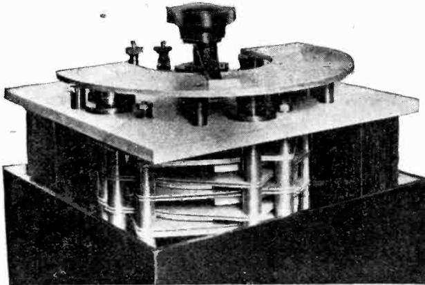
Fig. 3.—The Sullivan-Griffiths Precision condenser for use in accurate wavemeters. Adjacent dielectric gaps are electrically in series instead of parallel and are also complementary.
