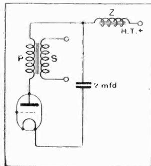
Fig. 1.—Circuit showing method of preventing L.F. back-coupling by the interposition in each H.T. lead of a L.F. choke.
