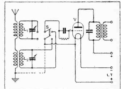
Receiving circuit for reducing interference. (No. 277,799.)
