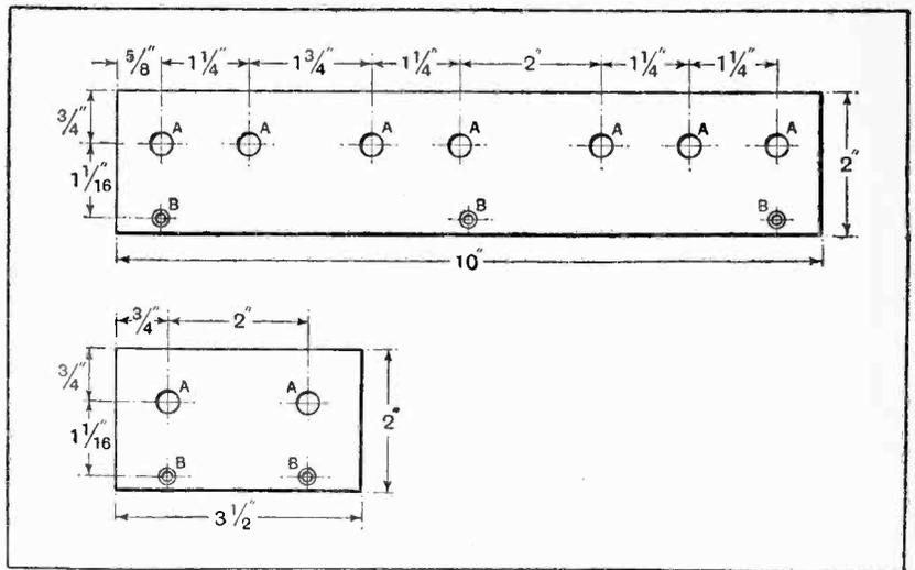
Fig. 8.—Drilling details of terminal strip; A, 5/16in. dia.; B, 1/8in. dia., counter-sunk for No. 4 wood screws.
