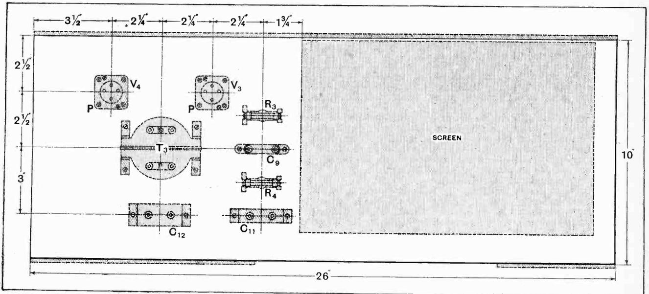
Fig. 5.—Position of the parts on the baseboard.
