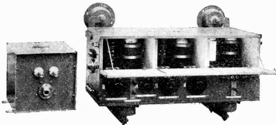
Fig. 1.—Marconi four-valve short-wave set in which one stage of neutralised H.F. amplification is employed. A doublet aerial is connected to the feeder box shown on the left which allows the receiver to be operated at almost any distance.
