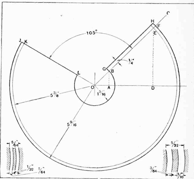
Details for obtaining the cutting out shape of a conical diaphragm. Sections of the gap are also given showing the position of the moving coil. In the narrow gap the moving coil former is made on a hard wood cylinder, 1-25/32in. in diameter. The diameter of the wooden cylinder for constructing the former for the wide gap should be 1-27/32in.
