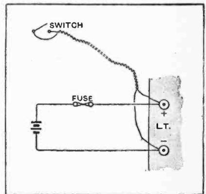
Switching off L.T. by means of a fuse.
