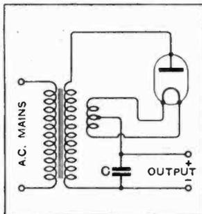
The unidirectional conductivity of the rectifying valve in a battery eliminator causes successive charges to be trapped in condenser C.
