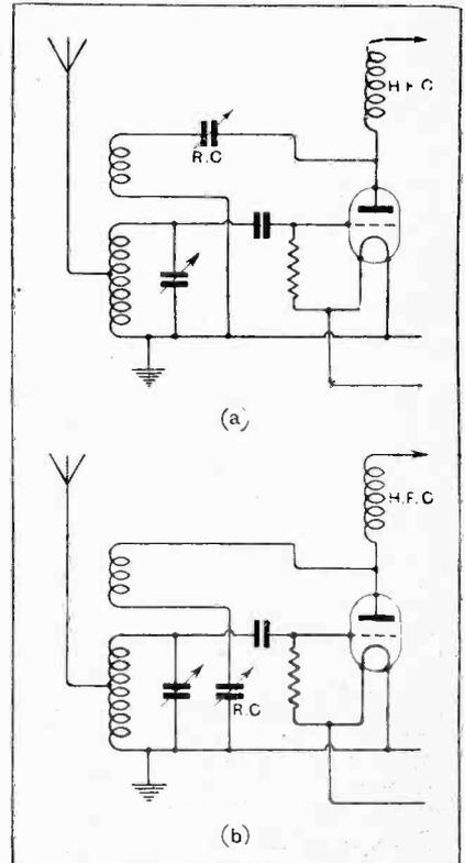
Fig. 2.—Reaction condenser connections; the arrangement in circuit (b) avoids hand capacity effects.
