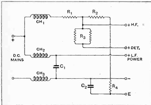
Fig. 4.—When the mains are very rough an additional choking coil may have to be connected as shown at CH<sub>3</sub>.
