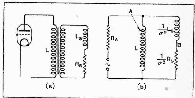
Fig. 7.—Output transformer feeding into a loud-speaker represented in (a) by  $L_s$  and  $R_s$ . The equivalent primary circuit is indicated in diagram (b).
