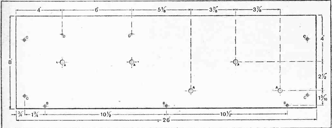
Fig. 6.—Drilling details of front panel. Sizes of holes are as follow:—A, 3/8in. dia.; B, 1/8in. dia., countersunk for No. 4 wood screws; C, 1/8in. dia., countersunk for 6B.A. screws; D, 3/32in. dia.
