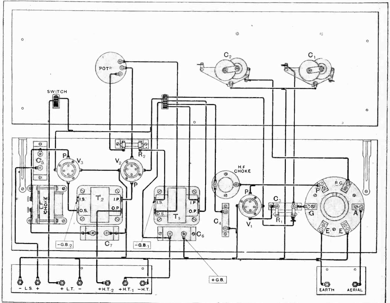
Fig. 9.—Complete wiring diagram; the lettering of the coil holder corresponds with the circuit of Fig. 1.
