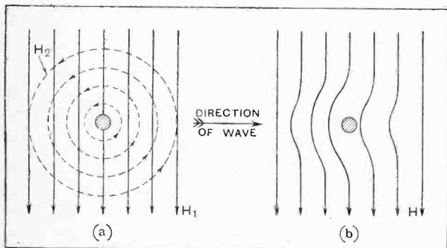
Fig. 5.—Distortion of magnetic field in the vicinity of a tree;  $H_1$  = field due to transmitter,  $H_2$  = field due to tree,  $H$  = resultant field.
