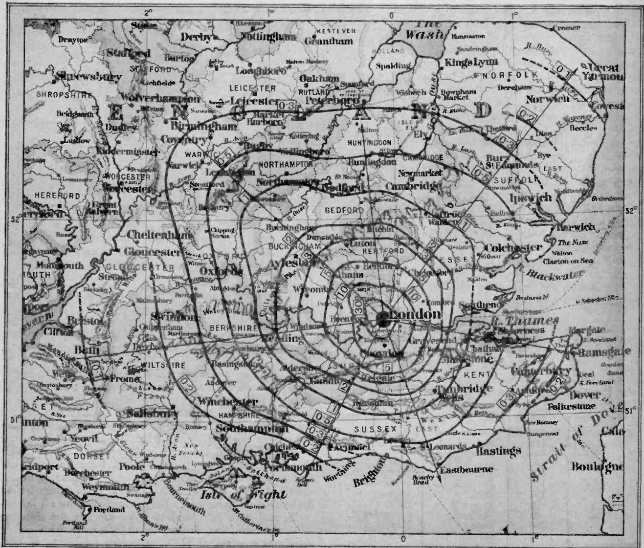
Fig. 2.—Contour map of field strength from 2LO. The radial lines indicate the directions taken by the travelling van, and the numbers represent the field strength in millivolts per metre.
