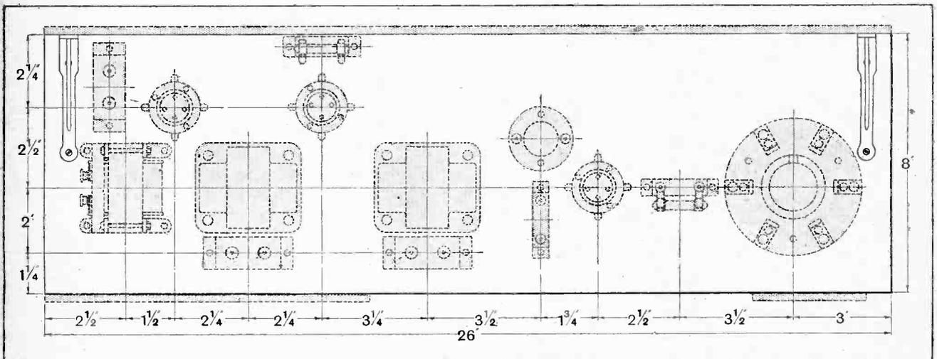
Fig. 7.—Dimensional layout of components on baseboard.
