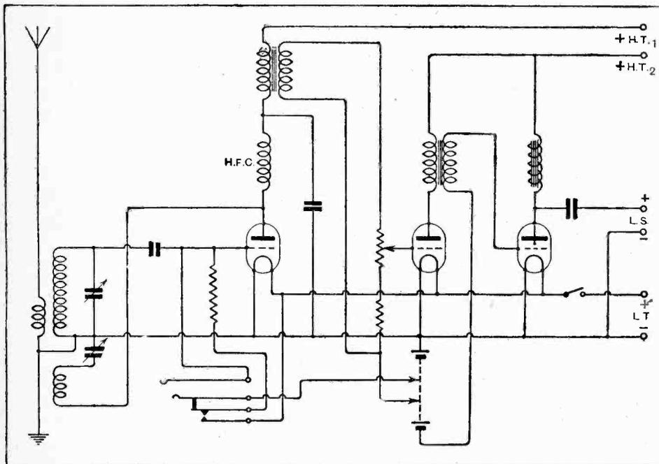
Fig. 2.—Alternative circuit in which three amplifying valves are available for the gramophone input.
