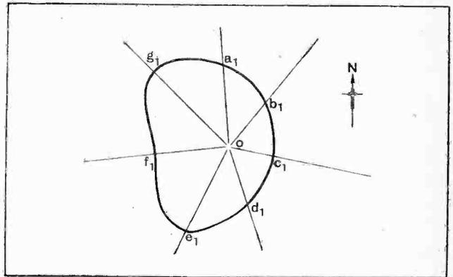
Fig. 3.—If  $oa$ ,  $ob$ ,  $oc$ , etc., in Fig. 2 be measured and their reciprocals plotted in the same directions, a diagram like Fig. 1, B, is obtained.
