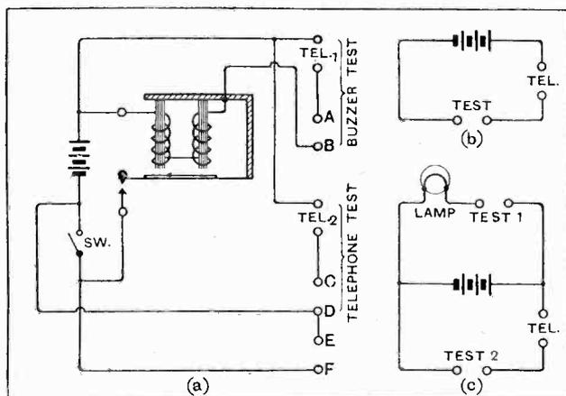
Three easily-constructed testing units.
