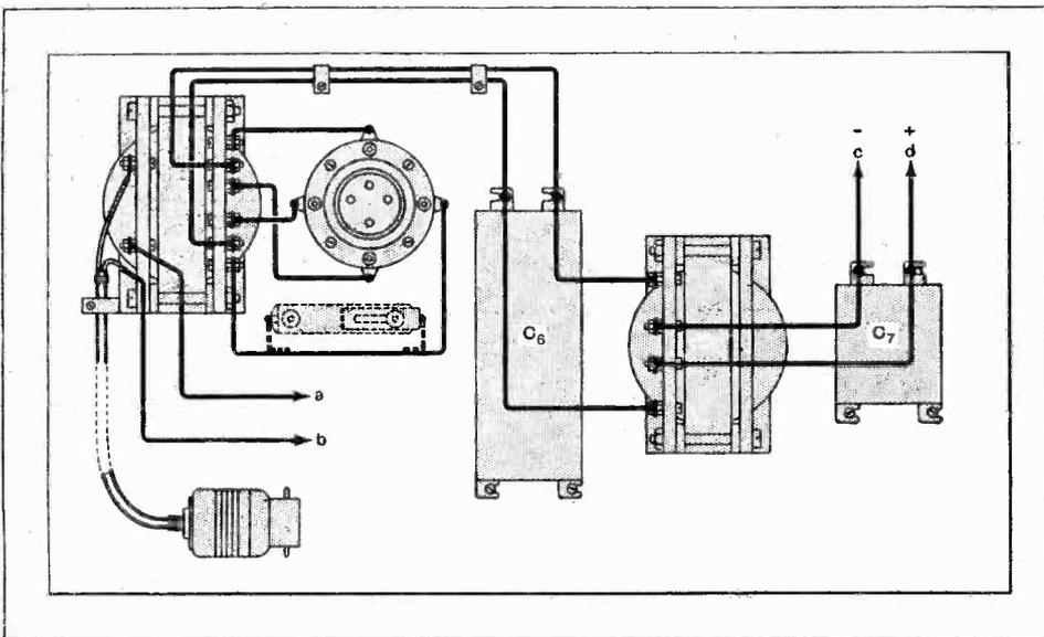
Wiring of simple A.C. rectifier. A filament rheostat is recommended for use with a valve of the U5 type. The reference letters show the connections to be made to the amplifier.
