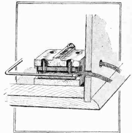
Sectional diagram showing method of fitting in receiver cabinet; holes are drilled for passing the battery leads through the back of the cabinet.
