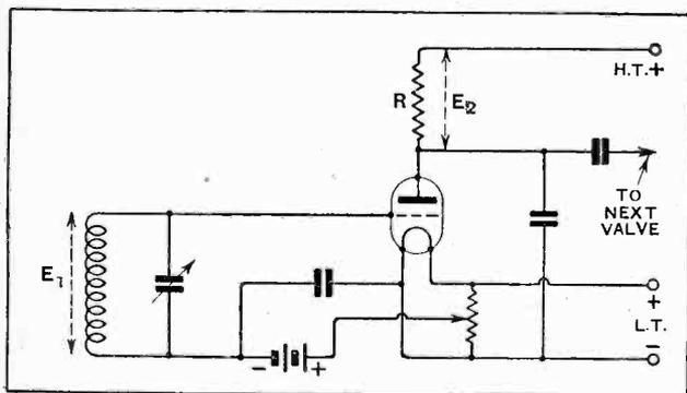
Fig. 2.—The equivalent circuit used to obtain practical data for anode bend detection.
