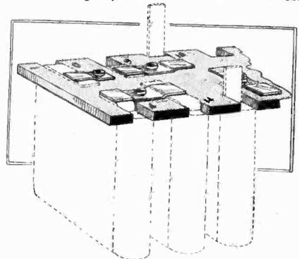
**"Simpsonic" connector panel for flash-lamp H.T. batteries.**
