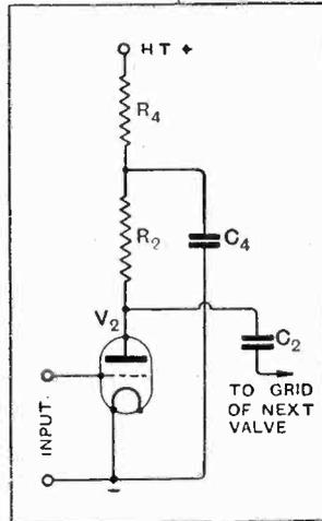
The anode feed scheme as applied to  $V_2$ . The speech currents are diverted from the H.T. battery and pass through  $C_4$  to earth.
