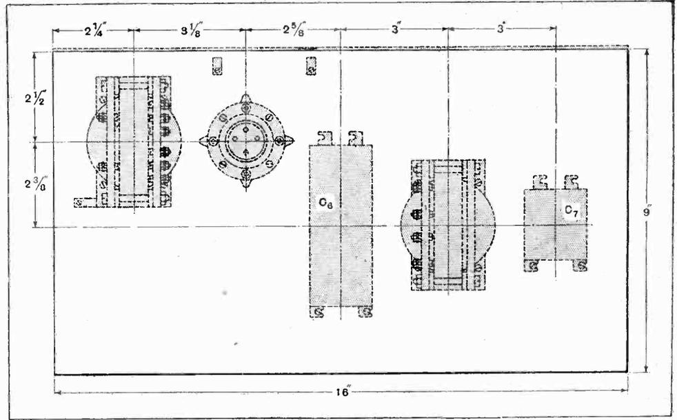
Layout of components forming the A.C. rectifier and smoothing circuit. When the lower base-board is fitted up for use with A.C. supply, it will be found advisable to clamp a thin sheet of copper foil under the battens of the upper board as a screen.
