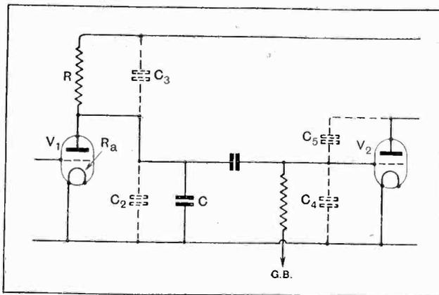
Fig. 5.—A resistance-coupled stage in which not only the incidental capacities but also the magnitude of  $R_a$  and  $R$  have a profound effect on the suppression of high notes.
