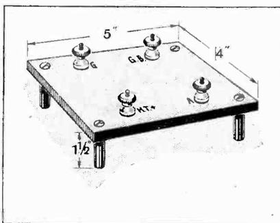
Fig. 2.—A small experimental unit for comparing the performance of various low-frequency coupling methods.
