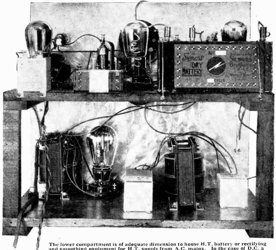
The lower compartment is of adequate dimension to house H.T. battery or rectifying and smoothing equipment for H.T. supply from A.C. mains. In the case of D.C. a potential divider takes the place of the transformer and rectifying valve.
