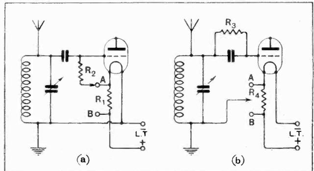
Fig. 1.—(a) Shows low potential end of grid leak connected directly to filament. (b) Shows grid bias applied through coil.
