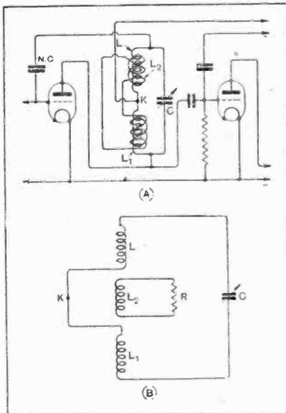
Method of minimising parasitic oscillations in tapped coils. (No. 278,812.)
