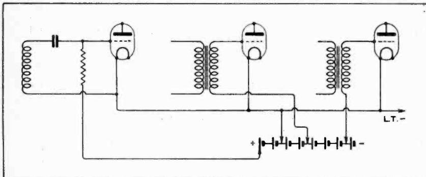
Fig. 2.—The application of positive or negative bias from a single bias battery.
