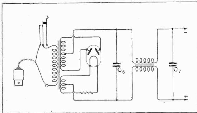
Circuit of A.C. rectifier.  $C_6$ , 6 mfd.;  $C_7$ , 4 mfd. The break switch is accommodated on the instrument panel. The contacts are, of course, insulated from the panel.
