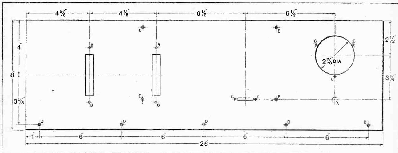
Fig. 7.—Panel dimensions. A, 3/8in. diameter; B, 5/32in.; C, 1/8in.; D, 1/8in. countersunk for No. 4 wood screws; E, 1/8in. countersunk for No. 6 B.A. screws.
