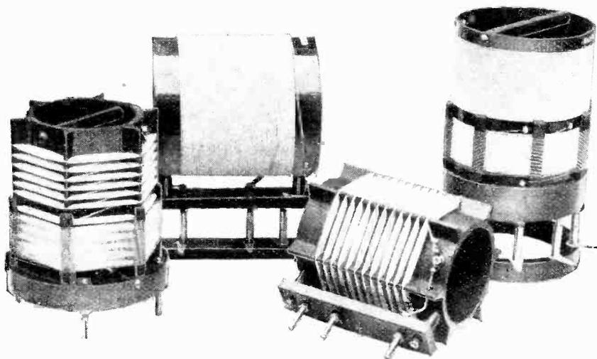
Complete set of "Berclif" coils and bases for the "Standard Four" receiver.
