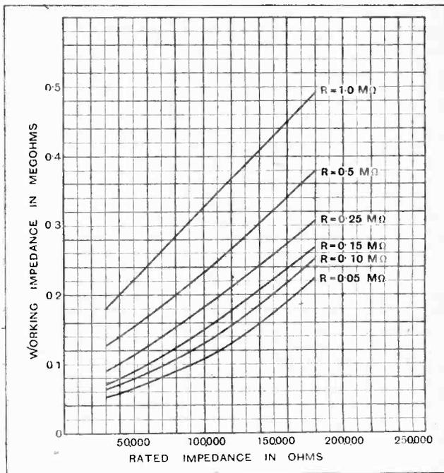
Fig. 7.—Curves showing relation between nominal valve impedance as given by makers and actual working impedance using various values of anode resistances.
