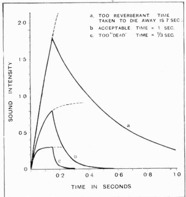
Fig. 1.—These curves represent the growth and decay in the intensity of a sound in three halls, similar in size though differently draped. In each the sound intensity is built up by the emission of a single syllable which if continued would grow in intensity as indicated by the dotted line.
