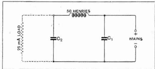
Fig. 2.—A practical smoothing circuit,  $C_1$  and  $C_2$  having the usual values. The load is that imposed by the valves in the set, and by any potential divider that may be used.
