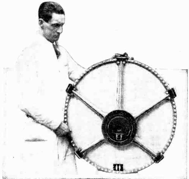
The loud-speaker consists of a stretched aluminium diaphragm of large diameter with the coil drive offset from the centre.
