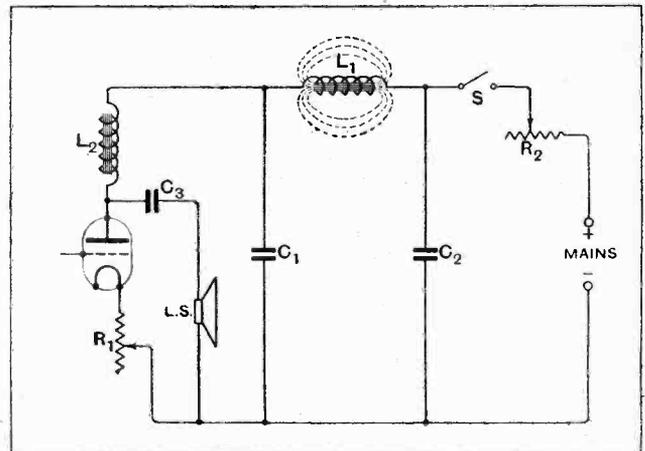
Fig. 1.—The maximum voltage produced across  $C_1$  or  $C_2$  is dependent on the rate of collapse of the lines of force around  $L_1$ .
