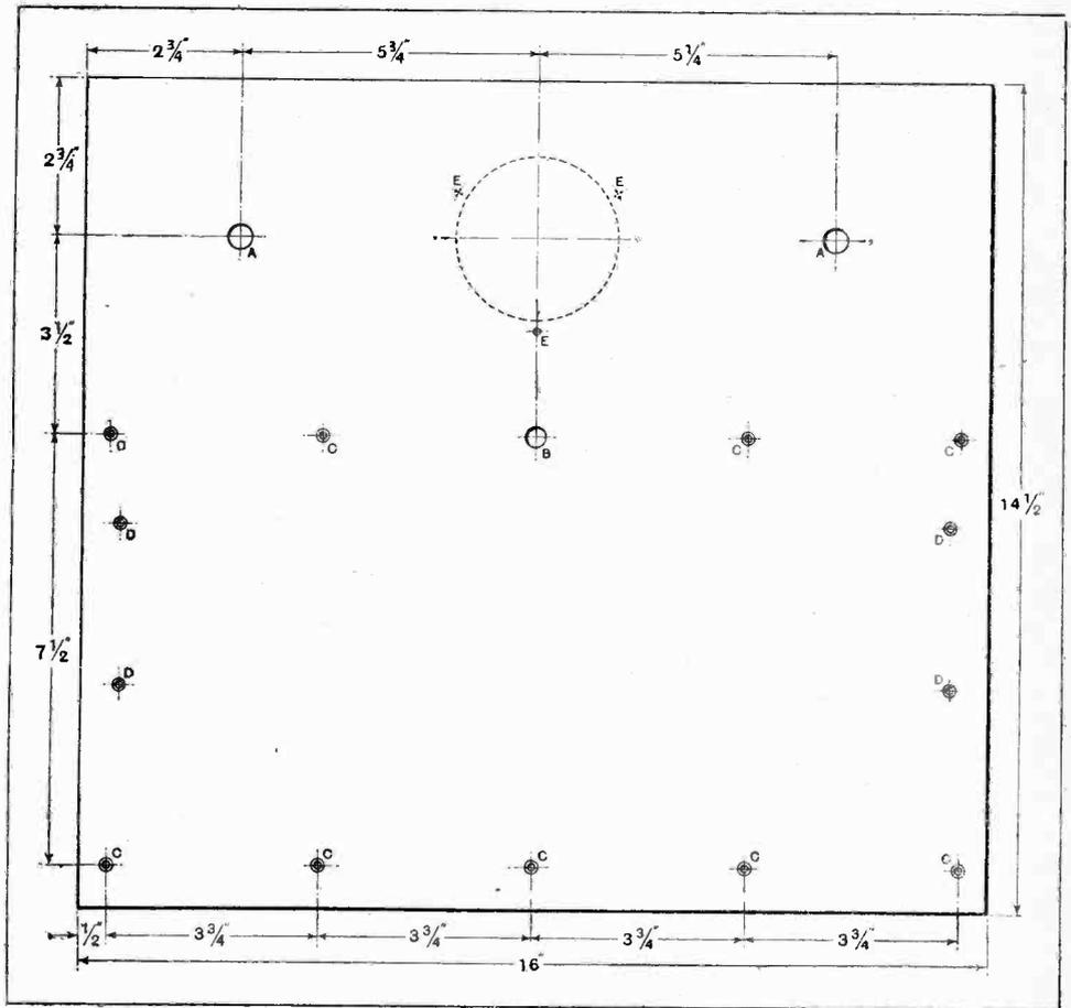
The front panel is constructed in this instance from No. 14 S.W.G. aluminium. A = 3/8 in., B = 1/2 in., C = 1/2 in. countersunk for No. 4 wood screws. D = 1/2 in. countersunk for No. 6 B.A. screws.
