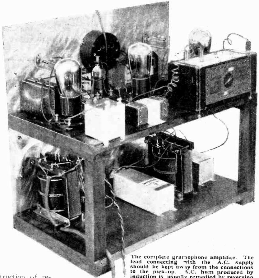
The complete gramophone amplifier. The lead connecting with the A.C. supply should be kept away from the connections to the pick-up. A.C. hum produced by induction is usually remedied by reversing the connections to the pick-up or running an additional lead from the frame of the pick-up to the L.T.—through a 1 mfd. condenser.
