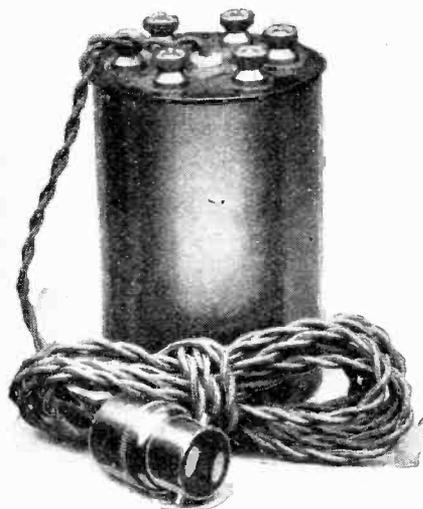
The Efesca Junior D.C. eliminator supplies H.T. and grid bias and contains a separate earthing condenser.
