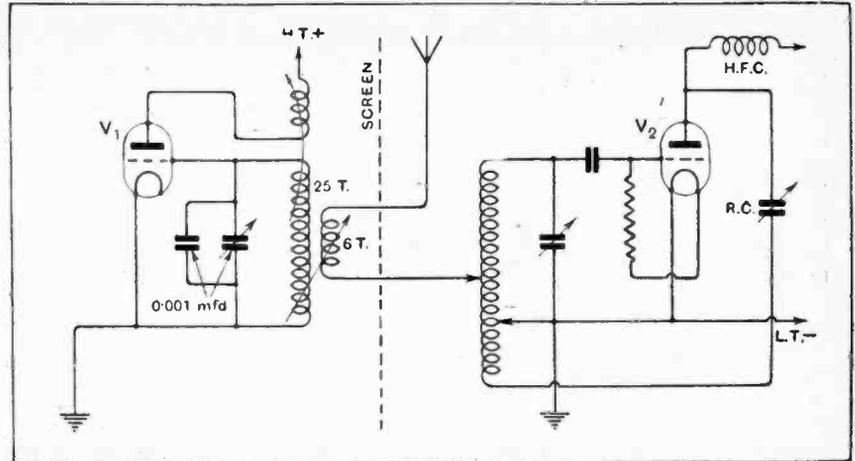
Fig. 1.—A separate valve rejector circuit.
