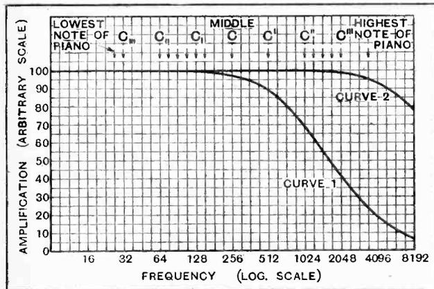
Fig. 9.—Curve 1 is the frequency response curve for the amplifier shown in Fig. 8. Note that the cut-off starts at about 200 cycles. Curve 2 shows the response curve to be expected from a 3-valve amplifier conforming to the conditions as stated in this article.
