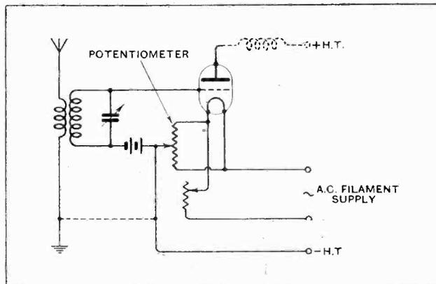
When heating ordinary valve filaments from A.C. mains additional grid bias is necessary to prevent grid current. The electrical centre of the filament is found by means of a potentiometer.
