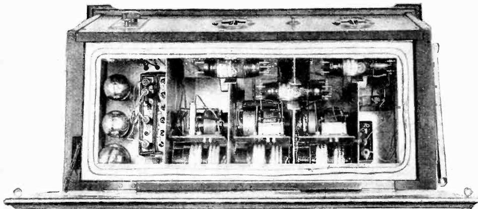
Interior of the Marconiphone Model 61. Note the braided metal beading for making contact with the metal lining of the lid.
