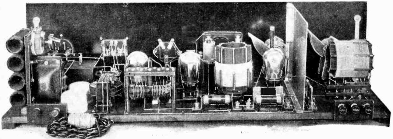
The rear view of the receiver. The current limiting resistance can be seen on the left and in the centre is the 20,000 ohms tapped resistance for supplying grid bias to the first L.F. valve.
