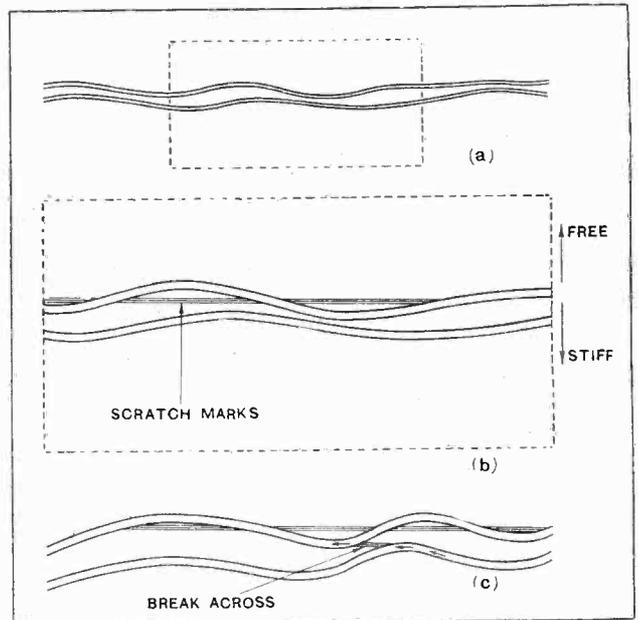
Fig. 2.—(a) Highly magnified section of record before playing. (b) The same section ploughed up by a damped pick-up. (c) Section showing where needle has jumped into next groove.
