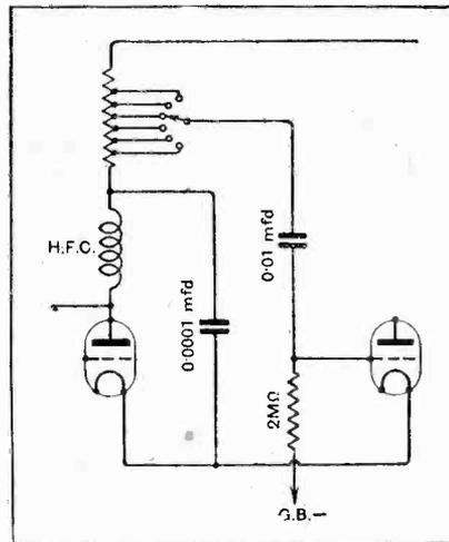
Fig. 2.—Method of controlling volume using a tapped anode resistance.
