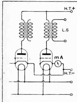
Fig. 4.—Alternative position of meter to show anode current of last valve.
