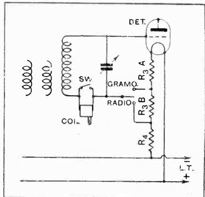
Fig. 2.—"Free" grid bias for alternative detection or gramophone amplification.
