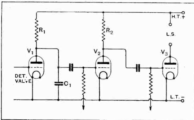
Fig. 8.—An anode bend detector followed by two stages of resistance coupling. If  $R_1$  and  $R_2$  are of the order of 2 megohms, and if  $V_1$  and  $V_2$  have high magnification factors, practically all notes at about 5,000 cycles will be lost.
