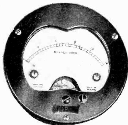
Ferranti flush-type milliammeter for panel mounting.
