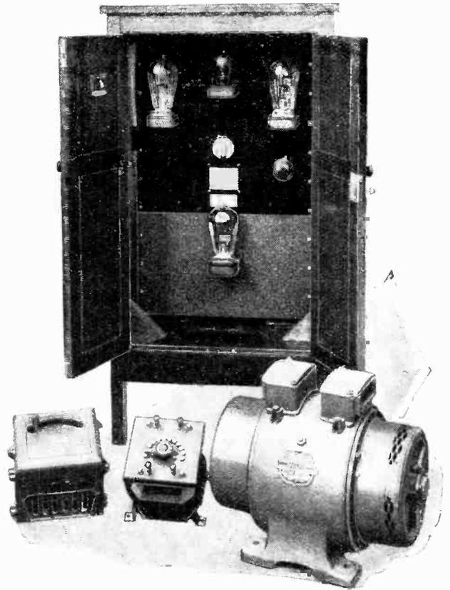
**THE AMPLIFIER.** The lower valve is associated with the metal fronted rectifier unit. The output of the small valve feeds the two larger valves which are push-pull connected. If the supply is D.C. a motor is used to create the necessary A.C. power input.
