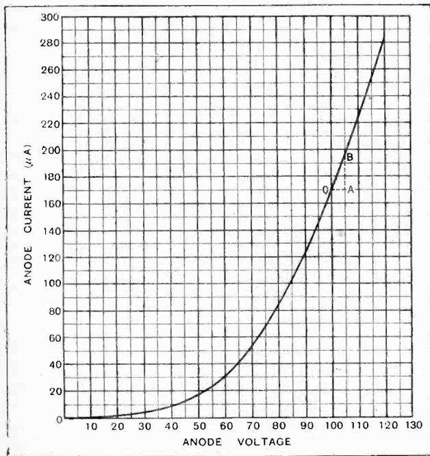
Fig. 6.—Anode current plotted against anode voltage for a B.T.H. B8 valve.  $\frac{OA}{AB}$  gives the A.C. resistance of the valve for the actual H.T. volts applied between plate and filament.
