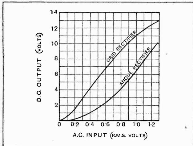
Fig. 3.—Curves showing that the superiority of D.C. voltage output from a grid rectifier diminishes as applied volts are increased.
