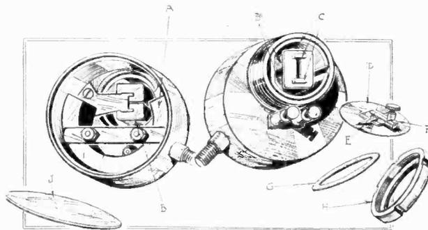
"HIS MASTER'S VOICE" GRAMOPHONE PICK-UP. A, field magnet; B, bobbins on divided end of magnet pole; C, the poles; D, the steel diaphragm; E, iron attachment for needle holder; F, brass end to prevent needles sticking; G, oil retaining washer; H, diaphragm clamping ring; J, back cover ring.
