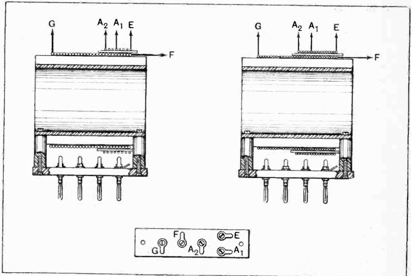
Fig. 4.—The two aerial-grid transformers. That on the left is for the 230-600 metres band of wavelengths, and the other for the long waves.
