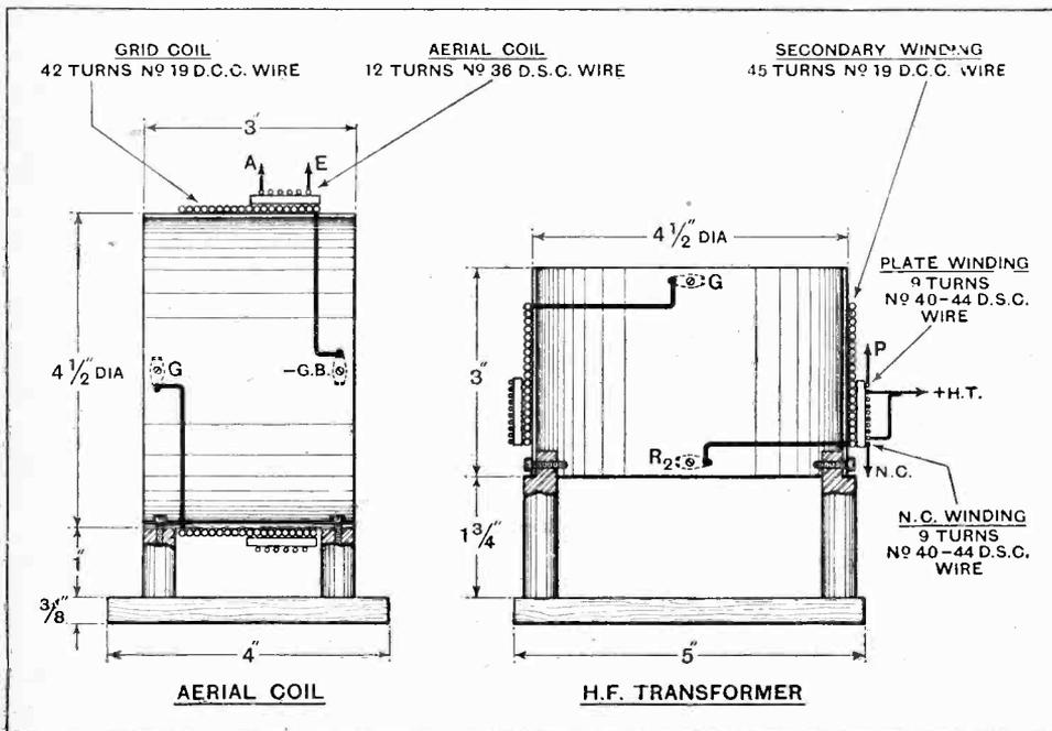
Fig. 5.—The dimensions and winding data for the aerial and H.F. transformers.
