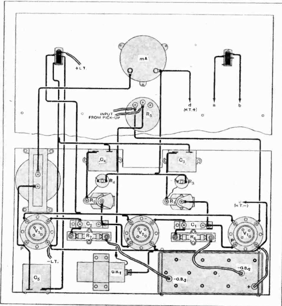
Appearance is greatly improved by using stiff wiring of No. 18 S.W.G., though No. 22 wire in sleeving is permissible and renders wiring much easier.
