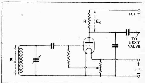
Fig. 1.—Grid rectification circuit. The D.C. volts developed across  $E_2$  were measured for various A.C. voltages applied at  $E_1$ .
