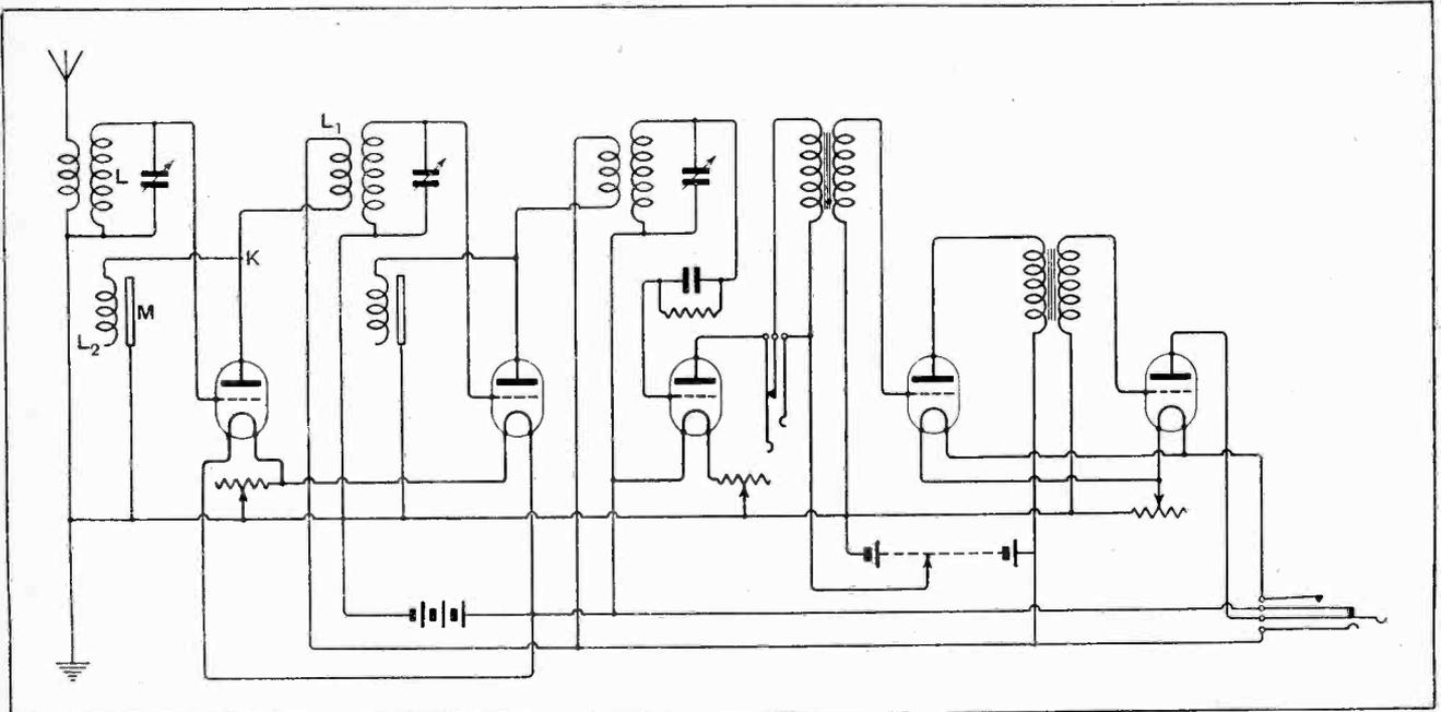
Method of balancing inter-electrode capacity by use of a plate. (No. 278,400.)
