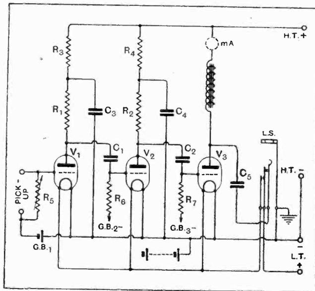
Values have been chosen to accommodate the increasing grid swing of each successive stage.  $R_1$ , 100,000 ohms;  $R_2$ , 60,000 ohms;  $R_3$ ,  $R_4$ , 20,000 ohms;  $R_5$ , 500,000 ohms maximum;  $R_6$ ,  $R_7$ , 3 megohms;  $C_1$ ,  $C_2$ , 0.01 mfd.;  $C_3$ ,  $C_4$ ,  $C_5$ , 2 mfd.
