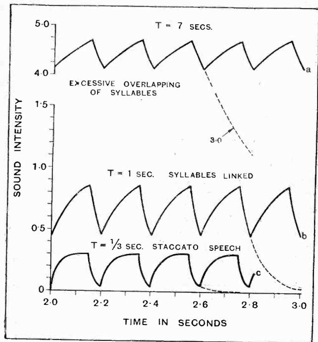
Fig. 2.—Relative rise and fall in sound intensity of single syllables issued at a rate of 5 a second under the same conditions as the curves of Fig. 1.
