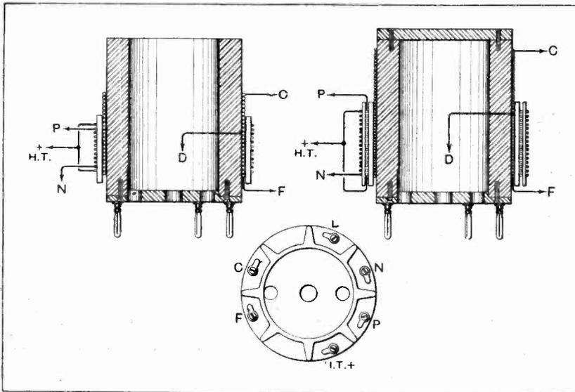
Fig. 5.—The intervalve high-frequency transformers. On the left is the transformer for the medium wavelengths, and on the right the transformer for wavelengths over 600 metres and up to 2,000 metres.
