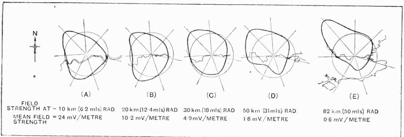
Fig. 1.—Field strength contours of 2LO for various distances up to 50 miles.
