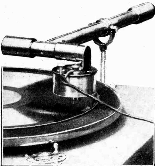
Fig. 1.—A form of tone-arm incorporating a balance weight.
