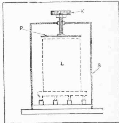
Varying the inductance of a metal-screened coil. (No. 278,208.)
