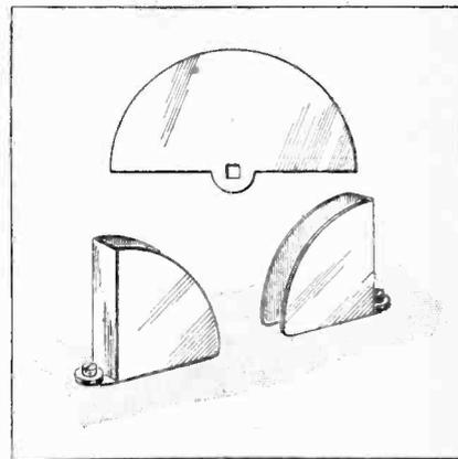
Fig. 4.—Making grid bias battery clips from old variable condenser vanes.
