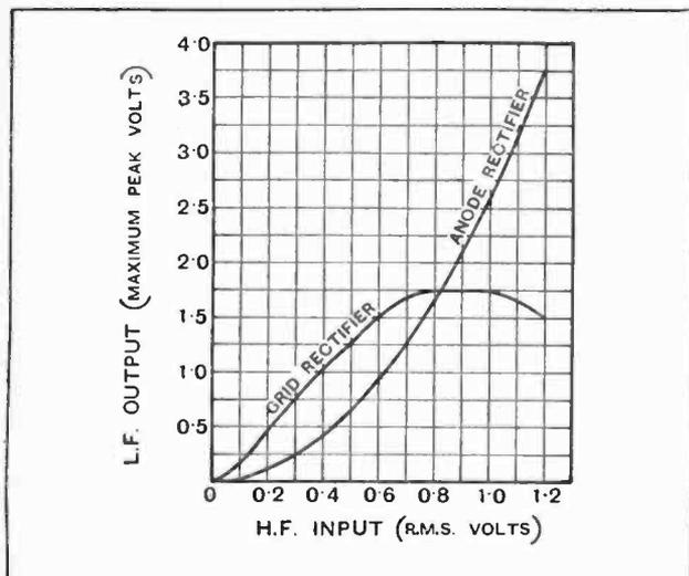
Fig. 5.—Curves showing actual L.F. peak-volts developed for various inputs of 20 per cent. modulation.
