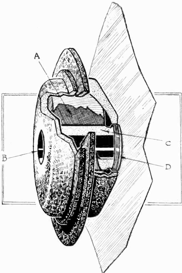
THE COIL DRIVEN DIAPHRAGM. A, field winding; B, ventilating hole through the pole; C, centre pole; D, moving coil attached to diaphragm.
