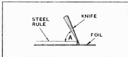
Fig. 1.—Constructing a simple fuse from tinfoil.
