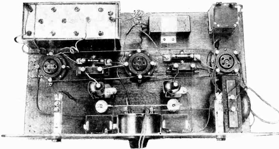
Plan view of the finished amplifier showing arrangement of parts and the easy method of wiring adopted.
