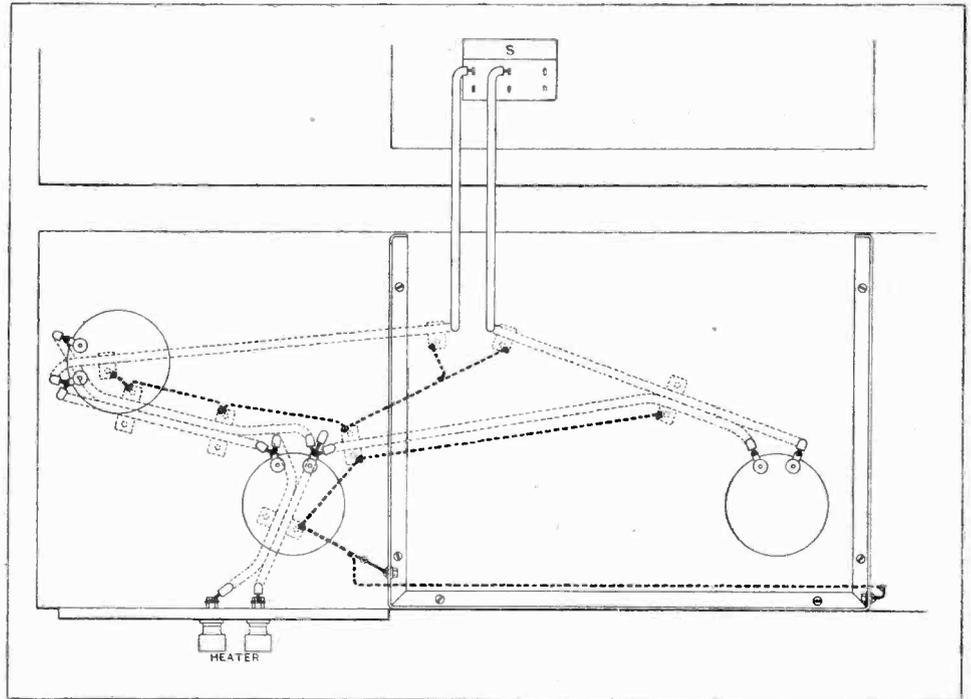
Fig. 10.—Wiring of the heater circuit. The thick dotted lines show the earthing leads to the clips holding the heater wiring.
