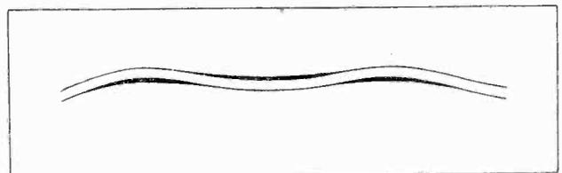
Fig. 3.—The result of artificially weighting the pick-up. Widening and rounding off the grooves have taken place.
