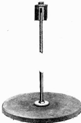
Holland earth plate constructed of porous carbon.
