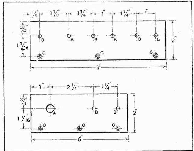
Fig. 6.—Terminal blocks. A, 3/8in. diameter; B, 5/32in.; C, 1/8in. countersunk for No. 4 wood screws.
