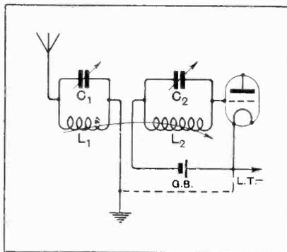
Fig. 1.—The connections of solenoid inductances in a tuned aerial coupler.
