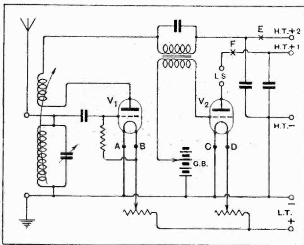
Diagram showing applications of a voltmeter and milliammeter.
