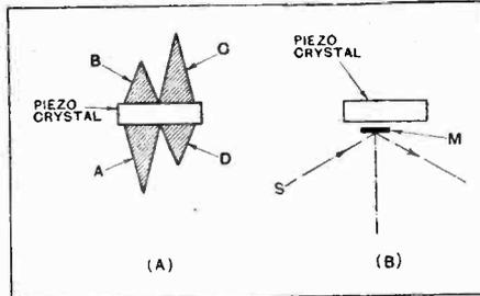
Method of indicating eddy-currents on surface of piezo-electric crystal. (No. 268,367.)
