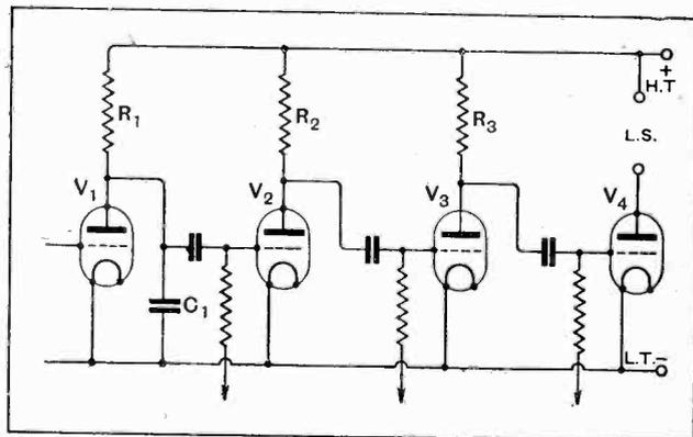
Fig. 10.—To avoid serious loss of high notes in a resistance amplifier and still retain good overall amplification it is necessary to employ three stages using low magnification valves and comparatively small anode resistances.  $R_1$ , 250,000 ohms;  $R_2$ ,  $R_3$ , 100,000 ohms;  $C_1$ , 0.0001 mfd.; coupling condensers 0.01 mfd.; leaks 5 megs.  $V_1$  (Det.) 50,000 ohms (makers' rating);  $V_2$ ,  $V_3$ , 15,000 ohms with mag. factor of 12;  $V_4$ , mag. factor 5.
