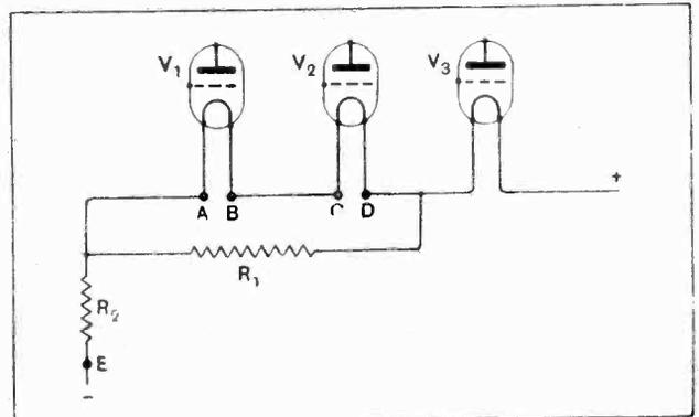
Fig. 3.—The method of obtaining negative grid bias when the filaments of the valves are connected in series.
