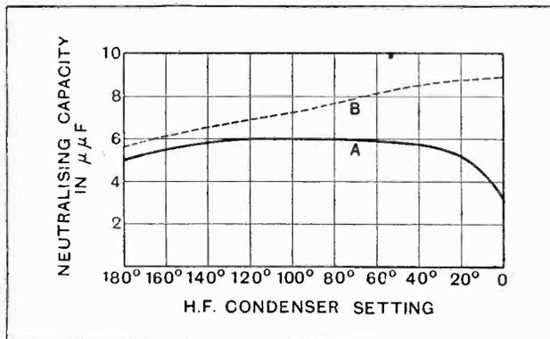
Fig. 12.—Neutralisation capacity plotted against the dial settings of the H.F. variable condenser. Curve A is for the high capacity outside aerial and curve B for the 6ft. indoor aerial. With a normal P.M.G. aerial the curve is practically a horizontal straight line.
