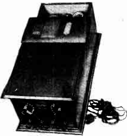
The Radille eliminator for A.C. mains is capable of providing half- or full-wave rectification as desired owing to the use of two half-wave valves.
