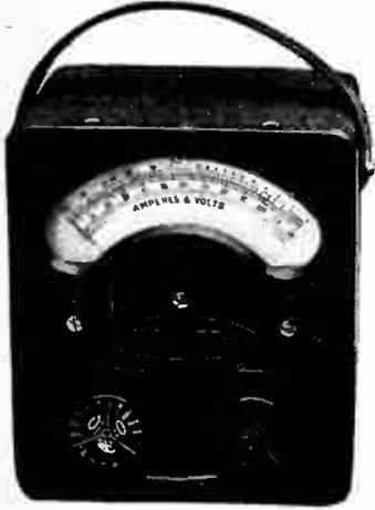
The Avometer, a universal testing instrument.
