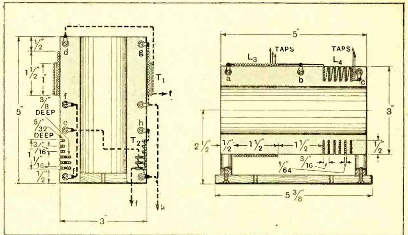
Fig. 4.—Sectional drawings showing construction of H.F. transformers and (right) long- and short-wave grid coils.
