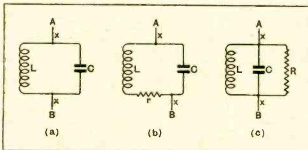
Fig. 1.—Three simple tuned circuits. In (a) there is no high-frequency resistance. In (b) the series resistance *r* represents the high-frequency resistance inseparable from any coil and condenser under practical conditions, whilst in (c) the resistance *r* has been replaced by *R* in parallel with *C*.
