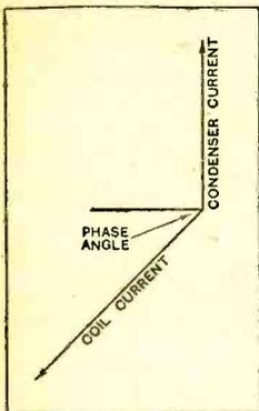
Fig. 2.—The condenser current leads the e.m.f. by 90° while the coil current lags by the phase angle.
