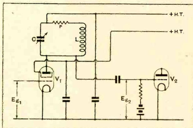
Fig. 4.—A screen-grid H.F. stage; to find the amplification obtainable we must use the dynamic resistance R in place of the series resistance  $r$ . The amplification =  $E_{g2}/E_{g1}$ .
