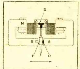
side. The pivot consists of a knife-edge let into the face of one magnet, and the reed is held against it by a small block of rubber.
