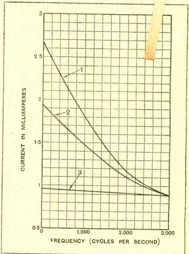
Fig. 6.—Curves showing current in the Lion loud speaker at various frequencies. Curve 1 = internal valve resistance = 3,000 ohms. Curve 2 = internal valve resistance = 5,000 ohms. Curve 3 = internal valve resistance = 40,000 ohms. It should be observed that there is practically no variation in current with the pentode (curve 3).
