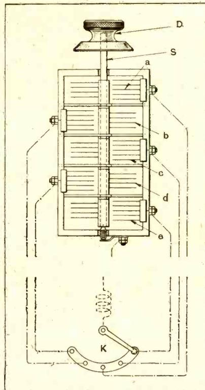
Switch-controlled selection of five differently tuned circuits. (No. 296,591.)
