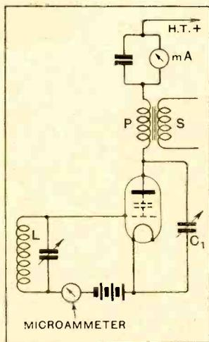
Fig. 9.—An experimental circuit to show the presence of an input load due to the interelectrode capacity of an anode bend detector.
