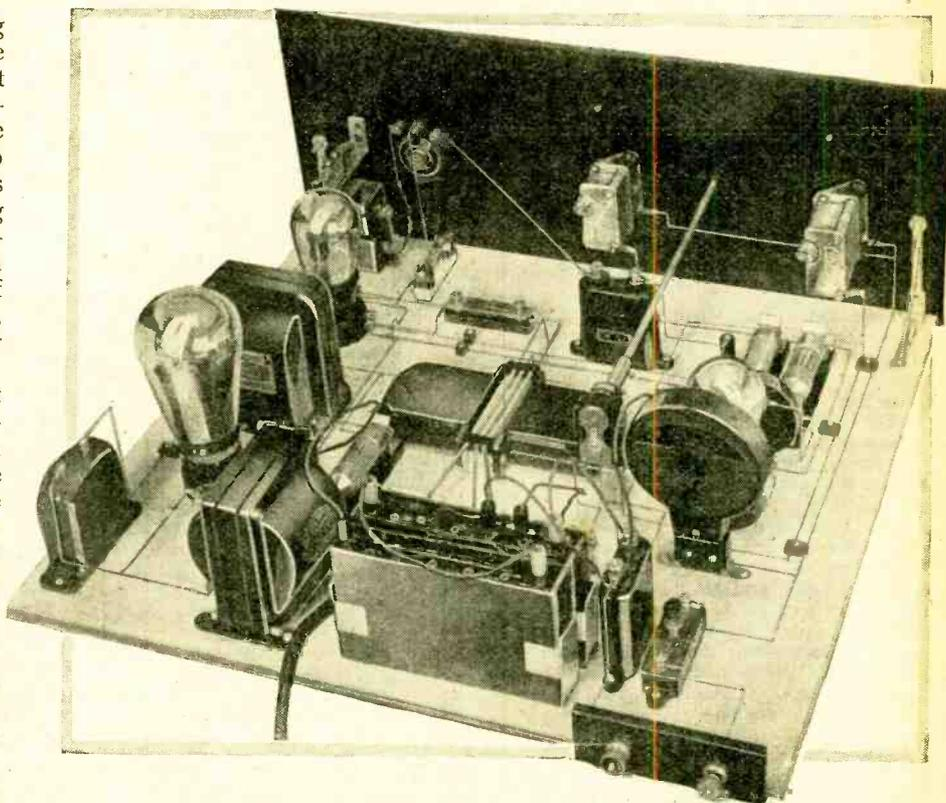
Rear view of the amplifier removed from the cabinet. Note the method of mounting the two 2 mfd. condensers to make room for the motor.
