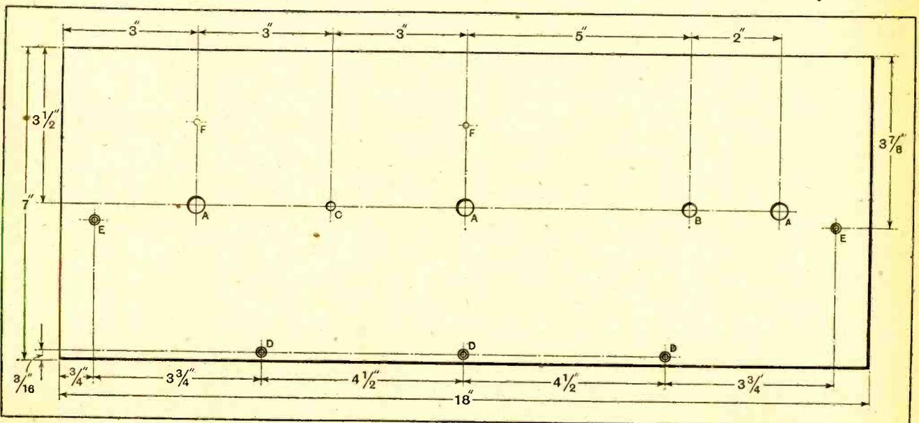
Fig. 2.—Dimensions and drilling data for the panel. A=3/8in. dia.; B=5/16in. dia.; C=3/16in. dia.; D=1/8in. dia., countersunk for No. 4 wood screws; E=1/8in. dia., countersunk for No. 6 B.A. screws; and F=1/8in. dia.
