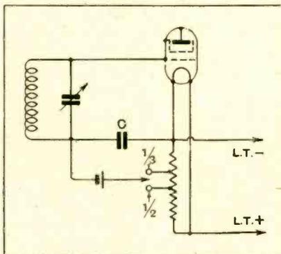
Fig. 1.—Use of tapped potentiometer for regulating grid voltage.
