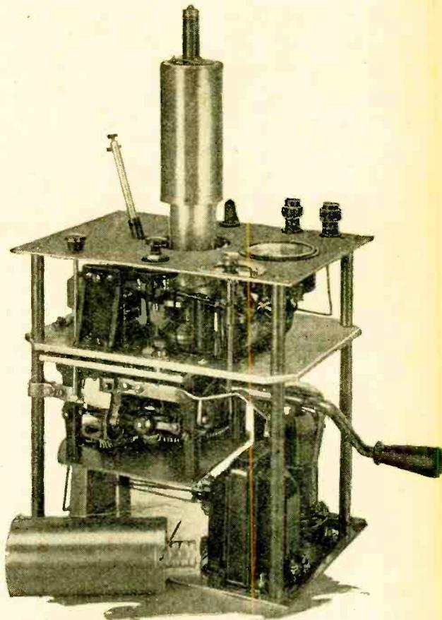
Case removed showing the sub-panel assembly. During reception a spare cylinder is loaded ready for dropping into position so as to avoid delay between successive pictures. Here the cylinder is removed exposing the inner driving drum.
