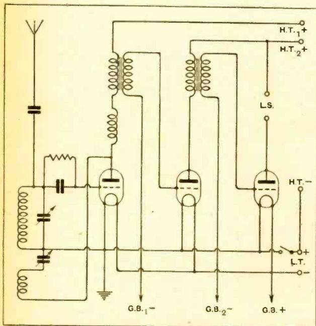
Fig. 1.—The circuit diagram, simplified by omission of waveband switching.
