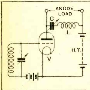
Fig. 10.—If the series resonance circuit CL across the primary of the transformer is tuned to the radio-frequency, the load on the input is released. Incidentally, CL short-circuits the H.F. component and prevents H.F. impulses from being amplified by the L.F. valve.
