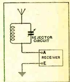
Fig. 3.—If a tuned circuit has no resistance it is a barrier to currents of the frequency to which it is tuned. The rejector circuit here shown makes use of this function.
