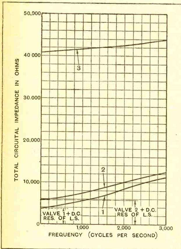
Fig. 5.—Curves showing total circuital impedance of valve and loud speaker. Curve (1) is for a valve whose internal resistance is 3,000 ohms. In curve (2) the valve resistance is 5,000 ohms, whilst in curve (3) the valve resistance is 40,000 ohms. By aid of the data in this diagram it is possible to calculate the current in the loud speaker at various frequencies.
