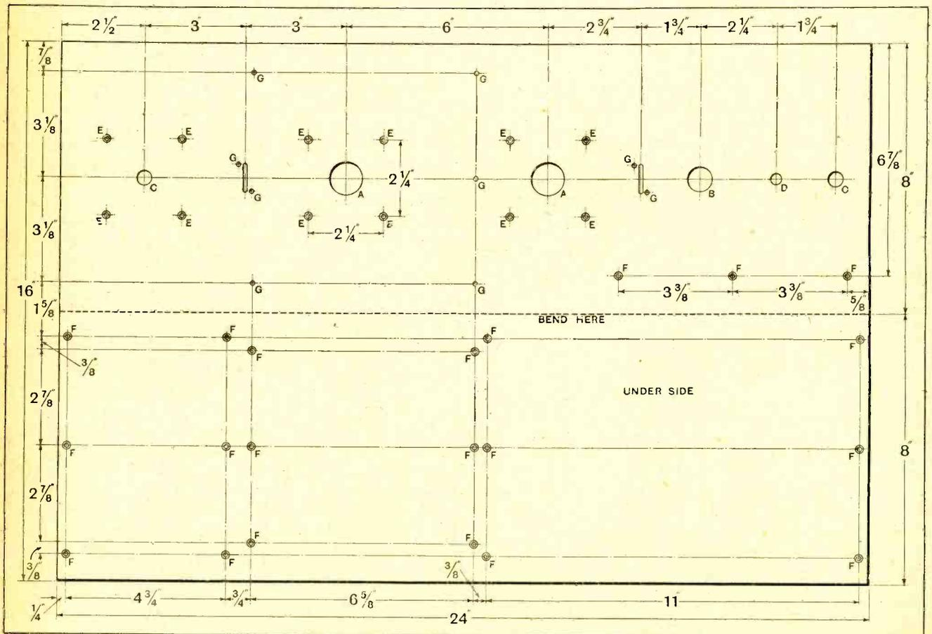
Fig. 5.—Drilling details of combined panel and base. A, 1in. dia.; B, 3/4in. dia.; C, 7/16in. dia.; D, 5/16in. dia.; E, 1/8in. dia., countersunk; F, 1/8in. dia., countersunk; G, 1/8 in. dia.
