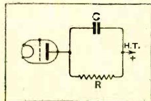
Fig. 1.—The anode load of an anode bend detector can be looked upon as a leaky condenser. The relation between C and R is important, for on it depends whether the audio-frequency envelope of the rectified carrier can be followed.
