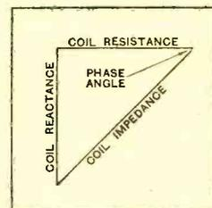
Fig. 4.—In a well-designed coil the phase angle is nearly 90° and the coil and condenser currents are nearly 180° out of phase. The slope in this diagram represents coil reactance/coil resistance.
