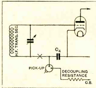
Fig. 1.—A short-circuited pick-up: It should be moved to the position marked X.
