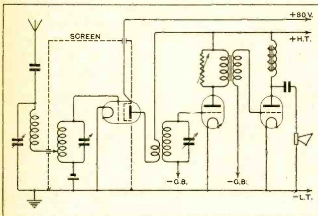
Fig. 1.—Simplified circuit diagram, without switching and decoupling devices.
