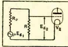
Fig. 6.—This scheme represents equally well either Fig. 4 or Fig. 5; in either case  $\mu + R_0$  stand for magnification factor and A.C. resistance of  $V_1$ , while R stands either for the dynamic resistance of the tuned circuit or the anode resistance of Fig. 5
