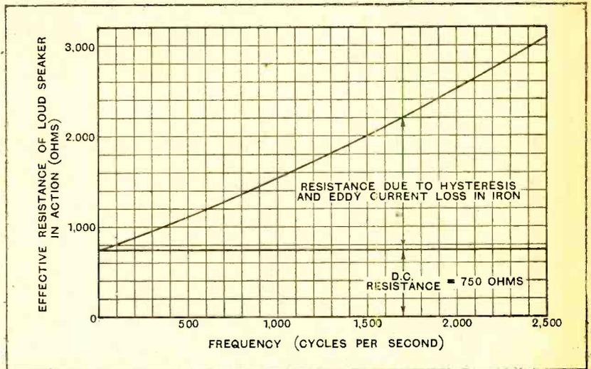
Fig. 3.—Curve showing effective resistance of the Lion loud speaker at various frequencies.
