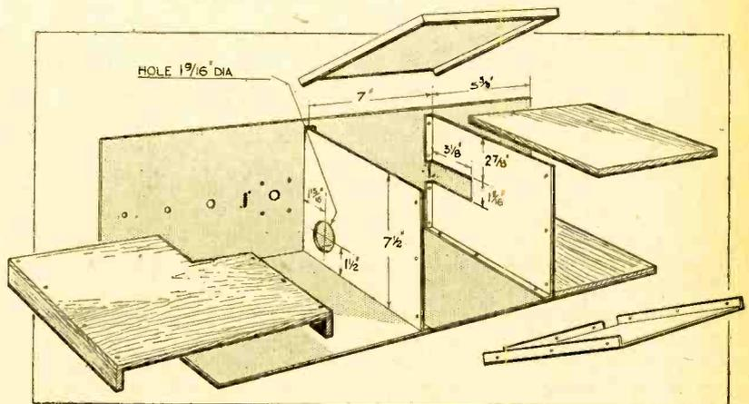
Fig. 3.—Construction of metal screens and baseboards.
