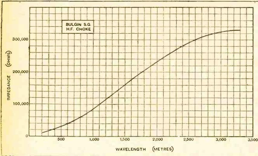
Impedance curve of Bulgin H.F. choke; external capacity 8 micro-mfd.
