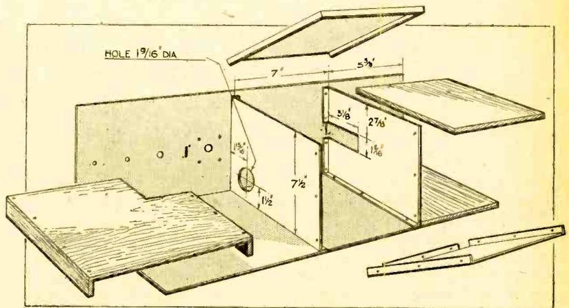
Fig. 3.—Construction of metal screens and baseboards.
