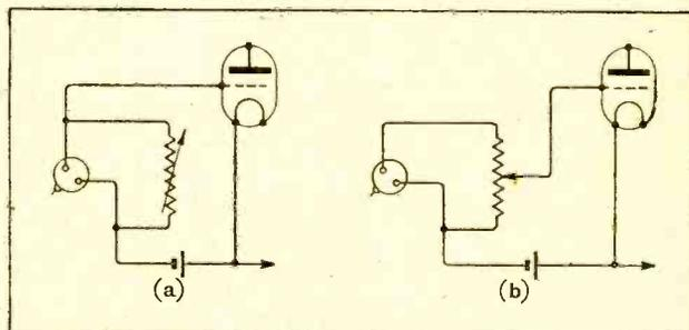
Fig. 4.—Parallel resistance and potentiometer methods of volume control.
