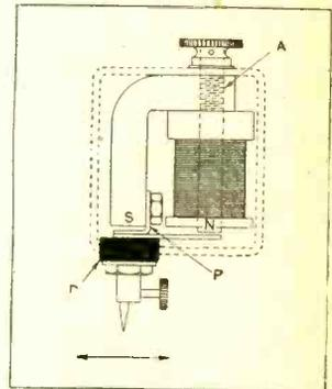
threaded core inside the pick-up coil, and the tests were carried out with the movement set for maximum sensitivity.
