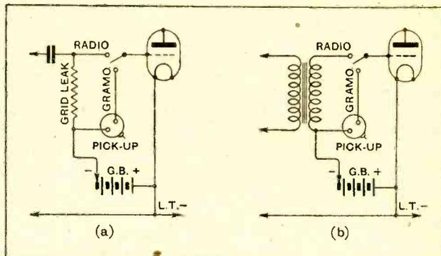
Fig. 3.—How to connect a pick-up to an L.F. amplifying valve.
