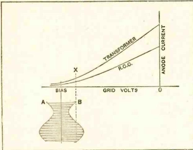
Fig. 5.—When applying a weak signal AB to an anode bend detector followed by a transformer the distortion is worse than when resistance coupling is employed. This is explained by the relative curvatures at X for two working valve characteristics. The increased impedance of the valve under these conditions makes transformer coupling again unsatisfactory.
