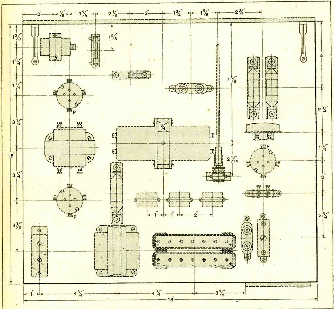
Fig. 3.—Layout of the components on the baseboard.
