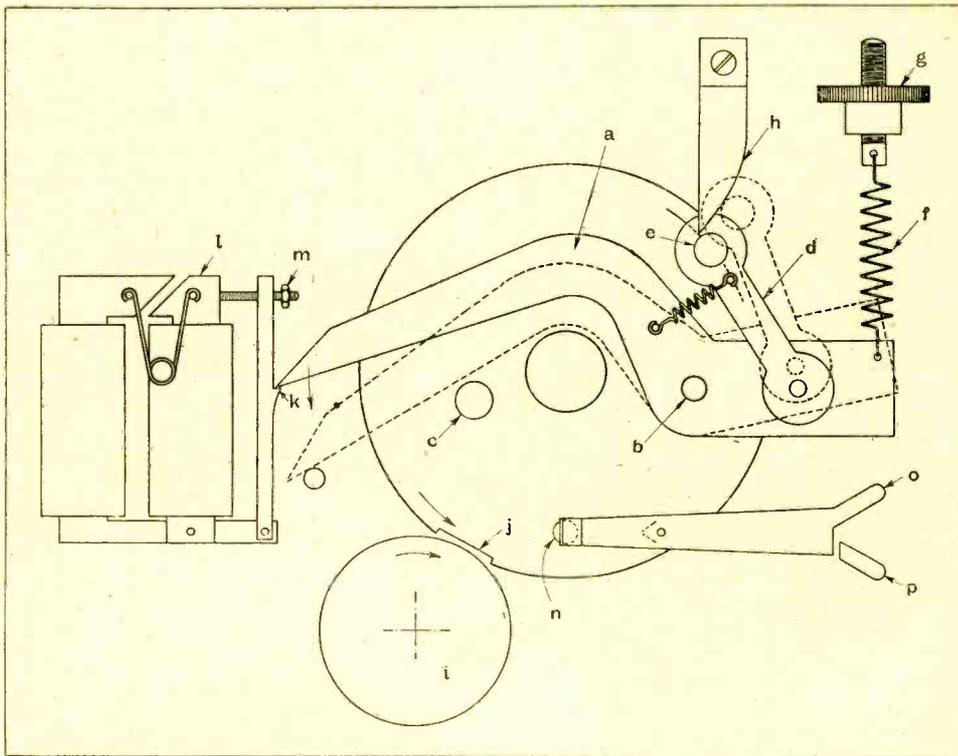
The starting mechanism. When the cylinder is stopped the driving motor is entirely relieved of load. A trigger action causes both wheels to be running at the same speed when engaging, so that the motor is not retarded by providing the starting load.
