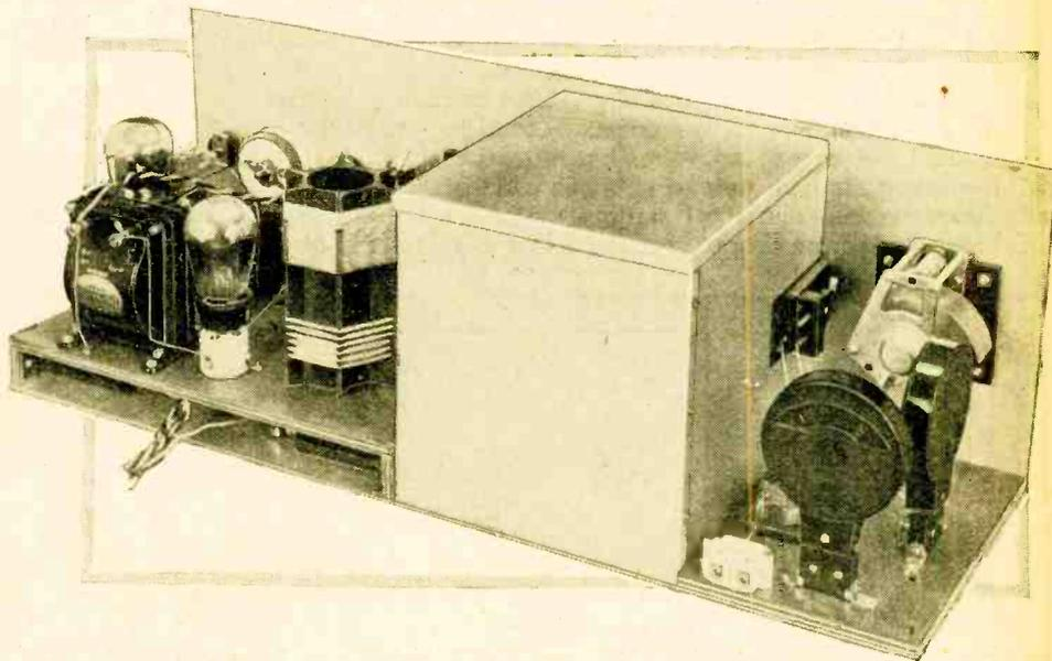
Rear view of the receiver. Note mounting of aerial-grid wave-change switch.
