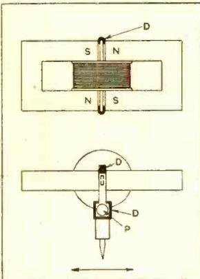
magnets, and the pick-up coil surrounds the armature. The dimensions of the unit are small, and the construction is unusually solid and compact. The output falls off gradually as the frequency is increased, and the general level requires three rather than two valves. At present the complete output of these pick-ups is being absorbed in the complete radio-gramophone sets made by this company.
