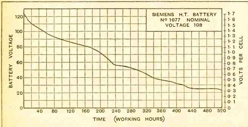
Discharge curve of the Siemens dry-cell H.T. battery Type No. 1,077.
