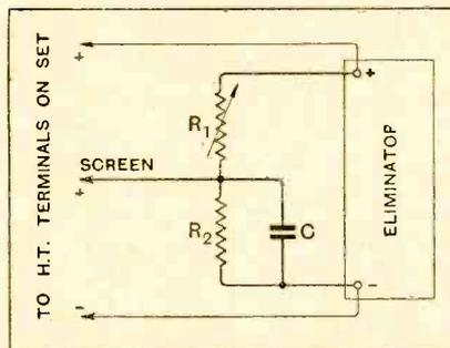
Fig. 1.—A potentiometer for screen grid voltage control.
