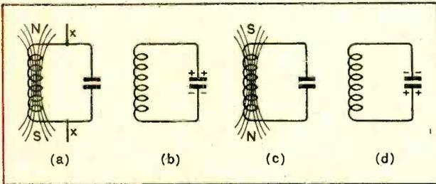
Fig. 2.—The cycle of events in a tuned circuit. The current flowing through the coil produces a magnetic field (a) and at the same time charges up the condenser (b); the current gradually ceases and the magnetic field around the coil vanishes. Now that the condenser plates are fully charged up, a current starts to flow through the coil in the opposite direction and creates a magnetic field with polarity reversed (c). At (d) the condenser plates are charged at an opposite polarity to (b).
