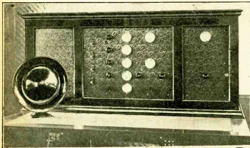
(Above) The combining receiver at the central station, and (below) the equipment at one of the substations of the receiving system.
