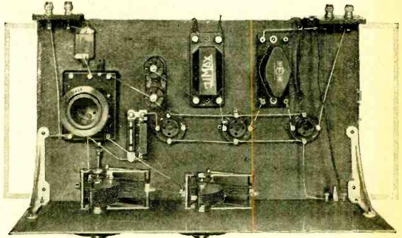
Plan view of the receiver, showing wide spacing of components and simplicity of wiring.
