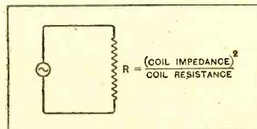
Fig. 5.—The equivalent of Fig. 1 when the circuit is tuned to the incoming frequency.
