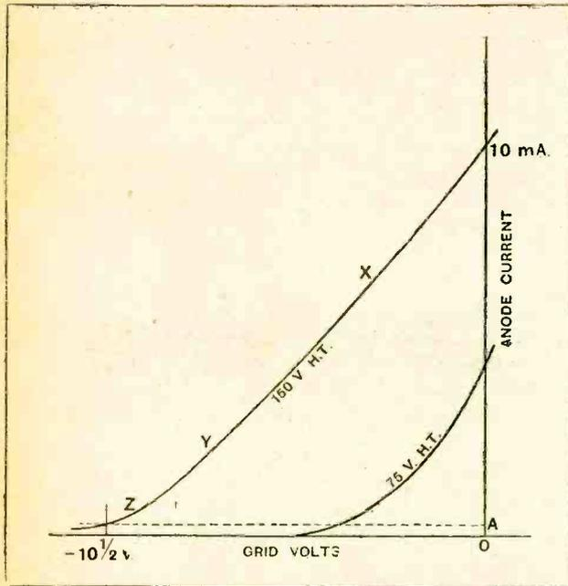
Fig. 3.—Two valve characteristics for typical modern anode bend detectors such as the PMD or DEL series. The 150-volt curve is sensibly straight for the greater part of its length whilst the 75-volt curve has no straight portion and is not suitable for anode bend detection.
