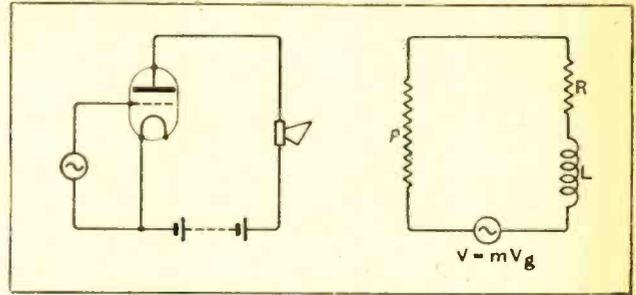
Fig. 7.—Diagram showing equivalent circuit of valve and loud speaker. V is the voltage of the fictitious alternator;  $\rho$  the internal A.C. valve resistance; R the effective resistance of loud speaker, and L the effective inductance of the loud speaker.
