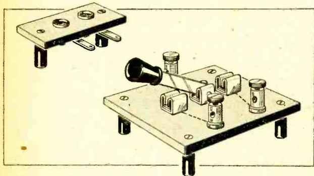
Fig. 2.—Terminal block and switch for baseboard mounting.
