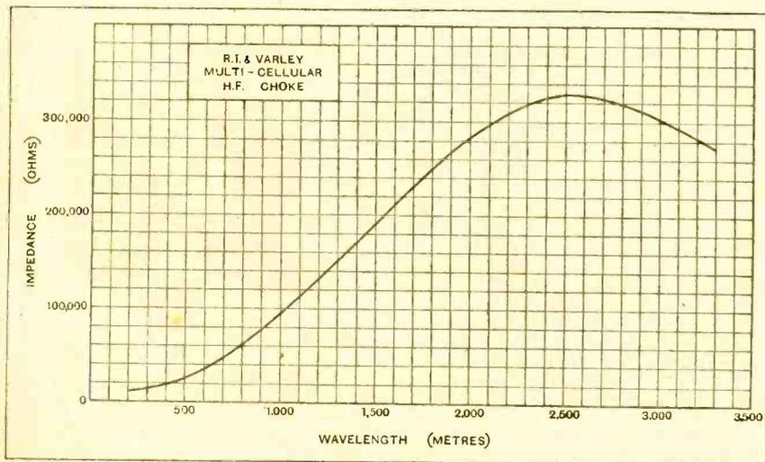
Impedance curve of the R.I.-Varley Multi-Cellular H.F. choke; external capacity 8 micro-mfd.
