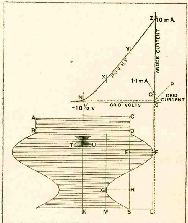
Fig. 4.—Diagram showing the application of a 10-volt (peak) 50% modulated carrier wave to an anode bend detector. Note that the total modulated swing ML is  $\frac{2}{3}$  of the peak KL.
