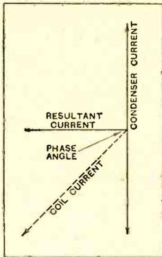
Fig. 3.—The coil current (dotted line) can be resolved into a horizontal and a vertical component.
