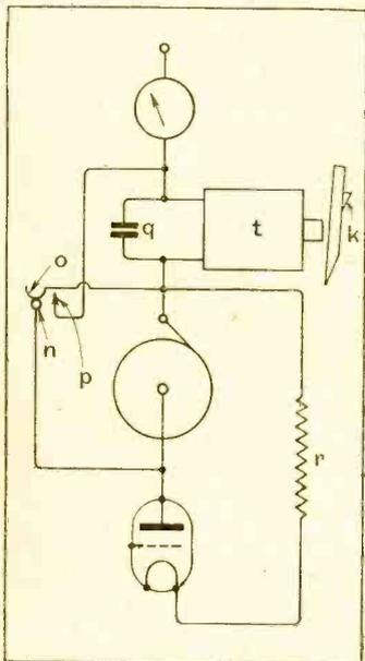
Anode circuit of the Colvergraph. The resistance provides the current for the threshold trigger adjustment. The use of a relay is abandoned. Only a single switch-over contact is needed.
