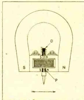
This surmise is confirmed by test, and the output at 4,000 cycles is practically the same as at 250 cycles. The movement is lightly damped, and record wear is very low. In every respect a first-class job.
