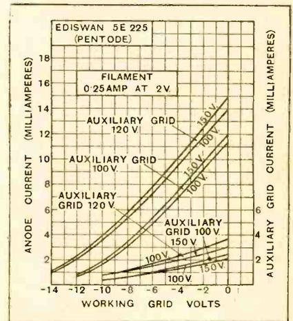
Average values, A.C. resistance, 83,000 ohms; amplification factor, 83; mutual conductance, 1mA./volt; under normal working conditions.
