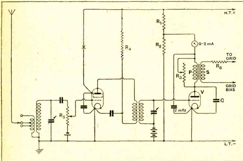
Fig. 8.—A suggested circuit containing a screen-grid valve followed by an anode bend detector. For local station reception pre- and post-detector volume controls ( $R_5$  and  $R_3$ ) are advised.
