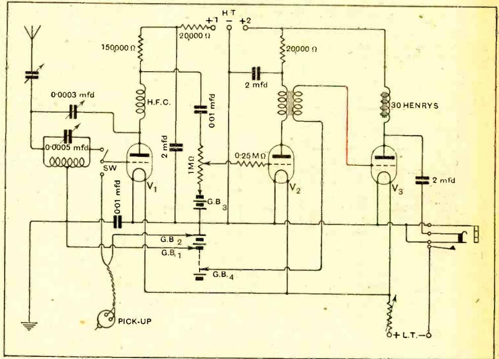
Fig. 1.—The theoretical circuit diagram. The semi-fixed aerial condenser is variable between 0.00025 mfd. and 0.0003 mfd.
