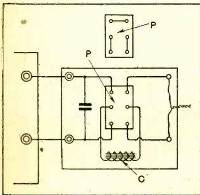
Method of switching a smoothing choke in a D.C. eliminator. (No. 300,383.)
