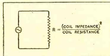
Fig. 5.—The equivalent of Fig. 1 when the circuit is tuned to the incoming frequency.
