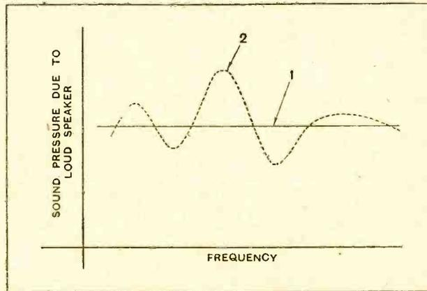
Fig. 1.—Hypothetical diagram showing response curves of ideal loud speaker; (1) in a perfectly damped room, (2) in an ordinary room where standing waves occur.
