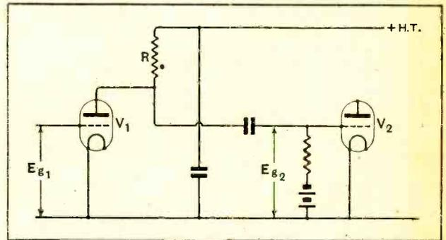
Fig. 5.—In this amplifier  $R$  fulfils exactly the role of the tuned circuit in Fig. 4; the two may be treated in exactly an identical manner.
