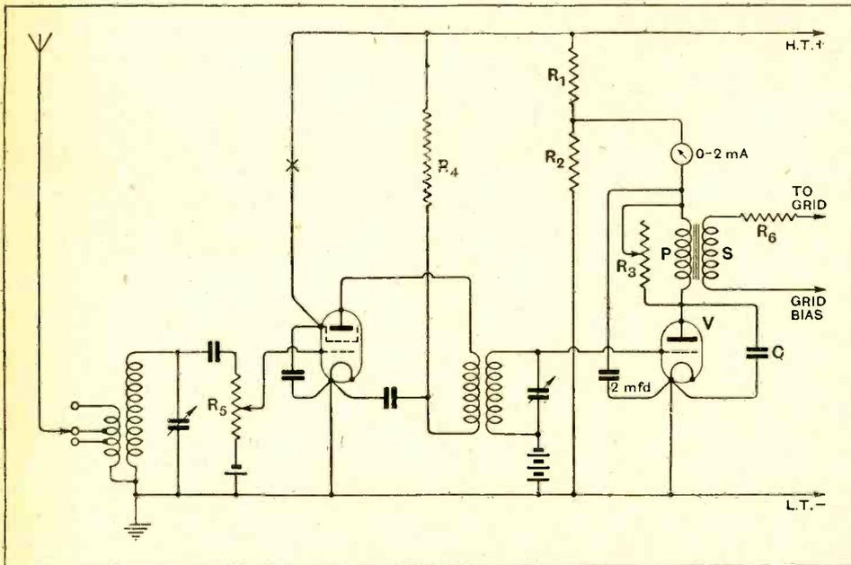
Fig. 8.—A suggested circuit containing a screen-grid valve followed by an anode bend detector. For local station reception pre- and post-detector volume controls ( $R_2$  and  $R_3$ ) are advised.
