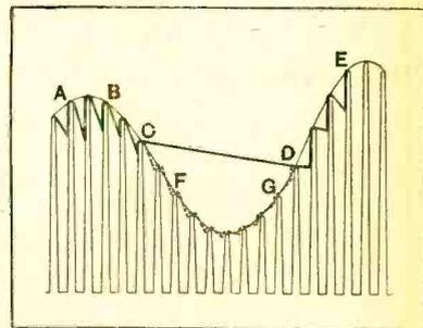
Fig. 2.—When the anode condenser is large and the leak has a high value (see Fig. 1) the energy cannot leak away fast enough, resulting in some such discharge as A B C D E. If the leak has a low value, such as in transformer coupling, the envelope A B F G E of the modulated carrier is followed more faithfully.
