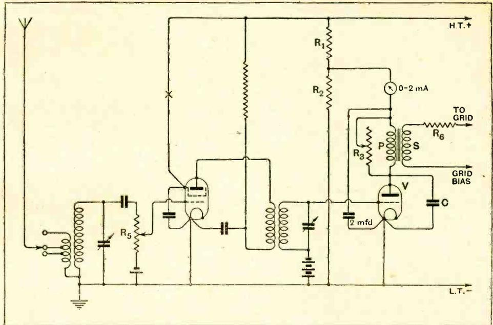
Fig. 7.—A suggested circuit to create large inputs for an anode bend detector. Constant maximum input without running into grid current is assured by the milliammeter, while the volume control  $R_4$  prevents overloading of the third valve (not shown).
