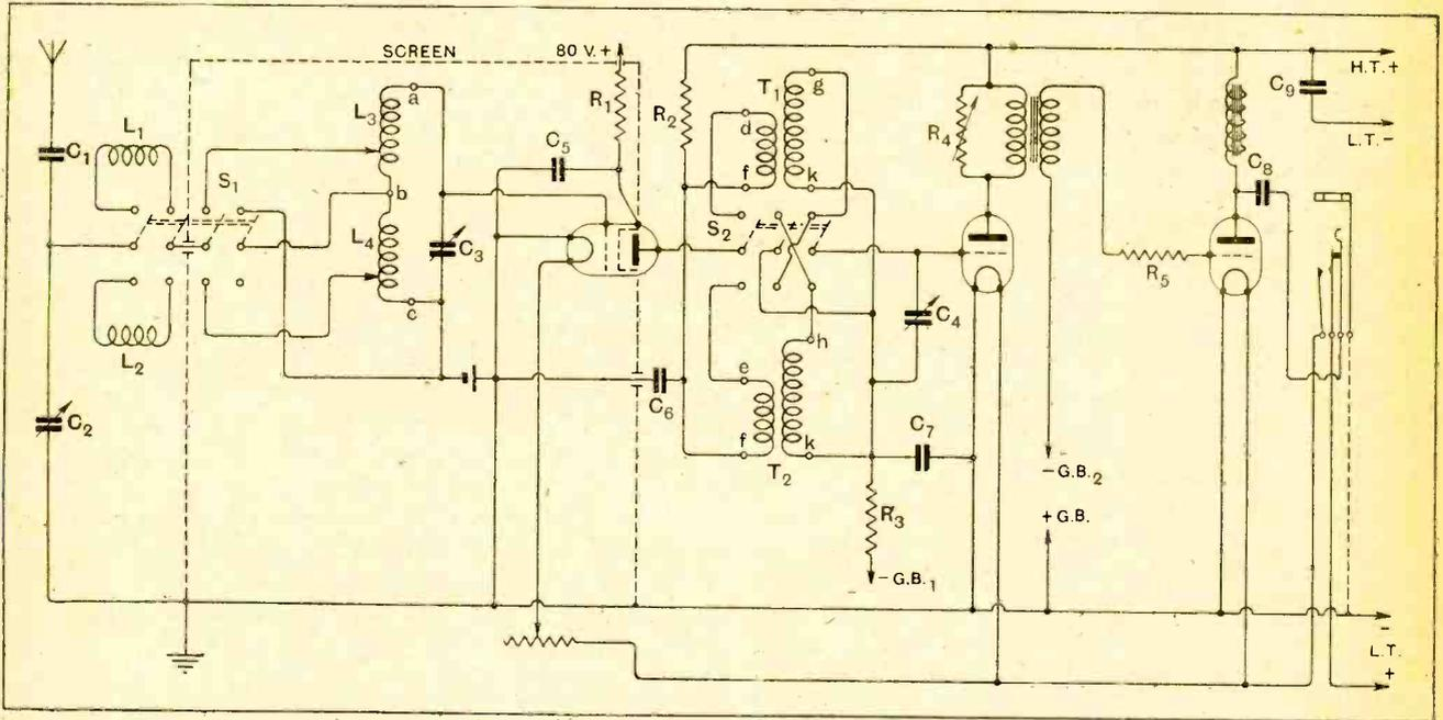
Fig. 2.—Complete circuit diagram.  $C_1, 0.00025$  mfd.;  $C_2, 0.0005$  mfd.;  $C_3, C_4, 0.0003$  mfd.;  $C_5, C_6, C_8, C_9, 2$  mfd.;  $C_7, 1$  mfd.  $L_1, L_2$ , aerial loading coils;  $L_3$ , short-wave grid coil;  $L_4$ , long-wave grid coil.  $T_1$ , short-wave H.F. transformer;  $T_2$ , long-wave H.F. transformer.  $R_1, R_2$ , decoupling resistances, 600 ohms;  $R_3, 20,000$  ohms;  $R_4$ , volume control resistance;  $R_5, 100,000$  ohms.
