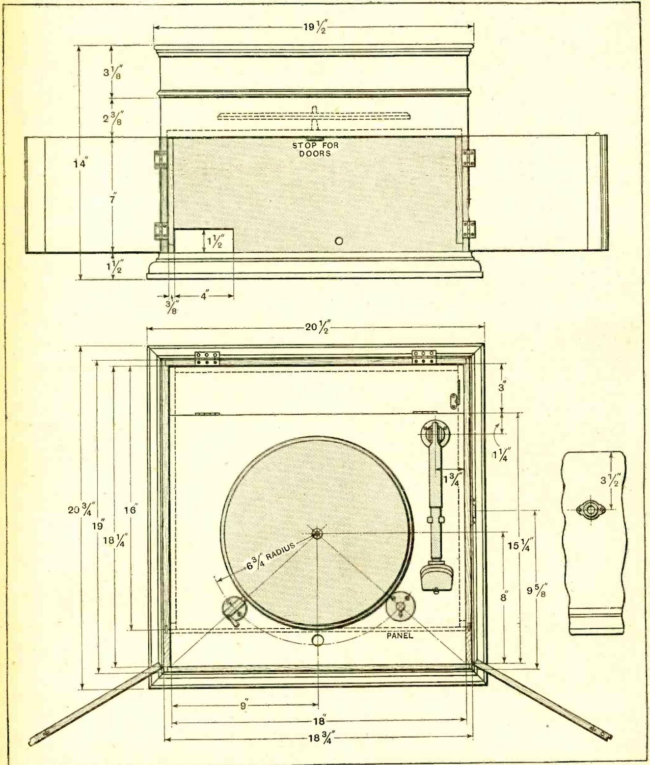
Dimensional drawing of the cabinet showing the position of the turntable and sub-deck fixtures.
