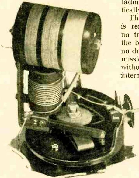
Close-up view of aerial tuner and selector switch.
