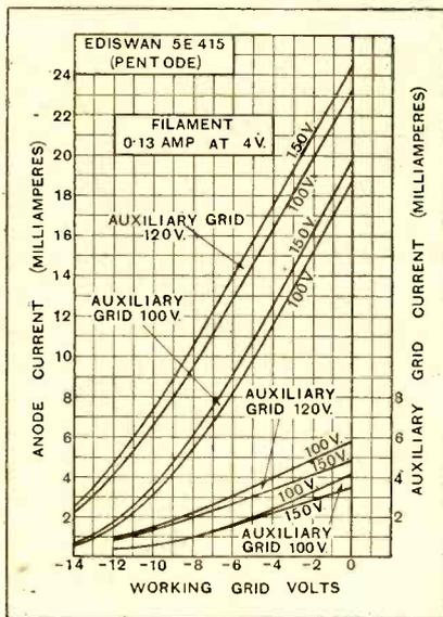
Average values, A.C. resistance, 59,000 ohms; amplification factor 83; mutual conductance, 1.4mA./volt, under normal working conditions.
