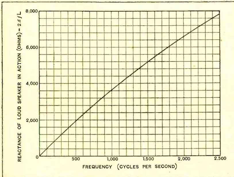
Fig. 2.—Curve showing reactance ( $2\pi fL$ ) of Lion loud speaker at various frequencies.
