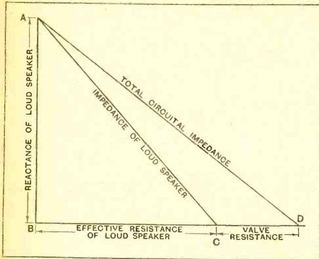
Fig. 4.—Vector diagram illustrating method of obtaining total circuital impedance of valve and loud speaker.
