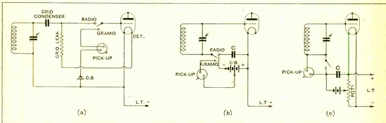
Fig. 1.—Converting the detector for amplification: methods of connecting a pick-up in its grid circuit.
