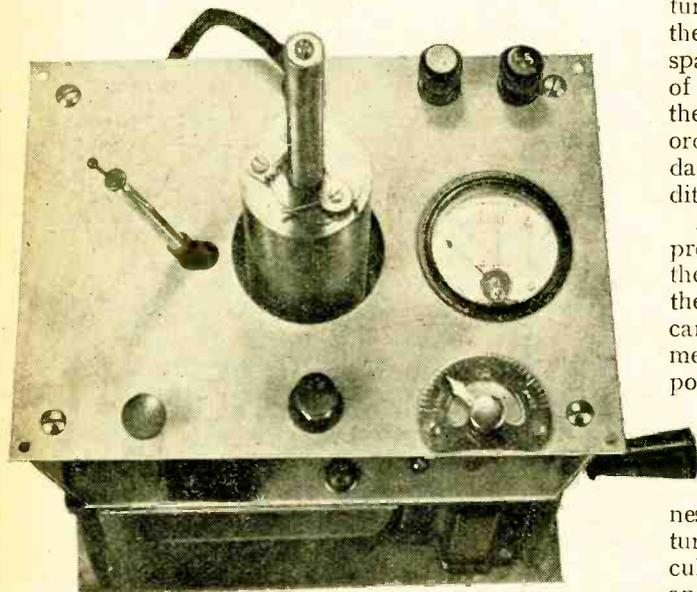
Plan view with paper-carrying cylinder withdrawn. Space is left on the top panel for accommodating other forms of recording gear than the electrolytic stylus. The stylus is stationary.
