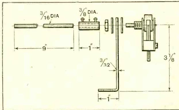
Details of the switch showing extension rod and bracket.
