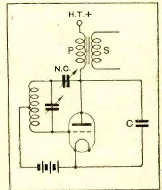
Fig. 11.—A neutralised anode bend detector. Input loading is prevented.
