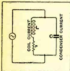
Fig. 1.—An alternator supplies current to a parallel tuned circuit; part of the total current passes through the coil and part through the condenser.
