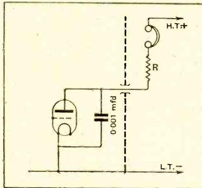
Fig. 1.—Locating instability: modified detector anode circuit.
