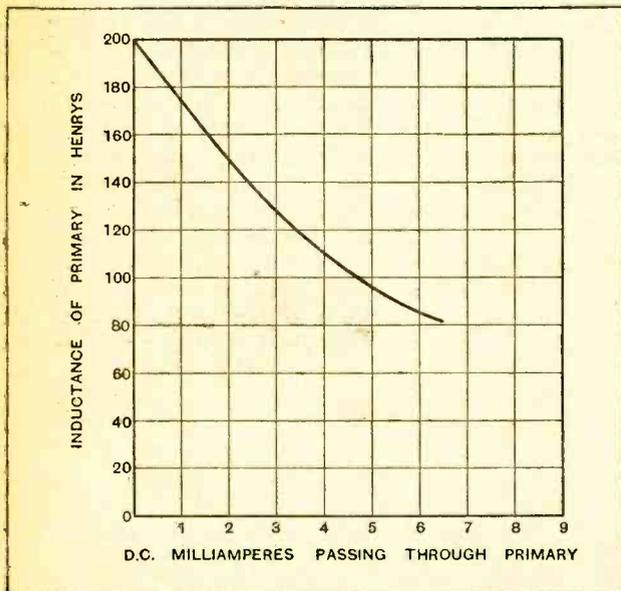
Fig. 6.—With the small anode current of 1 to 2 mA. passed by an anode bend detector the primary inductance of an interval transformer is not appreciably reduced. The curve is for an AF5 transformer.
