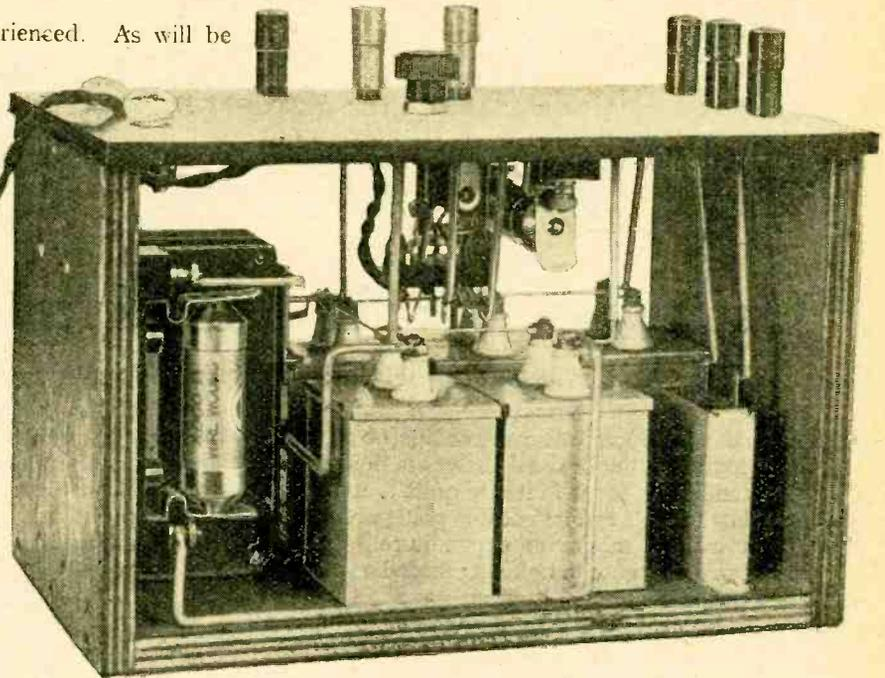
View of interior showing double-pole change-over switch.
