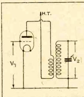
Fig. 1.—Skeleton diagram of H.F. stage using a transformer. The input voltage is  $V_1$ , the output voltage (to next valve) is  $V_2$ . The ratio  $V_2/V_1$  is the amplification afforded by the stage.
