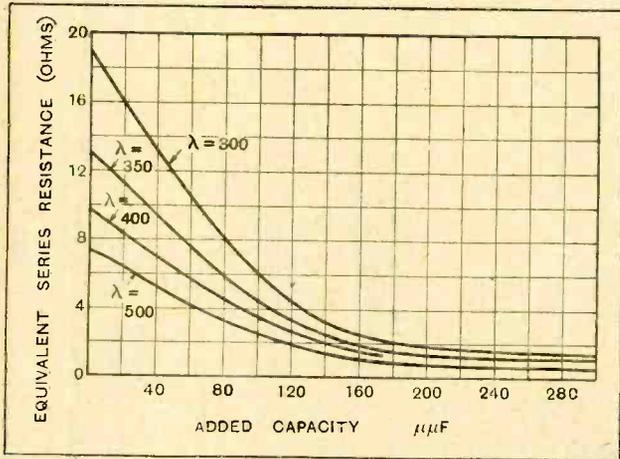
Fig. 9.—The results of Fig. 7 plotted on a capacity base for a number of fixed wavelengths.
