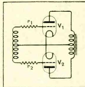
Fig. 25.—Diagram showing method of curbing parasitic oscillations in push-pull circuit.  $r_1$   $r_2$  are resistances to damp out parasitic oscillations of the two types described in the text.
