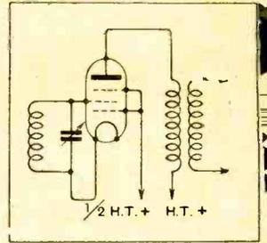
Fig. 8.—A triple-grid valve with five contacts.
