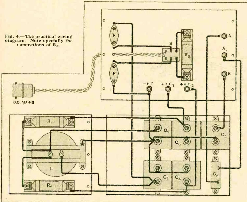
Fig. 4.—The practical wiring diagram. Note specially the connections of  $R_3$ .
