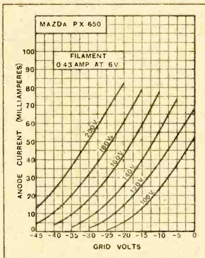
Average values under amplifying conditions; A.C. resistance, 1,600 ohms; amplification factor, 3.4; mutual conductance, 2.1 mA. per volt.
