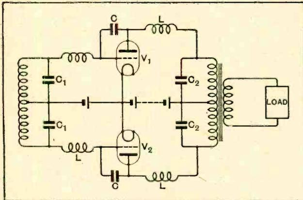
Fig. 18.—Showing arrangement of two valves in push-pull fashion, with coil ( $C_1 C_2$ ) and electrode capacities ( $C$ ) and inductance of leads ( $L$ ).
