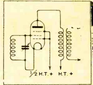
Fig. 8.—A triple-grid valve with five contacts.
