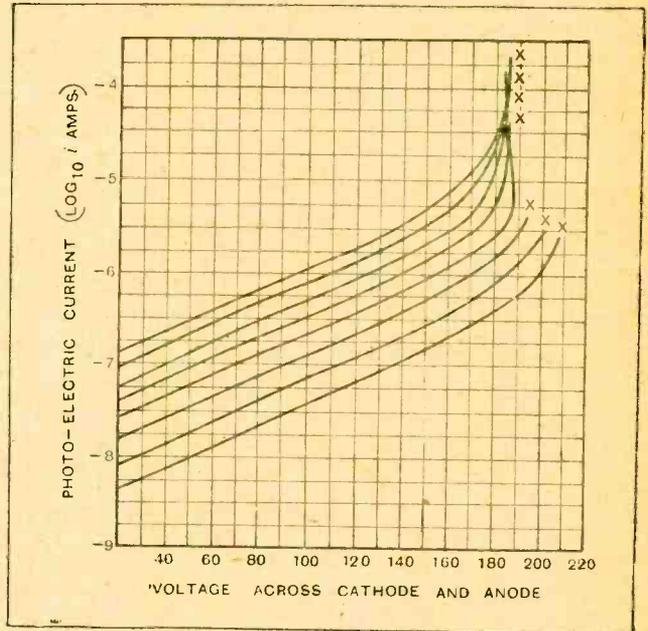
Fig. 2.—Curves showing relation between photo-electric current and anode-cathode voltage for various light intensities falling on the cell.
