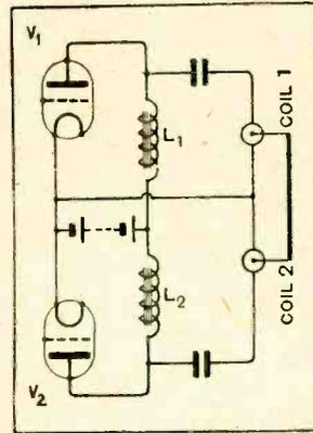
Fig. 15.—Diagram showing arrangement of output circuit when two magnetically separate but mechanically coupled high-resistance coils are used.
