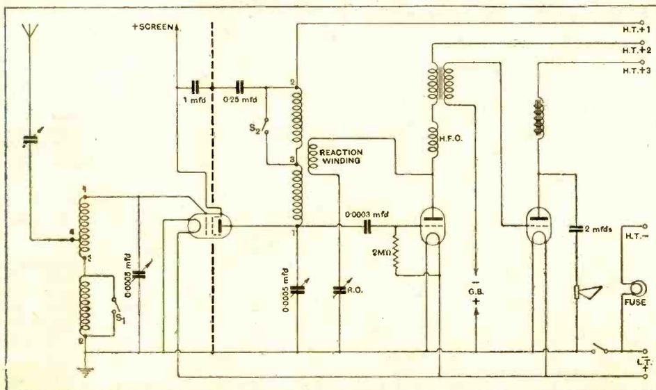
Fig. 1.—Complete circuit diagram. Numbering of the coil terminal points corresponds with the markings on the bases.
