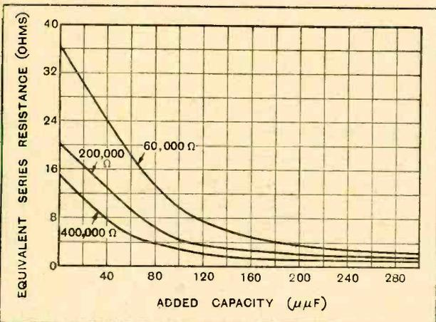
Fig. 3.—Relation between anode circuit capacity and equivalent series resistance of detector, for various values of external anode resistance. It should be noted that the equivalent series resistance due to the feed-back has a more marked effect on low-loss coils.
