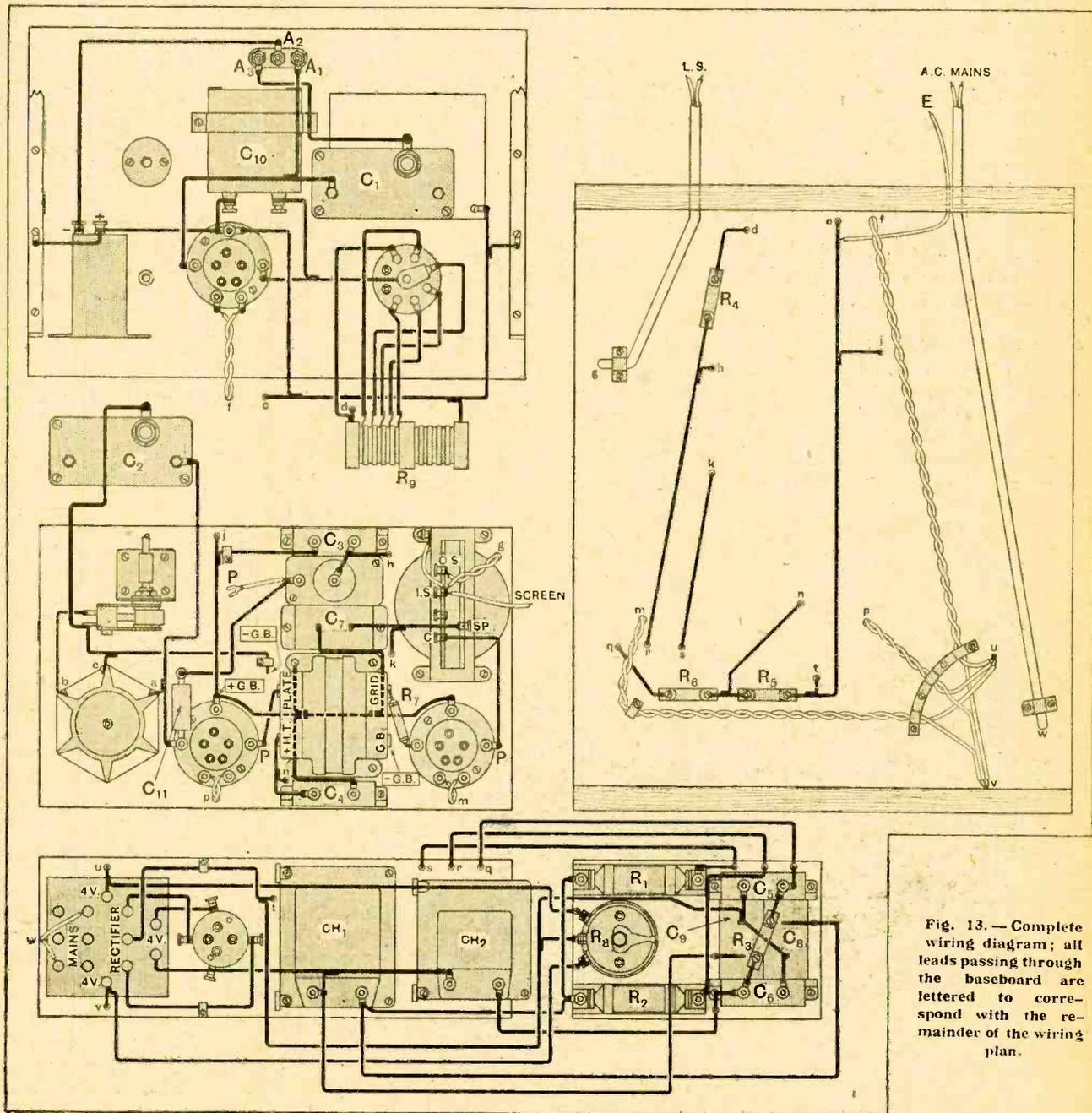
Fig. 13.— Complete wiring diagram; all leads passing through the baseboard are lettered to correspond with the remainder of the wiring plan.
