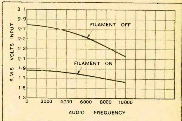
Fig. 11.—The upper curve shows the audio frequency characteristic of the input circuit unloaded by the detector. The lower curve shows the characteristic as modified by feed-back when the detector is in operation. Anode resistance 60,000 ohms; added capacity 135 micromicrofarads; wavelength 240 metres.
