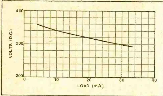
Fig. 5.—Regulation curve of Met-Vick combined "A" and "B" transformer and S.P. 42/U valve.
