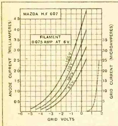
Average values under amplifying conditions: A.C. resistance, 19,000 ohms; amplification factor, 18.2; mutual conductance, 0.96 mA. per volt.
