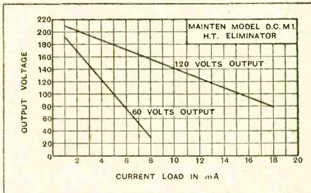
Voltage regulation curves of the D.C.M.1 model. Measurements were made of each output voltage under load separately.
