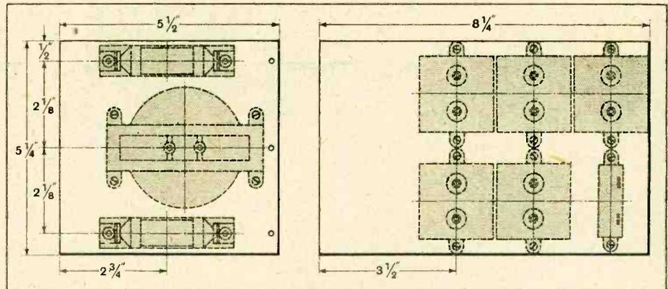
Fig. 3.—Layout of baseboard and side panel.
