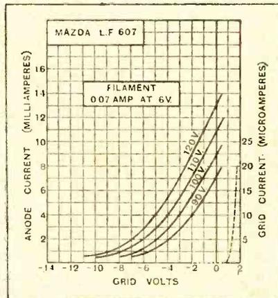
Average values under amplifying conditions: A.C. resistance, 6,700 ohms; amplification factor, 8; mutual conductance, 1.2 mA. per volt.
