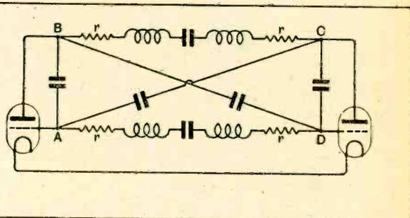
Fig. 29.—Showing damping resistances r in anode and grid circuits. It will be seen that each circuit has at least a damping resistance 2r.
