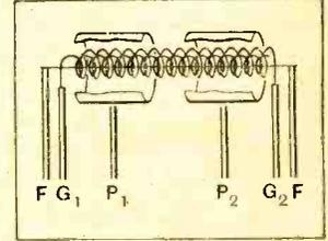
Fig. 10.—A two-plate, two-grid valve, type two.
