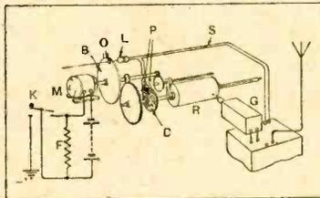
Schematic diagram showing synchronising equipment for picture reception.
