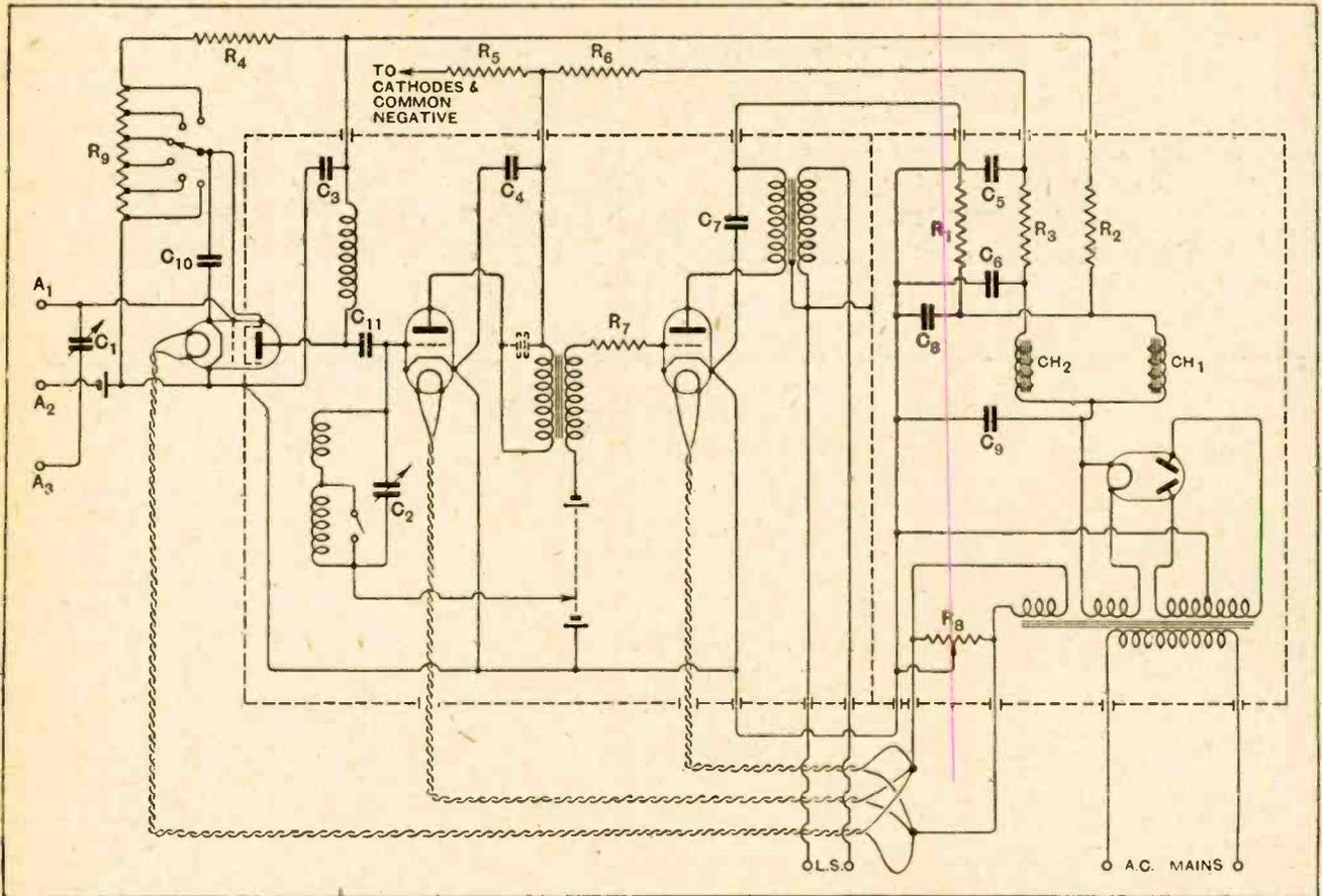
Fig. 14.—Complete circuit diagram.  $C_1, C_2 = 0.0005$  mfd. variable;  $C_3, C_4, C_5, C_6, C_7, C_8, C_9, C_{10} = 1$  mfd. (400v. D.C.);  $C_{11} = 2$  mfd. (25 A.C.);  $C_{12} = 2$  mfd. (Ferranti Type  $C_2$ , 500v. D.C.);  $C_{13} = 0.0002$  mfd.;  $R_1 = 8,000$  ohms, wire wound;  $R_2, R_3, R_4, R_5, R_6 = 25,000$  ohms, moulded;  $R_7 = 0.25$  megohms;  $R_8 = 400$  ohms;  $R_9 = 20,000$  ohms;  $CH_1 = 22/50$  henrys (50 mA.);  $CH_2 = 20/48$  henrys (7 mA.).
