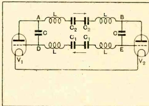
Fig. 20.—Circuit of Fig. 19 simplified by redrawing and omitting the connection from the junction of  $C_2C_2$  and of  $C_1C_1$  to the common filament lead. A B E D is an oscillatory circuit of supersonic frequency.
