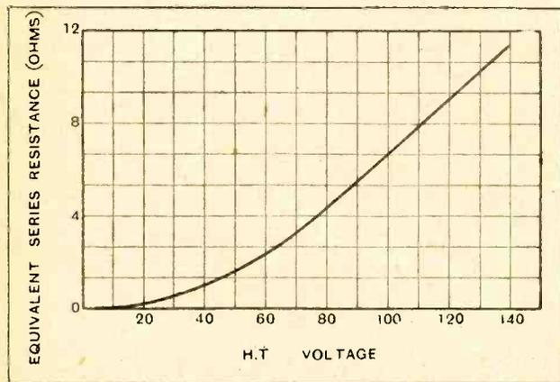
Fig. 6.—Effect of H.T. voltage on the input load of curvature detector. External anode resistance 60,000 ohms; added shunt capacity 135 micromicrofarads; wavelength 240 metres.
