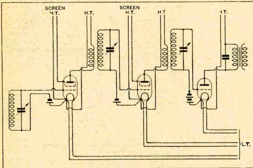
Fig. 2.—Individual feeds for each anode and screening-grid circuit, combined with non-inductive grid connections: scientific wiring as applied to a set with two screen-grid H.F. valves.
