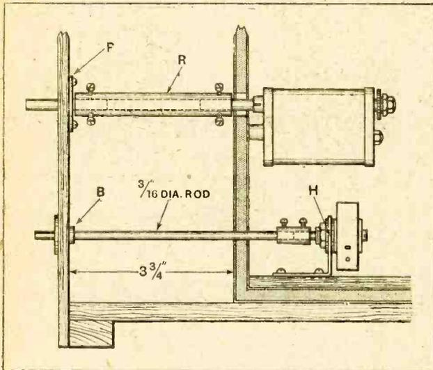
Fig. 9.—Details of extension rods for variable condenser and wave range switch. The diameter of the hole H in the switch bracket should be oversize to allow movement for centring.
