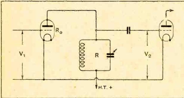
Fig. 4.—In this tuned anode circuit the overall amplification  $V_2/V_1 = \frac{\mu R}{R + R_0}$
