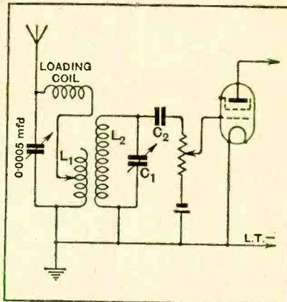
Fig. 1.—Tuned auto-coupled aerial circuit for the "Megavox" receiver.
