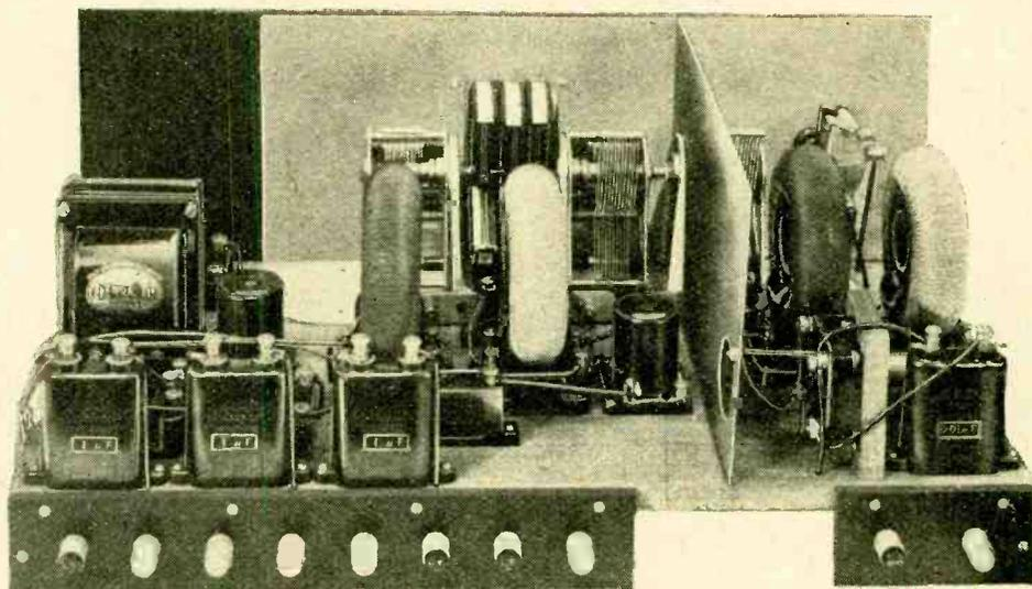
Rear view of receiver. Note triple condenser assembly, horizontal H.F. valve mount, and metal screen behind panel.
