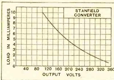
Voltage regulation curve from H.T. + 2 socket with vibrator adjusting lever at "maximum" setting.
