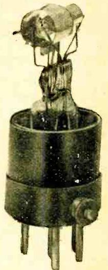
A typical two-grid, two-plate valve.
