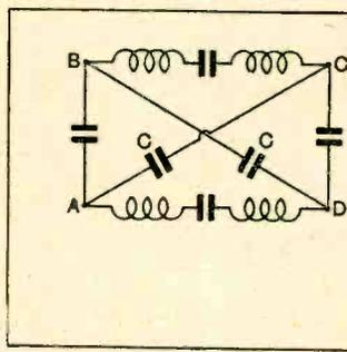
Fig. 28.—Showing additional circuits ABC, ACD, ABD, BCD introduced by neutrodyne condensers CC of Fig. 27.
