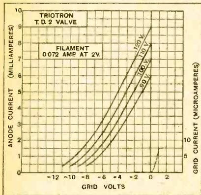
Average values under working conditions:—A.C. resistance, 11,700 ohms; amplification factor, 11; mutual conductance, 0.94 mA/volt.
