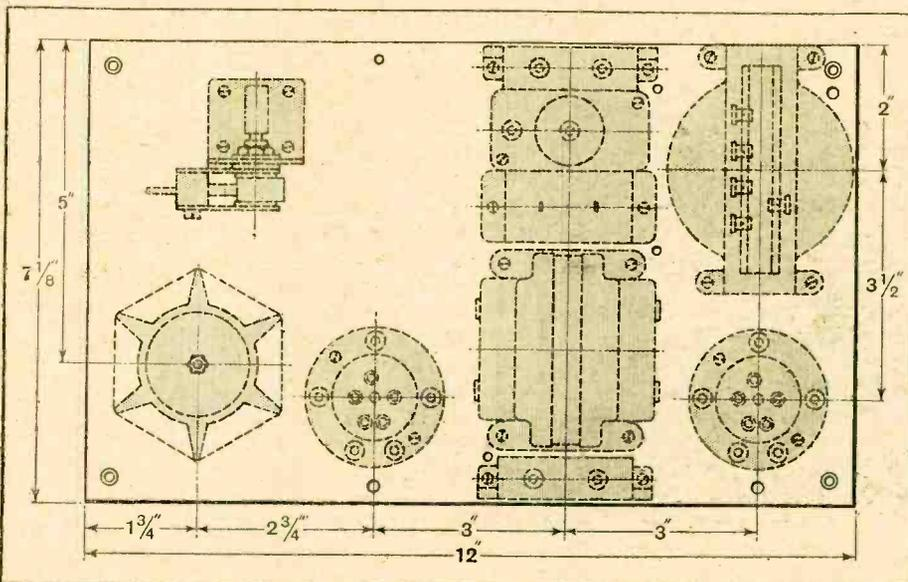
Fig. 11.—Layout of parts on the receiver sub-base.
