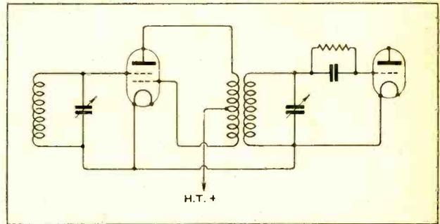
Fig. 3.—"Isodyne" circuit for high-frequency amplification.
