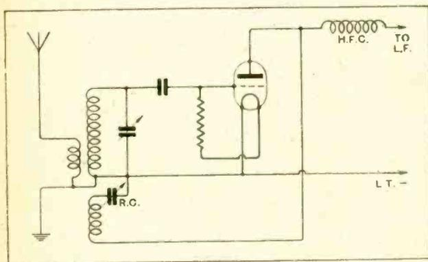
Fig. 1.—A conventional detector circuit with capacity-controlled reaction.
