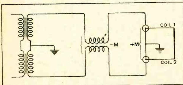
Fig. 14.—Circuit arrangement for annulling any electromagnetic coupling between coils of Fig. 13.
