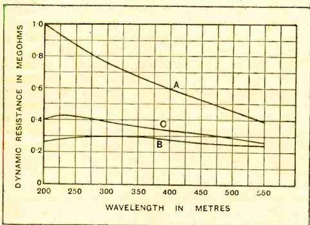
Fig. 4.—Curves showing frequency plotted against dynamic resistance.
