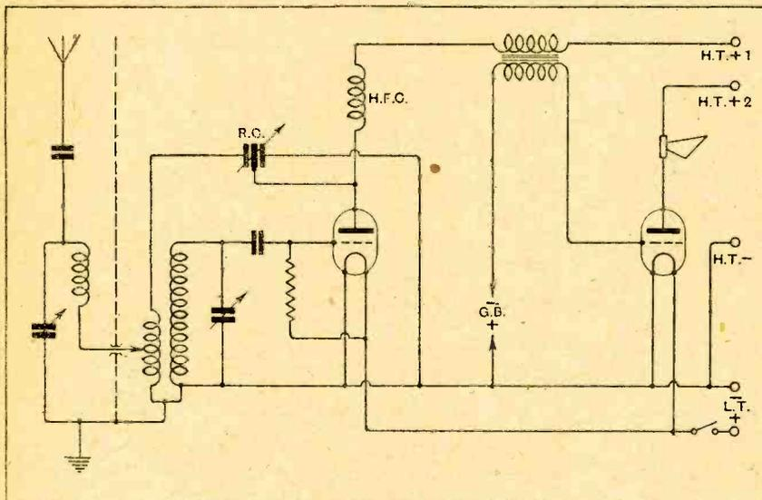
Fig. 2.—Tuned auto-coupled aerial circuit with reaction controlled by a differential condenser.
