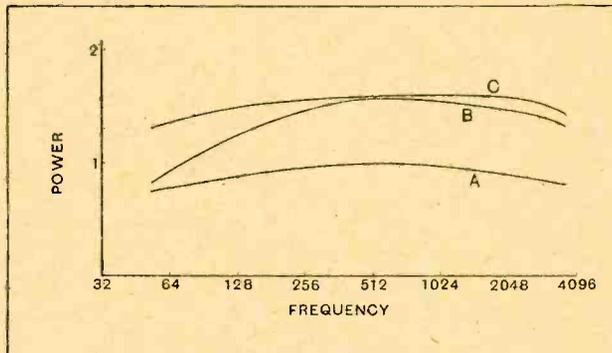
Fig. 2.—These curves show the change in frequency response of a given moving coil with changes in field strength. A, normal result with a field strength of 10,000 lines. B, field increased to 15,000 lines—note the relative lowering in the bass frequencies. C, the result of decreasing the number of turns, though maintaining the D.C. resistance, as well as reducing the weight, by using a smaller gauge of wire.
