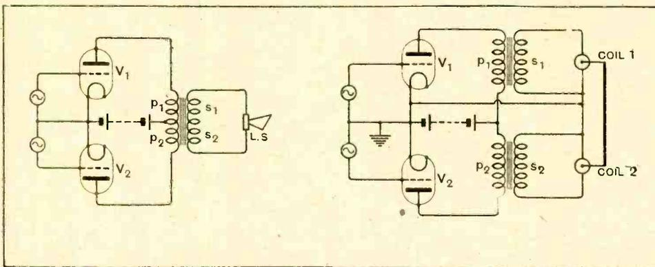
Fig. 10.—Diagram showing output transformer for push-pull arrangement, the primaries and secondary being wound on the same core.
