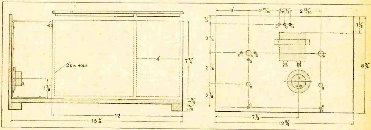
Fig. 8.—Overall dimensions of baseboard, screening box and front panel with drilling details for the latter. A, 1/2 in. dia.; B, 3/8 in. dia.; C, 1/4 in. dia.; D, 5/32 in. dia. countersunk for No. 4 B.A. screws; E, 3/32 in. dia.
