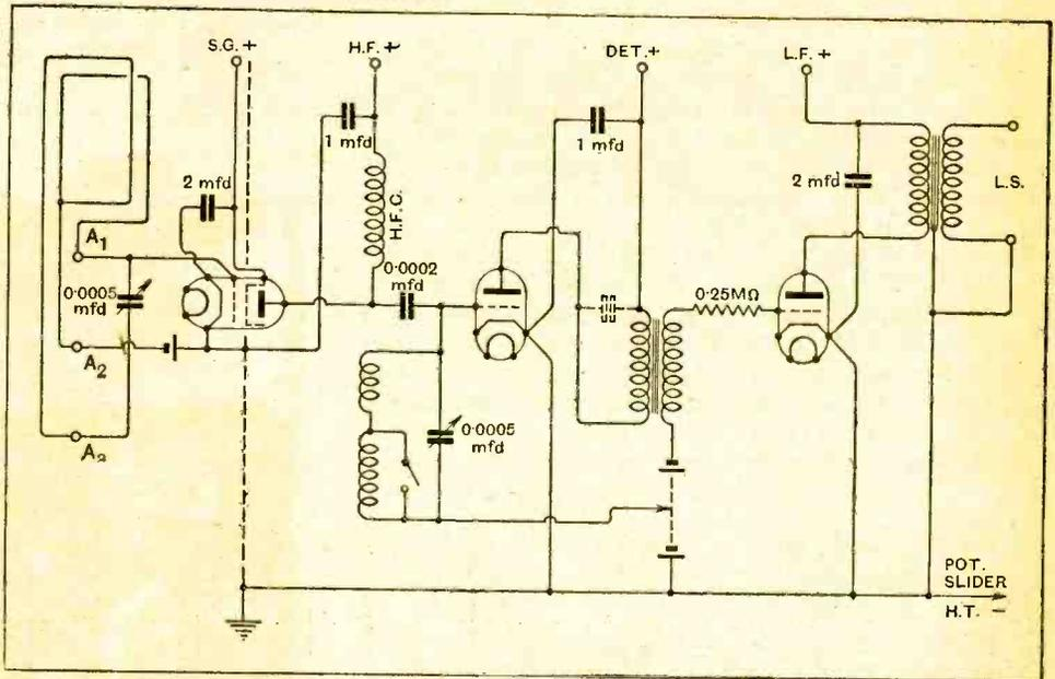
Fig. 1.—Schematic circuit diagram of receiver with filament circuits omitted.
