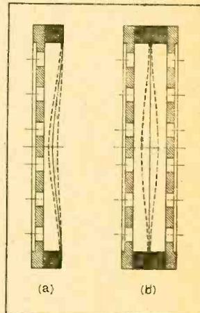
Fig. 4.—Comparison of the diaphragm movement in the earlier and new type Vogt loud speakers.
