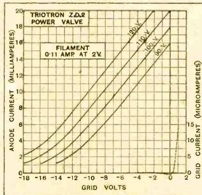
Average values under working conditions:—A.C. resistance, 4,760 ohms; amplification factor, 5.5; mutual conductance, 1.15 mA/volt.
