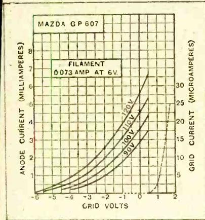
Average values under amplifying conditions: A.C. resistance, 19,000 ohms; amplification factor, 17; mutual conductance, 0.9. mA. per volt.
