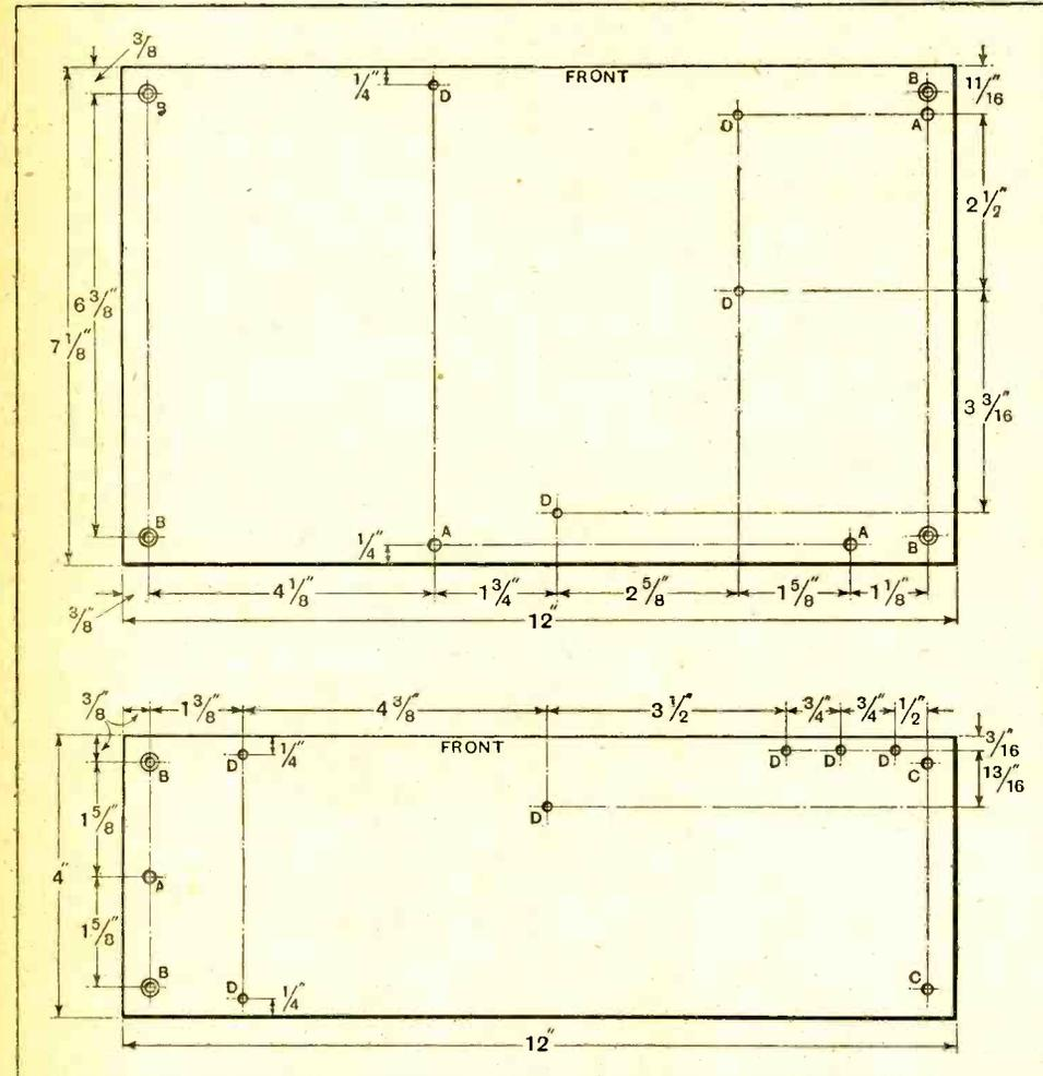
Fig. 7.—Drilling details of sub-panels for receiver and eliminator compartments of screening box. A, 3/16in. dia.; B, 5/32in. dia. countersunk for No. 4 B.A. screws; C, 5/32in. dia.; D, 1/8in. dia.
