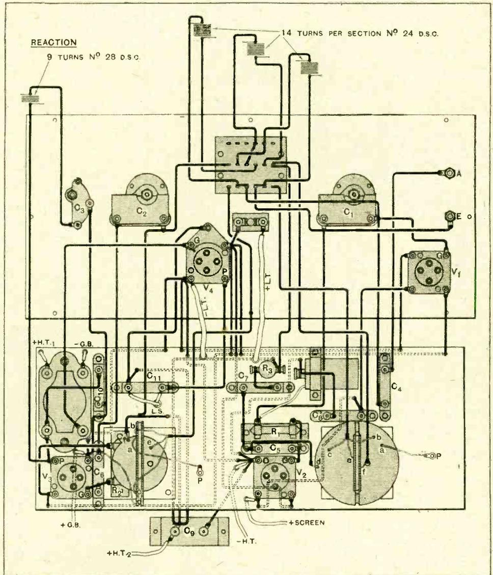
**Practical wiring diagram.** The leads are taken by the shortest path between the components on panel and baseboard. Leads beneath the baseboard are shown dotted and do not run by the paths indicated but by the shortest route from point to point.
