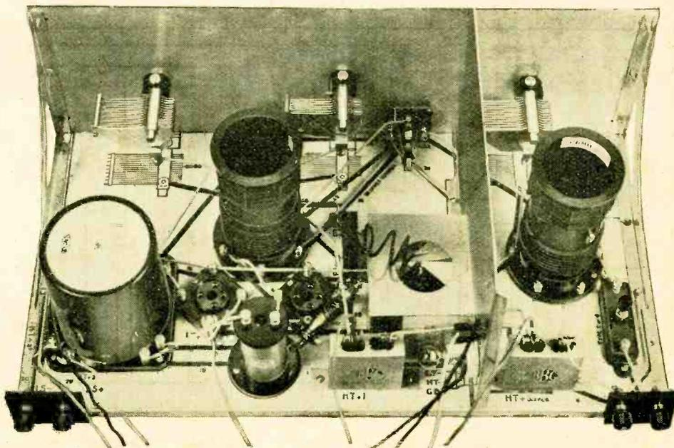
Set removed from container. Component positions and wiring are printed on the baseboard.
