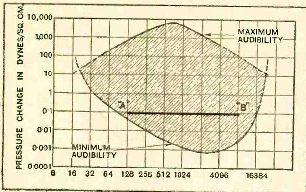
Fig. 1.—Audition area of a normal person. The average of sound intensity required by a normal person is represented by "A" "B".
