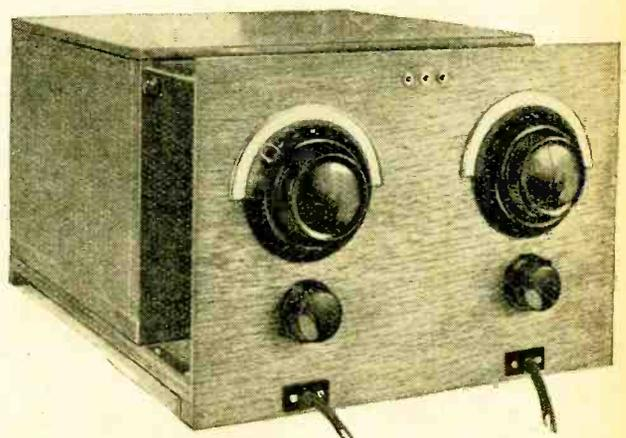
The complete receiver. Most of the parts are enclosed in the metal-lined screening box.
