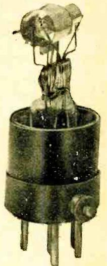
A typical two-grid, two-plate valve.
