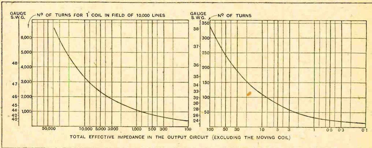
Fig. 3.—Curves giving the number of turns and gauge of wire for making a moving coil to match suitably the output impedance. It is a simple matter to adjust those figures for larger diameter coils and various field strengths.
