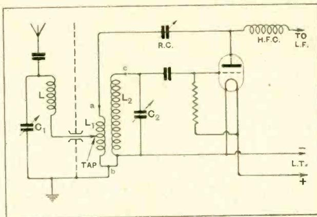
Fig. 2.—Tuned aerial circuit, specially adapted for adding to an existing receiver. C<sub>1</sub>, aerial tuning condenser; C<sub>2</sub>, secondary tuning condenser; L, loading coil; L<sub>1</sub>, coupling-reaction coil; L<sub>2</sub>, secondary coil; a, b, c, terminal points of coil, corresponding with Fig. 3.
