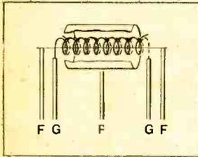
Fig. 4.—Showing the electrode disposition in a "mixed-grid" valve.
