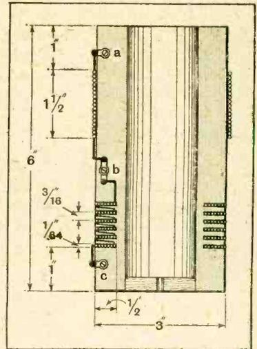
Fig. 10.—Sectional drawing of grid circuit coils. The short-wave winding consists of a single layer of 60 turns of 9/40 Litz and each slot of the long-wave coil contains 35 turns of No. 32 D.S.C.
