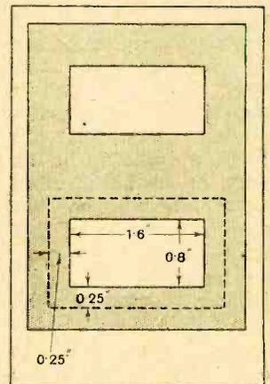
The mean iron path is shown by the dotted line and is  $2(1.6 + 0.5) + (0.8 + 0.5)$  in. = 6.8 in.
