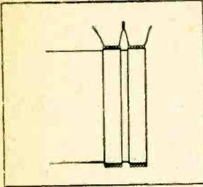
Fig. 13.—Diagram showing arrangement of mechanically coupled coils with small electromagnetic coupling.
