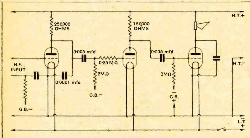
Fig. 2. Resistance-coupled L.F. amplifier for a portable receiver.
