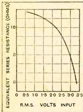
Fig. 5.—Variation of equivalent series resistance of the detector with signal strength. External anode resistance 200,000 ohms; added shunt capacity 55 micromicrofarads, wavelength 240 metres; input circuit inductance 100 microhenrys.
