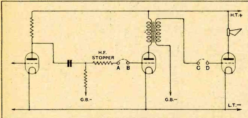
Fig. 2.—A safe method of providing for optional elimination of an intermediate L.F. stage.
