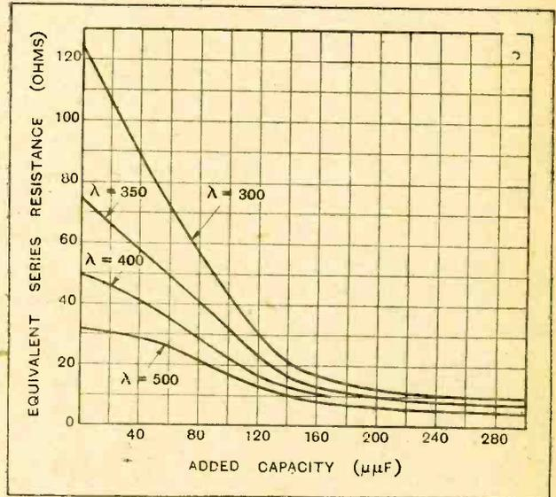
Fig. 10.—The results of Fig. 8 plotted on a capacity base for various wavelengths.
