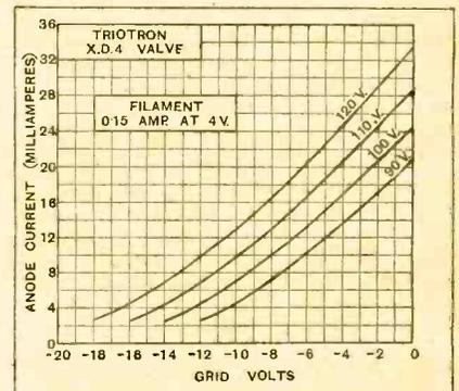
Average values under working conditions:—A.C. resistance, 2,900 ohms; amplification factor, 4.7; mutual conductance, 1.65 mA/volt.
