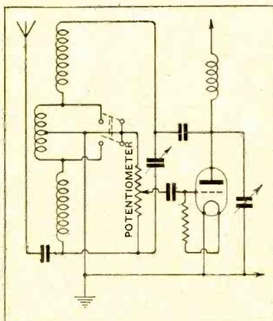
Fig. 1. H.F. potentiometer connected in a modified Hartley circuit.
