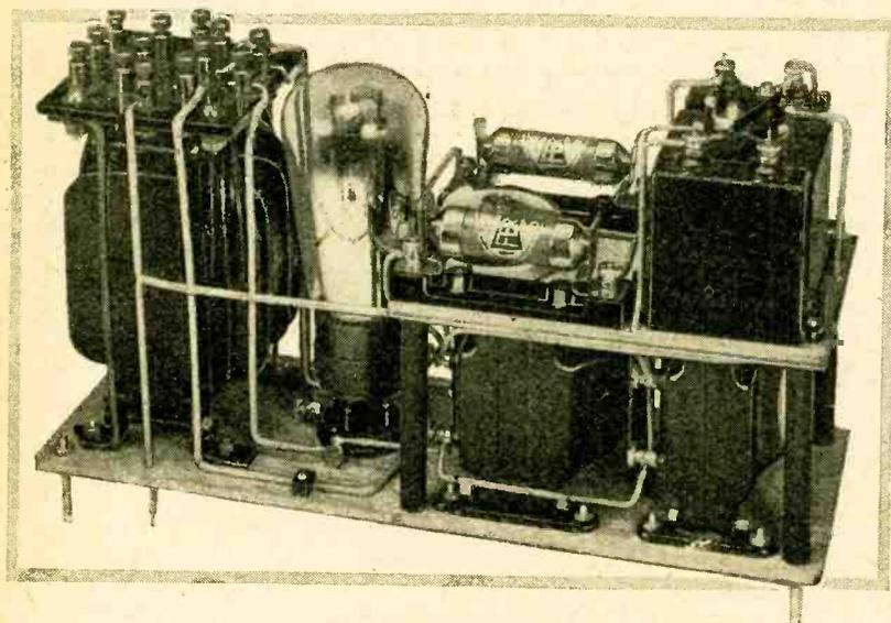
Rectifier and smoothing unit before assembling in screening box.
