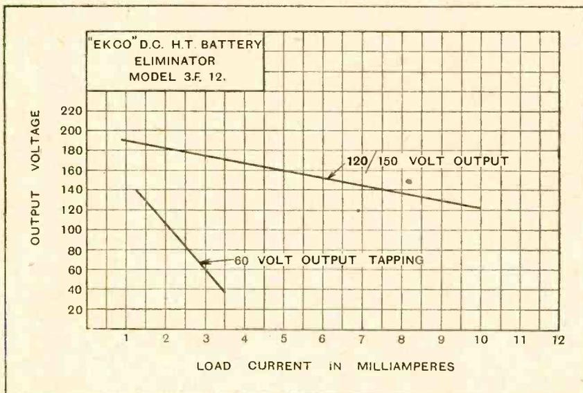
Voltage regulation curves for EKCO D.C. battery eliminator.
