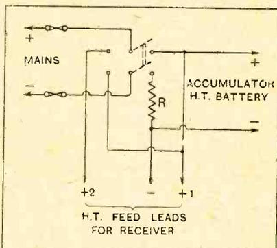
Fig. 1.—Switching scheme for connecting mains in series with H.T. accumulators for output valves.
