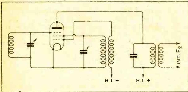
Fig. 6.—Triple-grid valve as frequency-changer.
