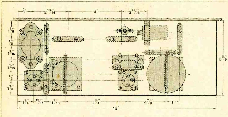
Dimensional layout showing the assembly of the components on the baseboard.
