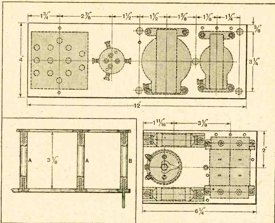
Fig. 12.—Layout of parts on the eliminator base and sub-stage showing method of mounting ebonite supports. The metal-cased 2 mfd. condensers on the sub-stage are held down by the moulded 1 mfd. condensers.
