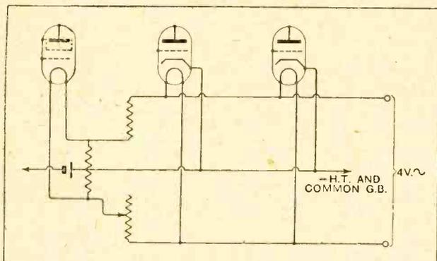
Schematic diagram of A.C. filament circuit.
