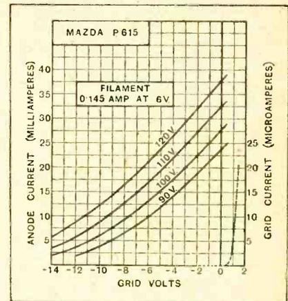
Average values under amplifying conditions: A.C. resistance, 2,700 ohms; amplification factor, 5.7; mutual conductance, 2.1 mA. per volt.
