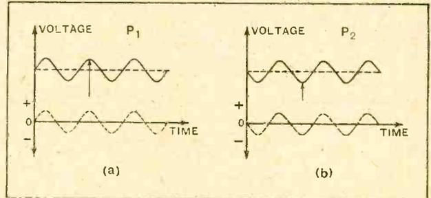
Fig. 2.—Curves representing the voltage conditions at the two outer plates of the Vogt differential loud speaker.
