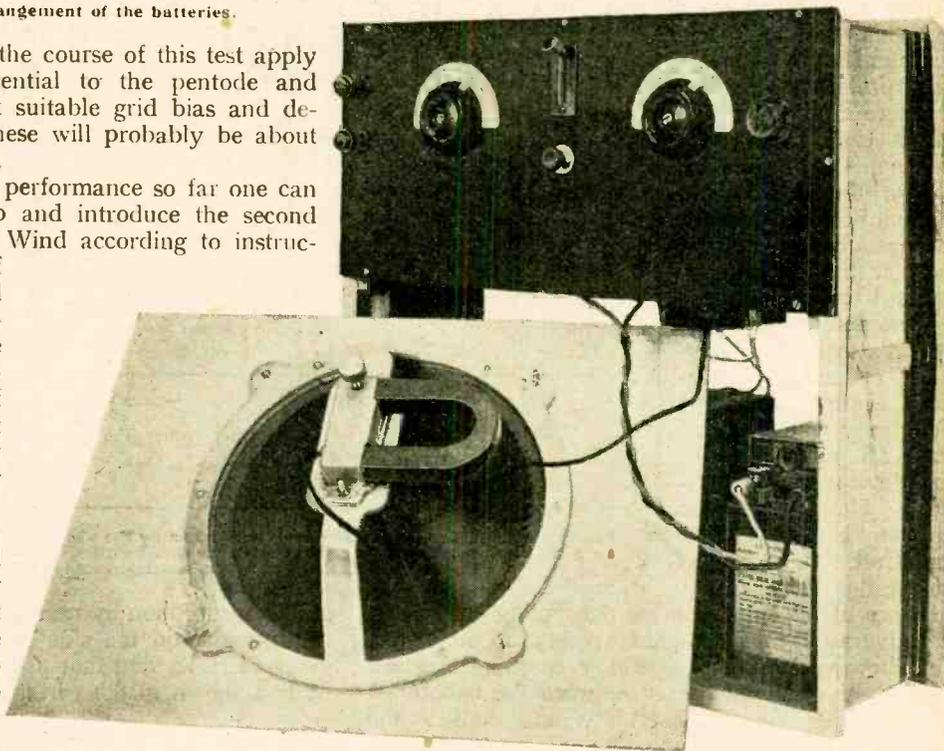
Receiver unit removed from the cabinet showing the frame windings and assembled loud speaker.
