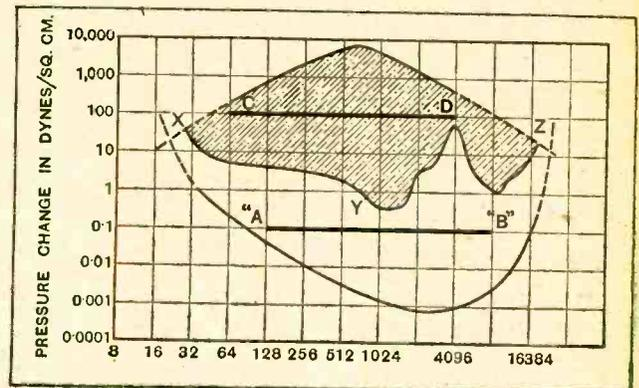
Fig. 2.—The standard of sound intensity required by a deaf person is represented by C D.
