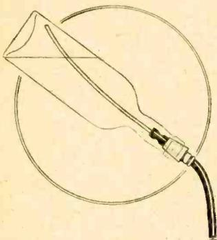
Disto filler for "topping-up" accumulator cells.
