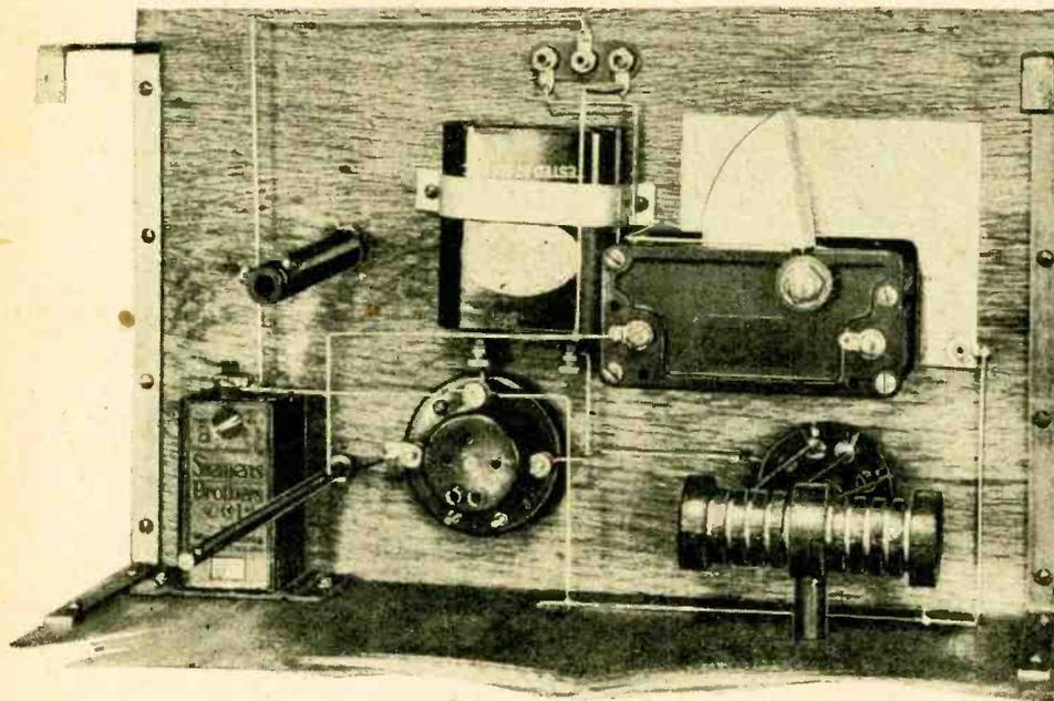
Components on the back of the front panel must be assembled and wired before fitting the screening box to the baseboard.
