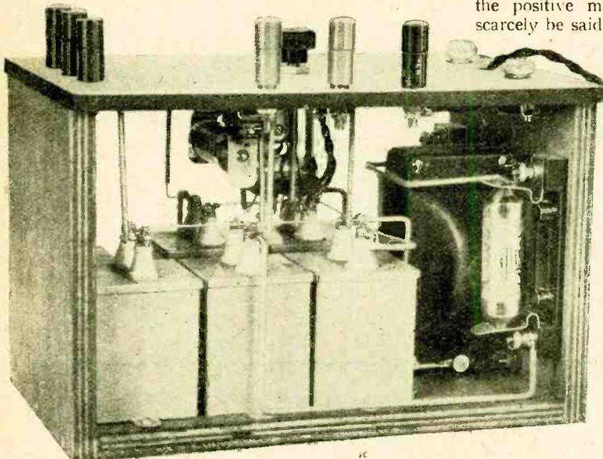
View of interior. The terminals at the left-hand side are for the connection of aerial, the aerial connection to set and the earth.
