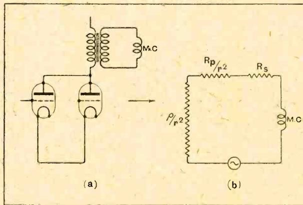
Fig. 1.—The output stage and its equivalent impedances.  $\rho$  = valve impedance,  $r$  = transformer ratio,  $R_p$  = resistance of primary,  $R_s$  = resistance of secondary.
