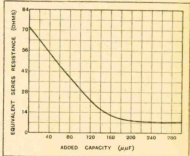
Fig. 4.—Curve representing the effect of capacity across the primary of an L.F. transformer on the equivalent series input resistance of the detector. With 0.0001 mfd. across the transformer primary there is a load equivalent to about 30 ohms added to the tuning coil.
