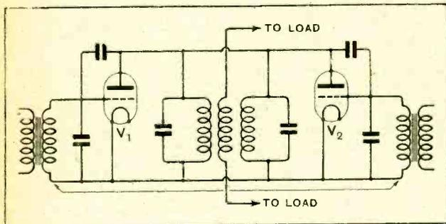
Fig. 23.—Showing that back-to-back valve circuits are equivalent to two paralleled tuned anodes.
