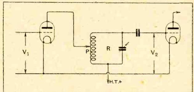
Fig. 5.—Here the amplification attained is variable within wide limits by changing the tapping point P. There is an optimum position for P.
