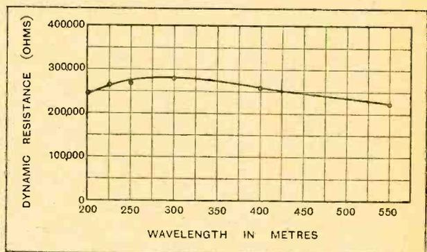
Fig. 3.—It will be seen from this curve that the dynamic resistance is approximately constant for the 200-550-metre waveband.
