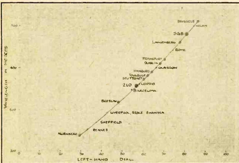
Fig. 15.—Calibration chart for the lower wave band made during a test at a place 20 miles north of London. Stations marked with one or more circles were enjoyed at full loud speaker strength without interference.
