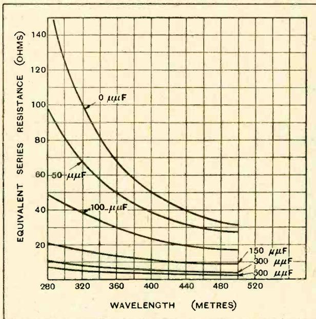
Fig. 8.—Similar curves to those in Fig. 7 for transformer coupling. It will be seen that with a shunted capacity of 0.0003 mfd. on a wavelength of 280 metres, the equivalent load resistance is about 11 ohms. A low-loss coil for this wavelength might have a high-frequency resistance of, say, 3 ohms; under the conditions specified this would in effect be increased to 14 ohms.
