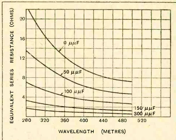
Fig. 7.—Effect of wavelength on the input load of detector for various values of capacity across an external anode resistance of 200,000 ohms. Input circuit inductance 160 microhenrys. As the wavelength is reduced the loading effect is increased.
