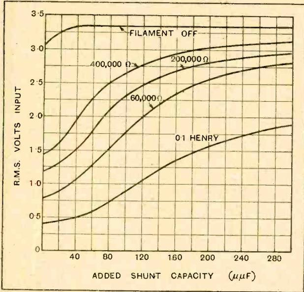
Fig. 2.—Curves showing effect of shunt capacity in the anode circuit on the input voltage with various values of external anode resistance, and a H.F. choke to represent the case of L.F. transformer coupling. The input circuit inductance is 100 microhenrys, the resistance 9.3 ohms and the wavelength 240 metres. The loading gets worse as the anode resistance and the shunted capacity are reduced.
