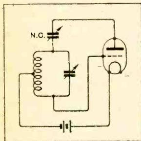
Fig. 12.—Divided or neutralised circuit to eliminate feed-back.
