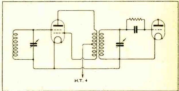
Fig. 3.—"Isodyne" circuit for high-frequency amplification.
