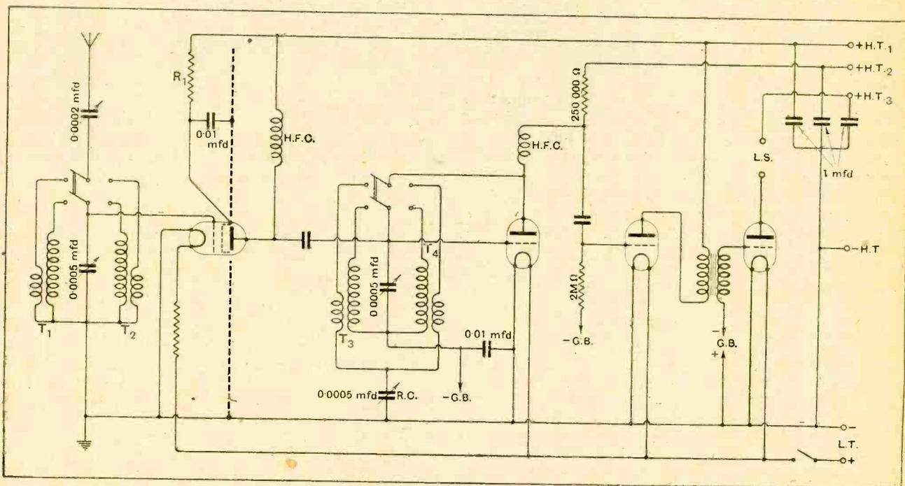
Fig. 1.—Complete circuit diagram. Wave-changing switches, shown separately to avoid complication, are actually linked together. T<sub>1</sub>, T<sub>2</sub>, aerial-grid transformers; T<sub>3</sub>, T<sub>4</sub>, detector grid coils with reaction windings.
