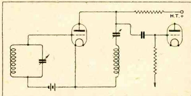
Fig. 13.—Series tuned circuit across external anode load to short-circuit virtually the H.F. component so that feed-back is eliminated. The low potential end of the coil can either be connected to L.T. negative (as shown) or to H.T. positive.
