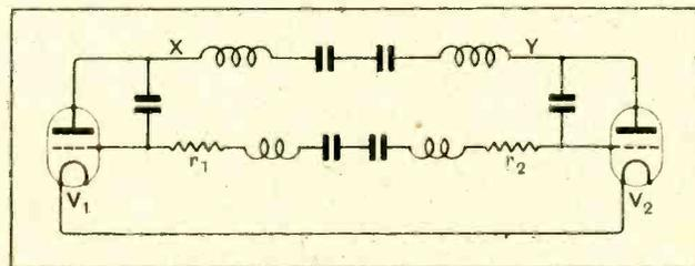
Fig. 26.—Showing circuitual position of damping resistances  $r_1$   $r_2$  of Fig. 25 for curbing parasitic mode of Fig. 20. Clearly resistances inserted at X and Y would also be effective. At high frequencies this is permissible since the resistance required is small, but at low frequencies it is large and would reduce the anode feed.
