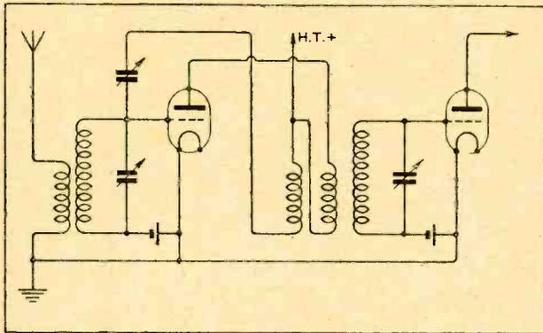
Fig. 2.—Practical receiver corresponding to Fig. 1.
