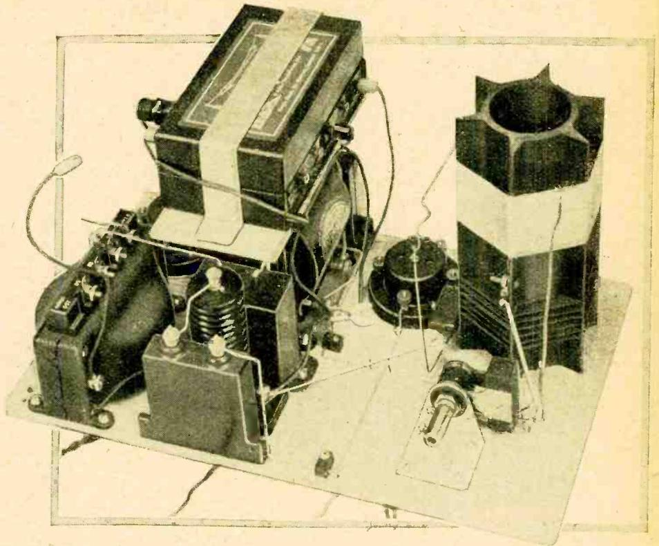
The receiver unit wired ready for assembly in the screening box.
