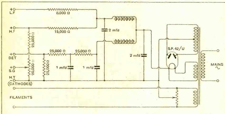
Fig. 4.—Schematic circuit diagram of rectifier unit.
