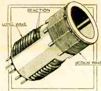
Fig. 2.—Construction of the anode coil assembly. The long-wave section is cut away to show pile windings.
