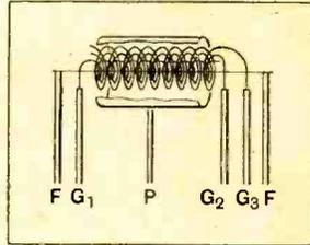
Fig. 5.—The electrode arrangement in a triple-grid valve.
