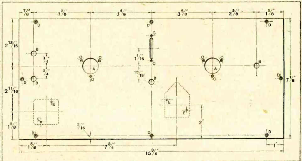
Drilling details of the front panel. A, 15/16in.; B, 5/16in.; C, 1/8in.; D, 1/8in. and counter-sunk; E, 1/8in. for 6.B.A. screws.
