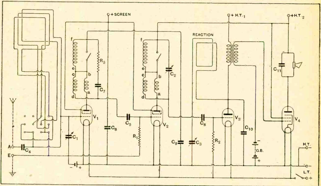
Portable receiver circuit with two screen grid stages and pentode.  $C_1, C_2, 0.0005$  mfd.;  $C_3, 0.0001$  mfd.;  $C_4, 0.0002$  mfd.;  $C_5, 0.0005$  mfd.;  $C_6, 0.0003$  mfd.;  $C_7, 0.0001$  mfd.;  $C_8, 0.003$  mfd. or larger;  $C_9, 2$  mfd.;  $C_{10}, C_{11}, 0.002$  mfd.
