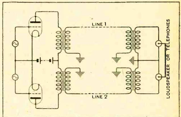
Fig. 12.—Diagram showing scheme of Fig. 11 applied to distant operation of reproducing apparatus.
