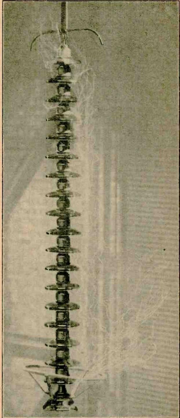
Fig. 3.—Photograph of an electrical discharge over a string of insulators about 7 feet long, with an applied pressure of about one million volts.
