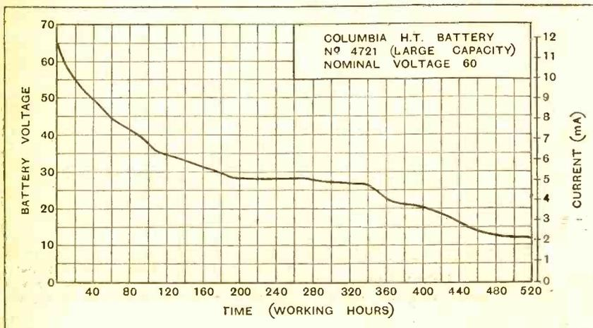
Discharge curve of the Columbia Type No. 4721 dry-cell H.T. battery.
