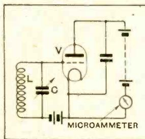
Fig. 3.—In this circuit a decapped valve V is used as an anode-bend detector. It had been calibrated as a voltmeter; the deflection of the instrument in the plate circuit for any H.F. voltage on the grid of the valve being known. The dynamic resistances given in the text apply to the above circuit as a whole.
