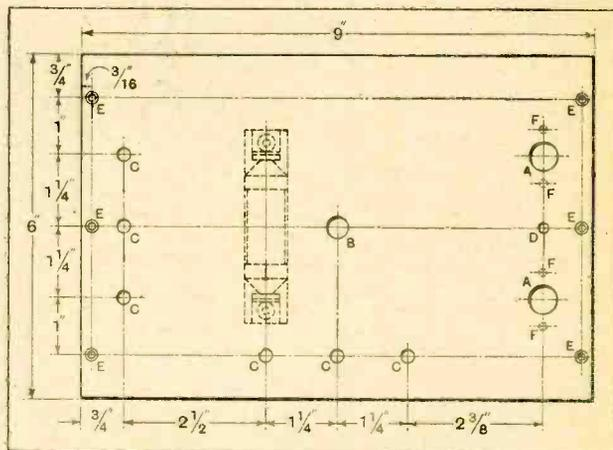
Fig. 2.—Layout of ebonite panel. Drilling sizes are as follows: A,  $\frac{1}{2}$  in. diameter. B,  $\frac{1}{2}$  in. diameter. C,  $\frac{3}{8}$  in. diameter. D,  $\frac{1}{2}$  in. diameter. E,  $\frac{1}{2}$  in. diameter and countersunk for No. 4 wood screws. F, drilled and tapped 6 B.A. blind.
