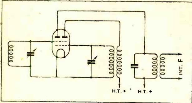
Fig. 11.—Using the two-plate, two-grid valve as a frequency-changer.
