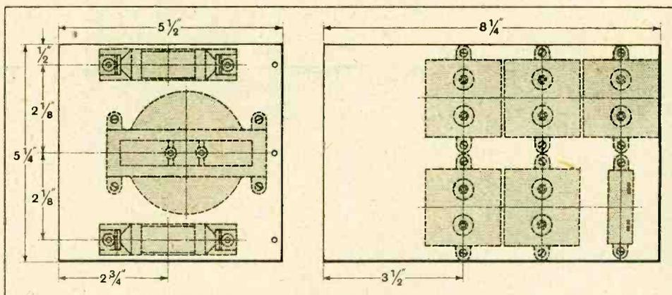
Fig. 3.—Layout of baseboard and side panel.
