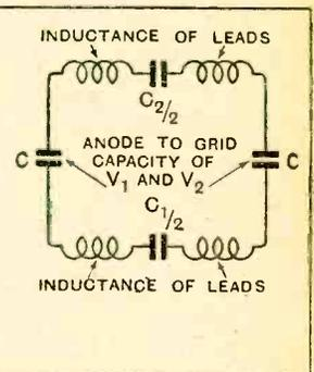
Fig. 21.—Diagram of Fig. 20 simplified to show that it is an ordinary oscillatory circuit. By "lumping" the inductances and condensers, it could be represented by a single inductance and a single condenser.
