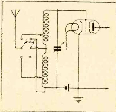
Fig. 1.—Modified grid circuit of A.C./S. valve with simple waveband switching.
