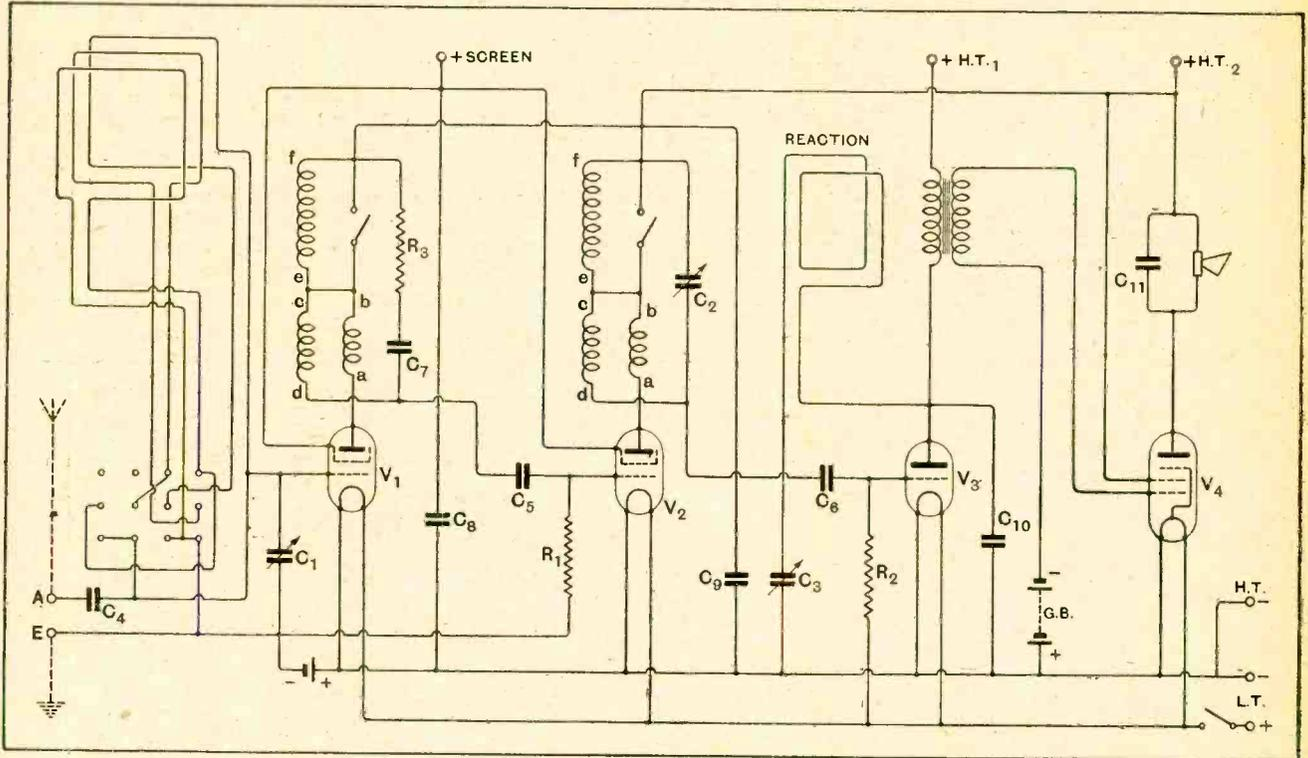
Portable receiver circuit with two screen grid stages and pentode. C<sub>1</sub>, C<sub>2</sub>, 0.0005 mfd.; C<sub>3</sub>, 0.0001 mfd.; C<sub>4</sub>, 0.0002 mfd.; C<sub>5</sub>, 0.0005 mfd.; C<sub>6</sub>, 0.0003 mfd.; C<sub>7</sub>, 0.0001 mfd.; C<sub>8</sub>, 0.003 mfd. or larger; C<sub>9</sub>, 2 mf.; C<sub>10</sub>, C<sub>11</sub>, 0.002 mfd.
