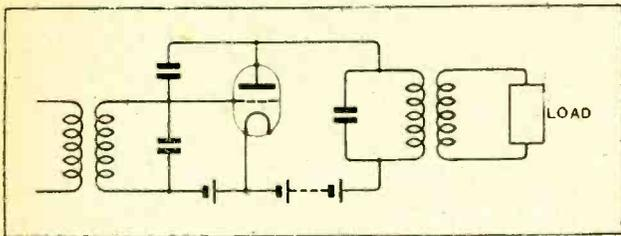
Fig. 22.—Showing that the circuit of one of a pair of back-to-back valves is akin to tuned anode.
