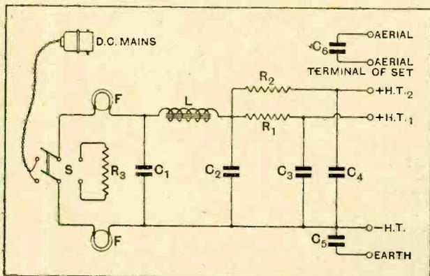
Fig. 1.—The theoretical circuit diagram. Values are as follows: C<sub>1</sub>, C<sub>2</sub>, C<sub>3</sub>, C<sub>4</sub> and C<sub>5</sub>, 4 mfd.; C<sub>5</sub>, 1 mfd.; L, 30 henrys; F, 3.5-volt flash-lamp bulb; R<sub>1</sub>, R<sub>2</sub>, according to mains voltage and valves used; R<sub>3</sub>, 40,000 ohms.
