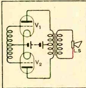
Fig. 17.—Simple push-pull circuit transformer-coupled to loud speaker.
