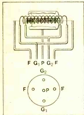
Fig. 1.—A double-grid valve and base. A straight filament is used around which there are two spiral grids and a cylindrical plate.
