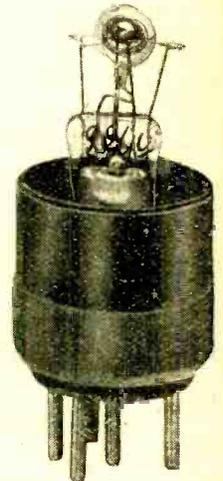
The electrode arrangement in the double-grid valve.
