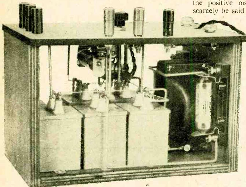
View of interior. The terminals at the left-hand side are for the connection of aerial, the aerial connection to set and the earth.
