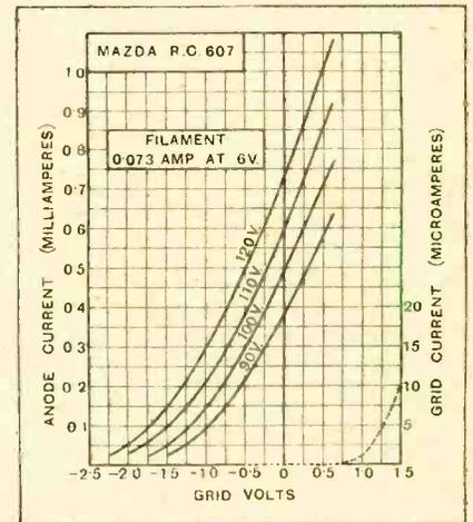
Average values under amplifying conditions: A.C. resistance, 75,000 ohms; amplification factor, 40; mutual conductance, 0.53 mA. per volt.
