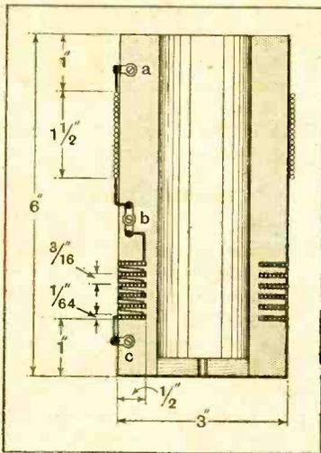
Fig. 6.—Sectional drawing of grid circuit coils. The short-wave winding consists of a single layer of 60 turns of 9/40 Litz and each slot of the long-wave coil contains 35 turns of No. 32 D.S.C.
