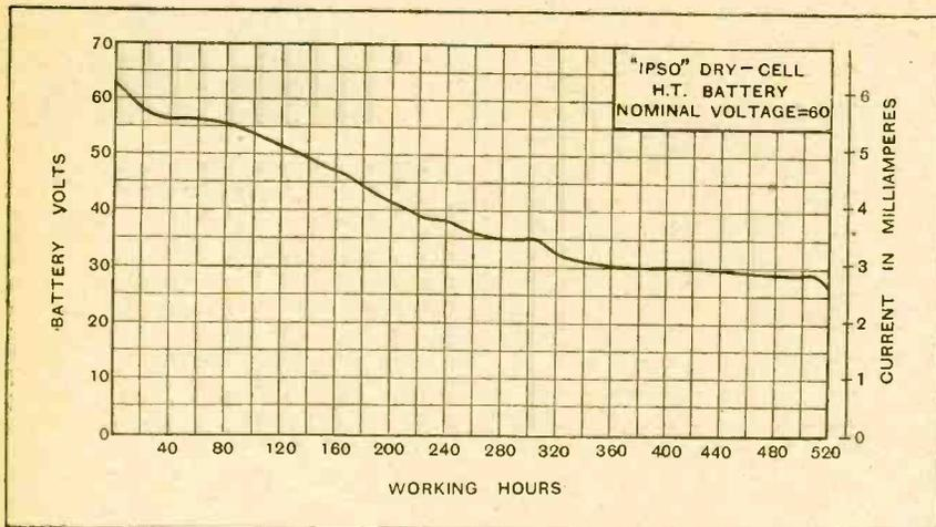
Discharge curve of the "Ipsos" 60-volt dry-cell battery.
