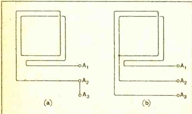
Fig. 3.—Frame aerial connections (a) for short waves (b) for long waves.
