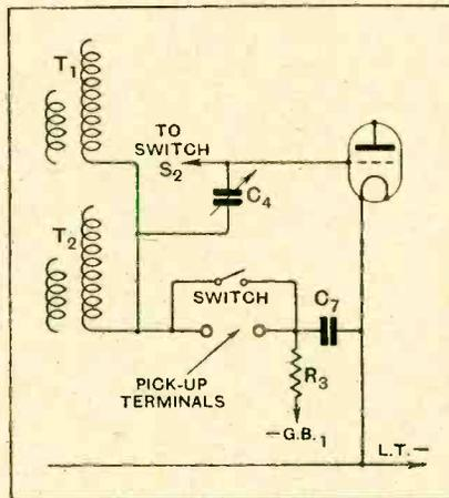
Fig. 1.—Modifying the "S.G. Regional Receiver" for gramophone amplification. Reference lettering corresponds to the original diagram.
