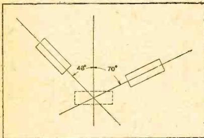
Showing the optimum cutting angles for quartz crystals.
