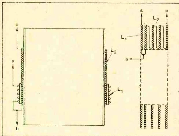
Fig. 3.—Sectional drawing showing construction of coils for medium and long wavebands.
