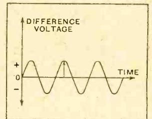
Fig. 3.—Resultant force on the diaphragm due to the alternating voltage applied to the two plates of the differential loud speaker.
