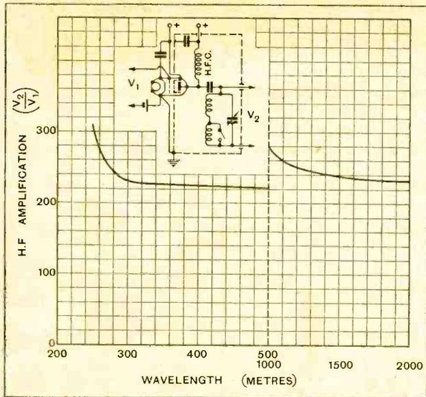
Fig. 2.—Amplification curves of the AC/S valve with parallel feed, tuned grid coupling; H.T. = 120 volts, screen-grid = 48 volts, G.B. = 1½ volt. The measurements were made with a Lewcos H.F. choke, a 0.0002 mfd. coupling condenser and the coils shown in Fig. 6.
