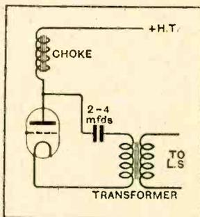
A choke-filter fed output transformer.
