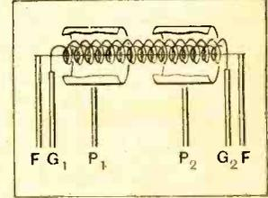
Fig. 10.—A two-plate, two-grid valve, type two.
