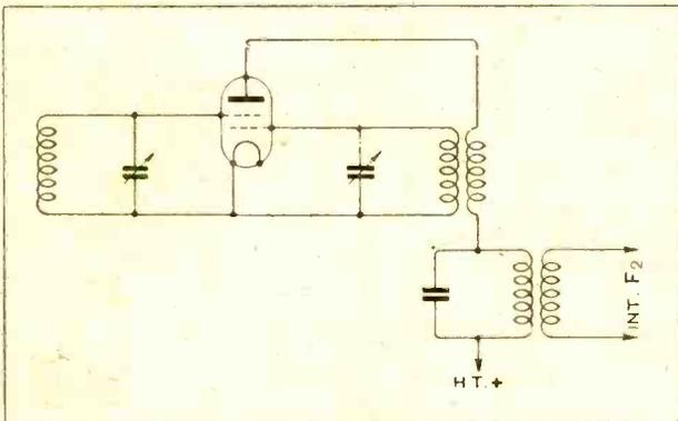
Fig. 2.—Standard frequency-changing circuit for double-grid valve.
