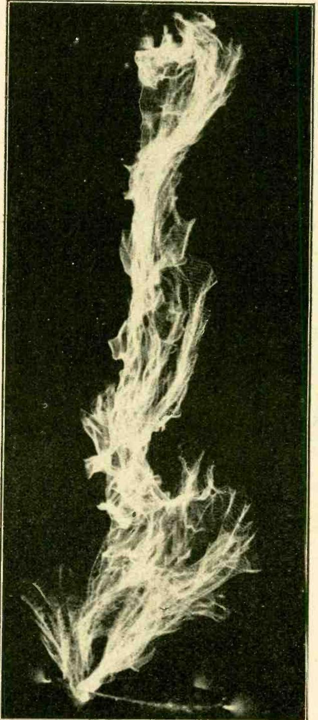
FIG. 2.—Photograph of an electrical discharge over a string of insulators about 7 feet long, with an applied pressure of about one million volts. (The insulators employed are seen more clearly in Fig. 3.)
