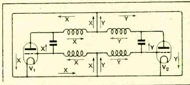
Fig. 24.—Showing "parallel" parasitic circuits in back-to-back amplifier.
