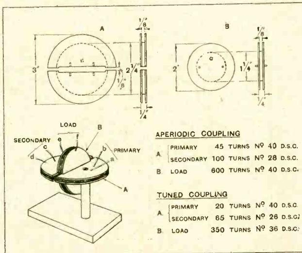
Dimensional details of the interlocking formers used for constructing the H.F. couplings. Although best made of turned ebonite, suitable formers can be made from cardboard.
