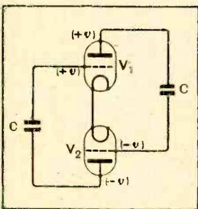
Fig. 27.—The anodes and grids of a symmetrical mid-point back-to-back arrangement are at equal and opposite potentials. The diagram shows how neutrodyning is effected.
