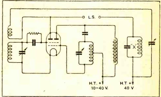
FIG. 12.—A super-reaction circuit with two-plate, two-grid valve. The tuned circuit X is a trap circuit tuned to the "howl" frequency.
