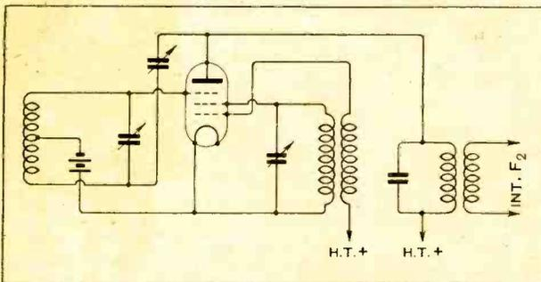
Fig. 7.—A frequency-changing circuit with reaction using triple-grid valve.
