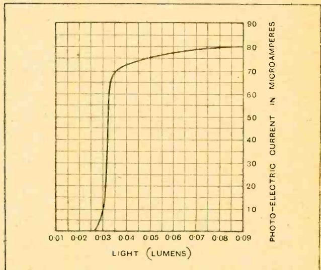
Fig. 3.—The photo-electric current plotted against light intensities when a constant anode-cathode voltage is applied
