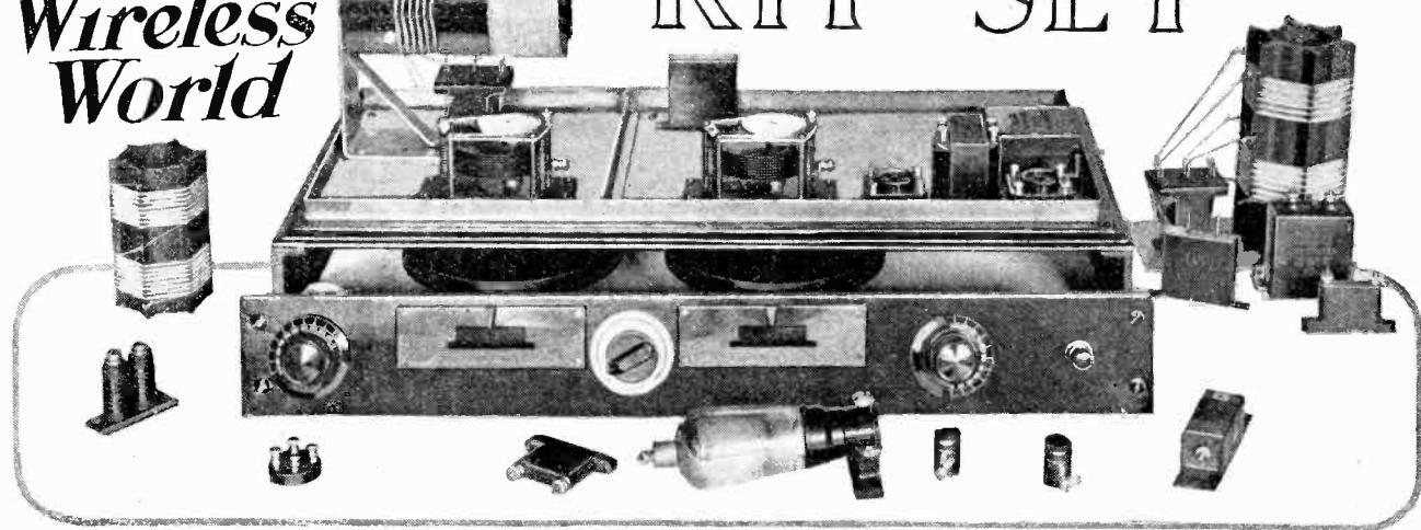
An Easily Constructed Three-valve Receiver of High Selectivity.
