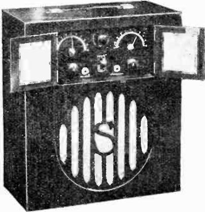
Four valves are used in this Selector trans-portable receiver. The tuned H.F. stage has a screen-grid valve.
