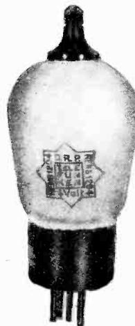
Telefunken screen-grid valve. The glass bulb is covered with an earthed metallic coating which reduces the residual inter-electrode capacity.
