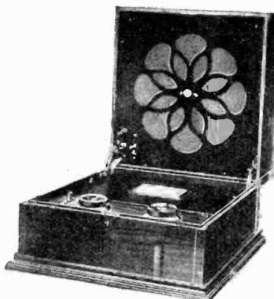
Gecophone four-valve screen grid table model.
