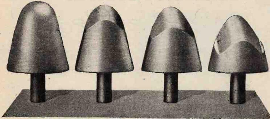
Fig. 3.—Progressive stages in the wear of a loud tone needle.
