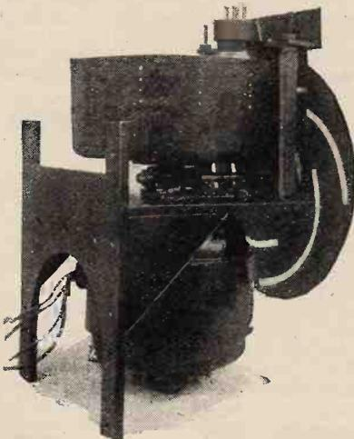
**TELEVISION IN AMERICA.** Regular television programmes are now broadcast by W2XCR, New Jersey, using the Jenkins apparatus. The photograph shows the interior of a Jenkins receiver. Note the rotating drum with its vertical scanning holes and neon lamp.
