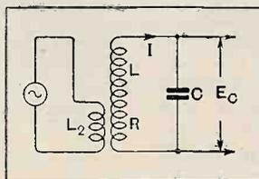
Fig. 1.—Simple series tuned circuit. If a voltage  $E$  is induced into the closed circuit  $LRC$  the voltage  $E_C$  is built up across it at the resonant frequency.  $\frac{E_C}{E}$  is the voltage magnification  $m$  of the tuned circuit and is equal to  $\frac{1}{R} \sqrt{\frac{L}{C}}$ .
