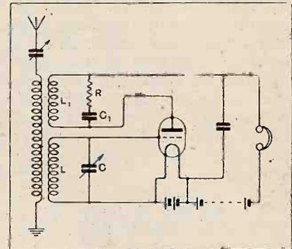
A constant reaction scheme with shunt circuit RC<sub>1</sub>. (No. 283,121.)
