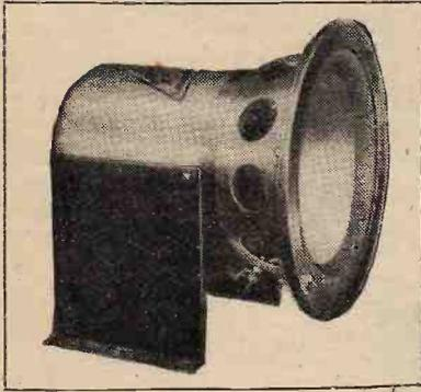
The Junior "R.K." Unit has a 6 in. straight-sided cone with moving coil having an impedance of 10-15 ohms at 50/4,000 cycles. Copper damping rings are fitted to reduce the impedance at the higher frequencies. Price £6 6 0
