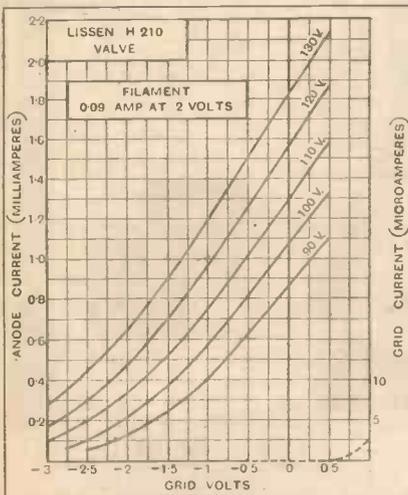
Average values under working conditions: A.C. resistance 50,000 ohms; amplification factor, 25; mutual conductance, 0.5 mA/volt.
