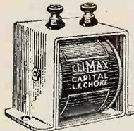
The Climax capital Choke forms an extremely efficient smoothing choke for eliminating the ripple in H.T. supply for A.C. or D.C. mains. Winding resistance 500 ohms. Current carrying capacity 50 milliamperes. Inductance 12-20 henries. Price - - - 8/-
