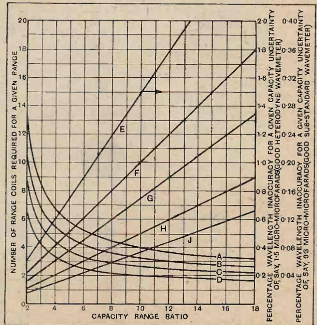
Fig. 3.—Showing the number of range coils and capacity ratio of condensers of wavemeters of various accuracies.
