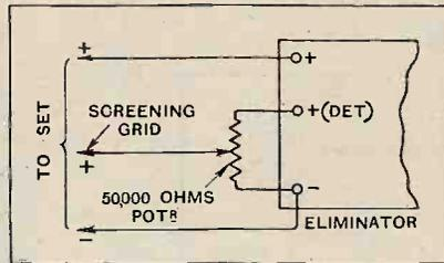
Fig. 1.—Critical adjustment of eliminator output voltage is obtained by adding an external high-resistance potentiometer.
