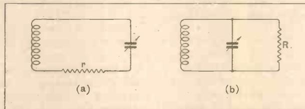
Fig. 1.—The losses in a tuned circuit and the components connected to it can be expressed either as a "series" resistance  $r$ , or as a dynamic resistance  $R$ . In the latter case, the more low-loss the circuit, the higher  $R$  becomes.
