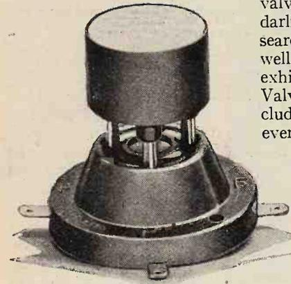
A new vacuo-junction device by the Cambridge Instrument Co., Ltd., in which the thermo-junction and the heater are enclosed in a highly exhausted glass bulb to eliminate air current effects.
