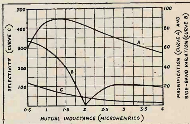
Fig. 3.—The same filter as in Fig. 2 but the curves are taken at 250 metres at which the coil resistance is 10 ohms.
