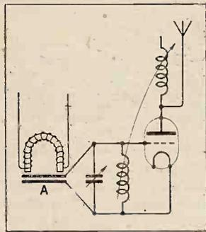
Fig. 1.—Speech currents vary the capacity of the condenser A and so the transmitter is modulated at speech frequency.
