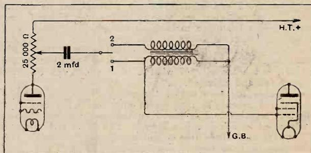
Switch in position (1) gives resistance coupling. As the resistance is only 25,000 ohms the output from the detector does not overload the pentode and no further volume control is needed. The high inductance of the transformer secondary is used instead of a grid leak. This coupling is used for the more powerful stations.
