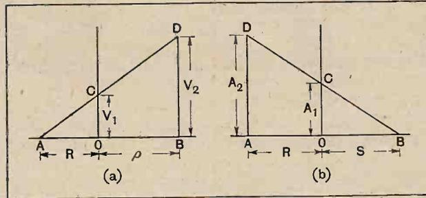
Fig. 2a.—Extended range  $V_2$  of voltmeter may be increased by the use of the larger series resistance  $\rho$ . Fig. 2b.—Extended range  $A_2$  of voltmeter may be increased by diminishing the value of the shunt resistance  $S$ .
