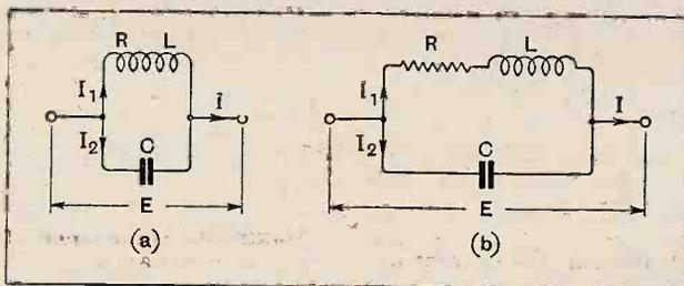
Fig. 1.—(a) Parallel circuit where resistance is present in the inductive coil. (b) Equivalent circuit.
