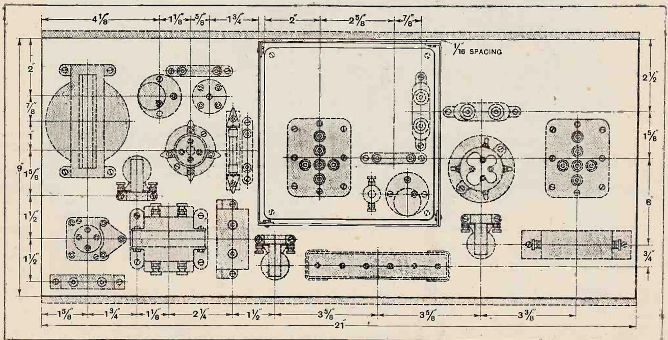
Fig. 6.—Disposition of the components on the baseboard.
