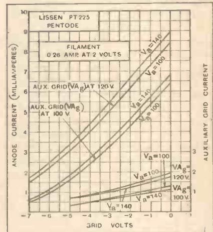
Average values under working conditions: A.C. resistance, 106,000 ohms; amplification factor, 114; mutual conductance, 1.1 mA/volt.
