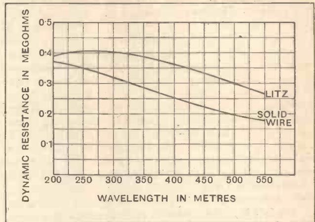
Fig. 3.—Dynamic resistance of tuned circuit with condenser and decapped valve in parallel with the coil.
