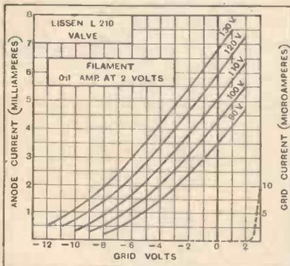
Average values under working conditions: A.C. resistance, 12,900 ohms; amplification factor, 7.7; mutual conductance, 0.6 mA/volt.
