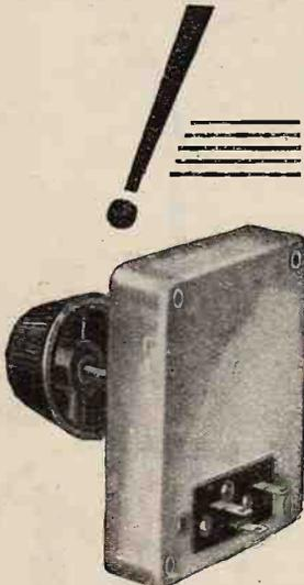
These new Electrad variable non inductive high resistances will safely dissipate 5 watts at any position of the contact, with one-tenth or more of the resistance element in circuit. The all-metal construction with the graphite resistance element fused to an enamel base obviates the necessity of using either a low current paper element or fine wire. The action is amazingly smooth, long lived and both mechanically and electrically perfect.
