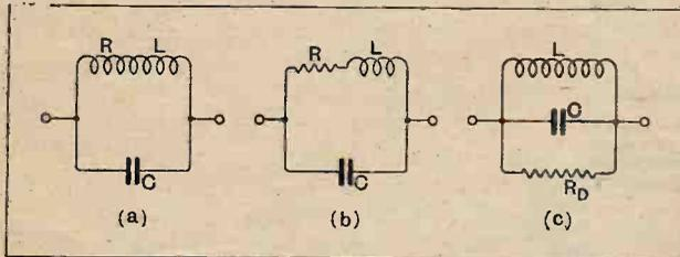
Fig. 1.—(a) Tuned parallel circuit with effective resistance  $R$  in the coil. (b) Equivalent circuit with internal resistance. (c) Equivalent circuit with whole of the resistance imagined in parallel. The equivalent parallel resistance is the dynamic resistance of the circuit.
