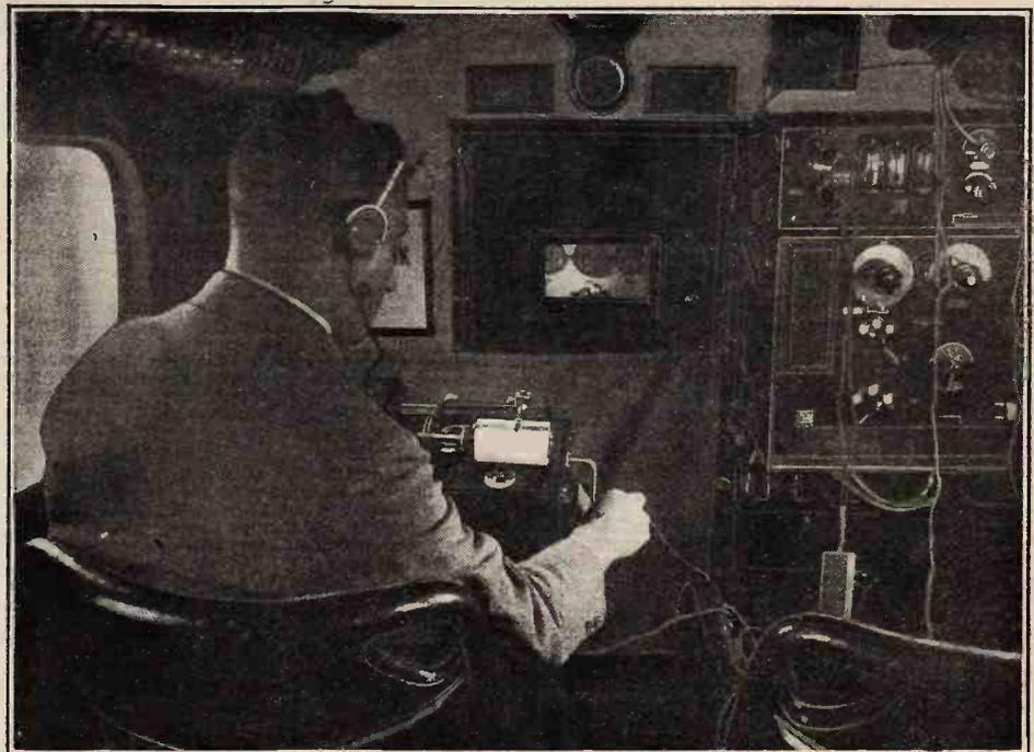
The Fultograph receiver in use in a Lufthansa aeroplane. To prevent spilling, a sponge soaked in potassium iodide solution was employed in the experiments. On the right is the Telefunken transmitter and receiver.
