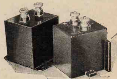
Remodelled T.C.C. 4 mfd condensers. Note the generous size of the terminals.
