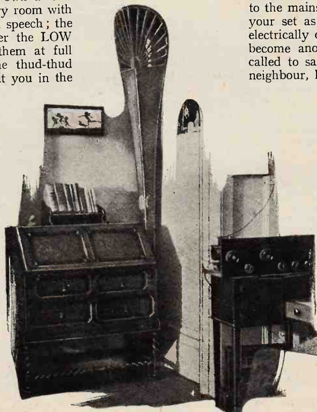
The author's 10ft. logarithmic horn speaker operating from a small reed-driven aluminium cone and mounted in an alcove to aid sound reflection.
