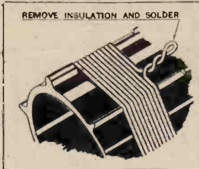
Fig. 2.—Tappings on the coil are made by twisting a small loop in the wire, as shown above.
