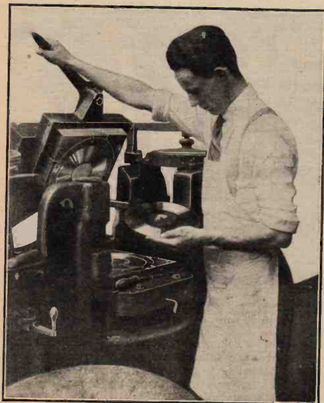
Fig. 8.—Withdrawing a completed record from the record press.
