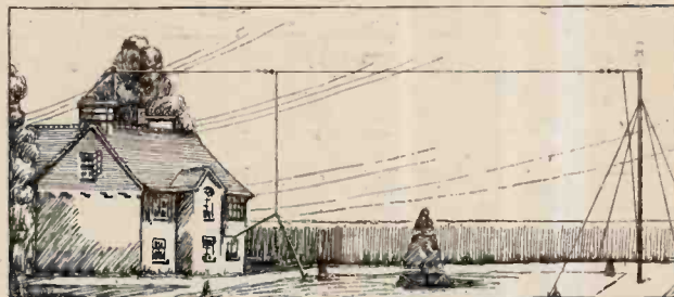
An efficient aerial-earth system is helpful when range must be combined with selectivity.
