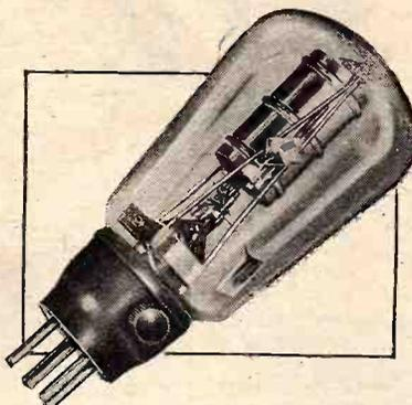
The indirectly-heated pentode—the Mazda AC/Pen. With a signal of 5 volts from a local transmission it is possible to obtain about 350 milliwatts output.
