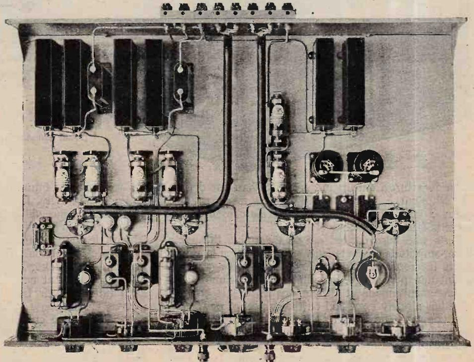
Underside of the push-pull detector and first L.F. amplifier unit.
