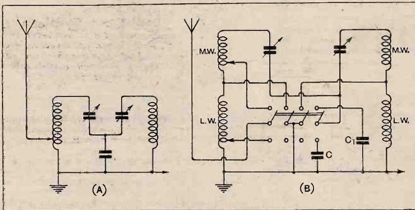
Fig. 2.—Conventional input filter circuit (A) and the same arrangement with waveband switching added (B).
