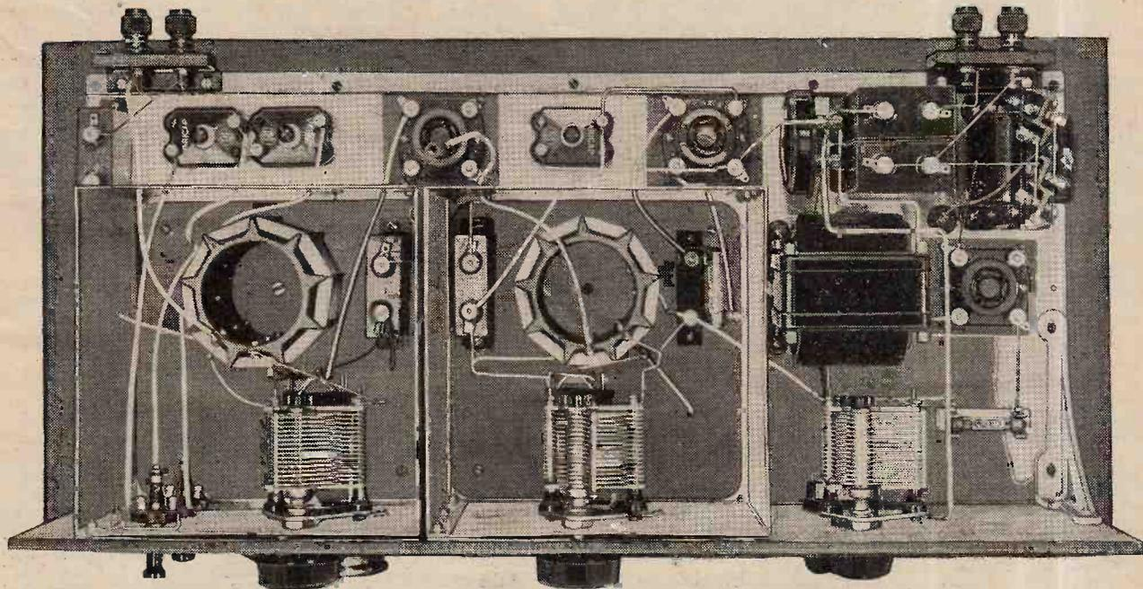
Plan view of the set with valves and screening box covers removed. The aerial-grid coil and the rejector condensers are on the left.
