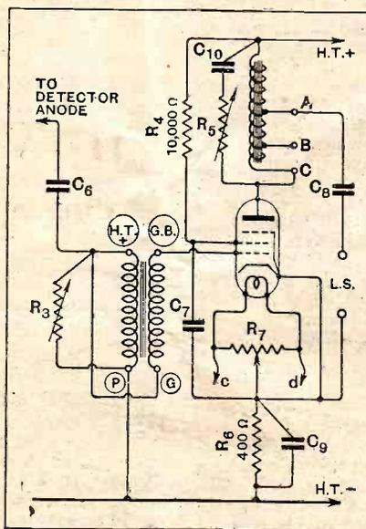
Fig. 1.—The "Power Pentode Two" with an indirectly heated pentode in place of the original directly heated output valve.
