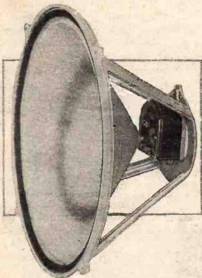
Lissen cone chassis with improved balanced-armature drive.
