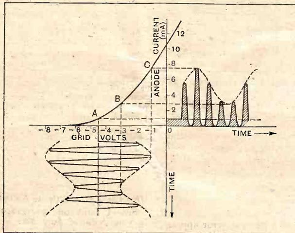
Fig. 4.—Diagram showing how the anode current varies when a modulated H.F. voltage is applied to the grid of a valve biased to operate on the lower bend of its anode characteristic curve.
