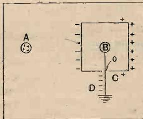
Fig. 2.—This diagram illustrates the change in the distribution of the charges when the apparatus B is connected to earth. If C is to continue to shield B, the earth lead D must be connected to C at its point of entry O.
