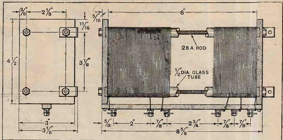
Details of the former for the large resistance  $R_9$ .
