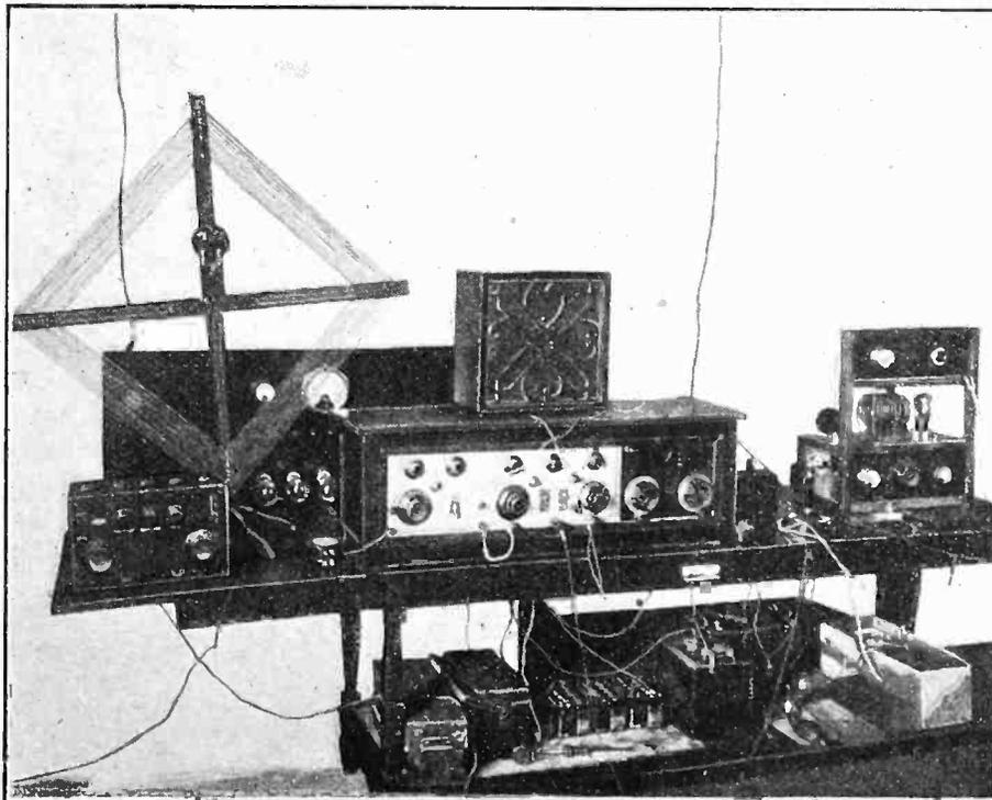
CT 2AG owned and operated by Fernando Hinte at Gorreana, San Miguel, Azores. The transmitter, on the right, is a Mesney using about 20 watts to a Phillips JB004/10 valve and coupled to a full-wave 42-metre Hertz aerial. The receiver in the foreground is an 8-valve superheterodyne.
