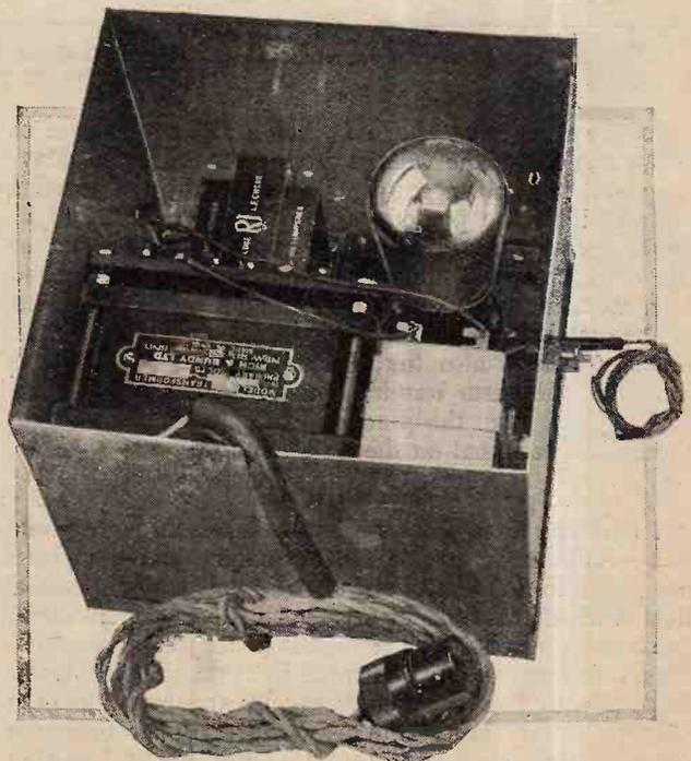
The separate eliminator unit housed in a small screening box. The very minimum of equipment is required for smoothing.
