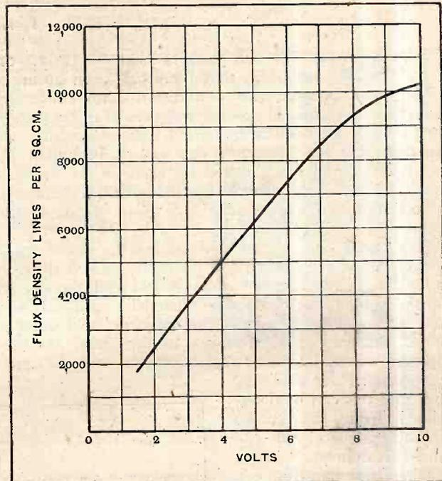
Fig. 2.—Curve showing the increase in flux-density by raising the field voltage.
