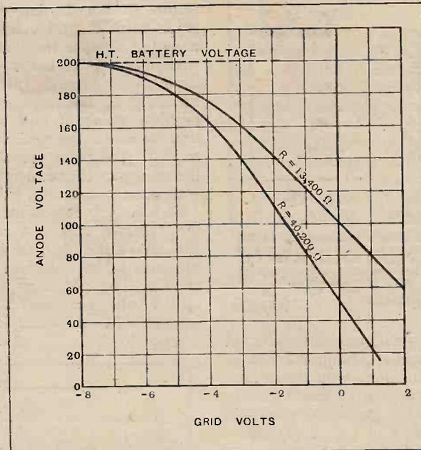
Fig. 4.—Curves showing how the anode voltage varies with grid voltage when two different values of resistance are connected in the anode circuit. The variation of anode voltage for 1 volt change of grid voltage gives the actual voltage amplification obtained.
