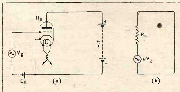
Fig. 1.—(a) A three-electrode valve with zero impedance in the external anode circuit and with a small alternating voltage  $V_g$  applied to the grid. (b) Simple circuit equivalent to the anode circuit in so far as the alternating components are concerned.
