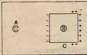
Fig. 1.—The effect of the charge at A on the apparatus situated at B is neutralised by the induced charge on the shield C.
