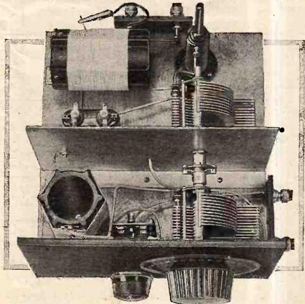
Plan view of the unit. In the compartment next to the panel are housed one member of the ganged condenser, the secondary coil with reaction winding, and the reaction condenser. A slow-motion dial will probably be found more satisfactory for controlling the ganged condenser.
