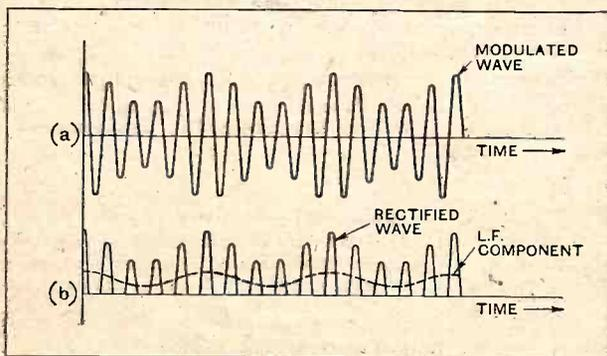
Fig. 1.—(a) Normal type of modulated wave representing the product of a high-frequency and a low-frequency component. (b) Rectified wave which is equivalent to the sum of high-frequency and low-frequency components, together with a D.C. component.
