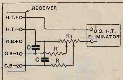
Fig. 1.—Adding a "grid bias battery eliminator" to a receiver deriving its anode current from D.C. mains.
