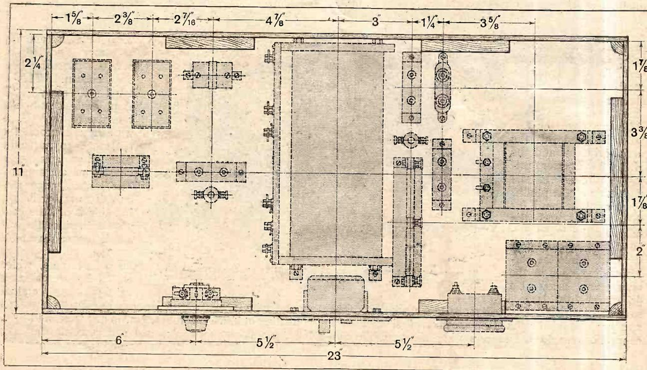
Layout of the smoothing equipment, grid bias resistances and H.T. supply resistances on the underside of the base.
