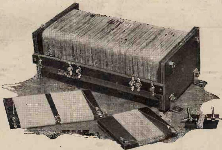
These resistances, which carry 250/280 milliamps. are wound with No. 28 Eureka wire. The principal resistance,  $R_8$ , is the rectangular assembly.
