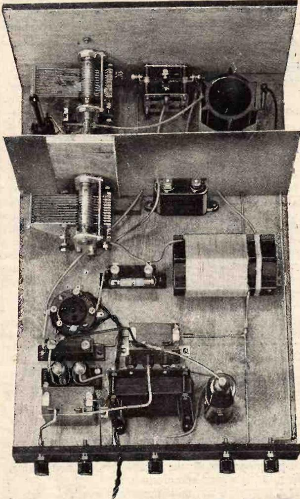
That the set is simple to construct is evident from this plan view. The centre terminal is for the H.T. + connection from the eliminator. The H.T. negative lead is joined to the earth terminal.
