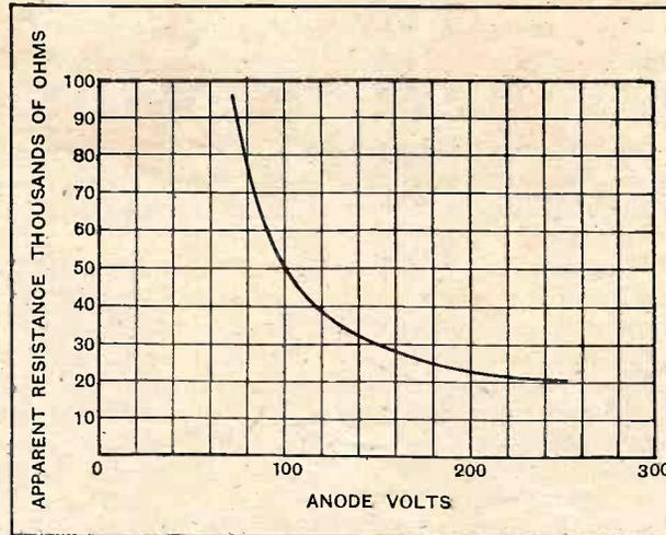
Fig. 2.—The apparent resistance of a valve obtained by dividing the anode voltage by the anode current. The curve is derived from the characteristic curve of Fig. 1.
