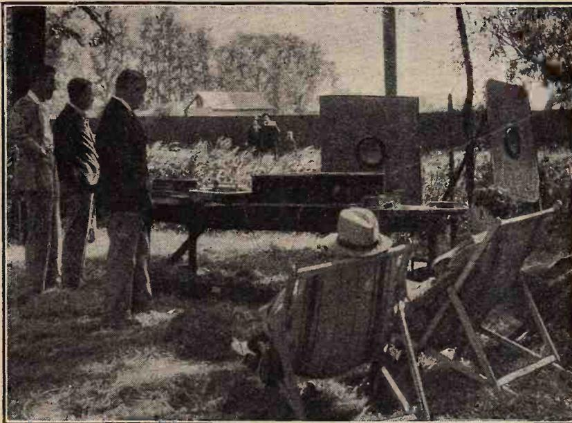
A SUMMER-TIME IDYLL. Members of the Hackney Radio Society conducting a loud speaker test at Hoddesdon. The amplifier, which operated on 400 volts H.T. from Exide accumulators, gave an undistorted output audible half a mile away. The society is planning another "outing" for September.
