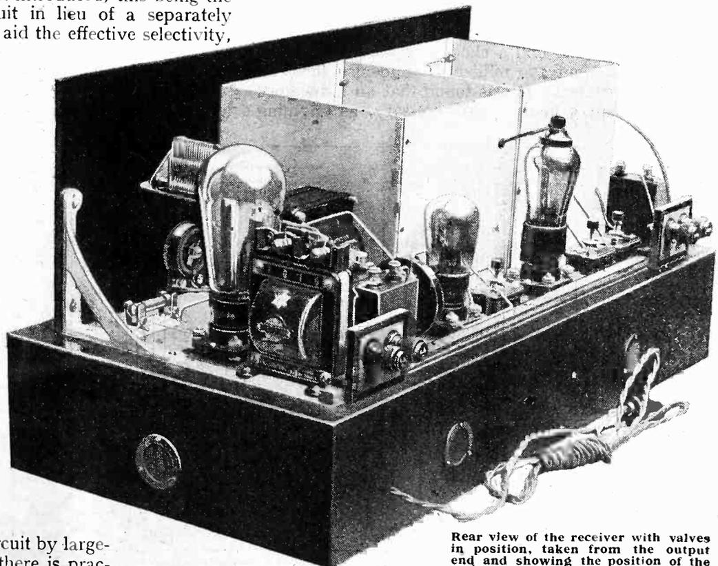
Rear view of the receiver with valves in position, taken from the output end and showing the position of the ventilating holes.
