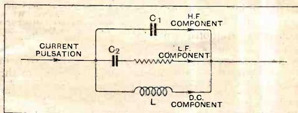
Fig. 2.—The current pulsations of Fig. 1 (b) are equivalent to the sum of a high-frequency component, a low-frequency component and a D.C. component. These three components can be separated by a circuit of the type shown.
