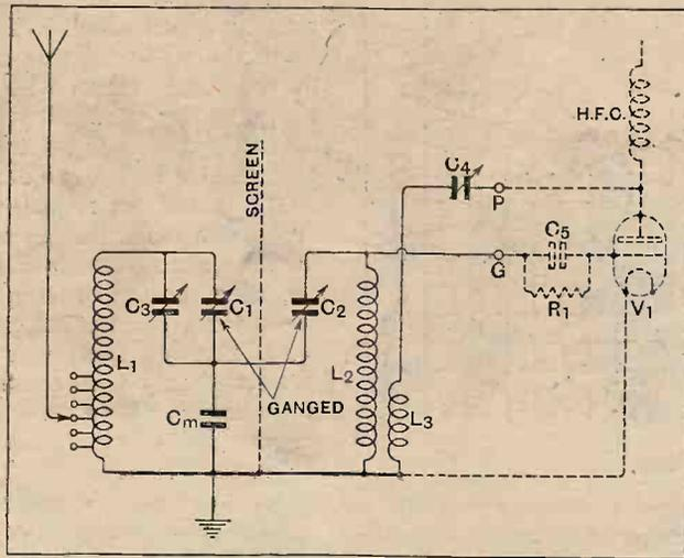
Fig. 1.—Circuit diagram of the band pass unit. The portion of the circuit in dotted lines represents the detector valve and its components which are not included in the unit.  $C_1, C_2$ , 0.0005 mfd. ganged condensers;  $C_3$ , 1.5 to 50  $\mu$ F. trimming condenser;  $C_m$ , 0.01 mfd.;  $C_1$ , 0.0003 mfd. variable condenser. The coil data are given in the appendix.
