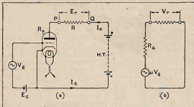
Fig. 2.—(a) A three-electrode valve with a resistance  $R$  in the anode circuit. The voltage  $E_r$  developed across  $R$  is proportional to the anode current. (b) Equivalent circuit relating to the A.C. components in the anode circuit when the grid voltage has an alternating component.  $V_r$  is the A.C. component of voltage developed across  $R$ . Voltage amplification  $n = \frac{V_r}{V_g} = \frac{\mu R}{R + R_a}$ .
