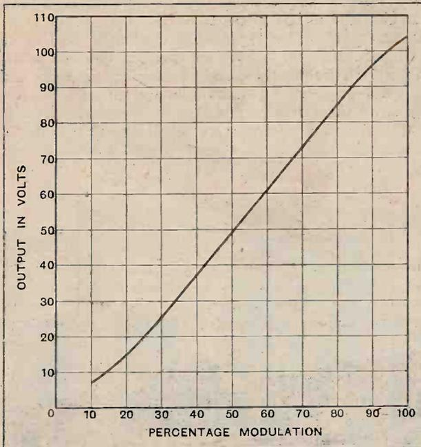
Fig. 5.—MODULATION-AMPLITUDE CURVE. Special B.B.C. test transmission on 356.3 metres, June 4th, 1930. The curve shows that distortionless demodulation (detection) is obtained for modulation up to about 90 per cent. The distortion for 100 per cent. modulation is small.
