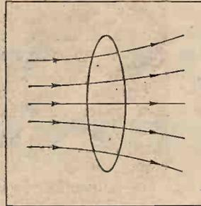
Fig. 3.—The magnetic field threading a conducting loop is opposed by the current which it induces in the loop.
