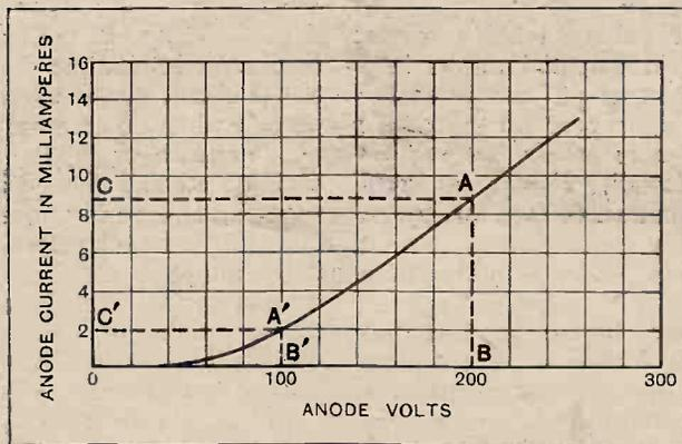
Fig. 1.—The anode voltage/anode current curve of a valve obtained with the grid potential fixed. At 200 volts the apparent or D.C. resistance is given by  $\frac{AC}{AB} = \frac{200}{0.0088} = 22,700$  ohms. At 100 volts the apparent resistance is  $\frac{A'C'}{A'B'} = 50,000$  ohms. Fig. 3 shows how the effective A.C. resistance is obtained.
