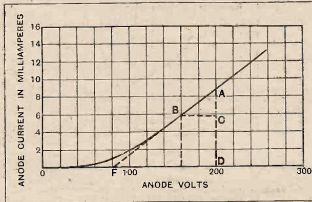
Fig. 3.—Diagram showing how the A.C. resistance or differential resistance is obtained from an anode voltage/anode current characteristic curve of a valve. The A.C. resistance is given by  $R_a = \frac{FD}{AD} = \frac{118}{0.0088} = 13,400$  ohms.
