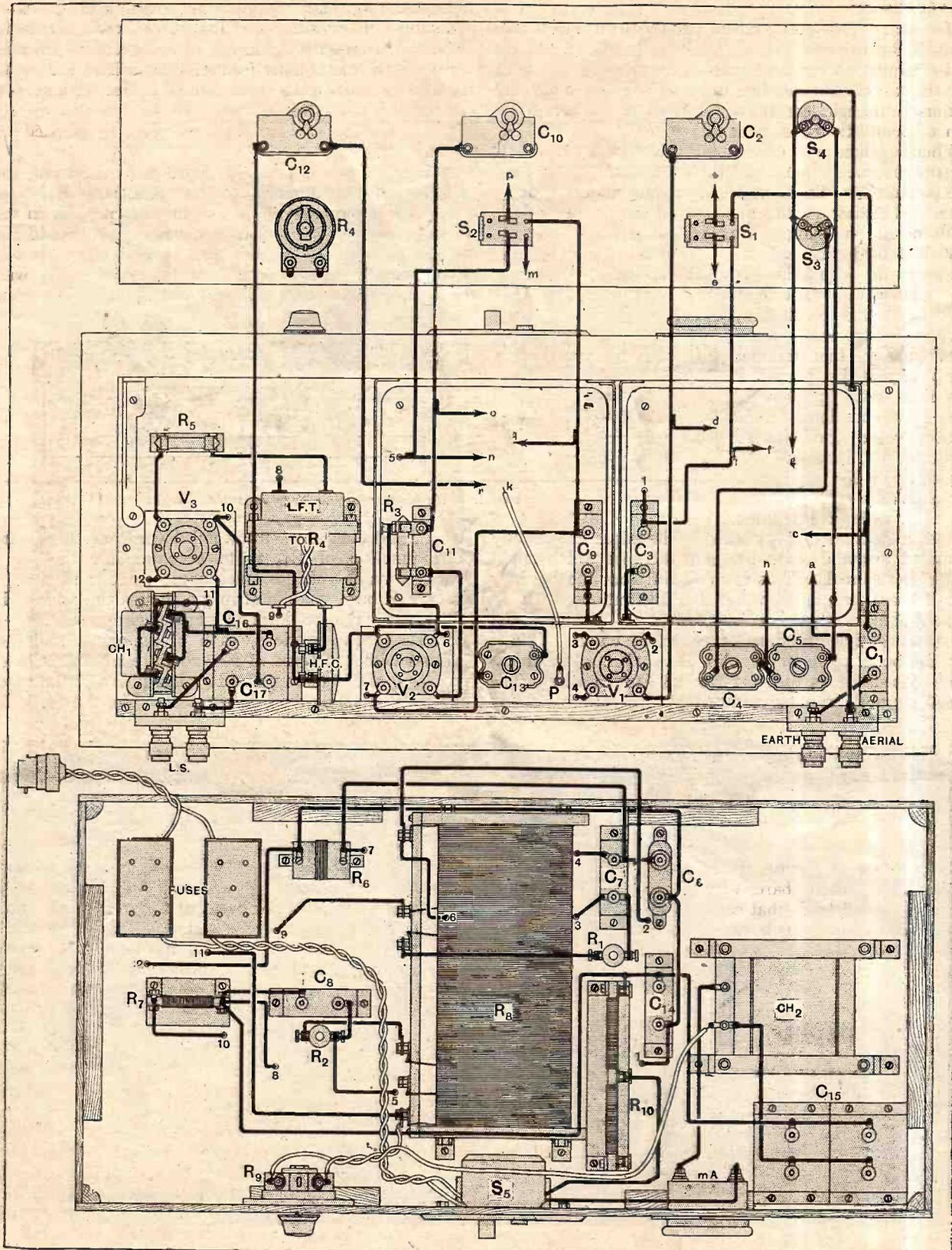
Practical wiring diagram. Figures indicate holes where leads pass through the base. The lettering refers to the coil connections and corresponds with similar lettering on the theoretical diagram.
