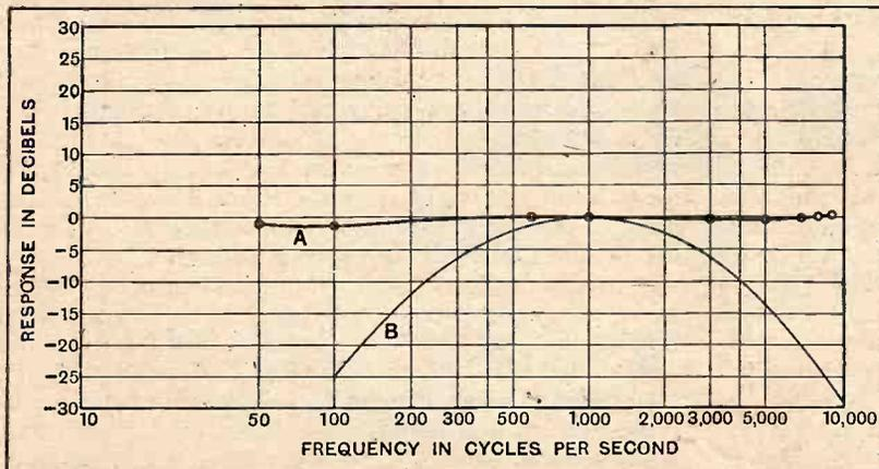
Fig. 4.—FREQUENCY RESPONSE CURVE. Special B.B.C. test transmission on 356.3 metres, June 4th, 1930. Curve A shows  $20 \log_{10} \left( \frac{v}{v_{1000}} \right)^2$  where  $v$  is the receiver output voltage and  $v_{1000}$  is the value of this voltage at 1,000 cycles per second. Transmitter modulation voltage constant. Curve B is for a small portable receiver measured under like conditions.
