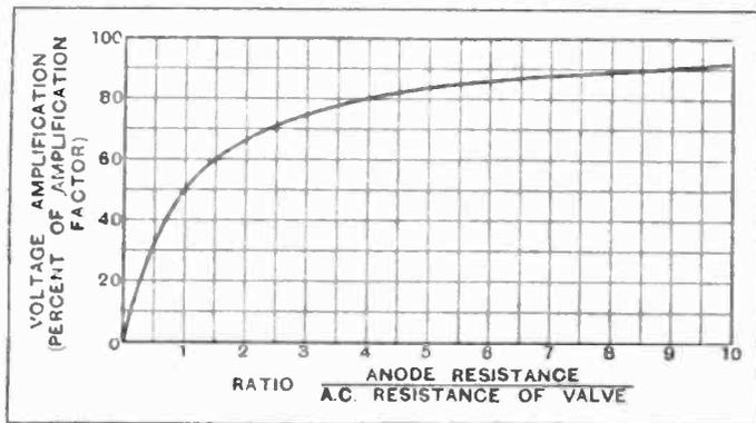
Fig. 2.—Curve showing how the voltage amplification, expressed as a percentage of the amplification factor of the valve, depends on the ratio of anode resistance to A.C. valve resistance. This curve applies to any three-electrode valve.
