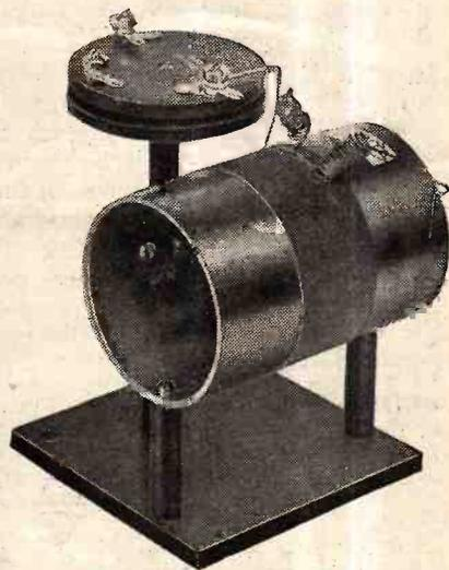
Dual range coils for the "Band Pass Four" made by Wright and Weaire.
