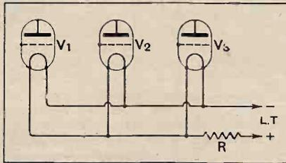
Fig. 1.—Illustrating the danger of over-running filaments when they are connected in parallel across a high-voltage source of supply.
