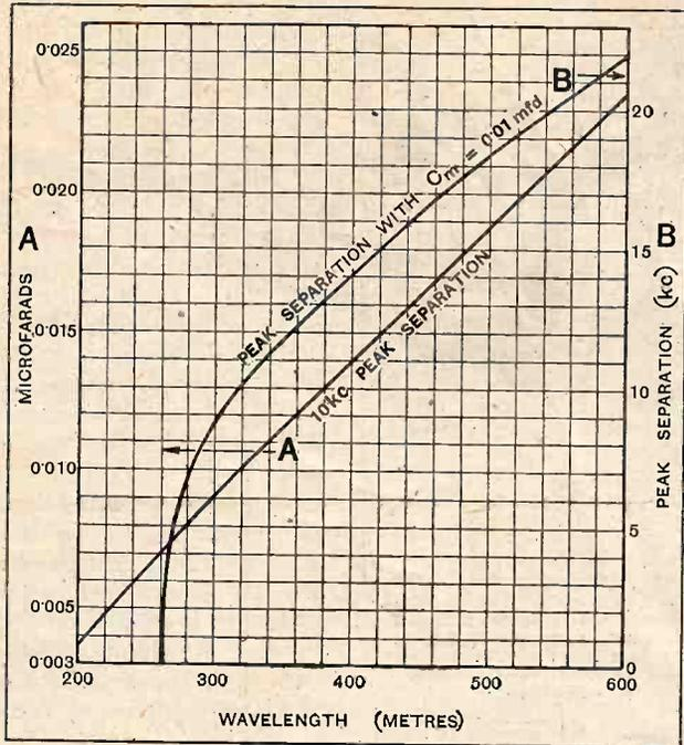
Fig. 3.—Filter characteristics of the band pass unit. Curve A to be read in conjunction with the vertical scale on the left shows the coupling capacity necessary to give the optimum peak separation of 10 k.c. at any wavelength between 200 and 600 metres. Curve B to be used with the vertical scale on the right gives the peak separation at various wavelengths which will be obtained when using a fixed coupling capacity ( $C_m$ ) of 0.01 mfd.
