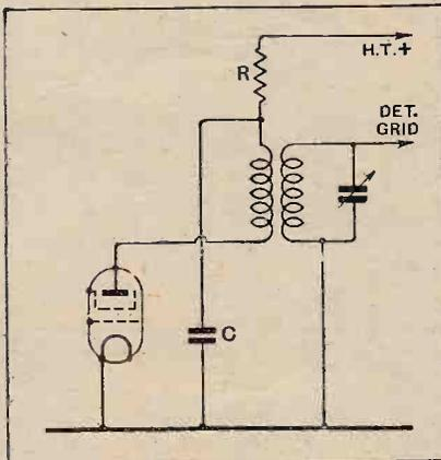
Fig. 1.—Showing where insulation failures may occur in an H.F. anode circuit.
