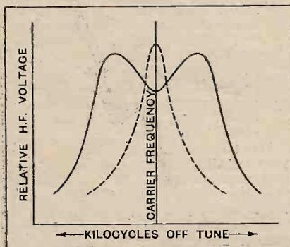
Fig. 2.—Resonance curves of a filter and of a single-circuit intervalve coupling.
