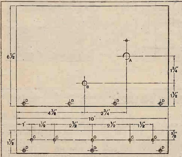
Dimensions and drilling data of the panel and terminal strip. A = 7/16 in. dia.; B = 5/16 in. dia.; C = 5/32 in. dia.; D = 1/8 in. dia. and countersunk for No. 4 wood screws.
