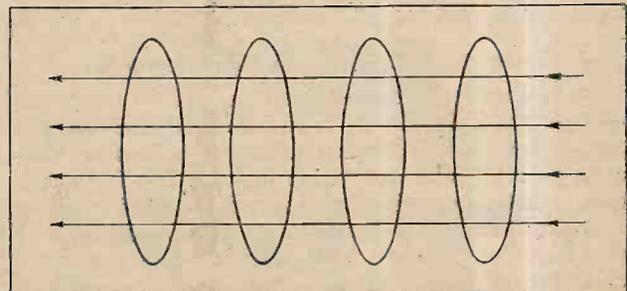
Fig. 5.—An arrangement of loops giving more effective screening for fields parallel to the axis of each loop.
