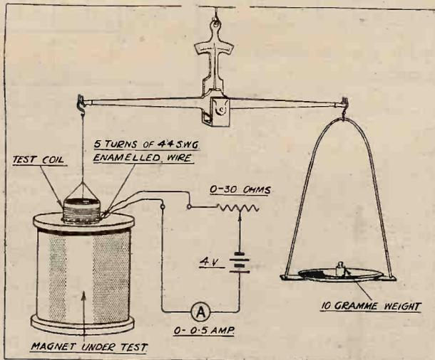
Fig. 1.—The arrangement of apparatus for the measurement of flux-density.
