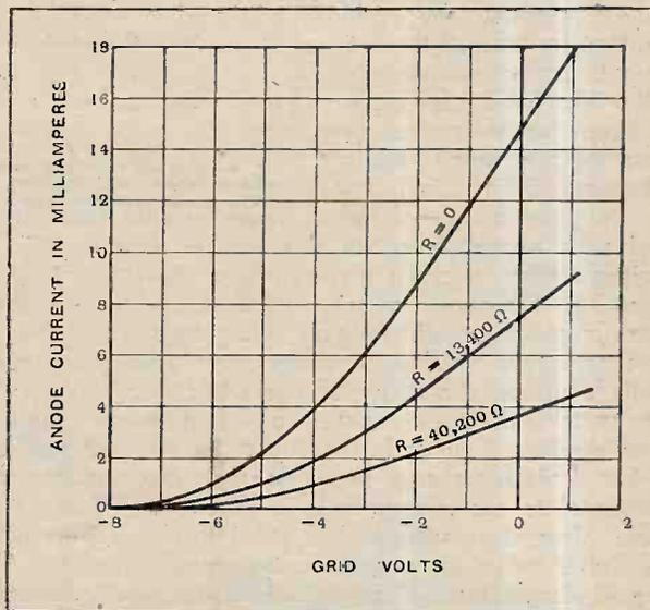
Fig. 3.—Curves showing how resistance inserted in the anode circuit affects the anode current of a valve. The A.C. resistance of the valve is 13,400 ohms and its amplification factor 36. The curves correspond to 200 volts H.T. supply throughout. The numbers attached to the curves indicate the resistance connected in the anode circuit.
