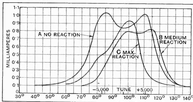
Fig. 6.—REGIONAL. M=12 turns. Showing effect of reaction.
