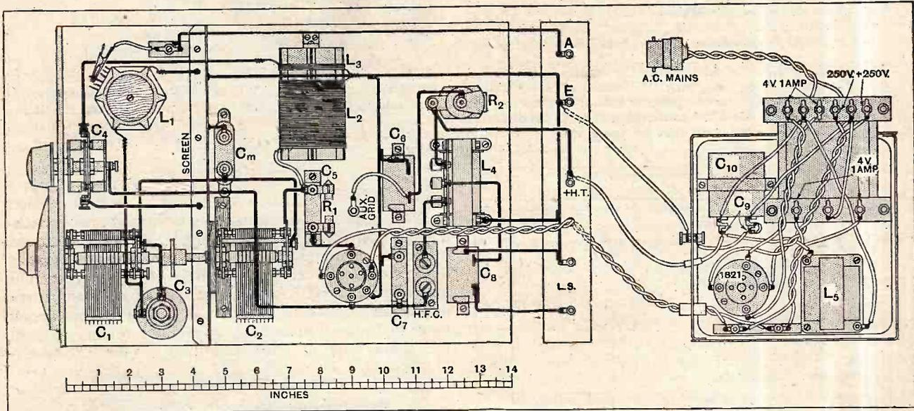
General wiring plan. The smoothing condenser  $C_{10}$  is held vertically above  $C_9$  by a small metal strap. The dimensions of the vertical screen are the same as those of the panel.
