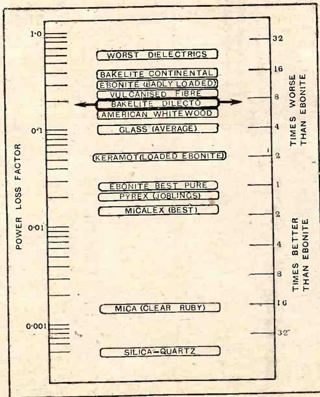
Fig. 1.—The relative power factor of Bakelite in comparison with pure ebonite is shown on the above chart.
