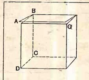
Fig. 7.—An incomplete screening box in which only the end surfaces are effective in screening fields perpendicular to A, B, C, D, until contact is made along the edge A G.
