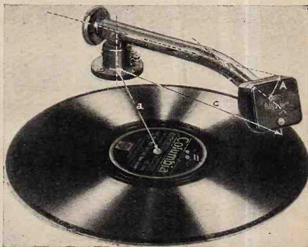
Fig. 2.—Correct needle-track alignment for practical purpose is obtained by setting the pick-up at an angle to the tone arm. The angle A is determined by the distances a and c.
