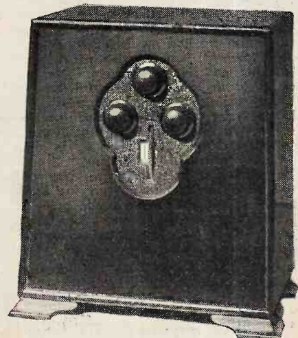
Ediswan Power Pentode Two receiver for all-mains operation.
