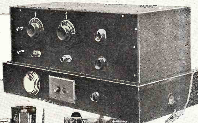
ALL D.C. THREE. Batteryless three-valve receiver with rejectors for the elimination of local stations. All valve current and grid bias are derived from the mains, and the set gives humless reception when plugged into any D.C. supply. ("The Wireless World," August 20th, 1930.)
