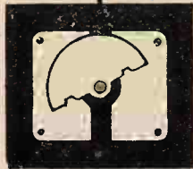
The vanes are carefully shaped to ensure that the capacity change will be the same for both halves and constant throughout the full range. Satisfactory operation of differential reaction depends upon accurate balance in the condenser.
