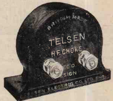
Telsen H.F. Chokes, designed to cover the whole wave-band range from 18 to 4,000 metres, extremely low self-capacity, shrouded in Genuine Bakelite. Inductance 150,000 microhenrys, resistance 400 ohms. Price 2/6 each.
