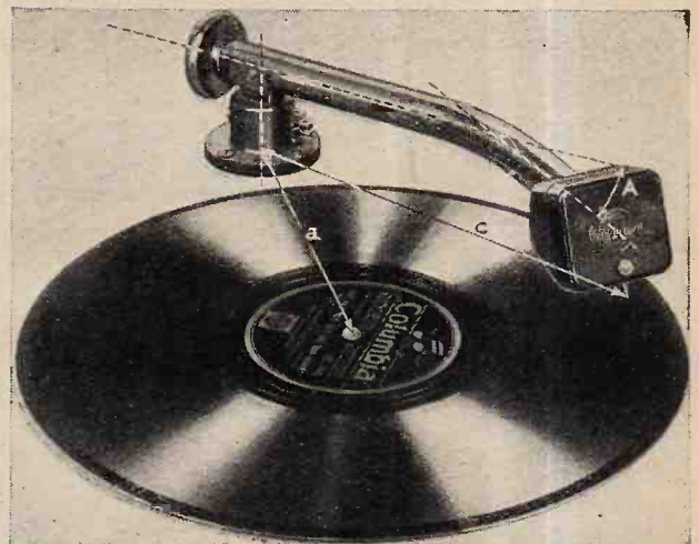
Fig. 2.—Correct needle-track alignment for practical purpose is obtained by setting the pick-up at an angle to the tone arm. The angle A is determined by the distances a and c.
