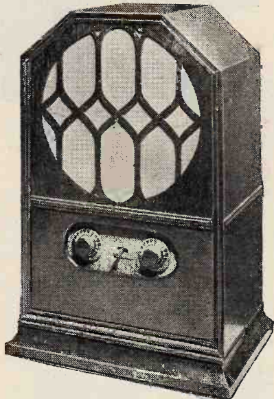
Truvox all-mains two-valve set, with exponential horn loud speaker.
