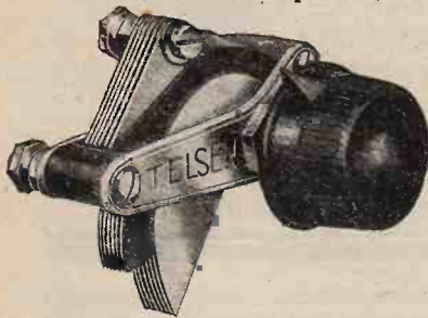
Telsen Variable Condensers (Bakelite Dielectric). Particularly designed for use as a reaction condenser, may also be used as a neutralising condenser where large capacity is necessary. All vanes are insulated with Bakelite which eliminates the possibility of a short circuit between the moving and fixed vanes. Made in three capacities:—.0005, .0003, .00015, supplied complete with pointer knob with one hole fixing for panel mounting. Price 3/- each.
