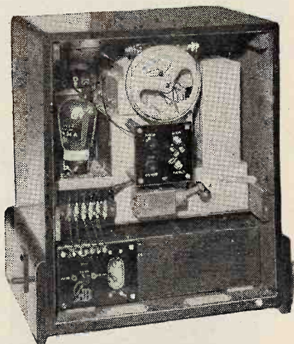
Interior view of the McMichael three-valve mains set.
