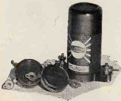
Formo eliminator and by-pass condensers.
