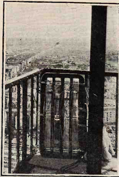
TWELVE-MILE VOICE. The giant Blatthaller loud speaker on the wireless tower at the Berlin Radio Show. It is claimed that the speaker was heard twelve miles distant. The "membrane" consists of corrugated aluminium sheet with an extreme movement of over \frac{1}{2} inch.
