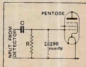
Fig. 21.—Owing to feed-back across the plate-grid capacity of the pentode a large effective capacity appears between filament and grid and tends to shunt the grid leak at high audio frequencies.
