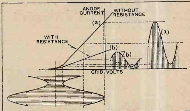
Fig. 29.—Anode bend detection. The effect of plate resistance in the detector valve circuit.
