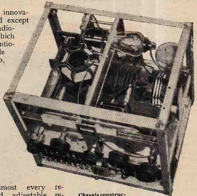
Chassis construction of the new Ferranti three-valve receiver. Transverse ganging of the tuning condensers is provided and trimming is accomplished by means of a rocking stator.
