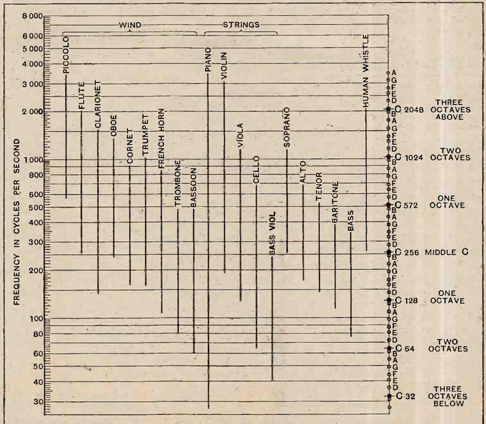
Fig. 5.—On the left is a logarithmic scale of frequencies, on the right are the notes corresponding to the white keys of the piano. The upper limits shown for instruments are not necessarily the highest notes that can be produced, but the highest notes found in orchestral scores.
