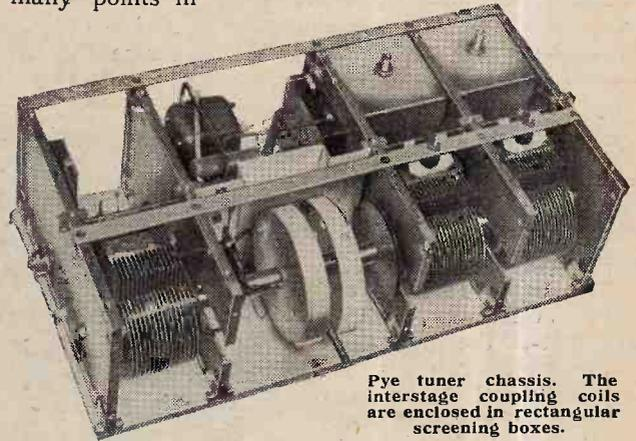
Pye tuner chassis. The interstage coupling coils are enclosed in rectangular screening boxes.
