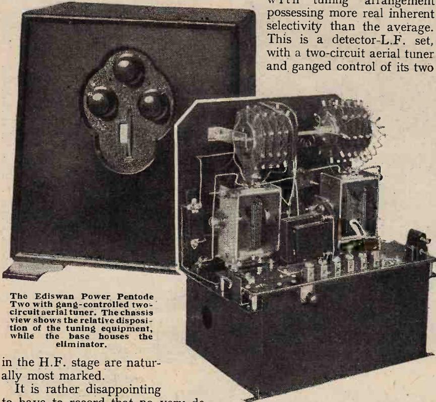
The Ediswan Power Pentode Two with gang-controlled two-circuit aerial tuner. The chassis view shows the relative disposition of the tuning equipment, while the base houses the eliminator.
