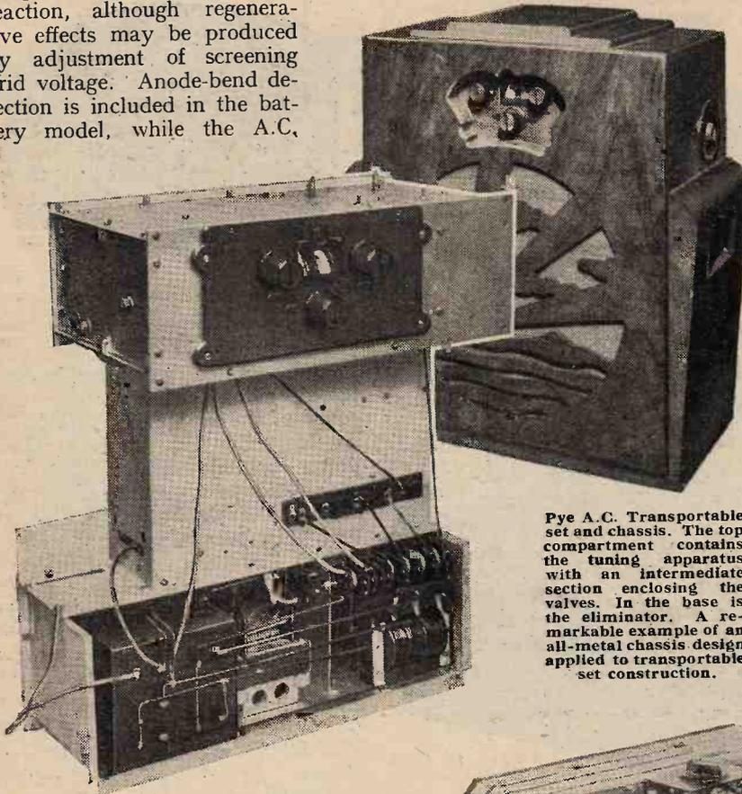
**Pye A.C. Portable set and chassis.** The top compartment contains the tuning apparatus with an intermediate section enclosing the valves. In the base is the eliminator. A remarkable example of an all-metal chassis design applied to portable set construction.
