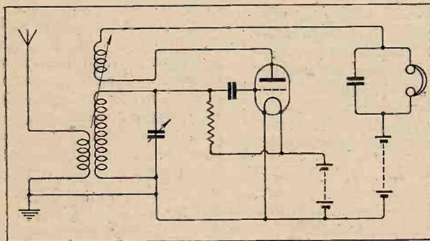
Fig. 1.—Single-valve receiver. This simple set will perform the frequency-changing operation which is the whole foundation of the superheterodyne receiver.
