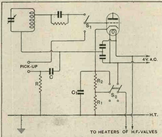
Fig. 2.—The method of adding a pick-up when the H.F. valves must be switched off. The resistance R is 0.25 meg.;  $R_1$  is the normal bias resistance of 100 ohms and  $R_2$  is 400 ohms. C and  $C_1$  are respectively 1 mfd. and 2 mfd.
