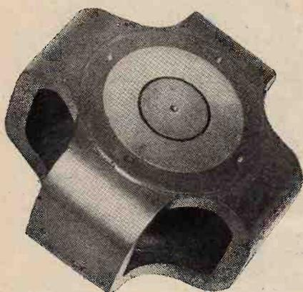
Swift, Levick permanent magnet with soft iron pole pieces. Flux densities of 8,000 lines per sq. cm. in a 1.5 mm. gap have been achieved with 9 per cent. cobalt alloy.
