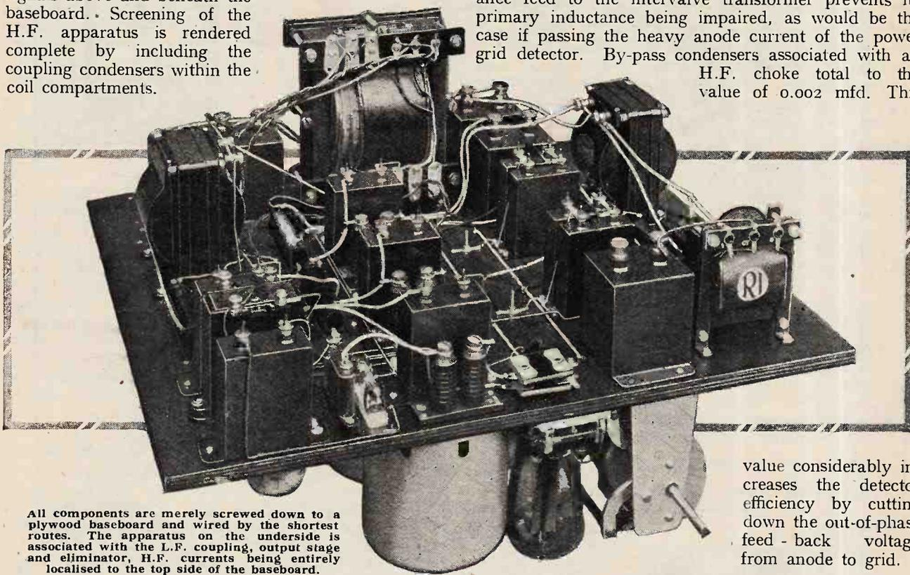
All components are merely screwed down to a plywood baseboard and wired by the shortest routes. The apparatus on the underside is associated with the L.F. coupling, output stage and eliminator, H.F. currents being entirely localised to the top side of the baseboard.
