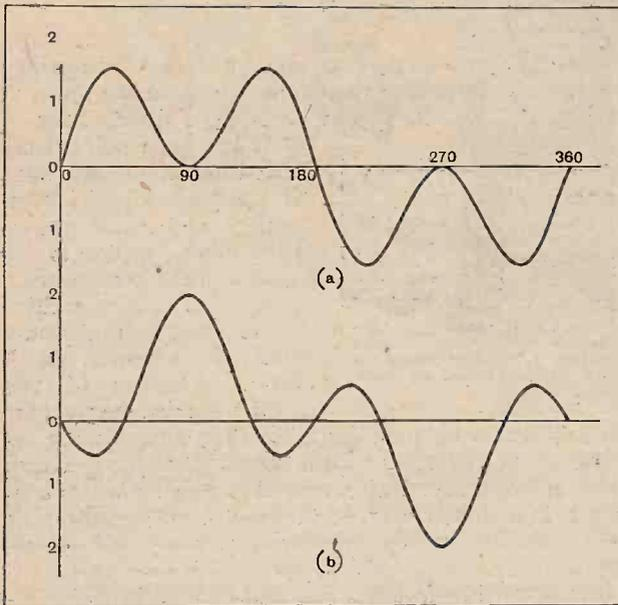
Fig. 4.—Pressure wave due to frequencies  $f$  and  $3f$  of equal amplitude; (a) fundamental and harmonic in phase; (b)  $180^\circ$  out of phase. The change of phase modifies the resultant wave profoundly.
