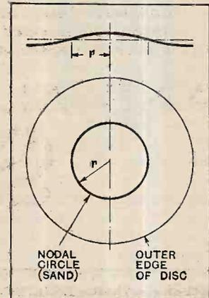
Fig. 3.—Diagram showing shape of disc when there is one nodal circle (exaggerated).
