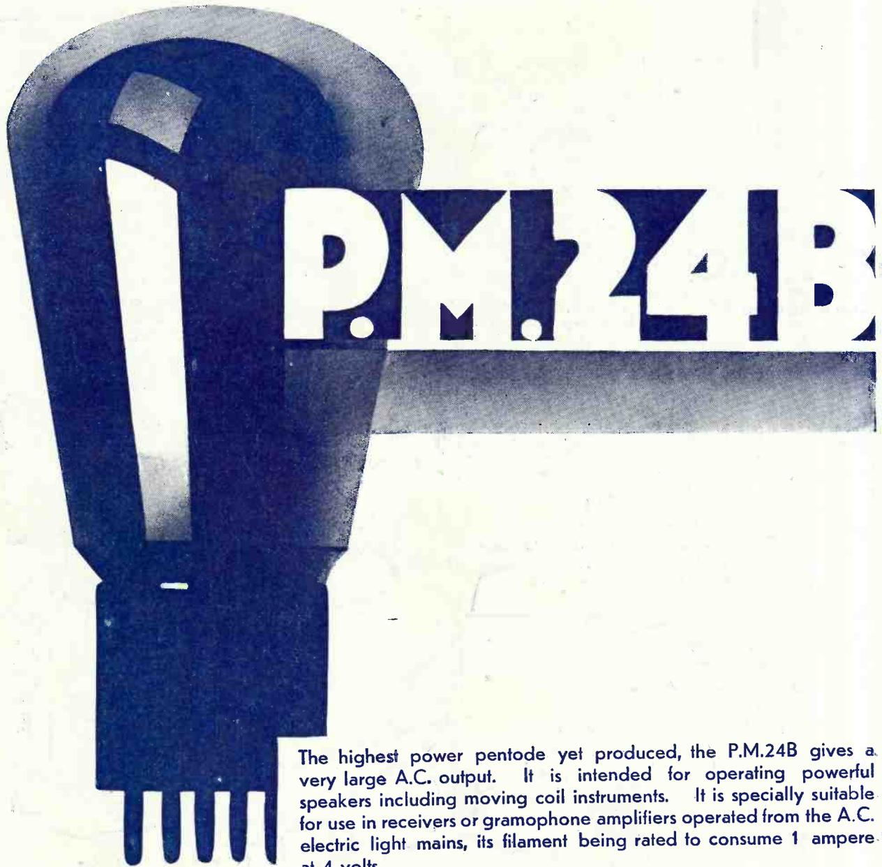
The highest power pentode yet produced, the P.M.24B gives a very large A.C. output. It is intended for operating powerful speakers including moving coil instruments. It is specially suitable for use in receivers or gramophone amplifiers operated from the A.C. electric light mains, its filament being rated to consume 1 ampere at 4 volts.
