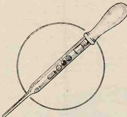
The Sopranoist battery tester (Kalisky).
