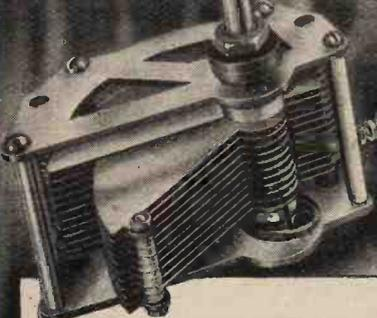
Truly logarithmic and definitely to the capacity stated, the Lotius Logarithmic Condenser ensures smooth firm tuning. Ample spacing is allowed to prevent any possibility of short circuiting of vanes.
