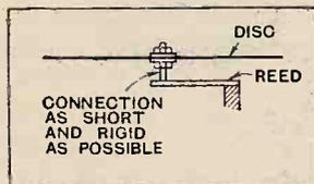
Fig. 1.—The force exerted by a reed at the centre of the disc is not felt instantaneously throughout the disc.
