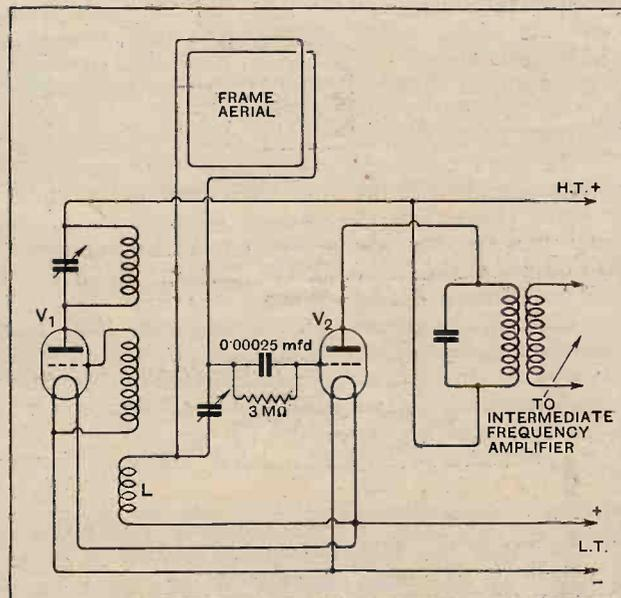
Fig. 1.—Circuit diagram of the frequency changer of an American superheterodyne (date about 1924), designed for use with UV.201a valves.  $L$  is coupled variably to the grid coil of the oscillator  $V_1$ . The valve  $V_2$  is adjusted as grid leak rectifier.
