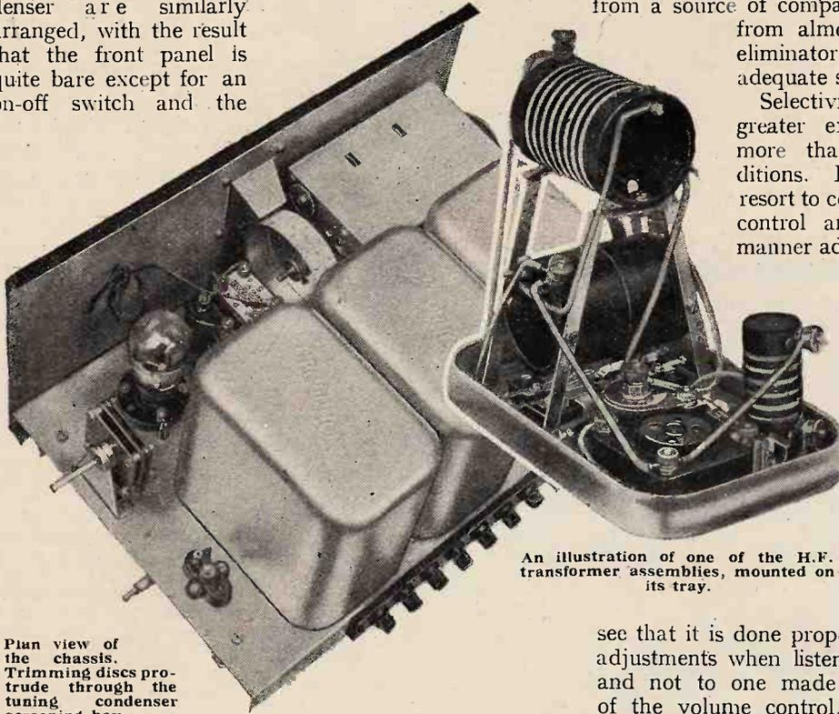
An illustration of one of the H.F. transformer assemblies, mounted on its tray.
