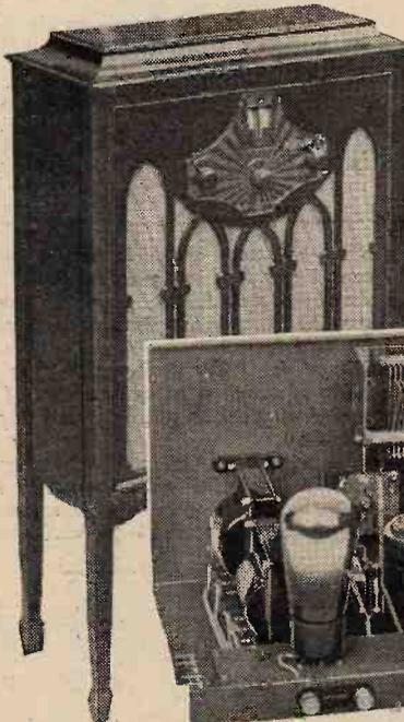
Burndep Type 1850 chassis, with semi-ganged tuning, large-diameter inductances and completely screened anode coupling coils, which are mounted behind the detector valve.
