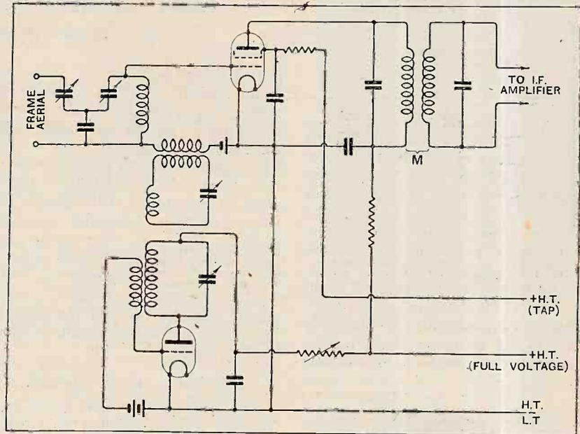
Fig. 5.—An elaborate frequency changer including precautions against most of the possible difficulties discussed in the text. There is a band-pass filter for the signal frequency, an intermediate tuned circuit between oscillator and detector, while the I.F.A. coupling takes the form of a band-pass filter. A screen-grid valve is used as anode bend detector, and the whole is fully decoupled.
