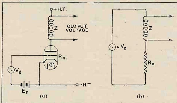
Fig. 1.—For a valve to act as an amplifier of voltages a high value of impedance,  $Z$  must be connected in the anode circuit. The simplified circuit shown at (b) is equivalent to the anode circuit of the valve as far as the alternating components are concerned. The amplification factor of the valve is  $\mu$ .
