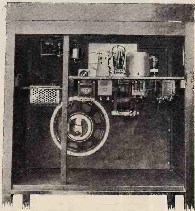
Interior of radio-gramophone showing the supports for the chassis with the loud speaker and gramophone motor in position.
