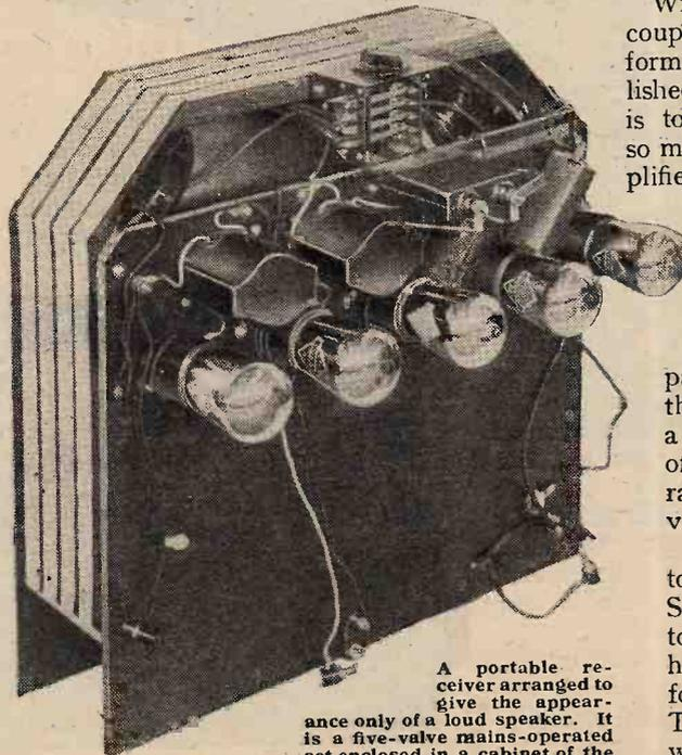
**A portable receiver arranged to give the appearance only of a loud speaker.** It is a five-valve mains-operated set enclosed in a cabinet of the normal dimensions of a table model loud speaker (Umello).
