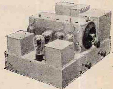
**Majestic "Super Screen Grid" chassis, with valve screen removed.**
