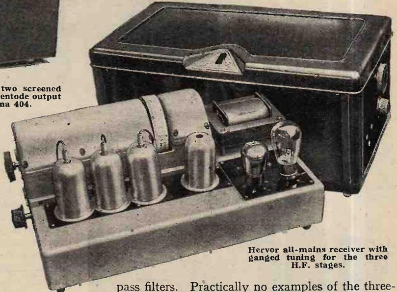
Hervor all-mains receiver with ganged tuning for the three H.F. stages.
