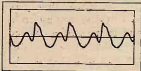
Fig. 2.—Pressure wave of organ note sounding at 256 c.p.s. as recorded by Prof. D. C. Miller. The note contains a large number of overtones.
