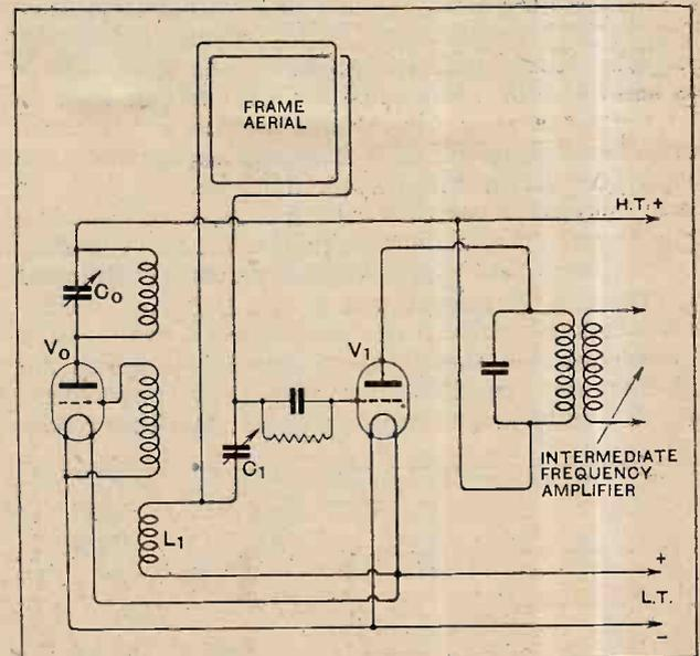
Fig. 5.—The frequency-changer of an American superheterodyne of good repute (the Haynes-Griffin).  $V_1$  is the first detector, and  $V_0$  the oscillator.  $C_1$  and  $C_0$  are the only two tuning controls, yet the set, which employed seven valves, was highly selective. The coupling coil  $L_1$  was used to apply the oscillations of  $V_0$  to the grid of  $V_1$ , through the frame circuit.
