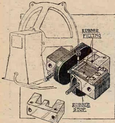
Lamplugh inductor loud speaker unit with die-cast end plate removed.
