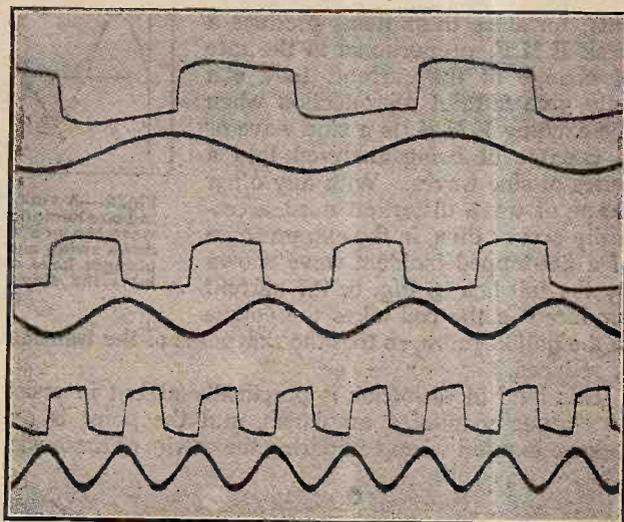
Fig. 7.—Reproduction of flat-topped waves by a 6-stage amplifier devoid of inertia. The sine curves are timing waves of frequencies 80, 150 and 300 c.p.s.
