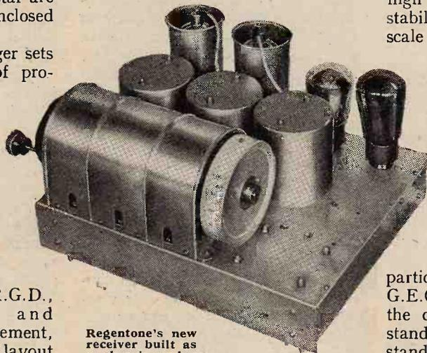
Regentone's new receiver built as a chassis and embodying ganged tuning, screened coils and valves, while the decoupling and voltage regulating equipment is carried in the recessed metal base.
