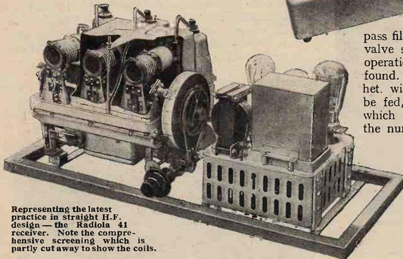
Representing the latest practice in straight H.F. design — the Radiola 41 receiver. Note the comprehensive screening which is partly cut away to show the coils.
