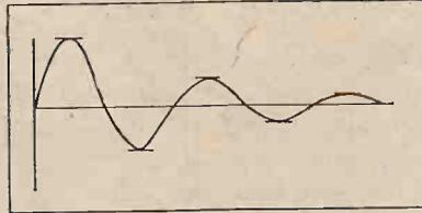
Fig. 8.—A train of damped waves acting on a loud speaker. In each complete wave the up swing is greater than the down swing and the forces on the diaphragm have a resultant tending to leave the diaphragm in a displaced position.
