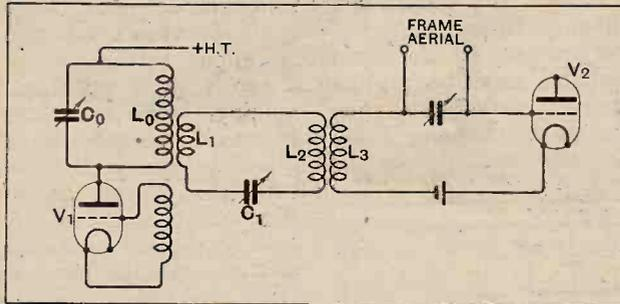
Fig. 3.—An intermediate tuned circuit  $L_1C_1L_2$ , interposed between the oscillator and the detector coupling coil  $L_3$ . This filters out harmonics generated by the oscillator if the coupling between  $L_1$  and  $L_0$  is not too tight. The condensers  $C_0$  and  $C_1$  may be ganged without much difficulty.
