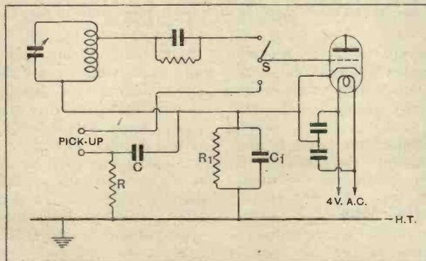
Fig. 1.—A simple method of adding a gramophone pick-up. R and C are the decoupling resistance and condenser of 0.25 meg. and 1 mfd. respectively, while  $R_1$  and  $C_1$  are the normal H.F. biasing resistance of 100 ohms and the by-pass condenser of 2 mfd.
