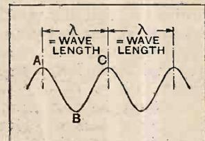
Fig. 4.—A simple waveform. With a frequency of 1,500 cycles per second the wave travels 1,500 times the distance AC every second.
