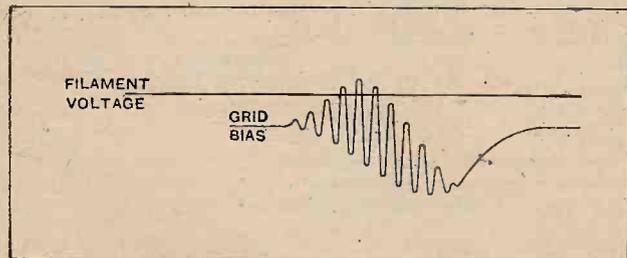
Fig. 20.—Blocking effect in power valve. If the grid happens to swing positive to the filament it becomes charged, and if the product RC (Fig. 17) is too large the valve is paralysed for an appreciable time.
