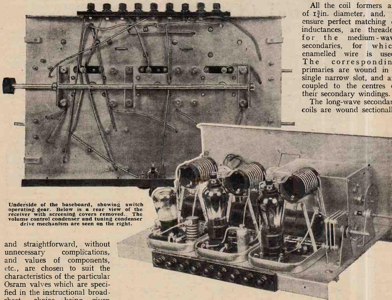
Underside of the baseboard, showing switch operating gear. Below is a rear view of the receiver with screening covers removed. The volume control condenser and tuning condenser drive mechanism are seen on the right.
