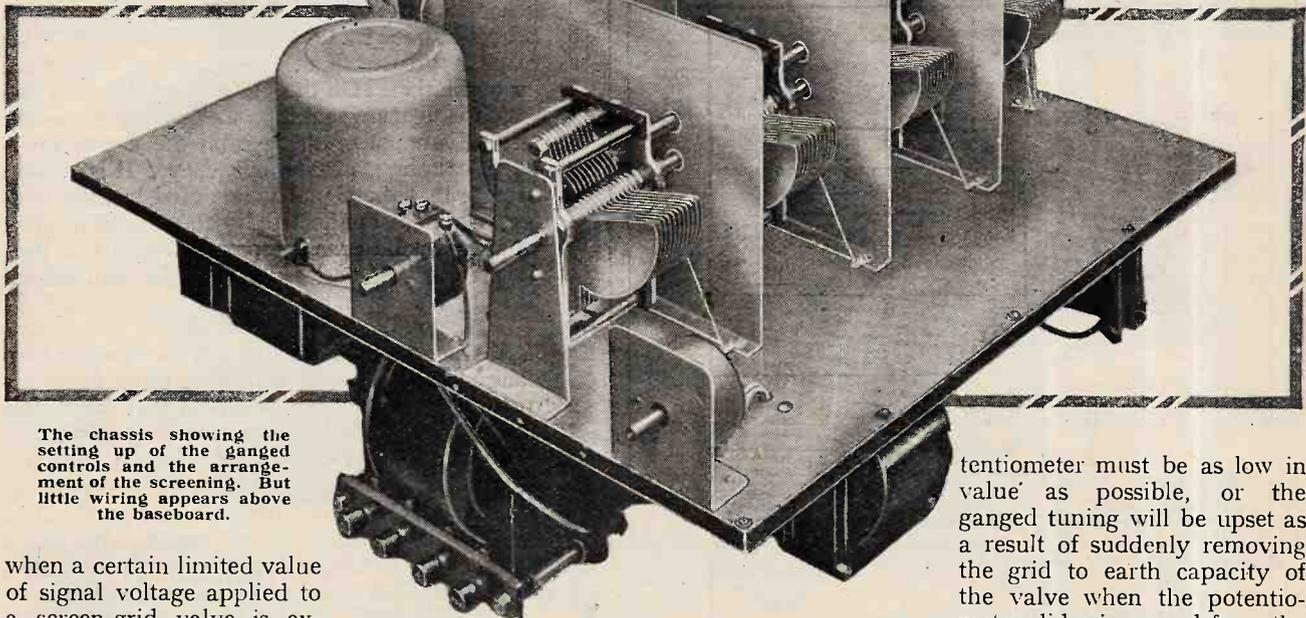
The chassis showing the setting up of the ganged controls and the arrangement of the screening. But little wiring appears above the baseboard.
