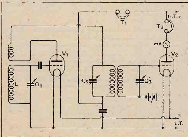
Fig. 3.—The simplest "superbet." The oscillating detector *V*<sub>1</sub> acts as frequency-changer, and the detector *V*<sub>2</sub> acts as receiver of the signals on the new frequency.
