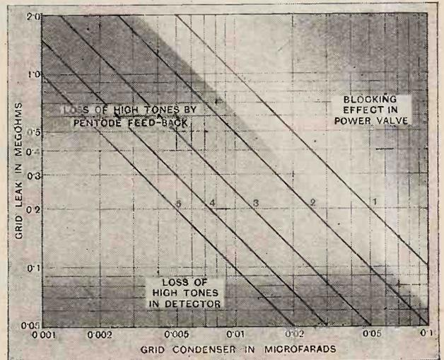
Fig. 18.—The product RC is constant along any of the numbered lines, with a different value for each line. The heavily shaded regions are to be avoided when using the set shown in Fig. 17.
