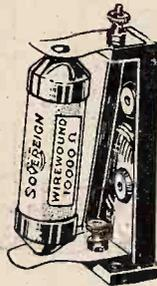
WOUND statically to avoid back coupling, with silk covered wire in a sectionalised manner on a bakelite former. The value of all resistances is guaranteed within 5% of stated figures. PRICES INCLUDING BASE:
