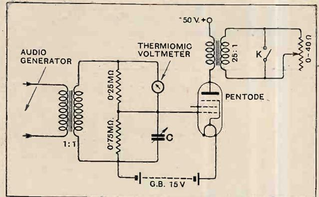
Fig. 31.—Determination of the grid input impedance of a loaded pentode.
