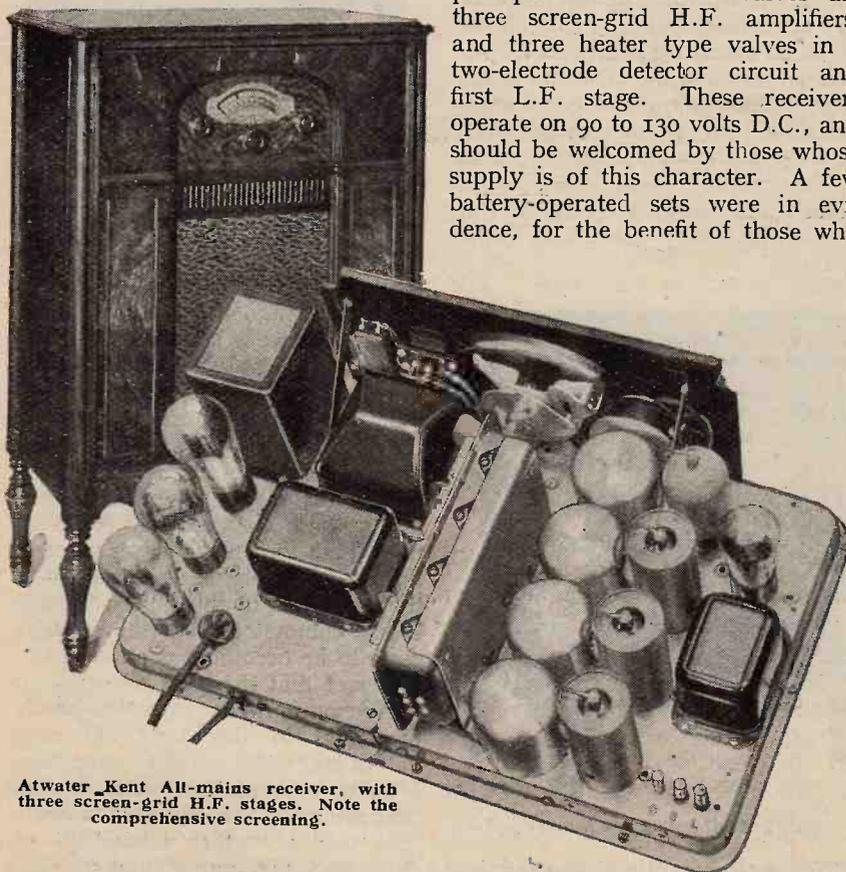
Atwater-Kent All-mains receiver, with three screen-grid H.F. stages. Note the comprehensive screening.
