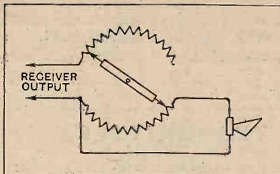
Fig. 1.—A "constant impedance" method of controlling volume.
