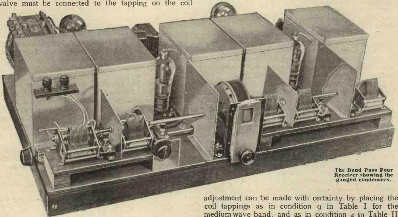
The Band Pass Four Receiver showing the ganged condensers.
