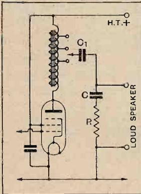
Fig. 4.— Output circuit (tapped choke) for pentode with moving-iron speaker. C<sub>1</sub> = 2 mfd., R = 10,000 ohms, C = 0.01 mfd. These last two values are subject to considerable variation to suit the speaker.
