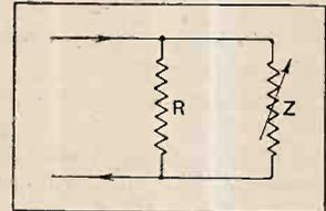
Fig. 3.—In this simplified diagram Z stands for the varying impedance of a moving-iron loud speaker while R is a compensating resistance.
