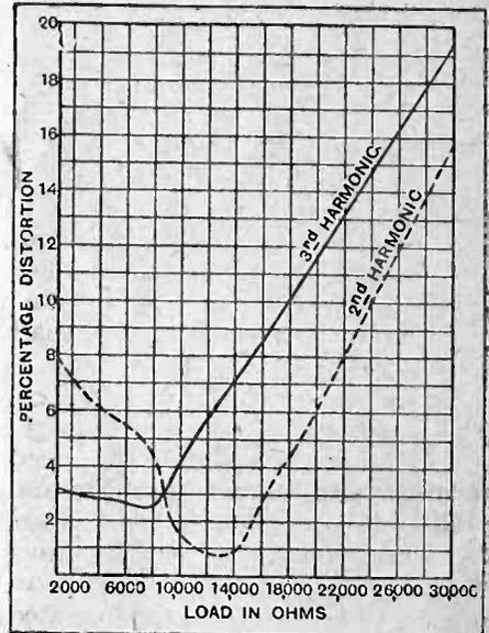
audible distortion when a small deviation is made from the optimum load, a pentode will give a poor
