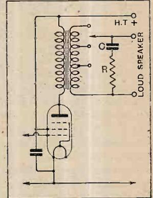
Fig. 5.— An equivalent circuit to that of Fig. 4, using a multi-ratio transformer in place of a tapped choke.
