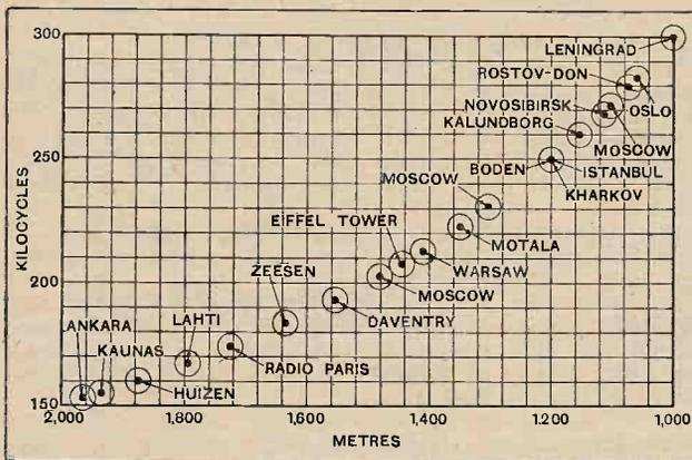
The above diagram has been prepared to illustrate the letter from the Chief Engineer of the B.B.C. The positions of most of the principal long-wave stations are indicated with their kilocycle separation. The circles drawn round each station are intended to indicate the spread, the width on either side of the carrier being taken as 5 kc.
