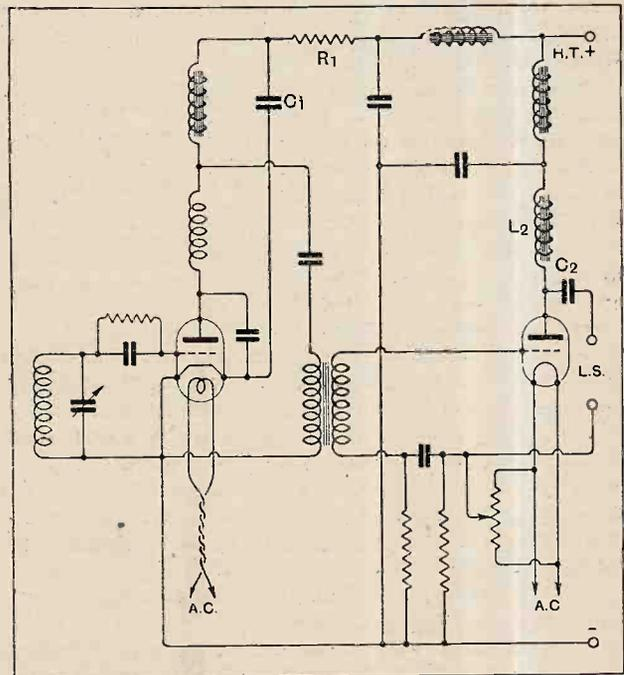
Fig. 2.—The complete choke transformer coupled circuit with a single output valve. As explained in the text, this circuit is not entirely satisfactory. With a 200 volts H.T. supply,  $R_1$  must be 8,600 ohms and  $C_1$  about 8 mfd., while the choke  $L_2$  must have an inductance of 50 henrys when  $C_2$  is 4 mfd.
