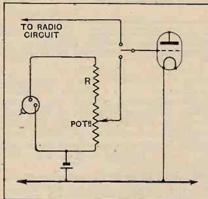
Fig. 1.—By connecting a fixed resistance in series with the controlling potentiometer, the maximum value of gramophone reproduction may be reduced to any desired extent.
