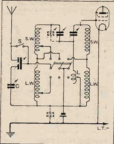
Fig. 2.—A band-pass filter with variable inductive coupling; the differential aerial input control may be short-circuited by the switch S. C. aerial capacity balancing condenser; L, coupling inductance; S.W., short-wave coils; L.W., long-wave coils.
