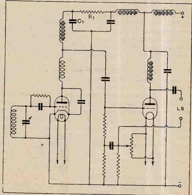
Fig. 4.—A satisfactory circuit with a single output valve; owing to the low amplification, feedback effects are very small. The resistance  $R_1$  should have a value of 8,600 ohms, with a 200 volts H.T. supply, and the condenser  $C_1$  a capacity of from 2 mfd. to 4 mfd.
