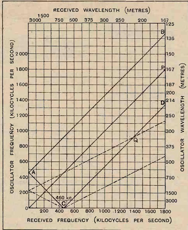
Fig. 2.—Relationship between received and oscillator frequencies for a superheterodyne using an intermediate frequency of 460 kc. (Kramolin.)
