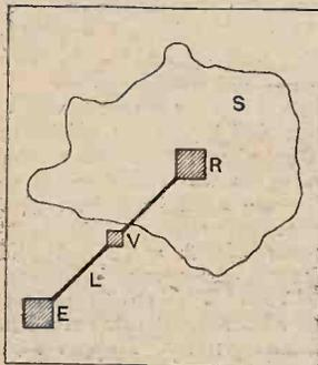
Fig. 1.—Schematic diagram of a field-strength amplifying equipment with land-line connection. S=Urban area; E=Central receiving station; L=Line connection; R=Relay transmitter; V=Intermediate high-frequency amplifier (Aperiodic).
