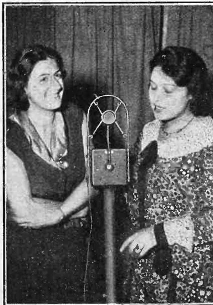
**A NEW MICROPHONE.** In this condenser microphone now used at the Munich broadcasting station the "A" amplifier is incorporated in the instrument.
