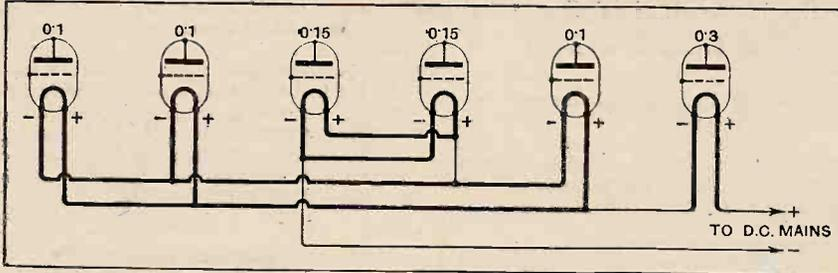
Fig. 2.—Series-parallel filaments. Each group (connections shown in heavy lines) consumes 0.3 amp. Polarity and current consumption of individual valves are indicated.
