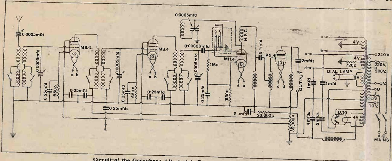
Circuit of the Geophone All-electric Four-valve Receiver, type B.C.3140.
