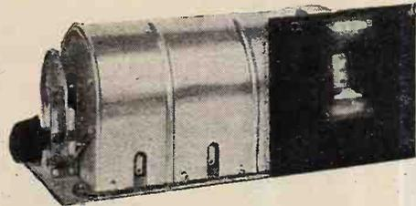
The "Tub" shown fitted with Drum Dial reading but controlled by end drive.
