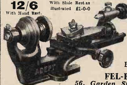
Many uses can be found for this handy tool. Cutting slots in Formers. Winding Coils and chokes to mention but three—besides ordinary lathe work. Takes work up to 3in. dia. Gap provided to increase centre to 2 1/4".
