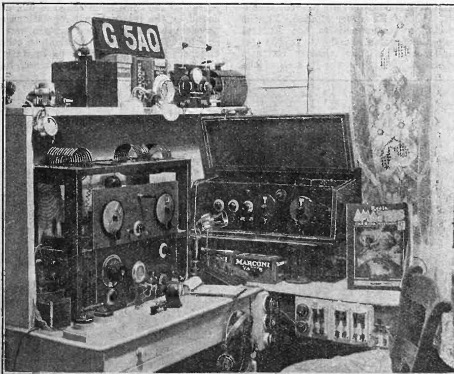
**AN ACTIVE TRANSMITTER.** G5AQ, owned and operated by Mr L. A. Carter at Putland Cottage, Heathfield, Sussex. The 10-watt transmitter consists of a crystal oscillator controlling a TP-TG oscillator. Choke control is used for telephony. The receiver shown is an O-V-2. Up to the end of September 37 countries had been worked on CW and most of Europe on telephony. Mr. Carter works regular schedules (phone and music) every Sunday from 9.30 to 10.0 a.m.
