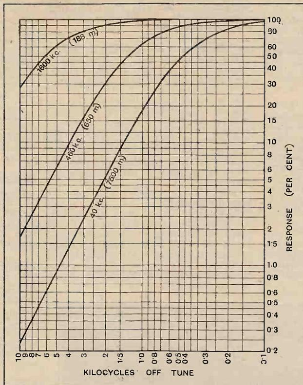
Fig. 5.—Comparative selectivity of intermediate amplifiers working at different frequencies. The very high selectivity associated with the superheterodyne method of reception is due entirely to the use of a very long wave for intermediate amplification.
