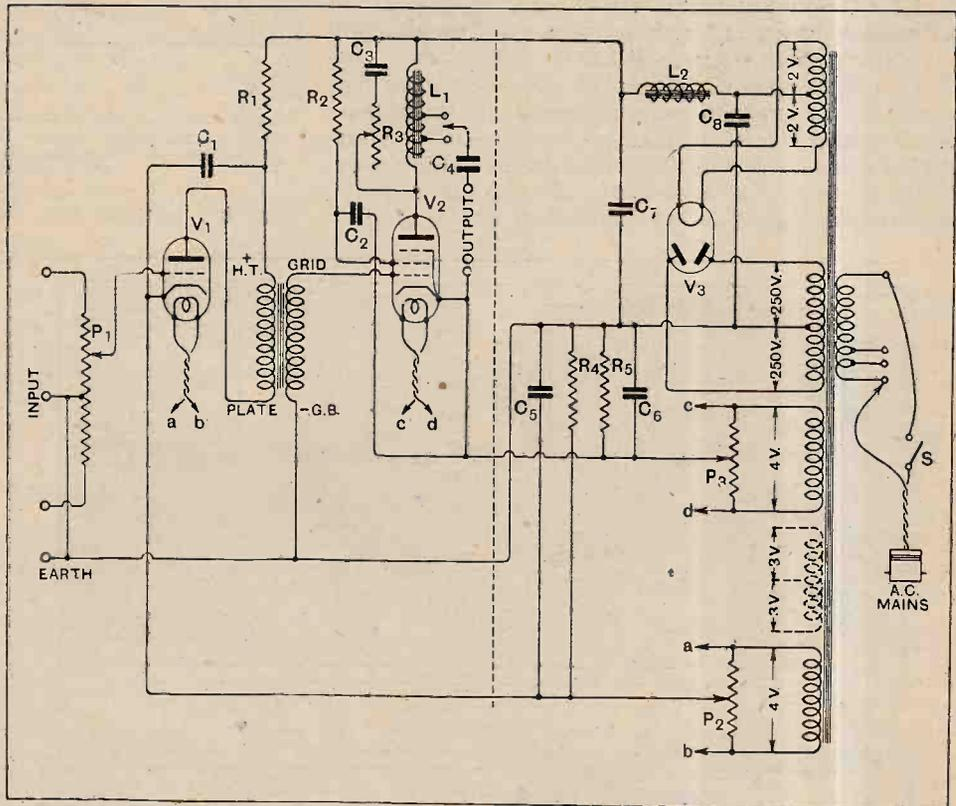
Fig. 1.—The theoretical circuit diagram. Values are as follows:  $P_1$ , 1 megohm;  $P_2$  and  $P_3$ , 50 ohms;  $R_1$ , 20,000 ohms;  $R_2$ , 10,000 ohms;  $R_3$ , 25,000 ohms;  $R_4$ , 750 ohms;  $R_5$ , 250 ohms;  $C_1$ ,  $C_2$ ,  $C_4$ ,  $C_5$ , and  $C_6$ , 2 mfd.;  $C_3$ , 0.01 mfd.;  $C_7$ , and  $C_8$ , 4 mfd.
