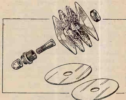
Tonax cone adaptor with felt fixing washers.
