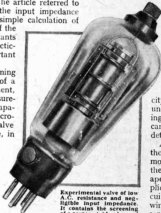
Experimental valve of low A.C. resistance and negligible input impedance. It contains the screening of a screen grid valve and a third earthed grid as used in a pentode.
