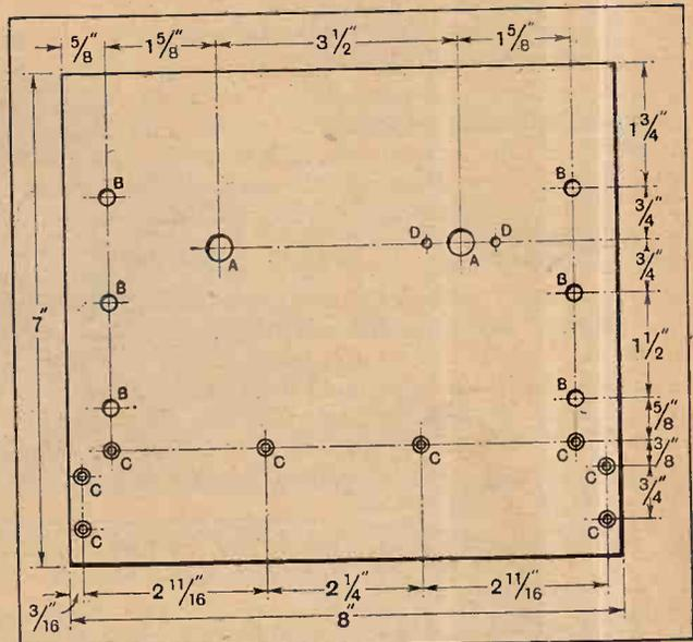
Fig. 3.—The panel layout. Drilling details are as follows: A, 1/2 in. dia.; B, 7/32 in. dia.; C, 1/8 in. dia., countersunk for No. 4 wood screws; D, 1/8 in. dia.
