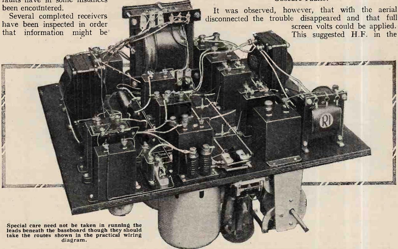
Special care need not be taken in running the leads beneath the baseboard though they should take the routes shown in the practical wiring diagram.
