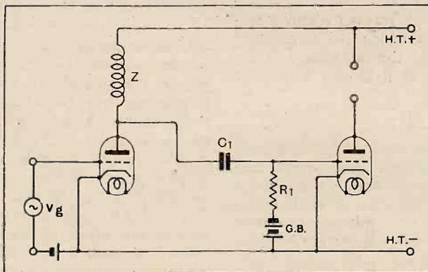
Fig. 1.—Connections for choke-capacity coupling.
