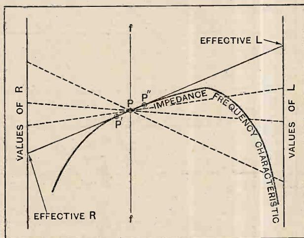
Fig. 7.—Alignment method of deriving effective values of  $L$  and  $R$  by means of the tangent to the impedance-frequency characteristic. The vertical line for frequency  $f$  is alone shown passing through  $P$ , the rest of the network being omitted.
