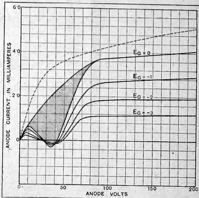
Fig. 4.—Typical curves of a modern A.C. screen-grid valve. The negative resistance or secondary emission area is shaded. The dotted curve gives the desirable  $E_g = 0$  characteristic for a low-impedance screened valve with a third grid. The increased grid swing minimises the risk of cross-modulation.
