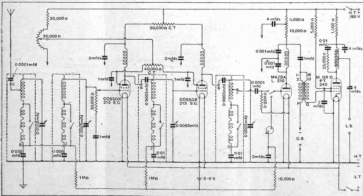
As far as possible the values given for the various components have been retained permitting of easy conversion for use with A.C. supply. The types of valves used are indicated.
