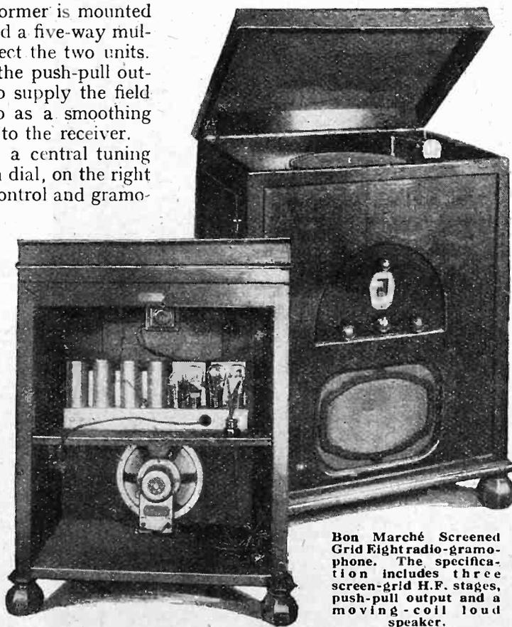
**Bon Marché Screened Grid Eight radio-gramophone.** The specification includes three screen-grid H.F. stages, push-pull output and a moving-coil loud speaker.
