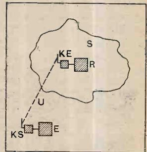
Fig. 2.—Schematic diagram of a field-strength amplifying equipment using ultra-short waves as a link. S=Urban area; E=Central receiving station; R=Relay transmitter; U=Ultra-short waves; KS=Ultra-short-wave transmitter; KE=Ultra-short-wave receiver
