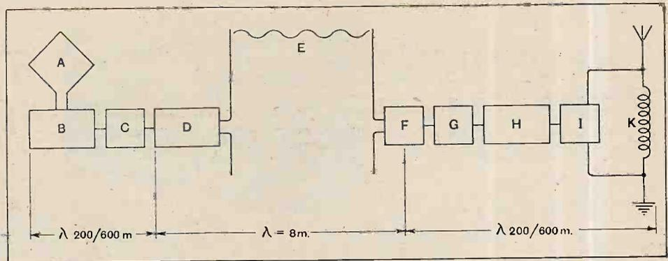
Fig. 3.—Schematic diagram of an aperiodic field-strength amplifying equipment. A—Aperiodic receiver; B—Band-filter; C—Aperiodic high-frequency amplifier; D—Ultra-short-wave transmitter; E—Ultra-short waves; F—Ultra-short-wave receiver; G—Preliminary amplifier; H—High-frequency power amplifier; I—Band-filter; K—Aerial circuit of relay transmitter.
