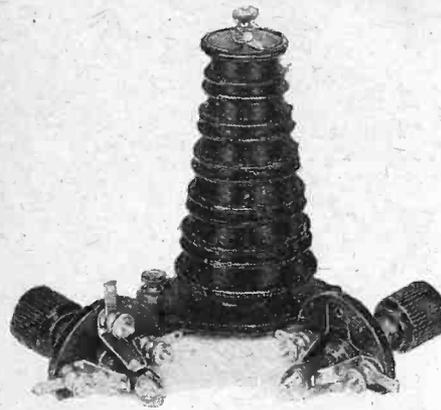
Tunewell H.F. choke, in which the sections are wound in alternate wide and narrow slots, and examples of new type push-pull switches. These components are made by Messrs. Turner and Co., Station Road, Old Southgate, London, N.11; the H.F. choke is priced at 6s. 6d., and the two- and three-point switches cost 1s. and 1s. 3d. respectively.
