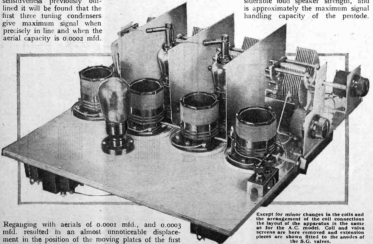
Reganging with aerials of 0.0001 mfd., and 0.0003 mfd. resulted in an almost unnoticeable displacement in the position of the moving plates of the first tuning condenser, being equivalent to less than half a division in the middle of the scale. Interchanging various detector valves resulted in a maximum displacement at the centre of the scale of 1½ divisions, so that
