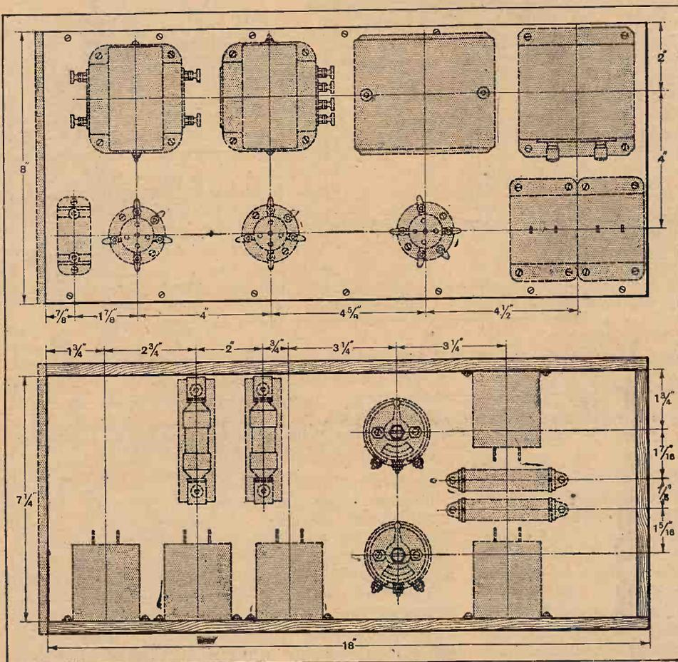
Fig. 4.—Layouts of the upper- and under-side of the baseboard.
