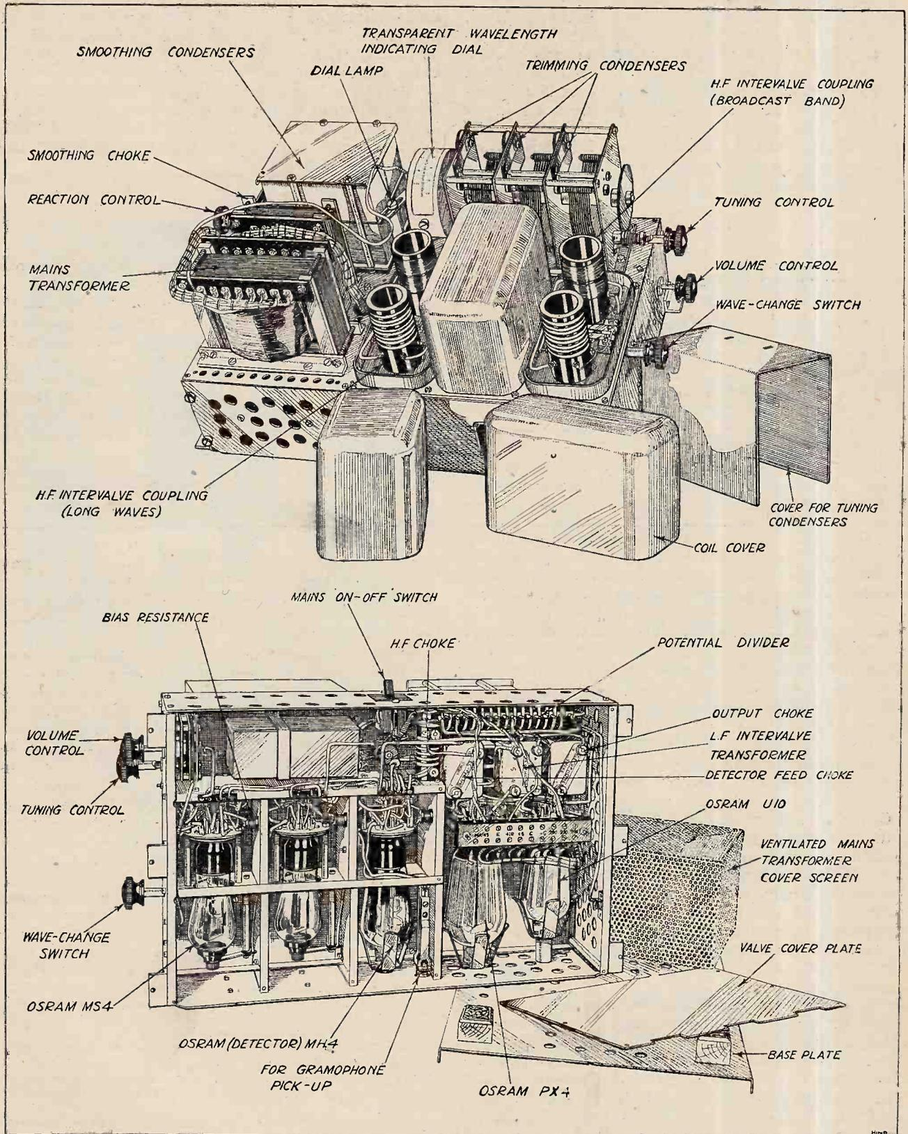
Chassis details of the Geophone All-electric Four-valve Receiver.
