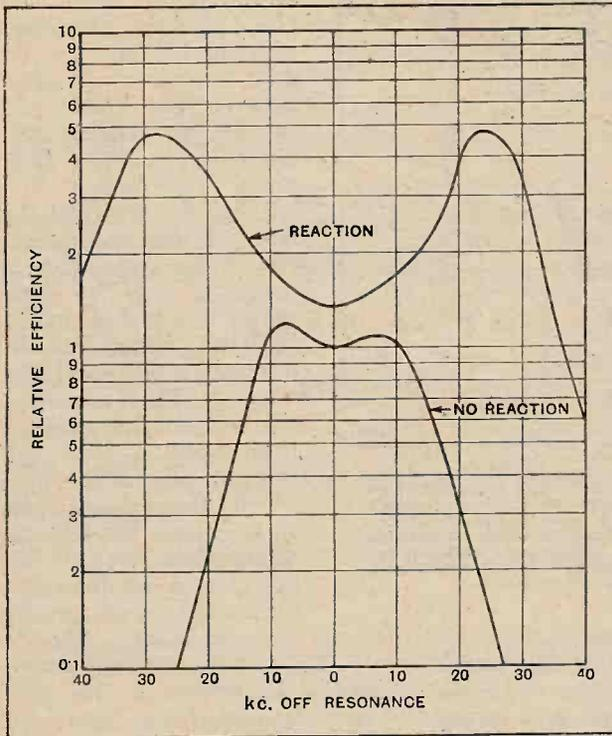
Fig. 2.—The effects of reaction upon a band-pass filter at 680 kc., 440 metres. The efficiency is only increased to a small extent, while the peak separation is considerably increased.
