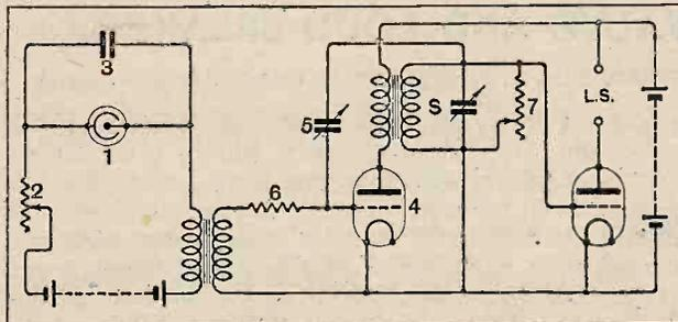
Fig. 1.—An experimental arrangement in which changes of frequency can be made in the Neon circuit and in the circuit marked S.
