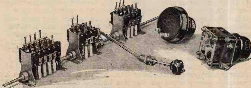
Groups of Magnum components including ganged switches, a differential condenser and wire-wound potentiometer.
