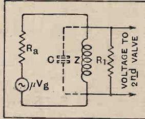
Fig. 4.—Equivalent A.C. circuit for choke-capacity intervalve coupling. The circuit is developed on the assumption that the reactance of the coupling condenser is sufficiently low to be neglected.
