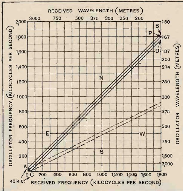
Fig. 1.—Relationship between received and oscillator frequencies for a superheterodyne using an intermediate frequency of 40 kc.
