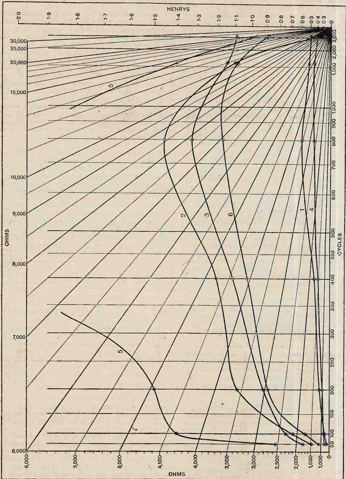
Fig. 8.—The impedance-frequency characteristics of six loud speaker units are plotted on the alignment diagram of Fig. 3. The effective values of resistance and inductance are obtained by means of the tangents to these curves at the different frequencies.
