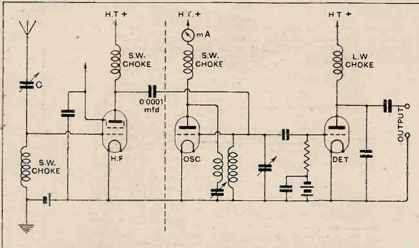
Fig. 2.—An aperiodic H.F. stage for the "Superheterodyne Short-wave Adaptor." Extra apparatus is shown on the left-hand side of the dotted line.
