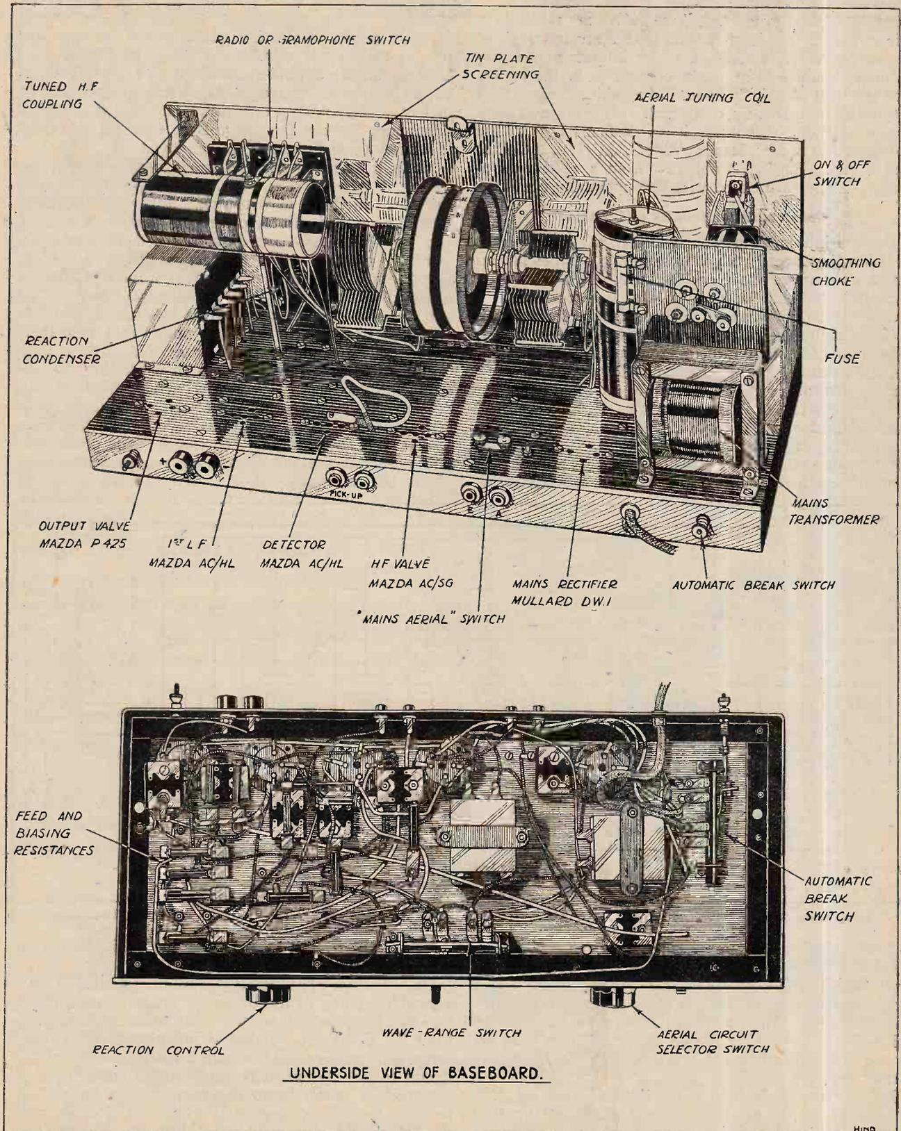
WATES ALL-ELECTRIC FOUR.—Back and underside views of the chassis.
