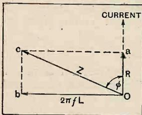
Fig. 2.—Voltage vectors for an inductive coil when the current is 1 ampere.
