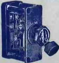
The provision of Silver Contacts in these Switches is designed to overcome all troubles due to oxidation, etc. Contacts are mounted on Bakelite base and provision is also made for connections by terminals or soldering lugs. Lever operated. One-hole fixing. Nickel plate finish. Dimensions, 2-pole type, 1 1/2" deep x 2" x 1".
