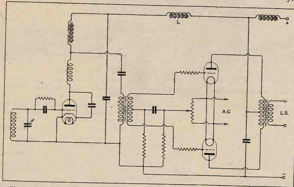
Fig. 3.—An economical and satisfactory choke-transformer coupled circuit. The H.T. supply needs no decoupling, and a proportional smoothing circuit can be used.
