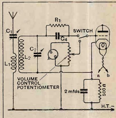
Fig. 1.—Gramophone pick-up attachment for the "Power Pentode Two."
