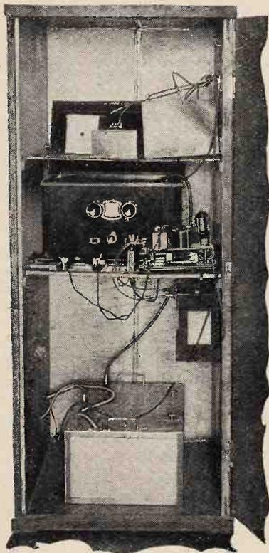
Fig. 4.—Arrangement of the central receiving station (experimental model). In the screened cupboard; short-wave band filter, broadcast receiver, and (below) high-frequency power amplifier.
