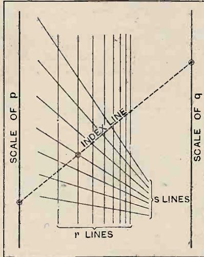
Fig. 2.—Scheme of four-variable alignment chart. A single application of the index line relates the values of  $p$  and  $q$  with those of  $r$  and  $s$ .
