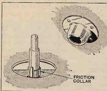
Friction collar on the turntable spindle of the B.T.H. motor.
