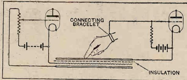
Fig. 3.—Volume control by the resistance of the human body.
