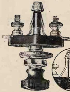
**A**N inefficient switch robs your valves of their power and soon produces "crackling." The new W.B. Switch ensures perfect contact. Its plunger terminates in double cones between which the powerful spring contacts are firmly gripped when in the "on" position. One hole fixing. Takes any size panel, from which it is completely insulated. Self-cleaning nickel-ilver contacts. Screw terminals and soldering tags for easy fixing. Price 1/3
