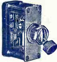
The provision of Silver Contacts in these Switches is designed to overcome all troubles due to oxidation, etc. Contacts are mounted on Bakelite base and provision is also made for connections by terminals or soldering lugs. Lever operated. One-hole fixing. Nickel plate finish. Dimensions, 2-pole type, 1 1/2" deep x 2" x 1/2".
