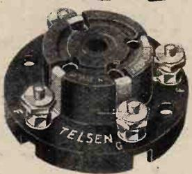
**TELSAN VALVE HOLDERS.** Pro. Pat. No. 20286/30. An entirely new design in Valve Holders, embodying patent metal spring contacts, which are designed to provide the most efficient contact with the valve legs. Low-capacity, self-locating, supplied with patent soldering tags, and hexagon terminal nuts. Fitted with nickel-silver shock-absorbing spring contacts. Price 1/- each.
