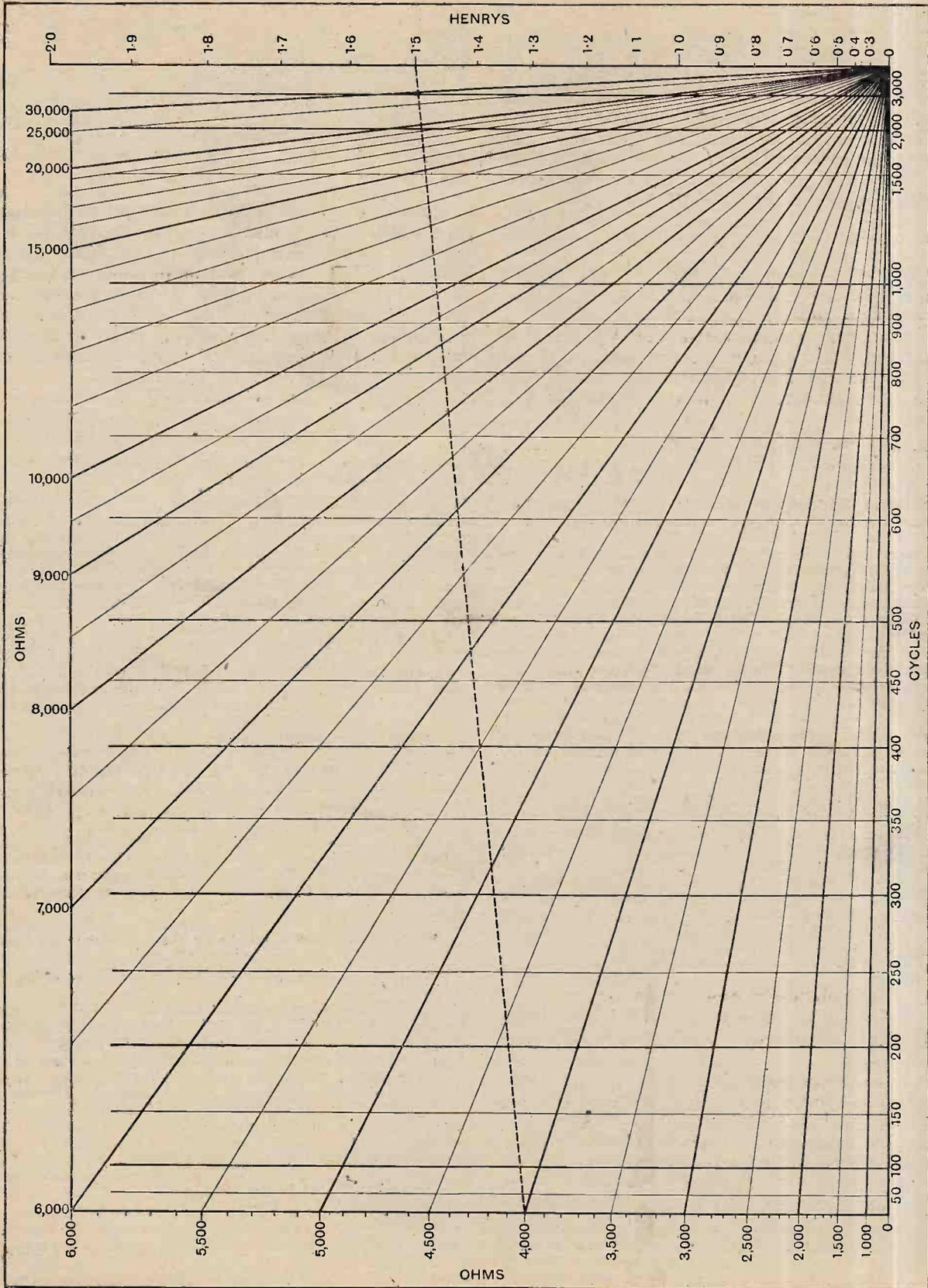
Fig. 3.—Four-variable alignment chart for impedance of an inductance in series with a resistance. The index line shows the case when  $L = 1.5$  henrys,  $R = 4,000$  ohms. At 400 cycles, the impedance is approximately 5,500 ohms.
