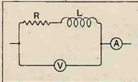
Fig. 4.—Method of obtaining impedance of loud speaker  $RL$  by taking simultaneous readings of valve voltmeter  $V$  and thermo-junction  $A$ .
