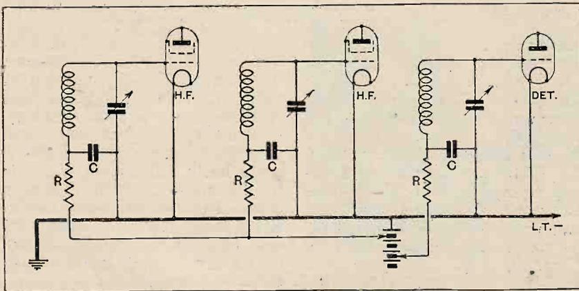
Fig. 1.—Grid bias system for 2 H.F. stages followed by an anode bend detector. The condenser rotors may be earthed, and the first by-pass condenser (C) may be the coupling condenser of a filter. Decoupling resistances are marked R.
