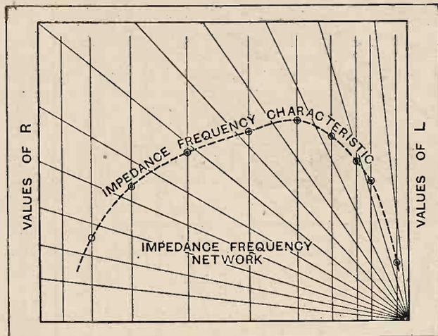
Fig. 6.—The experimental impedance-frequency characteristic of a loud speaker when plotted on the network of the alignment diagram is a curve, indicating that  $L$  and  $R$  can no longer be regarded as constants. Like Fig. 5, this diagram is schematic only.
