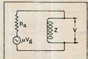
Fig. 3.—Equivalent A.C. circuit for a valve with impedance  $Z$  connected in the anode circuit.
