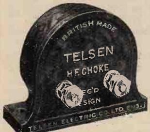
**TELSAN H.F. CHOKES.** Designed to cover the whole wave-band range from 18 to 4,000 metres, extremely low self-capacity, shrouded in genuine Bakelite. Inductance 150,000 micro-henries. Resistance 400 ohms. Price 2/6 each.
