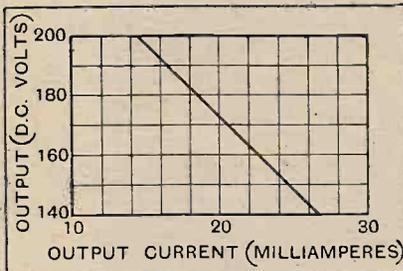
Fig. 1.—An eliminator regulation curve, showing relationship between output voltage and output current.
