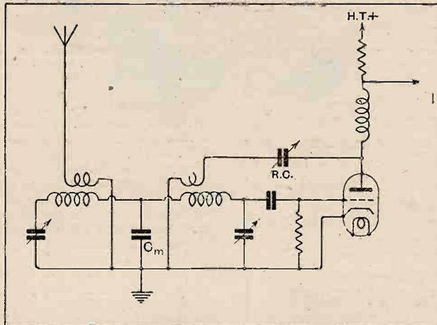
Fig. 1.—A simple capacity-coupled filter in which the tuning coils can consist of 80 turns of No. 26 D.C.C. close wound on a 2in. diameter former. The aerial and the reaction windings can be identical, and consist of 15 turns of No. 36 D.S.C. wound at the earthed end of the main winding. A suitable value of the coupling condenser  $C_m$  is 0.01 mfd., while the reaction condenser should have a capacity of about 0.0003 mfd. and the tuning condensers 0.0005 mfd.
