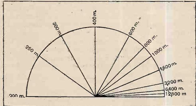
Fig. 4.—How the wavelengths fall on the oscillator tuning dial of a superheterodyne receiver of the "Infradyne" type. The whole tuning range is covered on a single swing of the condenser and the tuning is true "kilocycle tuning." At all points two stations removed by 9 kc. in frequency are separated by a shade over one degree on the dial.
