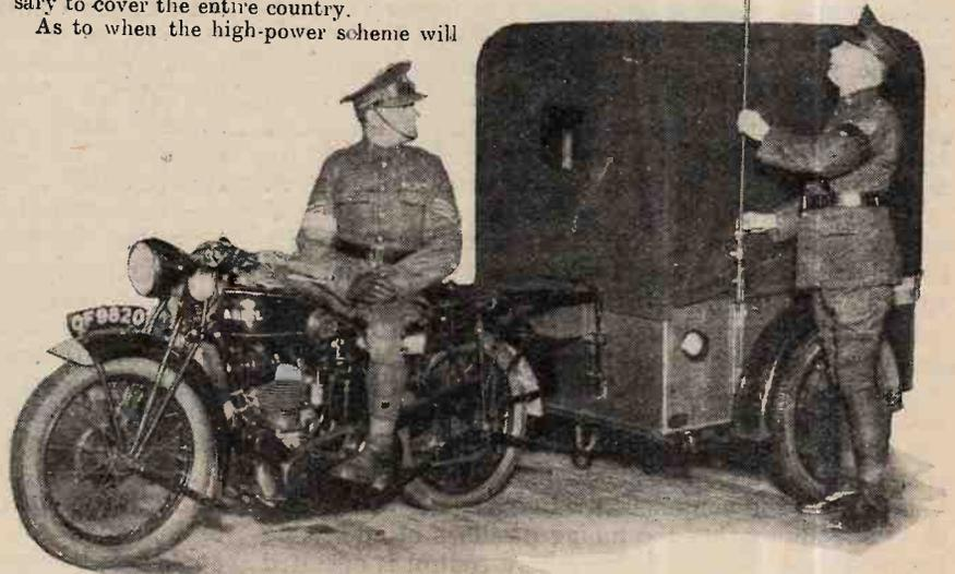
**MOTOR CYCLE WIRELESS UNITS.** The 47th (2nd London) Divisional Signals (Territorials) have equipped the first radio transmitting and receiving unit for use with a motor cycle. The trailer, seen in the photograph, carries a crew of two together with a complete radio installation. Messages have been accurately exchanged at distances up to three miles.
