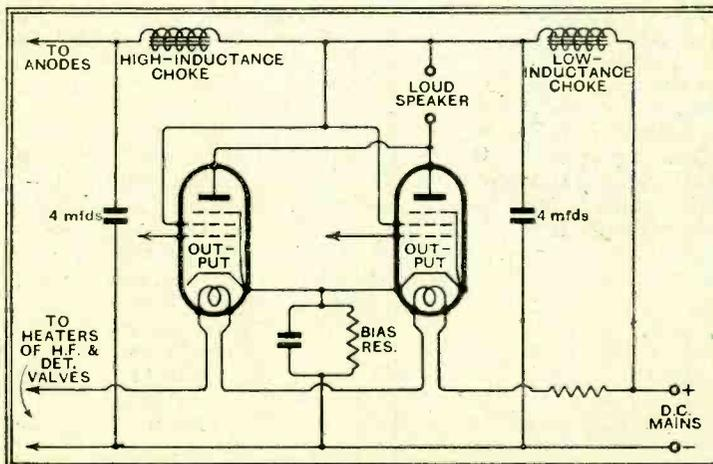
Fig. 2.—Progressive smoothing, as applied to a D.C. set with parallel output pentodes.
