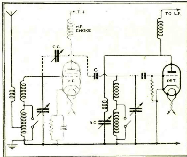
Fig. 2.—Eliminating an H.F. stage without sacrifice of selectivity.
