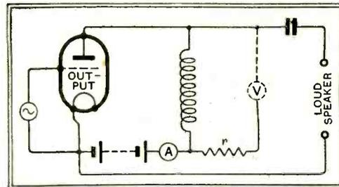
Fig. 4.—Typical output circuit including A, a milliammeter reading anode feed current, and V, a voltmeter in series with  $r$ , which is a measure of the anode feed current fluctuation. Distortion caused by anode rectification is not so unpleasant as that caused by grid current.
