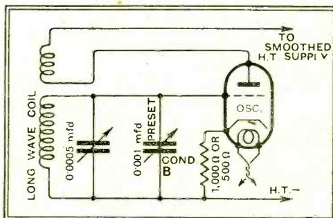
Fig. 1.—A simple oscillator for ganging which can be built from spare parts.
