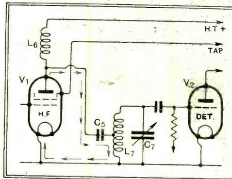
Fig. 25.—A portion of the circuit of the receiver of Fig. 9, the path of the signals round the anode circuit of  $V_1$  being marked out by arrows.
