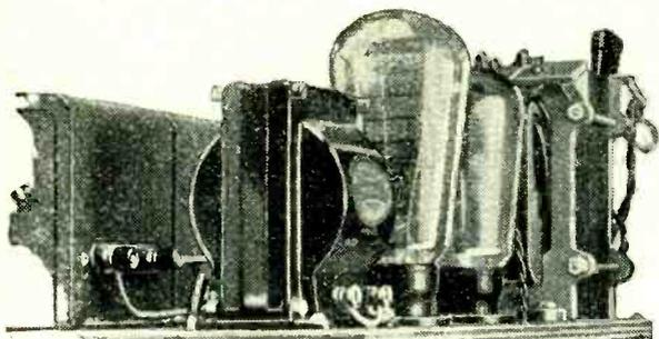
Mains supply and output stage of "The Modern Straight Five" receiver giving 5 watts speech energy.
