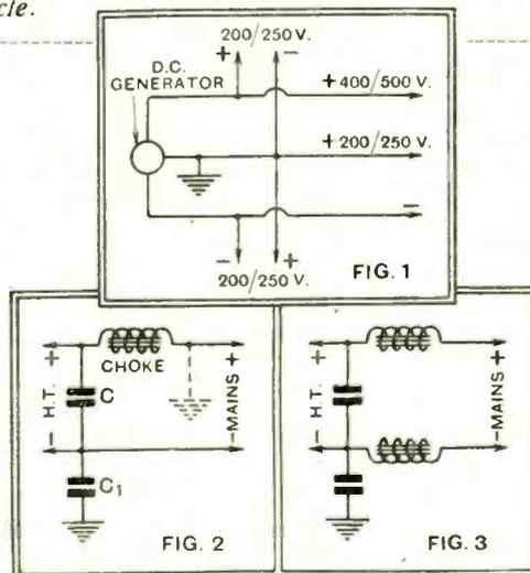
Fig. 1.—The three-phase system of D.C. mains supply, illustrating how the positive and negative earths occur. Fig. 2.—When the positive mains lead is earthed, the choke is effectively short-circuited by C and C<sub>1</sub> in series. Fig. 3.—It is usually advisable to include a choke in each mains lead, for the set is then not so greatly affected by the mains being earthed.
