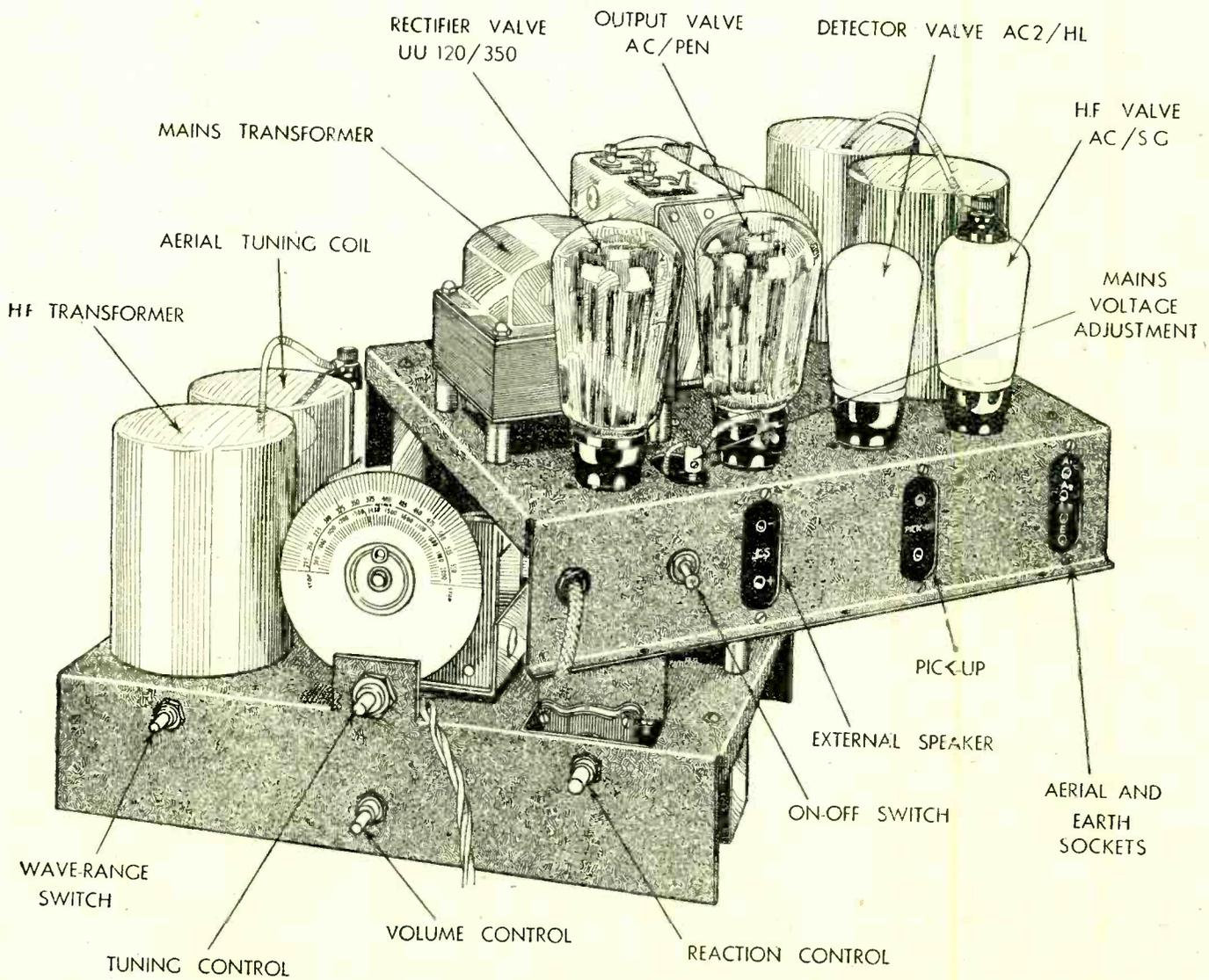
Circuit diagram and two views showing constructional details of the chassis in the Dominion S.G.P.3. mains receiver.
