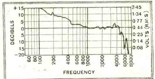
Open-circuit output characteristic of the British Radiophone type 351 pick-up with H.M.V. loud needle.
