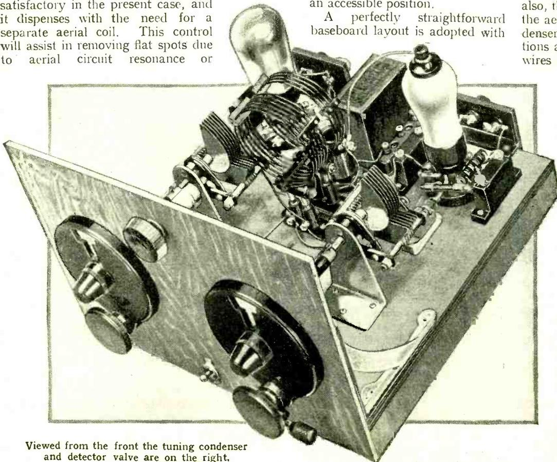
Viewed from the front the tuning condenser and detector valve are on the right.
