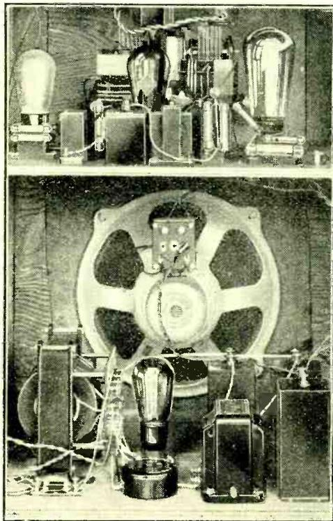
Showing the principal components of *The Wireless World* "Power Radio-Gram," the output stage of which is capable of a high volume level giving realistic reproduction.
