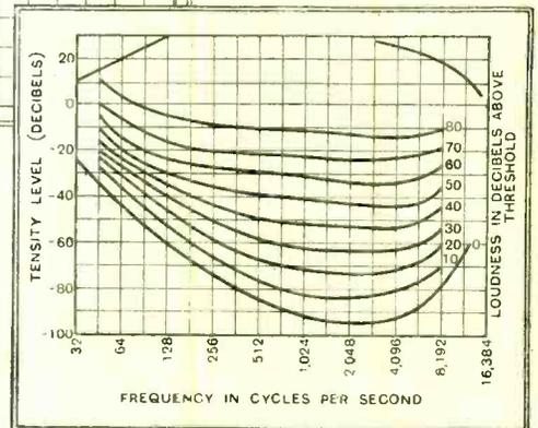
Fig. 2.—(Left) Diagram showing curves where the loudness is the same at all frequencies. (Right) Curves showing that the loudness in the lower register increases much more quickly than that in the upper register for equal increments above the threshold of audibility.
