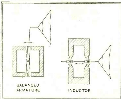
The inductor principle permits the development of larger amplitudes than the balanced armature, but is not always so sensitive.
