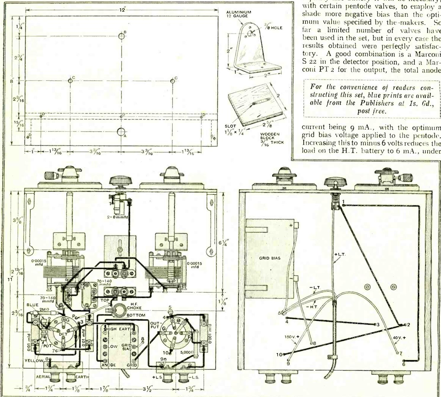
Layout of the components and the practical wiring plan, also dimensional details of condenser brackets and grid coil holder mounting. Panel drilling: A =  $\frac{1}{16}$  in. dia.; B =  $\frac{3}{8}$  in. dia.; C =  $\frac{1}{4}$  in. dia.; D =  $\frac{1}{8}$  in. dia.
