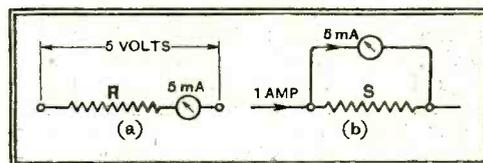
Fig. 2.—Use of a milliammeter as voltmeter (a), or ammeter (b). The values of  $R$  and  $S$  are found by the aid of Ohm's law.
