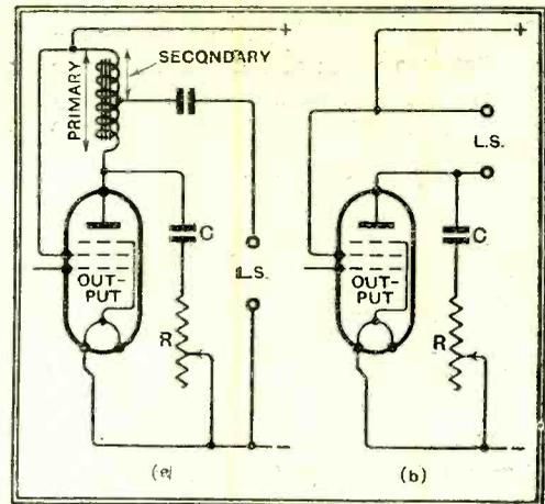
Fig. 3.—Pentode output circuits. (a) A centre-tapped choke will do duty as a 2 : 1 step-down transformer. R is here shown variable to act as tone-control. (b) For speakers containing a transformer tapped for pentode this is connected to the L.S. terminals shown. CR may or may not still be needed.
