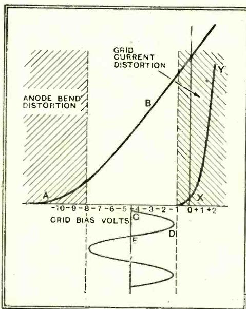
Fig. 1.—When a signal, CDE, is applied to a valve with a characteristic such as AB, the peaks must not enter the shaded danger zones of anode bend detection or grid current. A grid bias voltage of 4½ is seen to be necessary.
