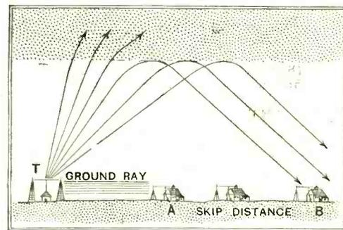
Fig. 7.—Showing how the skip distance occurs on short waves.
