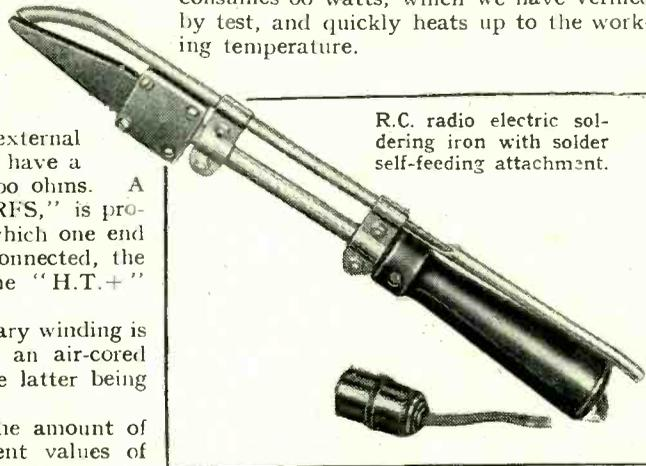
R.C. radio electric soldering iron with solder self-feeding attachment.
