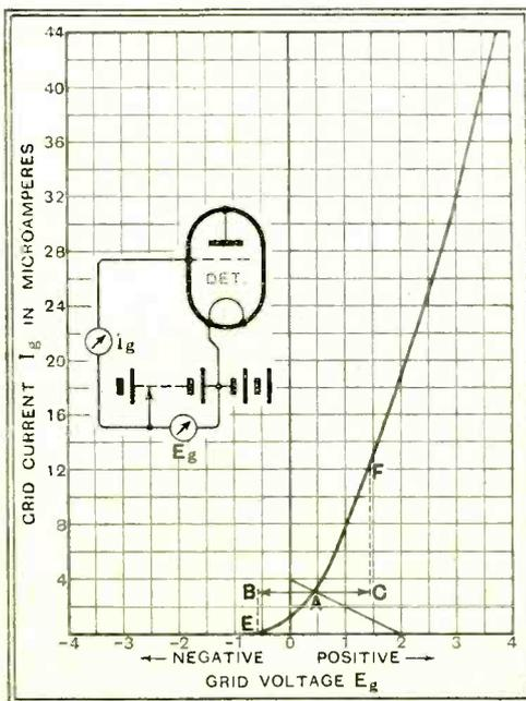
Fig. 26.—Curve showing the amount of grid current  $I_g$  flowing for different values of grid voltage  $E_g$ . (Inset) A suitable circuit for measuring grid current for different values of grid voltage.
