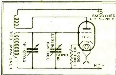
Fig. 1.—A simple oscillator for ganging which can be built from spare parts.
