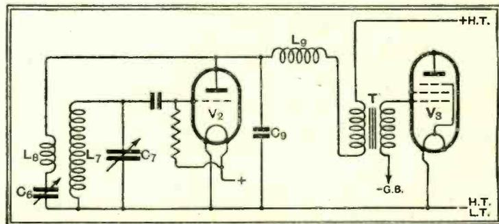
Fig. 32.—Showing an alternative method of connecting the transformer. The steady anode current of  $V_2$  now passes through the primary, and this may be injurious to the fidelity of reproduction.
