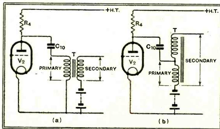
Fig. 35.—(a) Normal connection of transformer, in which primary and secondary are separate. (b) Auto-transformer connection, as used in the set, in which both windings form the secondary. The ratio is higher by one than in (a), using the same transformer.
