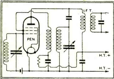
Fig. 2.—The connections of the self-neutralised pentode single-valve frequency changer used in *The Wireless World Baby Superhets*.
