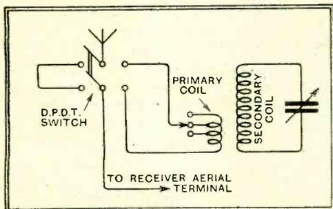
Fig. 1.—An aid to station identification: switching connections for inserting a wavemeter in series with the aerial.
