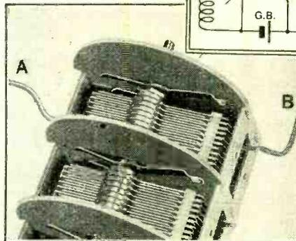
valve on one side of the condenser and the coil on the other, and it is a good plan in such cases to make use of both connection points in the manner suggested in Fig. 1, where the wires in question, which bear corresponding lettering, are shown both diagrammatically and pictorially.
