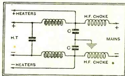
Fig. 5.—The inclusion of H.F. chokes in the mains leads removes whistles from a superheterodyne, and in some cases the connection of the local earth between condensers C gives increased efficiency.
