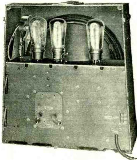
The tuning and reaction controls are located at the back of the receiver and can be seen on the left. The visual scale is at the front.
