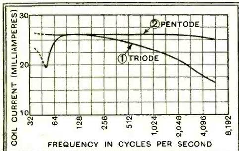
Fig. 3.—Curves showing variation in coil current when a loud speaker is used with one LS5A valve or one pentode. It is clear that there is no appreciable current variation with the pentode, which proves that the coil impedance is relatively negligible.
