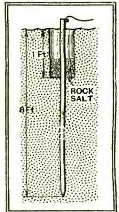
Fig. 2.—A special form of earth connection for which low resistance is claimed.
