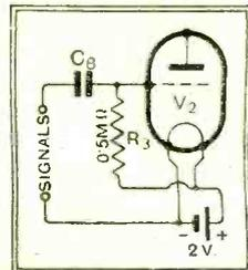
Fig. 27.—The essential circuit of the detector valve as used in the set:  $C_8 = 0.0001$  mfd.;  $R_3 = \frac{1}{2}$  megohm. Note that the bottom end of  $R_3$  is taken to L.T.+, making it 2 volts positive.
