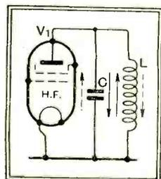
Fig. 23.—To nullify the stray capacities  $C$  which prevent Fig. 22 from giving high gain, an inductance  $L$  is added. The current through this must exactly neutralise that through  $C$ .
