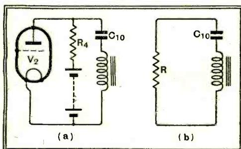
Fig. 33.—(a) The presence of  $V_2$  and  $R_4$ , in parallel, in series with  $C_{10}$  and the primary of the transformer prevent the low-frequency tuned circuit from resonating sharply; (b) shows the effective circuit,  $R_4$  and the valve resistance being amalgamated to give  $R$ .
