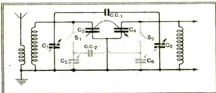
Fig. 1.—For twin station reception: the filter is tuned to the shorter wavelength by compression condensers  $C_1$  and  $C_2$ . A change-over to an alternative programme is effected by linked switches  $S_1$  and  $S_2$ .
