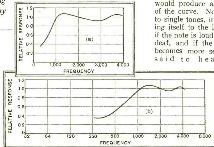
Fig. 1.—Response curves of the same loud speaker on (a) a linear frequency scale and (b) an octave or logarithmic frequency base. Curve (b) reveals that important information regarding the lower half of the musical scale is absent from curve (a).
