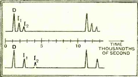
Fig. 8.—Reception of short-wave signals for measurement of layer heights.
