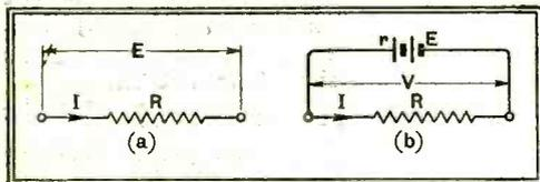
Fig. 1.—For the resistance at (a) the current is given by  $I = E/R$  amperes, whereas for the closed circuit (b) it is given by  $I = E/(R+r)$  amps., where  $r$  is the battery resistance, or by  $I = V/R$ .
