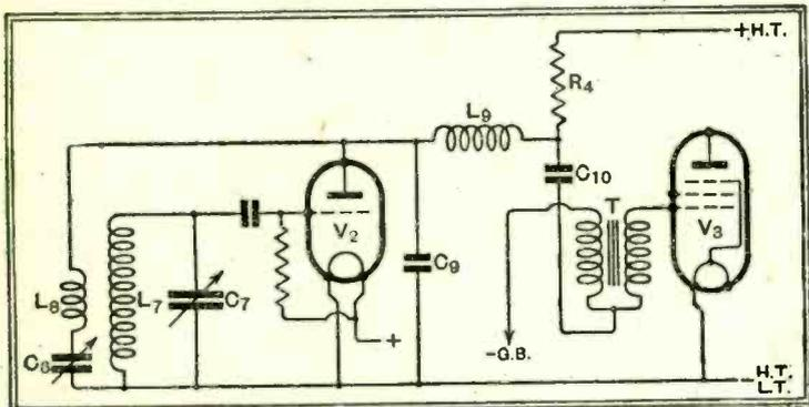
Fig. 31.—Portion of the complete receiver, showing components included in, and therefore affected by, the anode circuit of the detector  $V_2$ .
