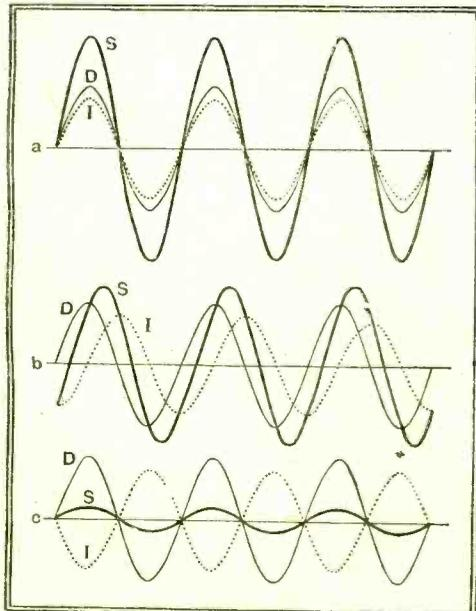
Fig. 4.—How fading occurs. The combination of two waves of nearly equal amplitude but with different phases.
