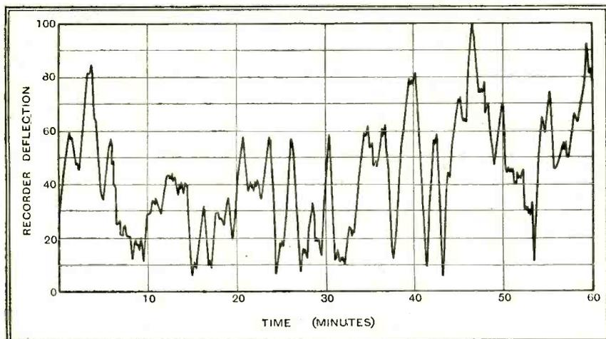
Fig. 6.—Fading-record of a German station received in London.
