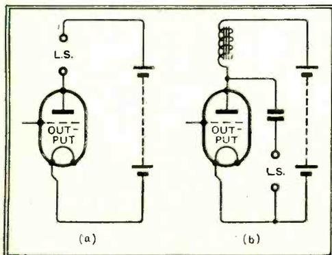
Fig. 1.—For Triodes only.—In both these circuits the loud speaker is effectively connected directly in the anode circuit. (a) Is suitable for battery receivers, but (b) is safer in mains sets since speech-currents go direct to filament or cathode.
