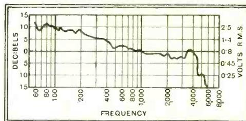
Characteristic of pick-up fitted to the Garrard record changer; measured with 100,000 ohm shunt and H.M.V. loud tone needle.
