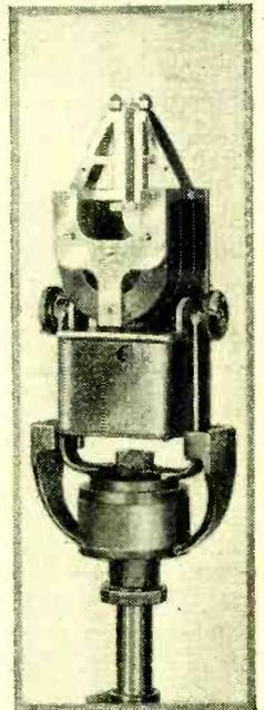
R.C.A. electromagnetic ribbon microphone which gives a response proportional to the air particle velocity.
