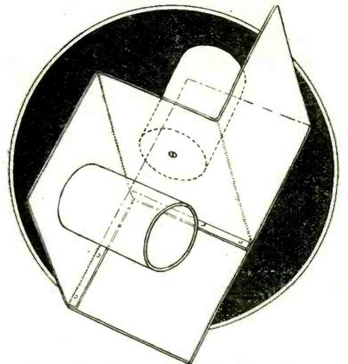
If corresponding points of each coil are equally spaced from the screens, inductance matching will be unaffected.
