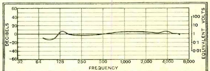
Fig. 3.—By crowding the units of the vertical scale and omitting the extreme ends, the decibel curve of Fig. 2 (b) can be made to appear substantially flat.
