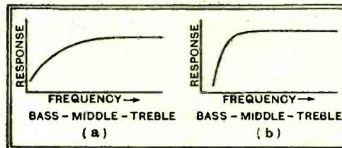
Fig. 34.—Type of response curves to be expected of transformers (a) without, and (b) with, series condenser  $C_{10}$ . A properly chosen condenser keeps the bass response up as far as a certain frequency, below which it tails off very rapidly.
