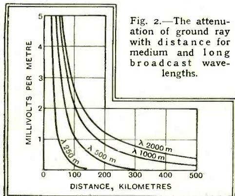
Fig. 2.—The attenuation of ground ray with distance for medium and long broadcast wavelengths.
