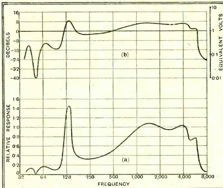
Fig. 2.—Curves of the same loud speaker plotted (a) in terms of relative response and (b) on a decibel scale. Note that on the decibel scale the unimportant dip at about 50 cycles in the region of low output is exaggerated, while the peak at 130 cycles is minimised.
