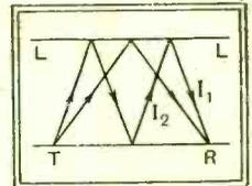
Fig. 5.—It is possible that two indirect rays may be received at R.
