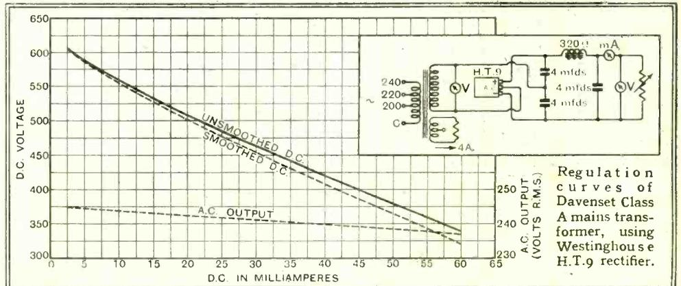
curves here reproduced show the rectified output before and after smoothing; in the one case correction has been made for the voltage dropped across the 320-ohm choke. From this the voltage available after smoothing can be calculated where chokes of different resistance are employed.
