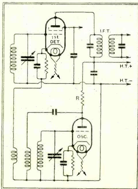
Fig. 1.—The circuit of a typical modern frequency changer showing the oscillator and first detector with mains-type valves.
