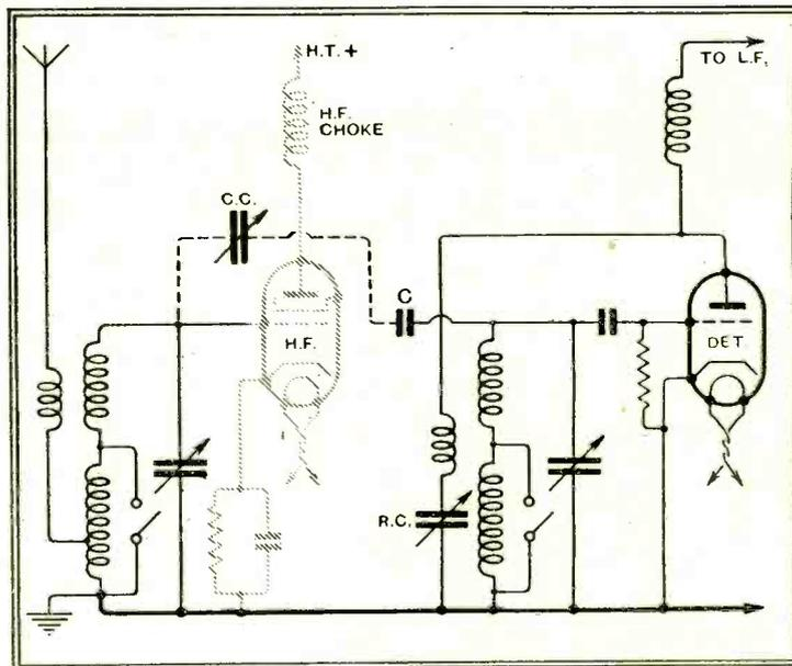
Fig. 2.—Eliminating an H.F. stage without sacrifice of selectivity.
