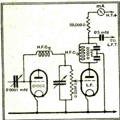
Fig. 1.—Visual indication of the behaviour of both tuning system and detector; a milliammeter added to the "Diode Quality Four."
