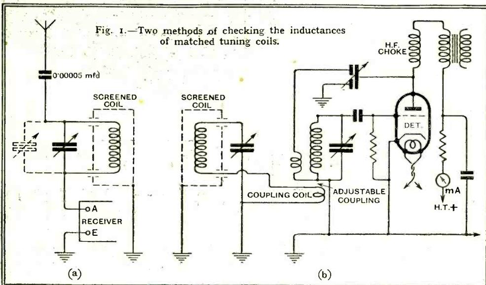
Fig. 1.—Two methods of checking the inductances of matched tuning coils.
