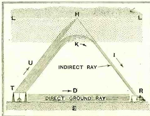
Fig. 1.—Showing the direct and indirect paths taken by the rays from a transmitter.
