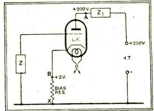
Fig. 2.—Typical distribution of voltage in the anode-cathode circuit of a valve with self-bias. The grid is connected to a point more negative than the cathode, and thus the bias voltage is of correct polarity.
