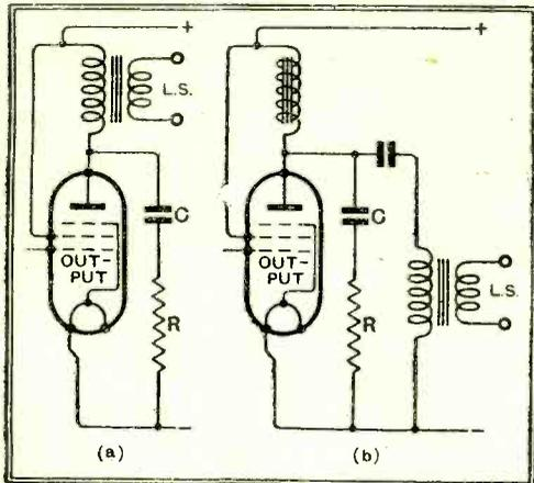
Fig. 2.—Pentode output circuits using step-down transformers, of ratio about 2½ to 1 for average speakers. C may be 0.002 to 0.01 mfd., and R, 10,000 to 50,000 ohms. Circuit (b) provides against motor-boating, and relieves the transformer primary of steady current.
