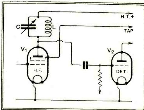
Fig. 24.—The practical form of Fig. 23 as it would be developed for use in a set. This is the tuned anode circuit.
