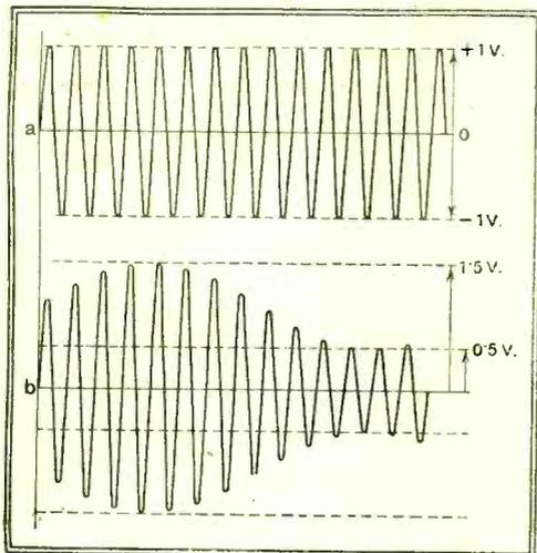
Fig. 28.—An unmodulated carrier of peak amplitude 1 volt is shown at (a) while (b) represents the same carrier modulated. The amplitude now varies from 0.5 to 1.5 volts at the frequency of the note being transmitted.
