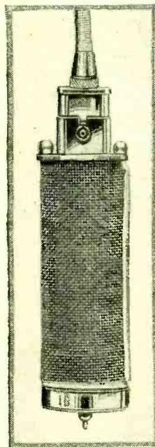
The Edison Bell (Voigt) electrostatic microphone gives an output proportional to sound pressure, is non-directional and does not introduce any appreciable obstacle effect when suspended in the sound field.
