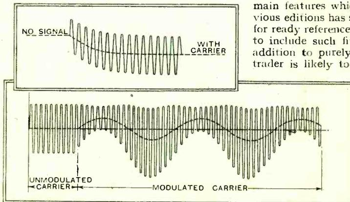
Fig. 30.—The actual grid voltage is shown in the upper diagram as a full line and the average grid voltage is given by a dotted line. In the lower diagram the grid voltage averaged over a long period (D.C. voltage) is given by the horizontal straight line. The average grid voltage is given by the wavy line.
