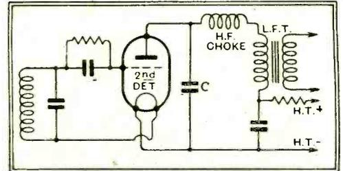
Fig. 3.—Anti-phase feed-back in the second detector is likely to be greater in a superheterodyne than in a straight set on account of the higher reactance of the by-pass condenser C.
