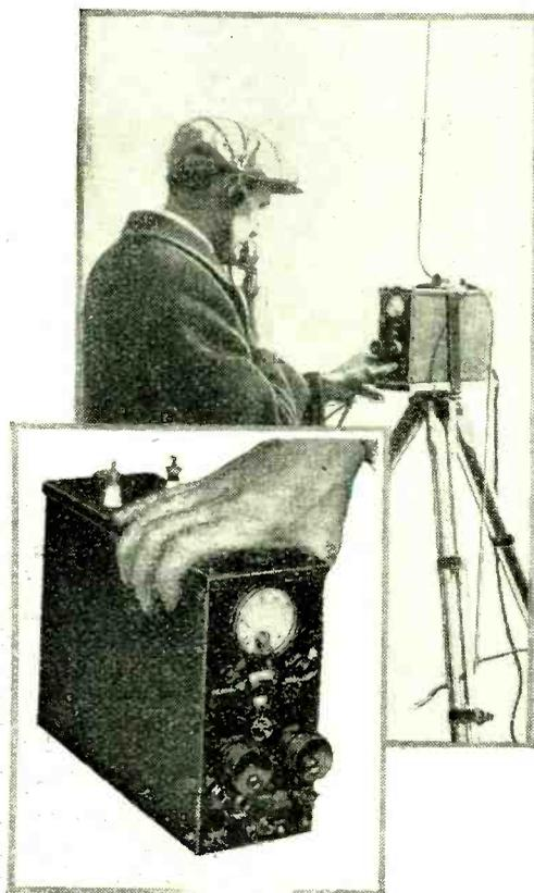
**A 5-METRE PORTABLE.** The new R.C.A.-Victor "Tranceiver," on which telephony can be transmitted or received on ultra-short waves at a moment's notice. Note the camera tripod. The weight of the instrument, including batteries, is only 22 lbs.
