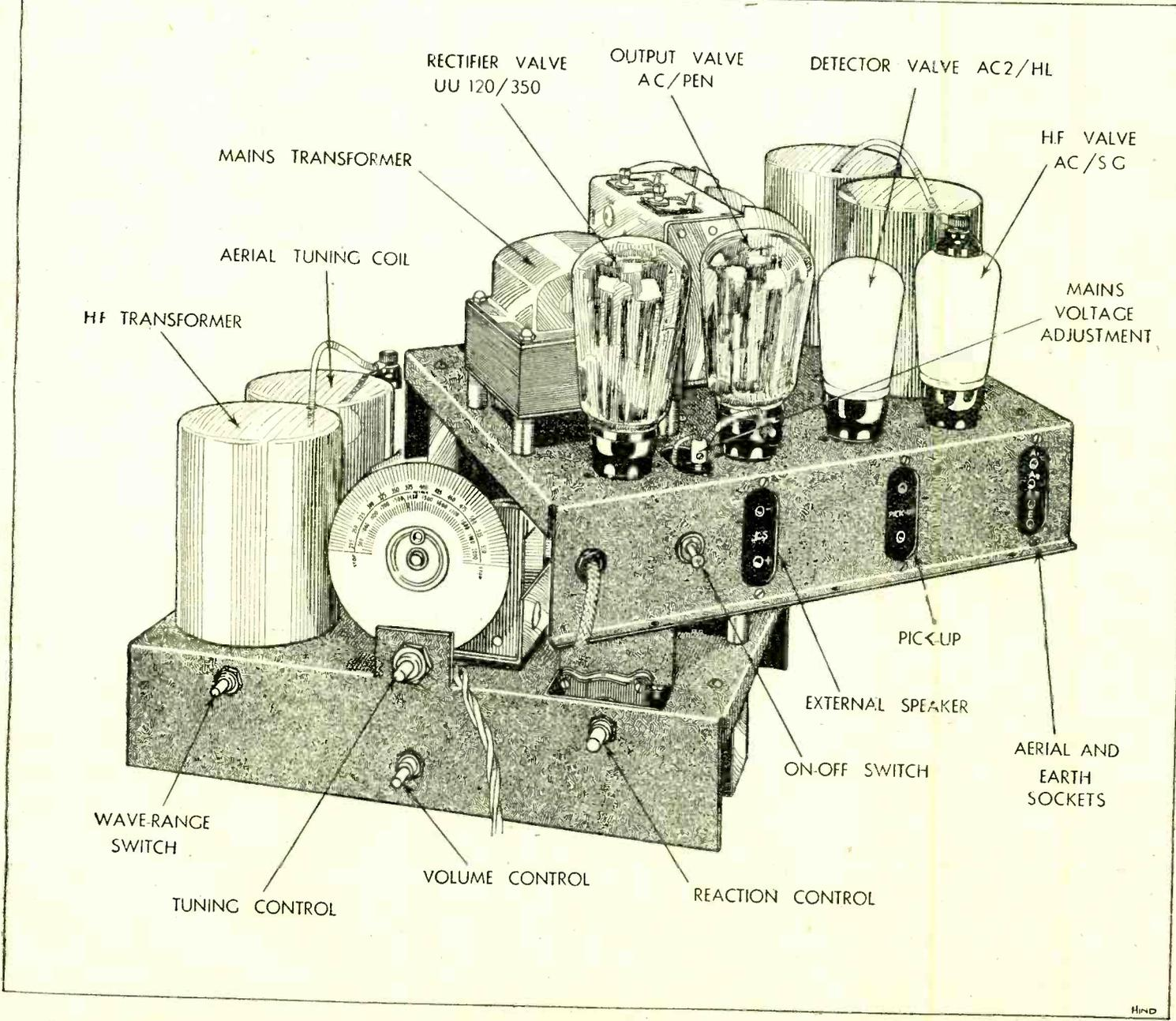
Circuit diagram and two views showing constructional details of the chassis in the Dominion S.G.P.3. mains receiver.
