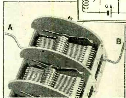
valve on one side of the condenser and the coil on the other, and it is a good plan in such cases to make use of both connection points in the manner suggested in Fig. 1, where the wires in question, which bear corresponding lettering, are shown both diagrammatically and pictorially.
