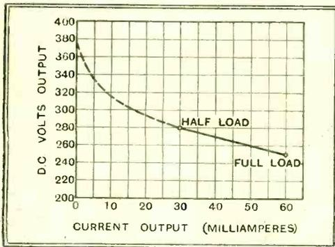
Fig. 1.—Regulation curve of a rectifying valve, prepared from the Valve Data Supplement.
