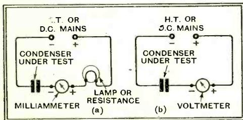
Fig. 1.—Practically any type of meter can be used in testing fixed condensers, but the precaution of inserting a limiting resistance, as in diagram (a) should be observed if there is any risk of exceeding the current rating of the testing instrument.
