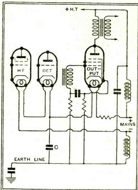
Fig. 4.—This skeleton circuit of a three-valve set illustrates the method of obtaining negative smoothing with an ordinary choke when indirectly heated valves are used.
