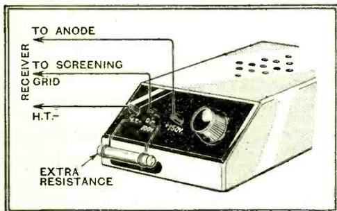
Fig. 1.—Screening grid voltage fluctuations may be reduced by adding an external resistance to an eliminator.
