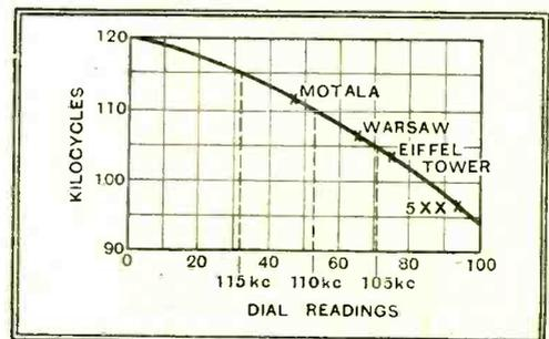
Fig. 2.—The calibration curve of the experimental oscillator.
