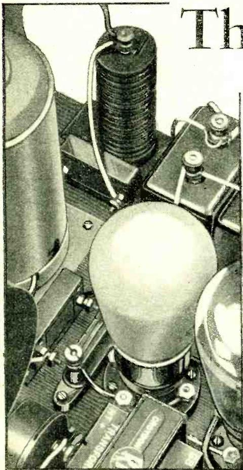
A typical modern detector stage, showing a metallised HL2 type valve.
