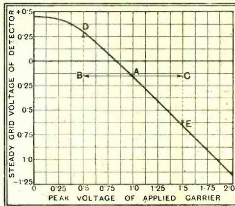
Fig. 29.—Curve showing final steady voltage taken by grid of detector when carrier oscillations of different amplitudes are applied to it.
