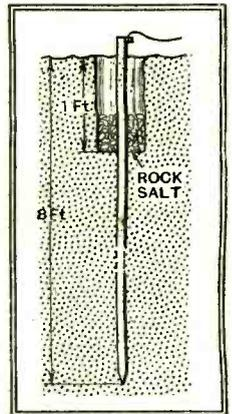
Fig. 2.—A special form of earth connection for which low resistance is claimed.
