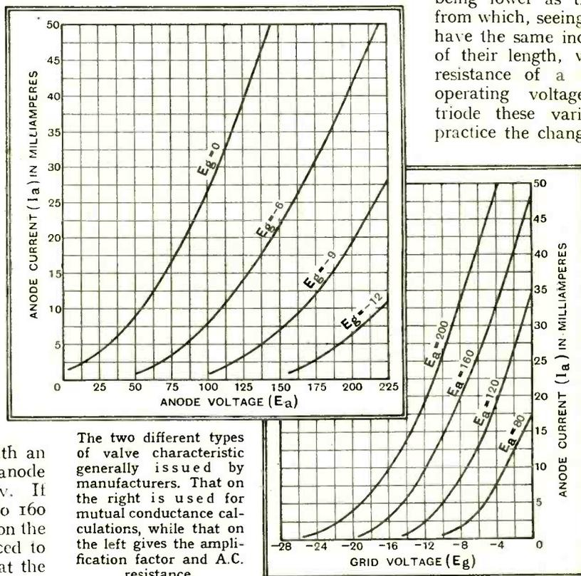
The two different types of valve characteristic generally issued by manufacturers. That on the right is used for mutual conductance calculations, while that on the left gives the amplification factor and A.C. resistance.
