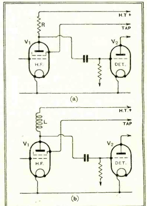
Fig. 22.—Resistance-coupled and choke-coupled H.F. stages, which at first sight appear to fulfil all the conditions necessary for high gain.
