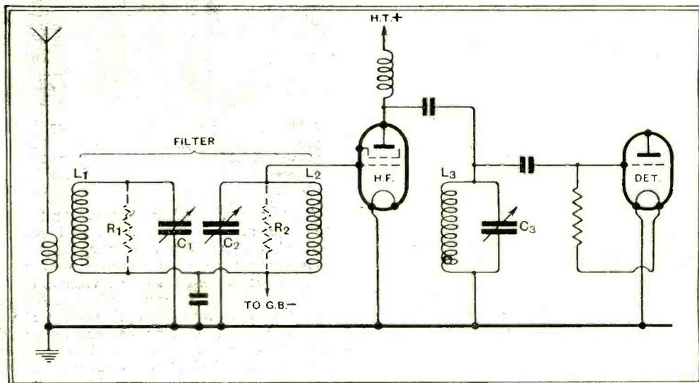
Fig. 2.—Adjusting a single-knob tuning system: to ensure that the circuit  $C_3, L_3$  is accurately tuned to an incoming signal, the efficiency of the remaining tuned circuits may be temporarily reduced by adding parallel resistances of 5,000 ohms, or even less.
