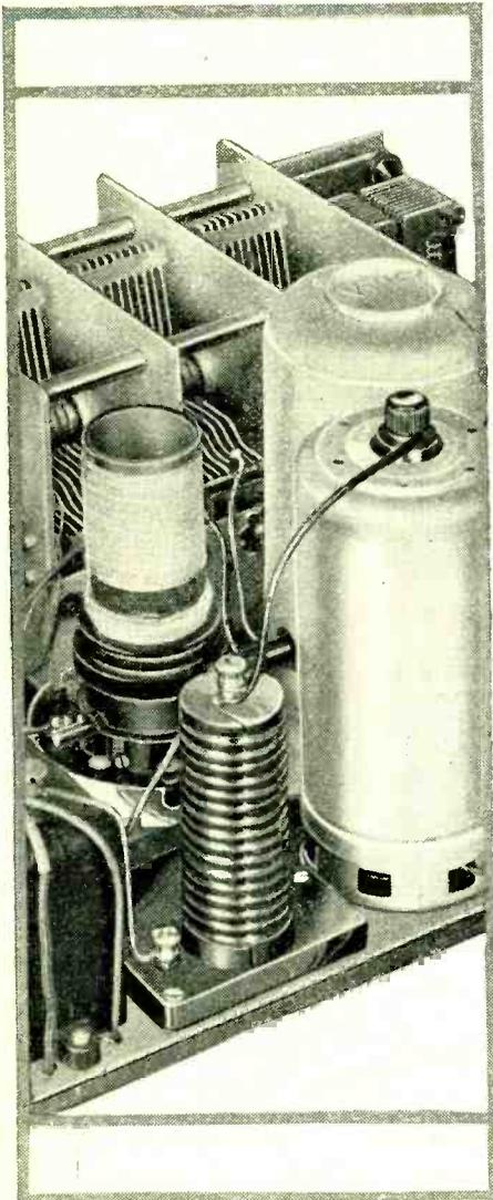
The principal components of an H.F. stage in a typical ganged receiver.
