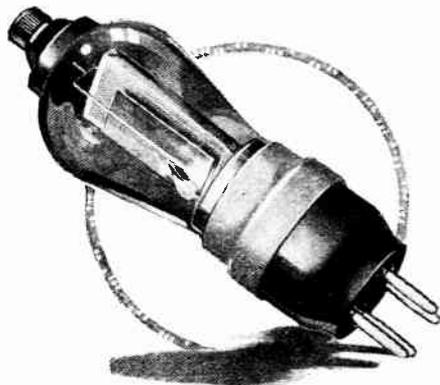
Fig. 43.—Securing a loose valve-base by means of a wide rubber band.
