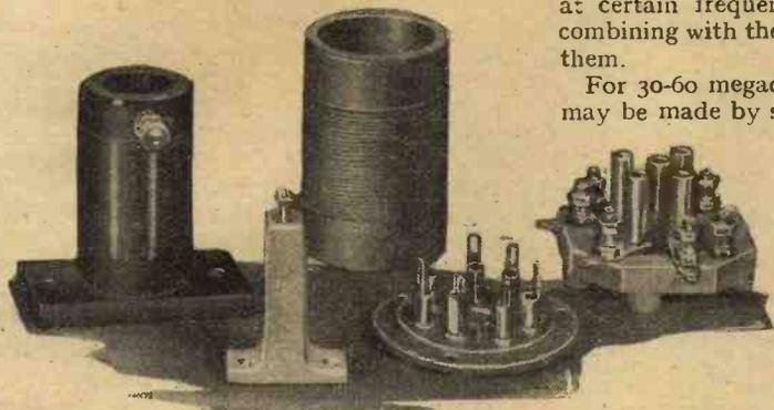
This group includes the Kinva and Gol-tone short-wave HF chokes, Bulgin 5-pin valveholder on steatite base and stand-off insulator, also Eddystone 7-pin chassis valveholder on base of new DL-9 insulating material.
