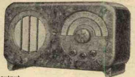
mounted in a circular case of moulded bakelite. This unusual form of construction is highly practical, as a large and therefore easily read tuning scale may be fitted without spoiling the appearance of the receiver. Table space is also saved.
