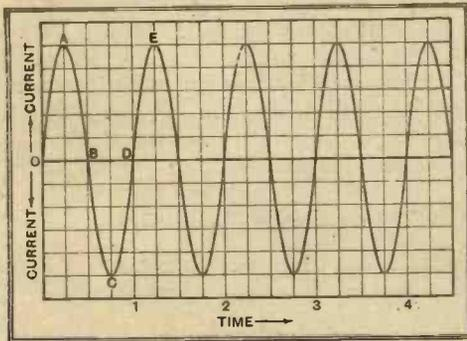
Fig. 18.—A curve showing the variation of the current in an oscillating circuit with time.
