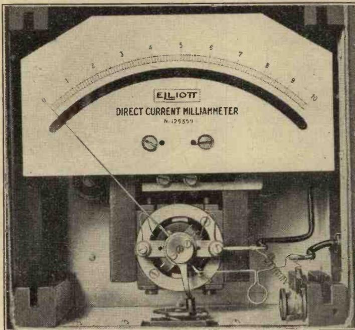
Milliammeter with front removed. The coil lies behind the pivot between the poles of the magnet. When moved by a current it sweeps the pointer over the scale.
