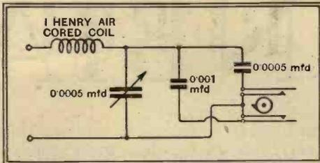
Fig. 3.—Circuit arrangement of a variable heterodyne whistle filter.
