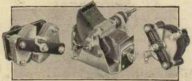
An Ormond air-dielectric midget condenser can be seen on the left, and a solid-dielectric differential reaction condenser of the same make on the right. In the centre is a Formo tuning condenser.
