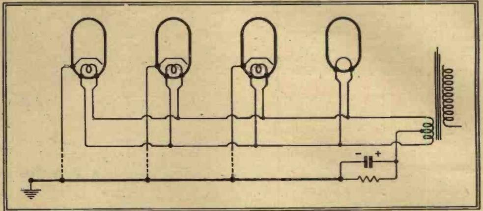
Fig. 4.—Automatic grid bias for a directly heated valve can be provided without needing a separate LT winding.
