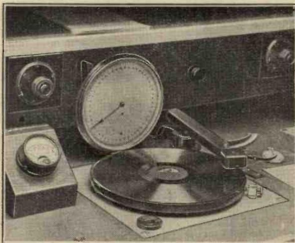
A close-up of one of the turntables of the transfer table. Behind the record is seen the calibrated scale showing the exact groove on which the pick-up needle is travelling. On the left is the pick-up volume control and meter.
