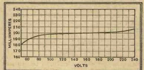
Fig. 5.—An appropriate barretter keeps the heater current for universal or DC valves at the correct value over a wide range of mains voltages.
