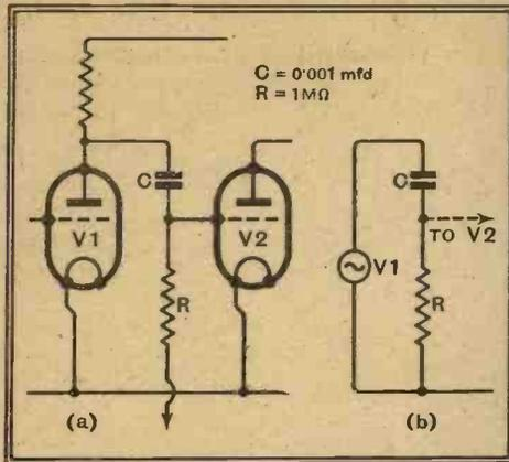
Fig. 31.—A low-frequency coupling between two valves. Diagram *a* shows the practical circuit and *b* the essentials necessary to calculation.
