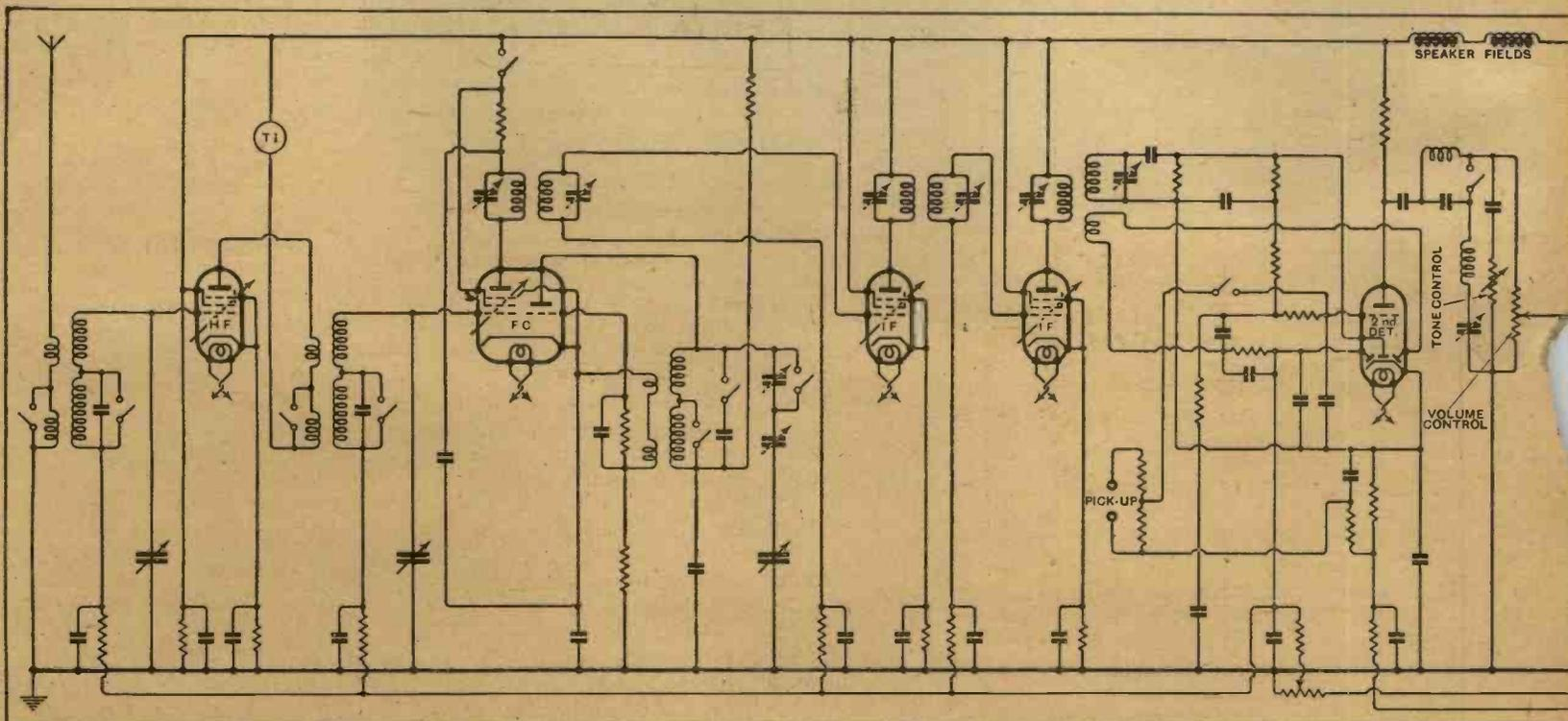
A signal-frequency amplifier and two IF stages provide a high degree of range and selectivity. The coupling of the IF circuits is adjustable, as is the
