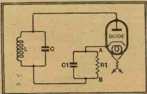
Fig. 1.—The fundamental diode detector circuit.
