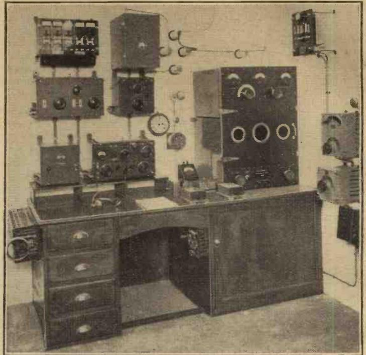
A standard 1.5-kilowatt Marconi installation for passenger ships.
