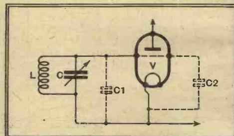
Fig. 3.—The total capacitance in a circuit comprises condenser C and small capacitances C1 and C2 representing wiring and grid/filament of valve.
