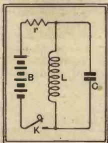
Fig. 14.—With the aid of this simple circuit the nature of high-frequency currents can be elucidated.
