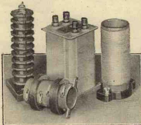
Special heavy-duty HF chokes for including in mains supply to receivers.
