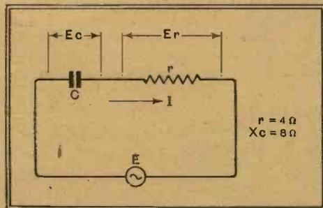
Fig. 29.—Condenser and resistance in series with an AC source. The generator-voltage  $E$  is equal to the total voltage due to the simultaneous presence of  $E_c$  and  $E_r$ . See Fig. 30.
