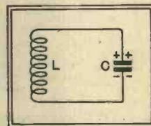
Fig. 16.—The collapse of the magnetic field round L has caused a current which has charged C.
