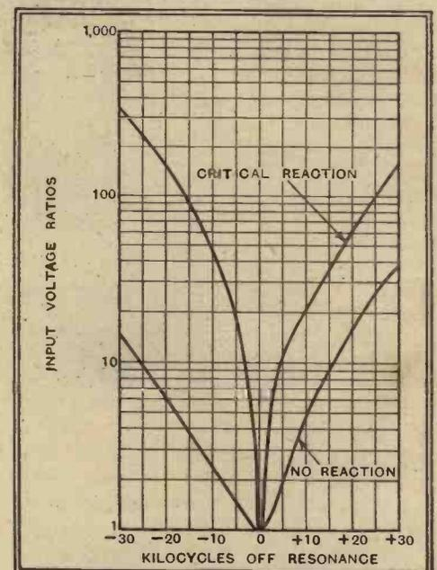
Fig. 4.—The selectivity, both with and without reaction, can be gauged from these curves.
