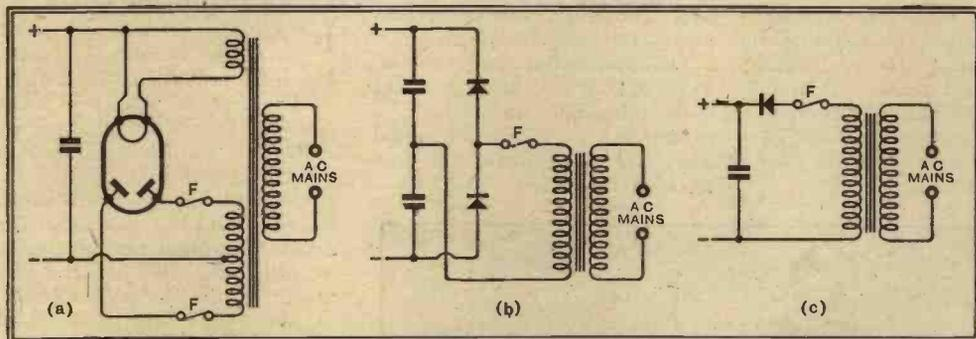
Fig. 1.—F indicates fuse positions for protecting the H.T. circuit with (a) a full-wave valve rectifier, (b) a voltage-doubling metal rectifier, and (c) a half-wave rectifier of either sort.
