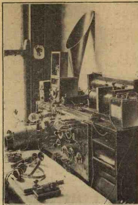
Typical of amateur stations of 1922, which worked on a wavelength of 180 metres.
