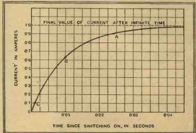
Fig. 25.—Showing slow rise of current in circuit of Fig. 24. Calculated for  $E=100$  v,  $L=1.0$  H,  $r=100$  ohms. By sufficiently rapid rotation of the switch, the current could be kept below A (1/40th sec.), below B (1/100th sec.), or even below C (1/1,000th sec.).
