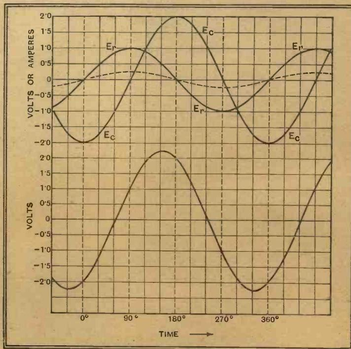
Fig. 30.—In the upper curve,  $E_r$  represents voltage across the resistance, and  $E_c$  voltage across the condenser, of Fig. 29. The lower curve shows the resultant total voltage; that which the generator must have to drive 0.25 amp. through the circuit.
