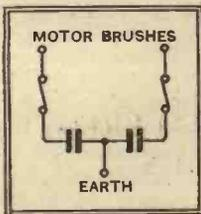
Fig. 1.—Simplest condenser arrangement for an electric motor.
