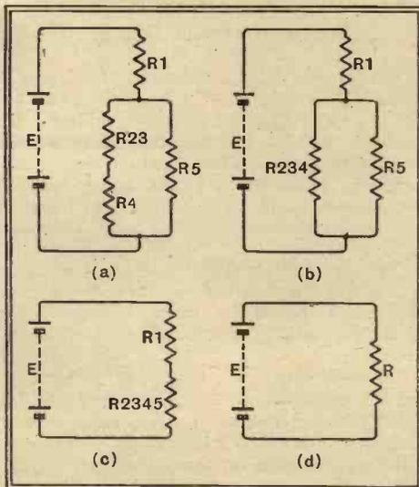
Fig. 11.—Successive stages in simplifying the circuit of Fig. 10. R<sub>23</sub> stands for the single resistances equivalent to R<sub>2</sub> and R<sub>3</sub>; R<sub>234</sub> to that equivalent to R<sub>2</sub>, R<sub>3</sub> and R<sub>4</sub>, and so on. R represents the whole system.
