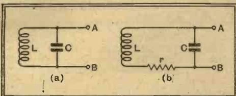
Fig. 1.—In a tuned circuit consisting of inductance  $L$  and capacitance  $C$  (a) the losses can be represented by a series resistance  $r$  (b).
