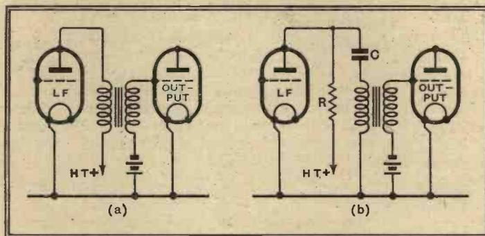
Fig. 1.—The direct coupling connections for an intervalve transformer are shown at (a) and the parallel-feed circuit at (b).
