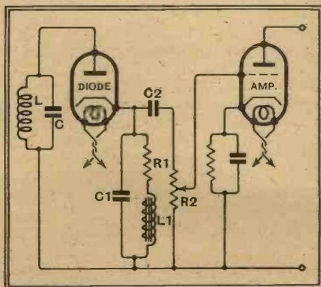
Fig. 5.—A modified coupling for distortionless detection.  $L_1$  has an inductance of 300 H.
