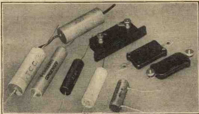
placed the mica, for it enabled condensers to be made in easily handled sizes, though this style would not, in the early days, stand up to high voltage, but they were quite satisfactory for use in receivers of the period, since it was the exception rather than the rule to employ more than 100 volts.
