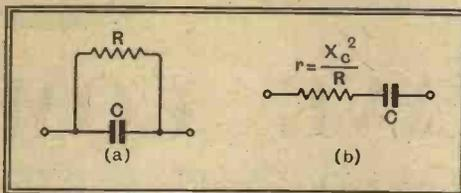
Fig. 2.—Losses in a condenser may be regarded as a shunt resistance R (a) which can be converted into a series resistance r (b) for computing the total loss in the circuit.
