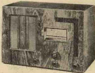
output rated at 2 watts. A special selectivity control is provided for use where receiving conditions are difficult.
