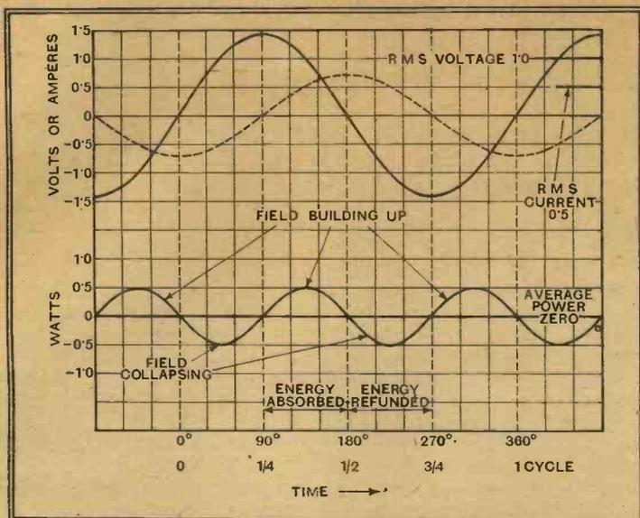
Fig. 28.—Relation of voltage, current and power in a purely inductive circuit. Note that the average power is zero, and compare Figs. 26 and 27.
