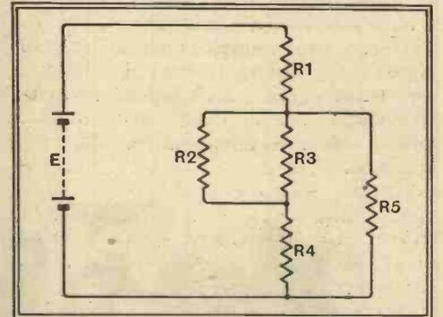
$R_1 = 100$  ohms,  $R_2 = 200$  ohms,  $R_3 = 500$  ohms,  $R_4 = 150$  ohms,  $R_5 = 1000$  ohms,  $E = 40$  volts.
