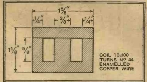
Fig. 7.—A suitable core for the 300 H. choke can be built from 25 pairs of varnished laminic stampings, 0.015 in. thick.
