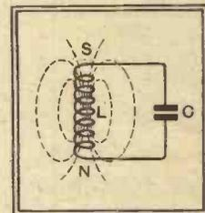
Fig. 17.—The discharge of C has driven a current through L, evoking a magnetic field opposite in polarity to that of Fig. 15.
