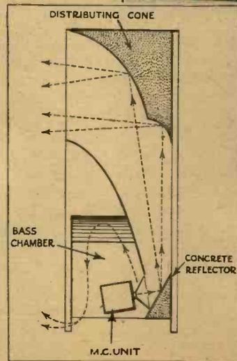
Front panels removed giving access to the bass-chamber and twin-diaphragm unit, and (left) diagrammatic section of cabinet, showing alternative sound paths.
