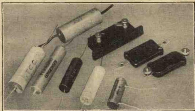
Modern small-capacity condensers are usually fitted with wire ends for suspending in the wiring.
