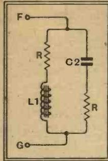
Fig. 6.—This circuit forms the diode load and if certain values are selected for components it acts as a pure resistance for all frequencies.
