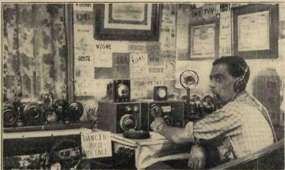
Mr. J. N. Roe (G 2VV) in his wireless room at St. Margaret's-on-Thames, Middlesex. The AC mains-operated transmitter is a single valve TP-TG using an LS6A or T25D type. The station maintains daily contact with the U.S.A on 20 metres, using 8 or 10 watts.
