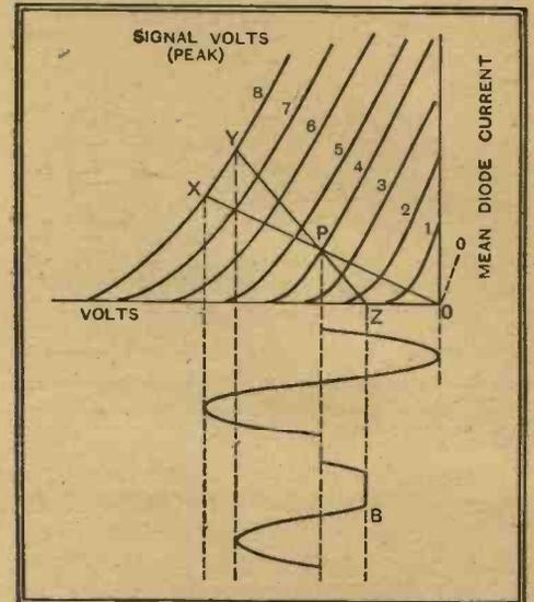
Fig. 3.—Typical diode curves are shown here with a DC load line XO and an AC load line YZ of different values. The resulting distortion is shown at B.
