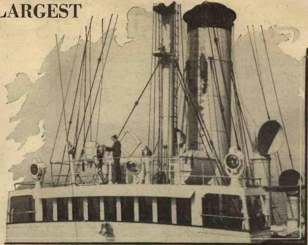
The speaker, seen on the upper deck, can be rotated in any direction required.
