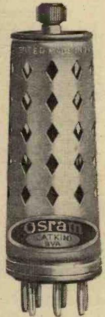
The VMP4K, an HF screen pentode with interelectrode capacity as low as the best screen-grid tetrode.
