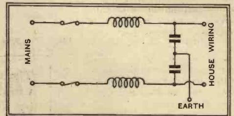
Fig. 2.—Arrangement of a choke-condenser filter for suppressing mains-borne interference.
