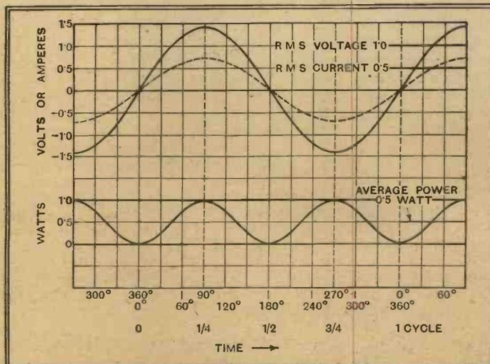
Fig. 26.—Relation of voltage, current, and power in a purely resistive circuit. Note that the complete cycle is indicated in degrees for easy reference.
