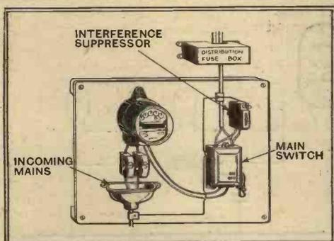
Fitting a Belling-Lee interference suppressor to incoming mains.
