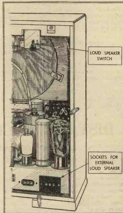
The addition of a switch to isolate the speaker on the set when the extension speaker only is required is provided on some of the Philips models.
