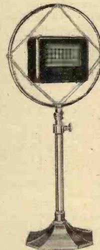
As with all microphones of this pattern the resistance is comparatively high—about 500 ohms in the present case—and conse-
