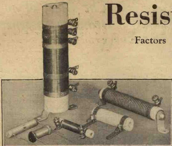
Types of wire-wound fixed resistances showing Bulgin mains, 40- and 10-watt; Dubilier 10-watt Spirohm; Watmel 3-watt and Amplion one-watt models.
