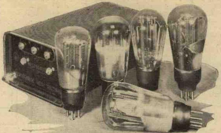
A Westinghouse metal rectifier is shown with a group of modern full-wave rectifier valves.
