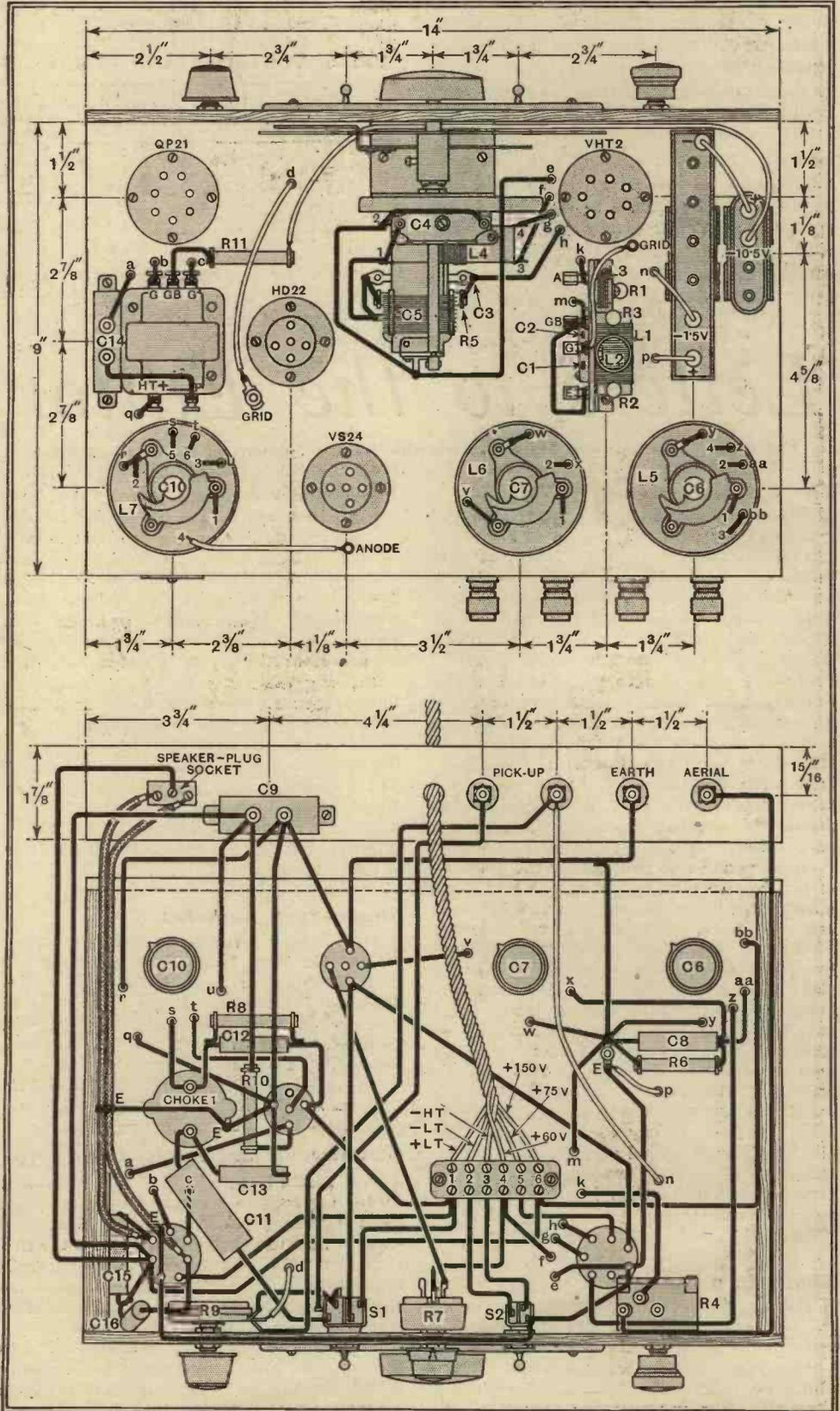
Full details of both the wiring and construction of the new receiver can be gleaned from the drawings.
