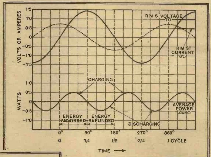
Fig. 27.—Relation of voltage, current and power in a purely capacitive circuit. Note that the average power is zero, and compare Figs. 26 and 28.
