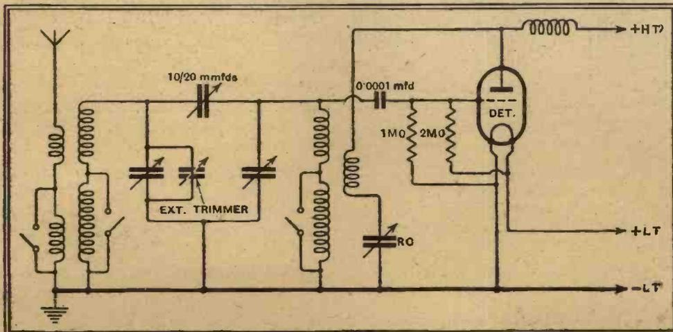
Fig. 1.—Suggested alterations to a reader's band-pass circuit; external coupling and trimming controls ensure best operating conditions.
