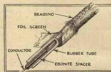
A method of providing air spacing (with consequent reduction in losses and self-capacity) for the conductor of screened aerial cable (Ward and Goldstone's “Metocel”).
