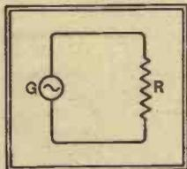
Fig. 19.—A high-frequency or alternating voltage is applied by the generator G (nature unspecified) to the resistance R.
