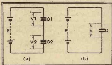
Fig. 13.—Condensers in Series. The voltage  $E$  is divided between the condensers; hence each takes less charging-current than if it were directly connected across  $E$ . For the same charging-current in the two circuits,  $1/C = 1/C_1 + 1/C_2$ .
