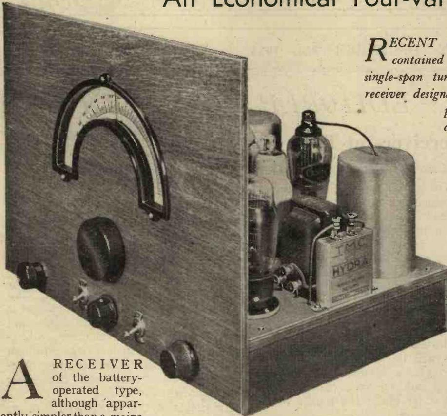
*RECENT* articles in "The Wireless World" have contained details of the latest developments in single-span tuning, which have been embodied in a receiver designed for economical battery operation. The points of special importance are the new aerial filter and a novel reaction system.
