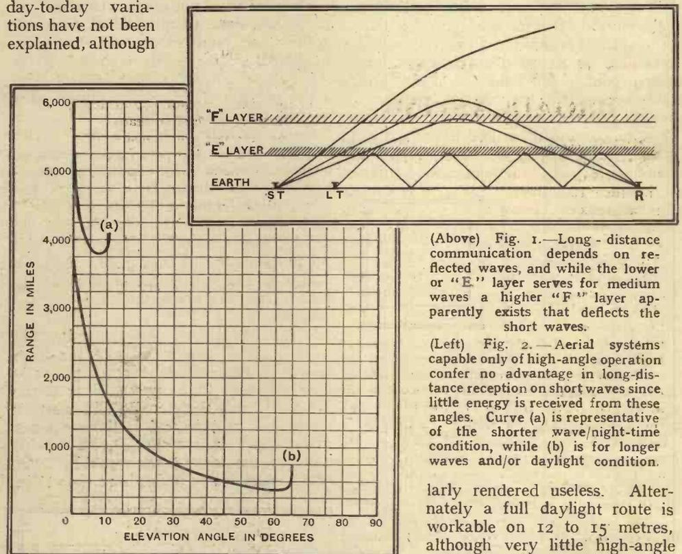
(Above) Fig. 1.—Long-distance communication depends on reflected waves, and while the lower or "E" layer serves for medium waves a higher "F" layer apparently exists that deflects the short waves.
