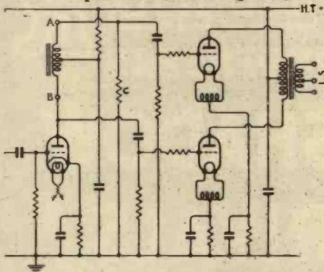
necessary current through the choke so that no D.C. potential exists across the points (A) and (B). Here we have an intervalve coupling matched to its valve and practically devoid of the evils of leakage inductance and self-capacity. As there is negligible D.C. magnetising current, advantage may be taken of the merits of a compact nickel-iron core in the con-
