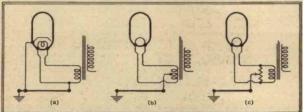
Fig. 3.—The LT winding for an indirectly heated valve is often connected to the rest of the circuit at one side (a), but with directly heated valves the connection must be made to a centre-tap (b), or potential divider (c).
