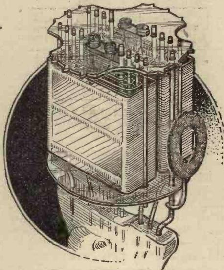
The QP21, a double pentode, which with proper precautions, can be used for the final stage as a class "B" output.
