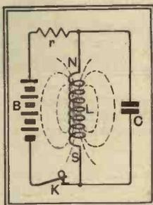
Fig. 15.—The circuit of Fig. 1 with the key K closed. Note the magnetic field round L.
