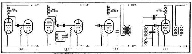
Fig. 1.-Positions in which HF chokes are commonly employed.
