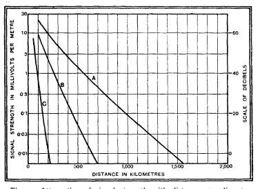
Fig. 1.—Attenuation of signal strength with distance according to Eckersley :— (A) Warsaw, 1,400 m, 120 kW. (B) typical regional station, 300 m, 50 kW. (C) short-wave station, 10 m, 25 kW.
