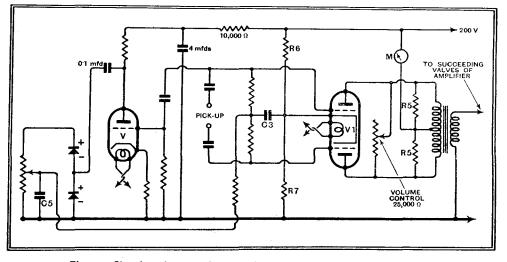
Fig. 4.-Showing the use of a transformer in place of a tapped choke.
