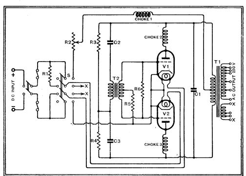
Fig. 3.—Complete circuit diagram of the inverter. RI, R2, see text; R3, R4, 5,000 ohms, 20 watts; R5, 5,000 ohms, 5 watts; R6, I0,000 ohms, 5 watts; CI, 4 mfd.; C2, C3, I mfd. (all 1,500 volts working); VI, V2, thyratron tubes.
