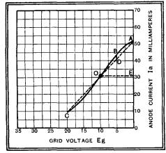
Fig. 124. Dynamic curve of pentode with 10,000-ohm load. Ideal characteristic giving zero 2nd and 3rd harmonics is shown dotted. Percentage 3rd harmonic  $= \frac{BD}{AE} \times 100$ .
