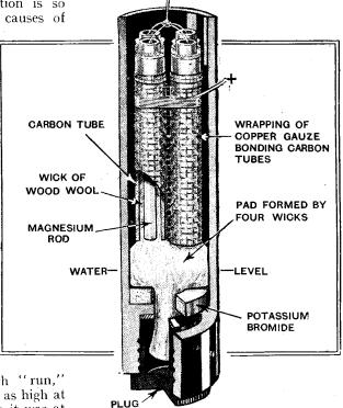
Fig. 2.—Drawing illustrating the construction of the Gordon cell and showing the four parallel units.
