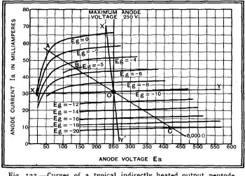
Fig. 122.—Curves of a typical indirectly heated output pentode. The load-line ABOC represents a usual load. Es = 200. Curves taken at
