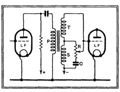
Fig. 3.—Connections of a tone-control transformer.
