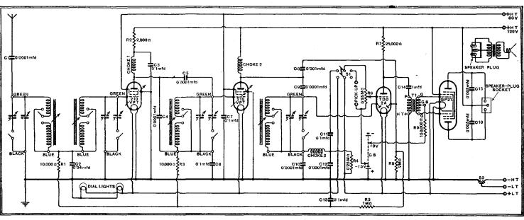
Fig. 1.—The complete circuit diagram shows that four tuned circuits are employed—two of them preceding the first valve. A duo-diode-triode provides detection, AVC, and LF amplification, while the output stage is of the QPP type.
