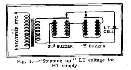
As will be seen, this device makes use of a pair of buzzers, and the advantage of the particular scheme of connections advocated is that the resistance of the buzzer coils is not in series with the transformer.
