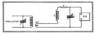
Fig. 105. —Method of measuring the resonance curve of a tuned circuit. The voltage across C is observed on the valve voltmeter VV for a number of different frequencies.
