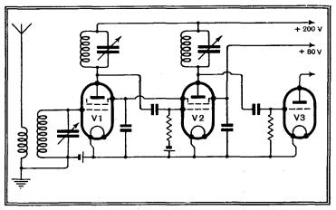
Fig. III.—Two-stage high-frequency amplifier, using tuned-anode circuit with screen grid valves.
