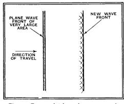
Fig. 2.—Every point in a plane wave sends out a wavelet : these wavelets combine to produce a new plane wave.
