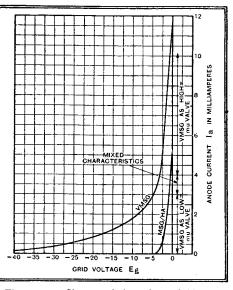
Fig. 114.—Characteristic of variable-mu valve (VMSG) compared with that of standard screen-grid valve. Note the increased signalhandling ability of the VMSG and the slow but steady change of slope with bias.
