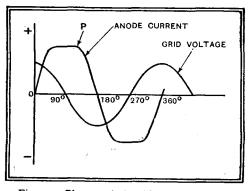
Fig. 2.—Phase relationship between grid voltage and anode current in a self-exciting inverter.
