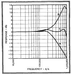
Fig. 10.-Curve A is again the same as in the preceding illustration, but curve B is now for values of  $L = 1,000 \ \mu$ H. and R = 2,670ohms, and curve C represents the overall characteristics.
