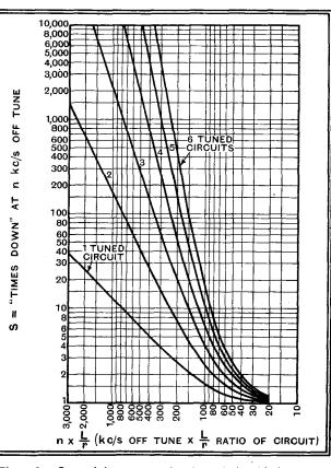
Fig. 108.—General data curves showing relationship between  $n \times L/r$  and s for 1 to 6 tuned circuits in cascade.
