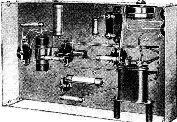
An under base view of the experimental amplifier. Note the in-sulating mounting of the metal-cased fixed condenser to avoid the effect described in the text.
