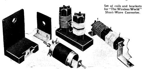
original coils, the winding occupies the same length on the former, so that the inductances are correct.
