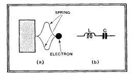
Fig. 5.--(a) An electron held by a spring force to an atom is equivalent to (b) a coil in series with a capacity.
