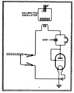
Fig. I.—The connections employed when a heterodyne wavemeter is available for calibration. The output of the test oscillator is shown by the crocodile clips.
