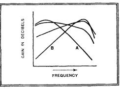
Fig. 4.—Various types of response curve obtainable from a tone-correcting transformer.
