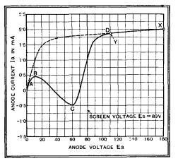
Fig. 116.—" Theoretical " (dotted) and actual (full line) curves of tetrode valve. The extraordinary shape of the latter between A and D is due to secondary emission from the anode. The introduction of a " suppressor " grid, turning the valve into a pentode, enables the dotted curve to be realised in an actual valve.
