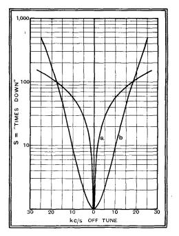
Fig. 109.—Resonance curves of one (a) and six (b) tuned circuits, chosen so as to give in each case 100 times reduction at 18 kc/s off tune. Note the enormous loss of side-bands in case a.
