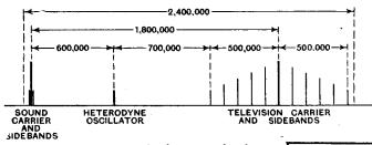
Diagram showing how the frequency bands are to be utilised.
