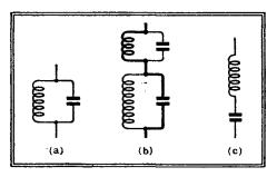
Fig. 3.—Illustrating the distribution of self-capacity.
