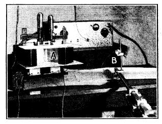
General view of associated apparatus showing (A) ribbon loud speaker unit and (B) exploring microphone mounted on radius arm.
