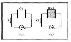
Fig. 4. --An ebonite condenser has a bigger capacity than an air condenser of equal size.
