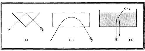
Fig. 7.--(a) Total reflection of light by a prism. (b) Continuous bending of wireless wave when ionisation increases in an upward direction. (c) Total reflection of wave when K=0.
