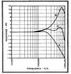
Fig. 9.—Curve A is the same as in Fig. 8, but, in curve B,  $L = 1,286 \ \mu$ H. and R = 3,000 ohms. This gives the overall response of curve C.
