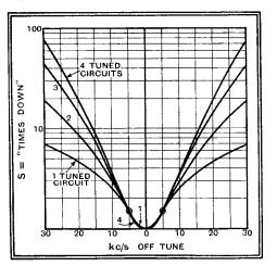
Fig. 110.—Overall resonance curves of one, two, three and four tuned circuits, in each case chosen to give "equal quality," represented by the same response to a 5-kc/s sideband.
