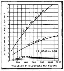
Fig. 2. -Curves showing the relation between attenuation and frequency range.
