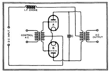
Fig. 1.—Illustrating the principles of operation of the thyratron inverter.
