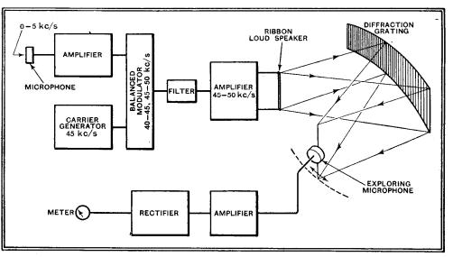
Fig. 1. Schematic arrangement of apparatus for producing and exploring acoustic spectra.
