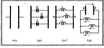
Fig. 6.—(a) Air condenser. (b) Equivalent of a mica condenser. (c) Equivalent of filling the space with free electrons.
