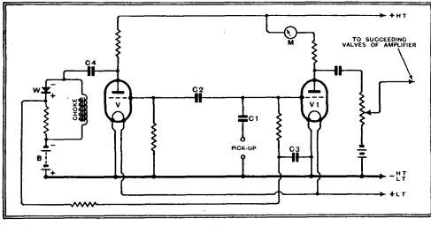
Fig. 1.-Skeleton circuit diagram illustrating the principles of volume expansion.
