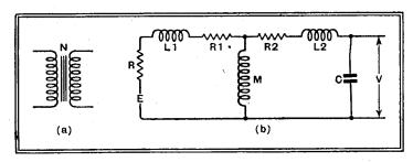
Fig. 1.-A normal LF transformer and its equivalent circuit.
