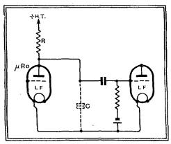
Fig. 119.—Showing stray capacities C in a resistance-coupled LF stage. High notes of frequency f receive 70.7% of the amplification of low notes when  $1/2 \pi$  fC = RRo/R + Ro.
