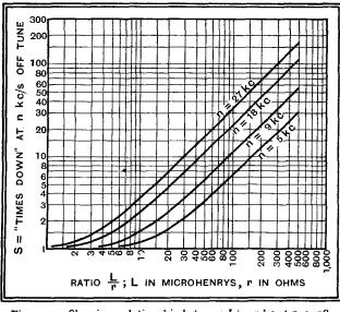
Fig. 107.—Showing relationship between L/r and s at 5, 9, 18, and 27 kc/s off tune.
