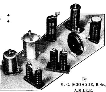
true of any sort of coil, such as a tuning coil. The position is further complicated by the fact that the self-capacity is not the same at all frequencies.
