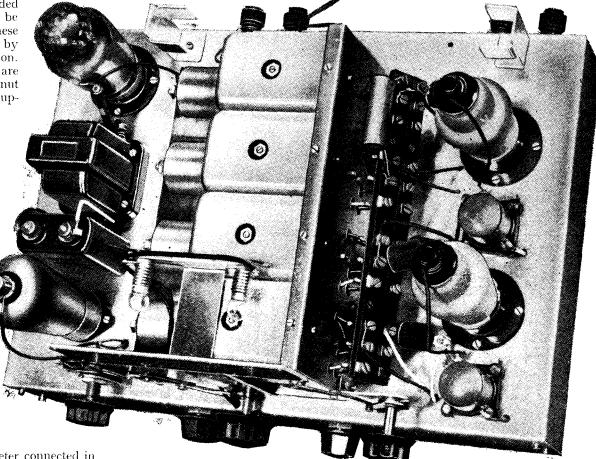
A bird's-eye view of the chassis in which the chief parts clearly stand out. The space to the left of the tuner is devoted to the LF equipment.
