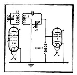
Fig. 2.—A practical circuit diagram showing the connections of a quartz crystal is given here. The crystal holder capacity is balanced by Cn, and, as explained in the text, the windings of the input transformer, LI L2, should be screened from one another.
