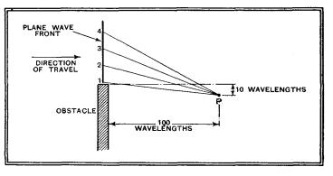
Fig. 3.—The wavelets from the plane wave tend to cancel out at  $\ensuremath{P}$  owing to phase differences.
