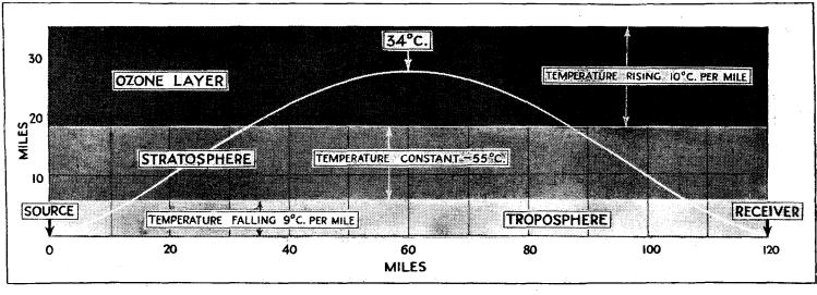
Fig. 2.—Abnormal travel of the sound of gun fire, due to refraction in the ozone layer.
