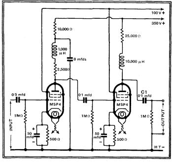
Fig. 11.-The circuit diagram of an experimental amplifier. With the values of components shown, the frequency characteristic is that of Fig. 13.
