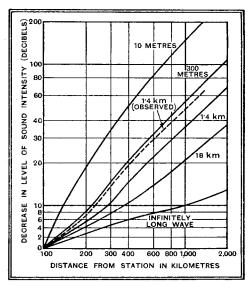
Fig. 5.—With a copper plated earth and no reflection from the sky, loud speaker intensity would decrease with increasing distance as shown.
