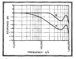
Fig. 12.—These curves represent the initial response with the amplifier of Fig. 11, and the high-frequency attenuation is due to excessive stray capacity in the output circuit. The substitution of a bakelite for a metalcased condenser, CI, altered the response from curve A to curve B.
