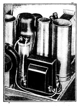
The tone-control transformer in practical use. A Multitone component incorporated in The Wireless World Universal AC-DC III.
