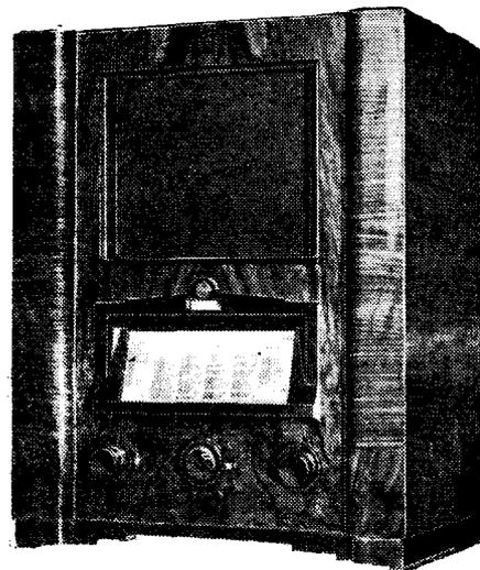
The Philips receiver has a signal-frequency HF stage and covers 16/50 metres as well as the medium and long wavebands.
