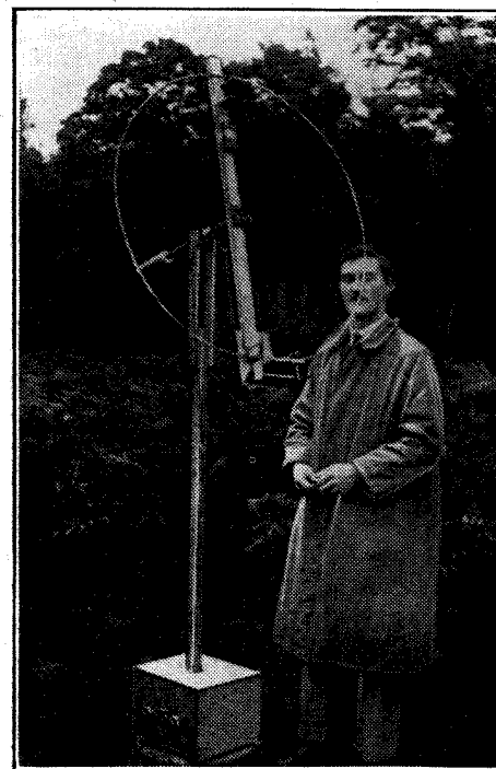
Fig. 3.—A loop of large diameter was used with this receiver, provision being made to orientate it in the vertical and horizontal planes for directional observation.
